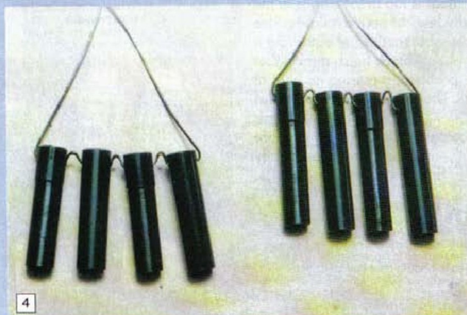
4: The test samples after blackening.
