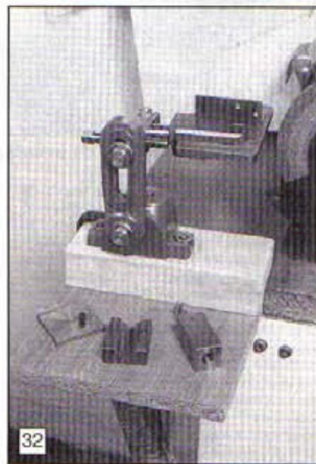
32: Mounting the grinding rest. The extension is firmly screwed to the front edge of the bench on which the grinder is mounted. Note the essential support below the extension to give the rigidity required.
