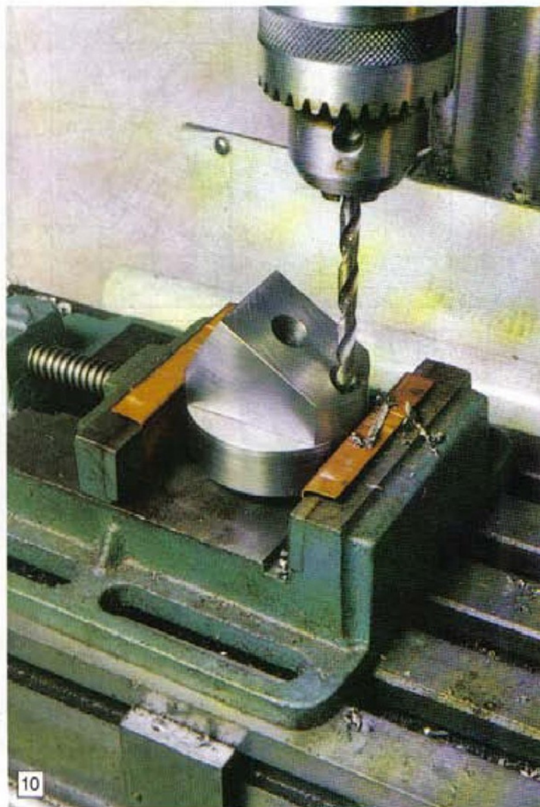
10: Drilling the turret for the plunger.
