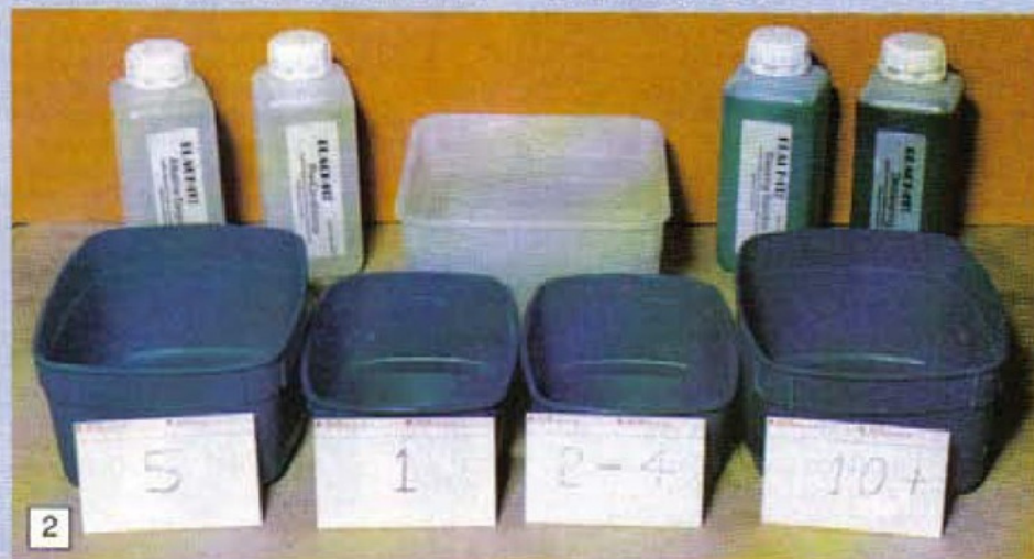
2: Set up, but waiting for the liquids to be placed in the containers. The numbers in front are the times in minutes in each liquid.
