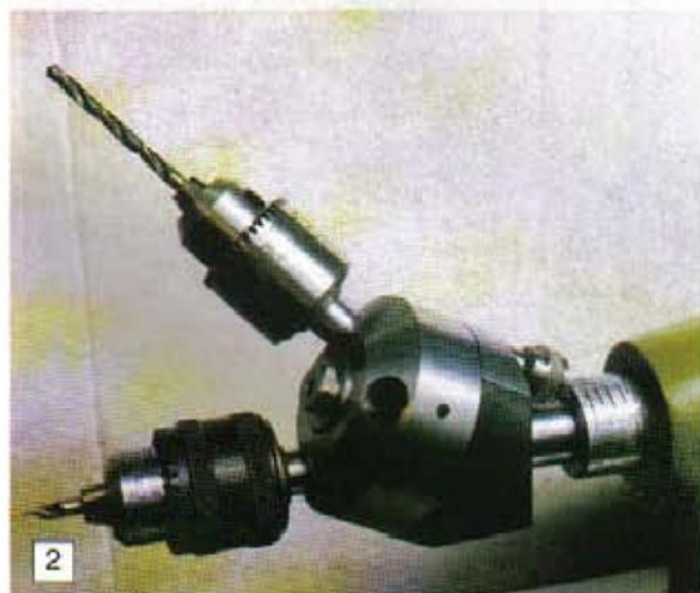
2: Fitted with centre and twist drills. The centre drill is ready for use.
