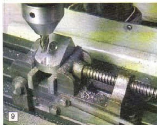
9: Making the recess for the plunger spring box.
