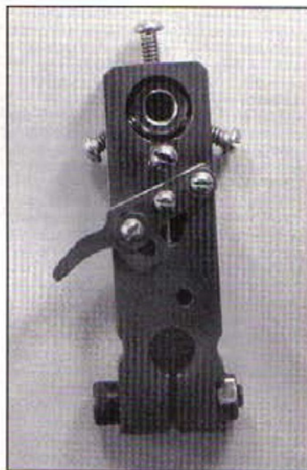
The drive link holding a solid M8 nut.
