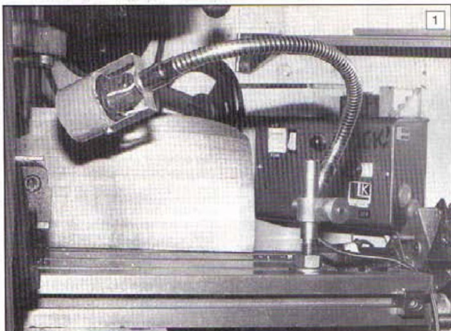
1: The lamp mounted on the milling machine.
