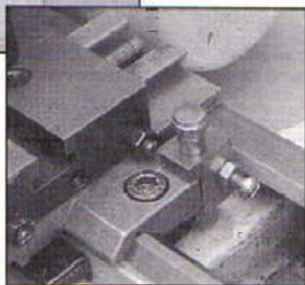
Two views showing how the saddle block and drive rod tail fit around the saddle casting.
