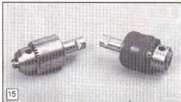
15: Two drill chucks, originally from hand drills and now fitted with adaptors for use in the turret.
