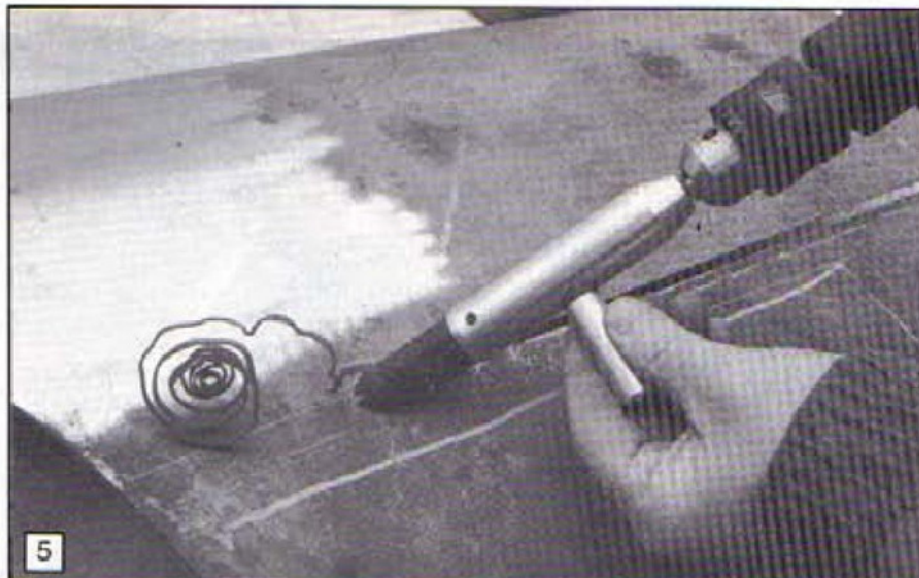
A cut in progress. Stopping the strip forming a spiral is essential when a longer cut is being undertaken, see text.
