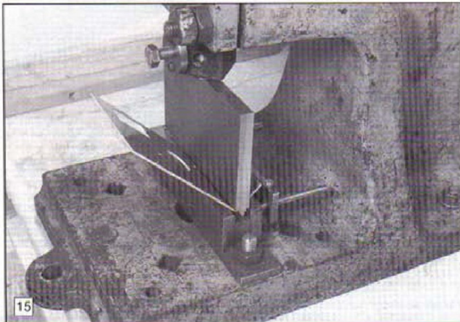
The vee (see text) bender in use.
