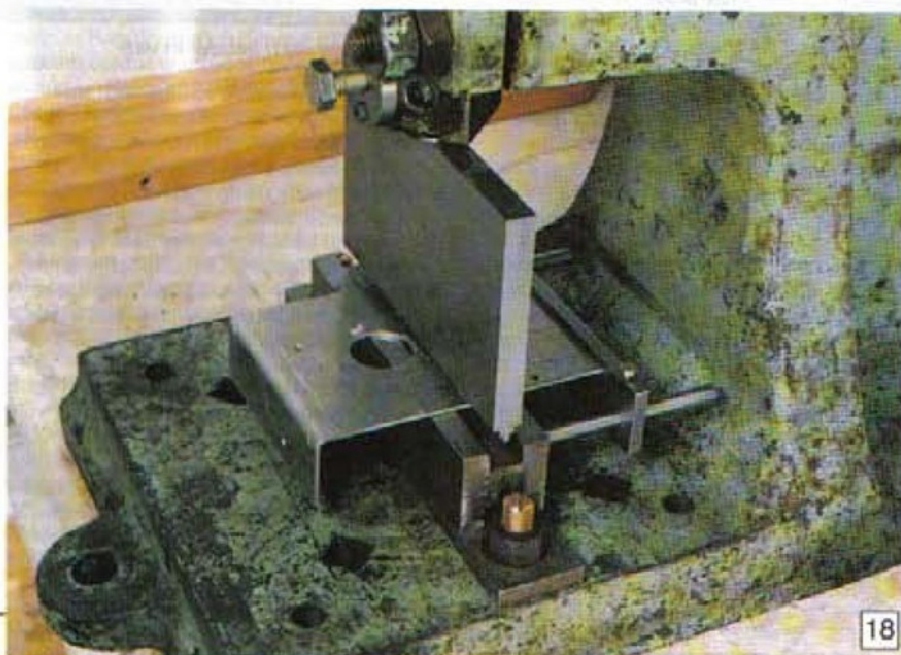
Above: Fitted with a back stop for accurate repetition work.
