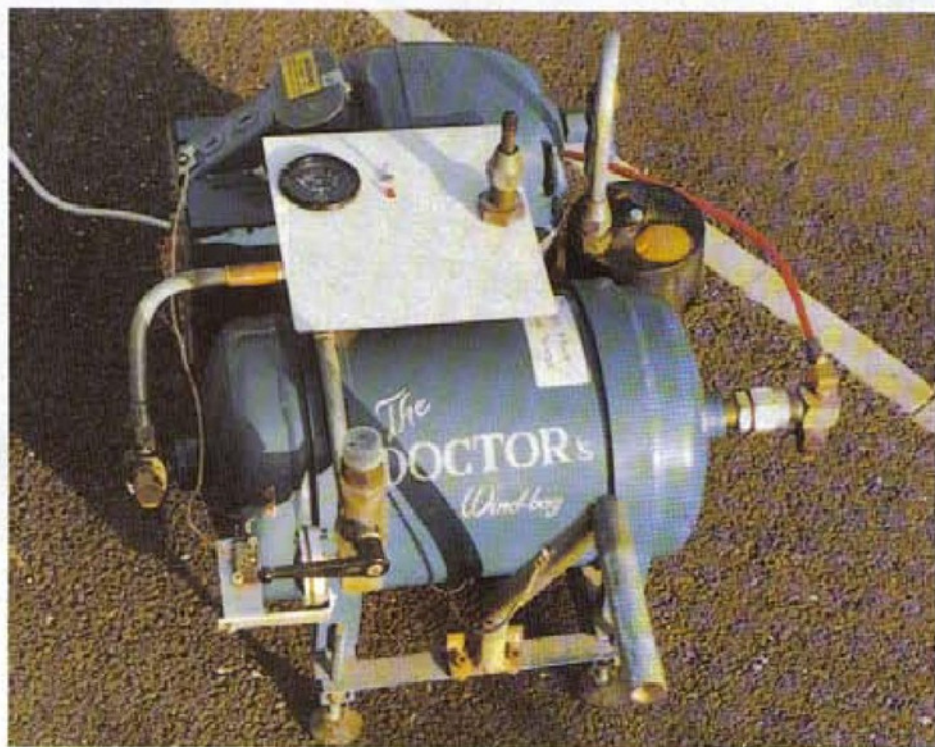
This unit has the air feed pipe to the tank forced inside the outlet pipe from the compressor and secured with adhesive.
