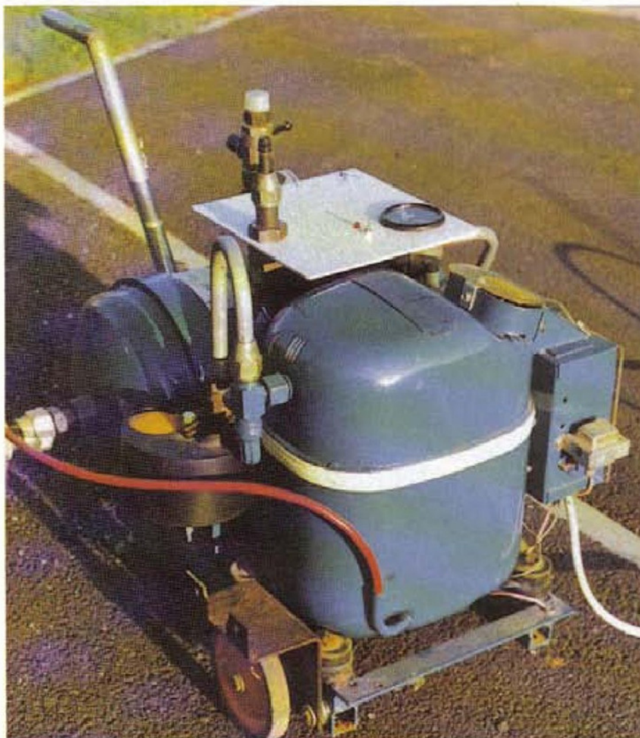
A general view of the compressor, the 12 volt transformer is mounted outside the main electric box to assist in preventing it from overheating.
