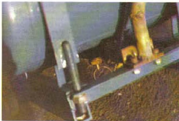
The underside of the reservoir showing the drain valve and mounting straps. The reservoir should always be drained after use by releasing the stored air through this valve.
