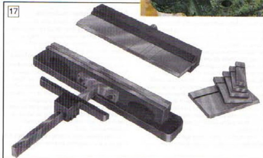
Above: Fitted with a back stop for accurate repetition work.
