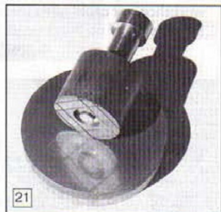
Jig for second attempt at lapping anvil flat.
