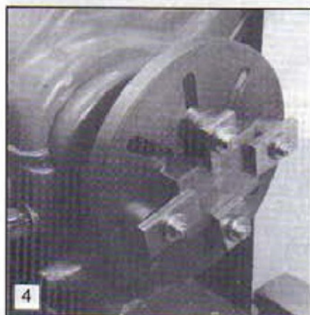
Showing the compact nature of the clamps when used on a faceplate.
