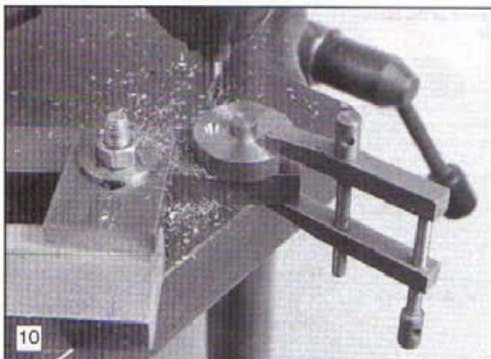
10 Marking the position of the second hole. Note the simple jig being used to make this an easy operation for a number of very similar parts.
