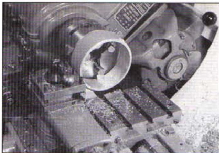
Facing off the sliding ring to length. This was sawn off in the previous operation for safety reasons.
