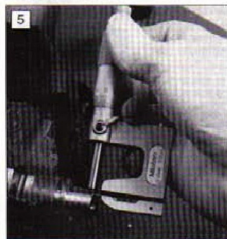
5: Measuring wall thickness using the 3mm circular anvil. By measuring outside diameter and wall thickness the inside diameter can be calculated. This is easier and probably more accurate than using the inside facilities of a vernier calliper.
