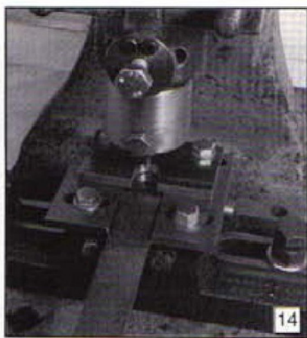
Set up for punching a 4mm hole in 3mm thick B.M.S. strip.
