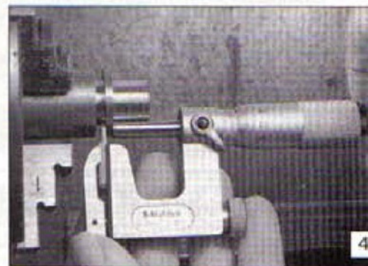
4: Fitted with the flat anvil, enabling measurements to be made from within a narrow slot.
