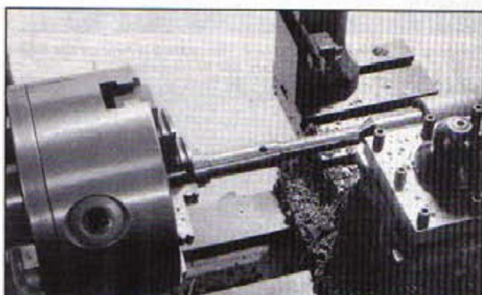
Precision turning an internal spindle extension. Read notes carefully as finished spindle run out is very important. Avoid heavy cuts.
