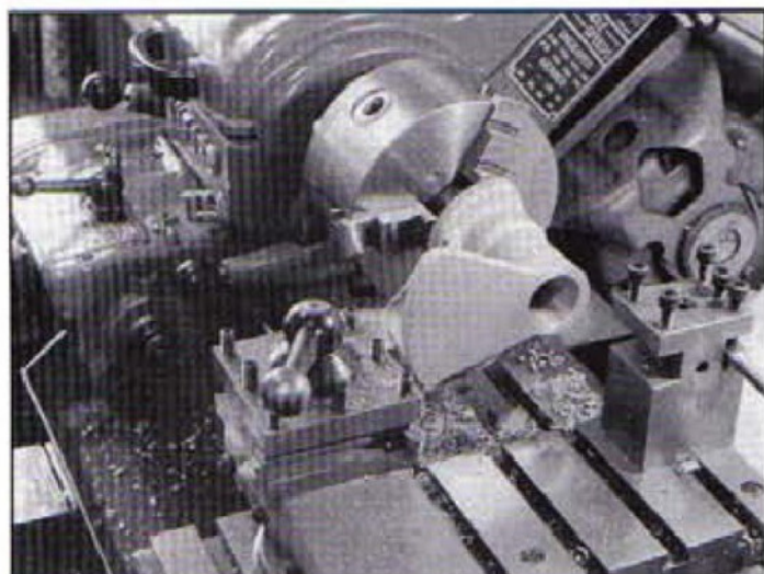
Machining the spindle housing motor guard mounting face with the casting mounted on the 26 T.P.I. spigot.
