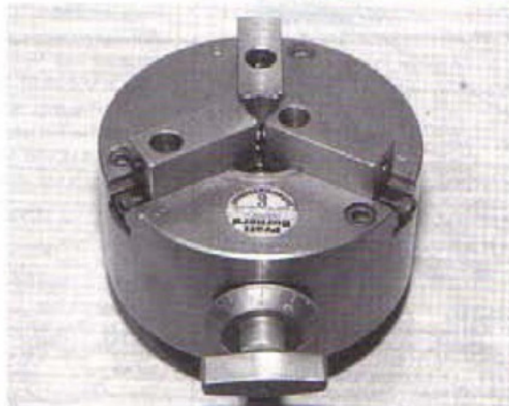
1: The finished boring adaptor, note the calibrated adjustment.
