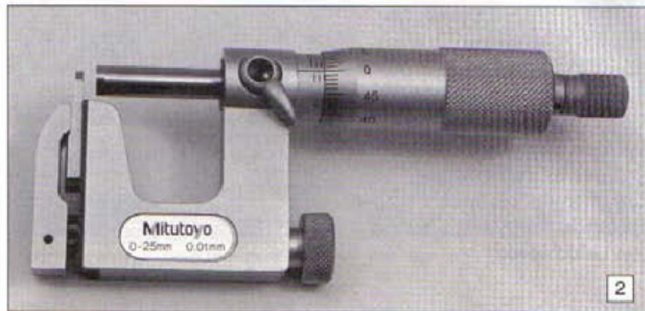
2: The Mitutoyo Uni Micrometer, series 117.
