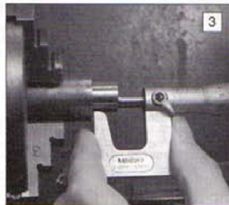
3: With the fixed anvils removed, using the micrometer for height measurement.
