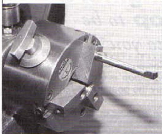
3: Mounted on the lathe with the cutter placed in jaw number one for machining smaller diameters. The key is, of course, removed whilst in operation.
