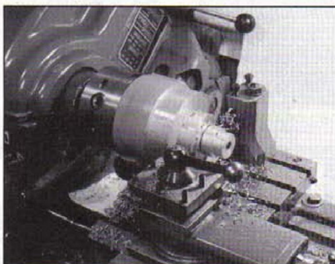
Machining the low/intermediate pulley from the casting stub and rough machining the inner component of the cup wheel guard.
