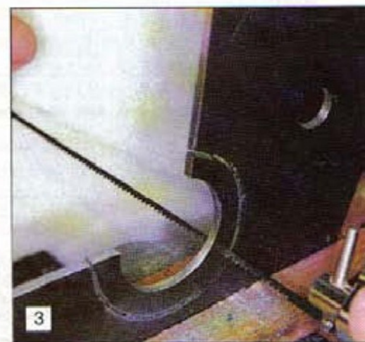
3: The frame centre being cut out with a coping saw.
