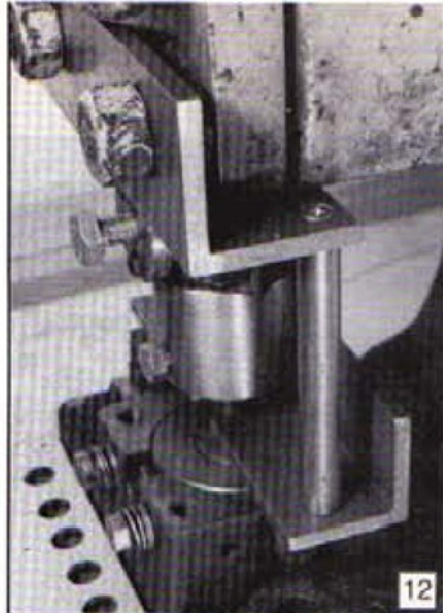
A stripper assembly that places no additional restrictions on the size of the material than can be worked.
