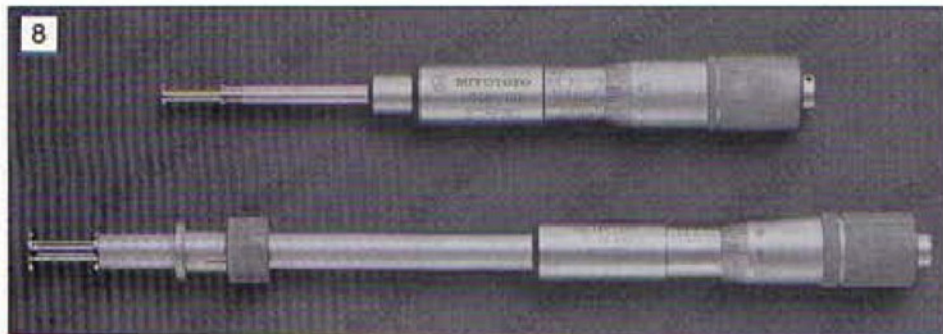
8: A groove micrometer designed for measuring grooves, recesses and shoulders located inside a bore. This is the Mitutoyo series 146 and is available in four sizes up to 100mm.
