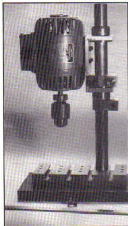
The Drilling Machine being assembled. The Base Board, Base plate and Column are together, the housing with its bushes and motor in place have been slid down the column to rest on a stop collar. The adjustable stop is also in position inside the housing on the column.
