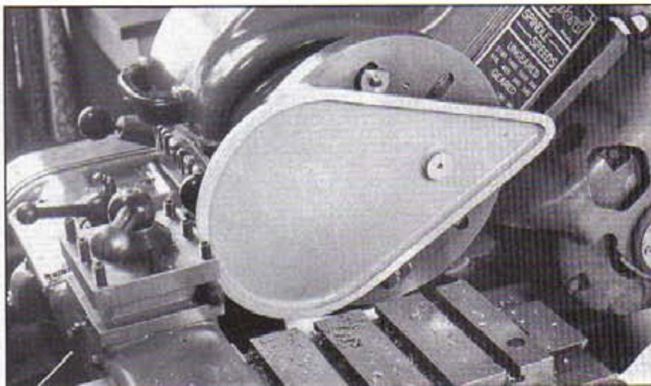
Machining the first prototype outer pulley guard. Latest castings feature support bosses to aid mounting; they are also curved to increase cover stiffness.
