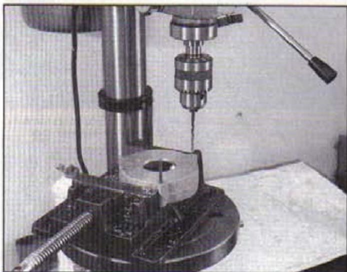
Drilling the outer guard fixing holes using the inner guard as a jig.
