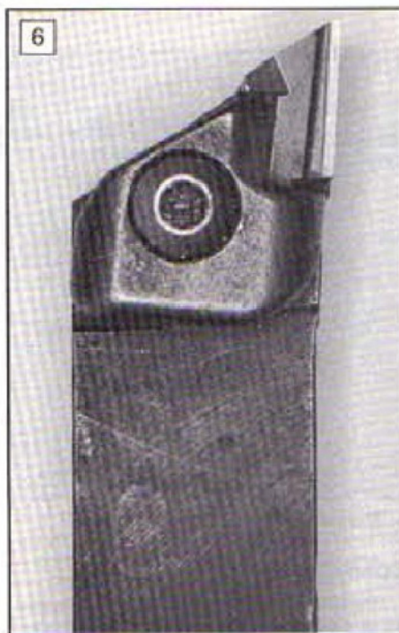
6: The cutting end of a large throwaway tool holder, showing the chip breaker.
