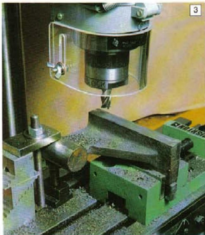
3: Machining the first edge, note the large tee nut and screw being used as a jack, for support, below the boss.
