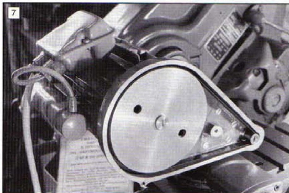
7: The high speed 28000RPM pulley set-up. This must only be used when operating with wheels of less than 1/4in. diameter.
