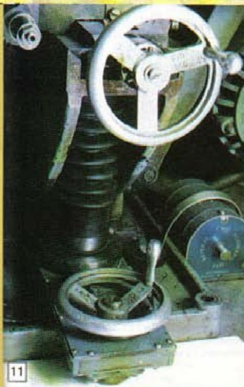
11: The modified Centec milling machine vertical traverse mechanism.
