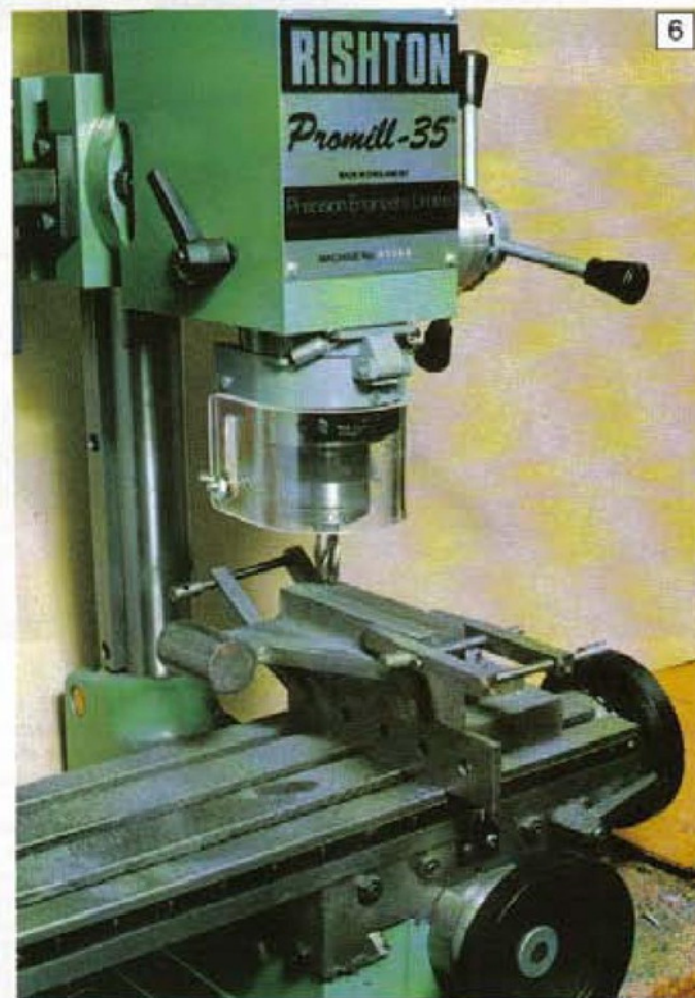
6: With the bottom now machined, the edges were again lightly machined for improved accuracy.
