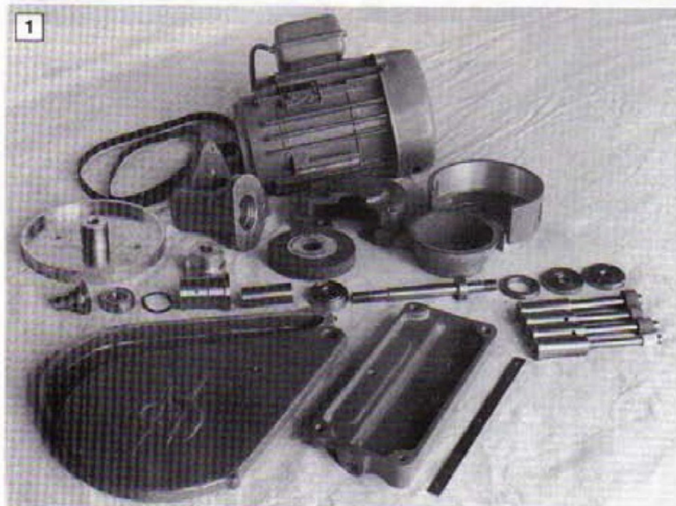
1: The parts of the Dynamic grinder seen here ready for assembly.
