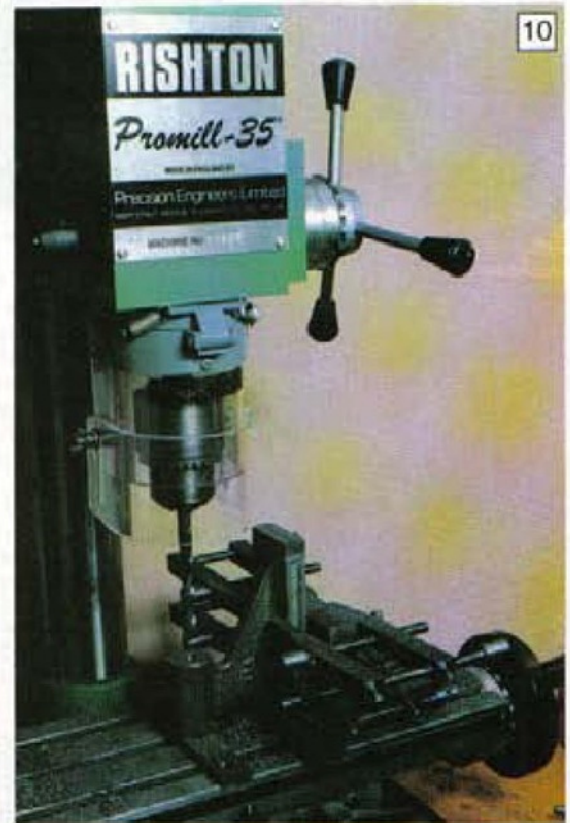
10: Drilling the hole in the boss, note the additional support under the boss whilst drilling.
