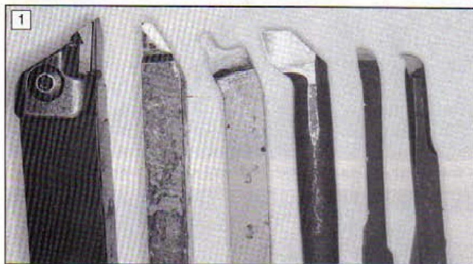
1: A mixed bag of types of turning tools. Left to right, a throwaway tipped tool, a brazed on tipped tool, a butt welded form tool, a butt-welded boring tool and two specials forged from K.E. 10. grade HSS.
