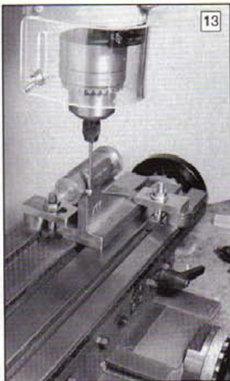
13: Using an edge finder to precisely position the spindle relative to the outer clamp ring.
