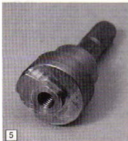
5: Close up of the new tee nut used for clamping the movable jaw at the curved slot.
