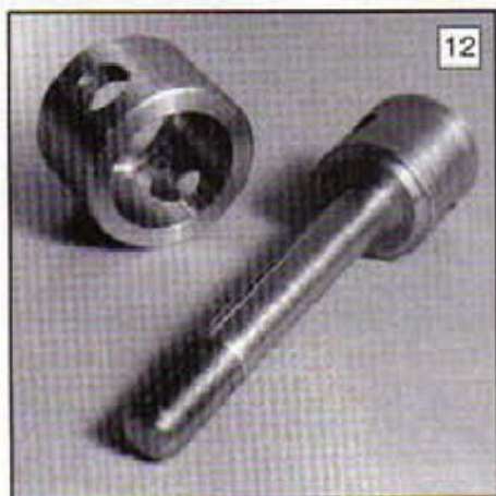
12: The completed clamp arrangement, note the small flange inside the outer ring to make it captive.
