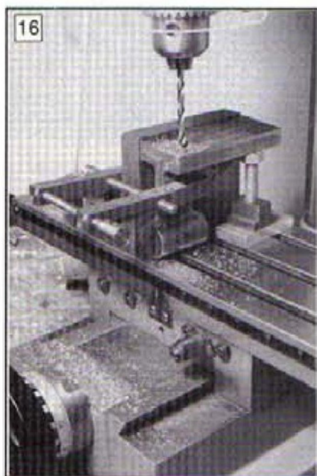
16: Drilling the fixing holes.
