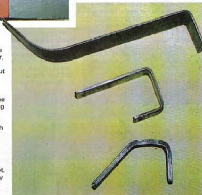
Some items that have been formed on the bender - top is 40 x 2mm, middle 12 x 3mm bar, bottom is 20 x 6mm bar.
