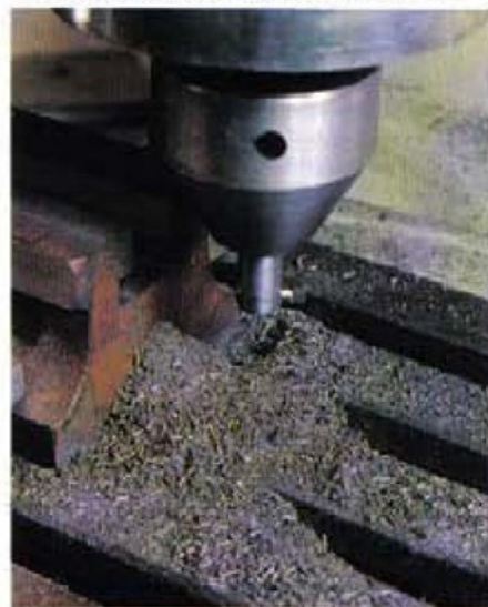
The Tee slot nearing completion.
