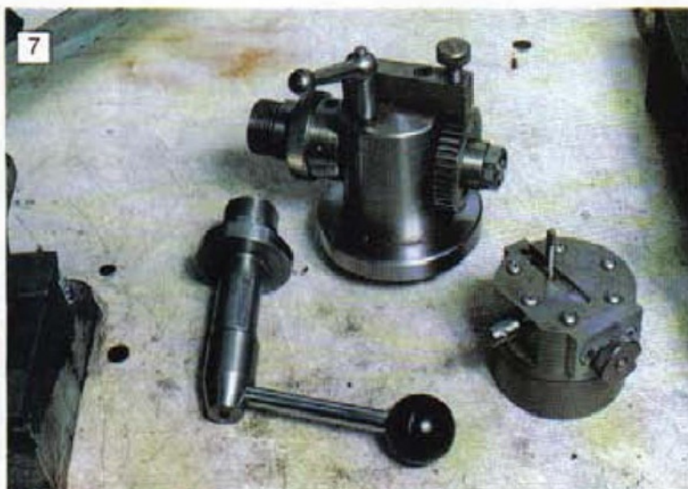
3: Close-up of the division line cutting tool. The turret automatically indexes and sets the length of the line made. Adjustment is by means of packing washers placed under the screw heads.
