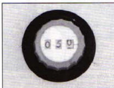
This inverter potentiometer has a digital frequency calibration which is directly proportional to the speed of the motor.
