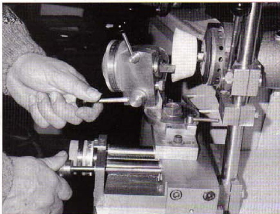
Close up of grinder sharpening a lathe tool.
