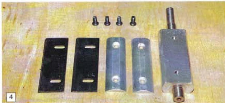
4 Cutter spindle parts. The flats seen on the clamping bars are not acceptable, the photo being taken before a second set were made using the correct material.
