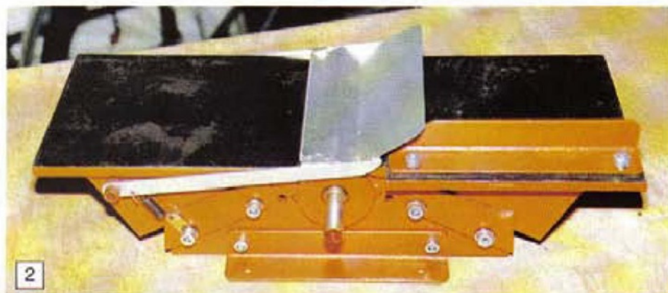
2 Drive side view but without pulley and guard fitted. Note cutter guard arrangement.
