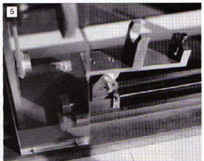
5: The guide rails showing slide assembly and the leadscrew.
