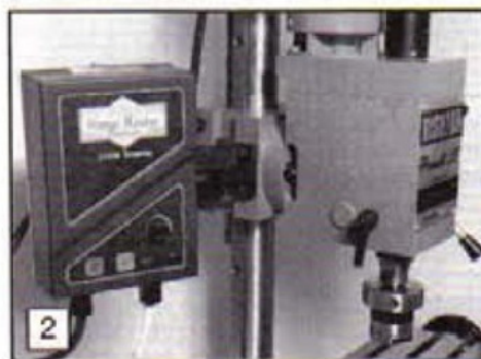
The single to three phase inverter fitted to the machine.
