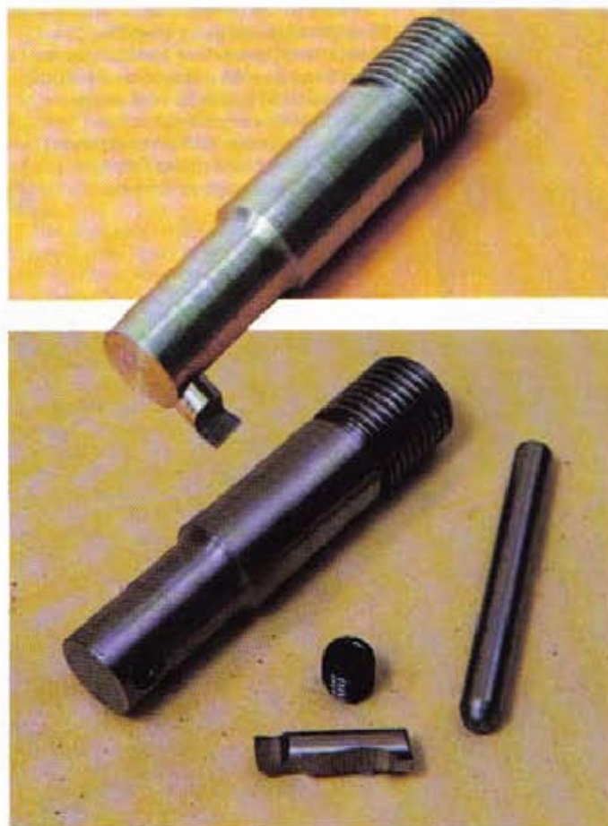
Top: A view of the completed and assembled cutter.
