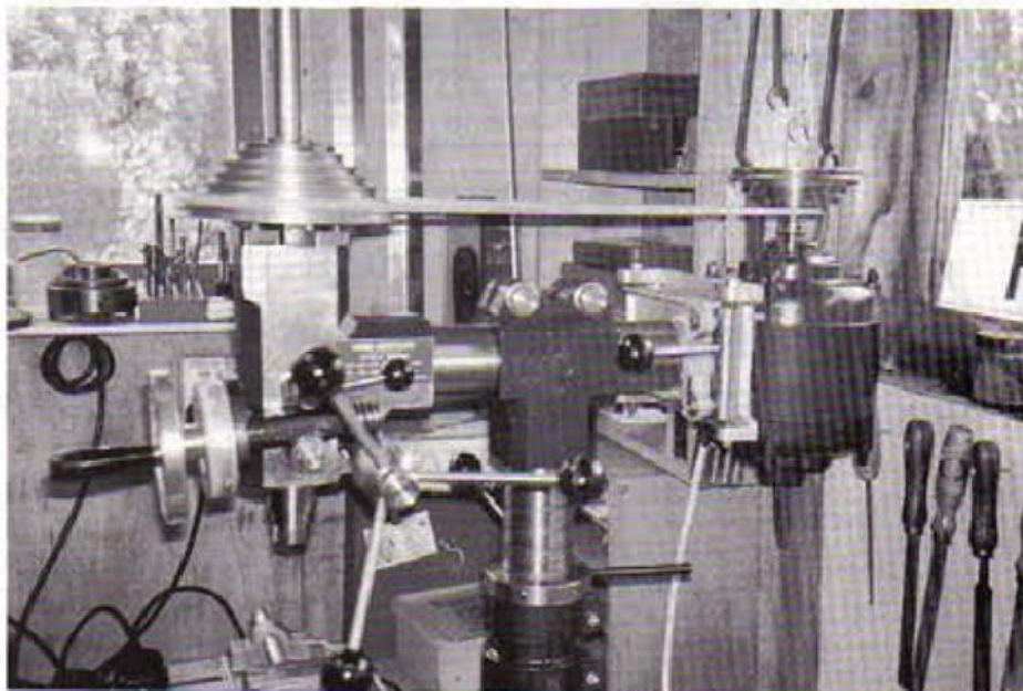
The drive arrangement, this one without gearbox.
