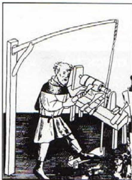
Fig. 2: A pole lathe, from a drawing of about 1395 (Mendelesches Bruderbuch).
