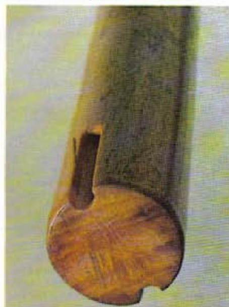
The two ends of the stick, with the actuating parts shown. Note the varnish coating on the wood in order to prevent the ingress of workshop dirt and grime.
