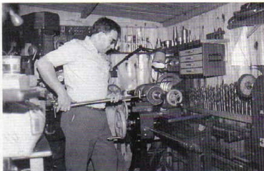
The author at work on his c.1912 Henry Milnes lathe which is used for all his spinning activities.
