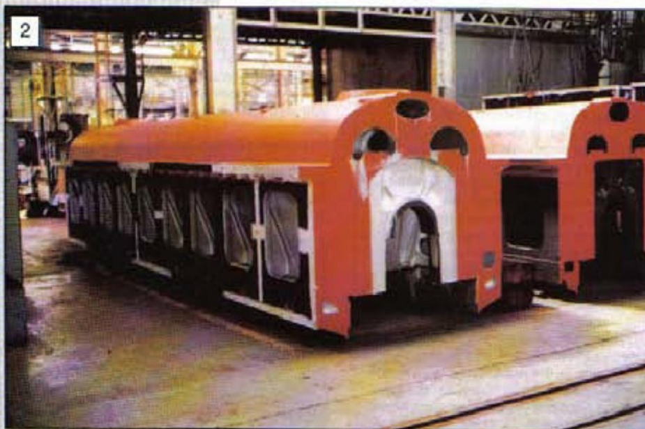
2: In an inverted position two nodular iron crankcase castings, for 16 megawatt medium speed diesel engines, await the next step of manufacture.
