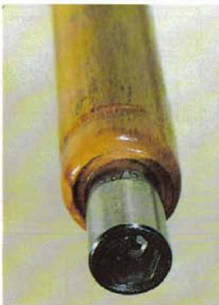
The two ends of the stick, with the actuating parts shown. Note the varnish coating on the wood in order to prevent the ingress of workshop dirt and grime.
