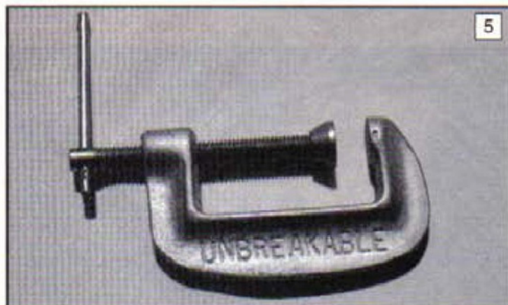
5: A "G" clamp. The frame is a malleable iron casting.
