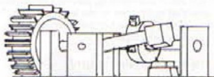
BELLY KELVE Used for wrought iron forging
