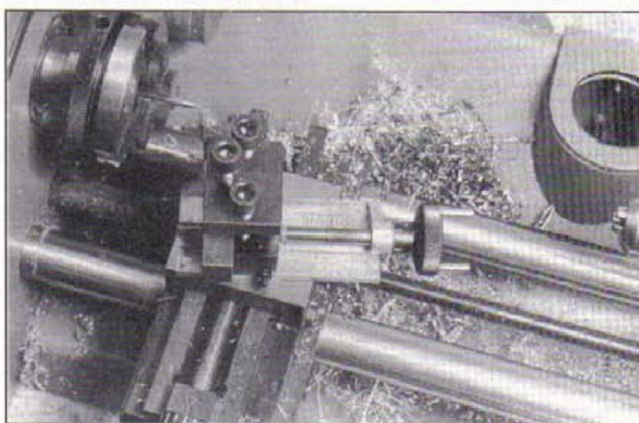
With the top slide accessory fitted to the Unimat the scriber point can be made.
