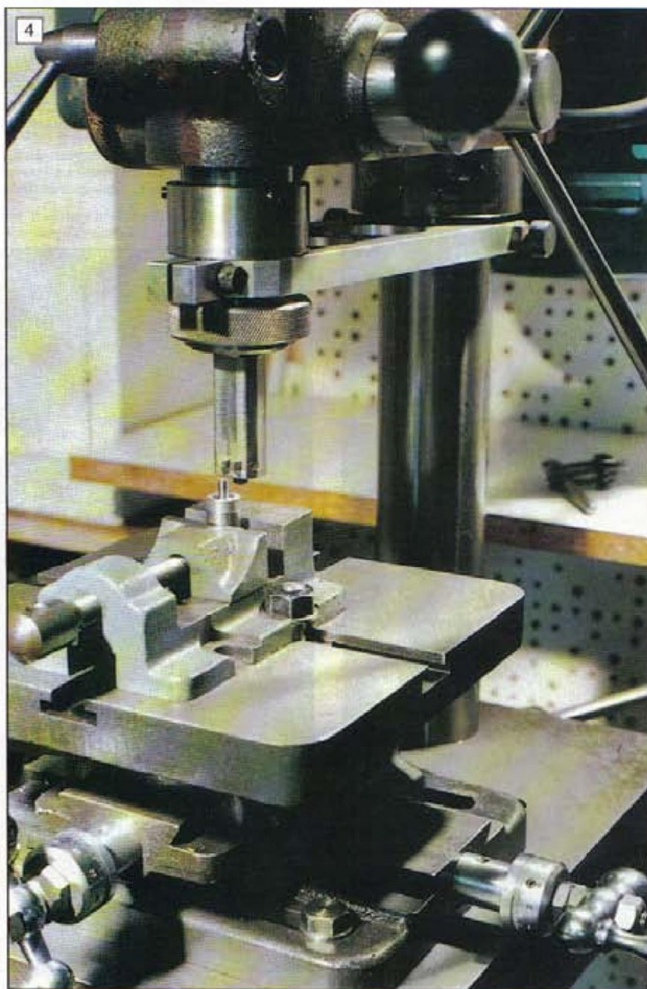
4: The complete set-up on the author's drilling machine. There is no workpiece in position, so that the undercut on the spigot is visible. The method of operation is self evident from the photograph and drawings.
