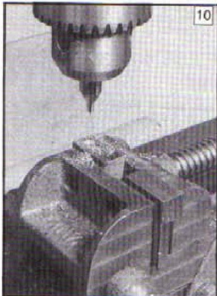
Marking with a centre drill the position for drilling the clamp pieces.
