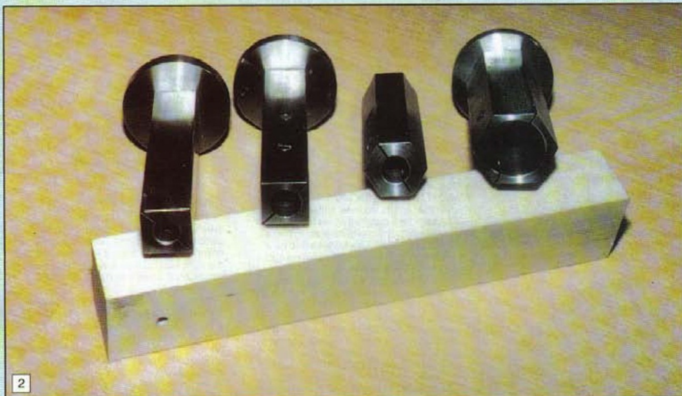
2: Four cutter chucks, one not yet fitted with its flange.
