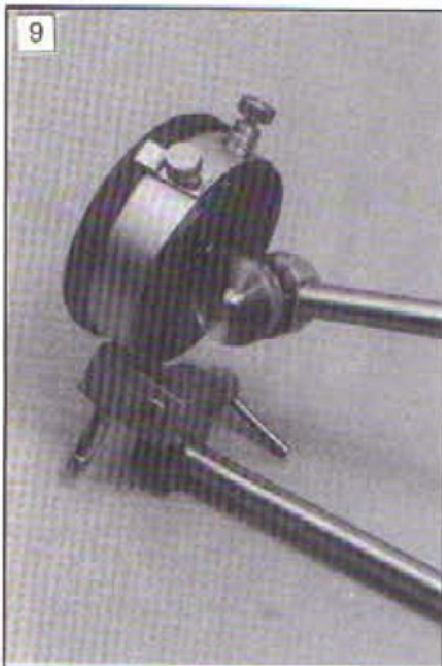
This shows the two alternative methods of mounting a DTI.
