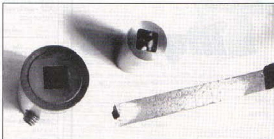
The drill and guide plate made by the author, together with a square hole drilled in a piece of brass.
