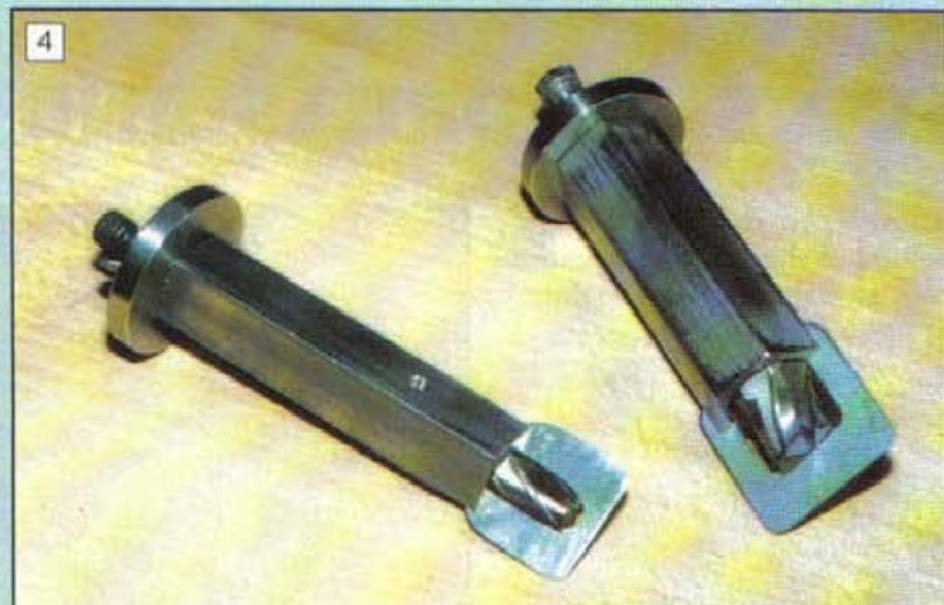
4: Two chucks fitted with cutters and shown with the locating plates being used to position the end mill/slot drill.
