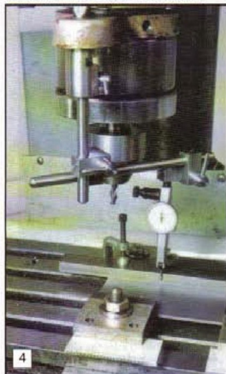
Mounting a DTI on the milling machine. This uses the arm holder which is intended to be permanently fitted to the bottom of the down feed stop bar assembly.
