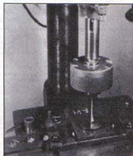
The commercial way of doing the job; the drill is held in a special chuck, and passed through the guide plate which is mounted as a drill bush would be. (Courtesy Drill Services (Horley) Ltd.)
