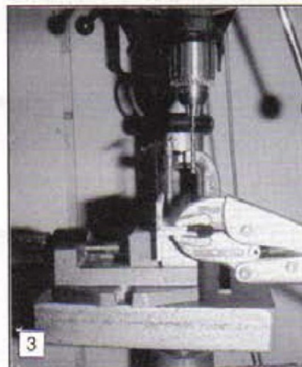
3: Drilling the base angles.
