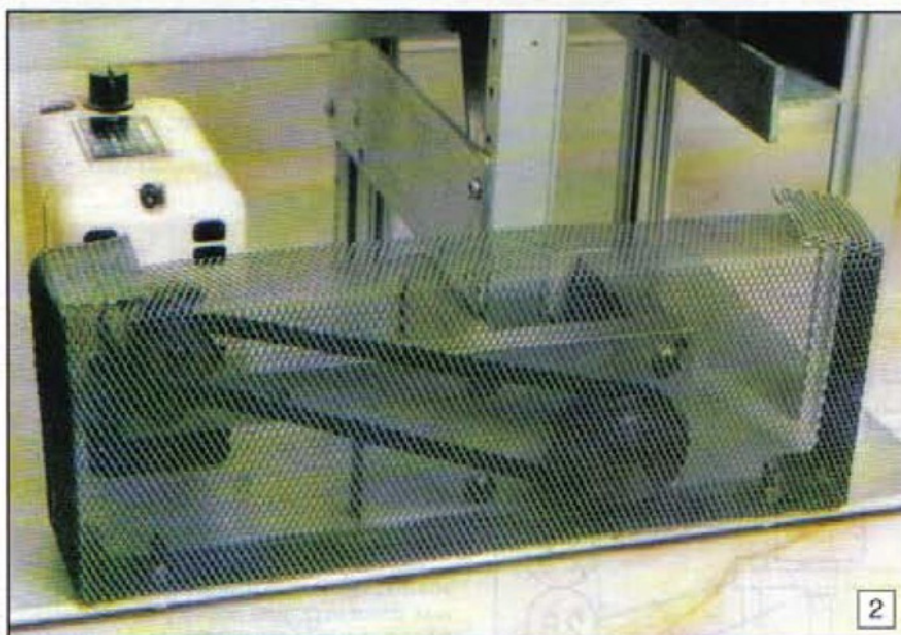
1. Drive arrangement without guard. 2. The belt guard, not detailed in the drawing. 3. Top arm pivot arrangement. 4. The lower arm guide assembly. 5. The tension stud pivot.
