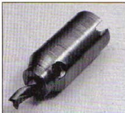
A small 1/4" shank cutter fitted into a non-split collet for use in a normal milling machine cutter shank.
