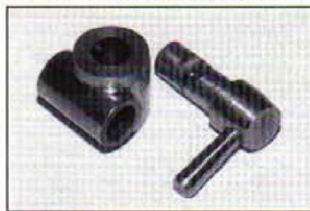
Down-feed stop with cotters exposed.
