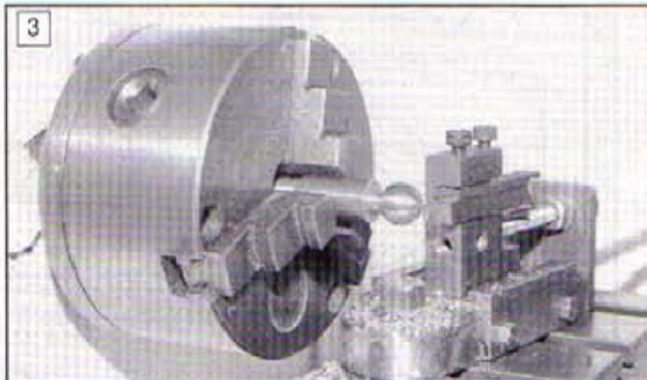
3: A few minutes later, the ball is formed on one end of the blank, all that remains is to turn the other ball and remove the surplus material between the balls.
