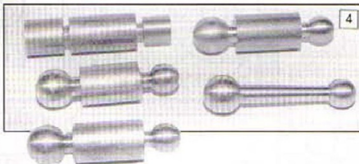
4: Some of the work in progress, from blanks to ball ended handles.
