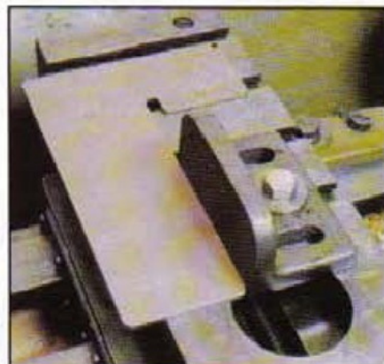
Using the centre finder as a normal square for positioning an angle plate on the lathe cross slide.
