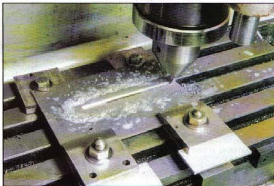
Shaping the plate on the vertical milling machine.
