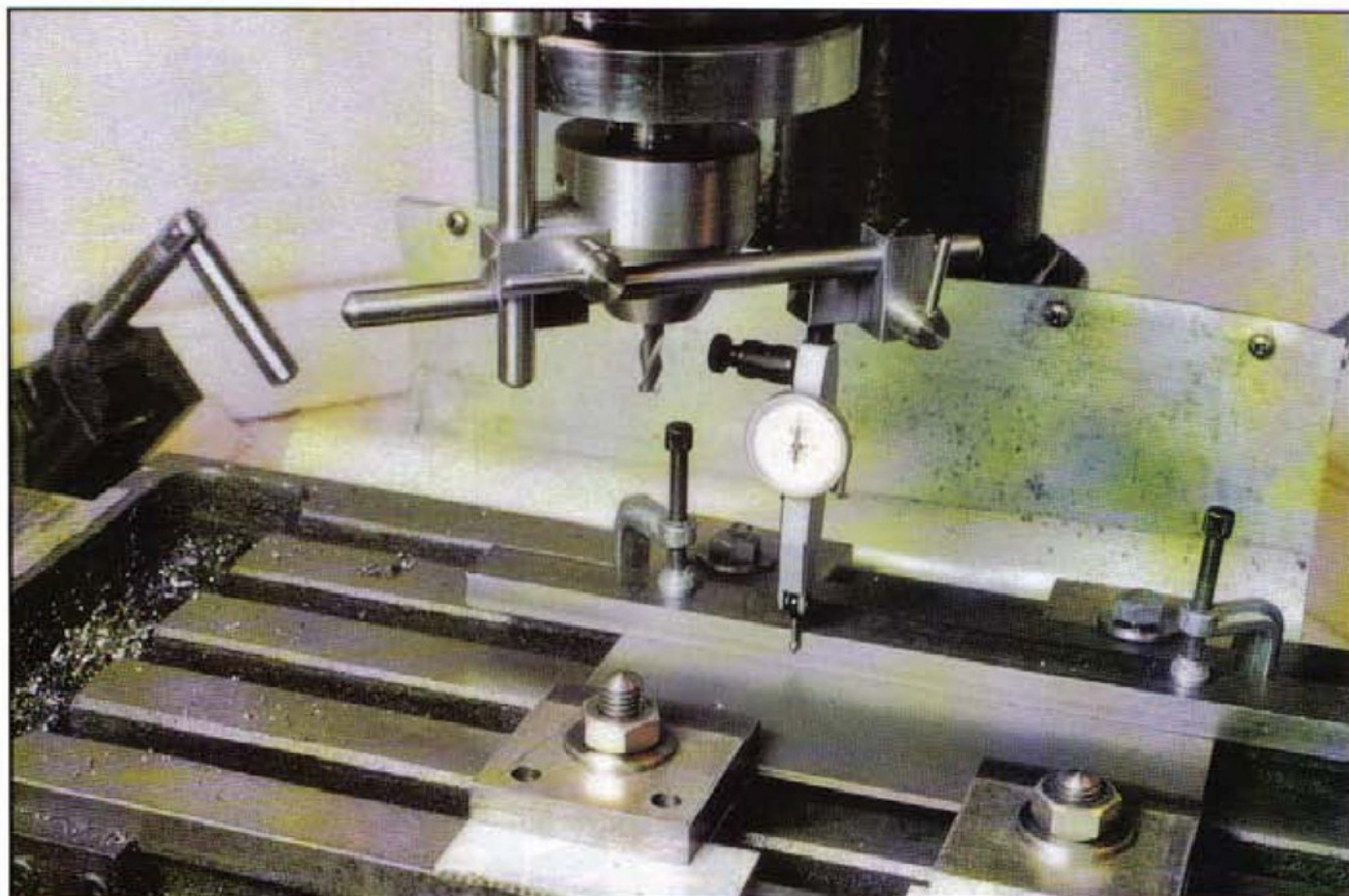
Use of the milling machine to make the square; positioning the plate for shaping.
