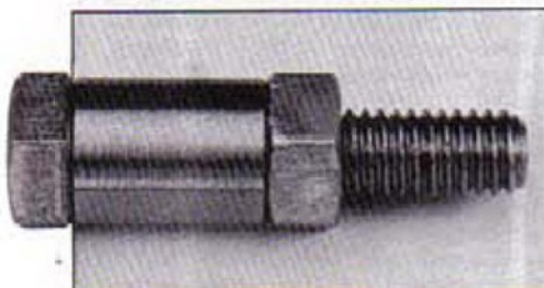
With the bush diameter equal to the A.F. of the hex., the screw can be held in the three jaw chuck for drilling.
