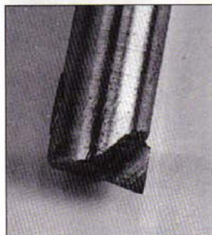
With the cutter ground as shown, it can be used for hole sizes almost as small as the bar itself.
