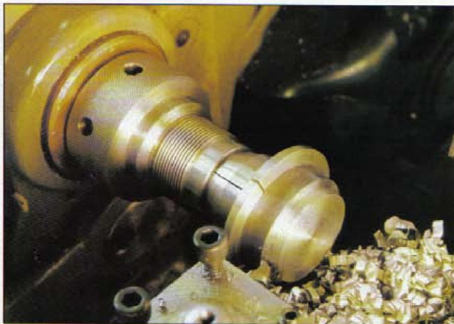
Photo 3: A finished loose jaw collet gripping a 1 1/2" dia. piece of BMS having a 1/8" wide cut made on it.
