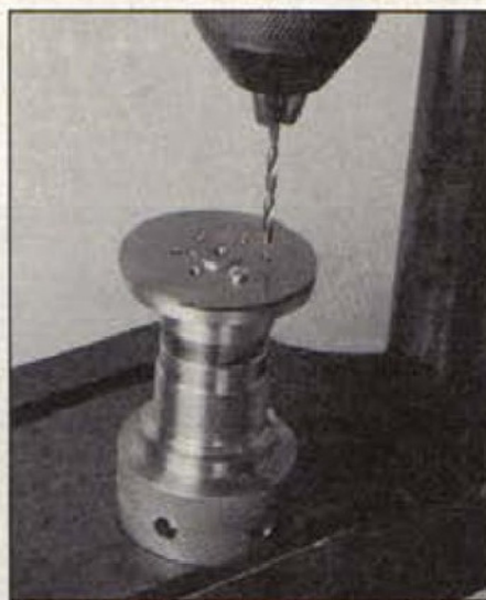
Photo 8: Drilling the loose jaw collet using first jaw as a jig; holding was overcome by use of the collet assembly body stage.
