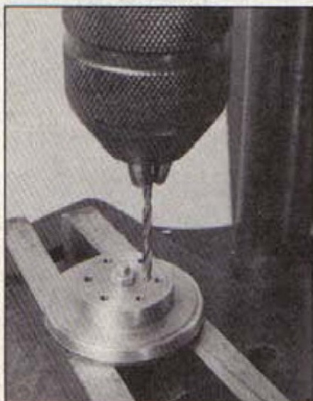
Photo 7: Using the drilling jig to drill a loose jaw.
