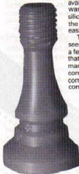
Try Cut can be turned, threaded, milled, etc.; lots of workshop applications.
