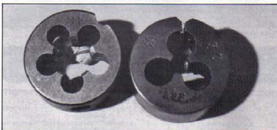
Two types of die, one typically British, the other continental; note lack of slot on continental die on left.
