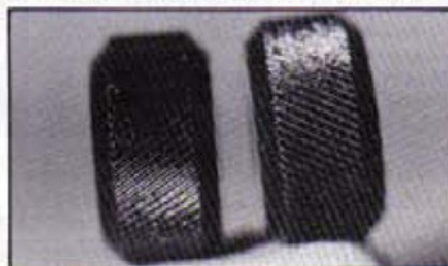
A pair of knurling wheels of diagonal pattern; used as a pair, they will produce a diamond marking.
