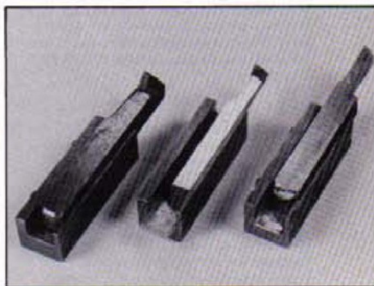
The shims seen in this view ensure that the tool is immediately ready for use at the correct height when mounted on the top slide.
