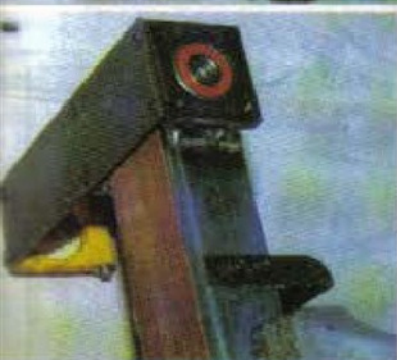
Sander can be used horizontally, vertically or at any convenient angle in between (top left). Top right, close-up of tensioner detail. Above left, underside view; note the simplicity of the bracket. Above right, the modified drive and table are evident in this shot. Unit uses a standard Bosch 500 portable drill.
