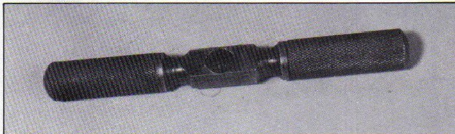
A typical tap wrench; the square on the tap fits into the 'V'.
