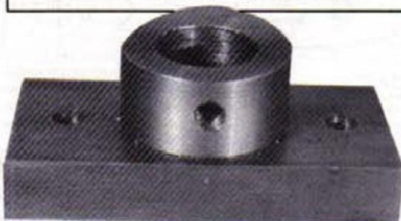
Two views of the base; note the tapped hole for the locking screw.
