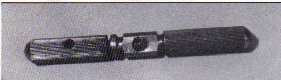
This tap wrench has worn round where there should be a 'V'; using it could lead to tap breakages.
