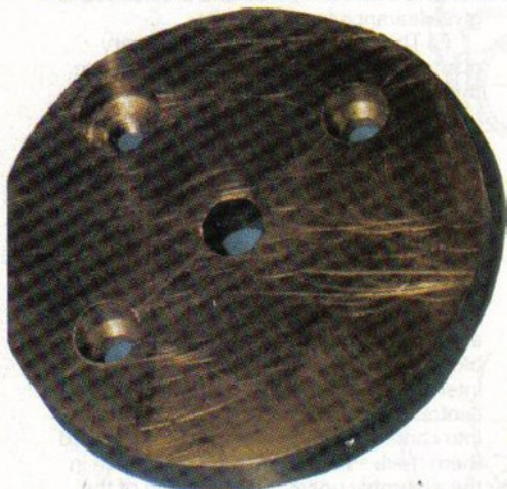
The base of the tool; ignore the central hole — it just happened to be in the scrap material used!
