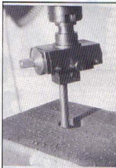
Fig. 4. Boring the hole for the top-slide spigot.
