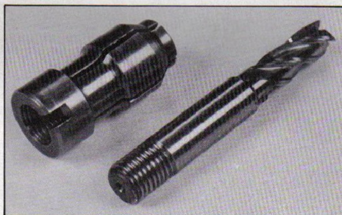
A collet shown with a typical cutter; note the thread in the rear end of the collet and the anti-turn slot. Close-up of chuck internals at left.
