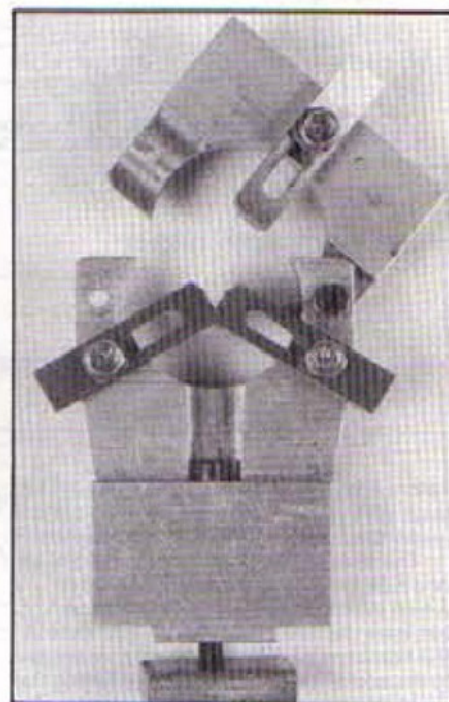
It can be seen here how the top hinges, allowing parts to be removed and replaced without losing the setting.
