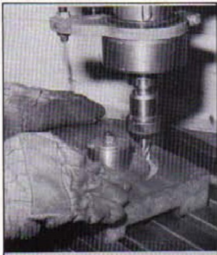
Fig. 6. Misusing an end mill to cut a circular slot.
