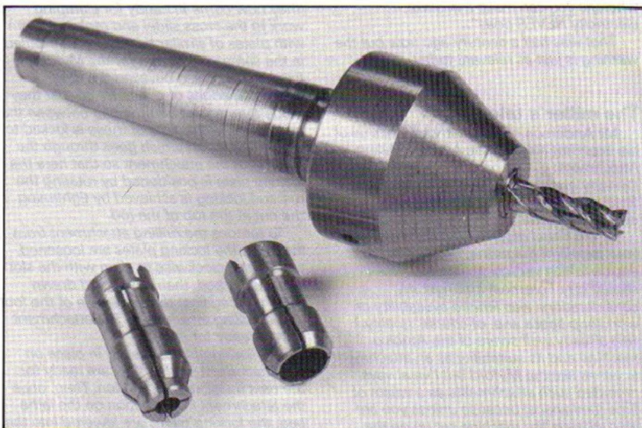
Completed chuck and collet set for use with \frac{1}{4} in. shank cutters; a non-slotted version for this size using a grub screw for fixing the cutter would be useful.
