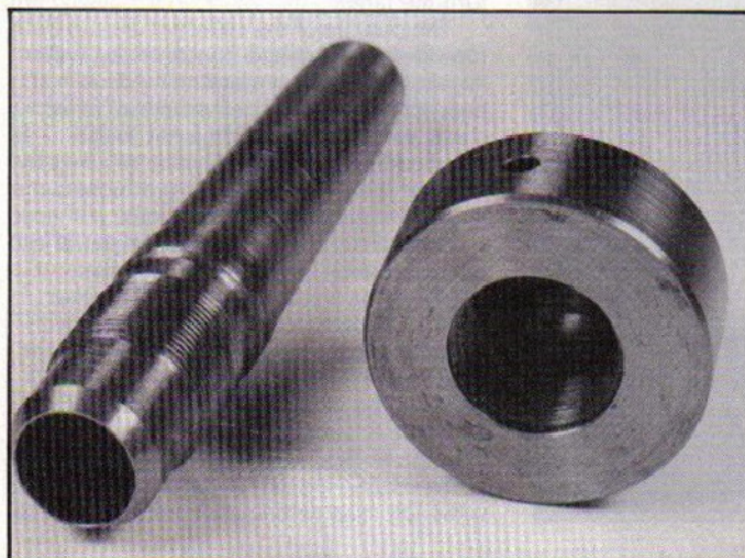
A collet shown with a typical cutter; note the thread in the rear end of the collet and the anti-turn slot. Close-up of chuck internals at left.
