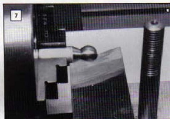
Photo 5. The cutting tool for boring the taper – in this case a modified half-round tool is excellent. Photo 6. The tool in action taking a smoothing cut. Photo 7. Turning ball with formed tool (top clamp removed).
