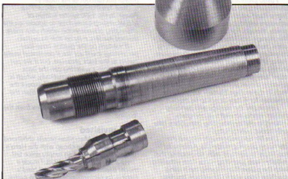
The three main components; note the short parallel portion at the left hand end of the morse taper, used to support the part in the fixed steady whilst the bore is machined.
