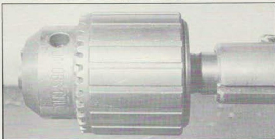
The normal type of tailstock chuck; usually retained by a Morse taper, it is used to hold drills and other small tools.
