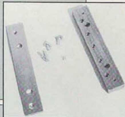
Parts for the sprung jaw; the backplate is attached with countersunk screws and keeps the sprung plungers in position.
