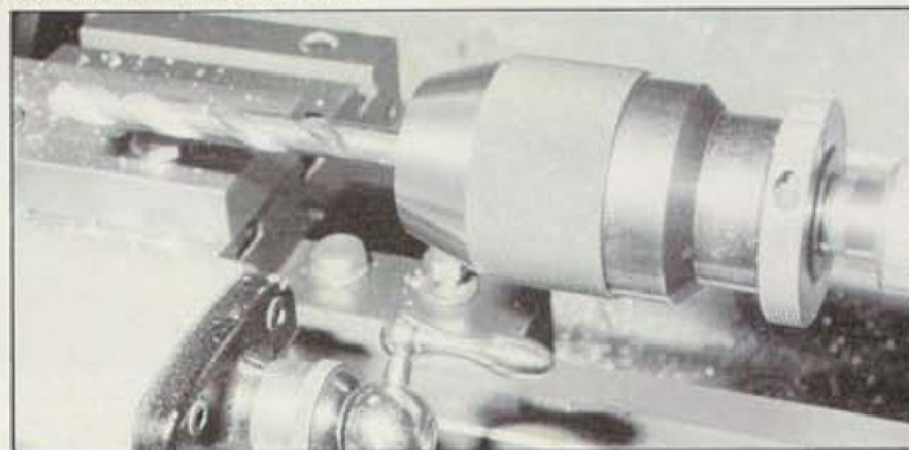
The Keyless chuck (above) is useful where a number of drills need changing. Right, a set of bell chucks. These are used for holding thin, large diameter work and we'll show you how to make a set in a future issue.
