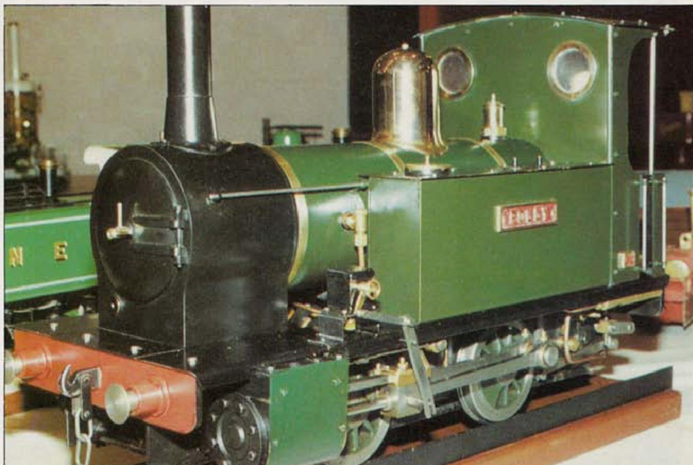
Outside rods and valve gear on a 'William' 2-6-2T in 3 1/2 in. gauge by G. Hammond (above); a rotary milling device like that described is ideal for this sort of work.
