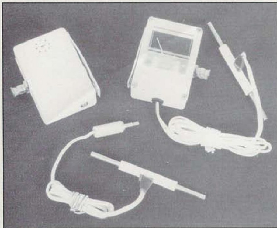
The two completed devices; at left, the acoustic edge-finder/tester and meter at right. The probe is in the foreground.
