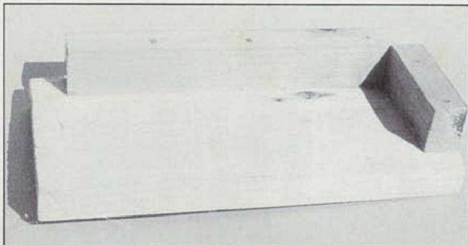
When soldering, the use of a simple jig is an advantage. A wooden one such as this allows joints to be made at 90 degrees with precision as long as the jig is accurately made.
