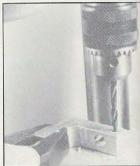
Drilling the bracket which is held in a large toomaker's clamp while the operation is carried out.
