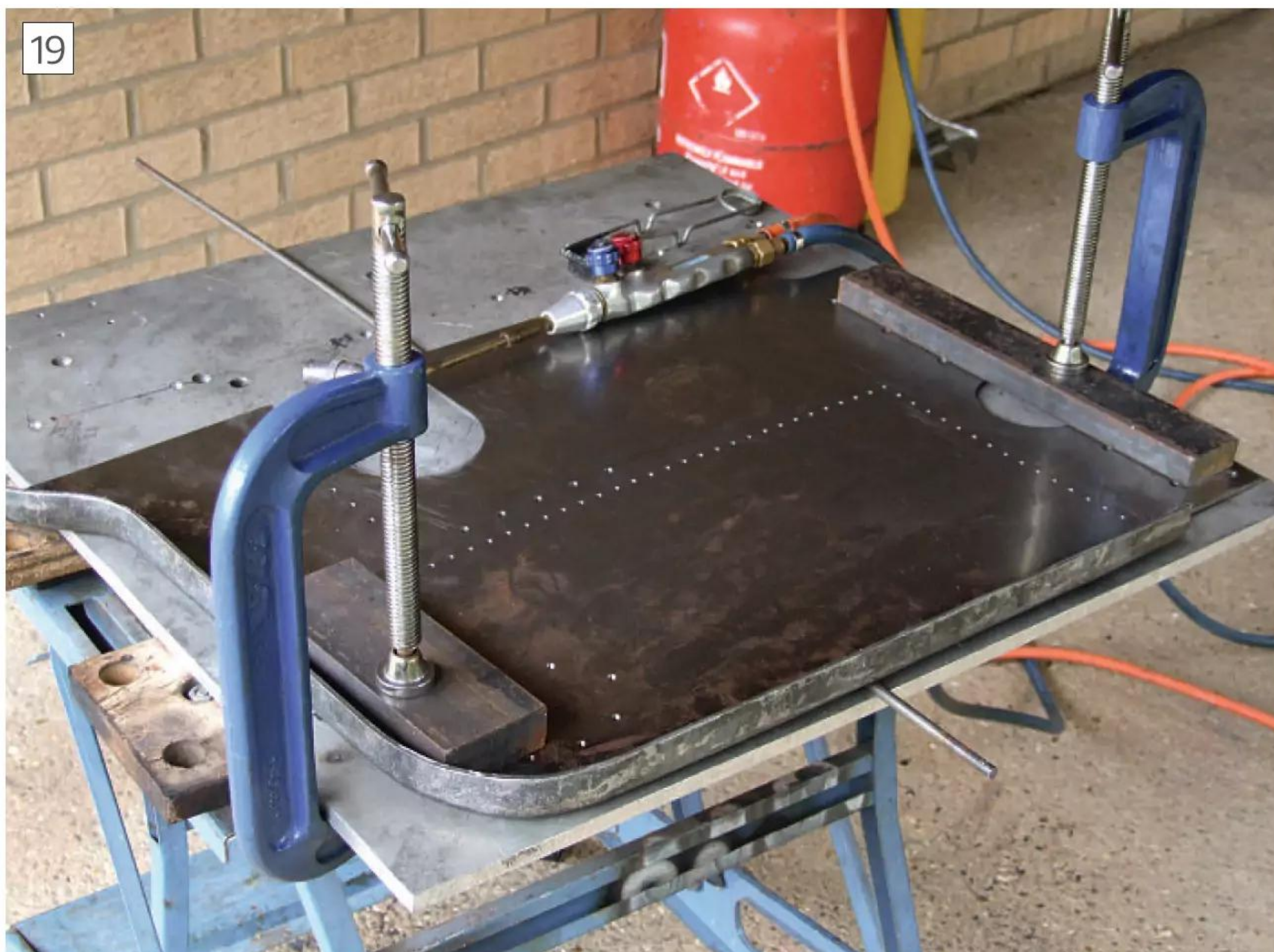
Set Up for Correcting Lengthwise Bowing
