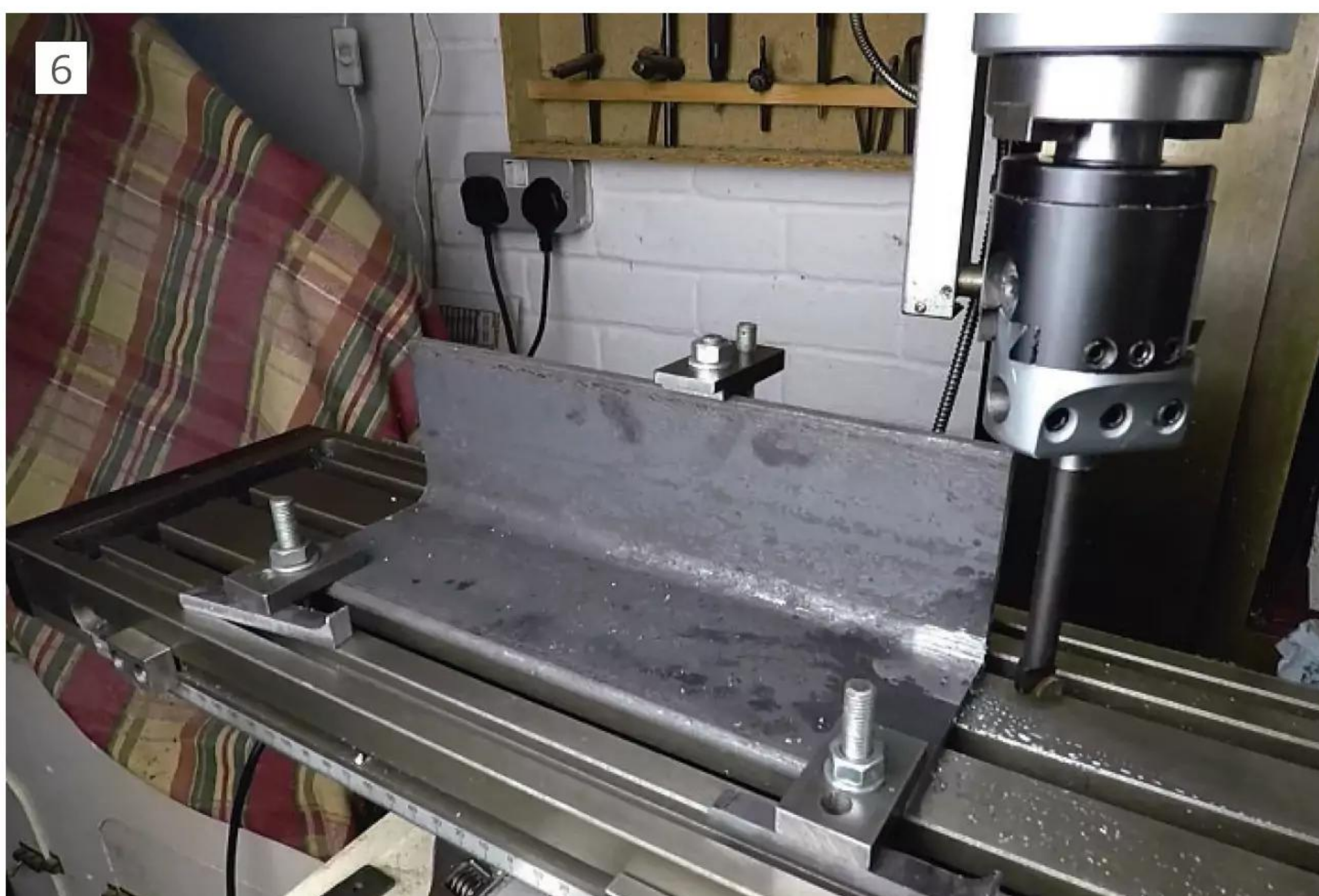
Using a boring head to machine the flats on the angles ready to receive the hinges.
