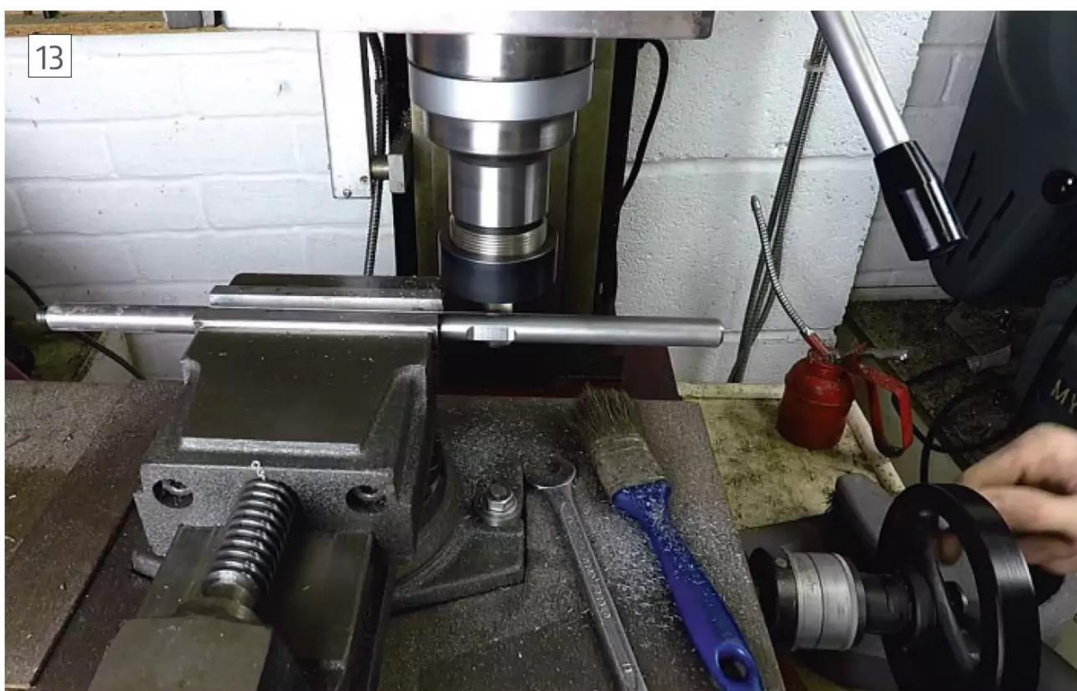
Machining the spanner flats on the handles using the side teeth of an end mill. The mill table stops were used to set the length of the flats.
