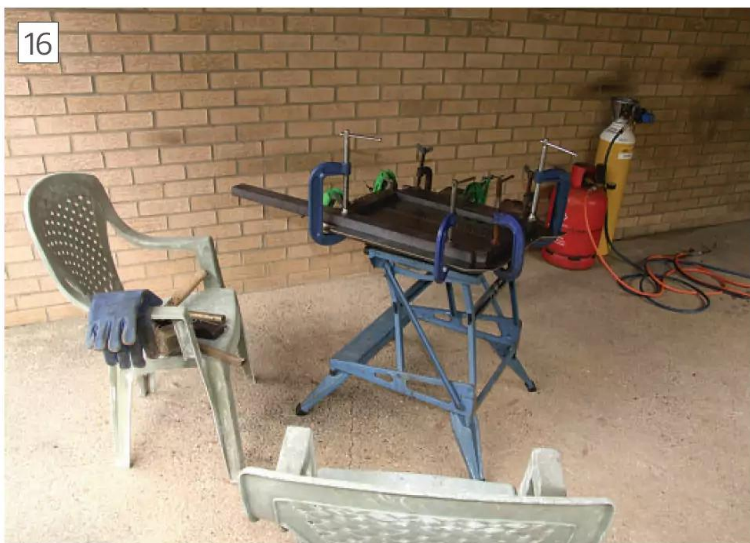
Set Up for Flanging Tender Sides
