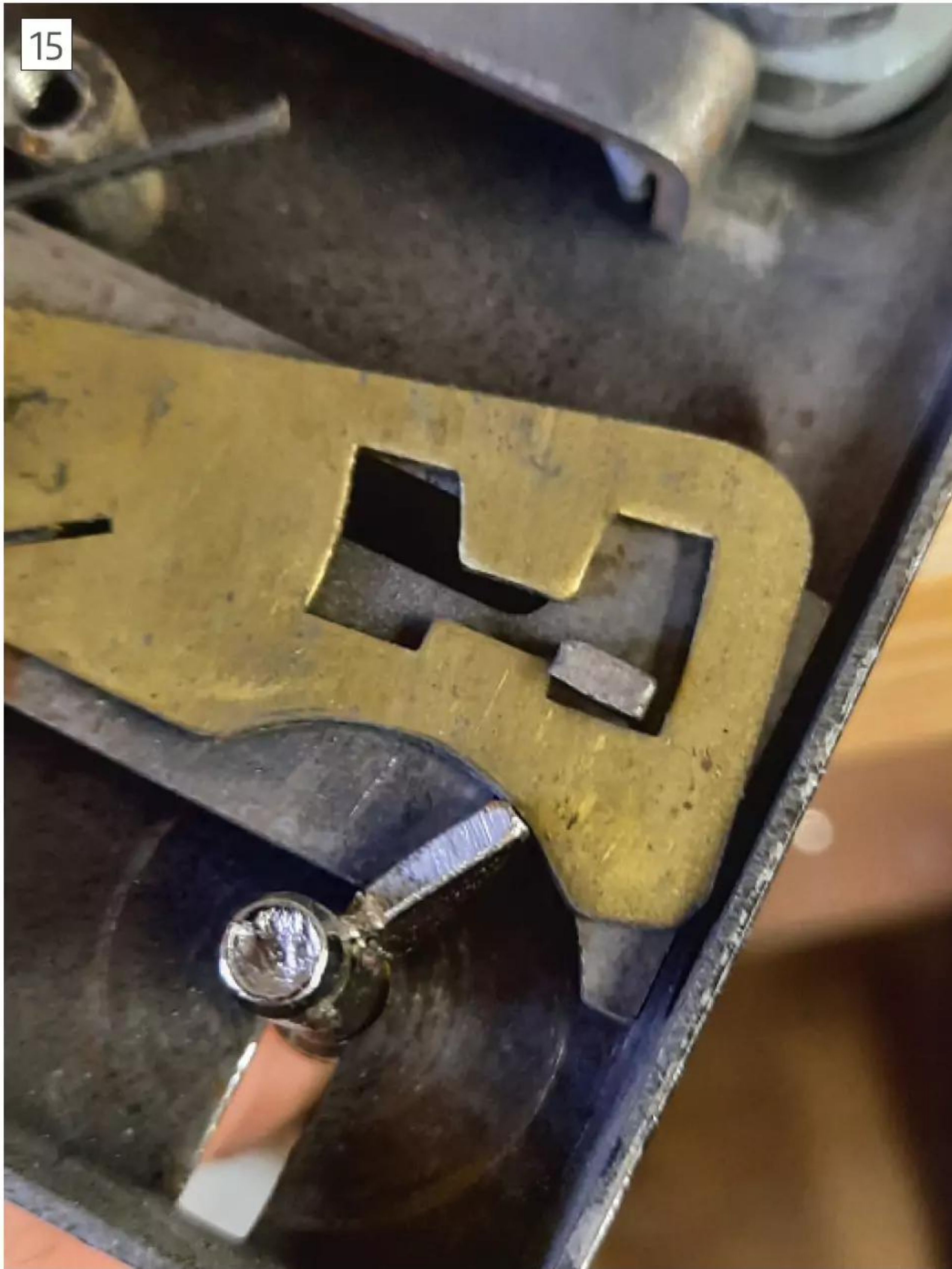
The key needs to be cut to fit the levers as the stump fouls the bar.
