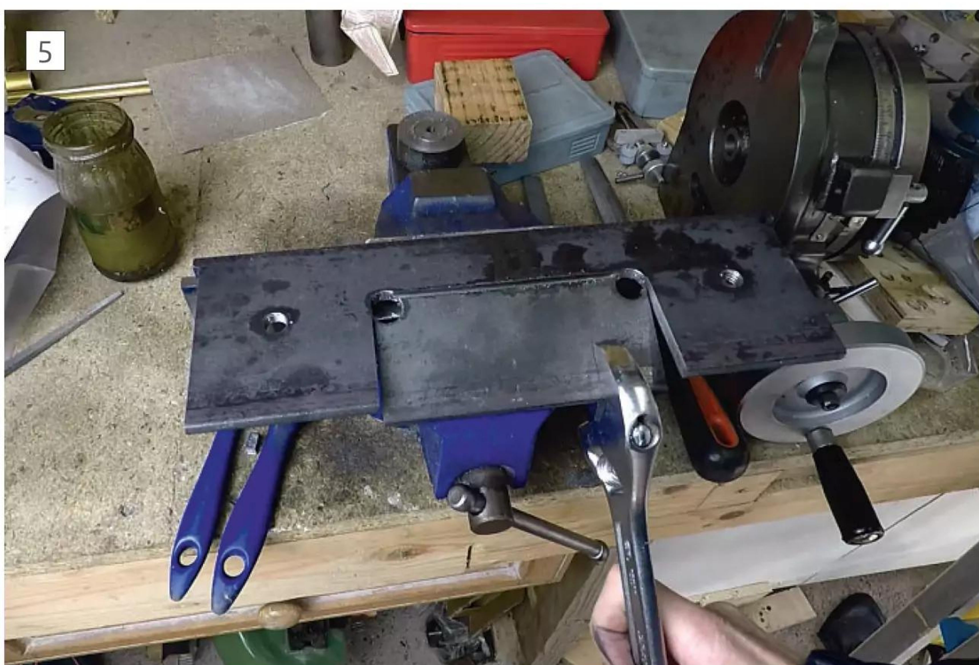
Breaking away the waste section with an adjustable spanner.
