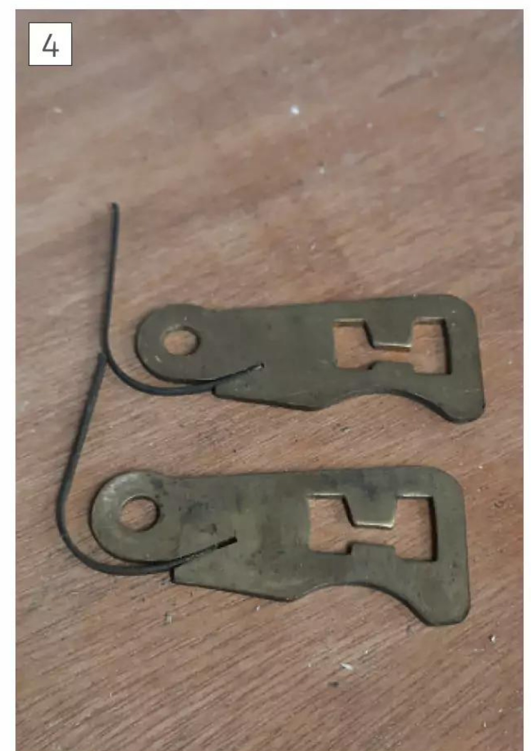
The two brass levers with steel springs. A three lever lock has two of these, a five lever has four and so on.
