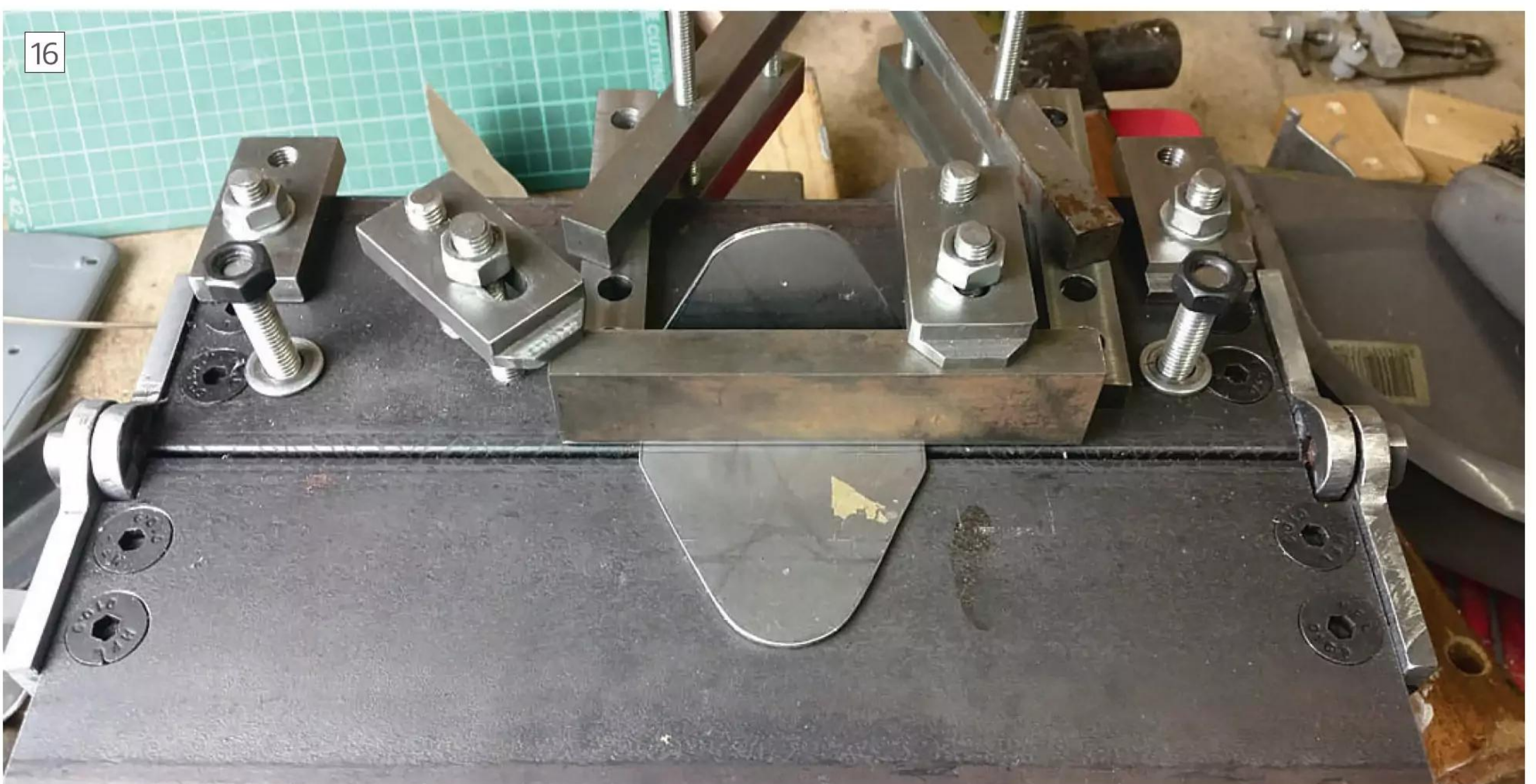
16 The clamping arrangements necessary to hold a U-shaped workpiece. The first bend has already been formed and the clamping block is being used to prepare for the second bend.
