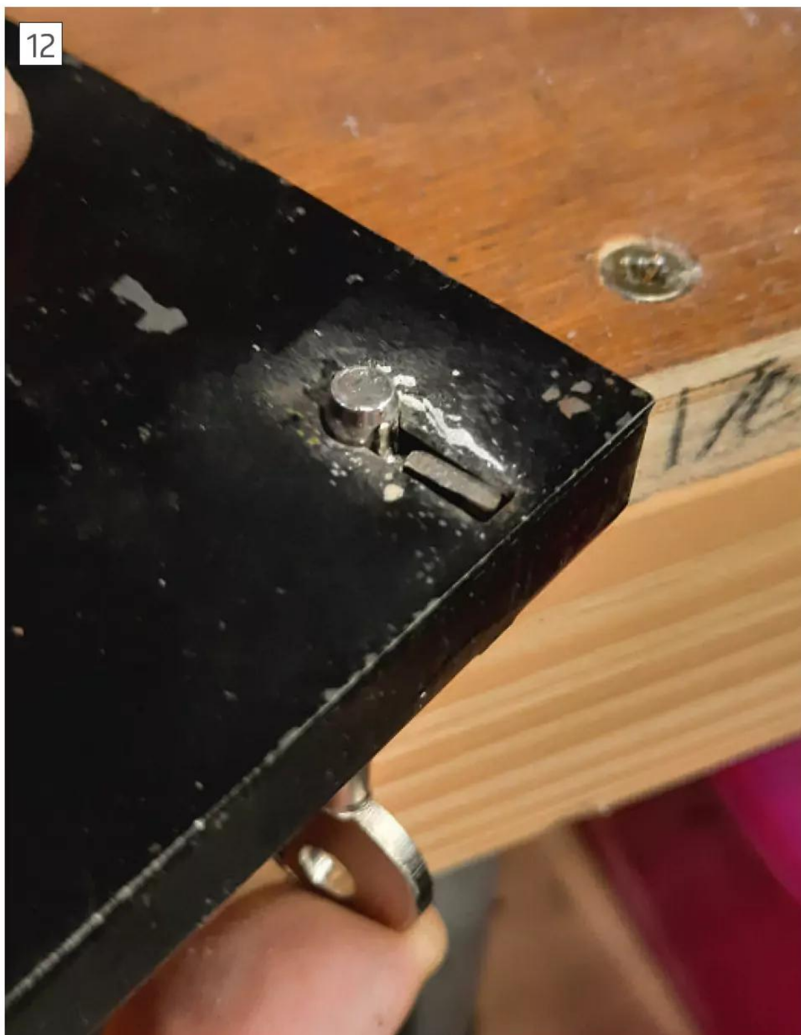
With the case cover in place the key must not foul the edges of the far keyhole.
