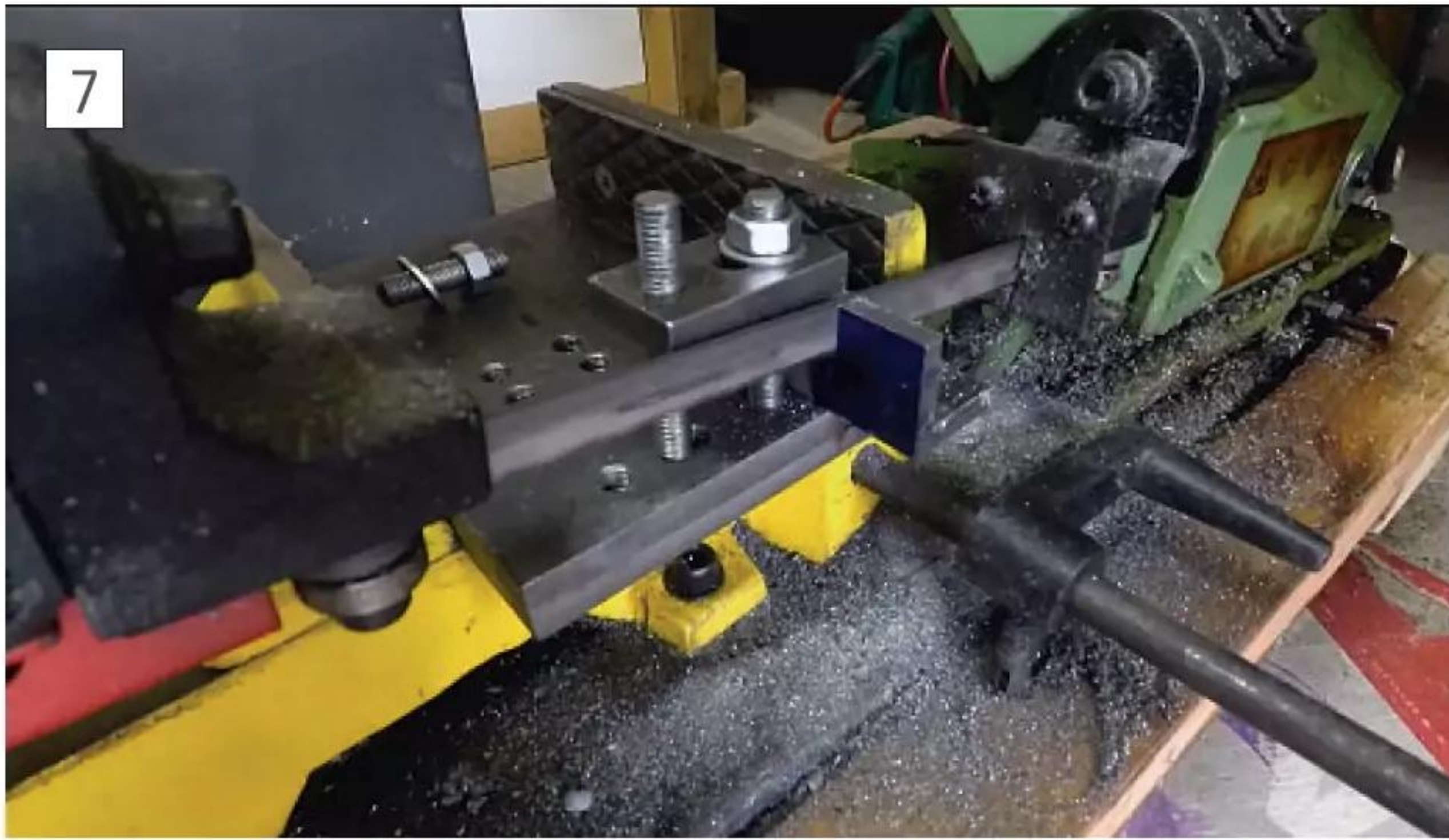
Using a fixture held in the bandsaw vice to secure the hinges for cutting operations.
