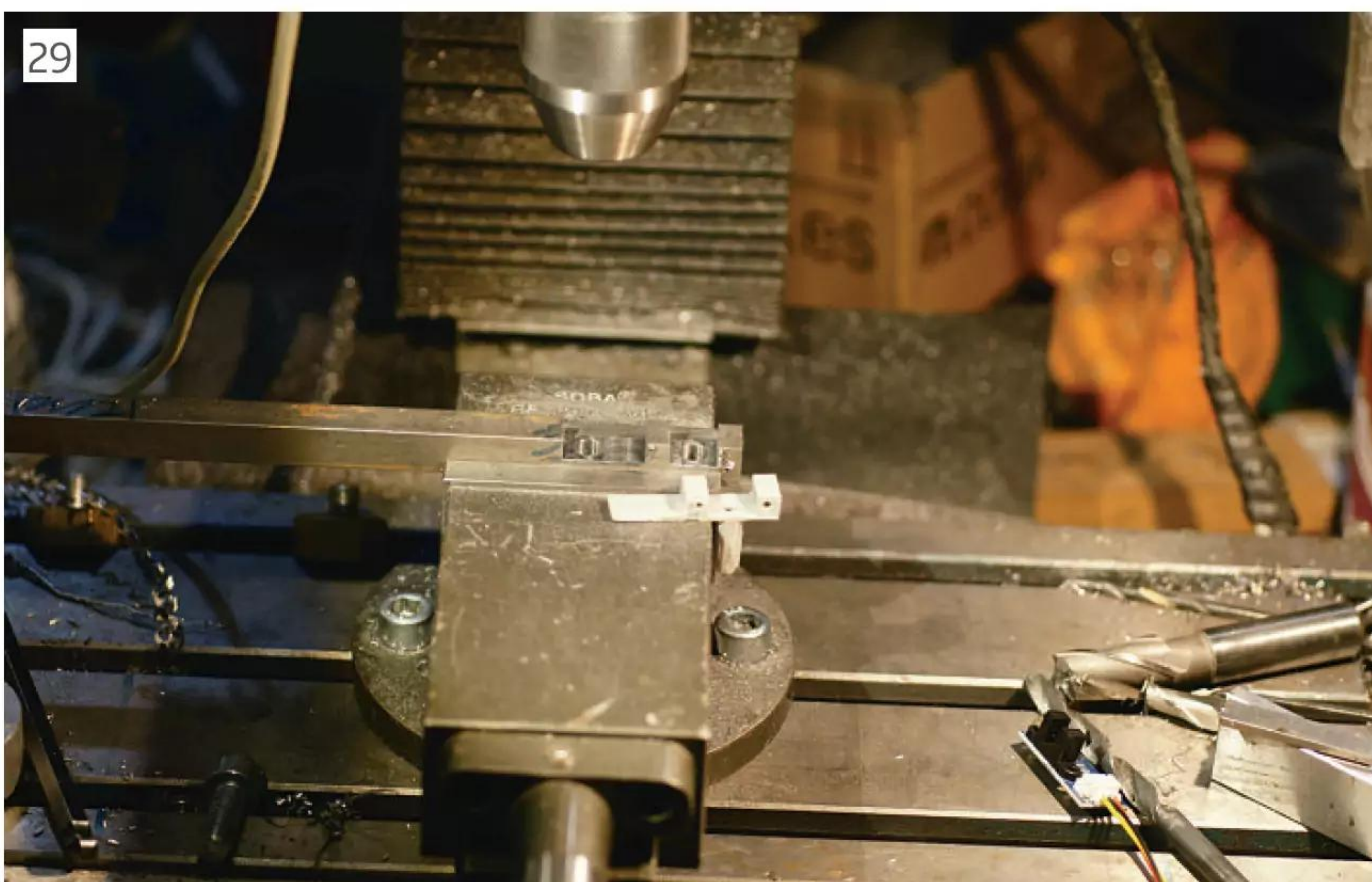
Slots hacked out and holes machined for the two rods. The 3D printed concept piece in the foreground.
