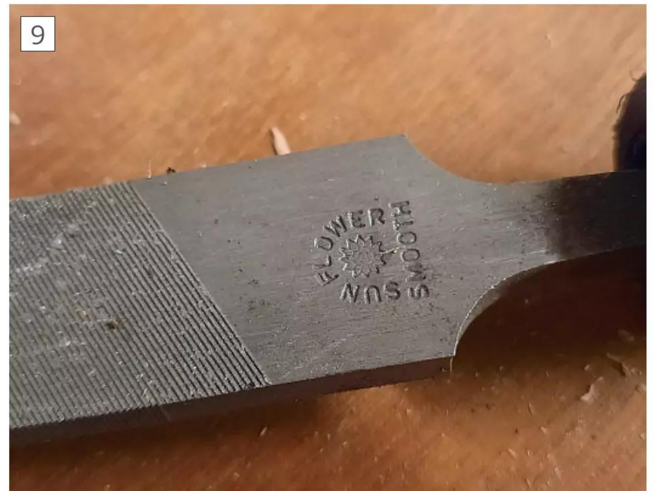
I chose a smooth cut file to avoid the risk of removing material too quickly.
