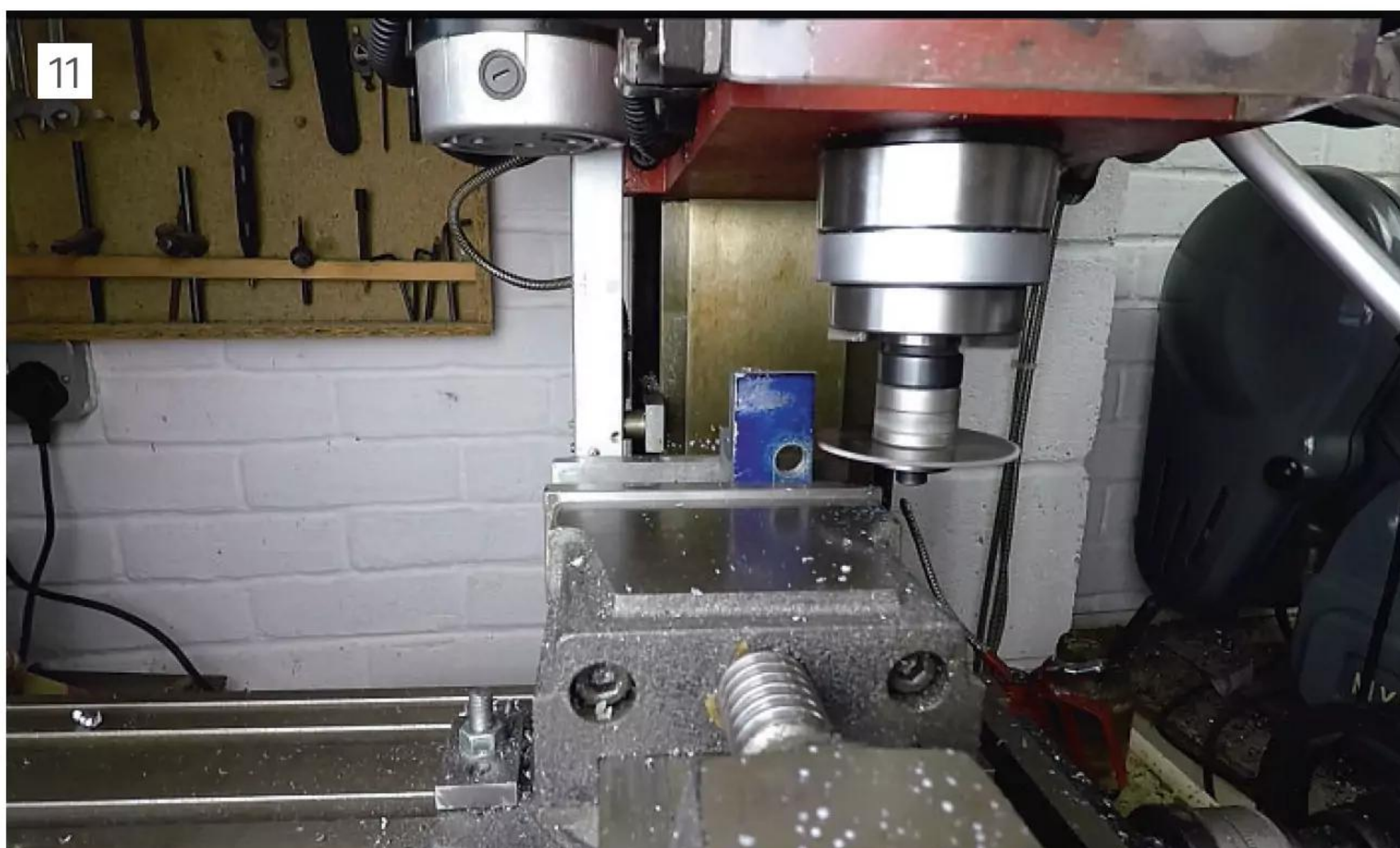
Removing waste material from the hinges using a slitting saw. A drilled hole forms a nicely filleted corner to the work.
