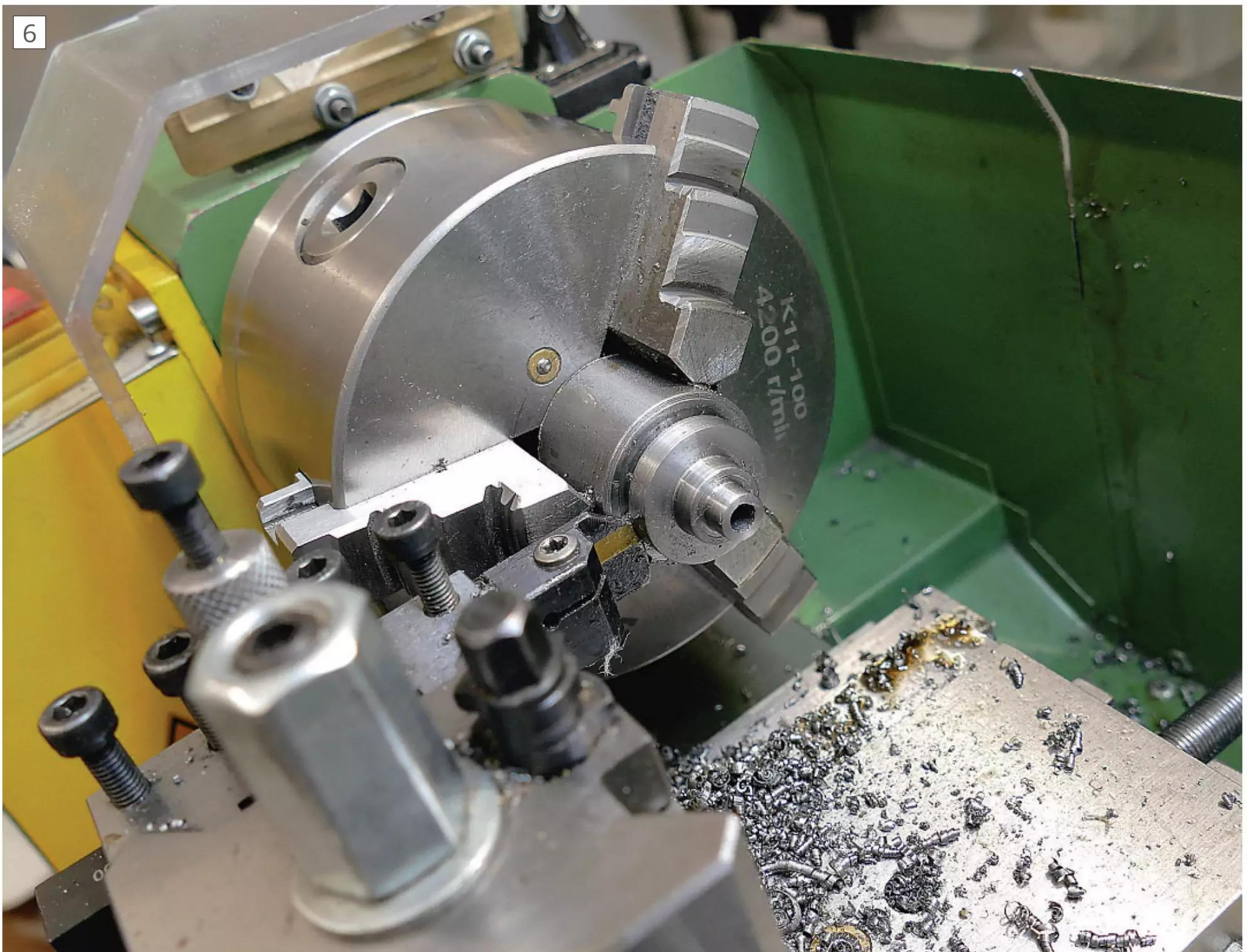
6 Parting off the last insert (8mm).
