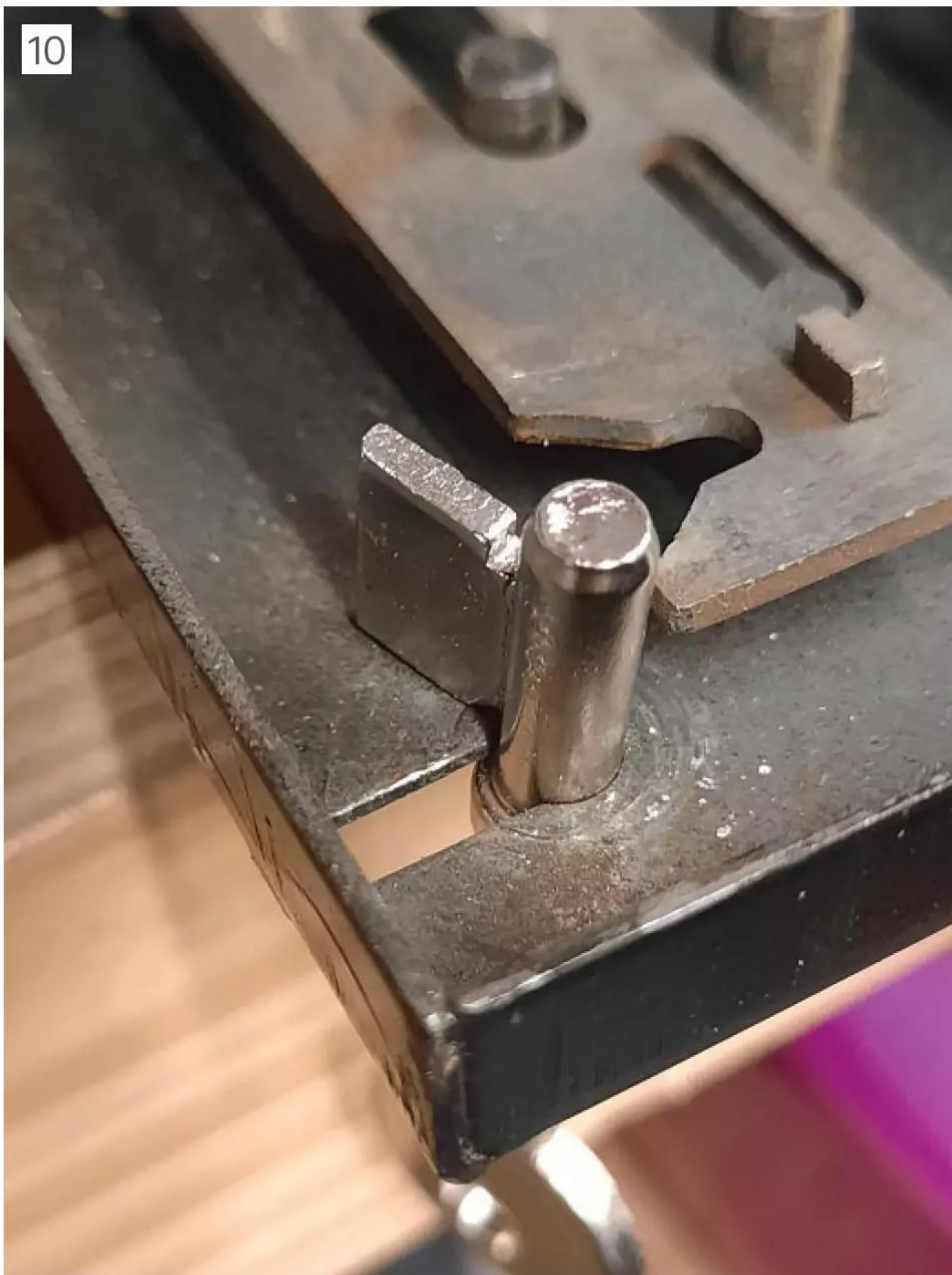
The collar to bit distance had to be increase slightly.
