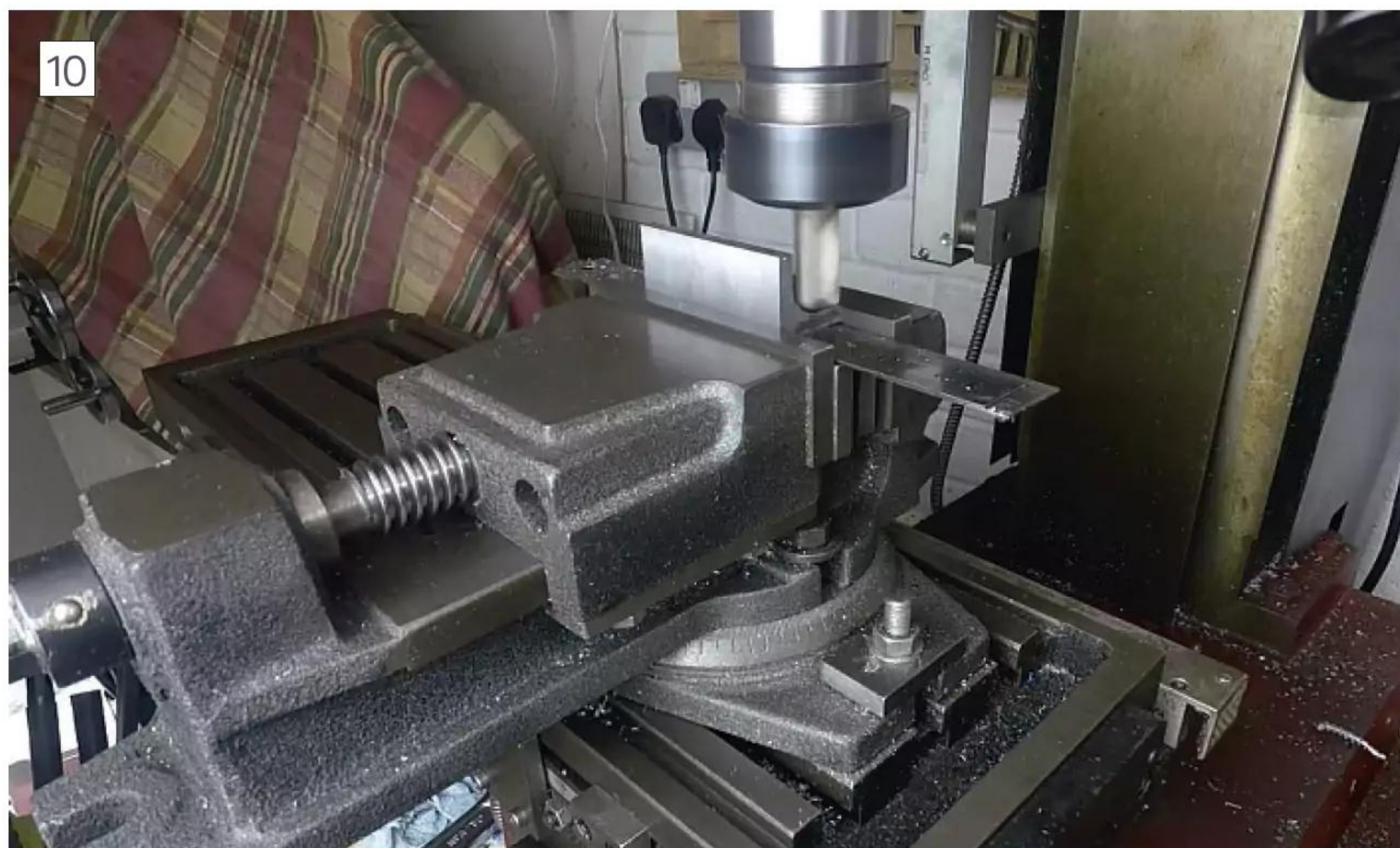
Removing the fillet on the inside corner of the hinges to create a sharp angle. An end mill was used and the work has been positioned on parallels in the vice to keep it square. The steel rulers are acting as spacers to bring the work to the correct height.
