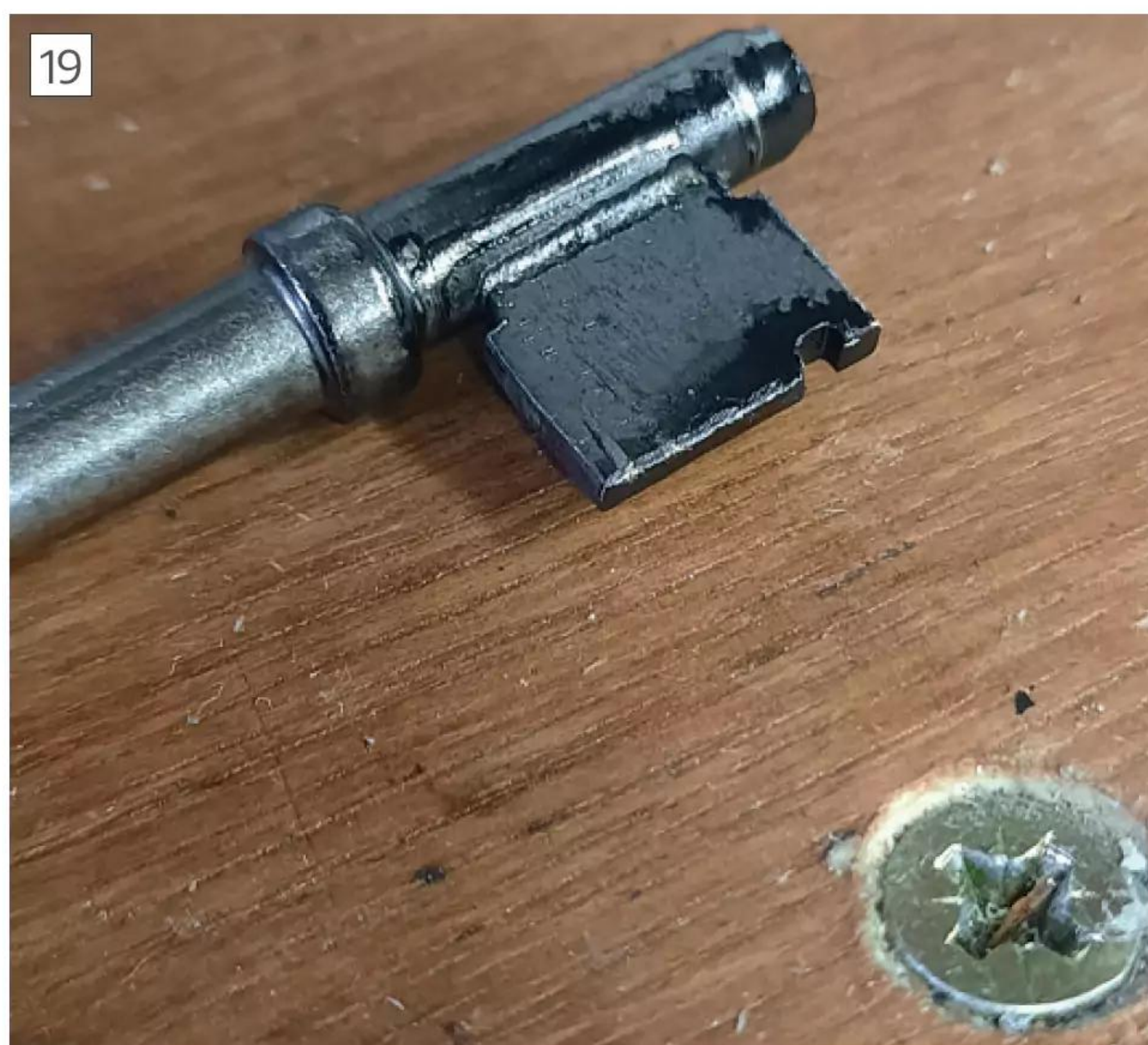
Key sprayed and used from the other side of the lock, the two scratch marks show where it contacted the levers.
