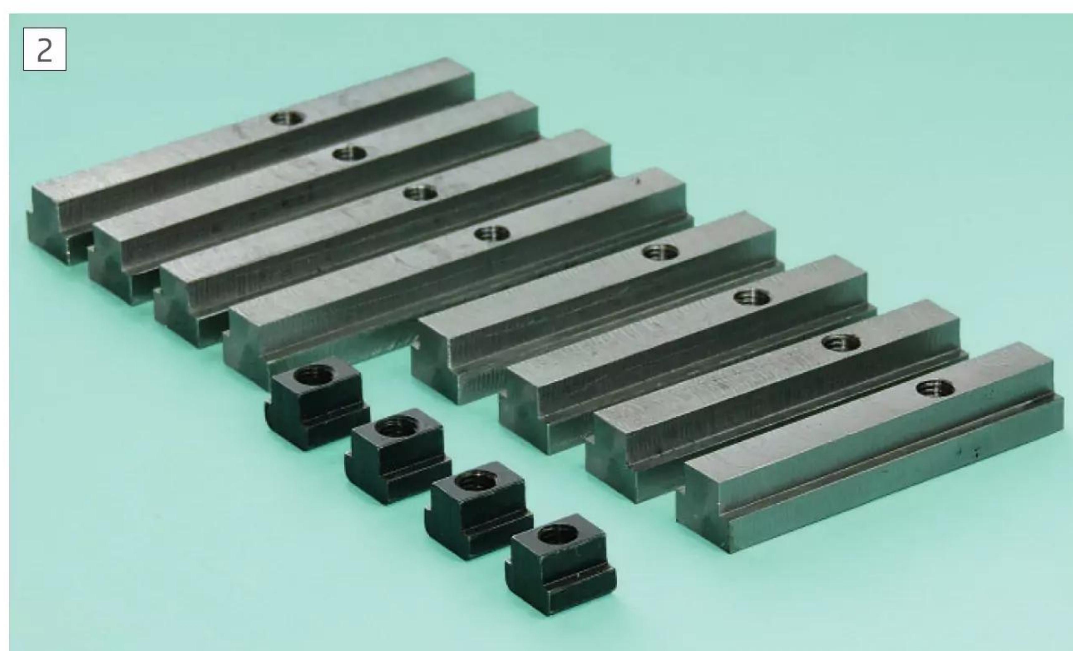
The two sets of extended length tee nuts that were made for the Rishton milling machine table, shown with the small tee nuts that were used previously.
