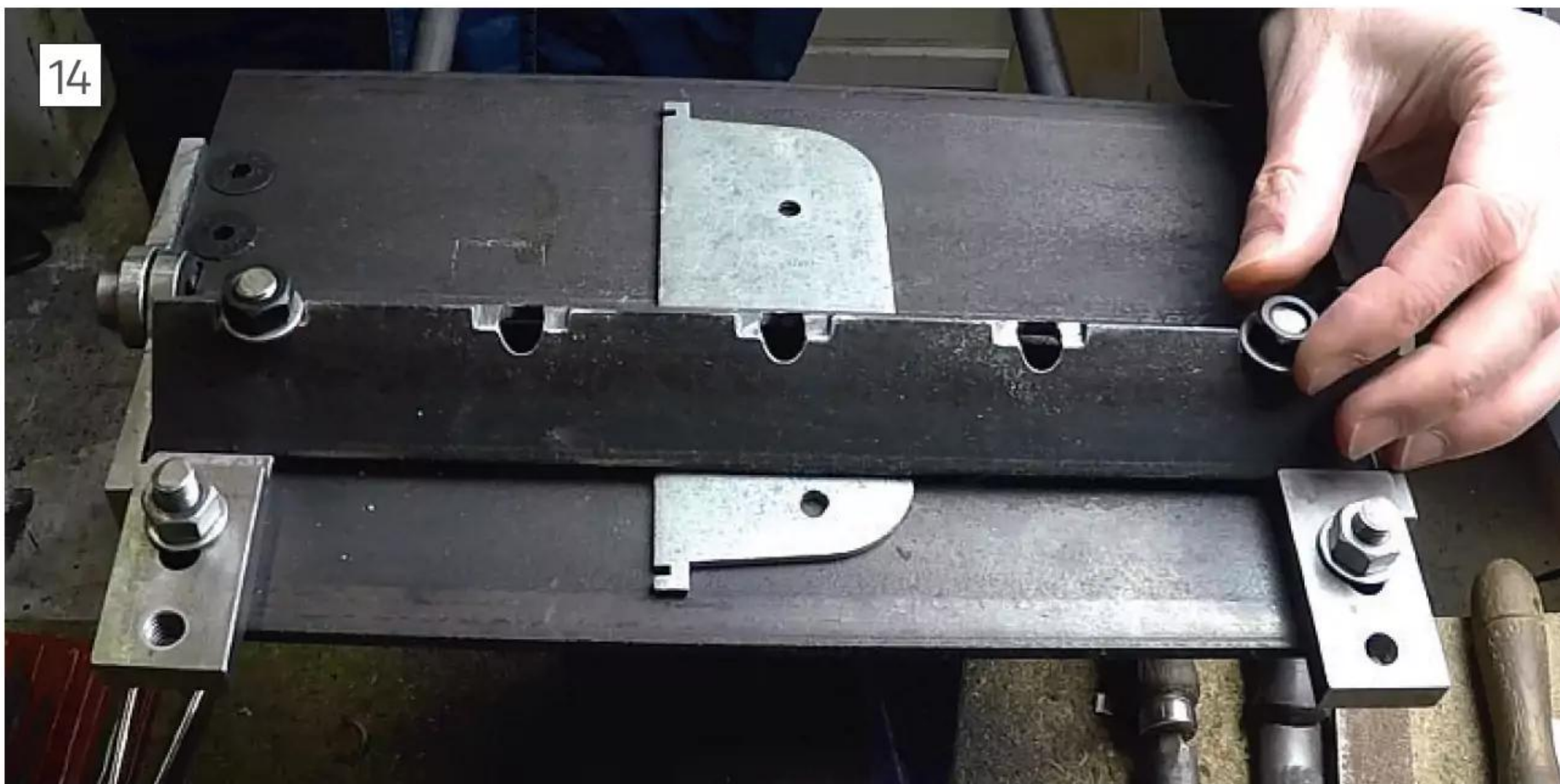
14 Setting a test piece ready for bending. The clamp is bolted down onto the work and the two dogs prevent the clamp from moving under the considerable bending forces.
