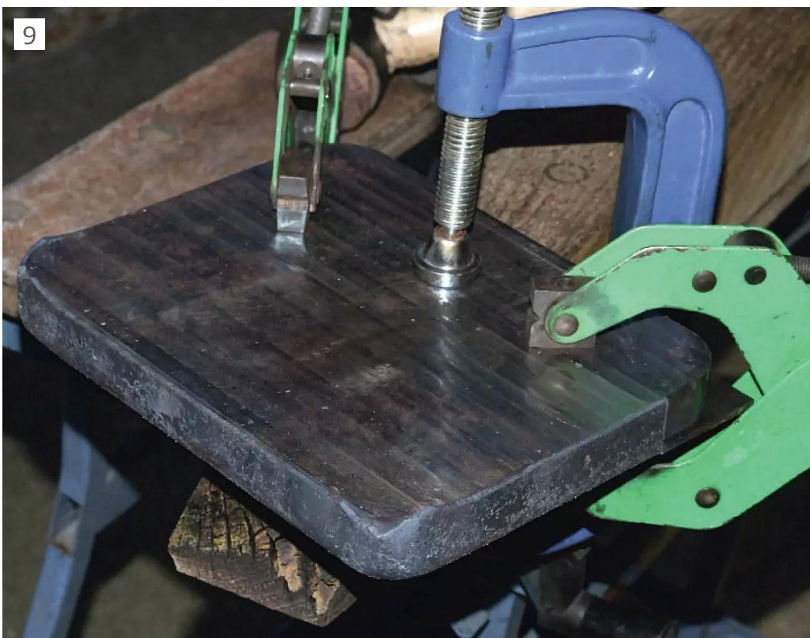
Underside of Spectacle Plate After Flanging
