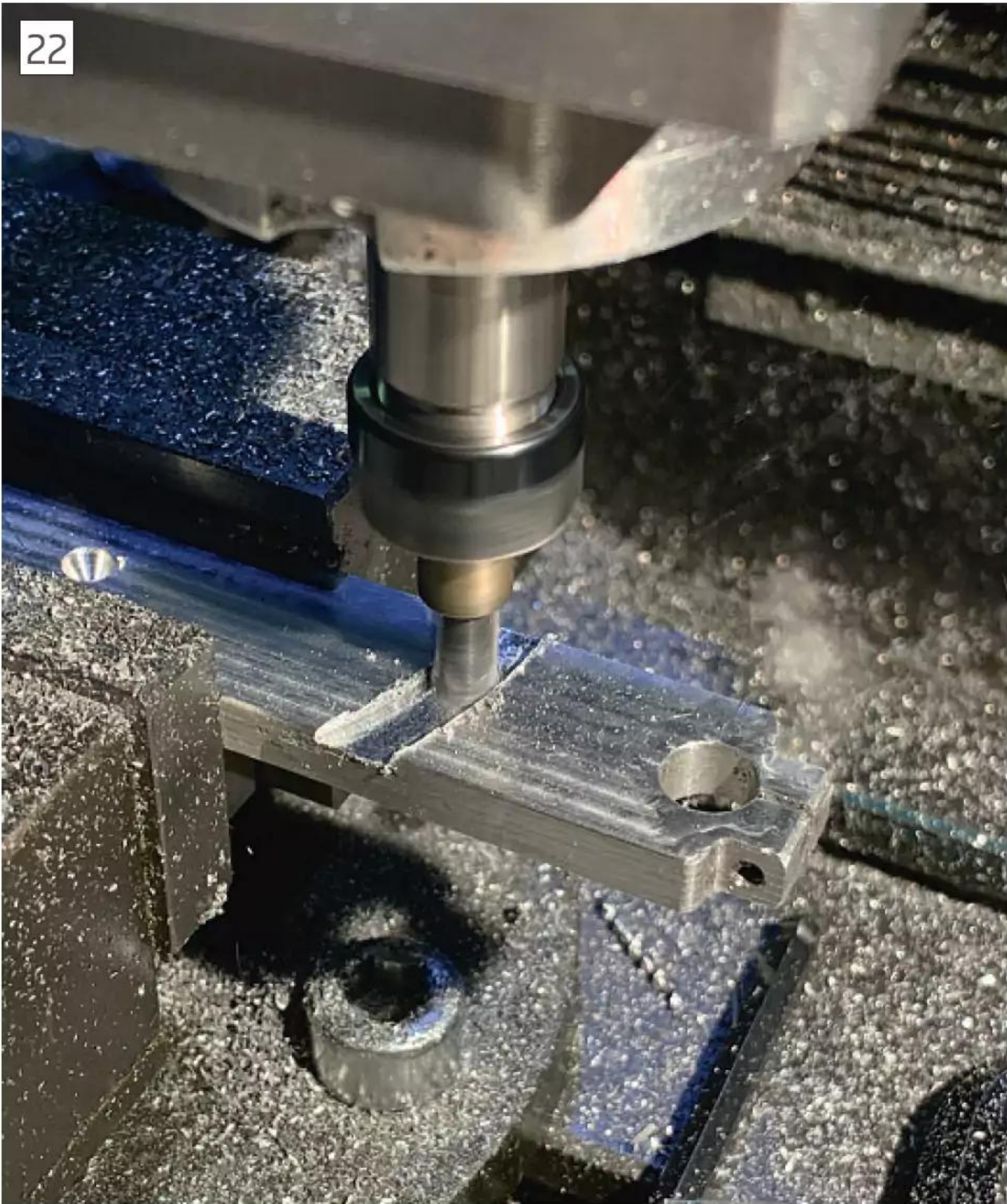
Re-purposing the original vertical support for the locking cam.
