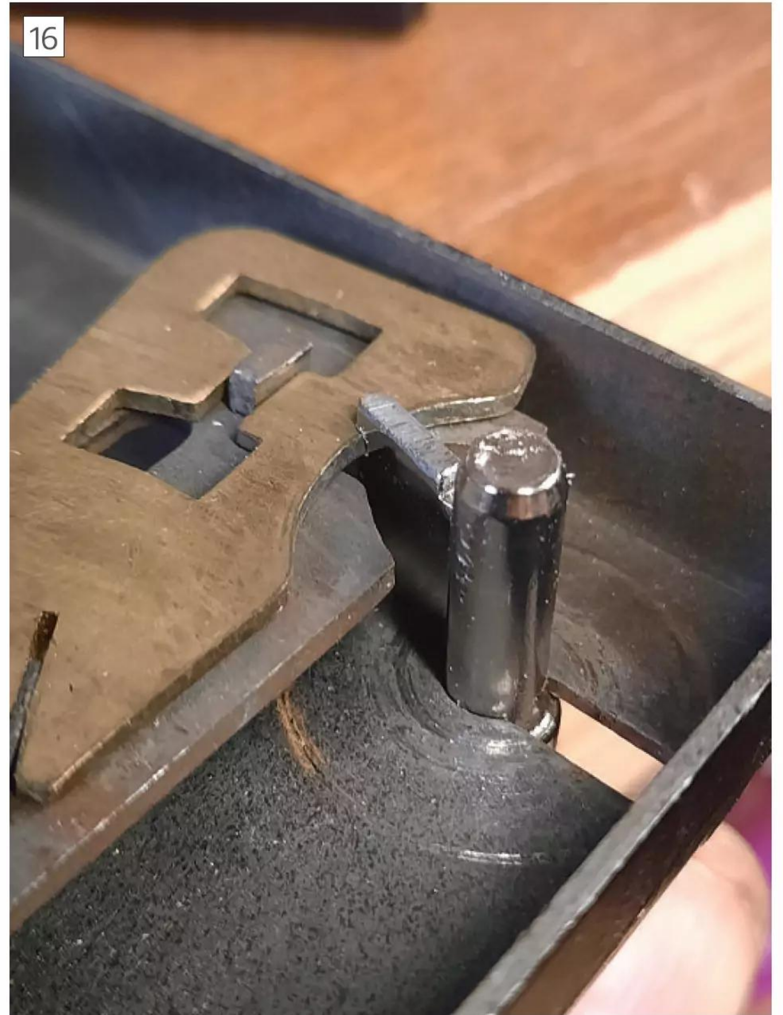
The first tooth is cut and the key now raises this lever so the stump can pass through the gating.
