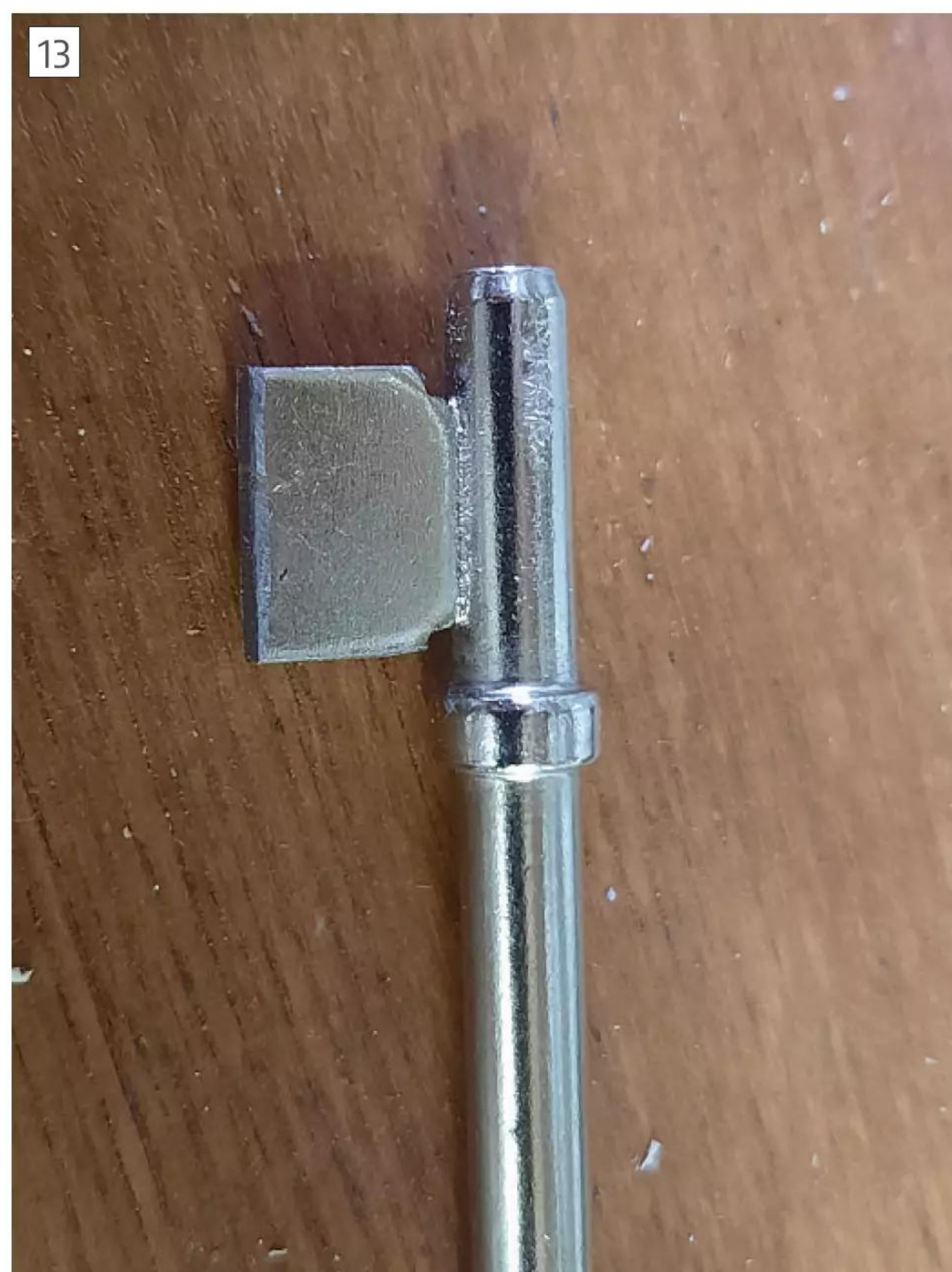
The blank now fits the lock, but is not yet fitted to the levers.
