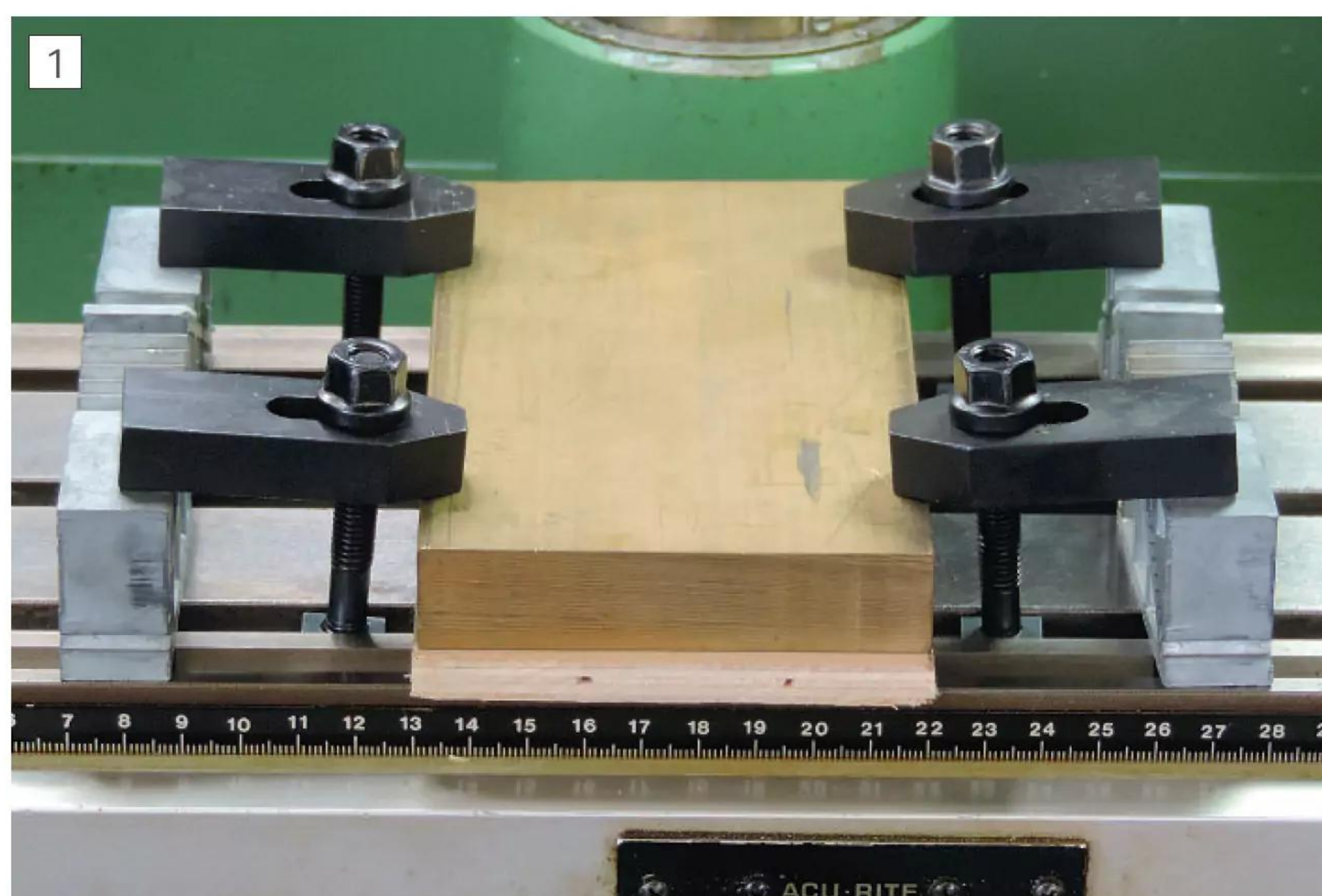
Workpiece clamping on the milling machine using the usual size of tee nuts in the table tee slots.
