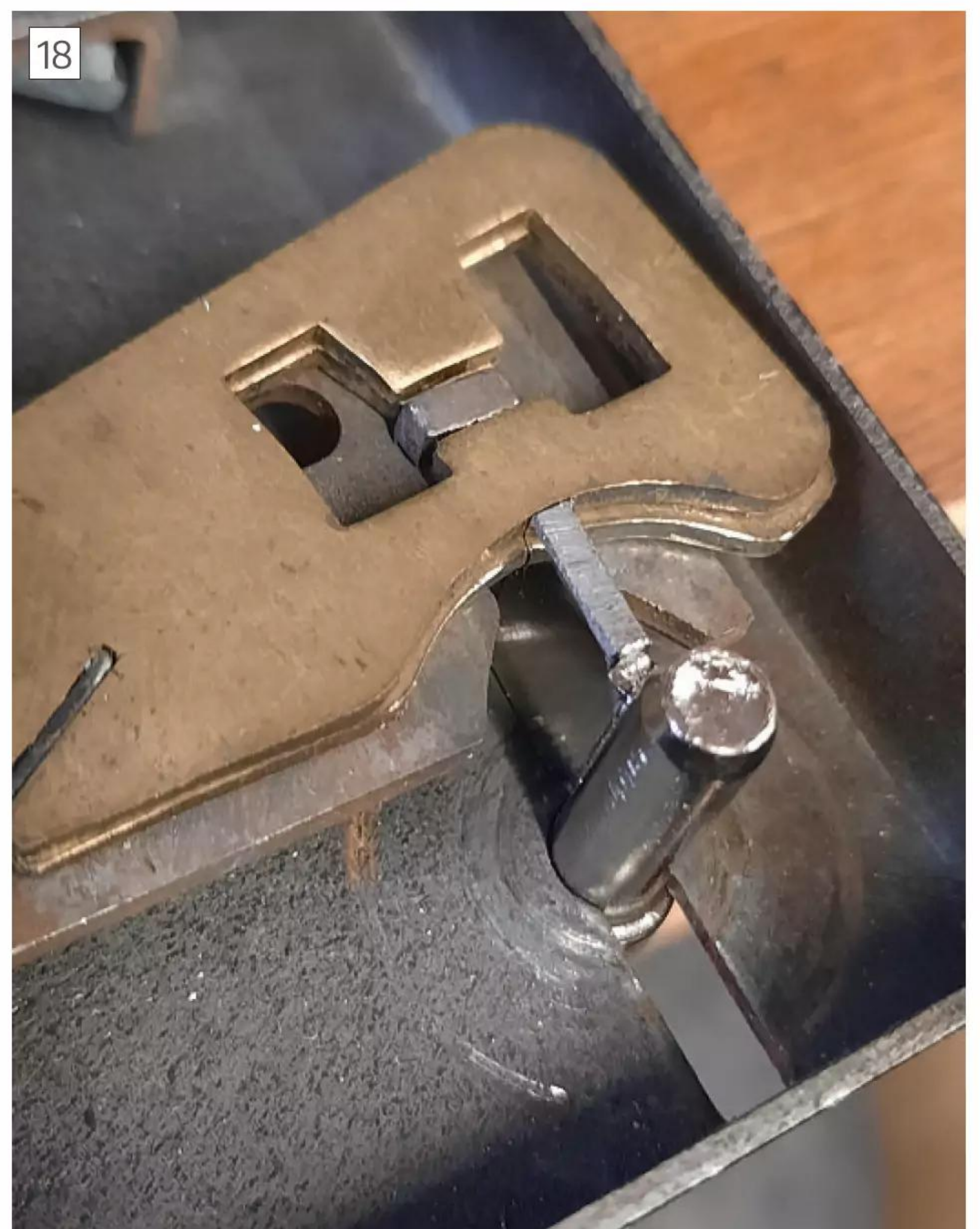
With the second tooth cut, the key can now operate both levers. >
