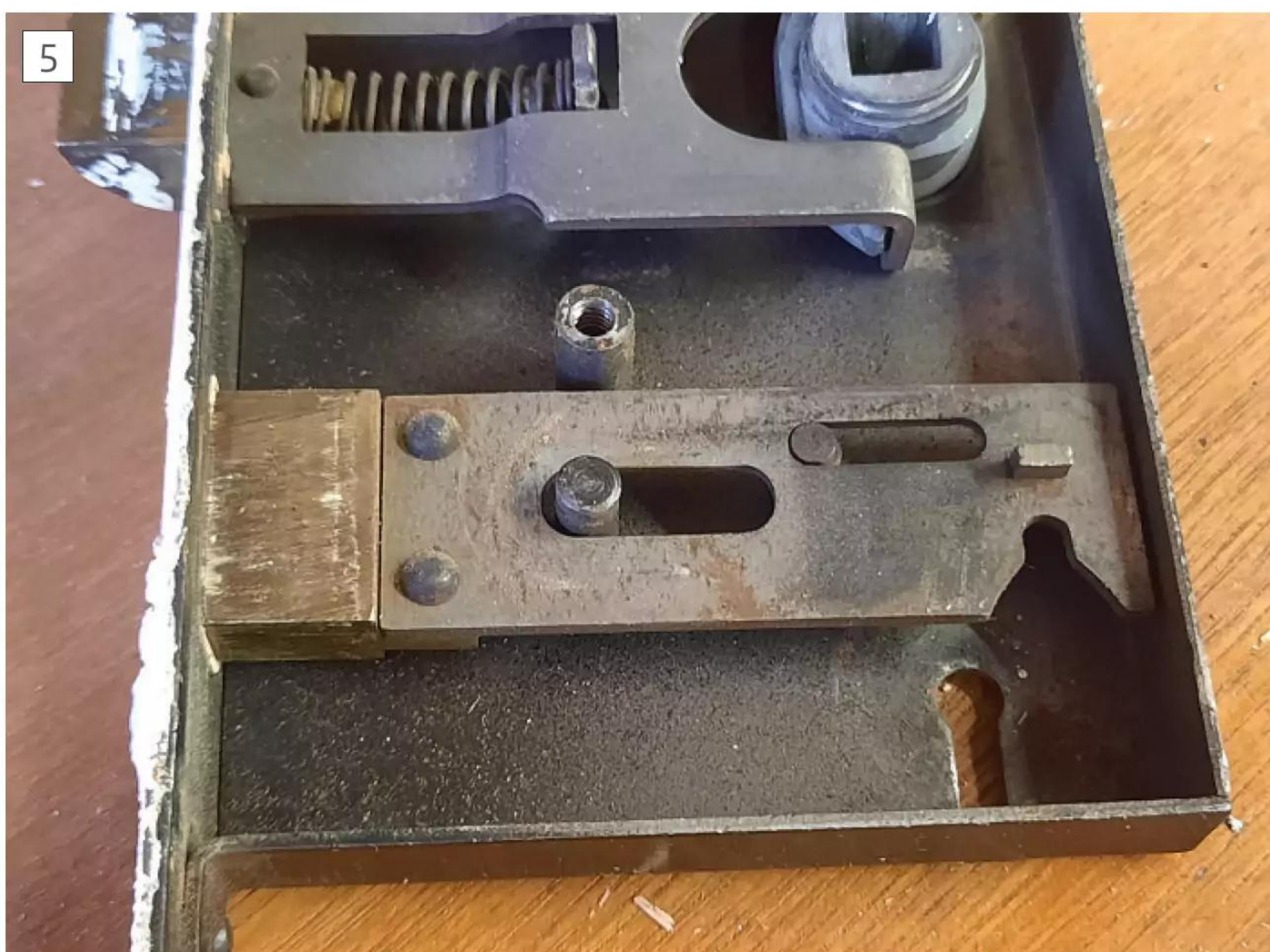
The final lever is the bolt lath, note the bolt stump and 'talon' beneath it.
