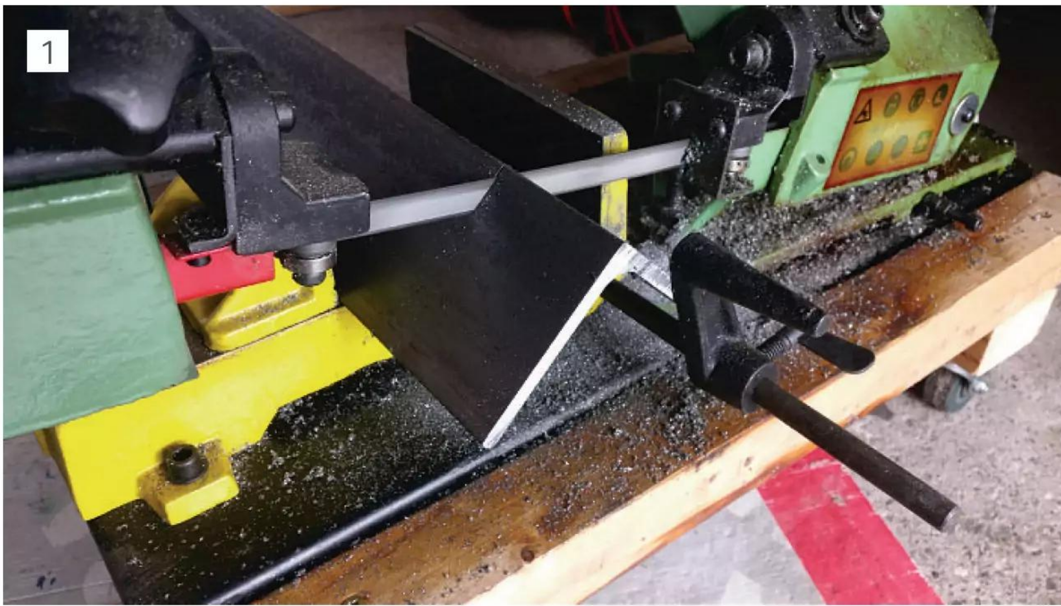
Cutting the angle iron in the bandsaw.
