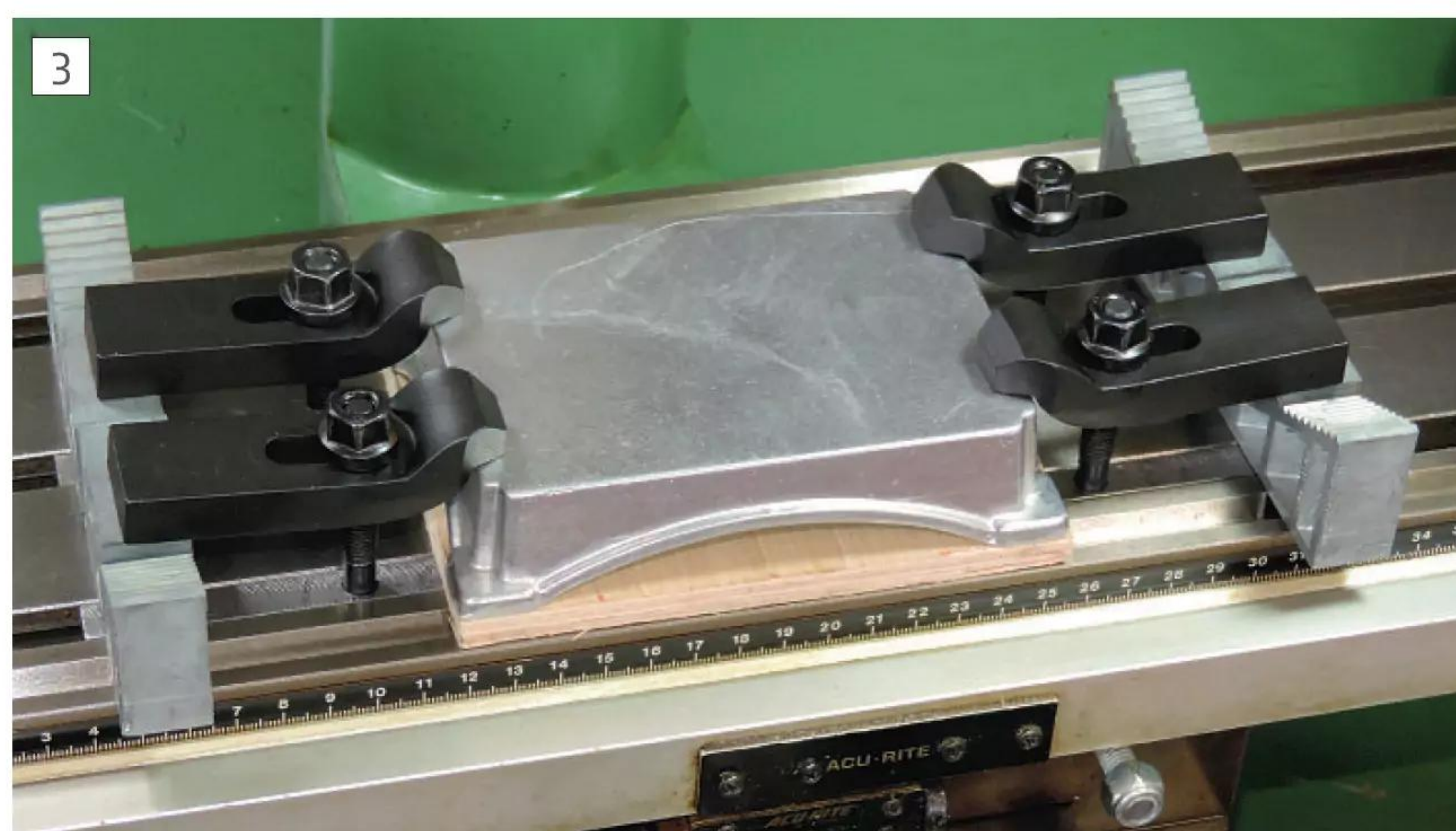
Clamping using the longer length tee nuts with cranked clamping bars.
