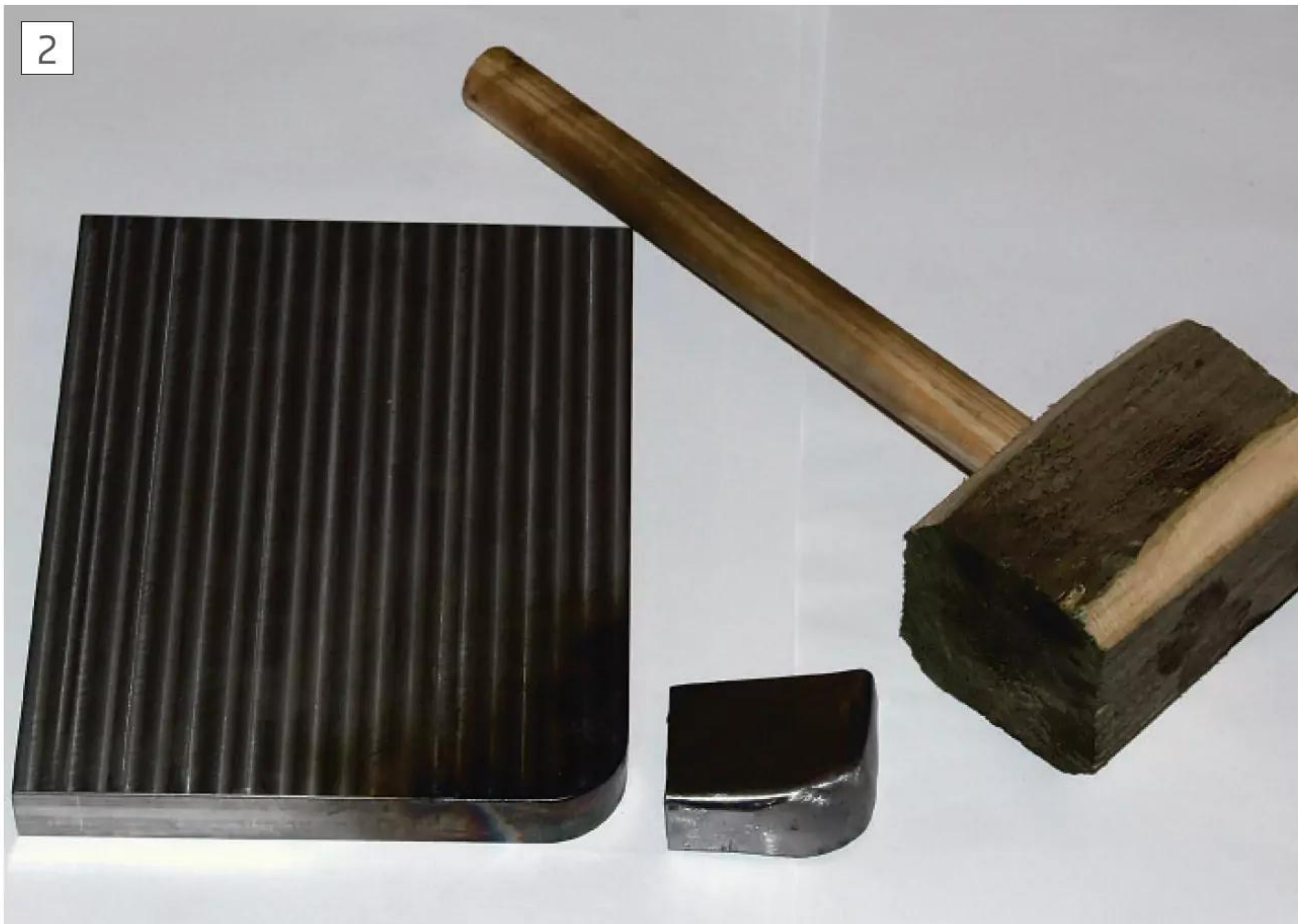
Partial Former and Trial Corner Bend
