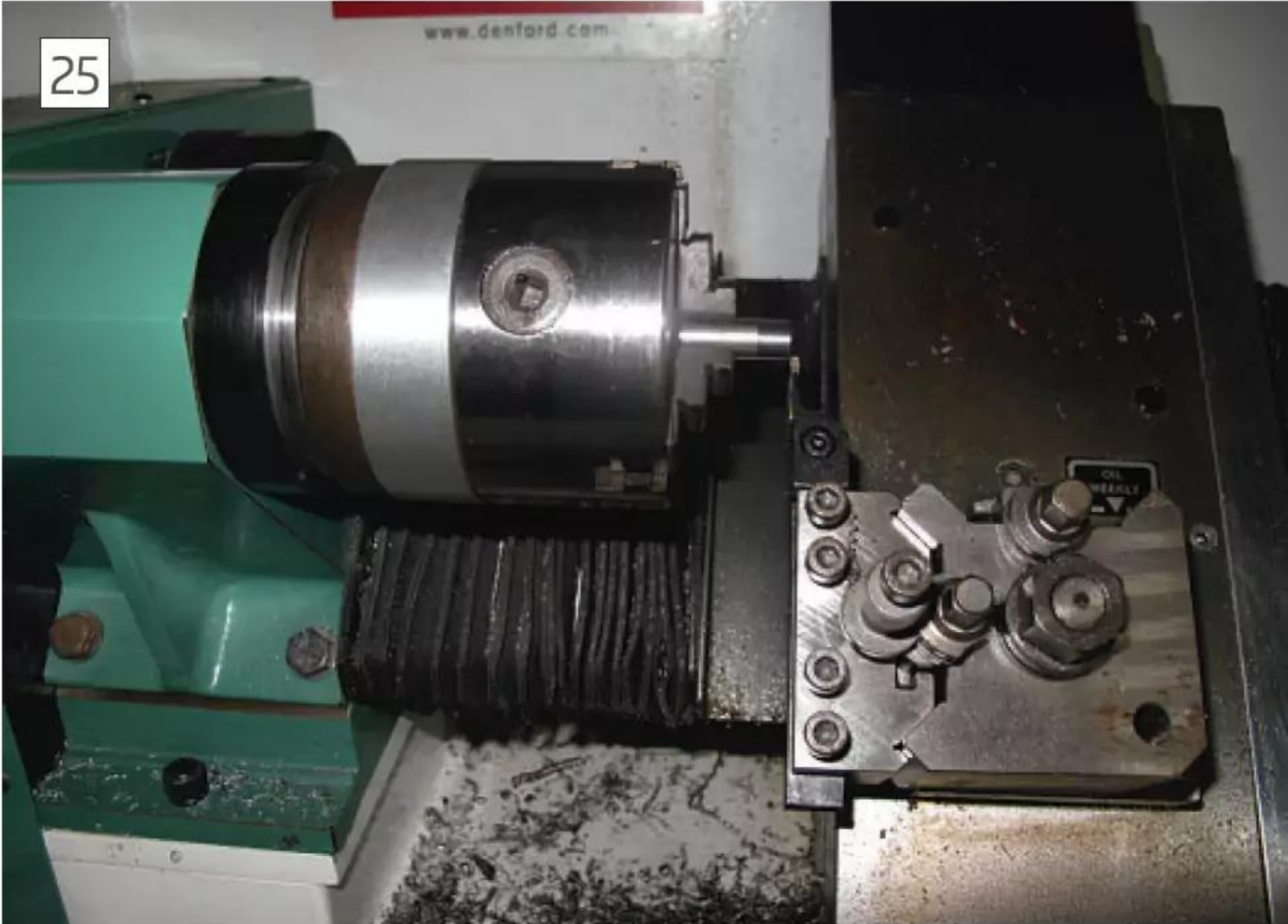
Establishing the Z zero offset for T07
