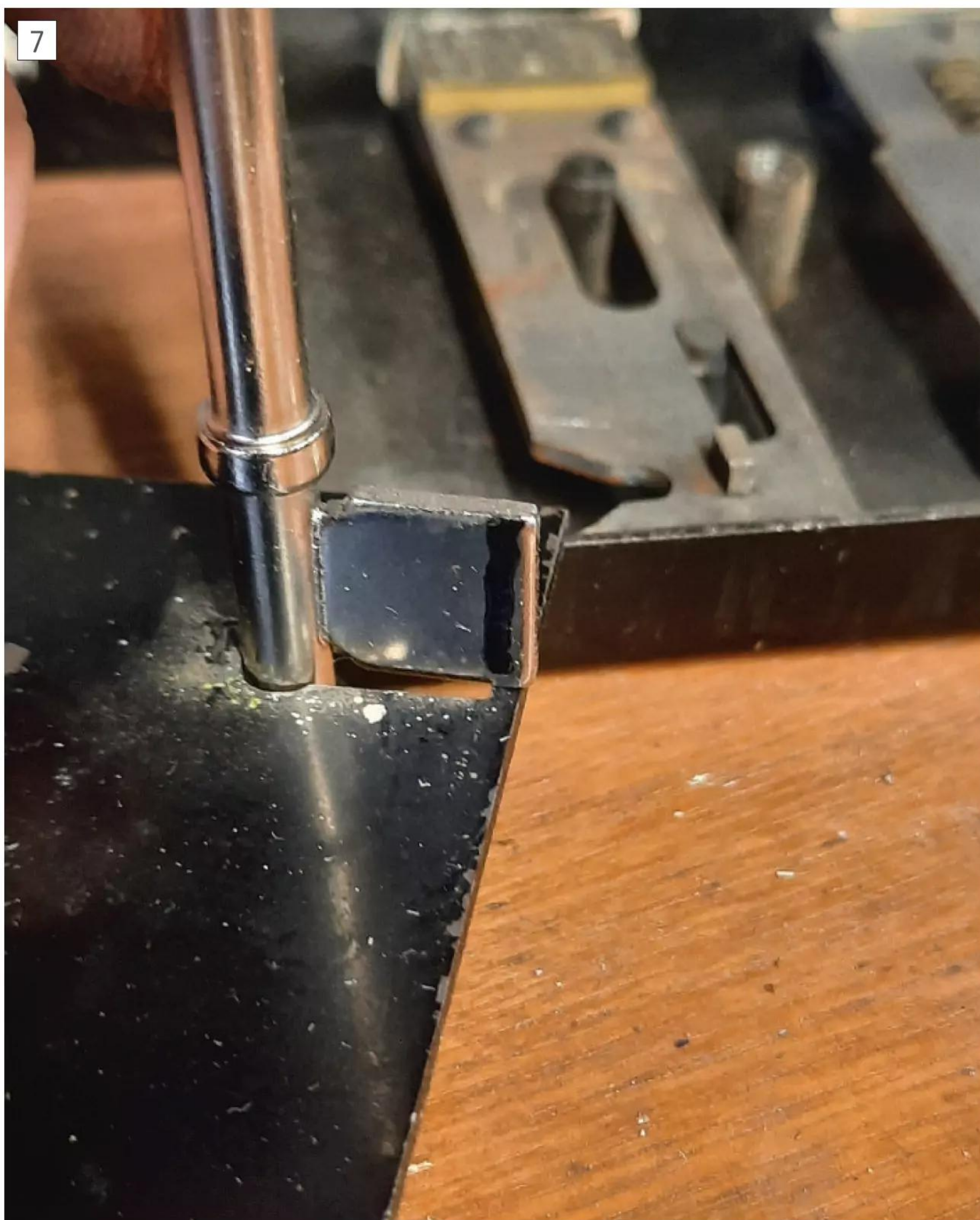
The bit of the blank was noticeably oversize.
