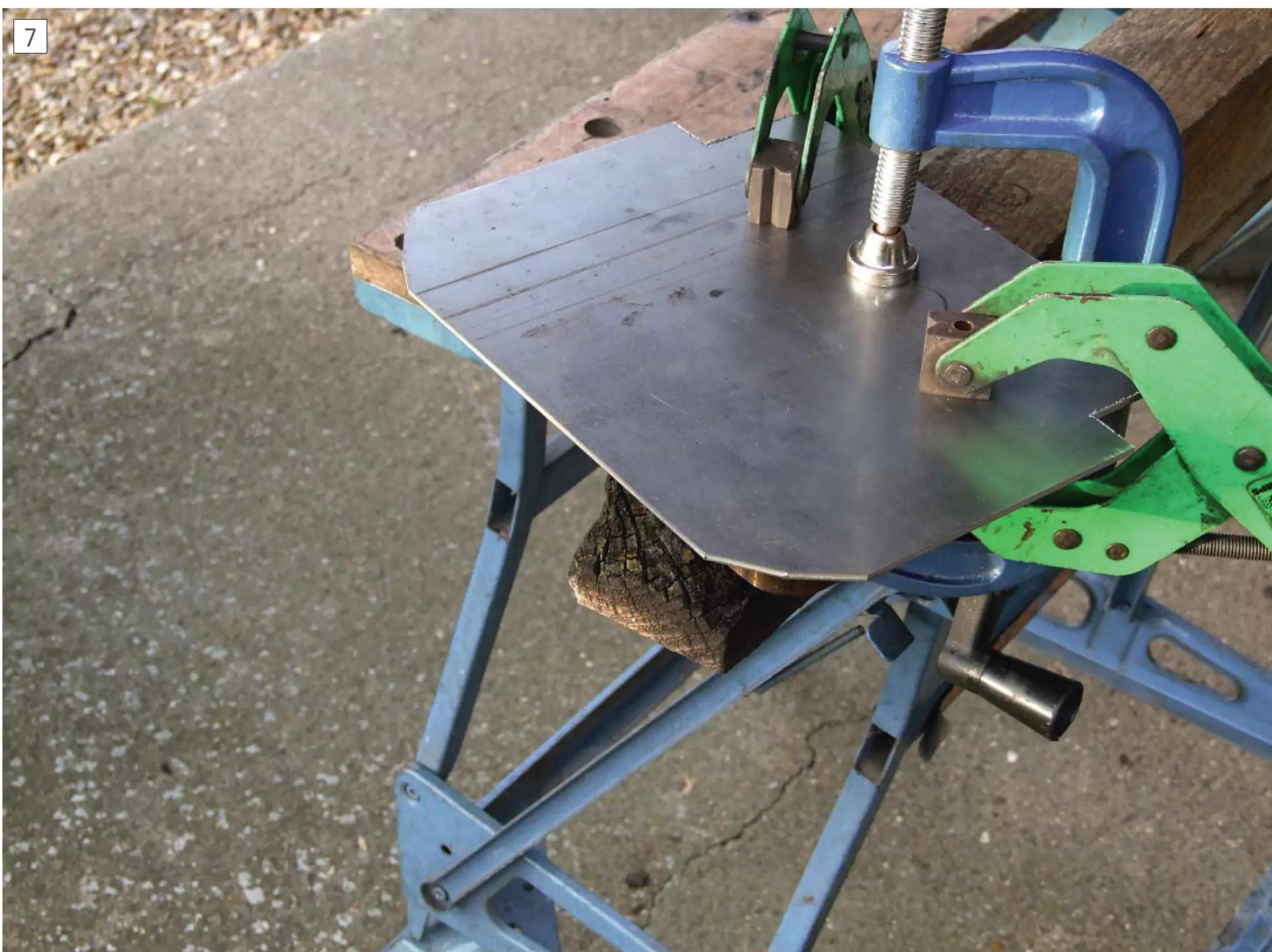
Close Up of the Plate Prior to Flanging
