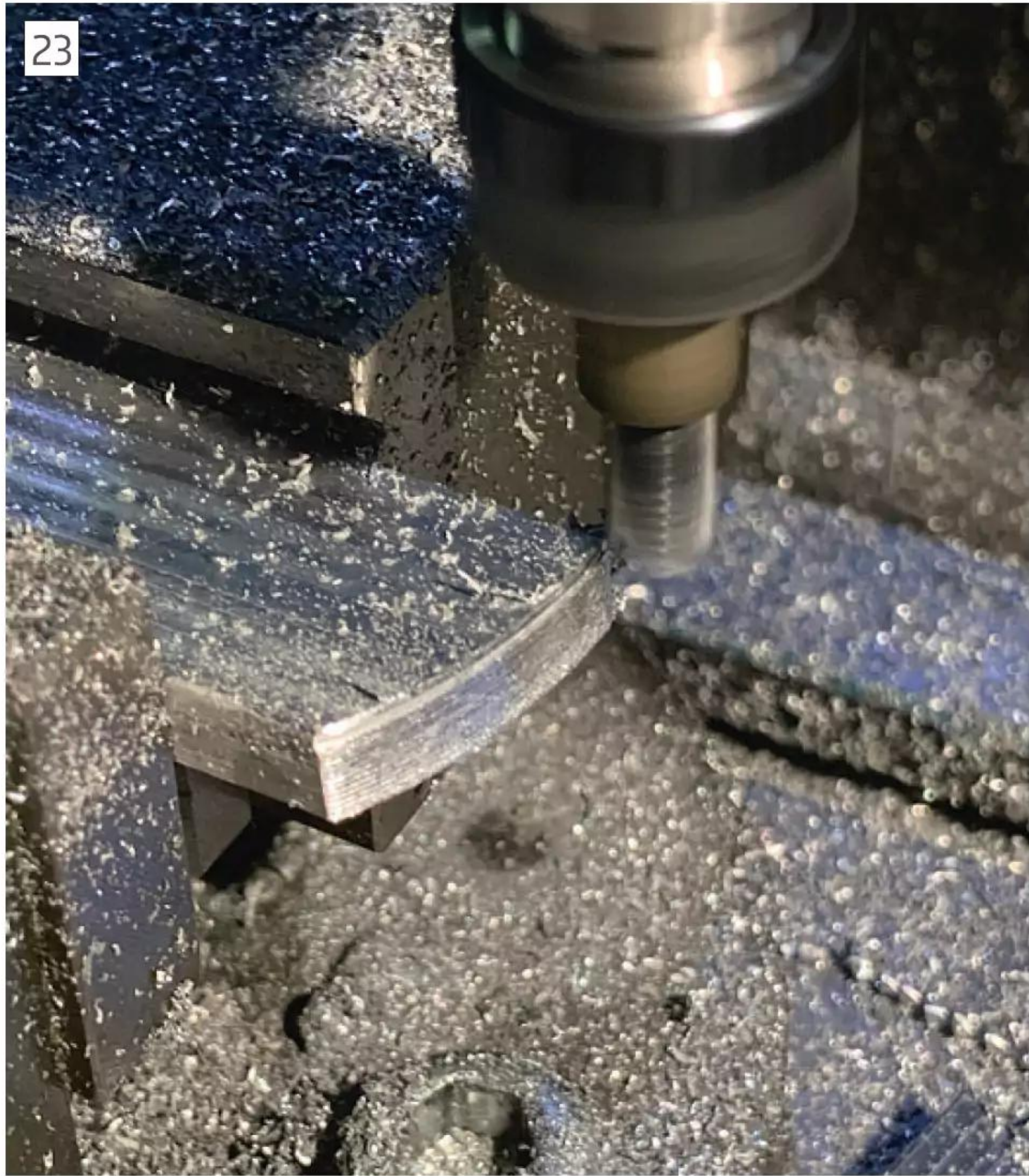
Finish machining the cam under CNC. A radius table could perform the same task.
