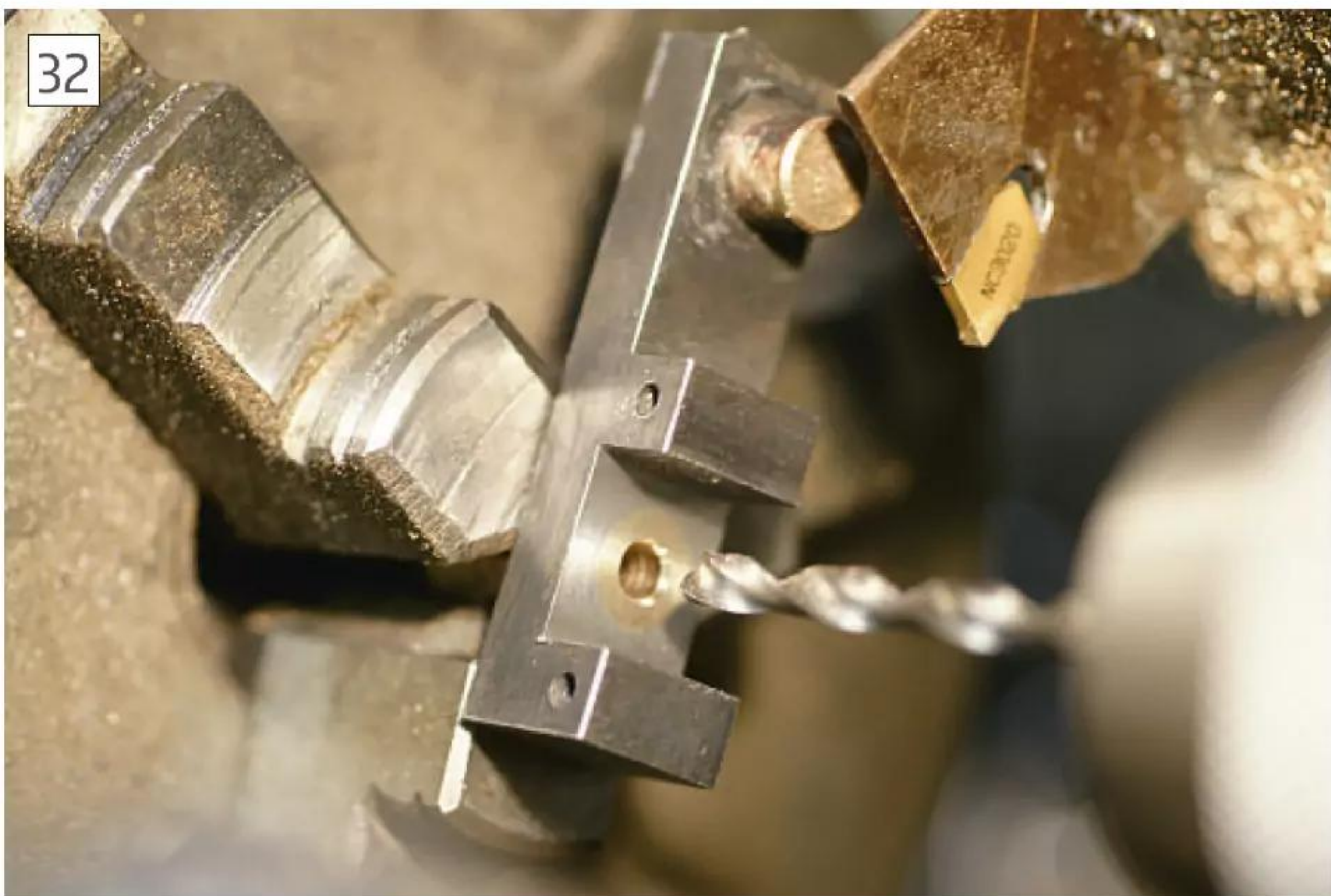
Drilling for the beam breaking rod. The parting off tool is photo-bombing and plays no part in the machining.
