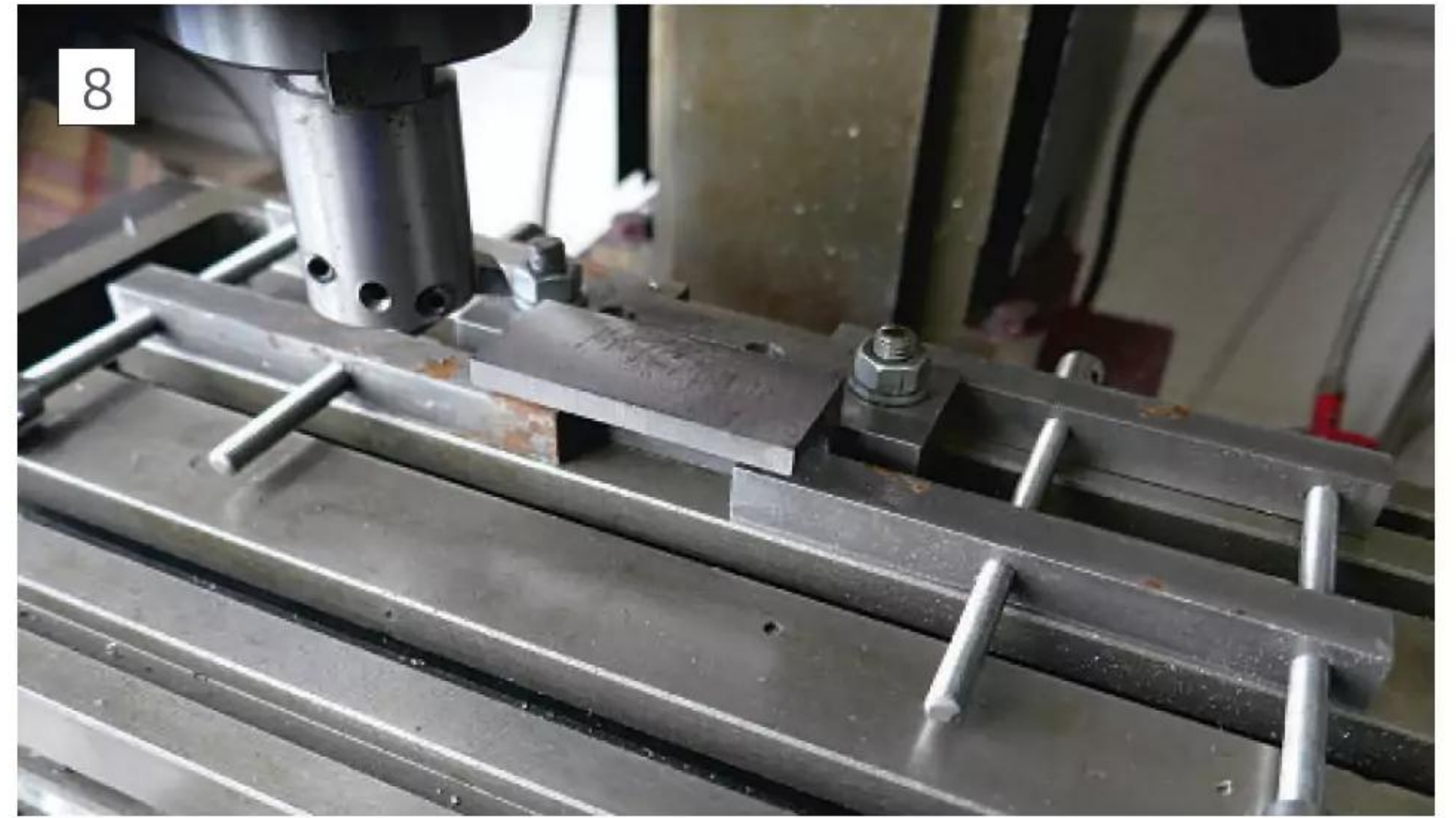
Squaring up the hinges using a flycutter in the mill. The work is held against a squared block with two engineer's clamps.
