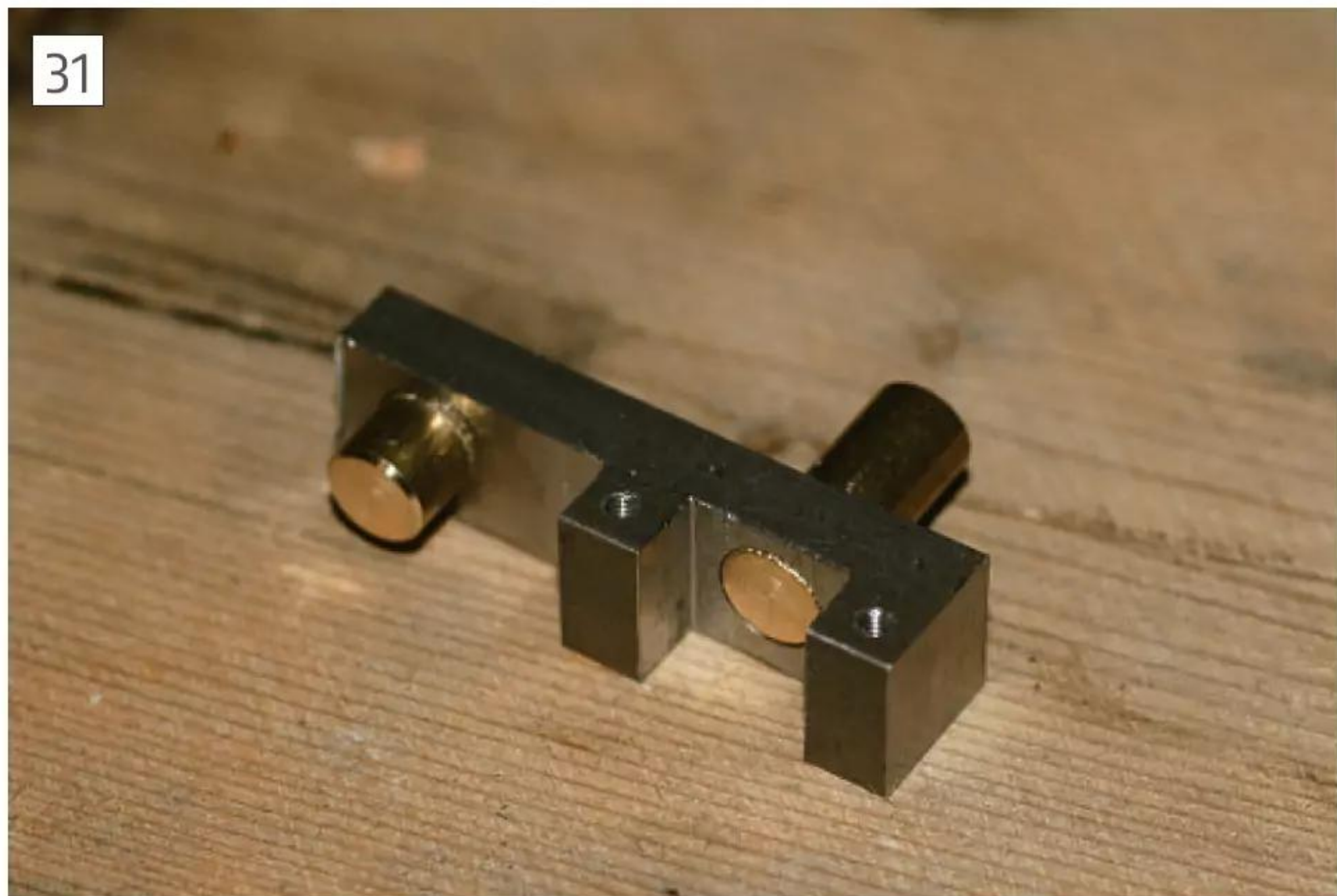
Ready for silver soldering. The rod shaft bar was a bit undersized so I knurled it for a fit prior to silver soldering.
