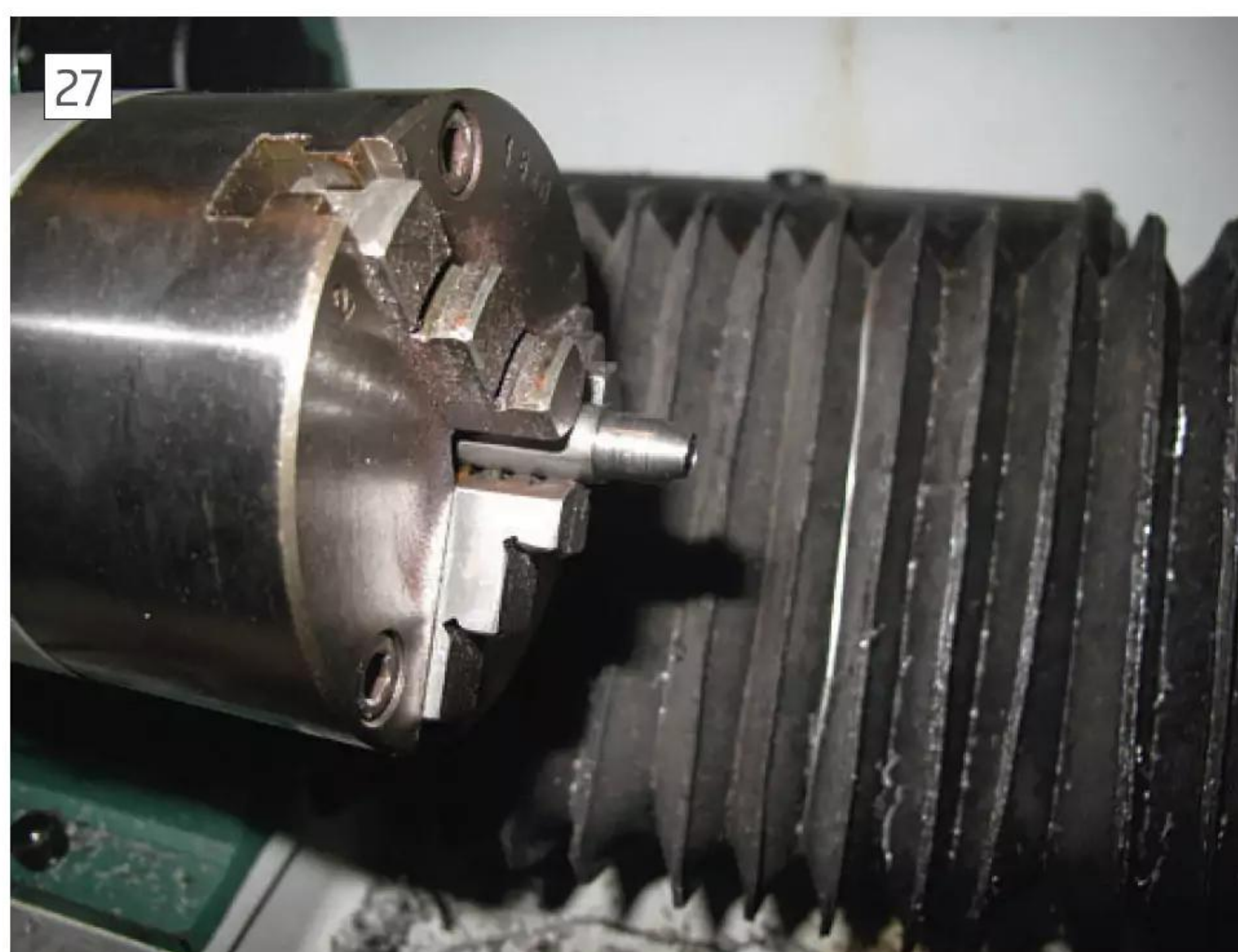
The component prior to parting.
