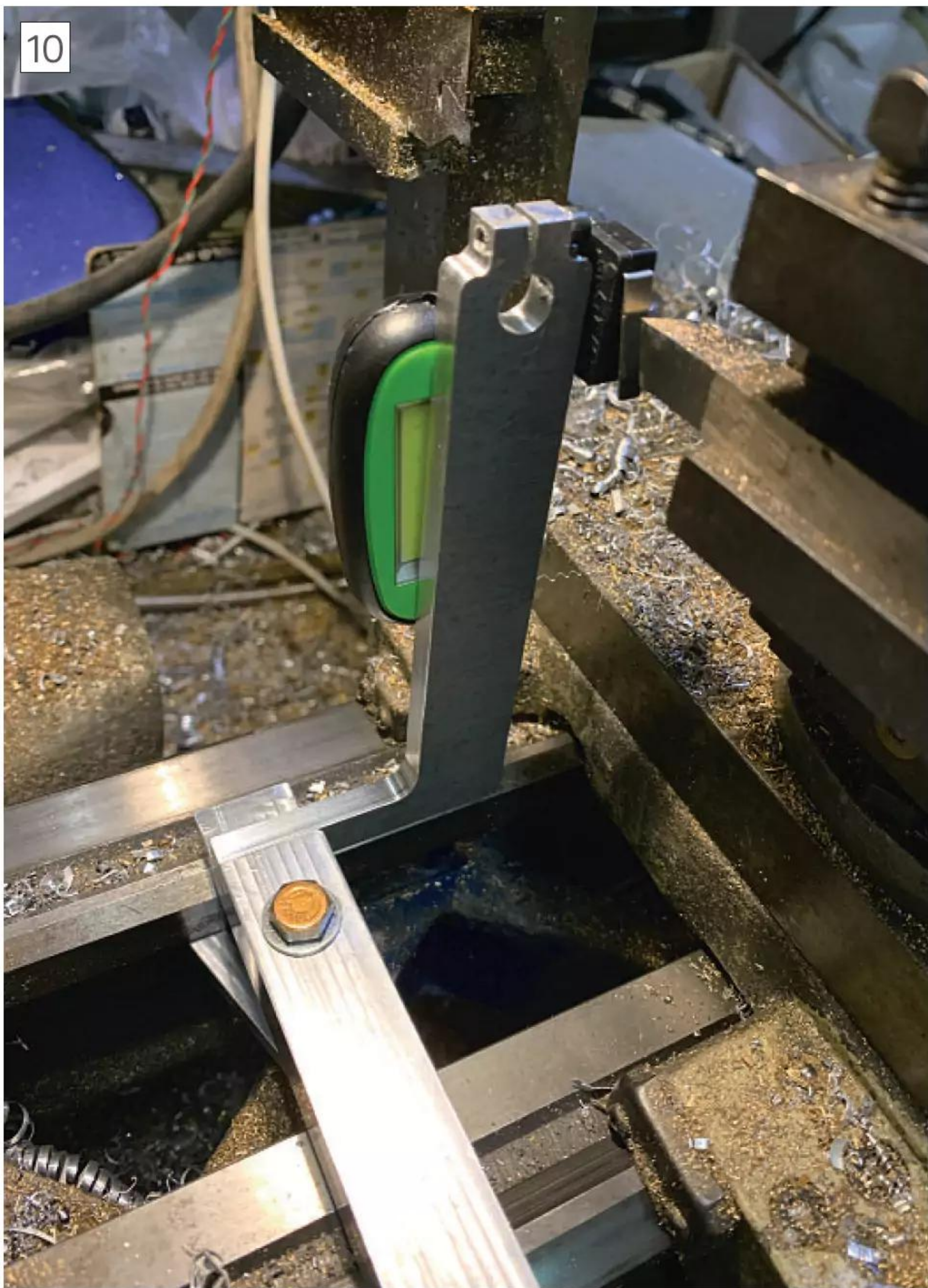
Version 1 with microswitch installed. The apparently problematic lever on the microswitch is clearly visible.
