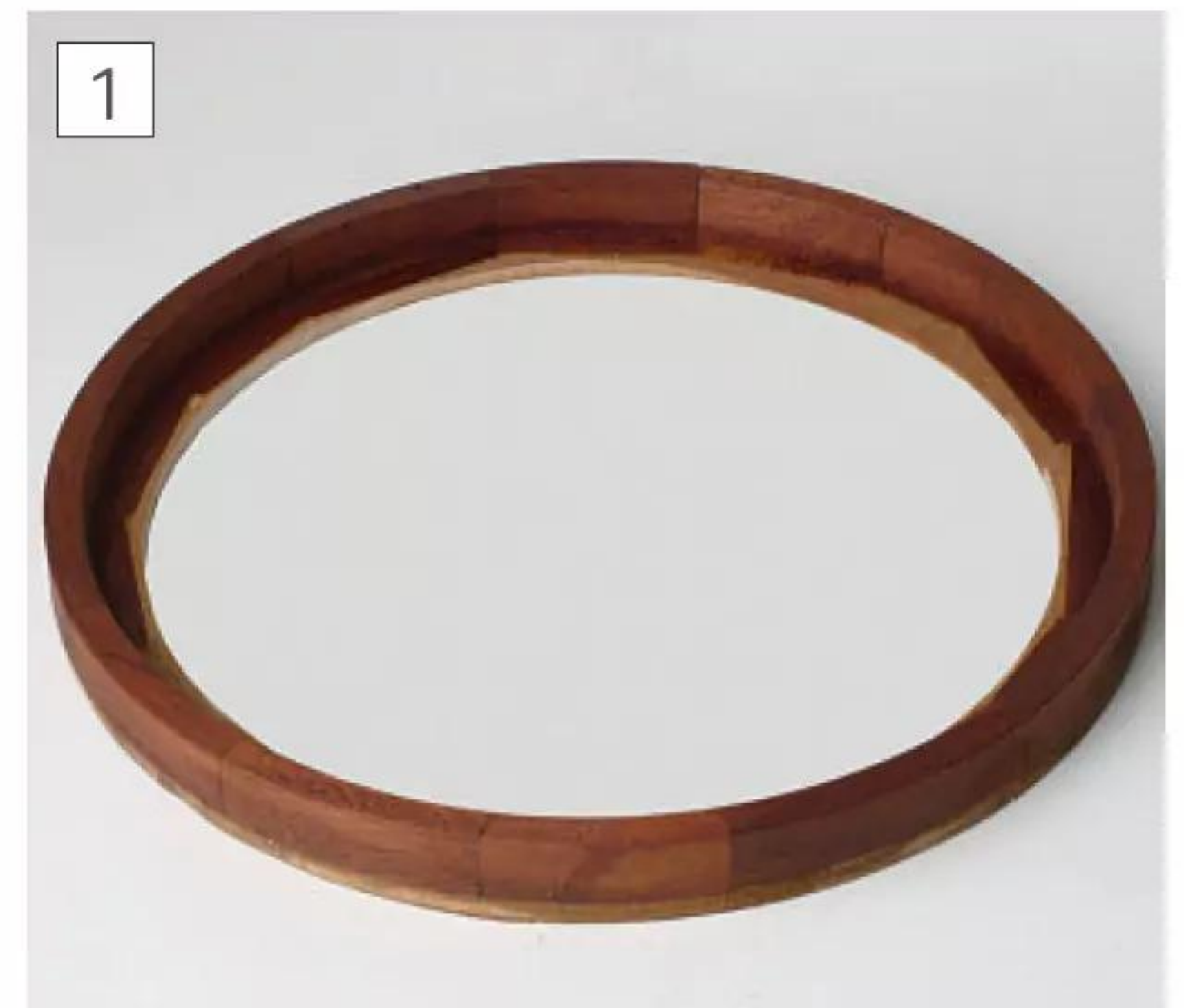
The wooden pattern of the bezel with a waste "lip" sent to the casters for the brass castings (Photograph by Jake Sutton)
