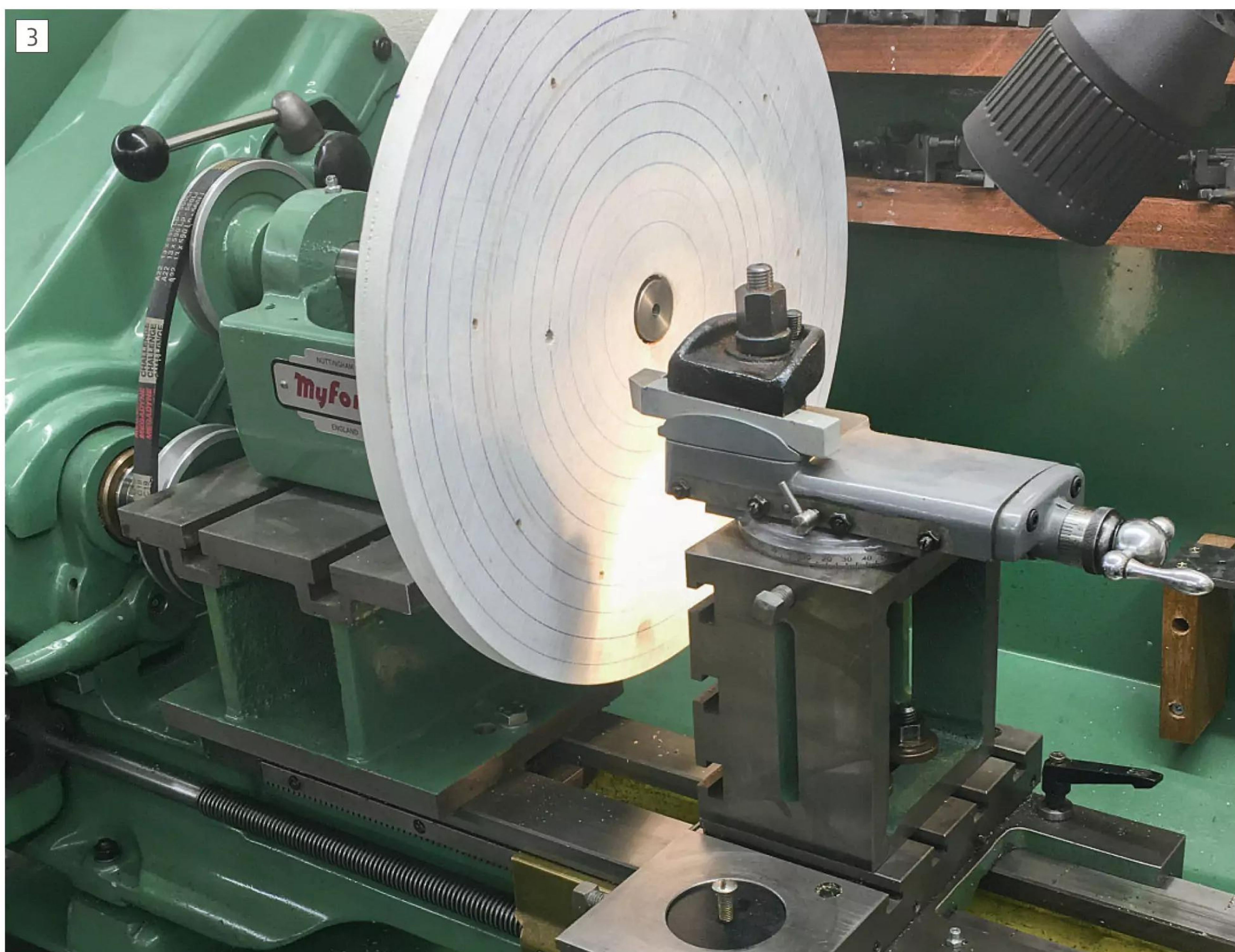
The cross slide and tool holder correspondingly raised on a block (Photograph by Jake Sutton)
