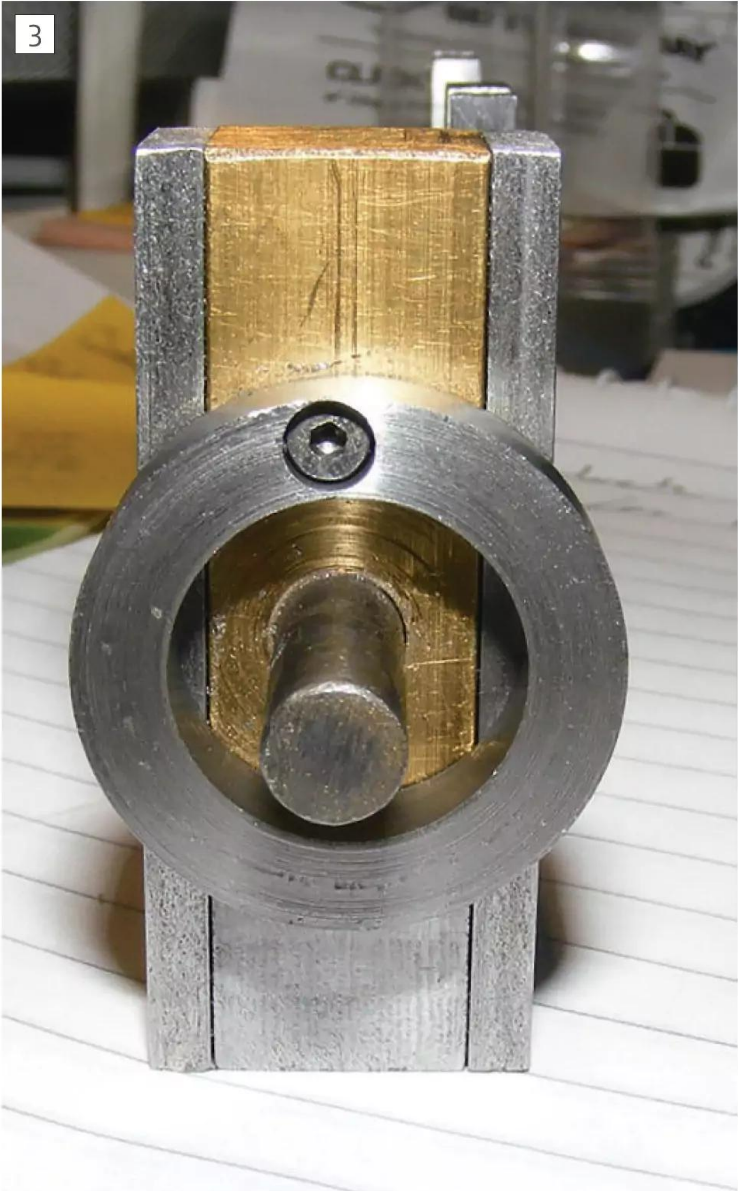
Showing collar attached to the front bearing block.
