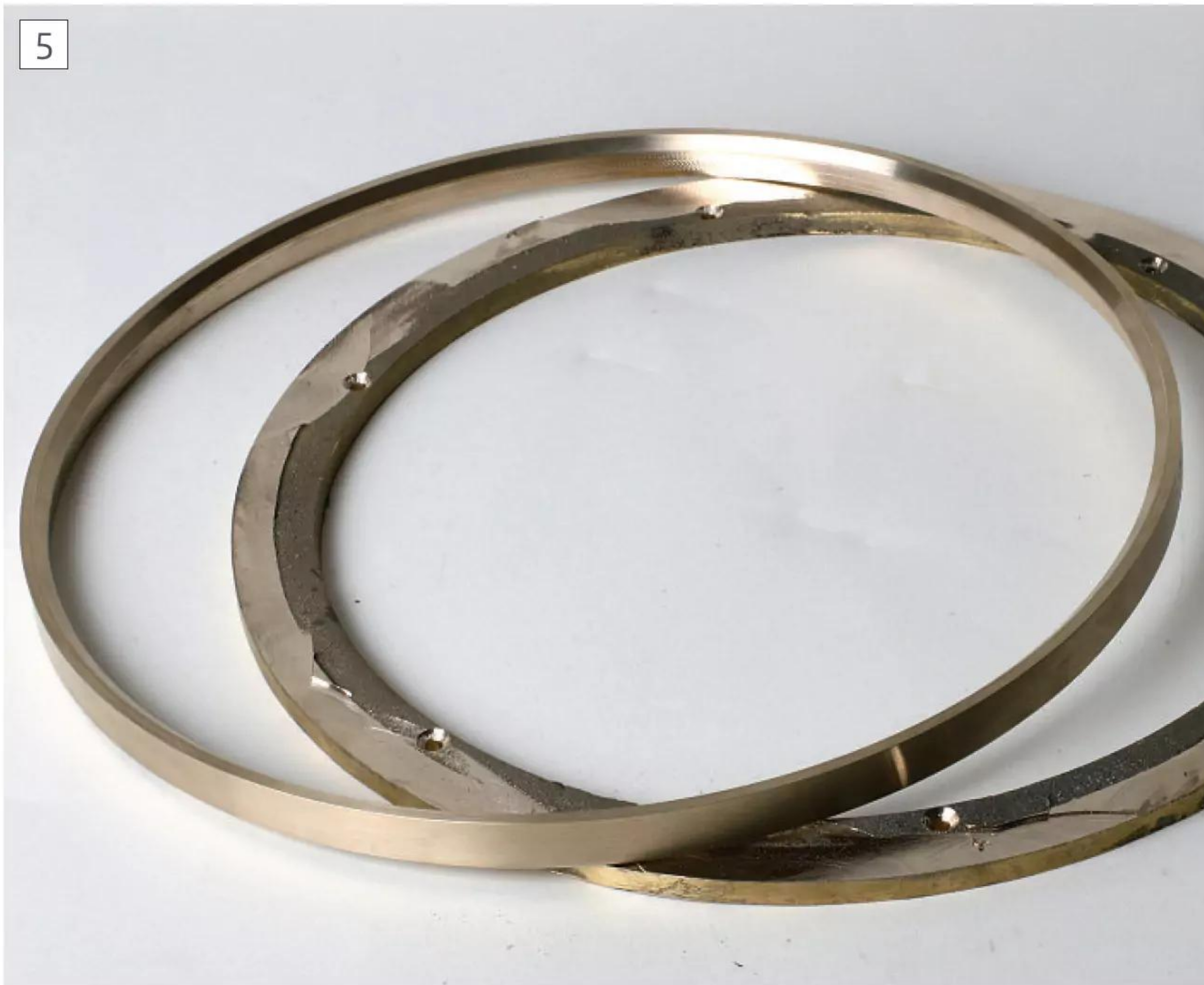
The completed bezel and waste "lip" after parting off in the lathe (Photograph by Jake Sutton)
