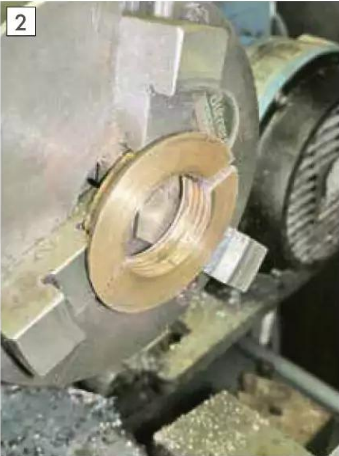
A temporary collet from a plumbing fitting.
