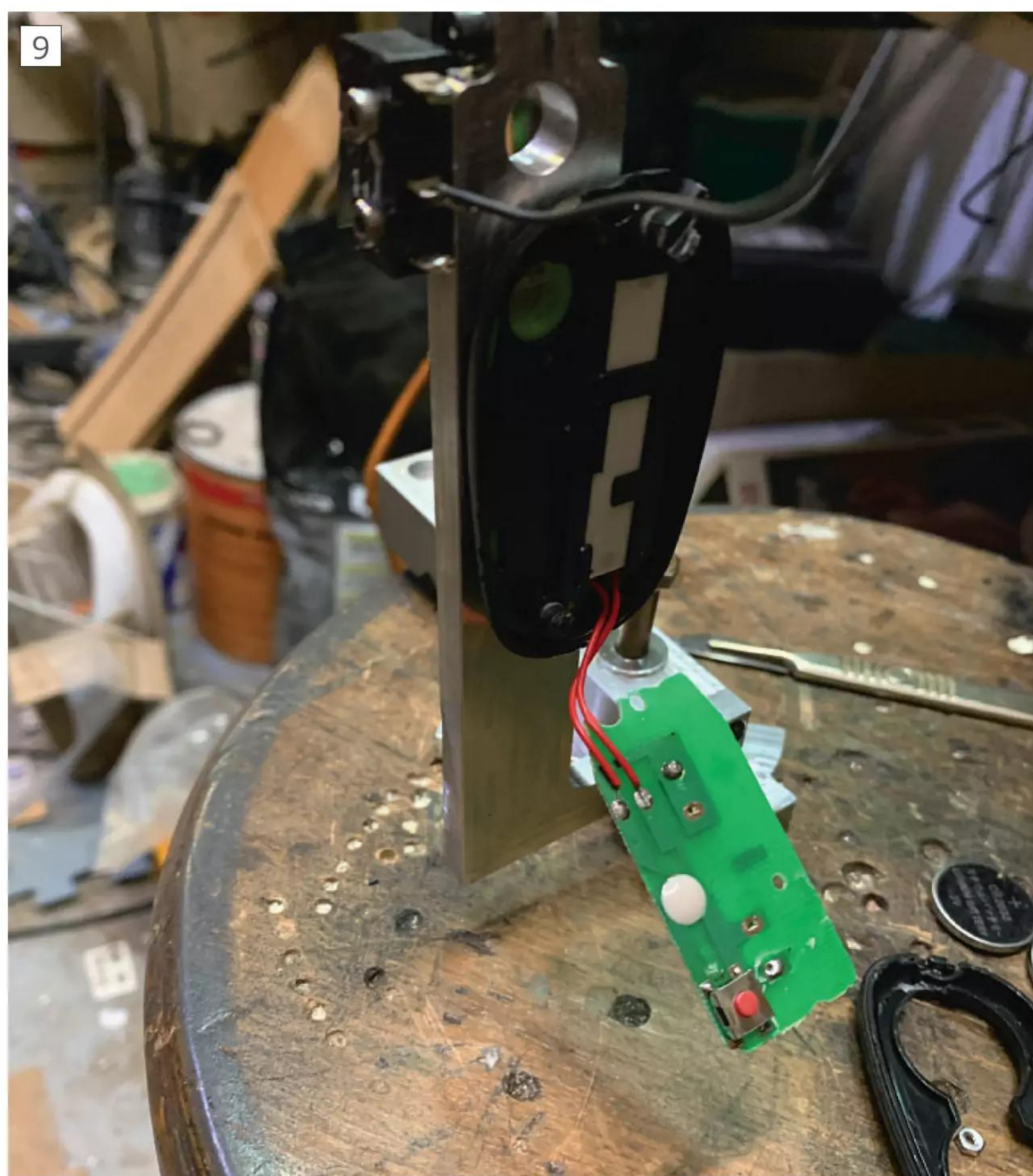
Replacing the DTI with a LED torch. Frustratingly, the torch didn't simply come on with a button press so a brutal piece of re-wiring was required. I was probably simpler to wire up a LED, resistor and batter but hindsight is a wonderful thing.
