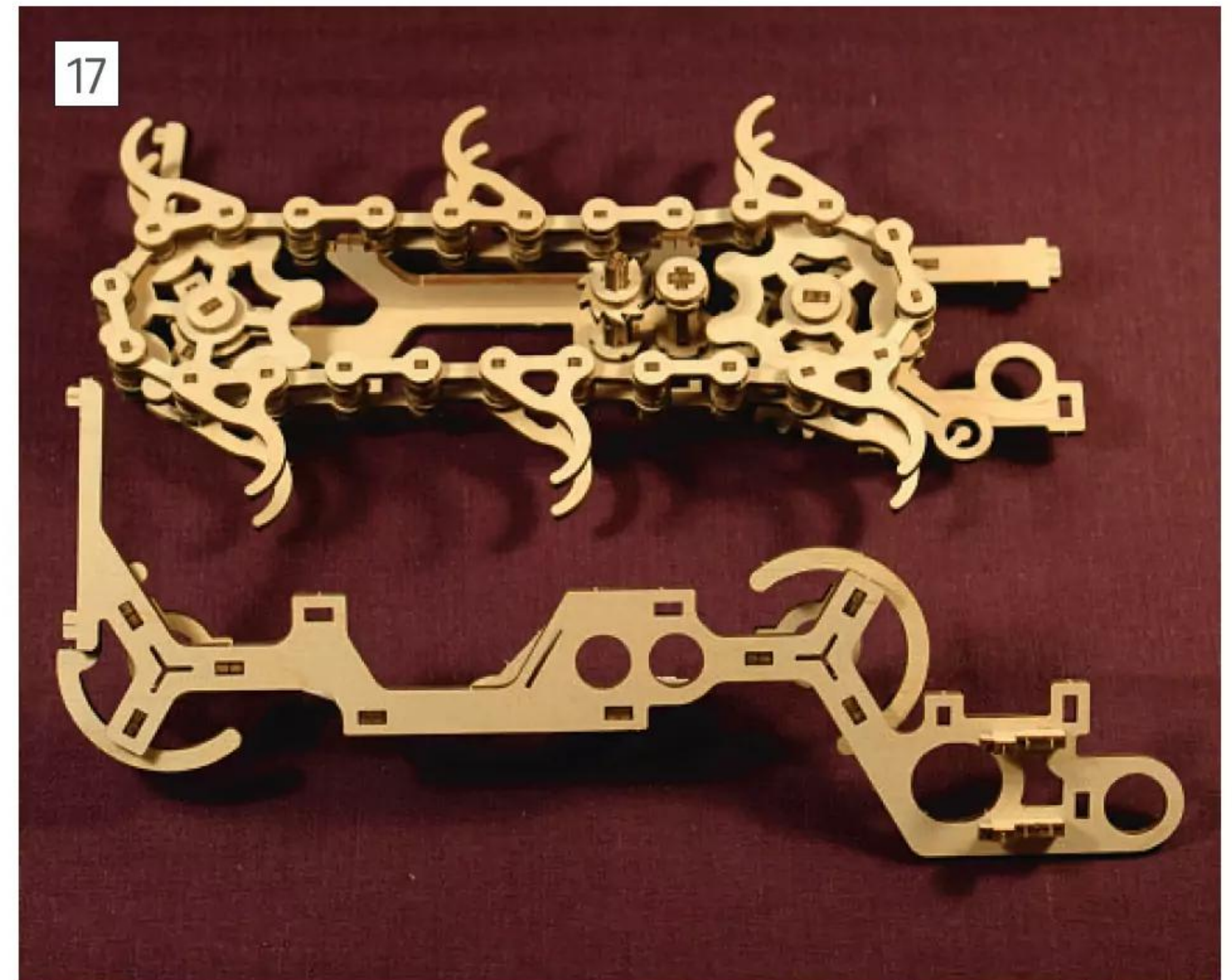
Here the chain has been mounted on the two sprockets awaiting the opposing side to be attached.
