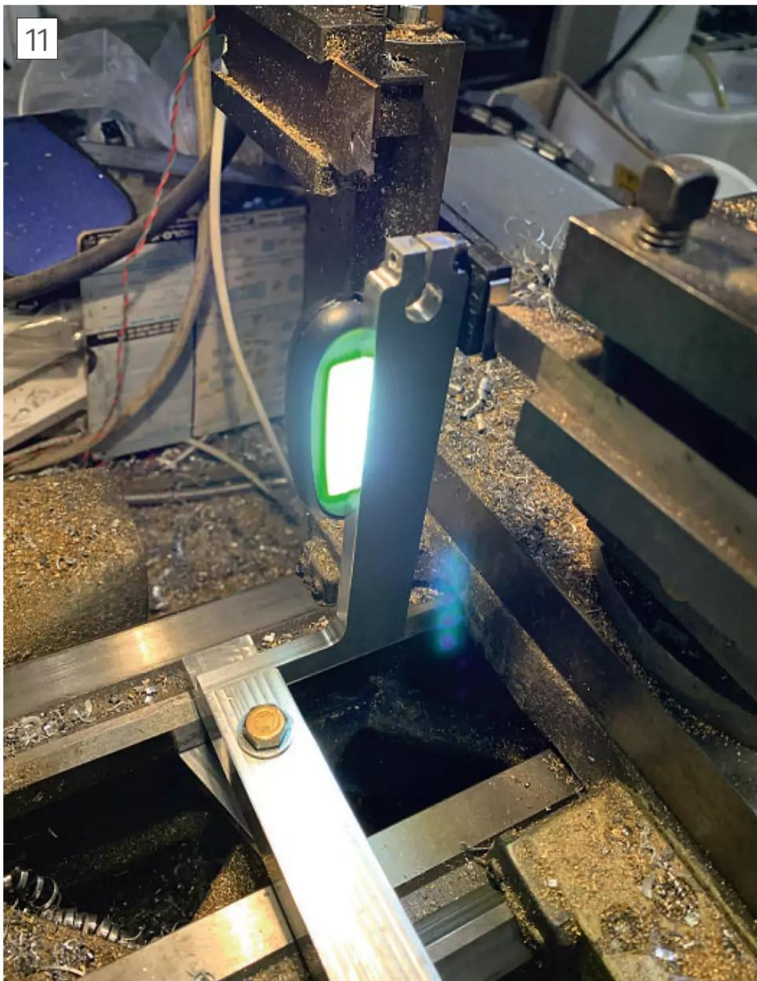
Contact! The torch was glued partially behind the vertical support because the light was rather too bright. If this solution had worked, some significant dimming of the LED would have been required.
