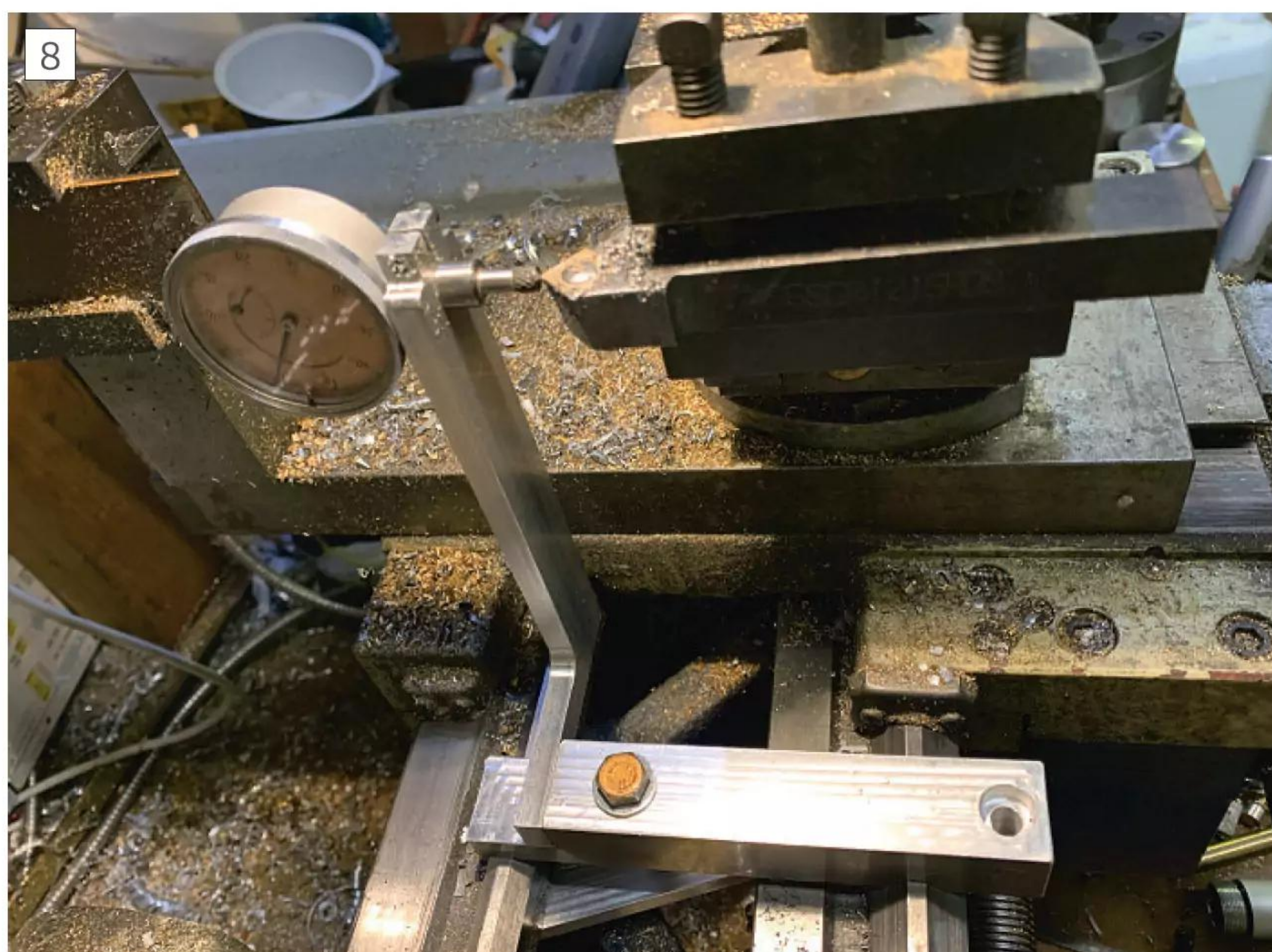
Version 1 from a different angle showing how the tool tip locates on the DTI plunger and that a flat plunger face would be necessary in future if this solution was adopted.
