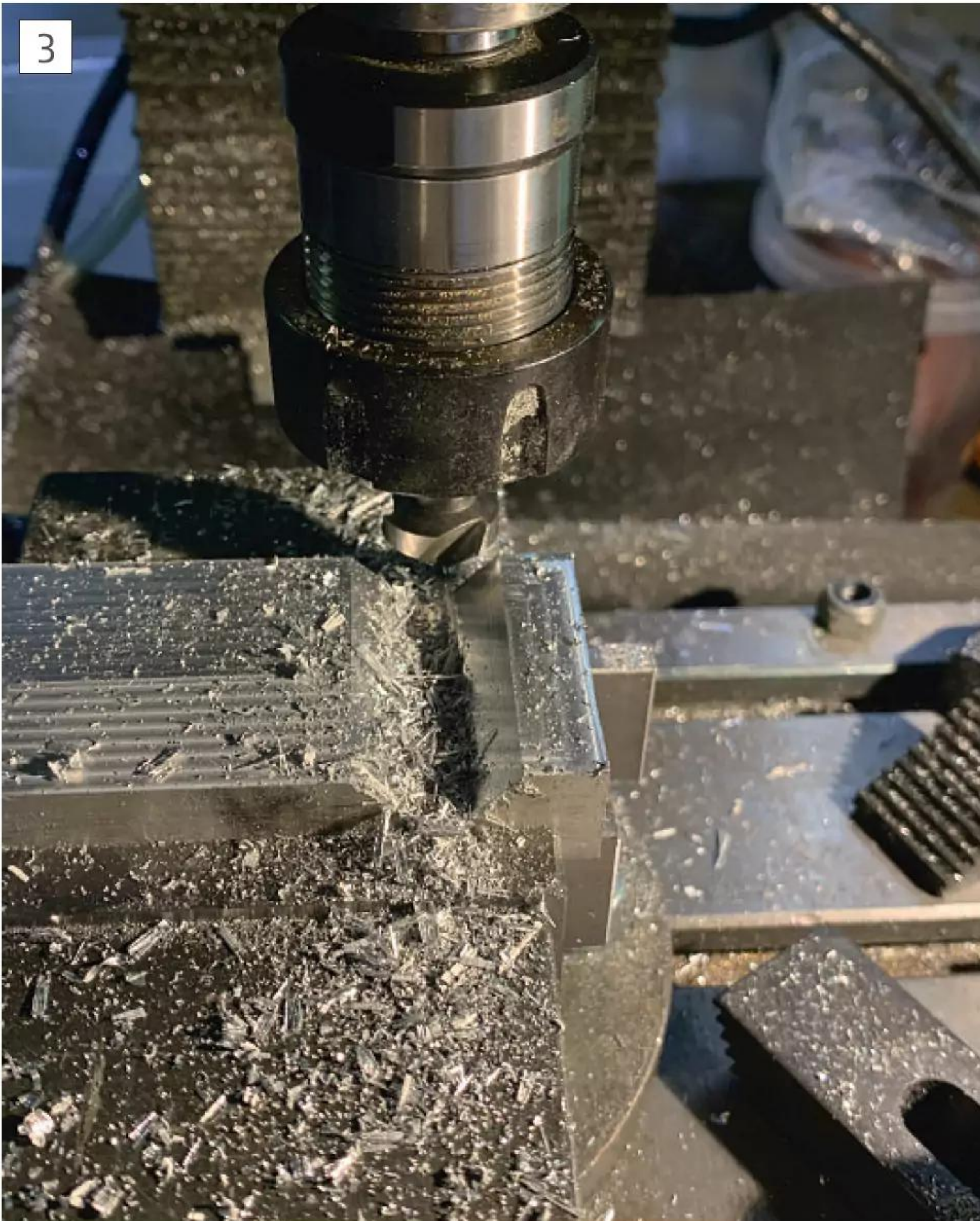
Finishing the V slots with a countersink.
