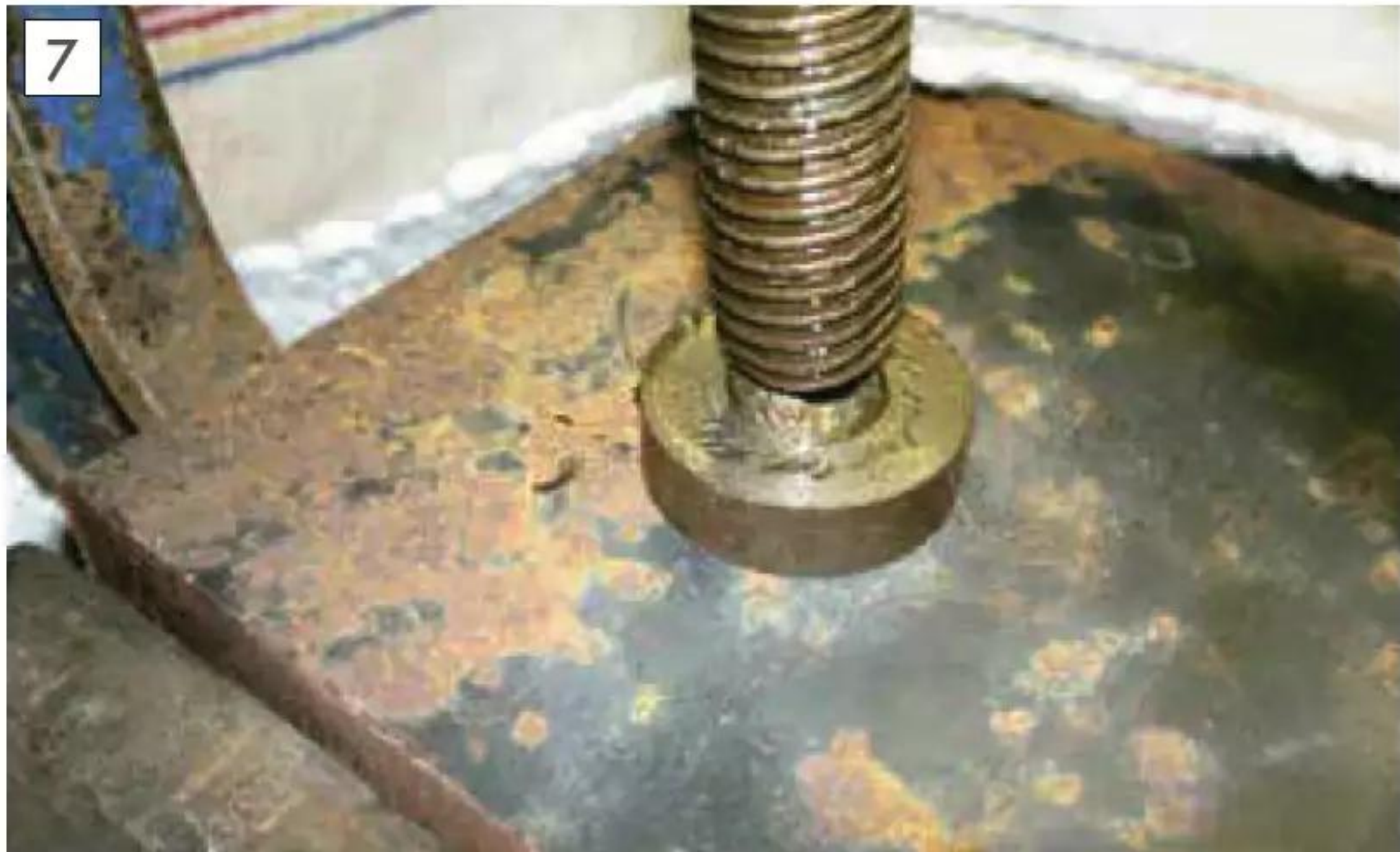
Fitting the foot to a clamp.
