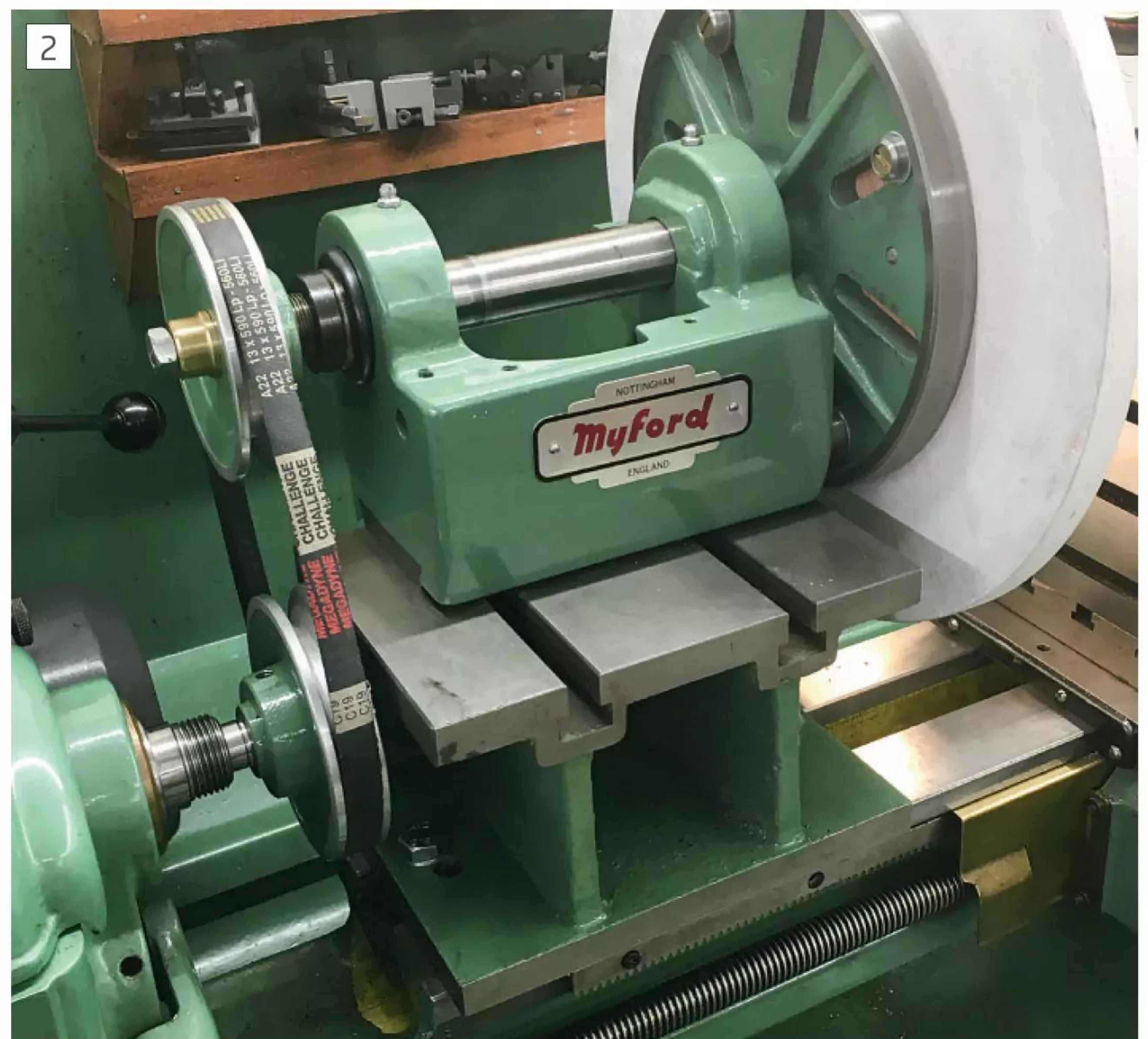
The spare Myford headstock mounted on a block to form a raised head (Photograph by Jake Sutton)
