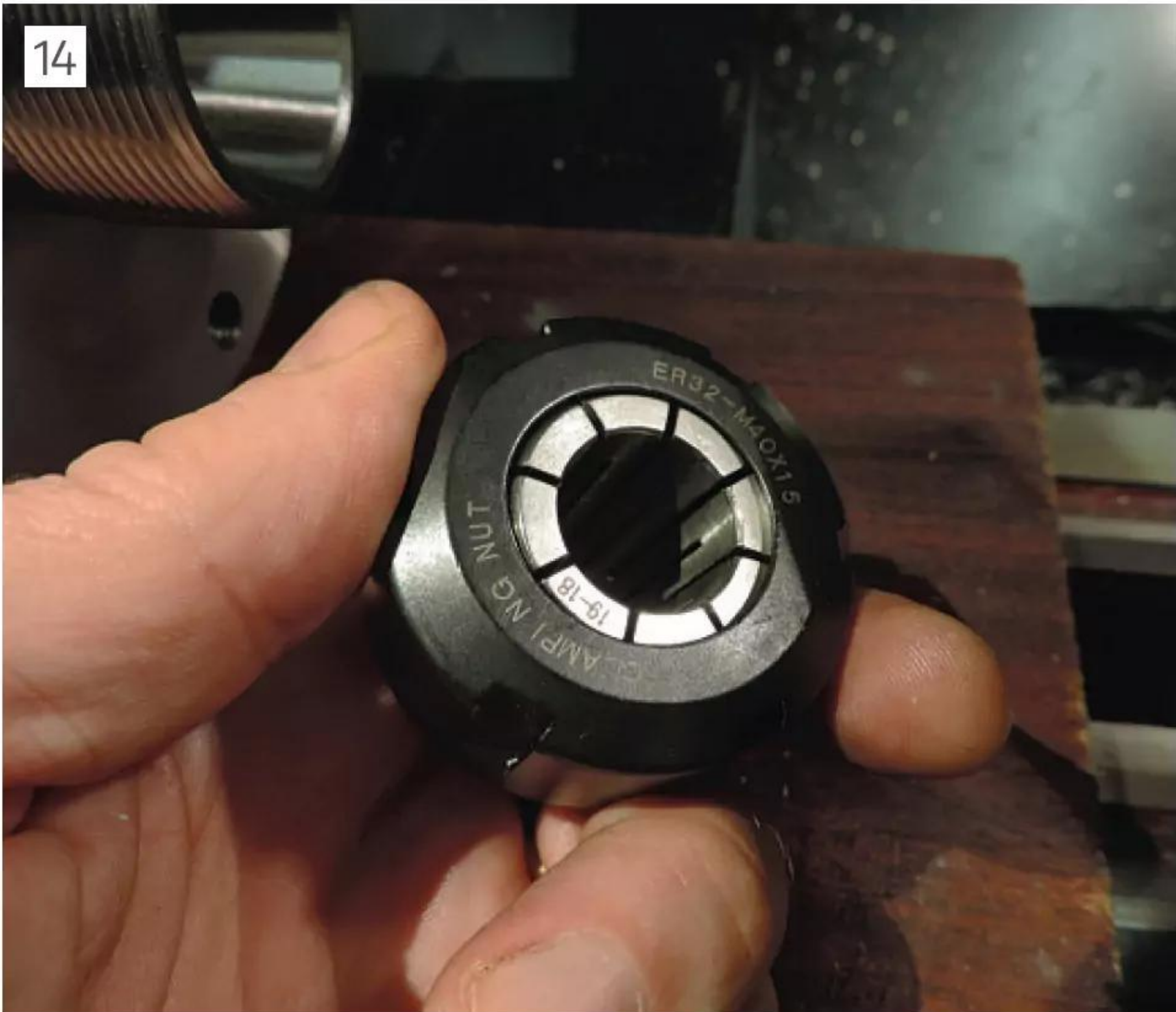
How a fitted collet should appear.
