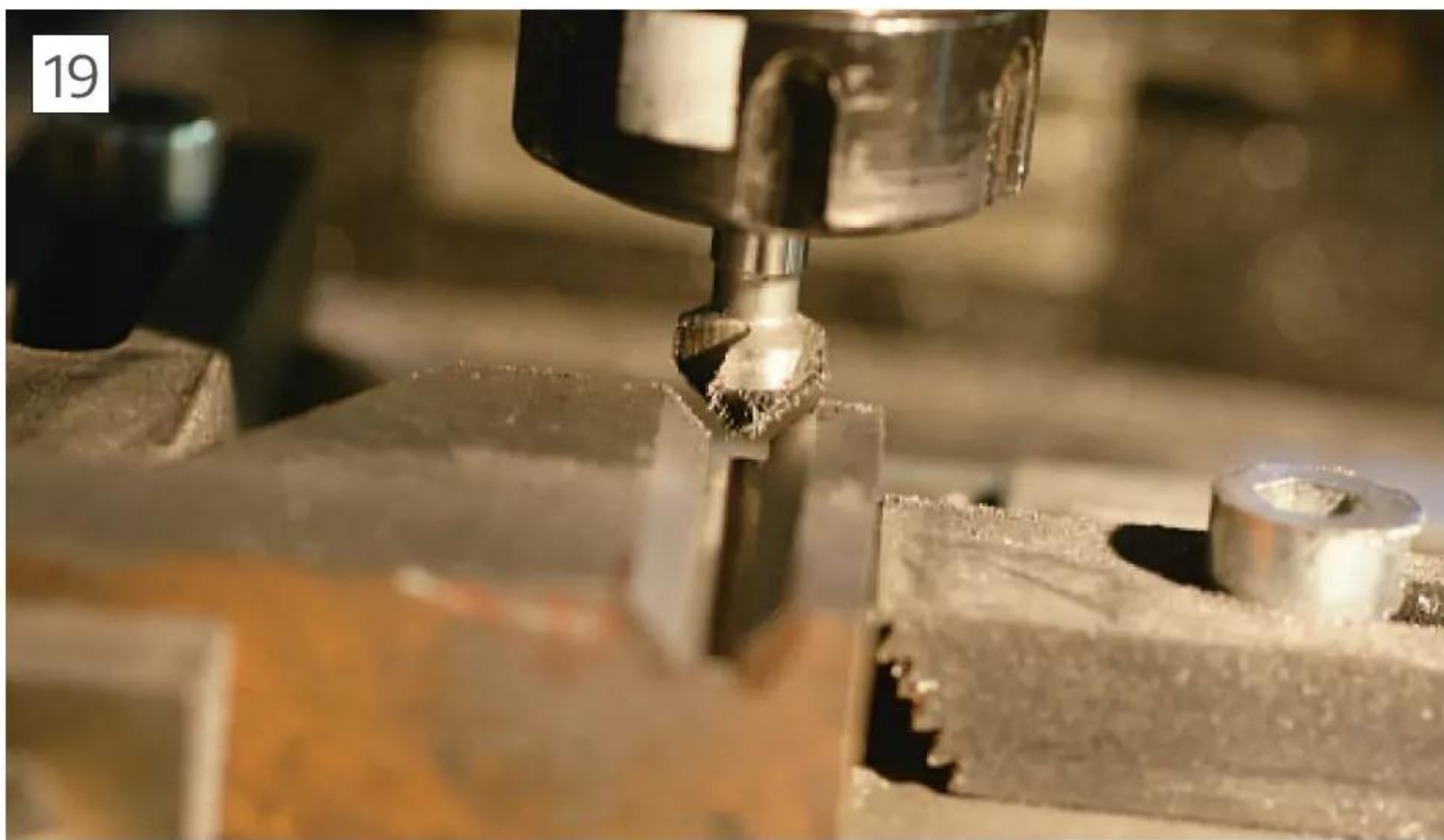
19 Unusual use of a countersink – a subsequent re-machining used a 'proper' 90° V end mill.
