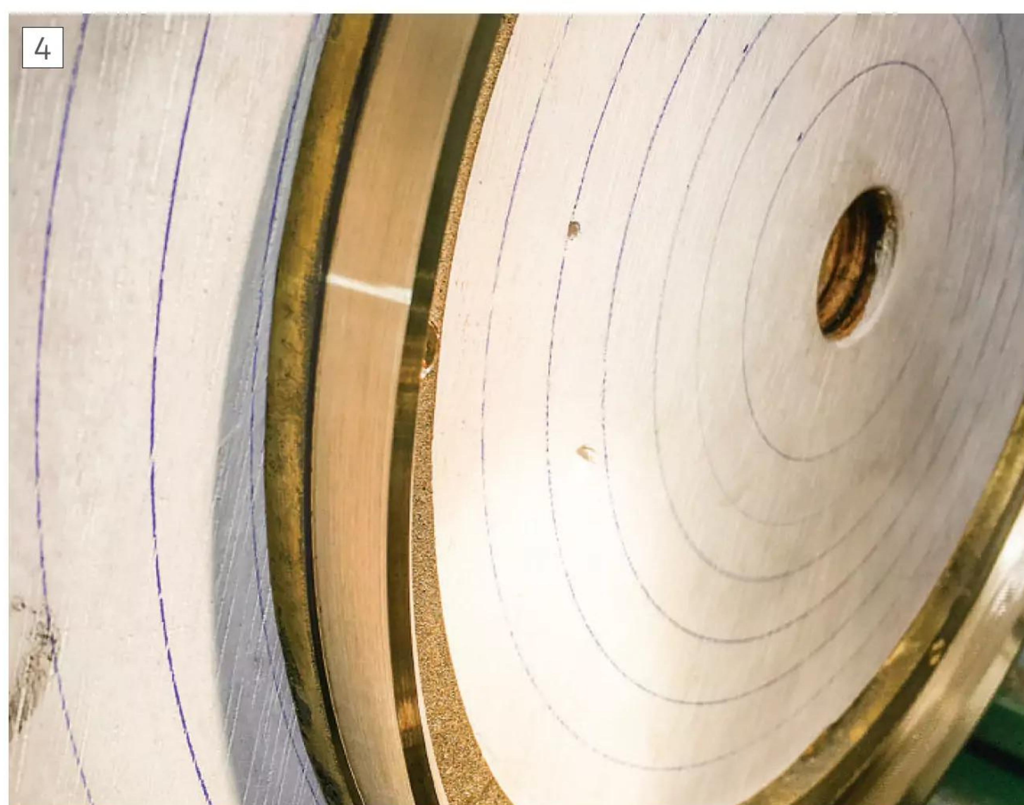
The part turned bezel. Note the rings drawn on the wooden support to make centering easy. (Photograph by Jake Sutton)
