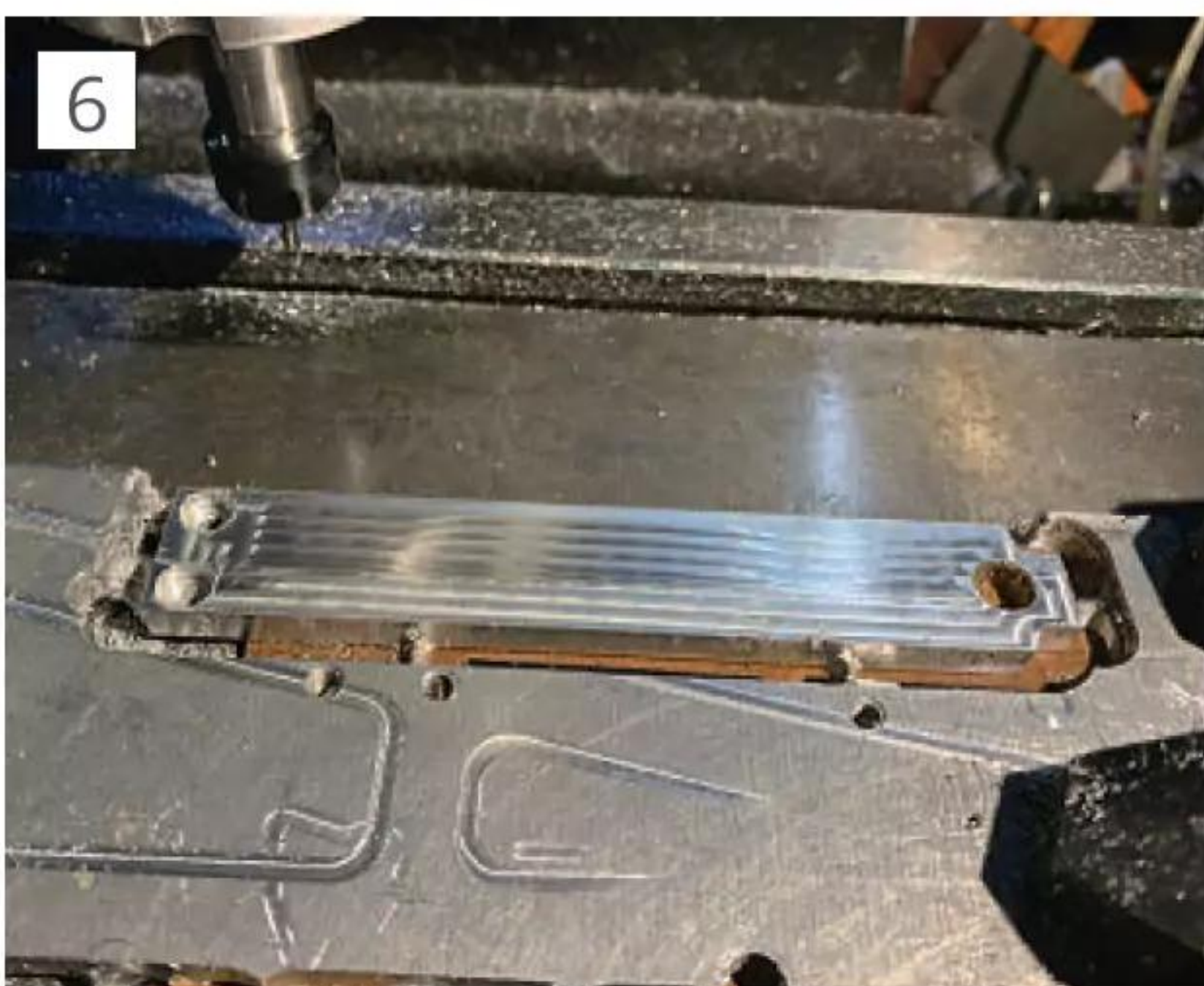
Original vertical support before I realised that it would not place the DTI near enough to the tool tip.
