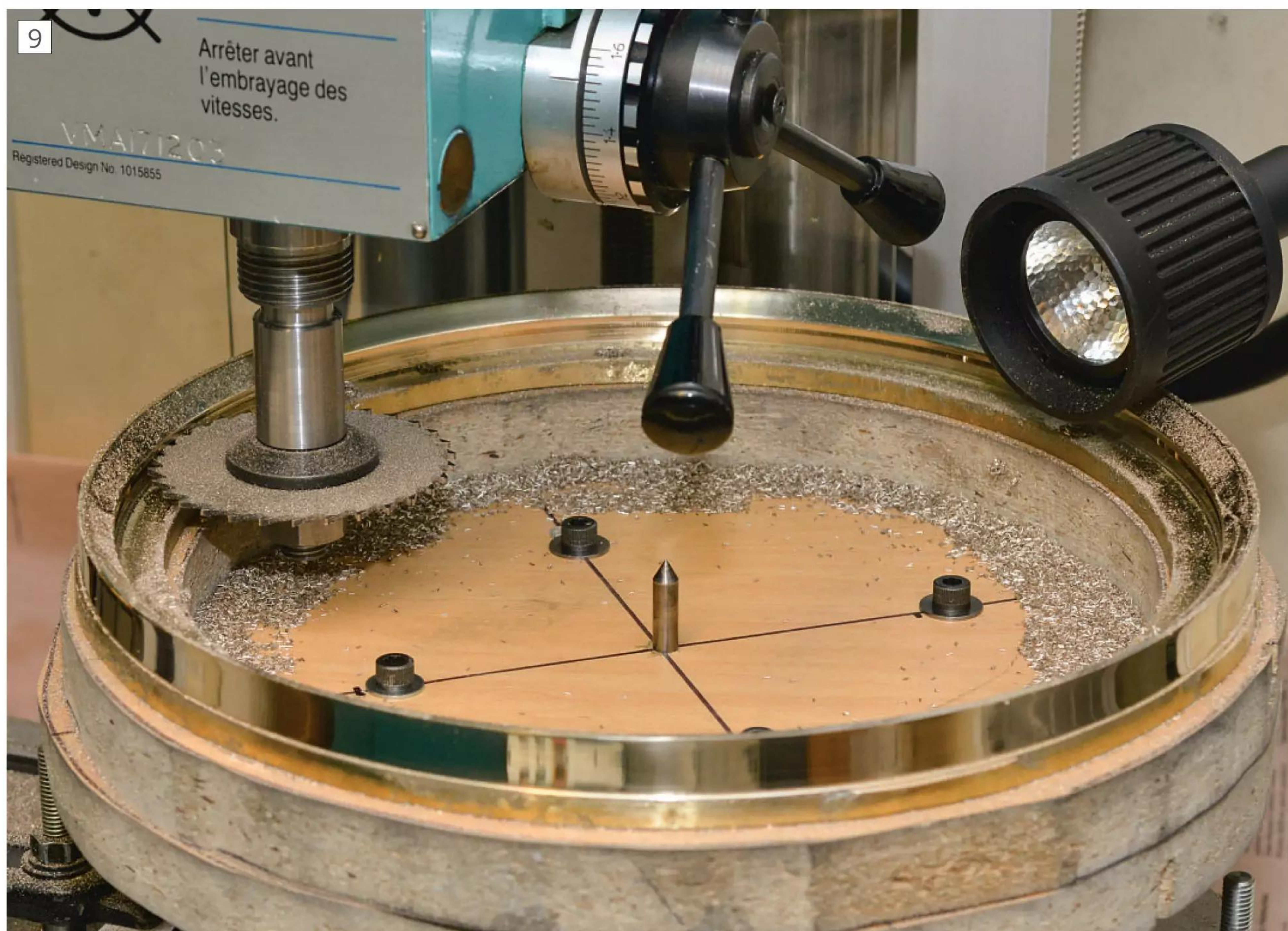
9 Cutting the inner step with the slitting saw.
