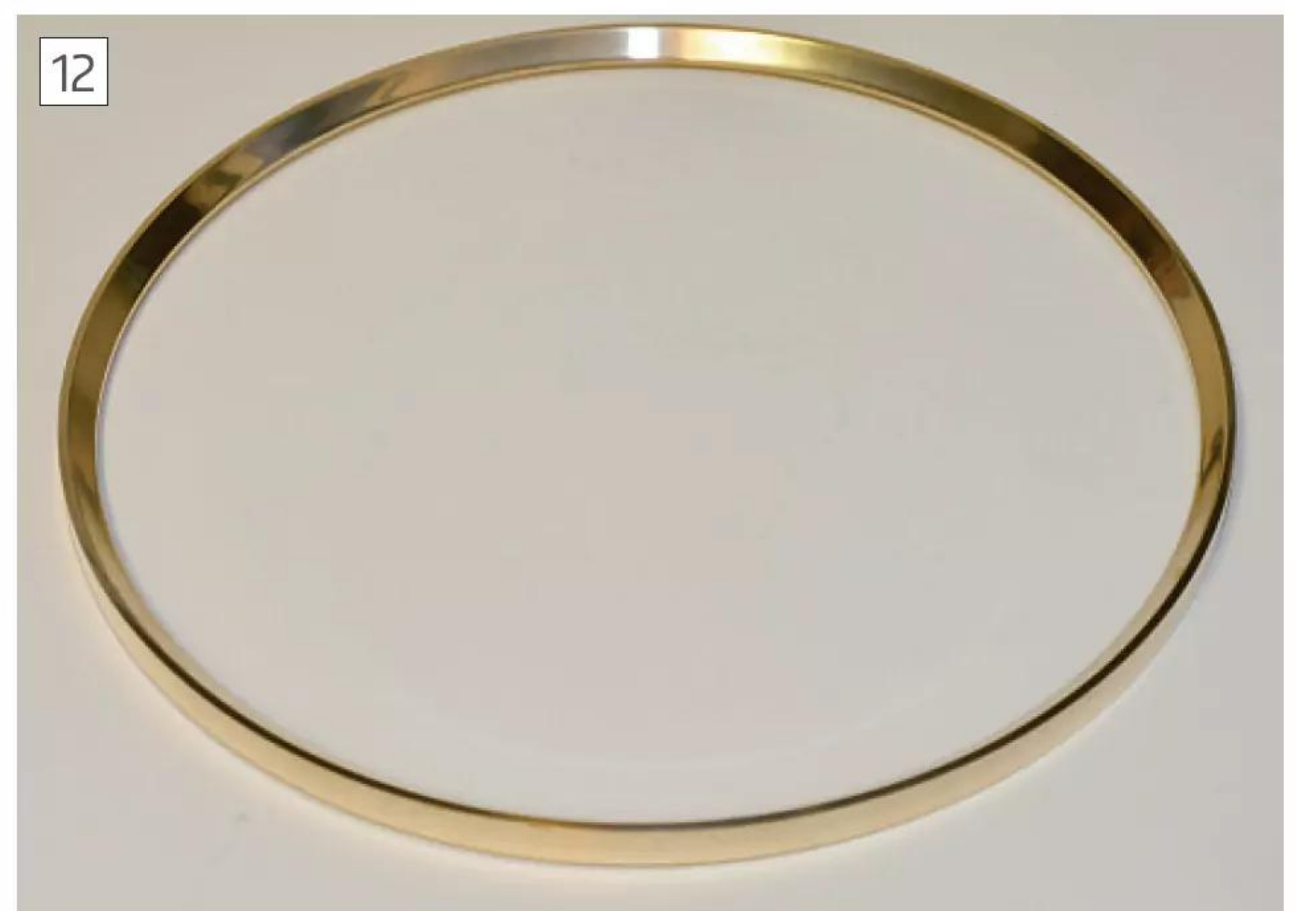
The rear face of the bezel has a step into which the face is mounted. This is secured by 8BA screws (still to be polished and blued in the photograph). Take care when drilling for these screws – do not to go too deep and ruin your bezel!
