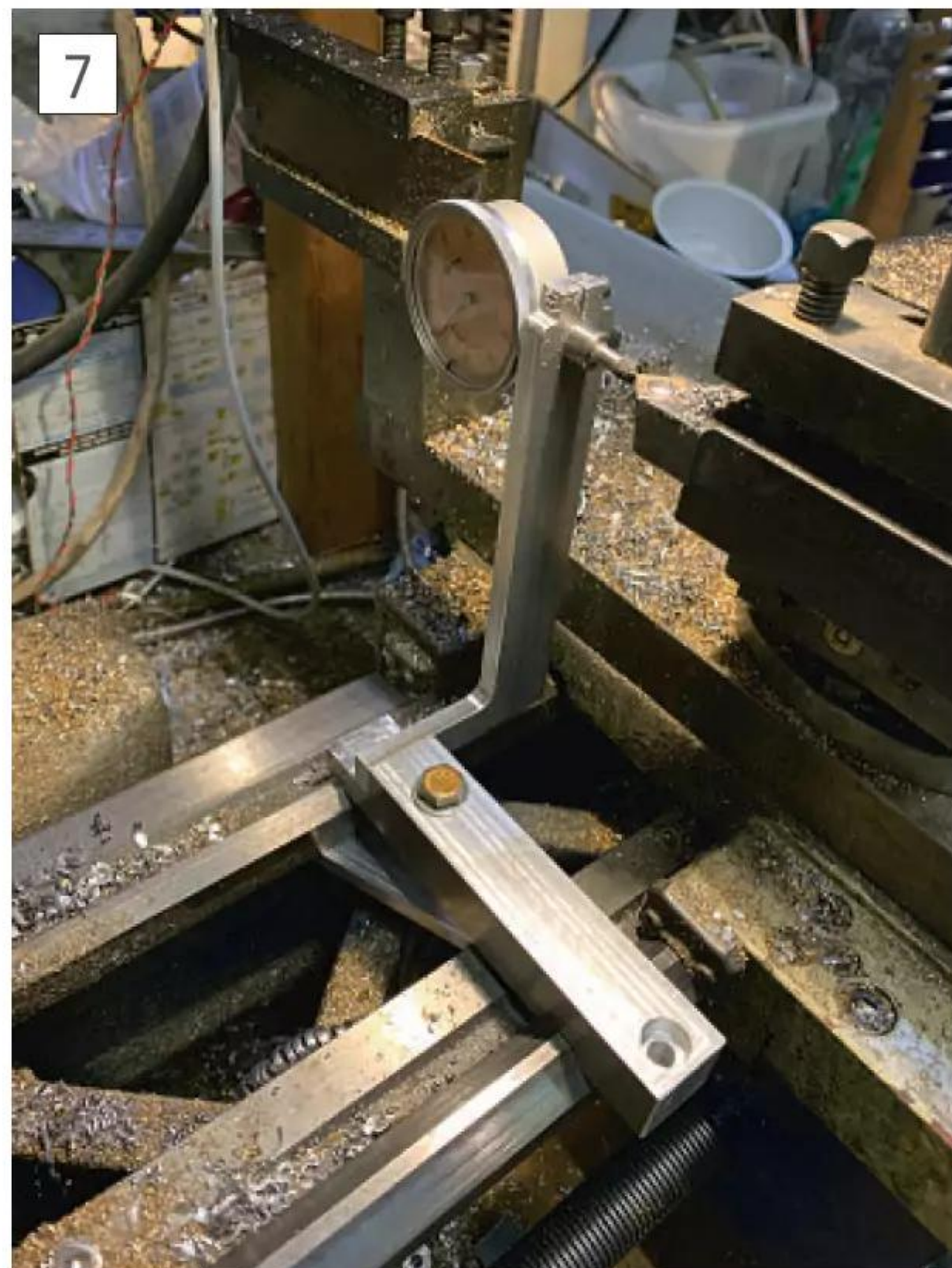
Version 1 installed with a DTI for the initial tests. Note the cranked vertical support after discovering that a simple straight support would not access the tool tip under normal circumstances.
