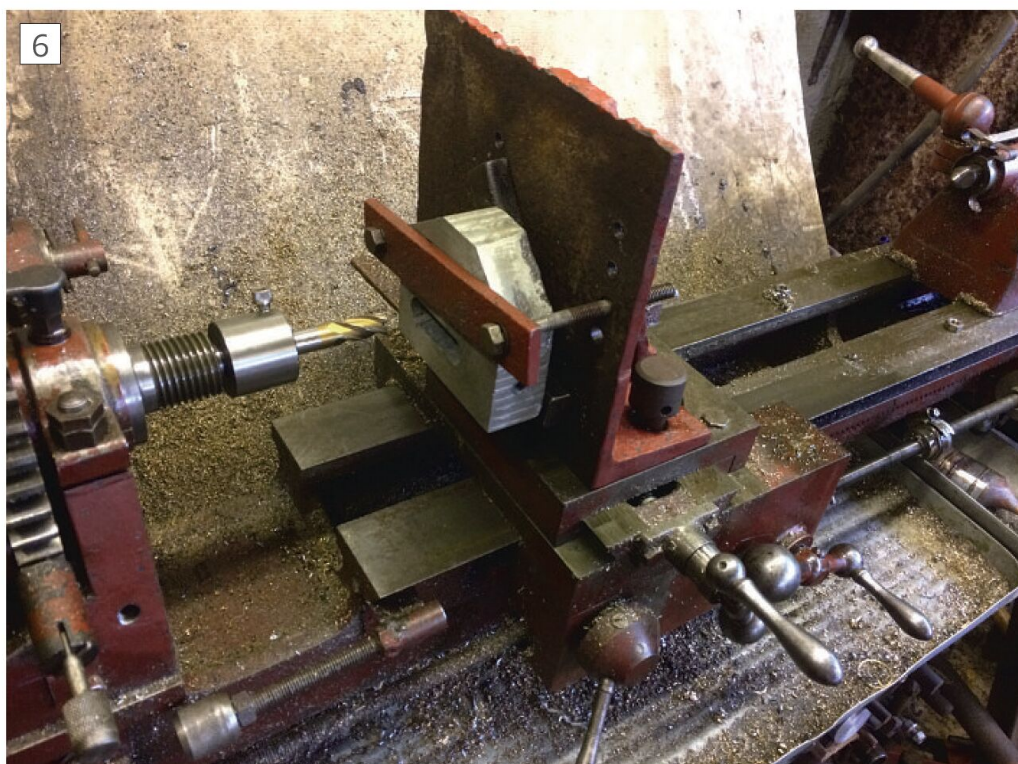
Milling the end support slots.
