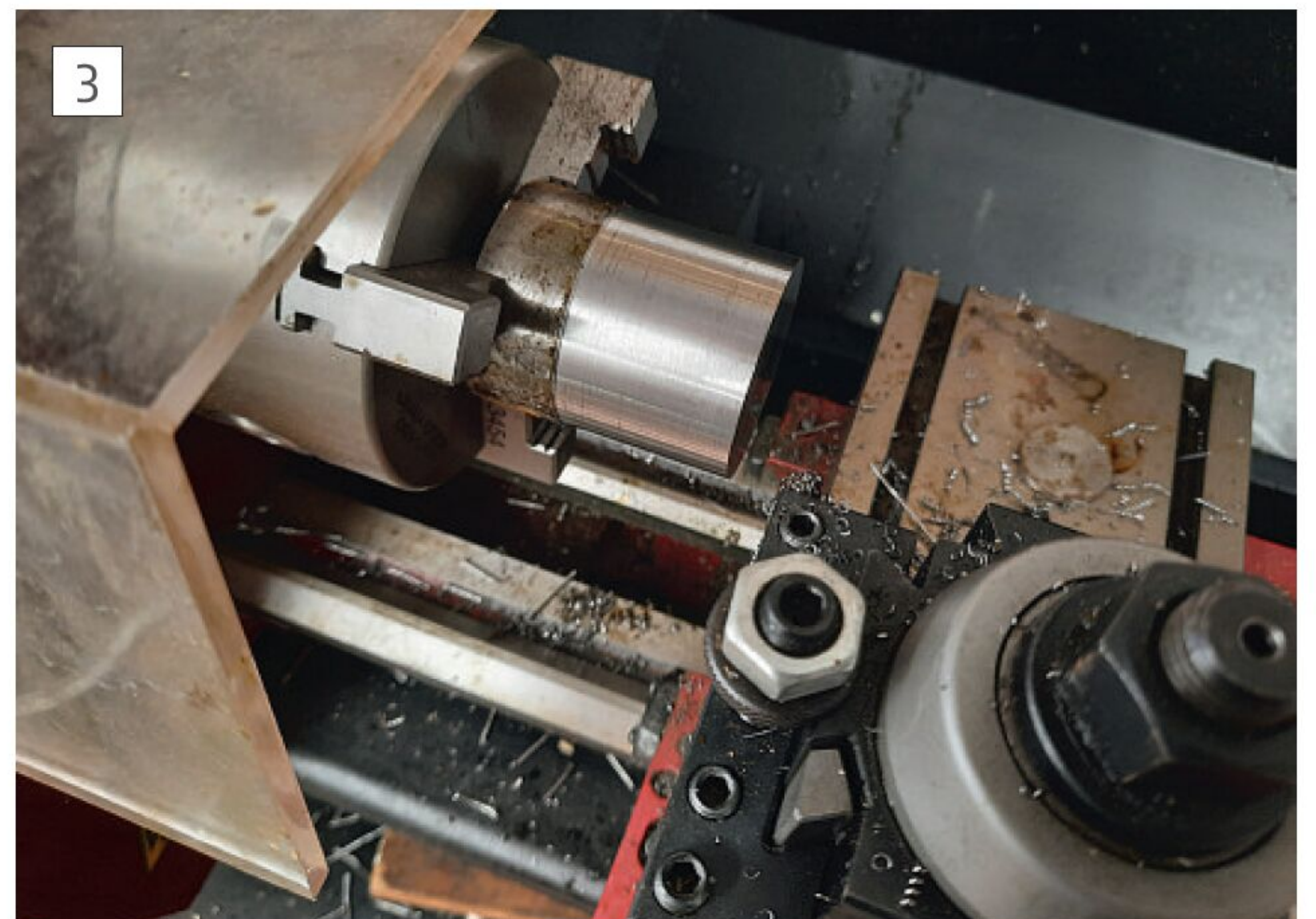
Taking a skim along the surface of the bar with the same tool.
