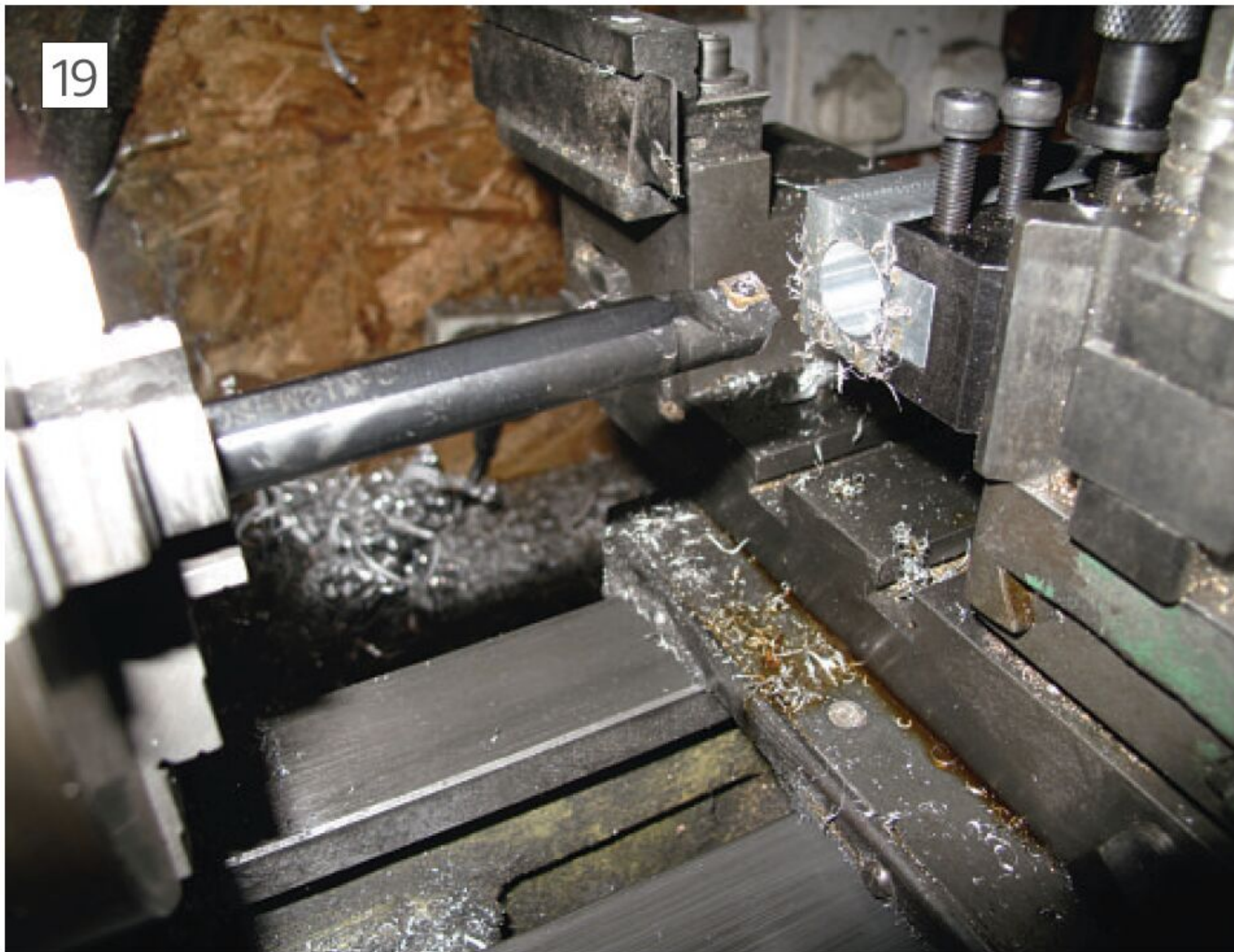
Turning the bore parallel.
