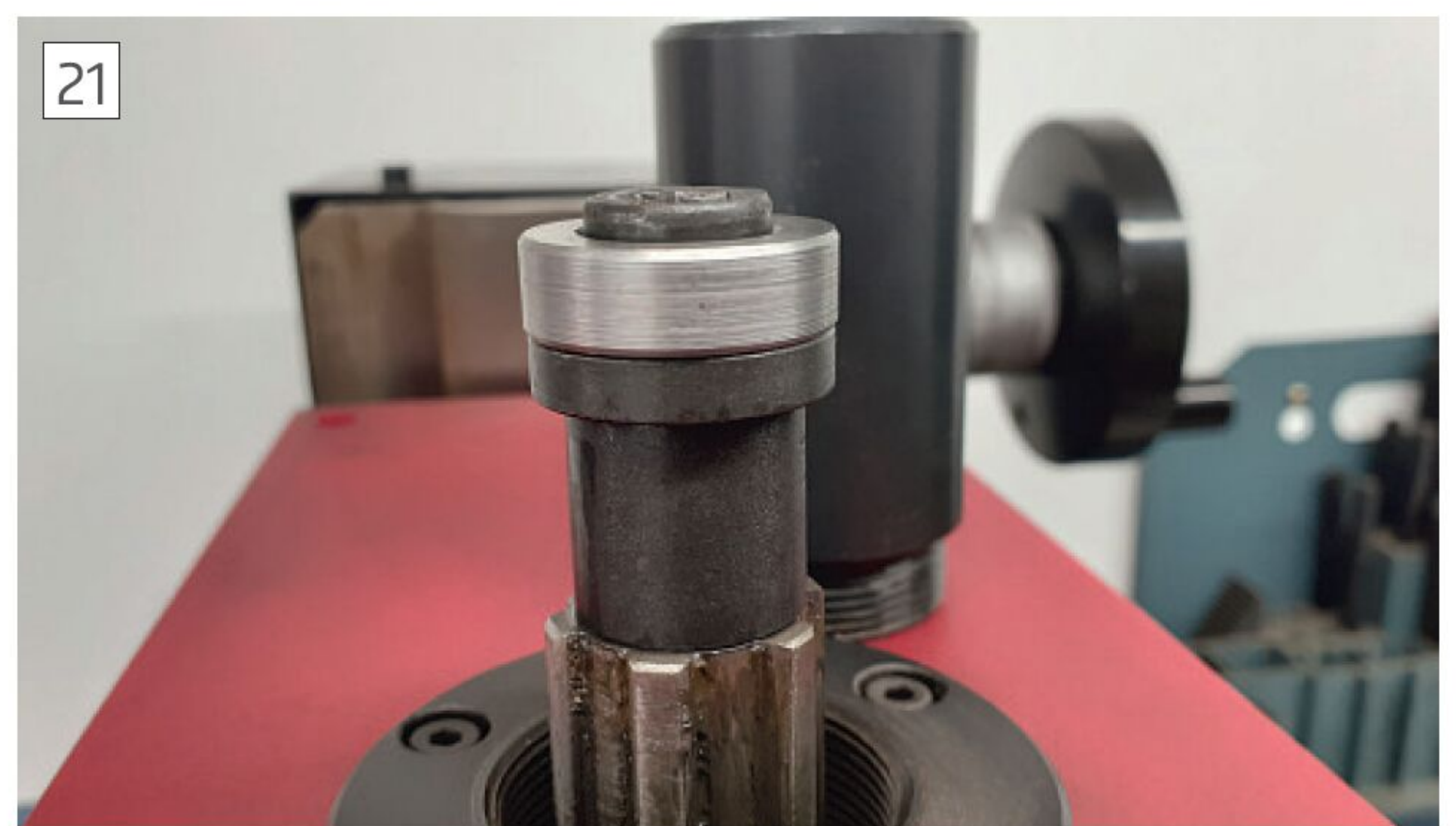
Draw bar spacer ring in place
