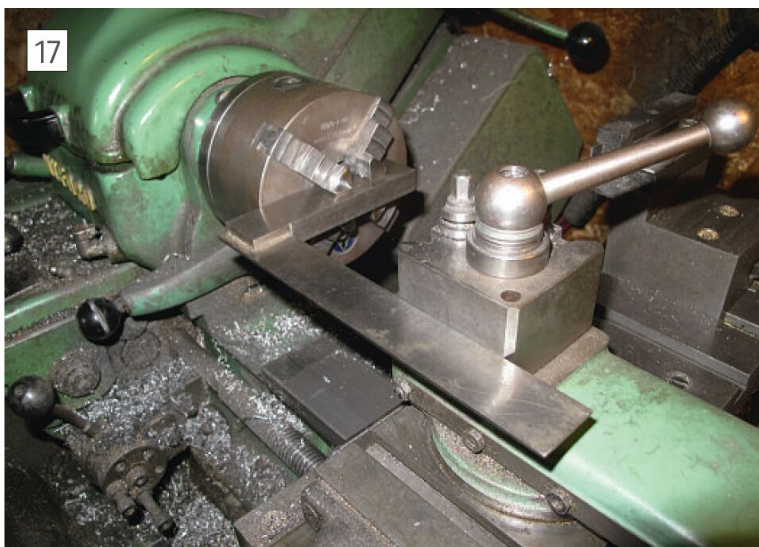
Setting the tool post square to the spindle.
