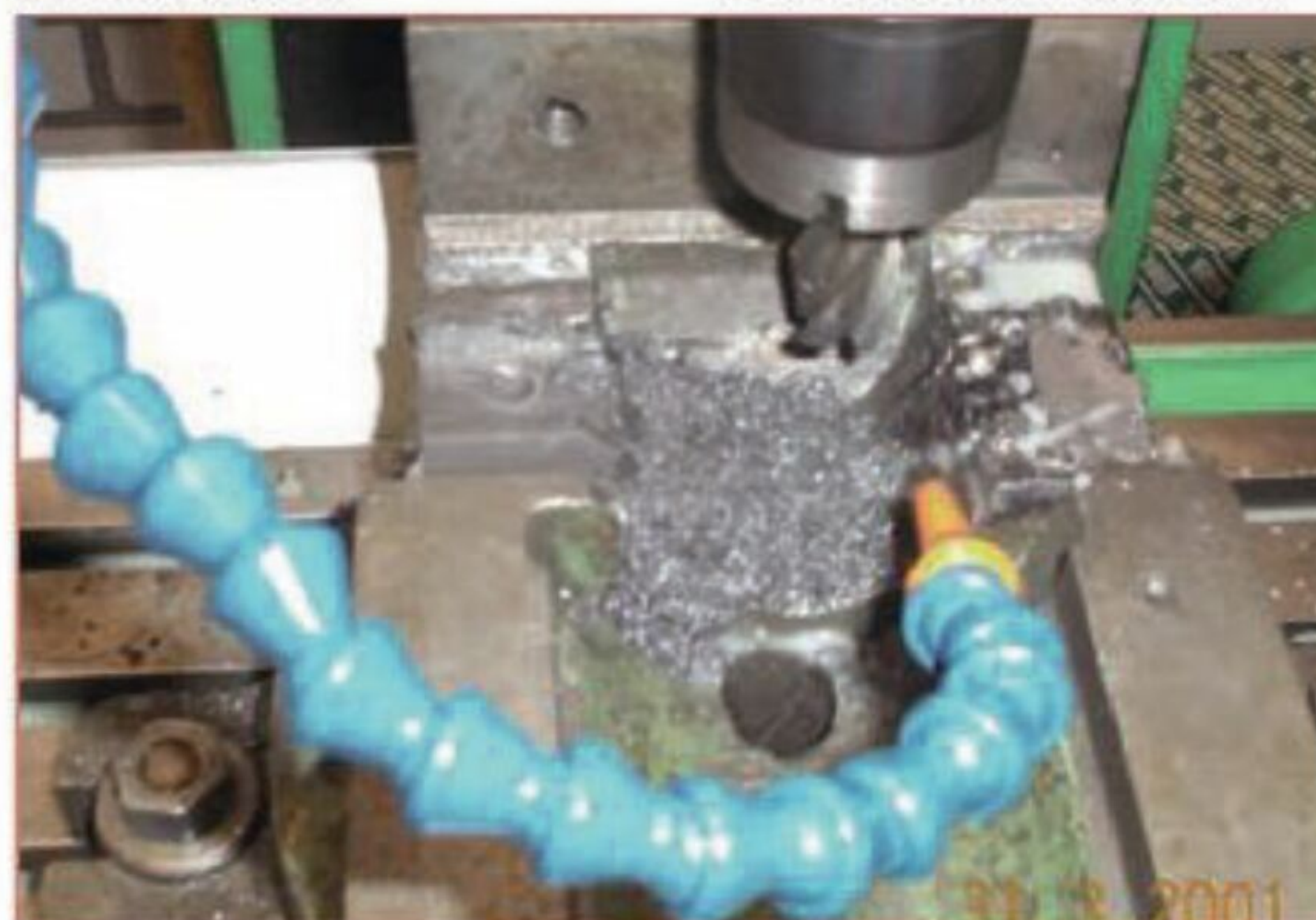
3. Machining the recess for the insert
