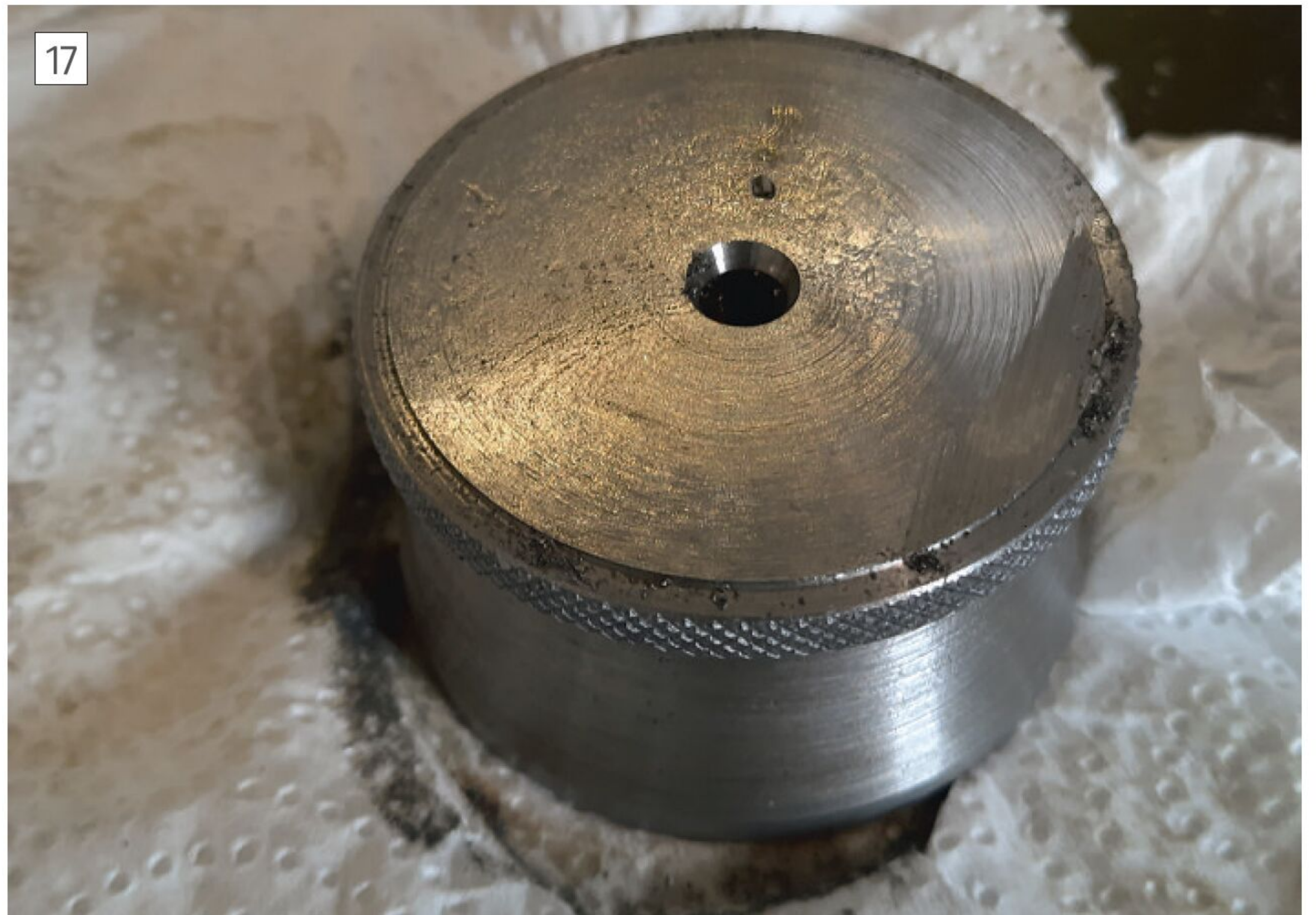
Weight before degreasing with soda crystals (washing soda).
