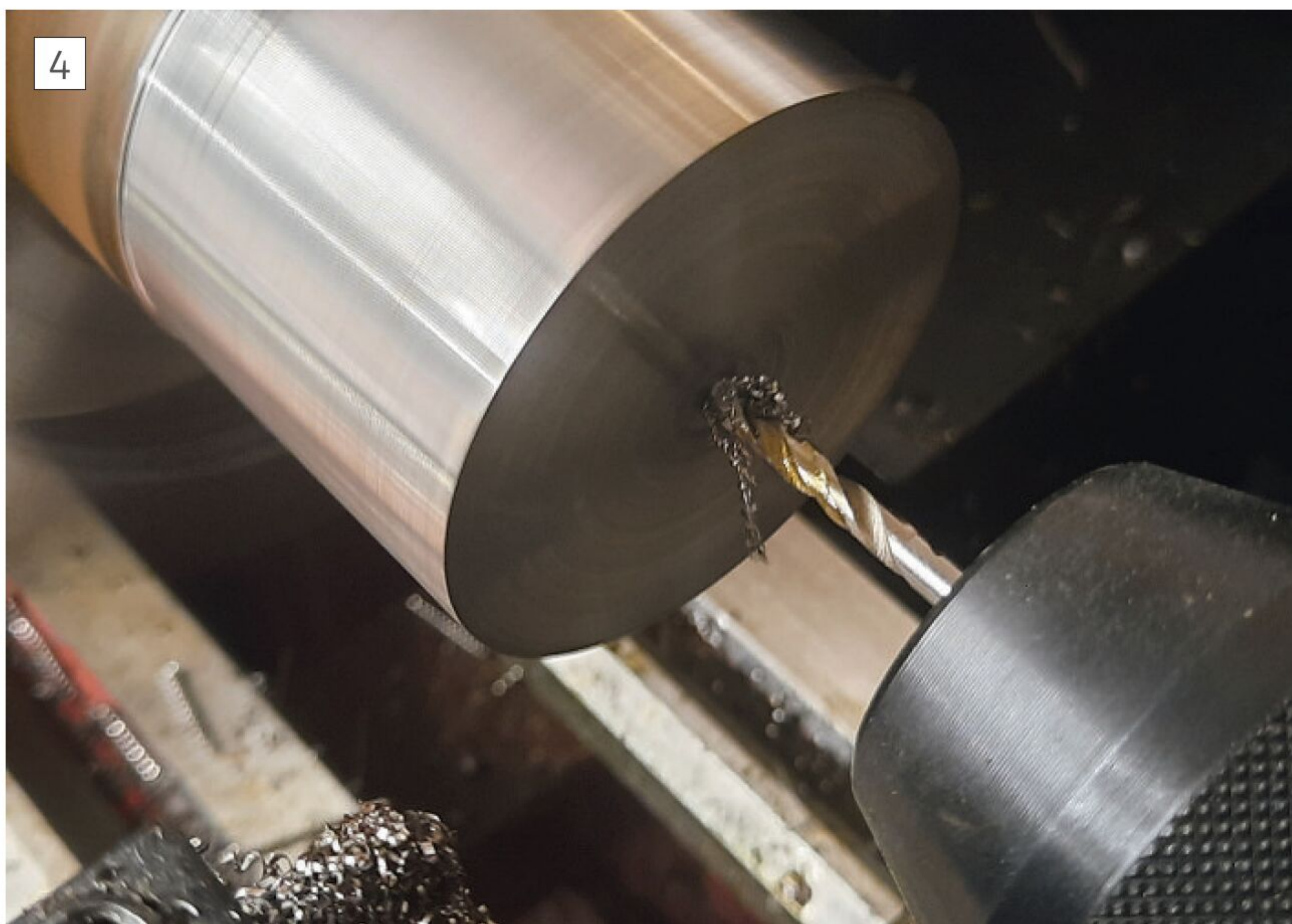
I prefer a spotting drill to a centre drill.
