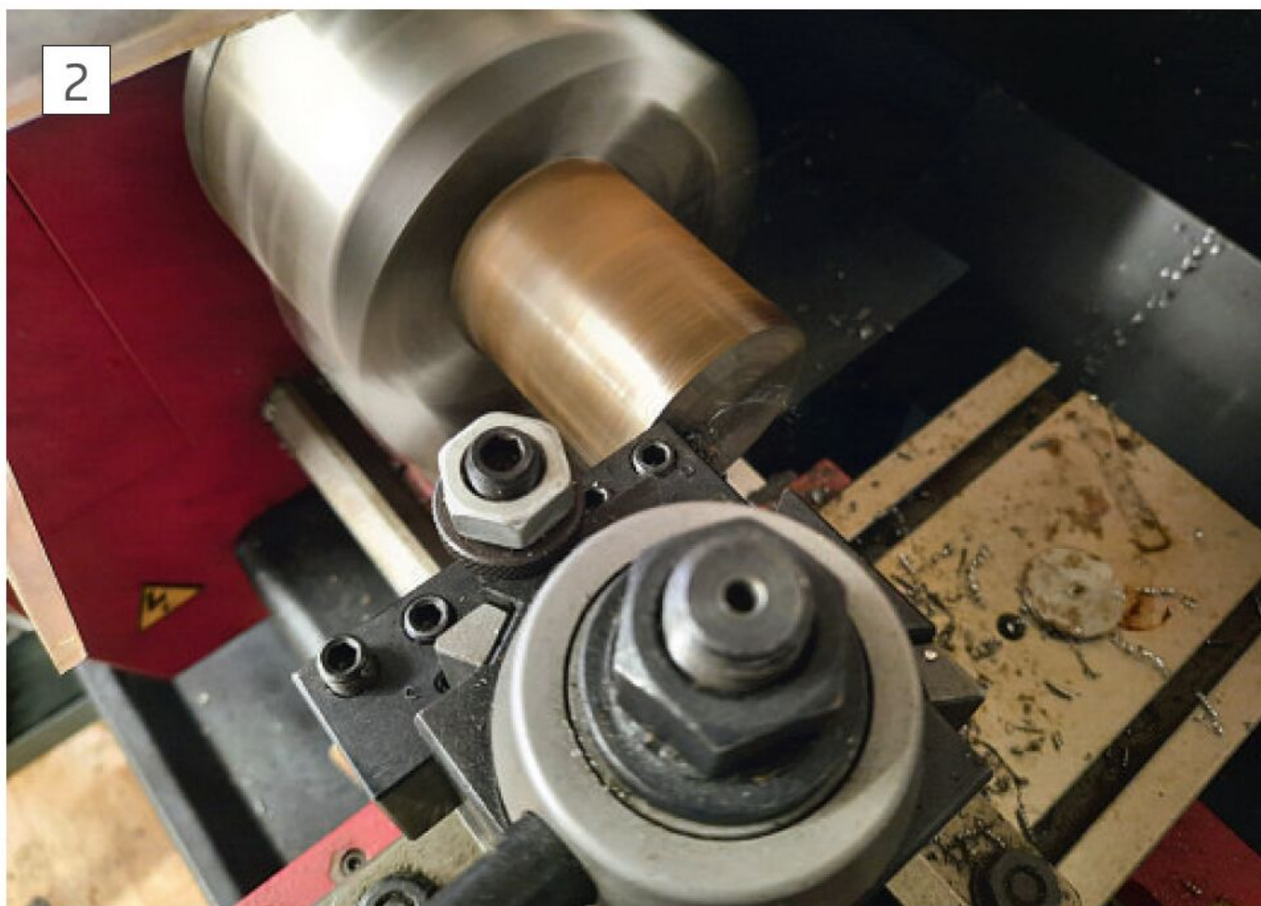
Facing the end of the blank with a right-hand tool.
