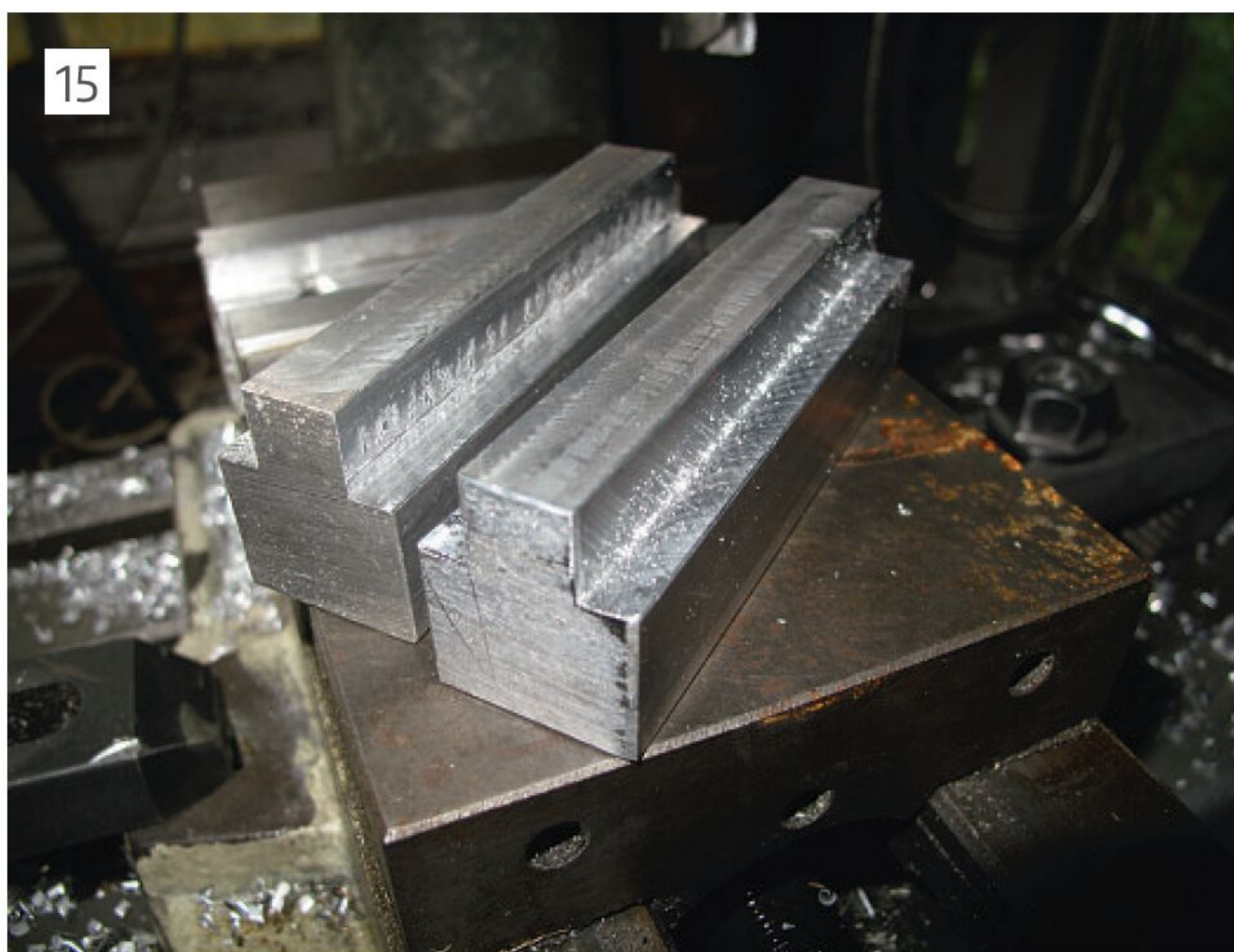
Initial machining of the tool holding blocks.
