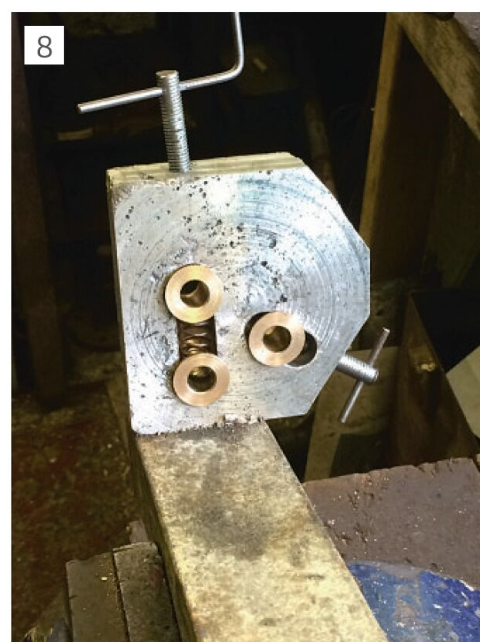
End support with bushes and adjusting screws.
