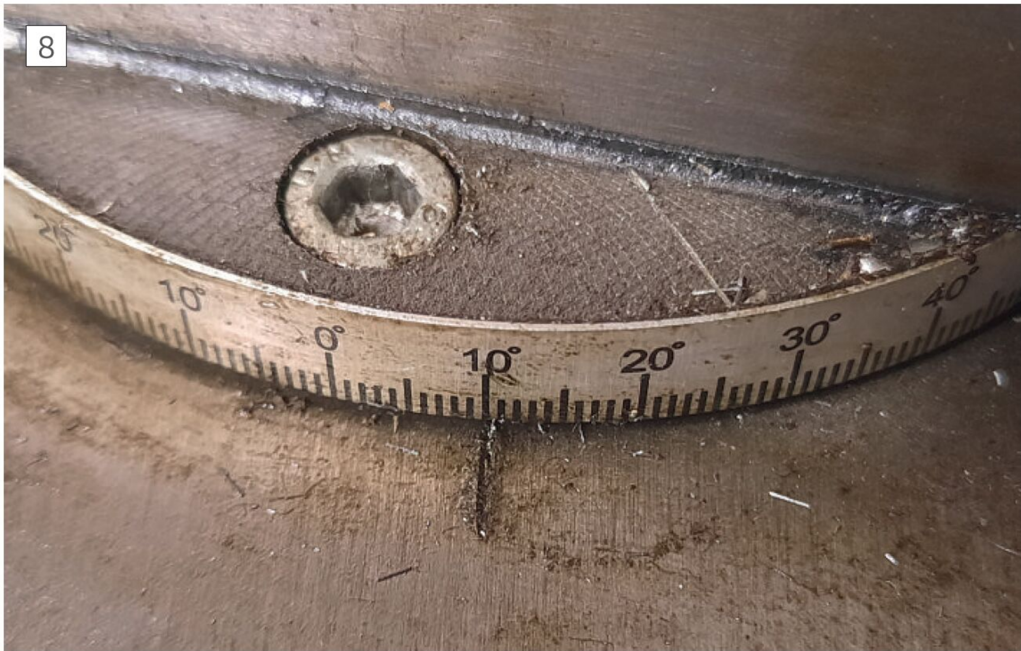
Setting the topslide for taper turning.
