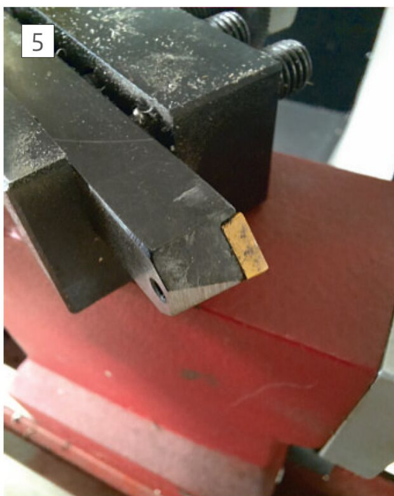
90-degree turning and chamfering tool modified for recessing the end of a bar.
