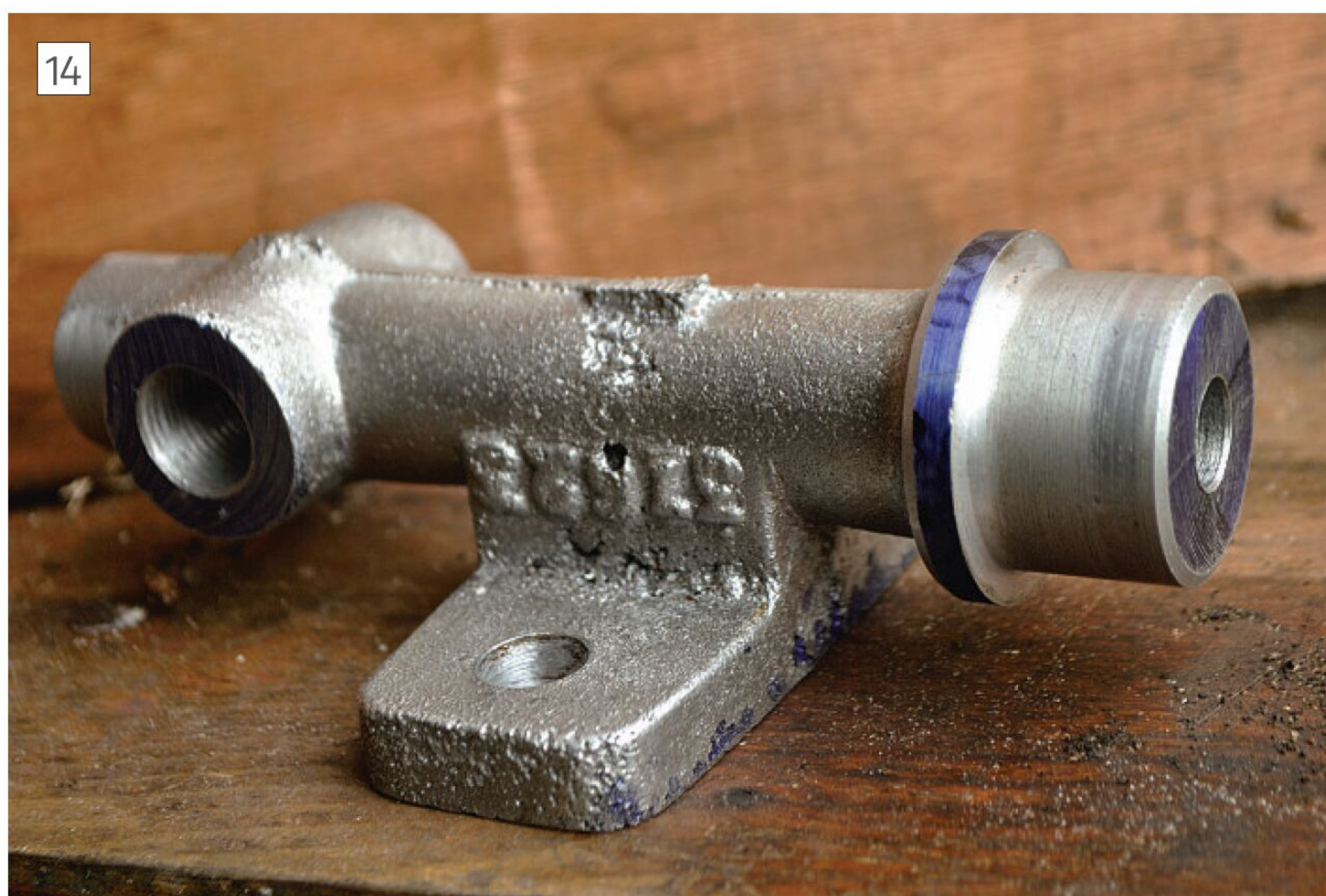
The alloy test casting fully machined.
