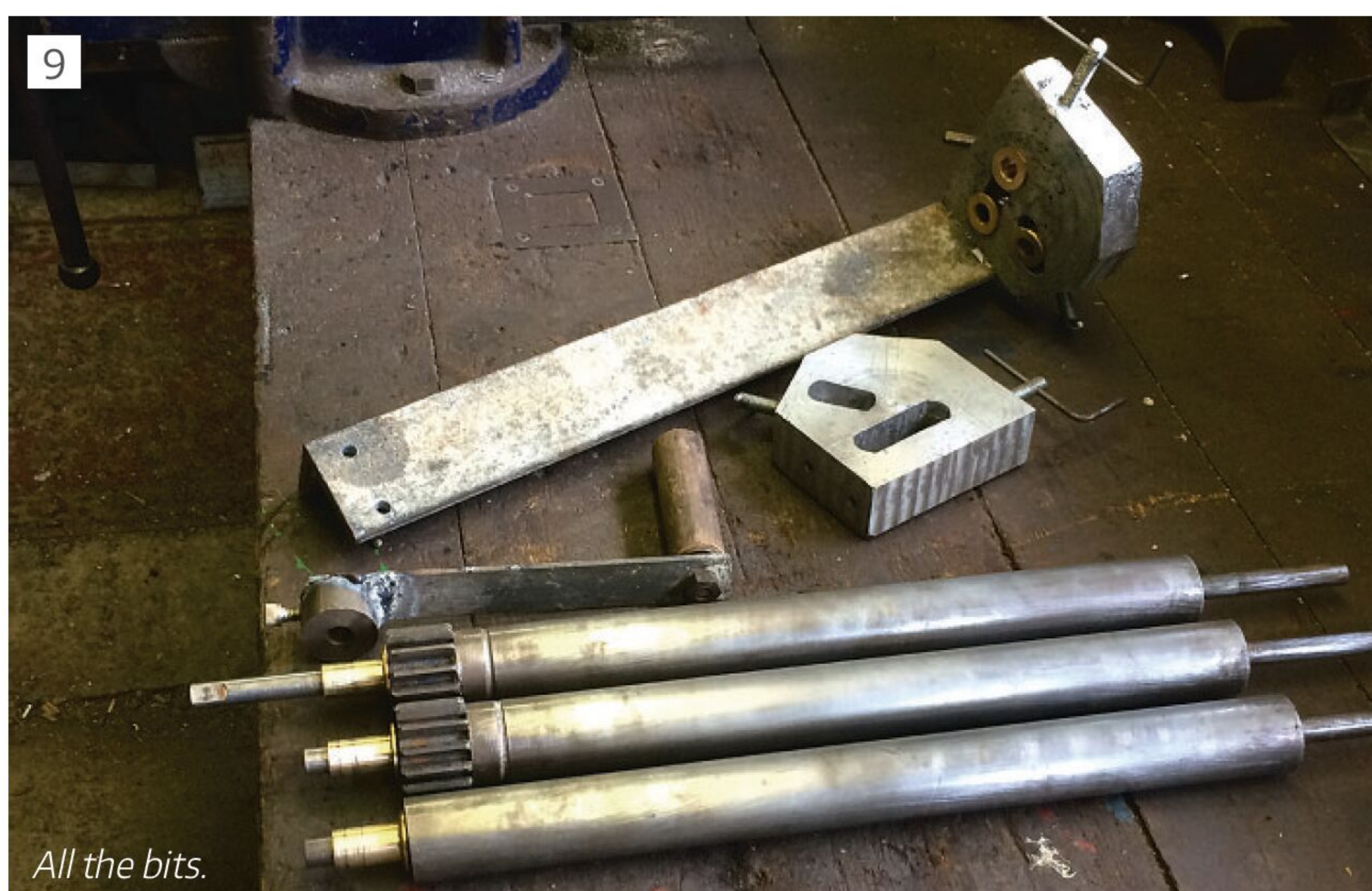
Rollers at the gear end. Bushes and spindles in place. Grooves for wire rolling shown.
