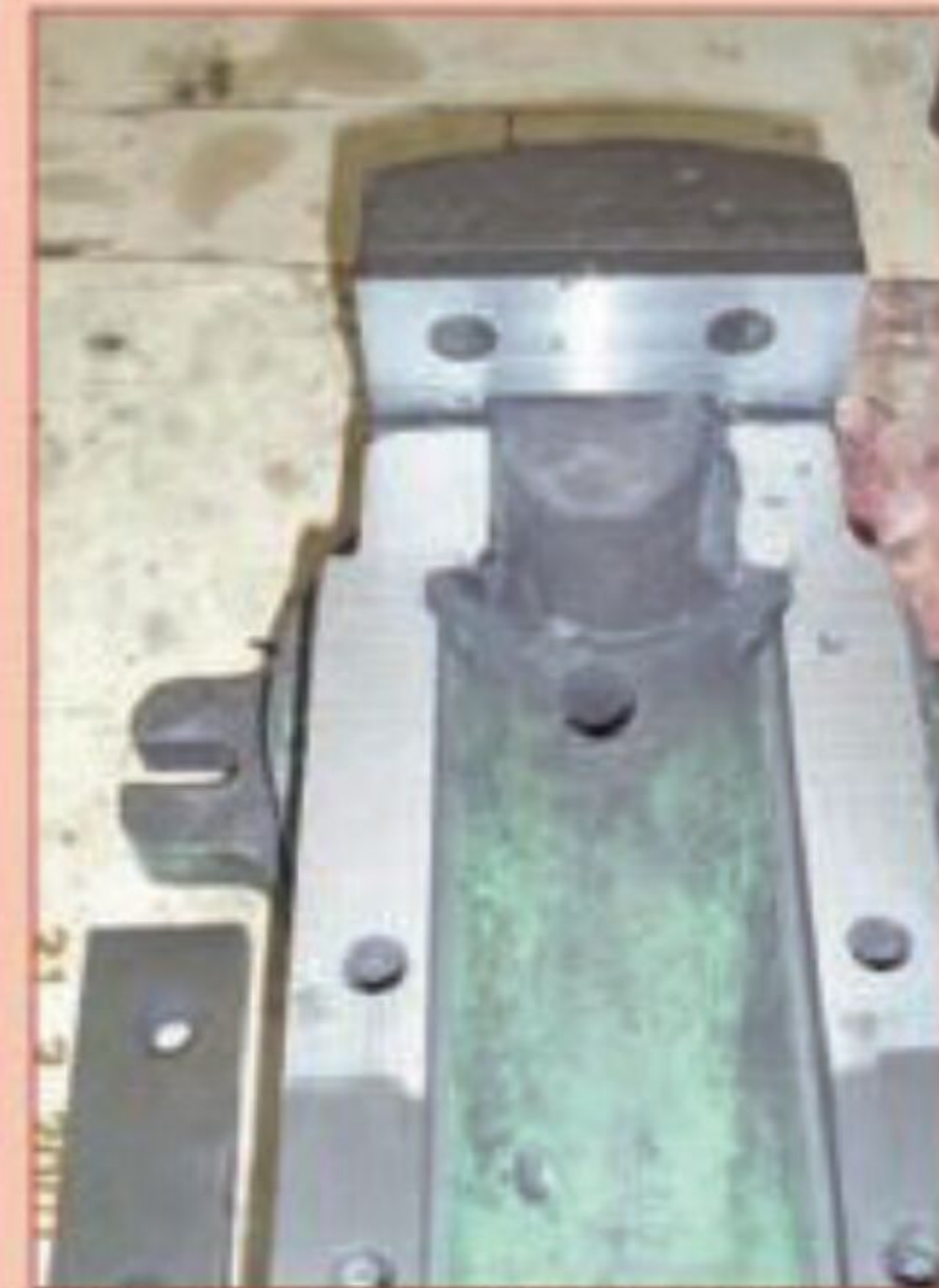
5. The appearance after re-grinding
