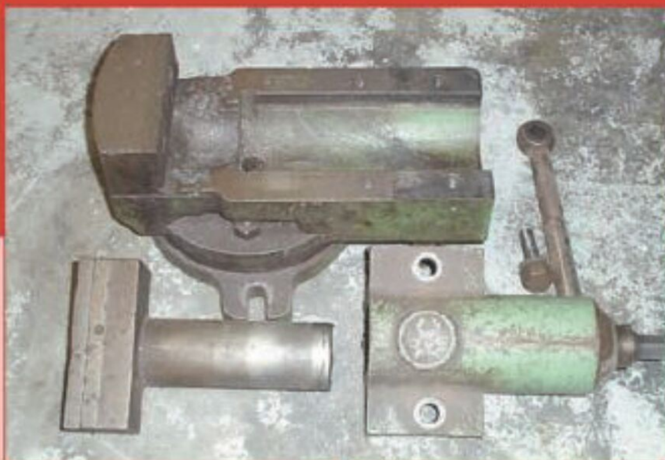
1. The components of the machine vice, showing the generally poor condition
