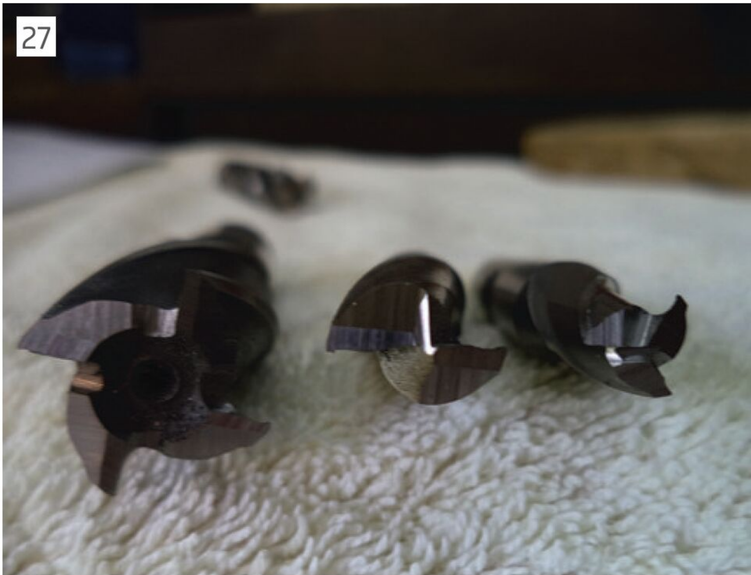
From left to right: end mill, two flute slot drill, three flute slot drill.
