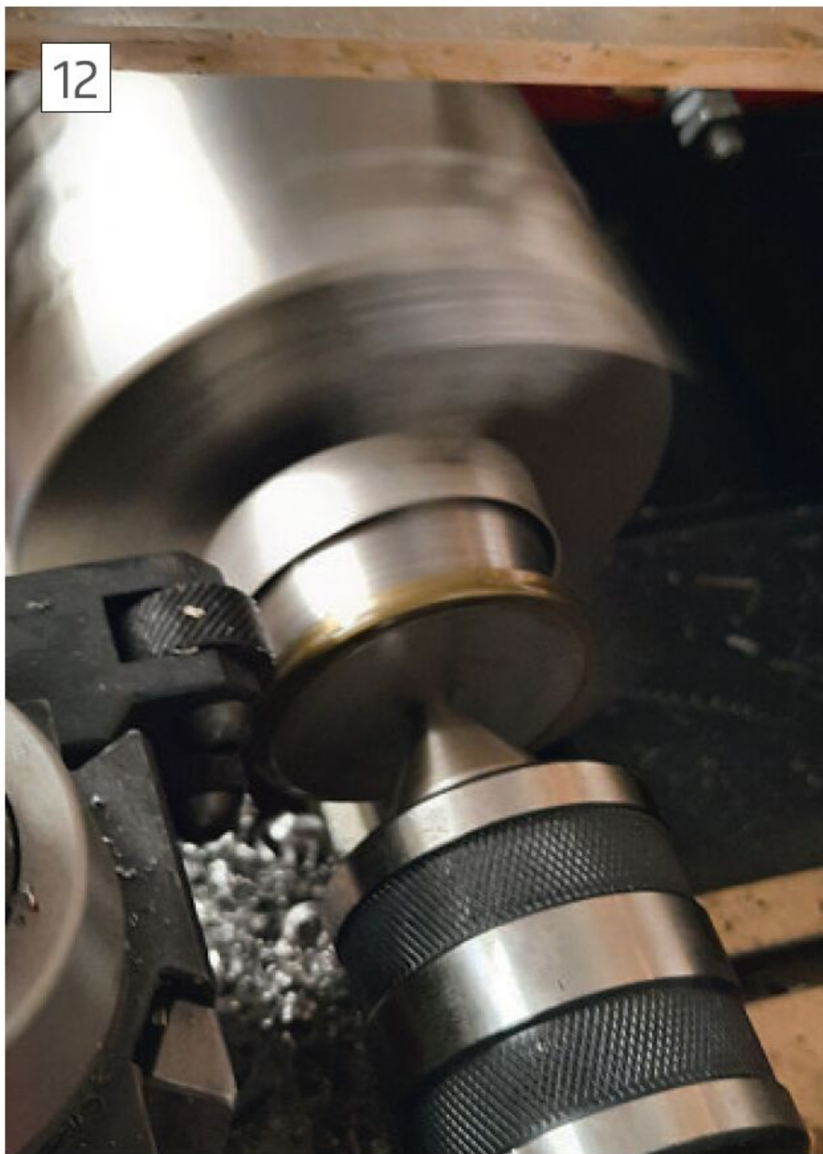
Just the lower knurl is cutting here.
