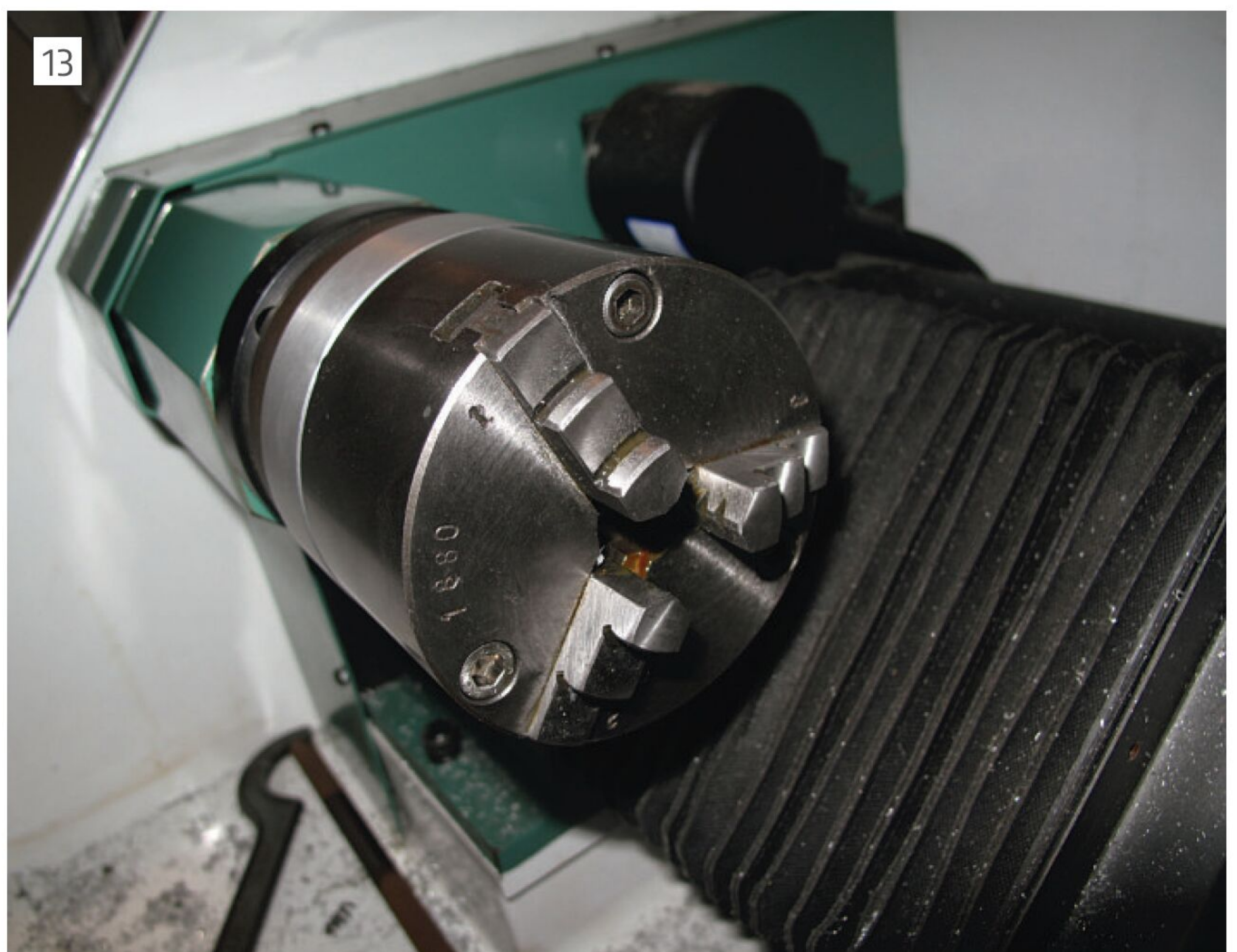
Chuck mounted 20 mm. forward from original position.
