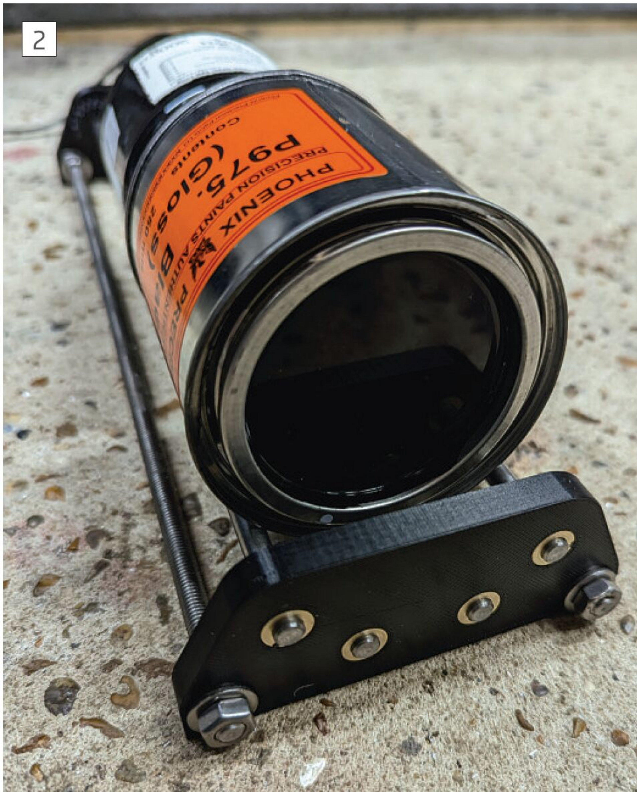
End view showing bearings.
