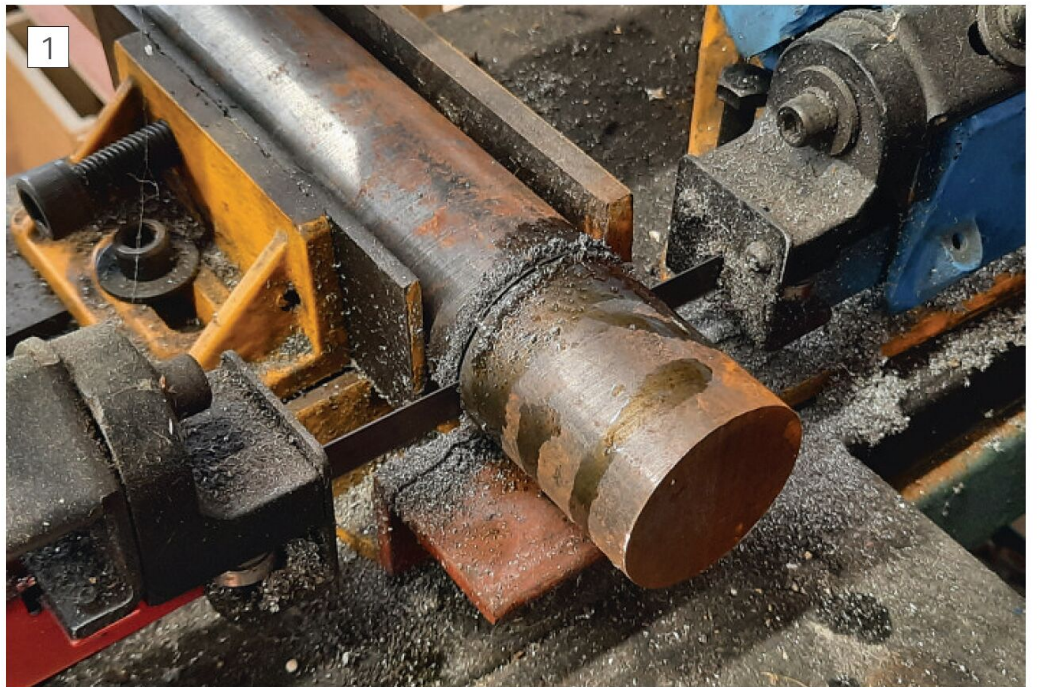
Sawing off a blank in the bandsaw.
