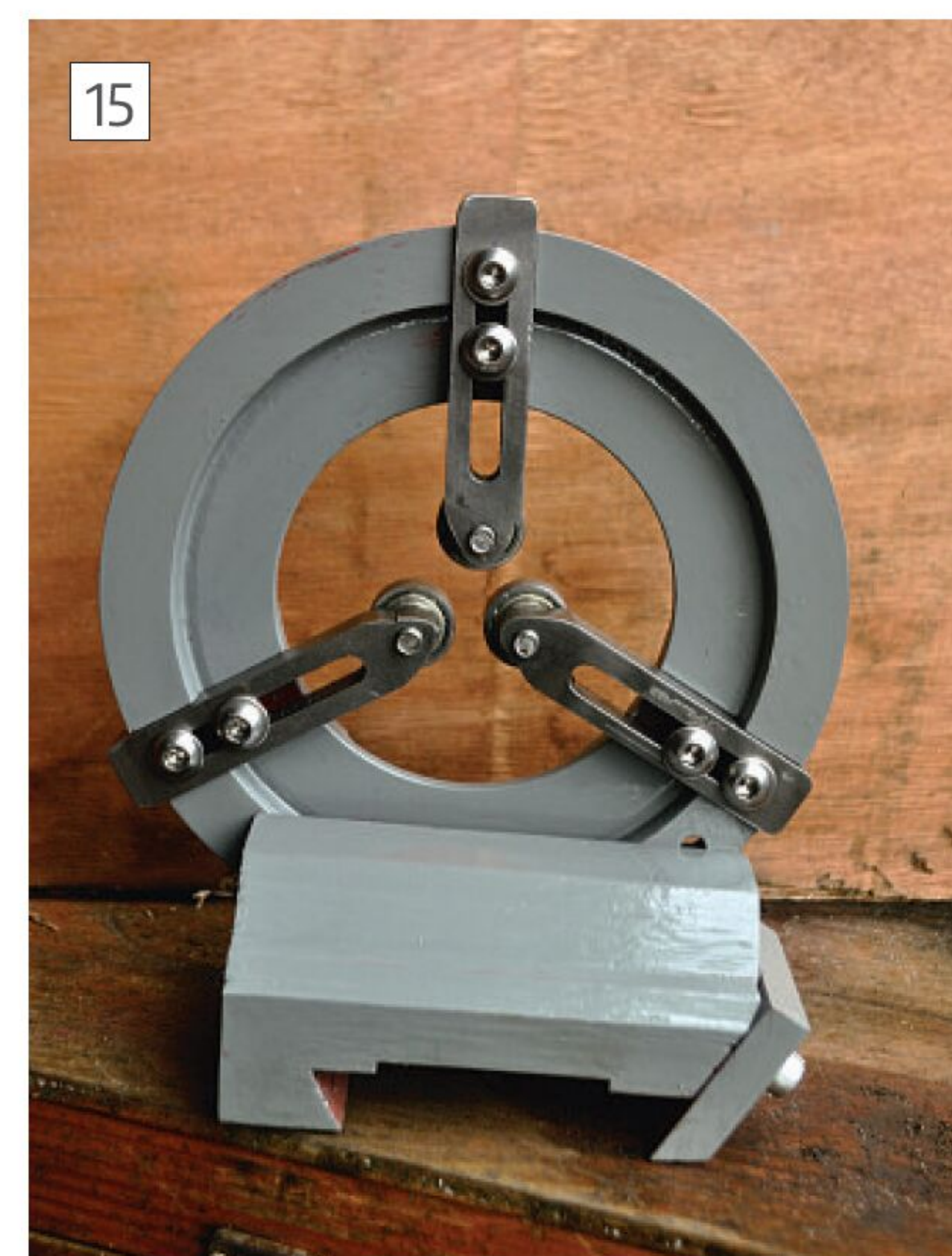
The fixed steady after a coat of machinery enamel.
