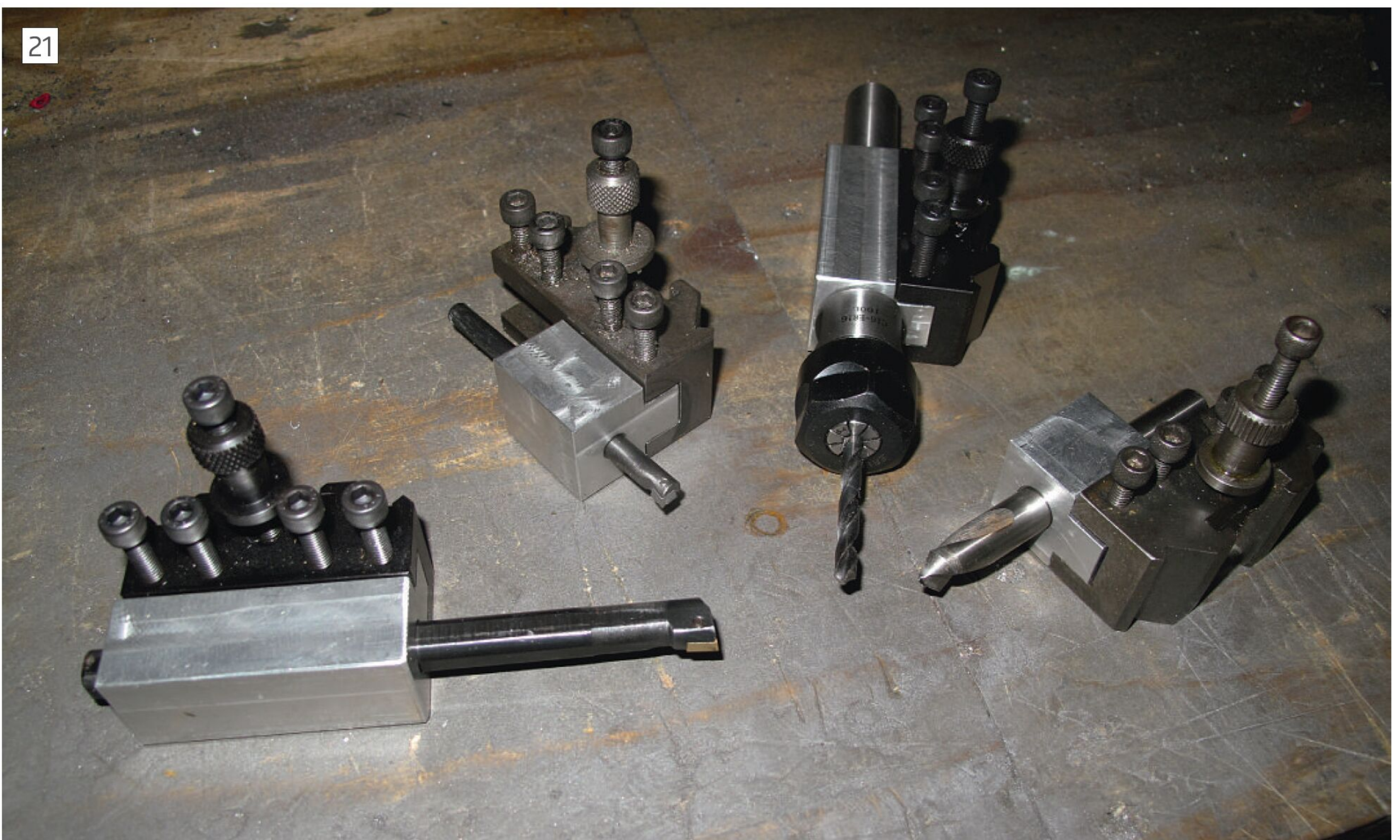
Four completed tool holders.
