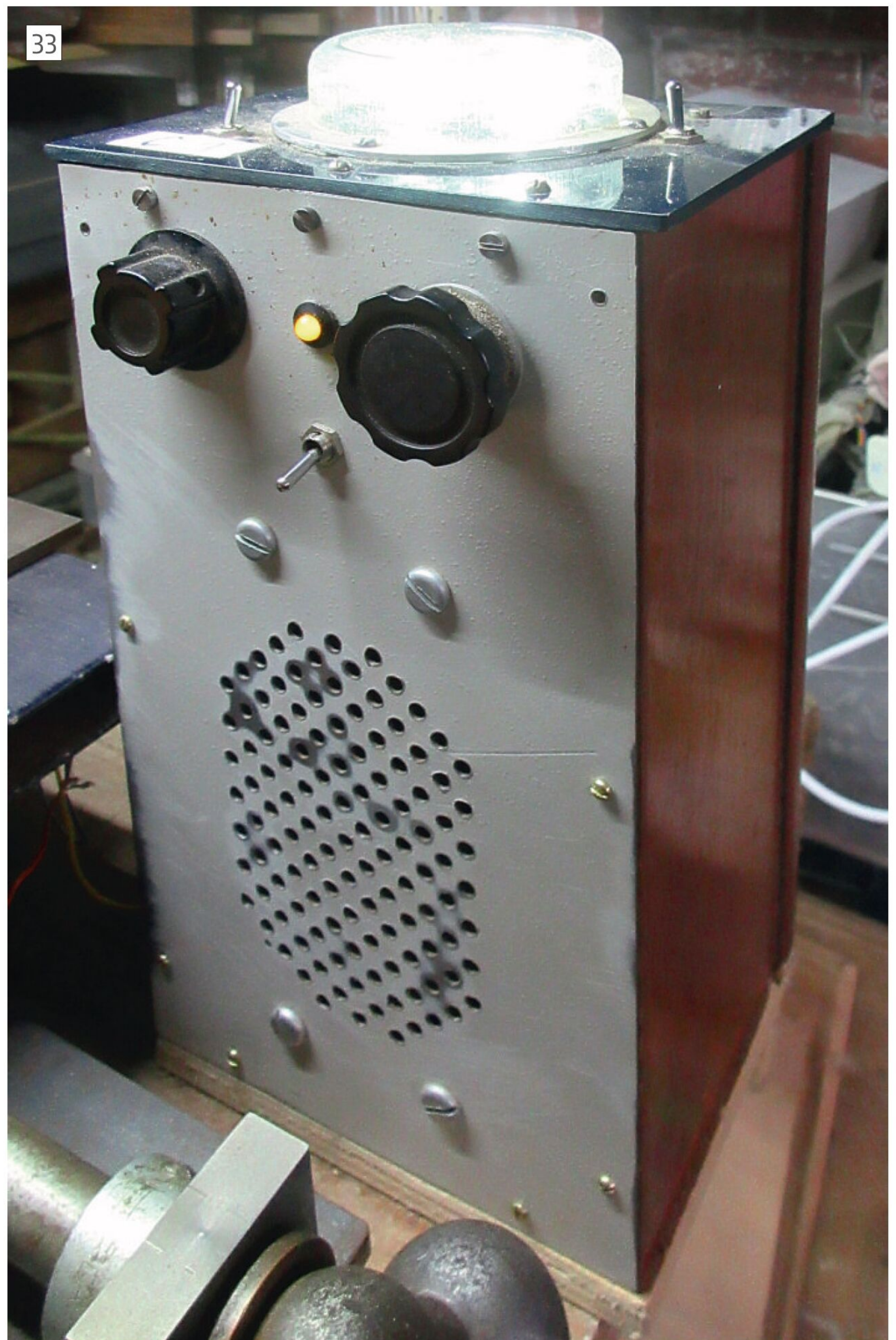
Electrical continuity detector to detect when the follower contacts the template, or the cutter contacts the work piece. The knobs adjust detection sensitivity and volume of the sound emitted
