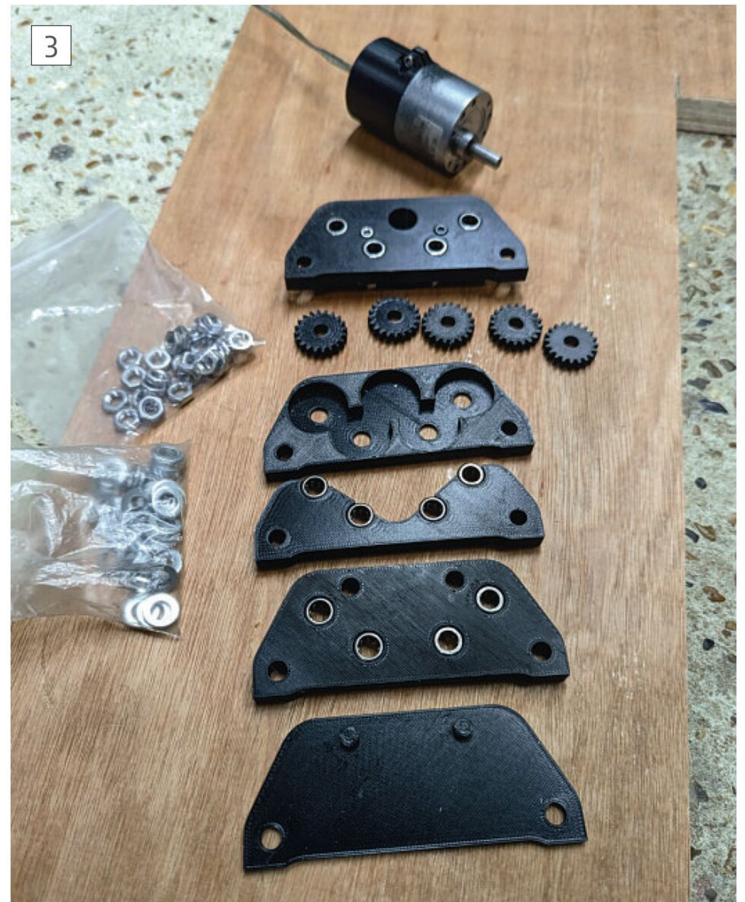
The 3D printed parts and geared motor.
