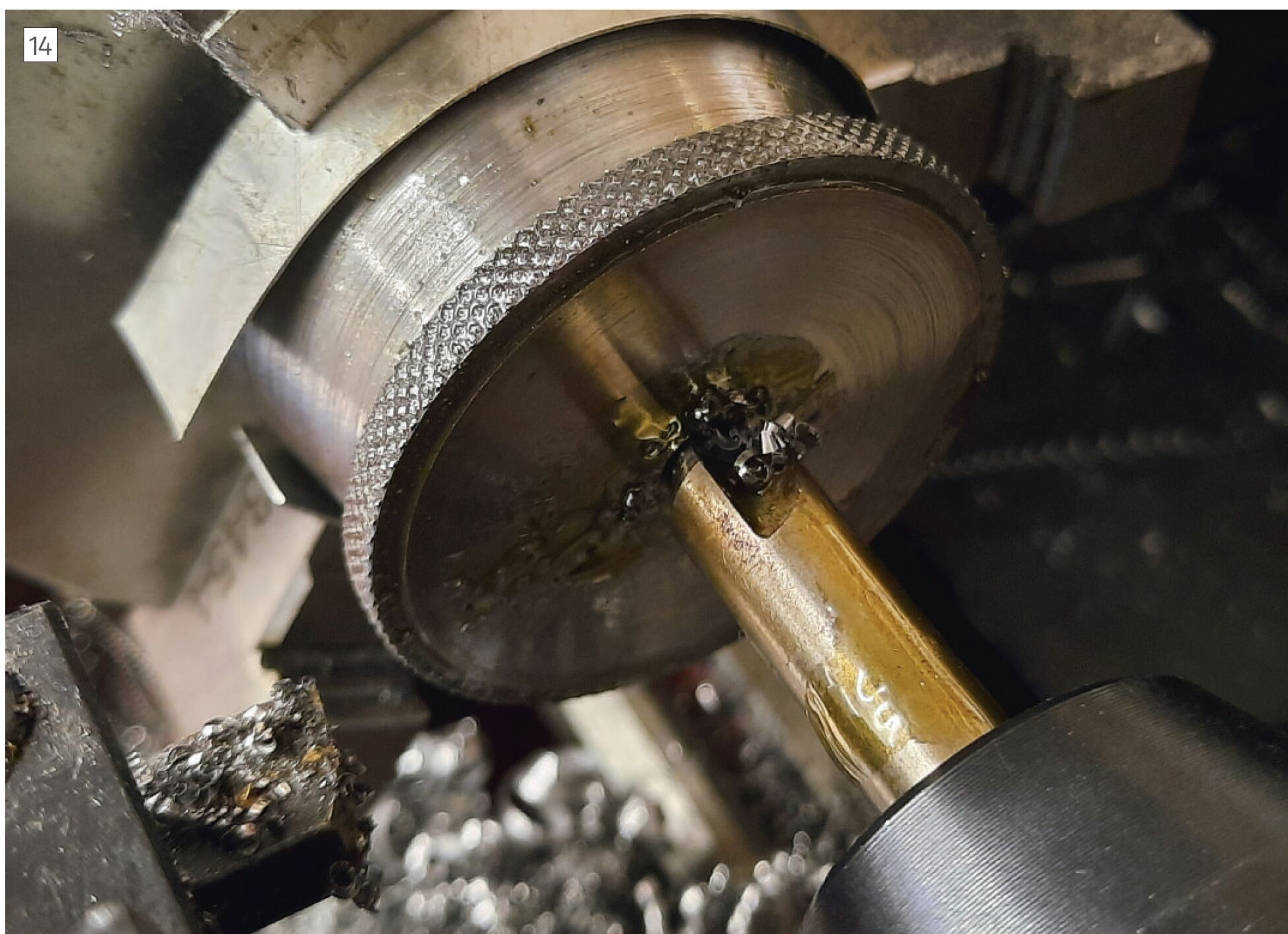
Countersinking the top of the central hole.
