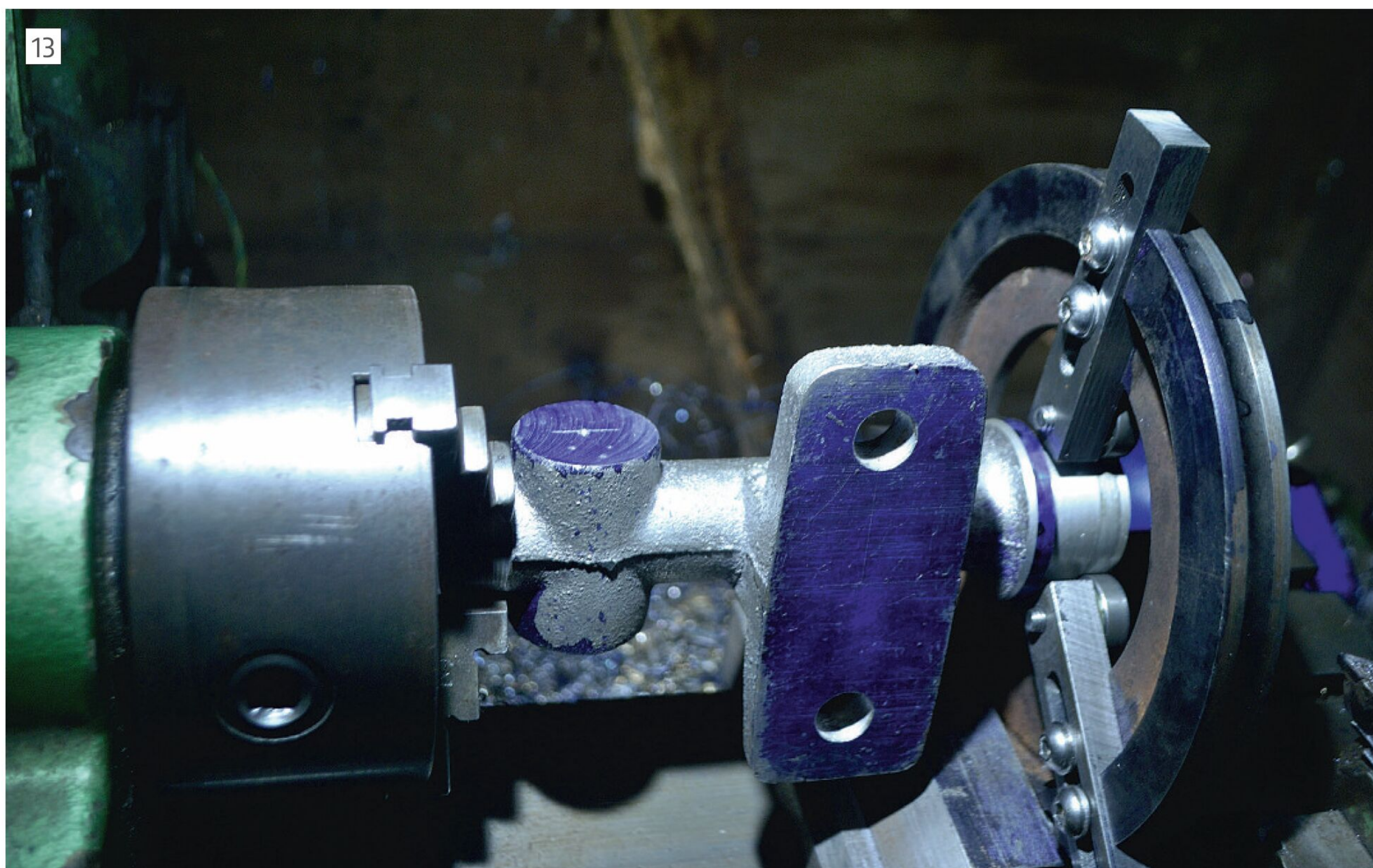
The casting set up ready to bore and ream in the fixed steady.
