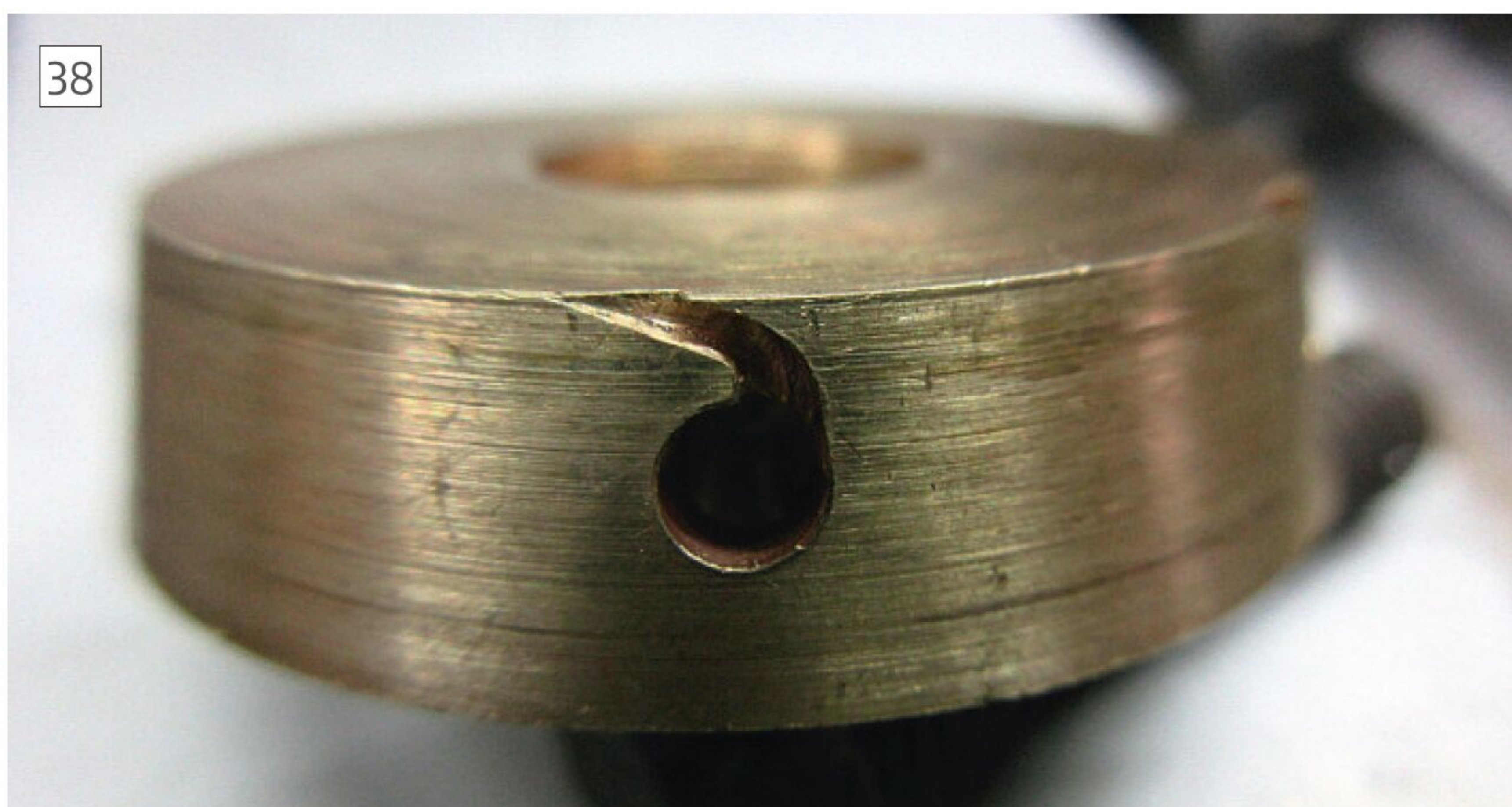
First product made using the contraption were slots cut in the periphery of a tapered disc tapered disc when the disc is inserted into a matching taper a casing ring of the turbine. This nozzle is 0.027 in. wide at its outlet.
