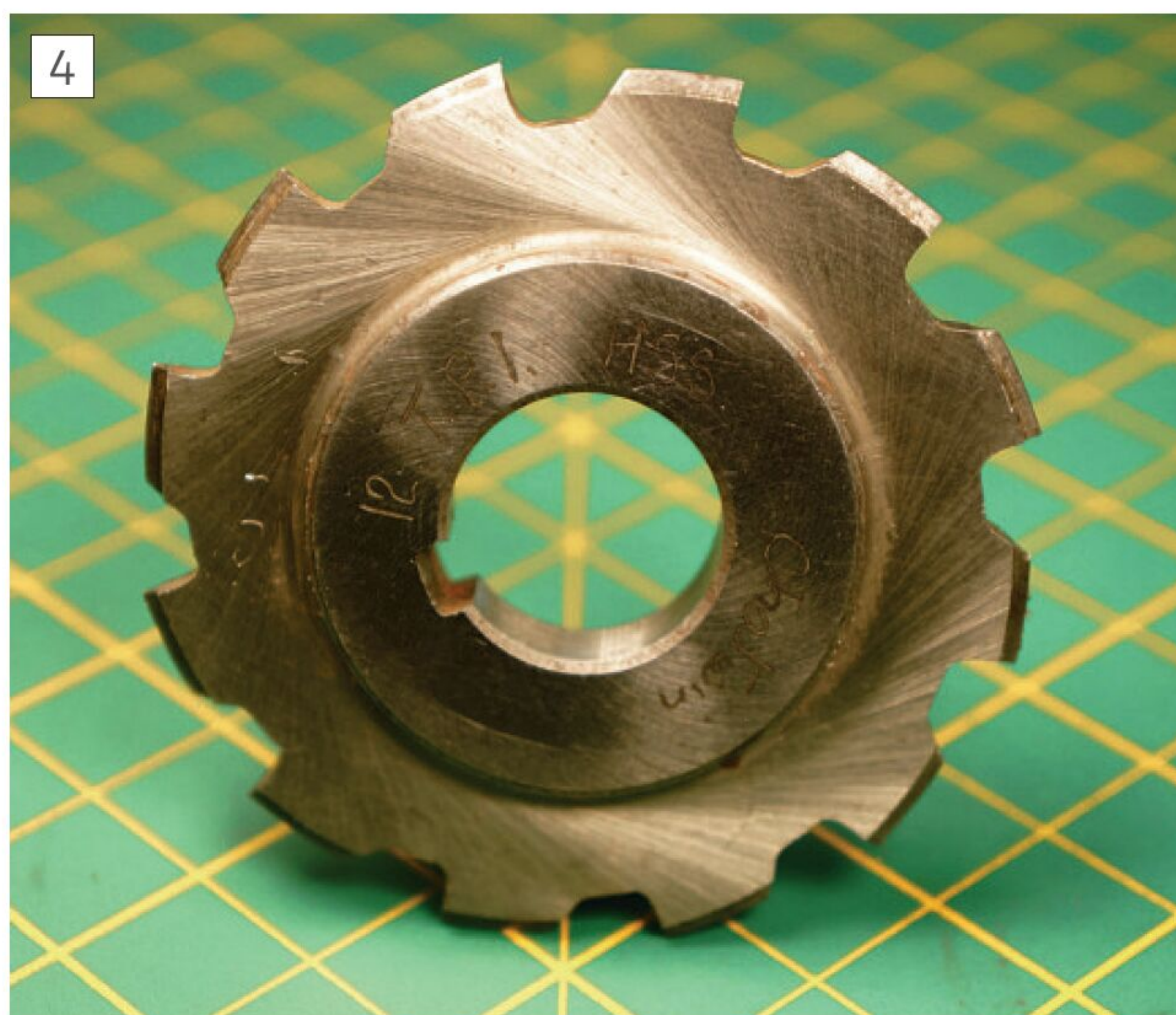
Full form cutter 1/2" Whitworth.
