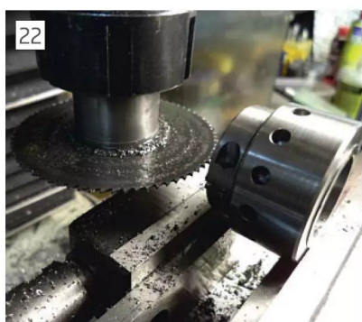
Slitting index ring to make pinch clamp.
