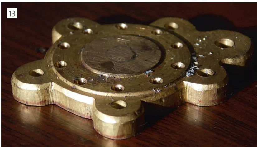
Cylinder base made using filing buttons.
