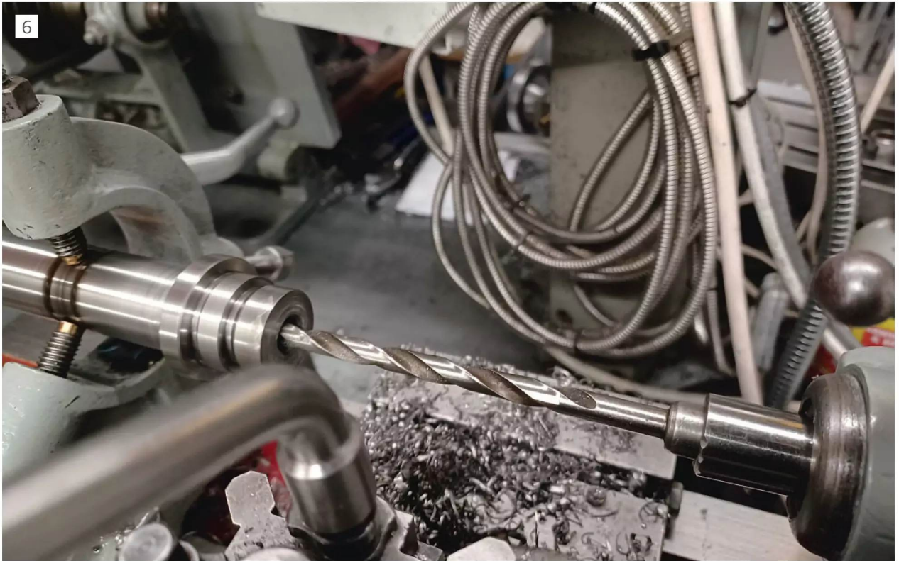
Drilling the spindle.
