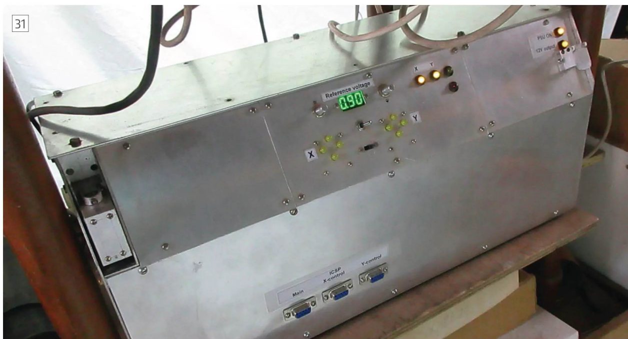
The main electronics case housing the power supply and circuit boards for the master PIC and for PICs that control the stepper motors. The small block set into the left-hand end of the case is a removable memory device.
