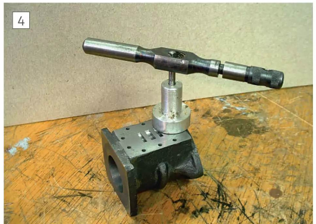
Tapping cylinder face with a guide.
