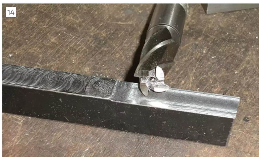
Finish before and after regrind.
