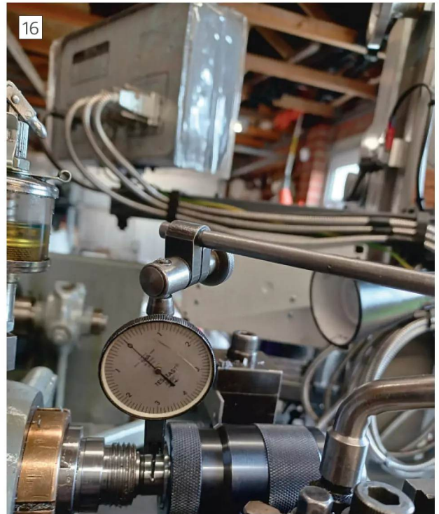
Testing runout of new morse taper.
