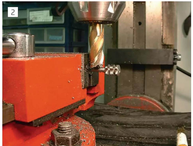
Milling the cutting teeth.
