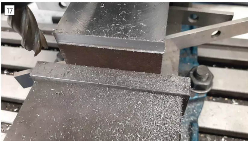
Burrs and crumbly swarf resulting from a blunt cutter
