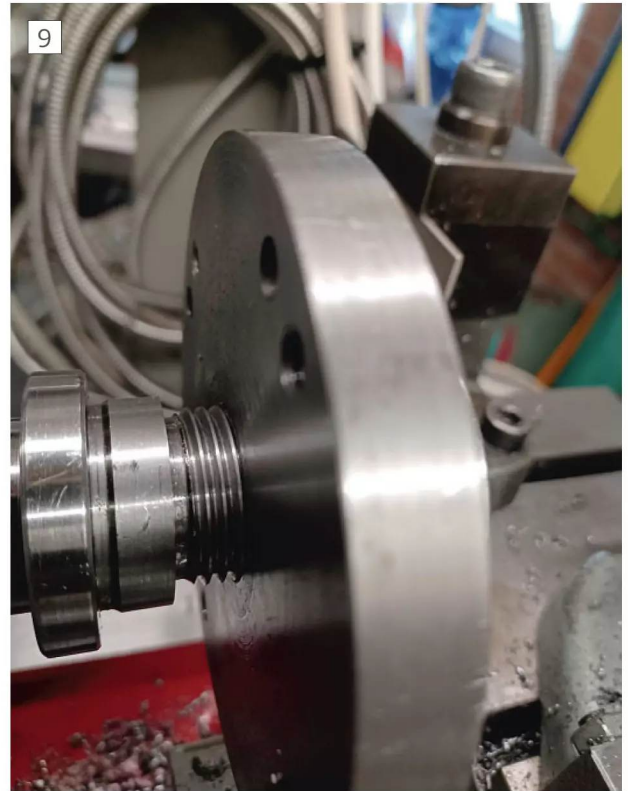
Testing with a chuck backplate.
