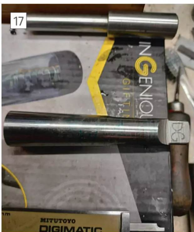
Testing for fit with engineers' blue.
