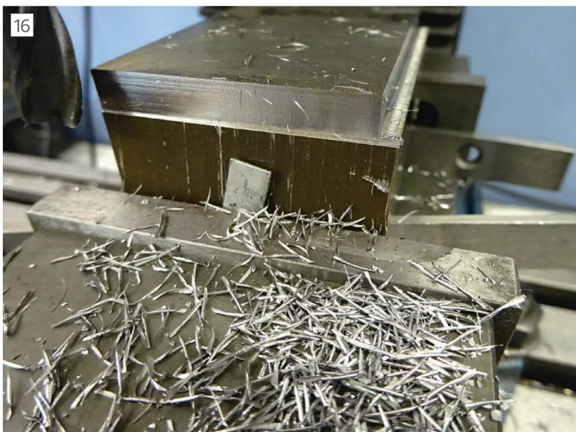
Clean edges and swarf produced by a sharp cutter
