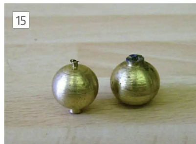
Brass balls made with the form tool.
