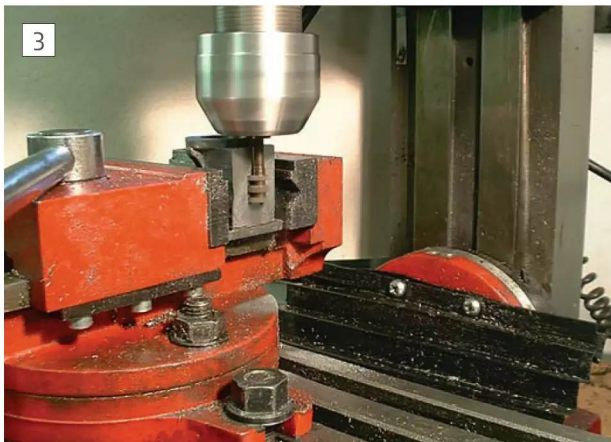
Port milling in progress.
