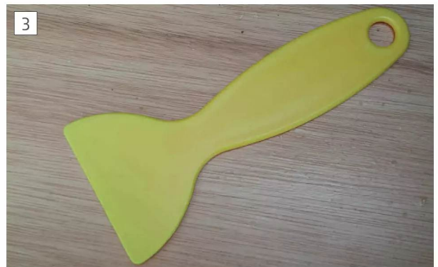
A typical plastic scraper. Do not use a metal scraper on the FEP.
