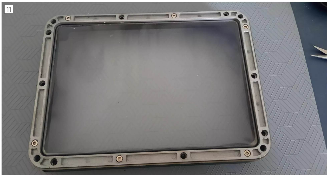
11 All screws fitted and gradually tightened to secure and stretch the FEP.
