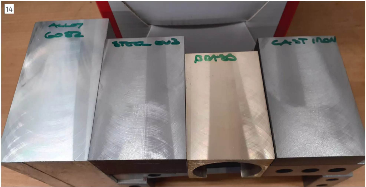
Finish on assorted metals cut with APKT "non-ferrous" inserts
