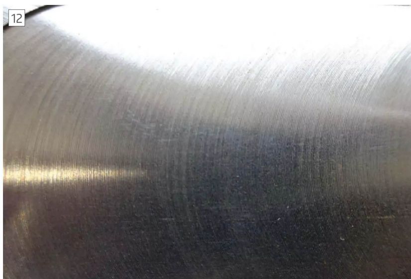
Close up of steel cut with APKT "Polished" inserts
