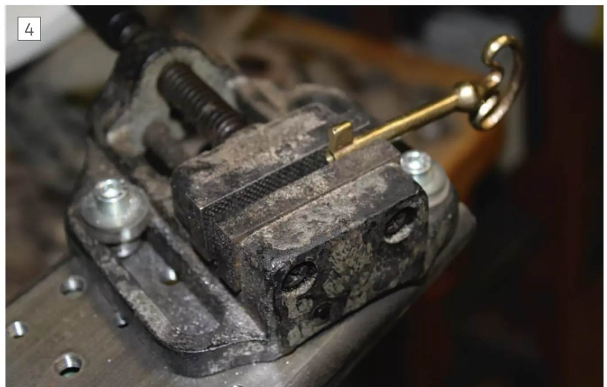
Using as a sub-table for a smaller vice.
