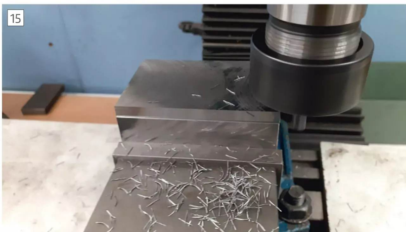
Typical finish from a side cut on steel
