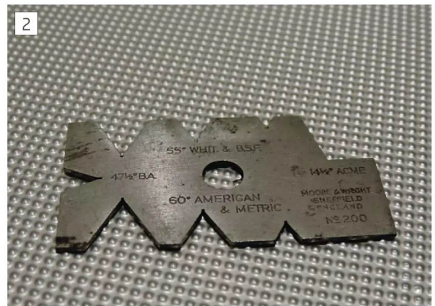
The Moore and Wright screwcutting gauge, note the tiny slots at the tip of each notch.
