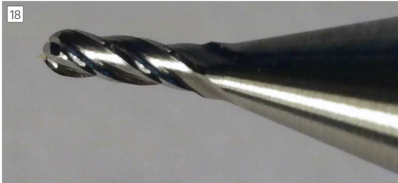
Two-flute ball-nosed Accupro milling cutter, 0.5 mm diameter
