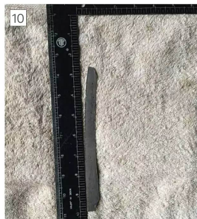
Strip after straightening
