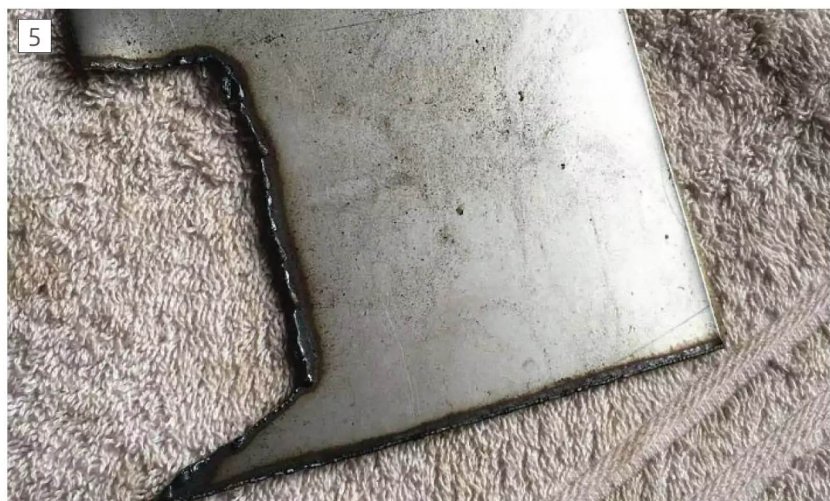
Typical edges cut with plasma cutter
