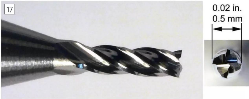
Four-flute square ended Accupro milling cutter, 0.5 mm diameter x 1.5 mm.
