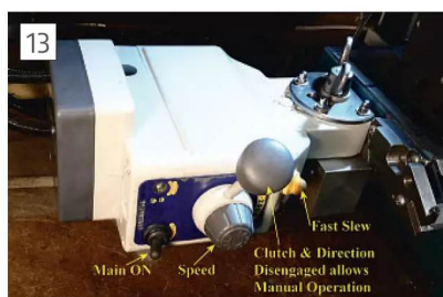
Mounting of Align Power Feed Unit to Ensure Accurate Gear Meshing
