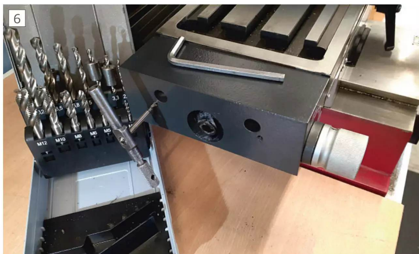
Removing paint from threaded holes
