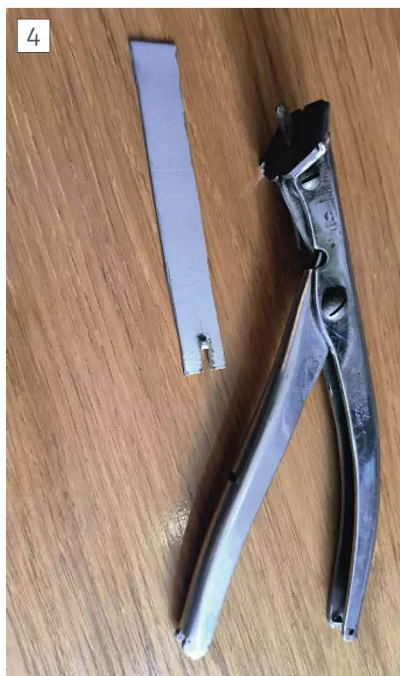
Monodex cutter showing wide kerf and rolled swarf
