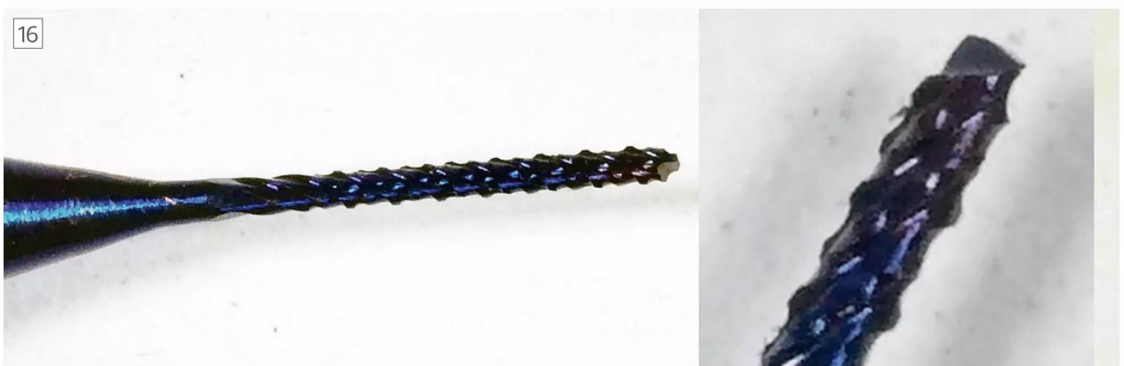
Toothed tungsten carbide milling cutter, 0.5 mm diameter blue nano-coated.
