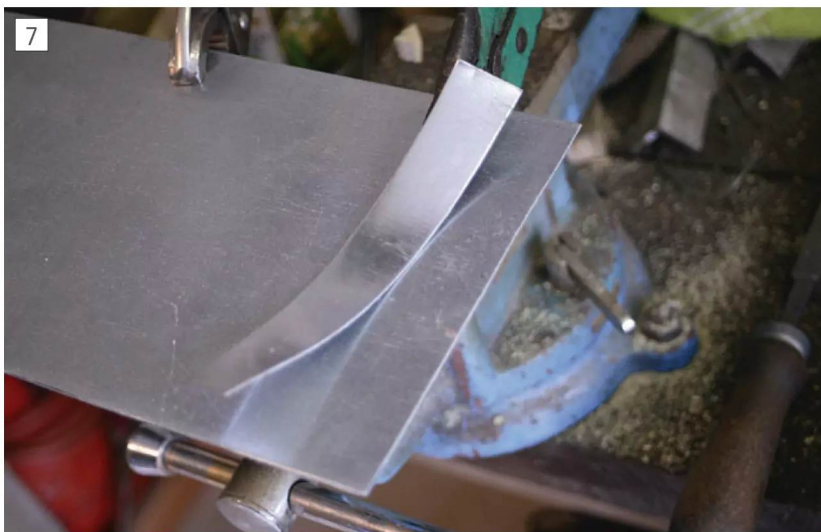
Sample cut using electric shears
