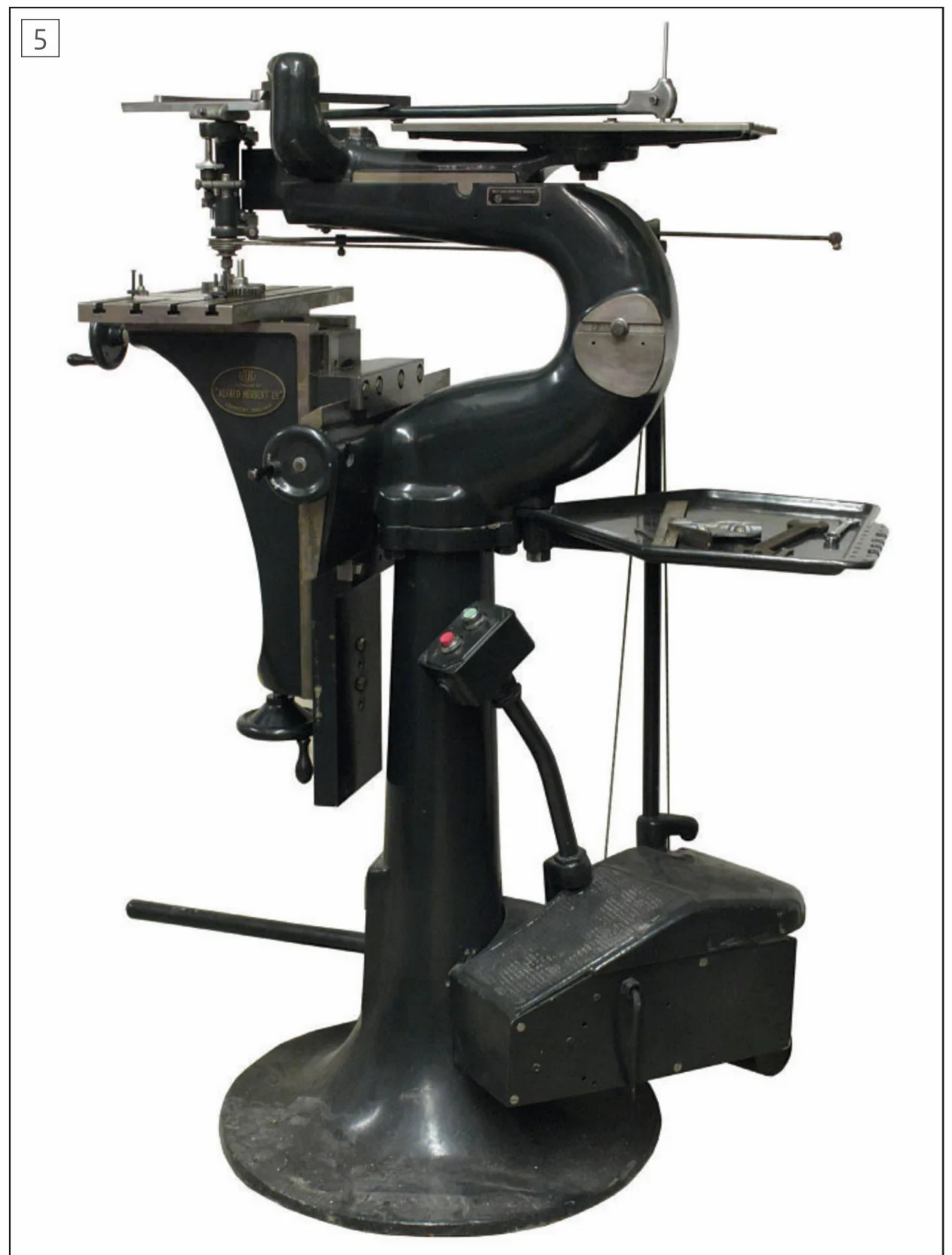
Taylor Hobson type CXL pantographic engraver. (Photo courtesy of David Knight who has an interesting web-site: http://g3ynh.info/index.html )
