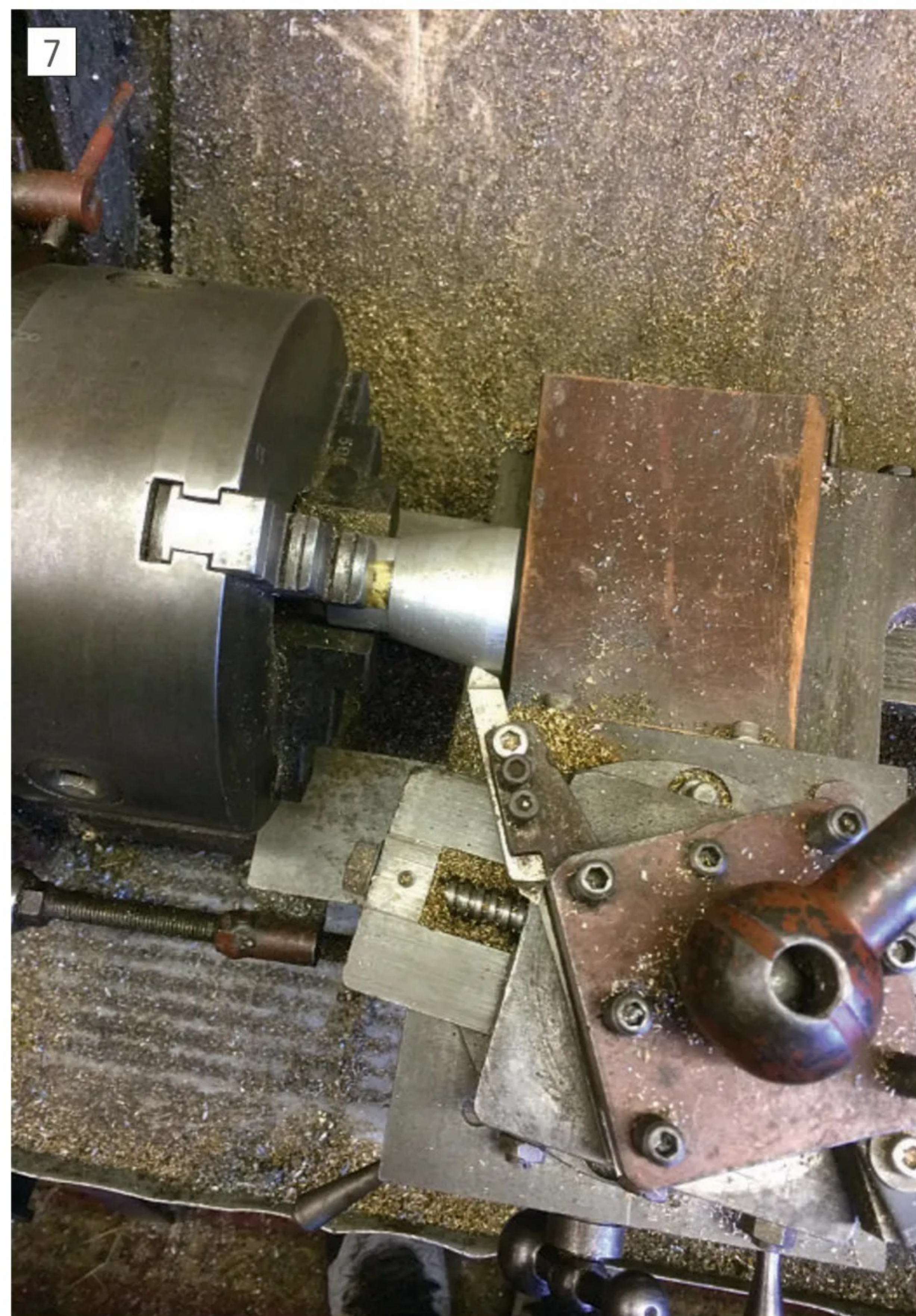
Cutting external taper
