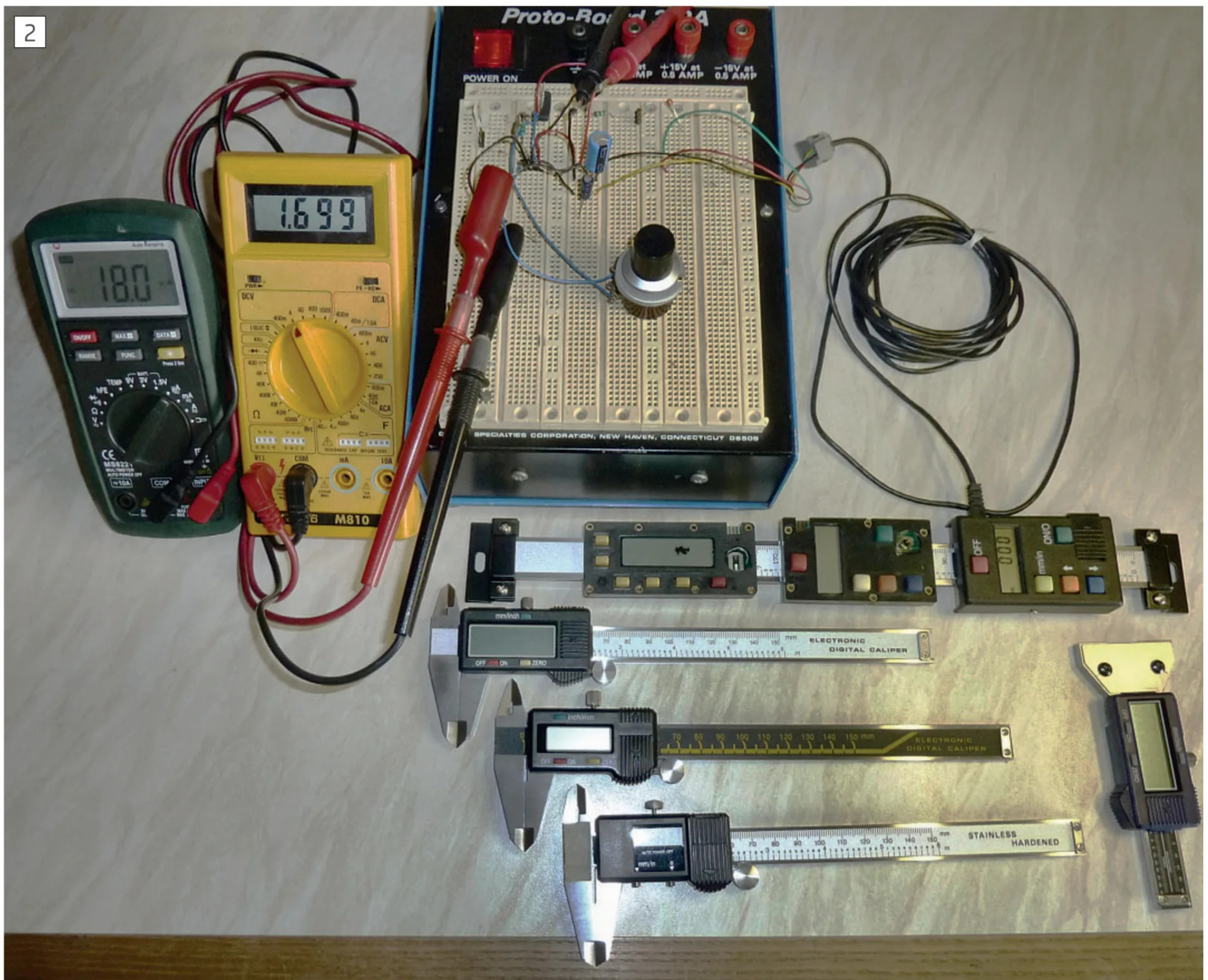
The Scale Units Measured, and the Setup to Investigate the Current Consumed
