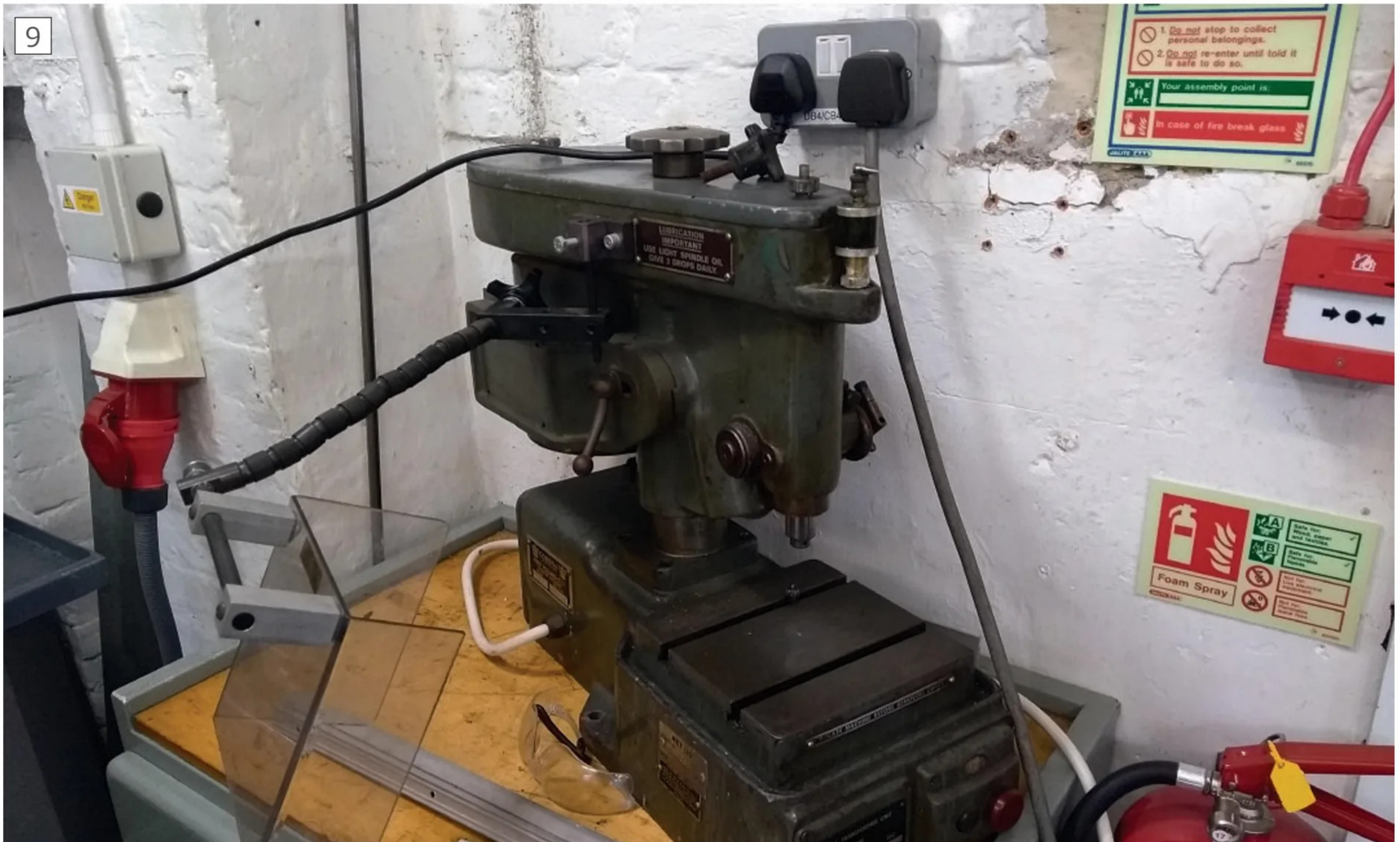
Corona high speed drilling machine.
