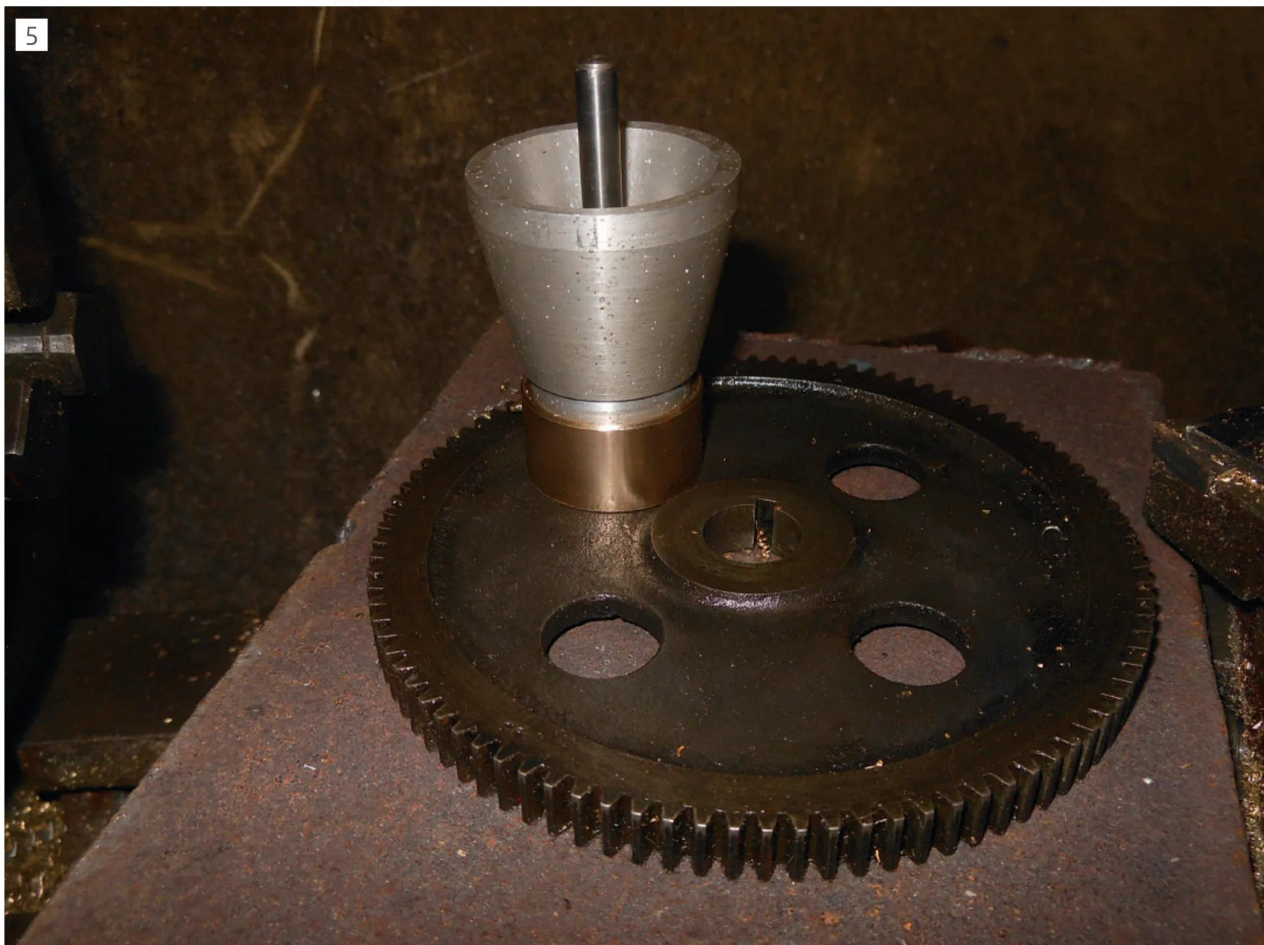
Centring hole. Brass ring ensures finder is kept vertical.
