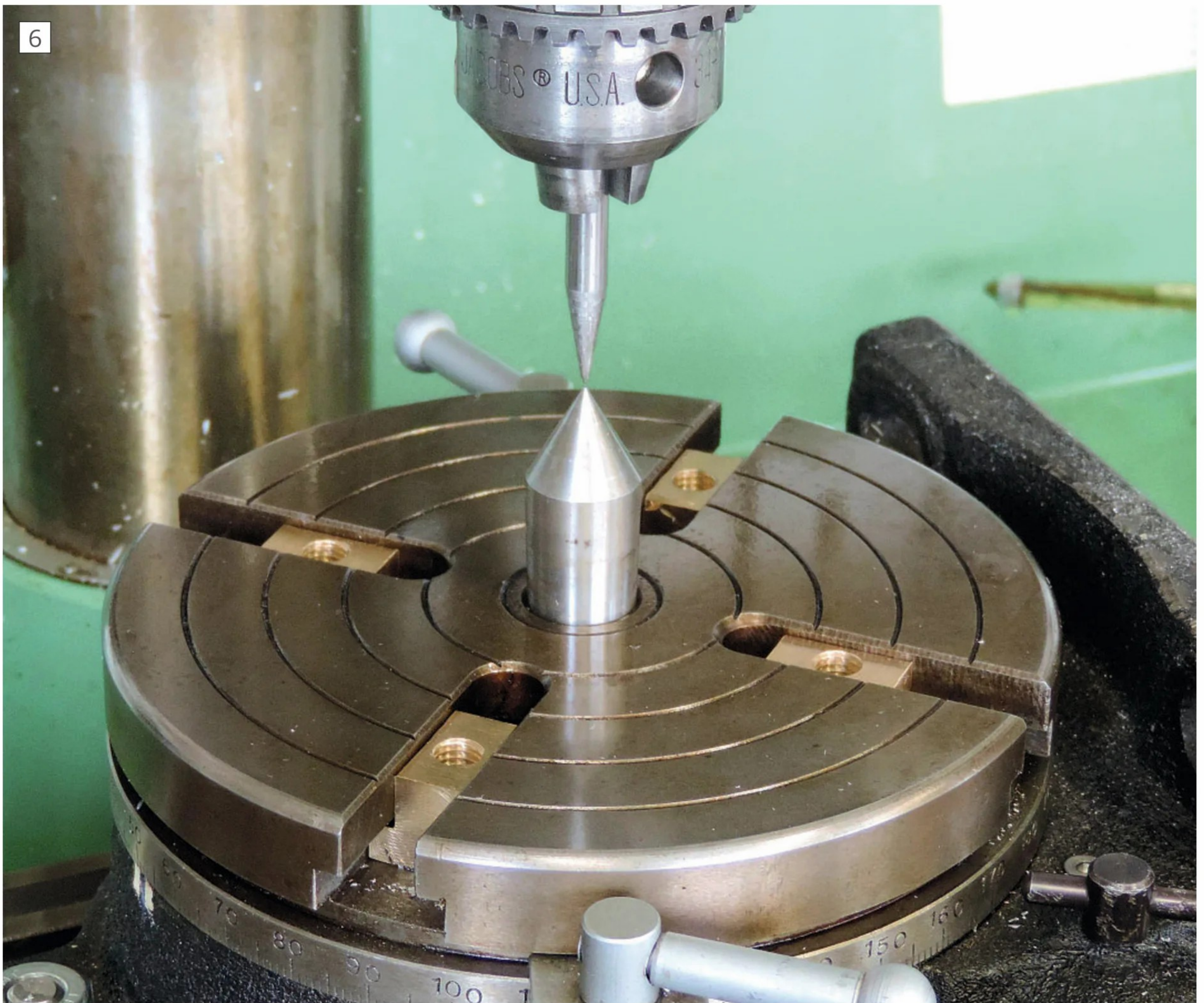
Setting the milling table to the centre of the rotary table.
