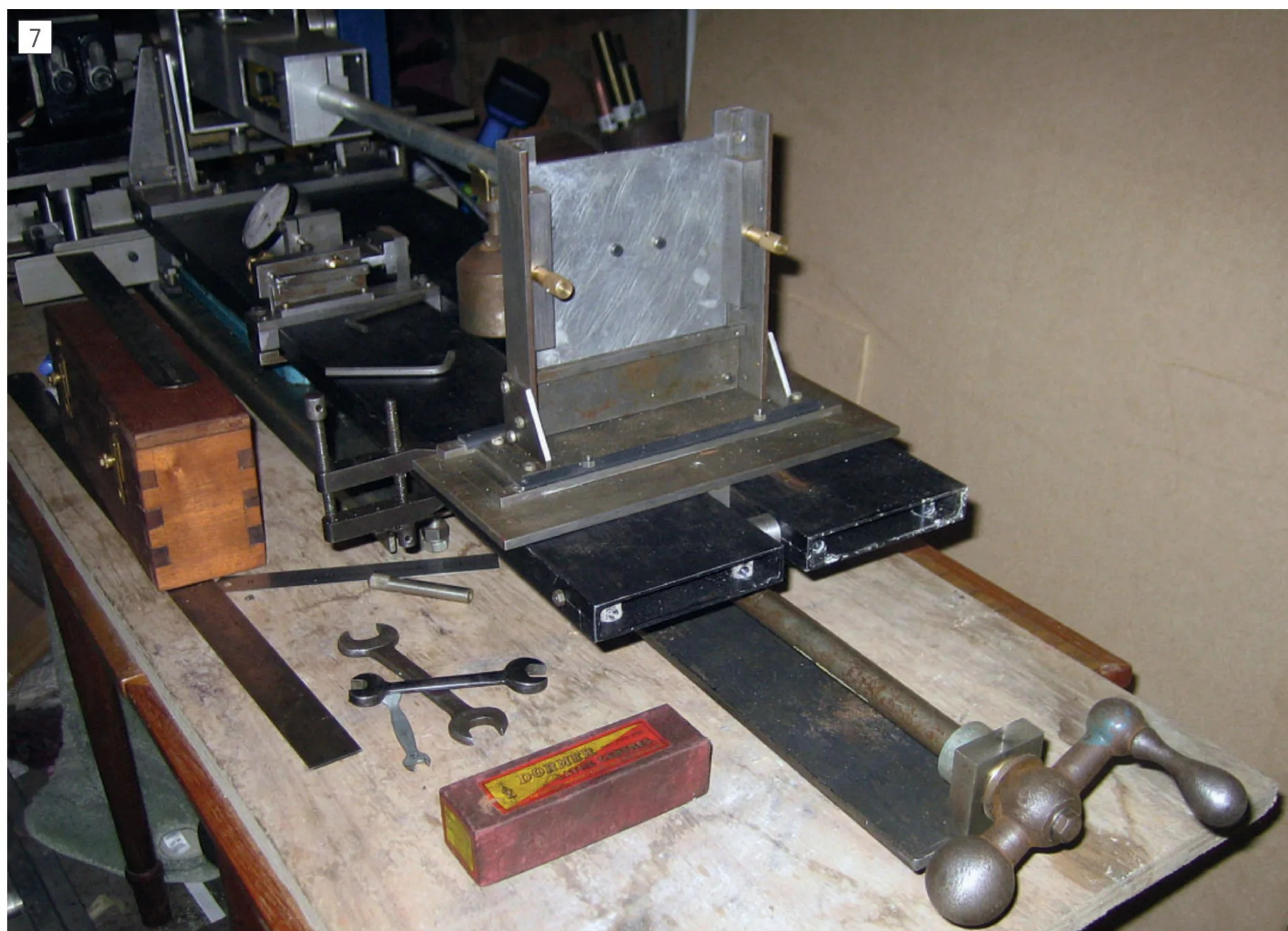
Template holder near the end of the two hollow aluminium planks forming the platform that carries the milling spindle.
