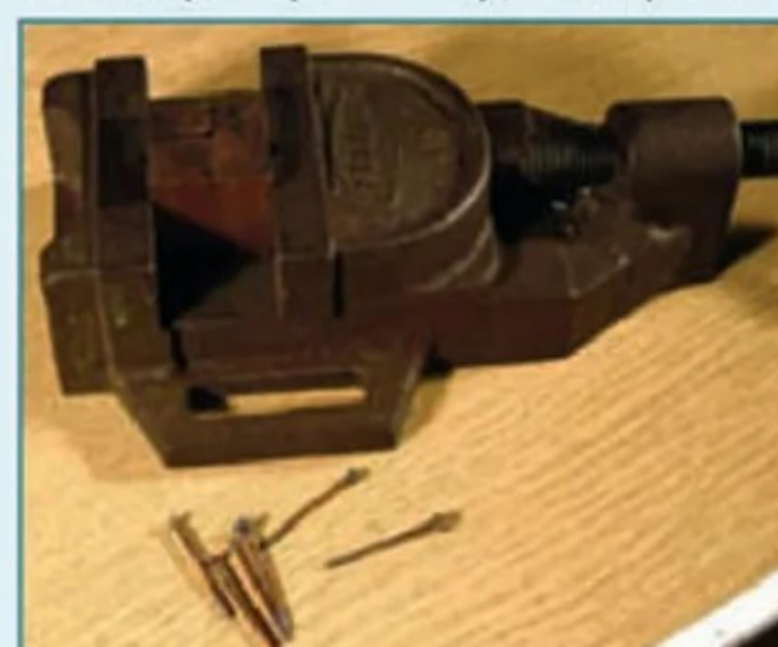
3. Wire clamped in dies ready for application of welding torch.
