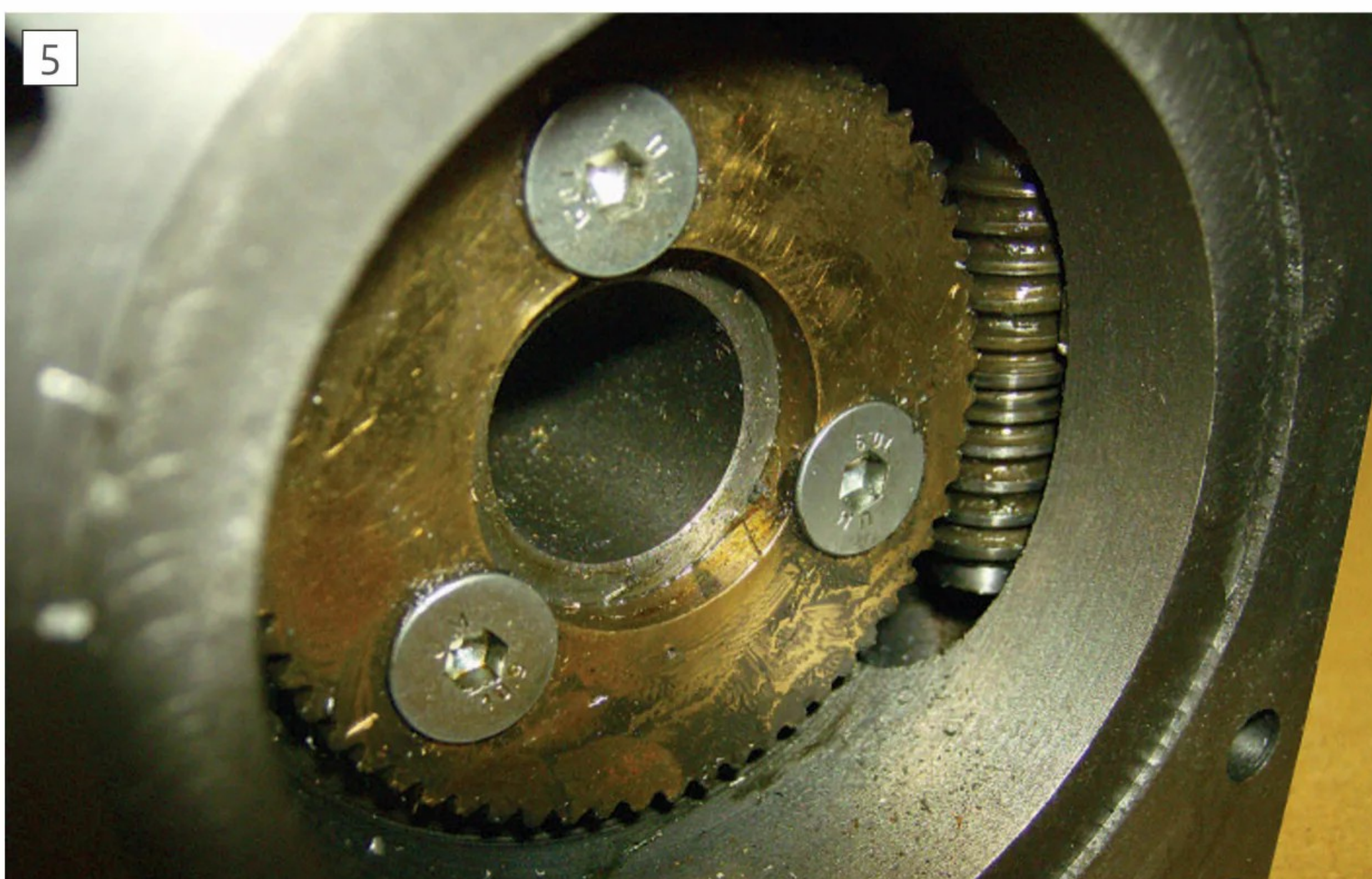
Shop made 60:1 worm and wheel in a rotary table.
