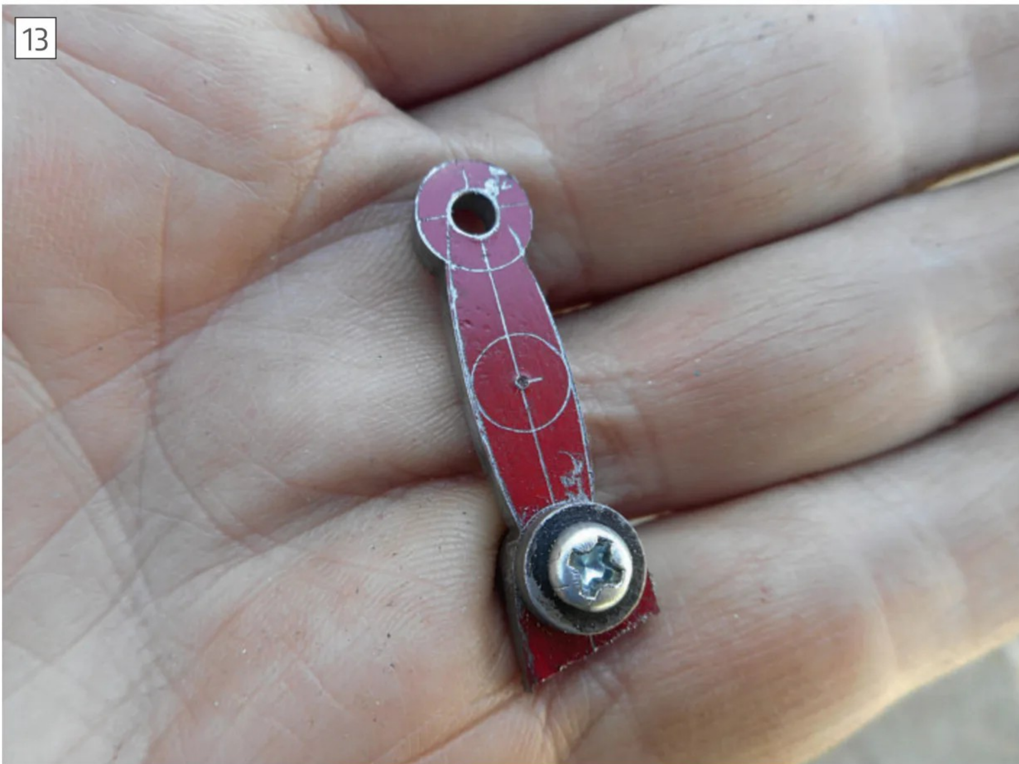
Filing button in use on the connecting link after the fish-belly was filed down to the markout line.
