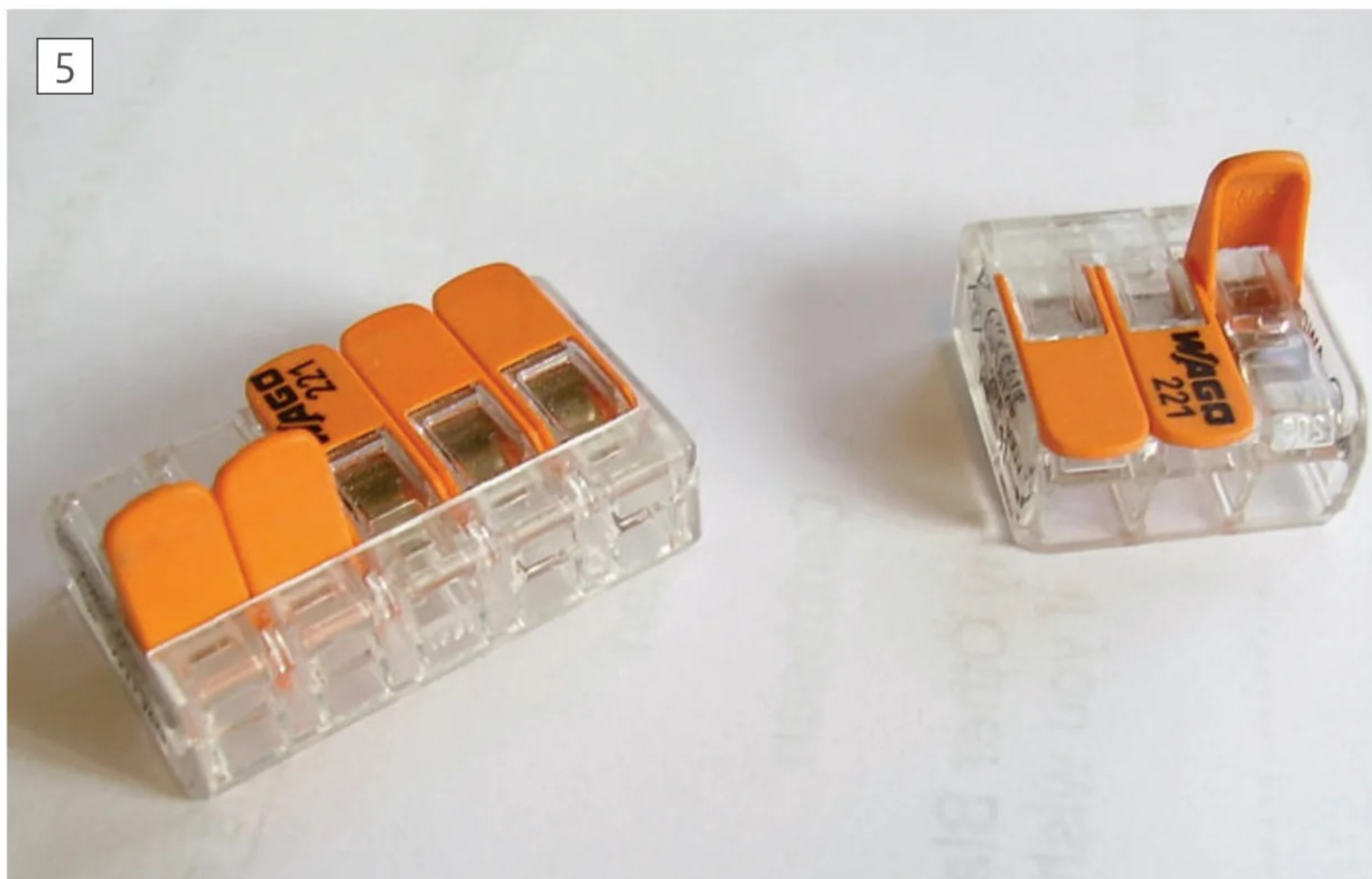
'Wago' connectors – lift the lever, insert stripped wire and close lever.
