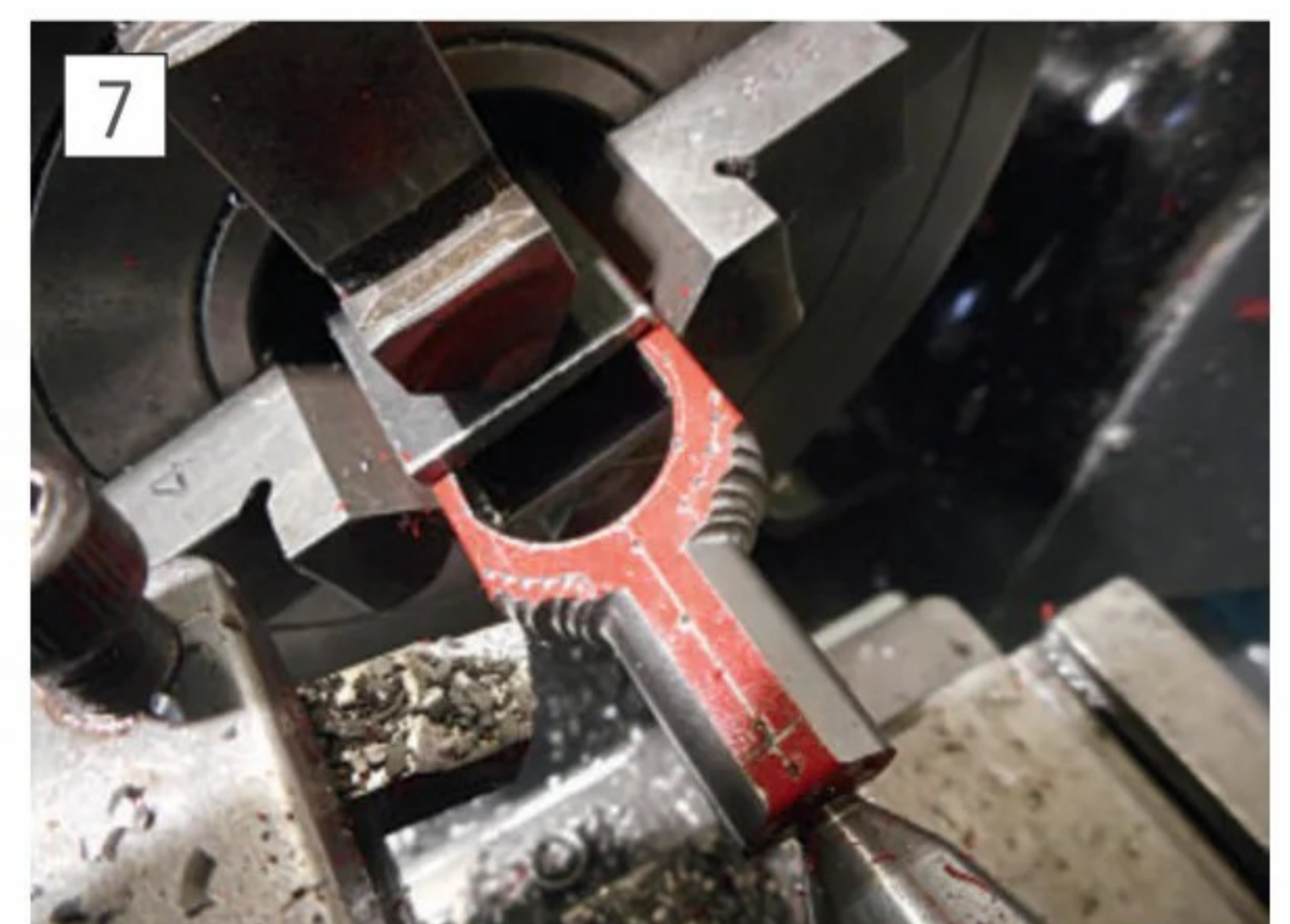
The block's outside profile is turned down to the line in rough steps.
