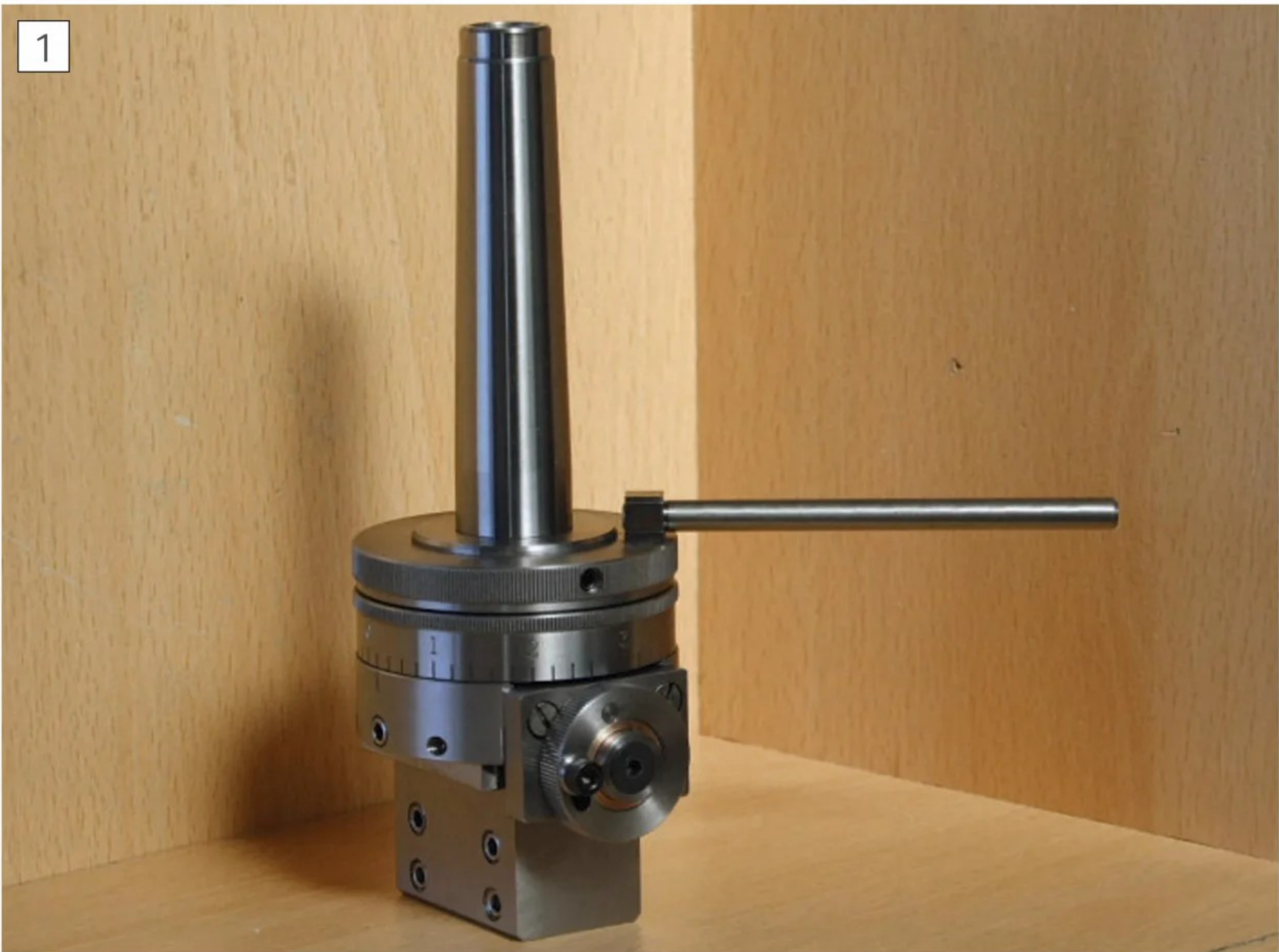
The new boring head
