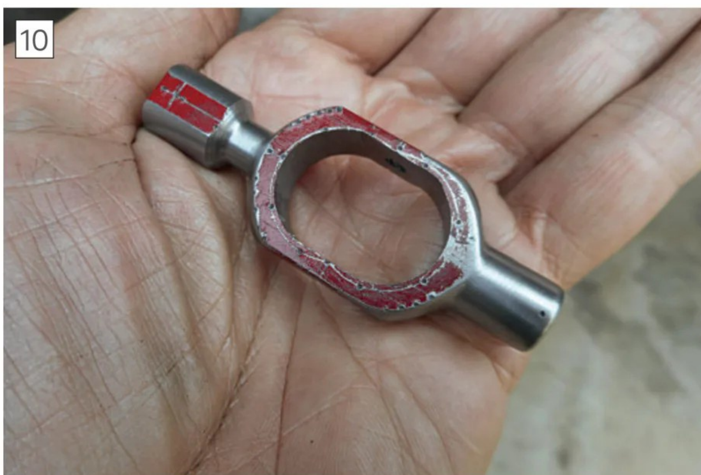
Machining very close to the markout lines is possible, ready for final hand finishing by file and emery cloth.
