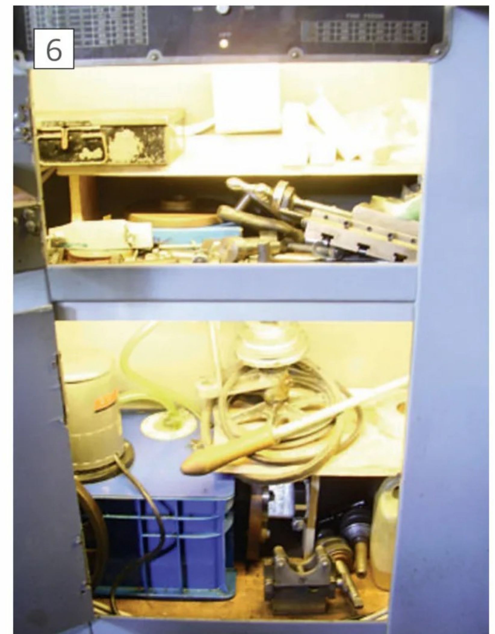
Lighting installed on lathe.
