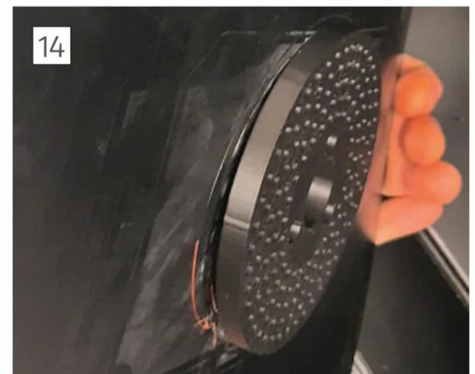
Peeling a division plate off the flexible bed.
