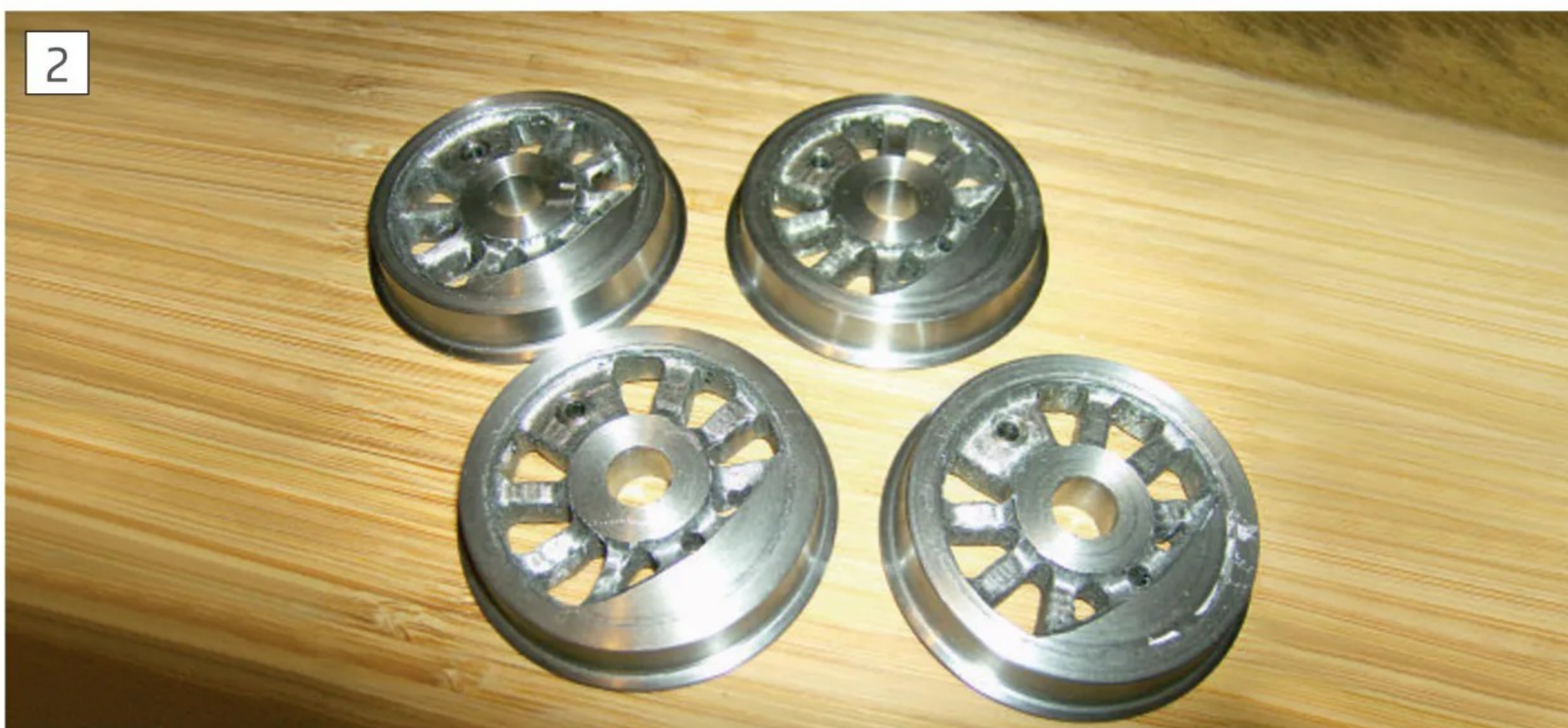
2 Fabricated wheels made using a rotary table.
