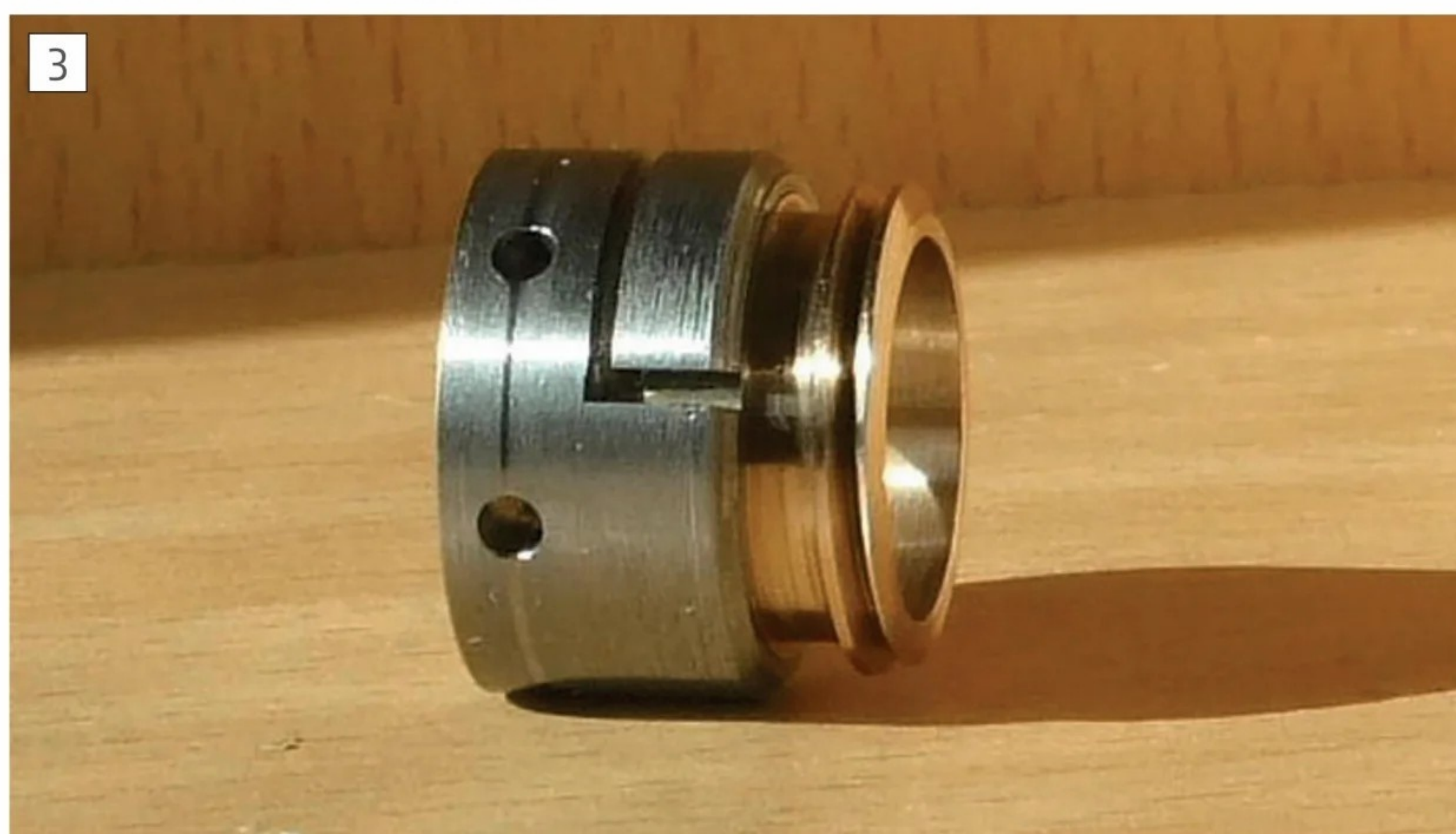
Composite worm silver steel and phosphor bronze.
