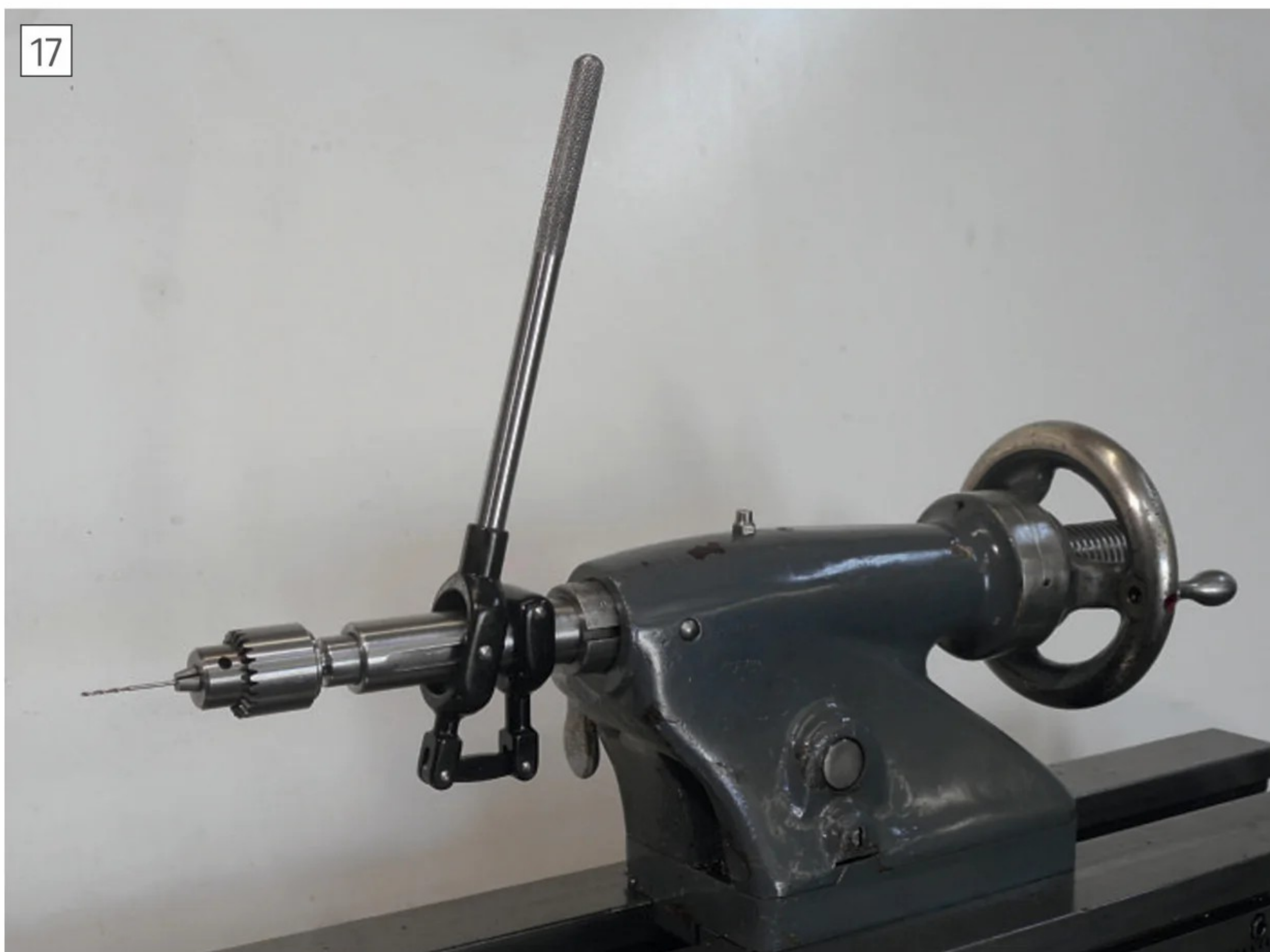
All the style of the jazz age: The sensitive driller matches the Myford's classic lines but would be just as useful on a modern machine.
