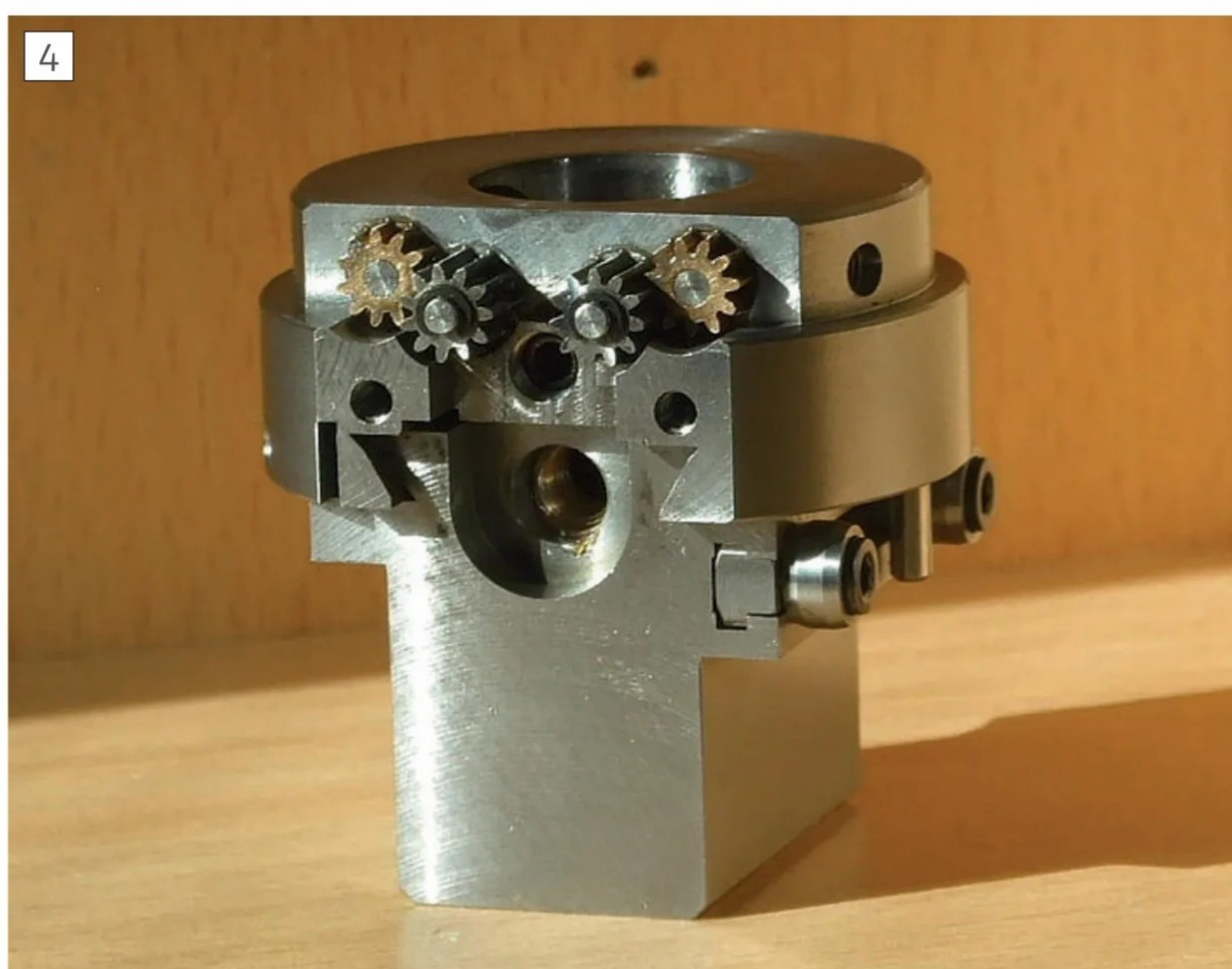
Output gears and idler gears note E-clip positions to miss endplate.
