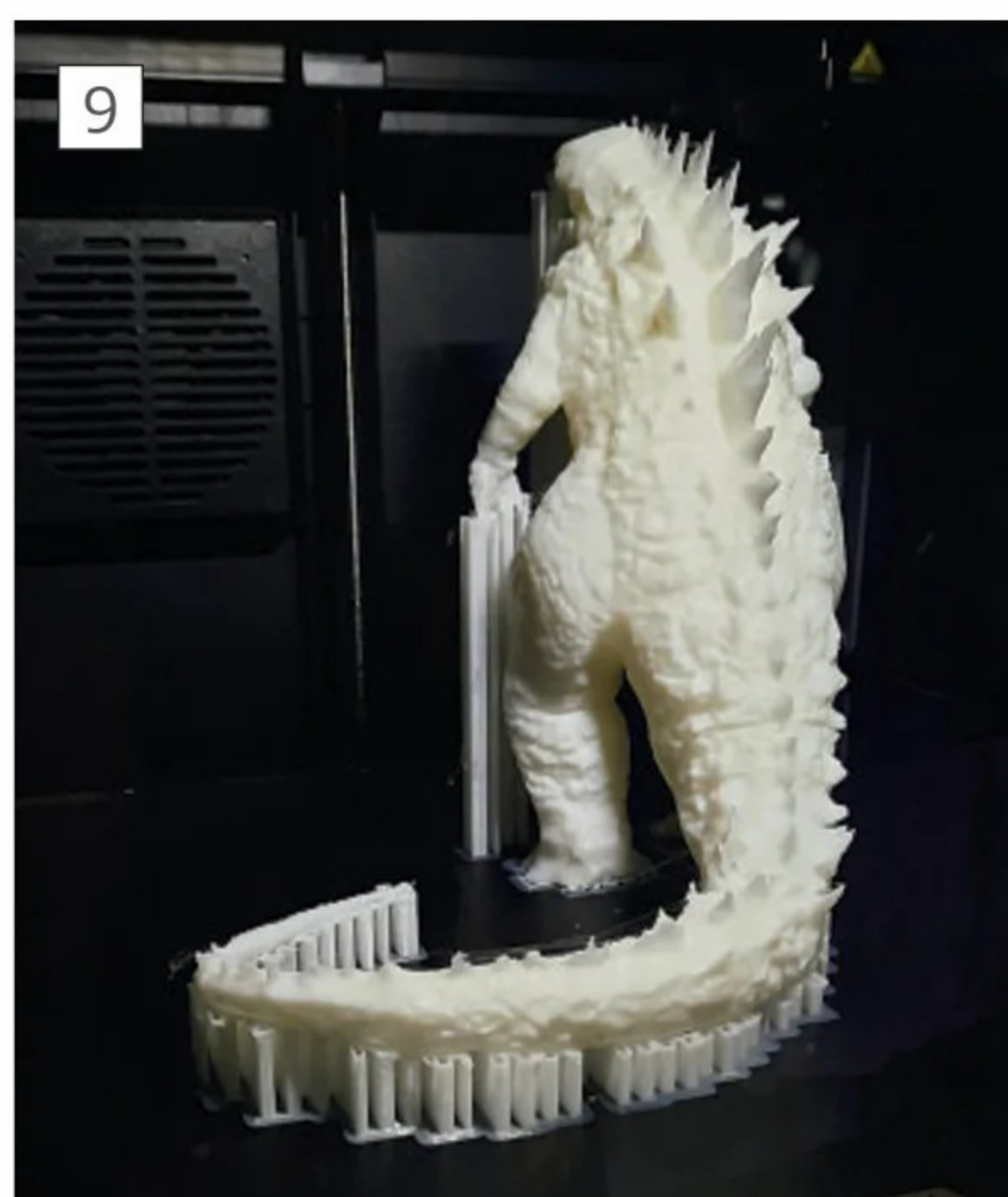
This print used about 200mm of the available 300mm build height.
