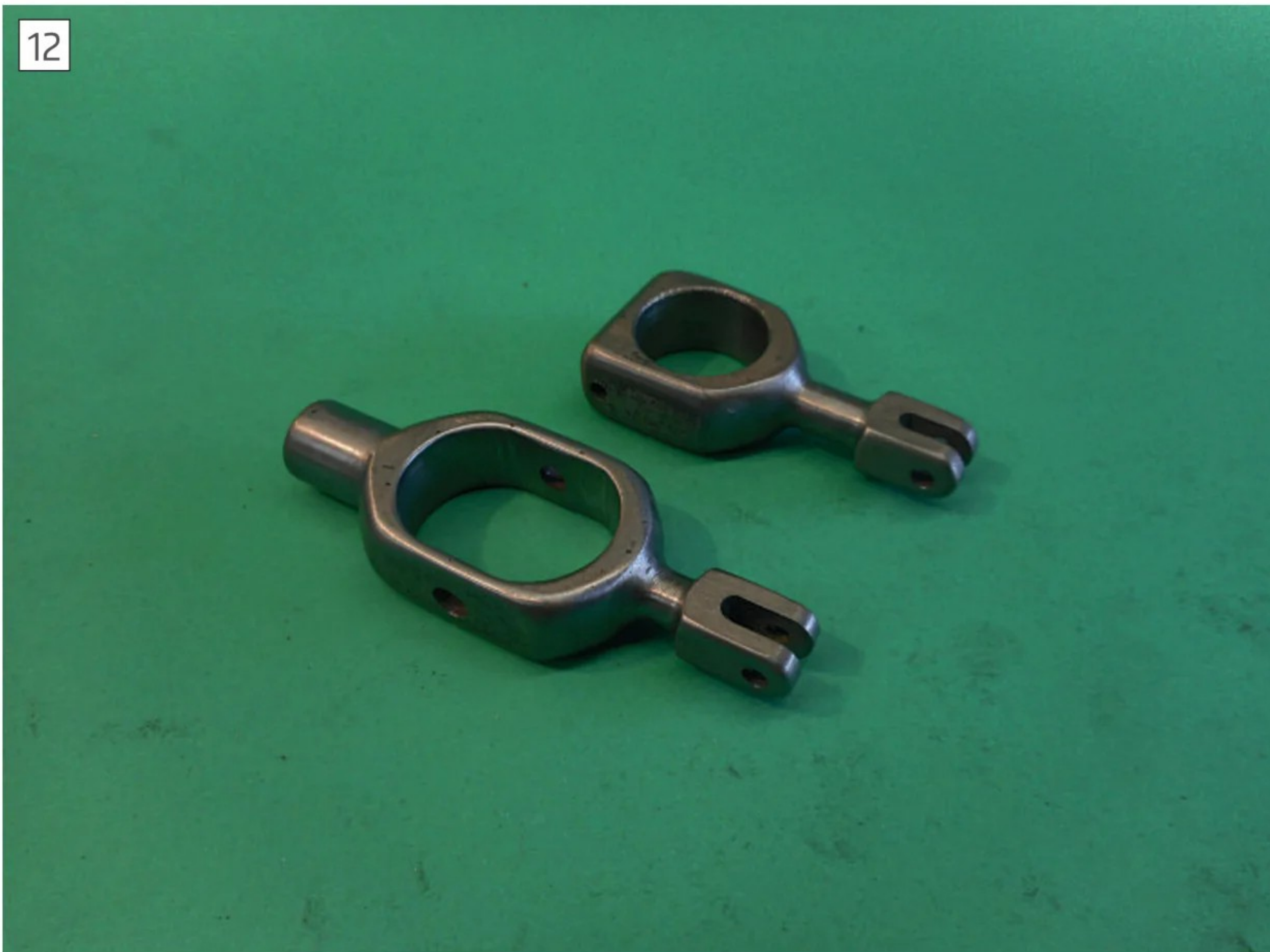
The finished actuating lever link and fixed member have the clevis ends rounded by use of hardened filing buttons.
