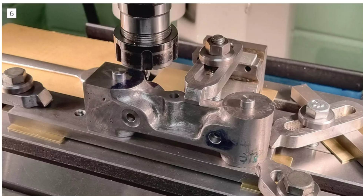
6 Drilling the clamp pad anti-rotation pin holes in the sensitive drilling arm.
