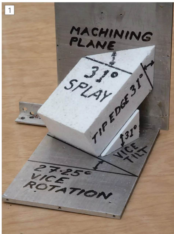
Trialling the angles with a polystyrene block.
