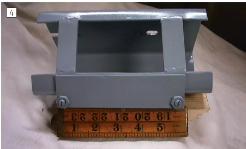
The front face of the angled fixture with 'gib' screws
