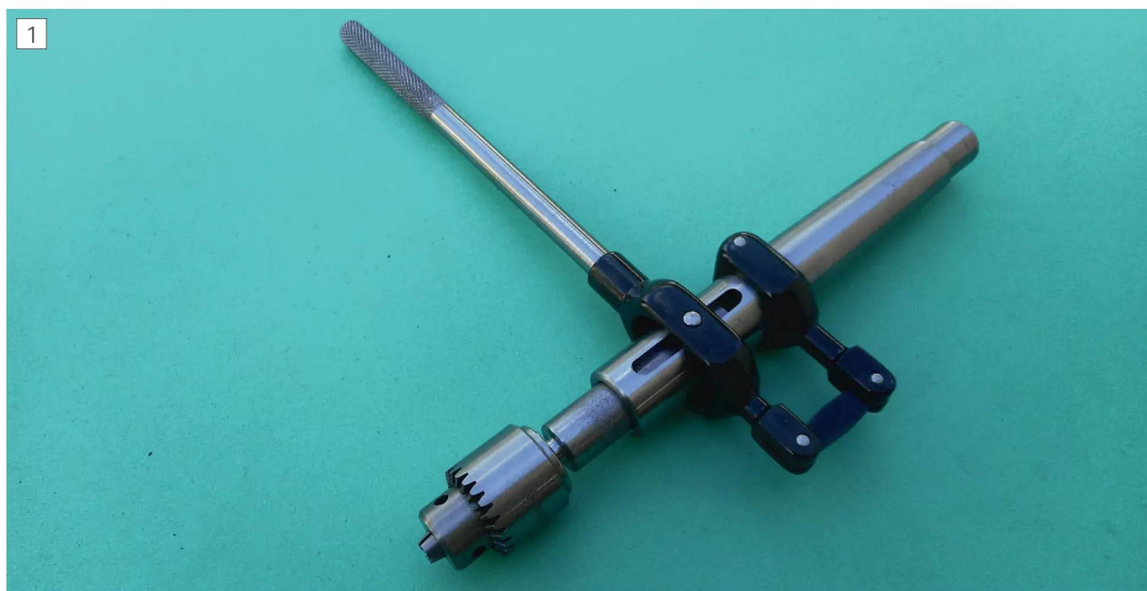
The sensitive drilling attachment provides force but fine control via its lever handle
