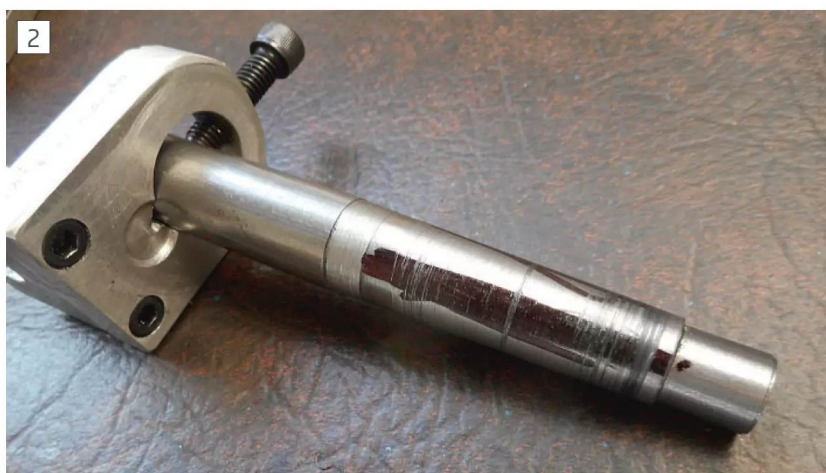
Felt pen marks show contact along full length of the taper before finishing cuts are taken
