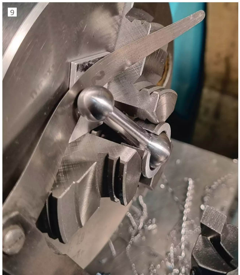
Setting up ball handle for boring spindle hole at correct angle.
