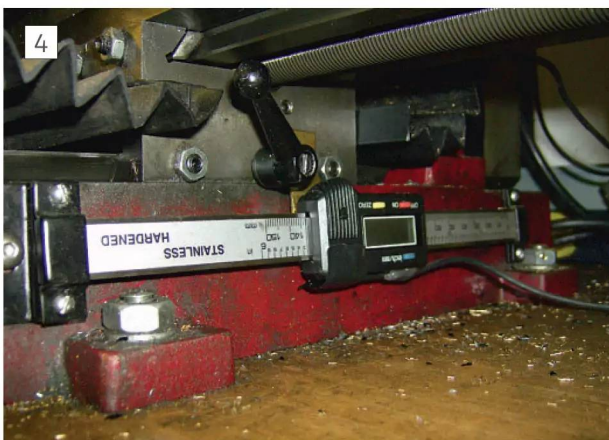
X-axis readout attached to base of mill.
