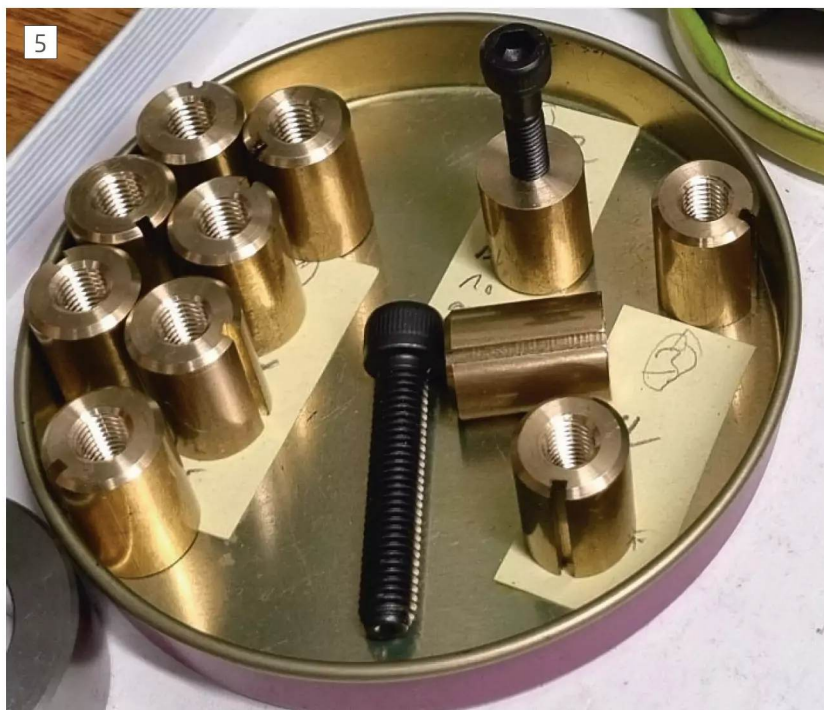
5 Grooved clamp pads ready for temporary insertion into arms for machining pillar matching radius. The quantity of clamps shown in the image exceeds the number required for the project.
