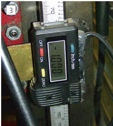
Cable soldered in place and sealed with hot melt adhesive.
