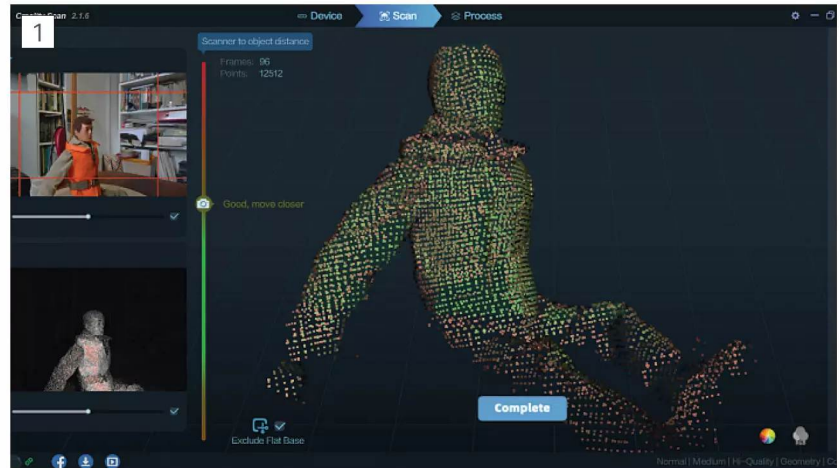
Using the Scan Ferret in Creality Scan. At left are the visible light and infra-red depth images, to the right is the emerging point cloud.
