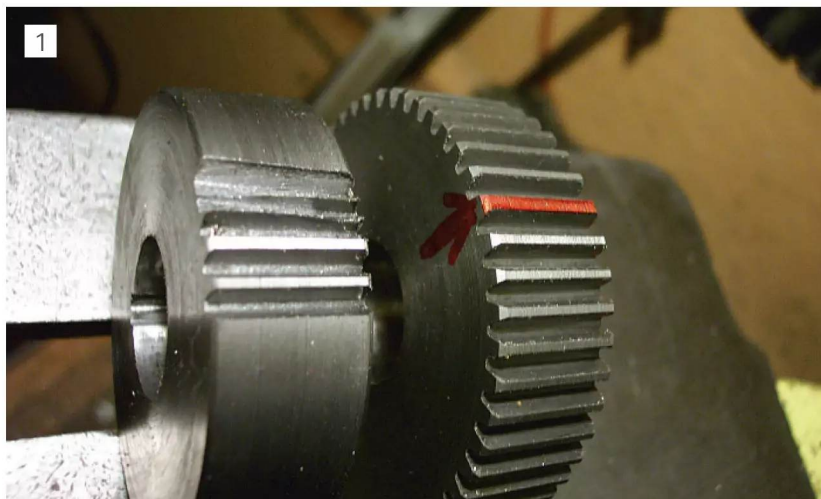
Fat gear tooth, the reason for making this fixture
