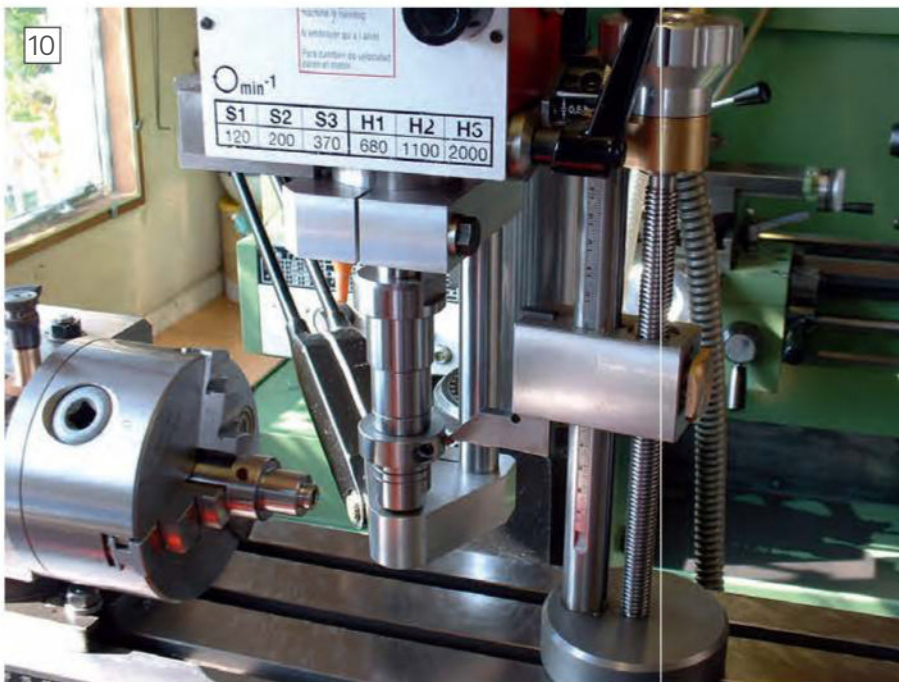
Setup for single point cutter.
