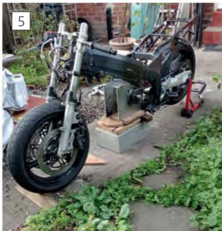
Offering the engine up to the frame.
