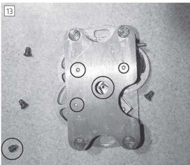
Reverse side of the movement showing oiling points.
