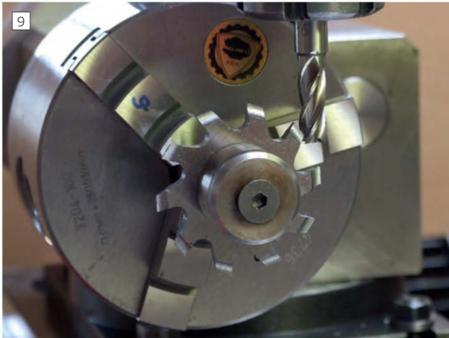
Using milling cutter to approximate a circular involute cutter.
