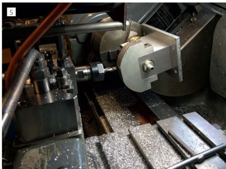
Milling quadrant on the lathe.
