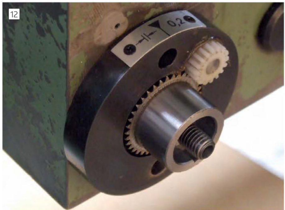
Dial backplate with one gear and pinion visible.
