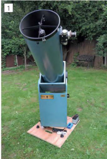
1 Telescope mounted on the equatorial platform
