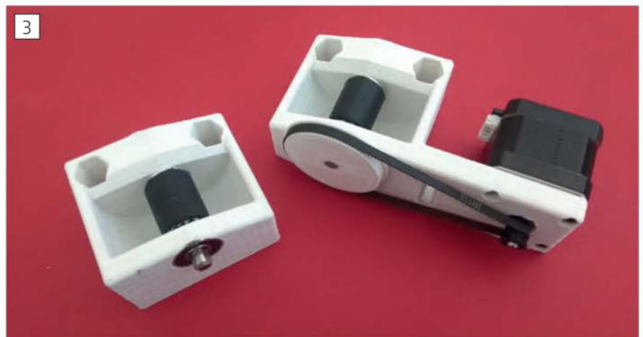
3 The roller boxes showing the platform drive.
