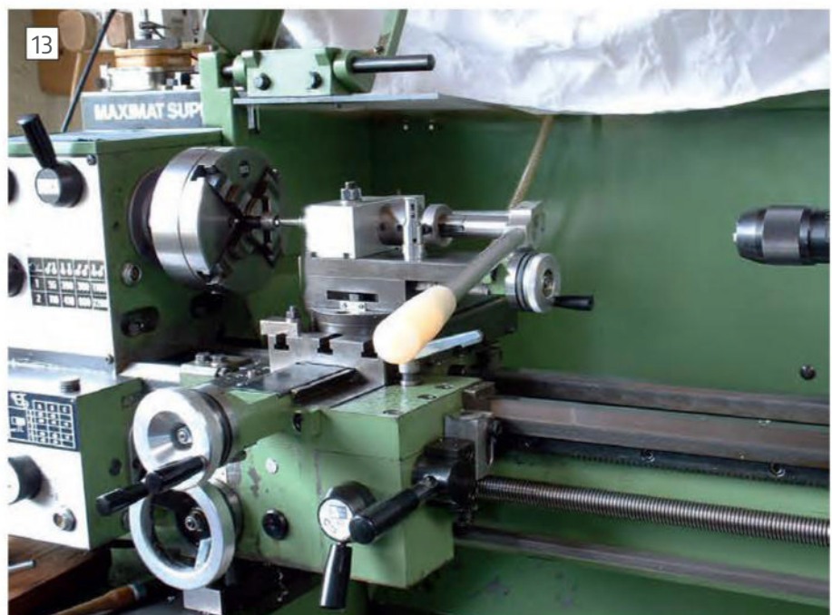
Using lever attachment to cut keyway.
