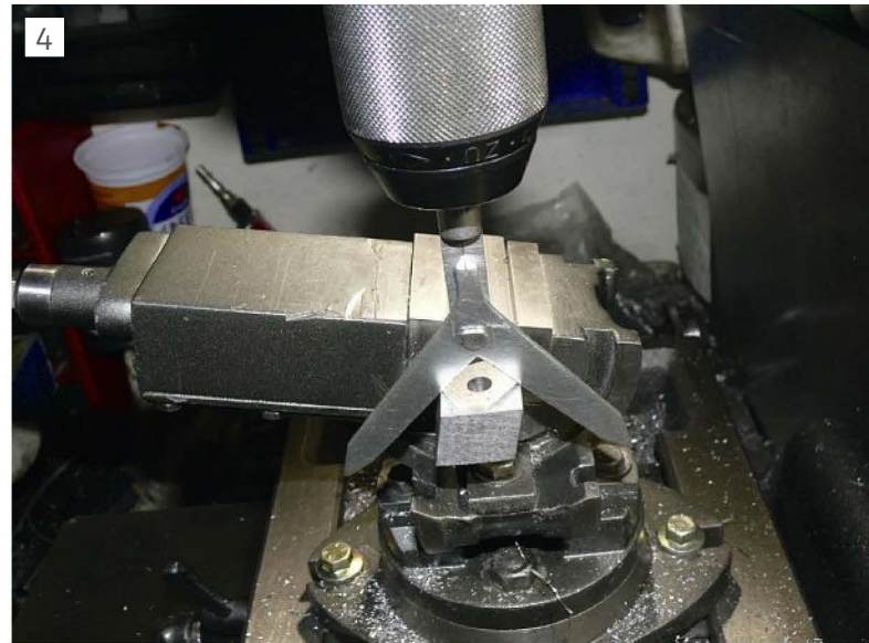
Staged picture of centring the tool holder.
