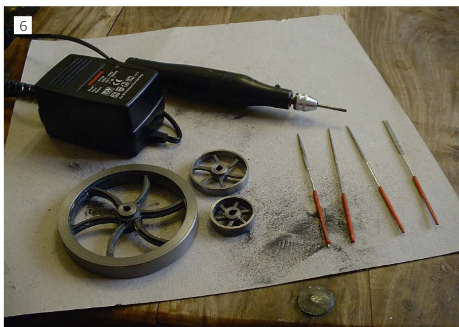
Using a venerable 'Woolworths' multi-tool and diamond files to tidy up iron castings.
