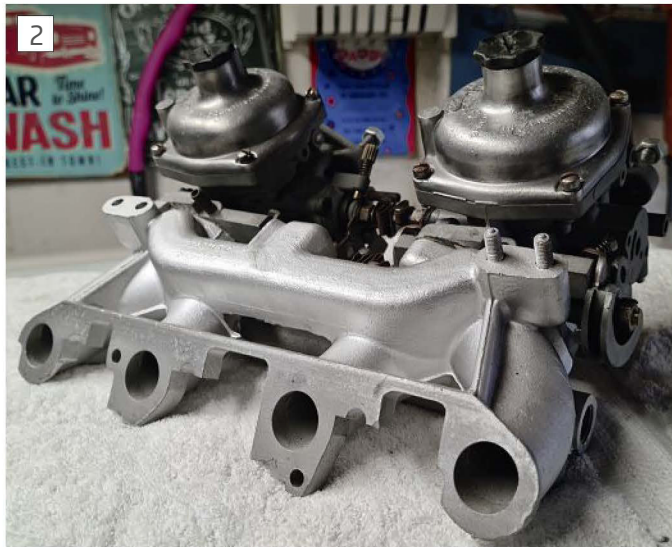
Twin Stromberg carburettor and manifold refurbishment.
