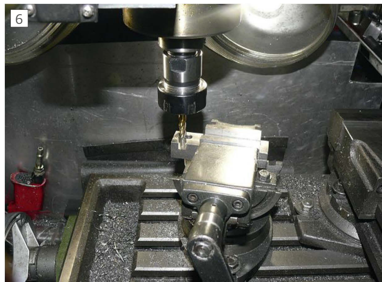
Milling the slot for the toolbit.
