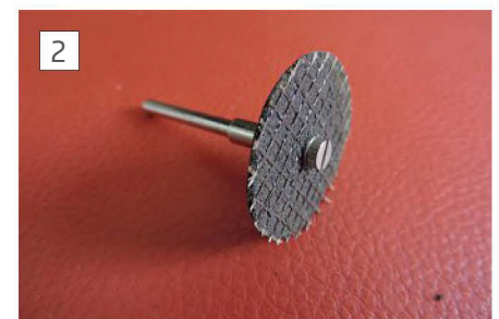
Reinforced cutting discs are thicker but more robust than the brown carbide type. ➤
