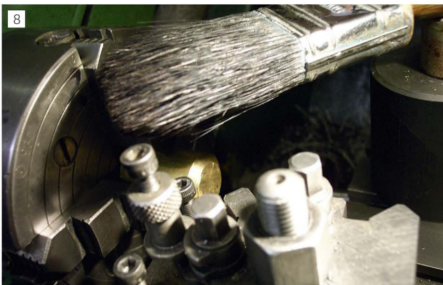
Brush deflecting chip spray from brass/bronze turning work
