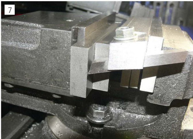
Using a parallel to set toolbit protrusion.
