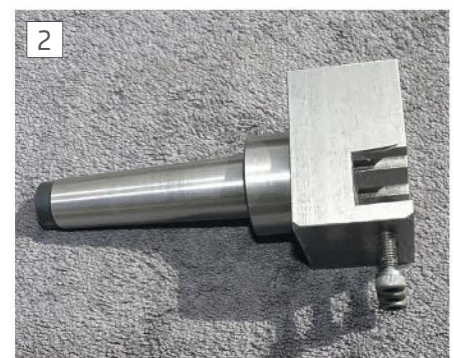
Widened slot in tool holder block.
