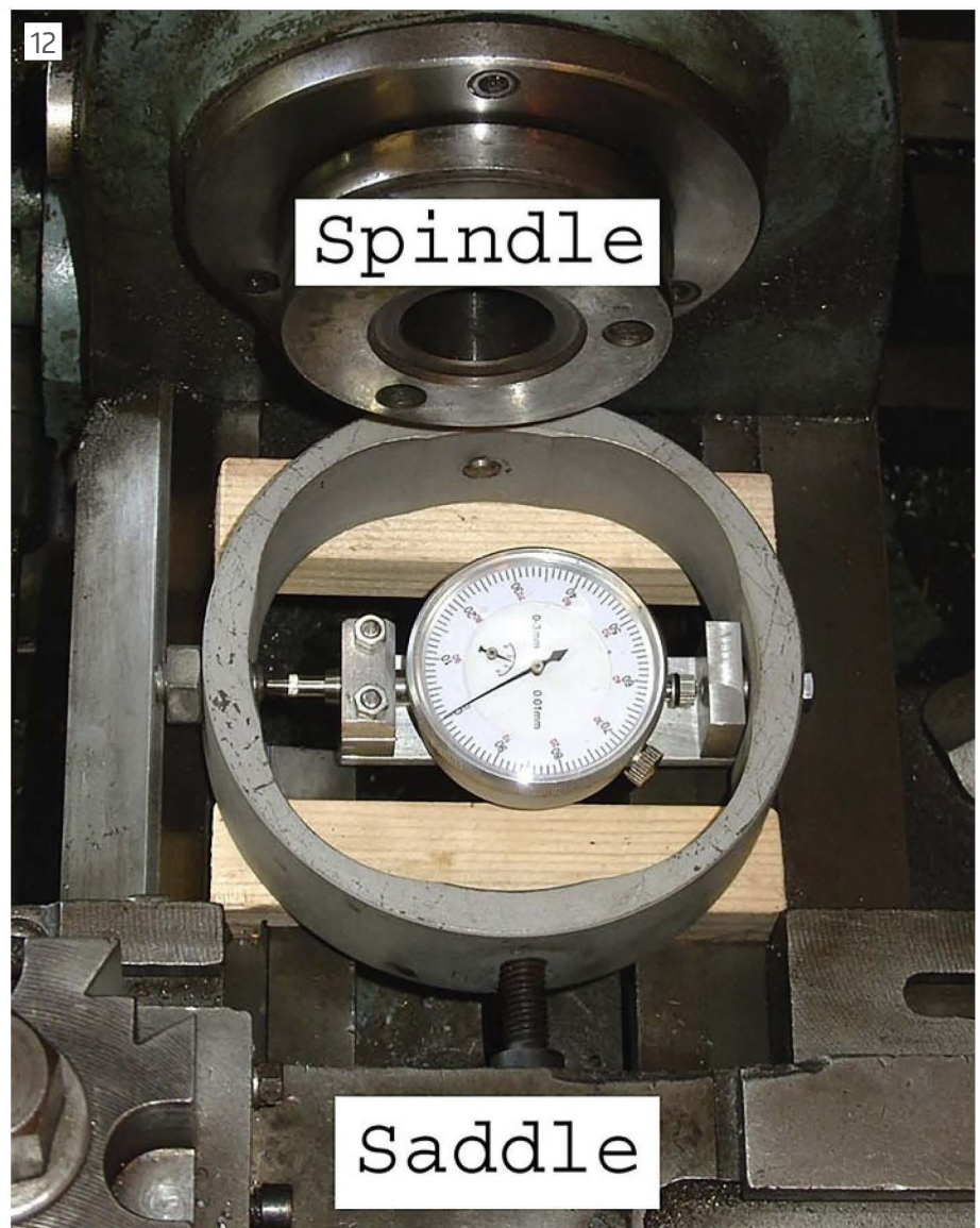
Using a ring dynamometer to measure spindle torque.
