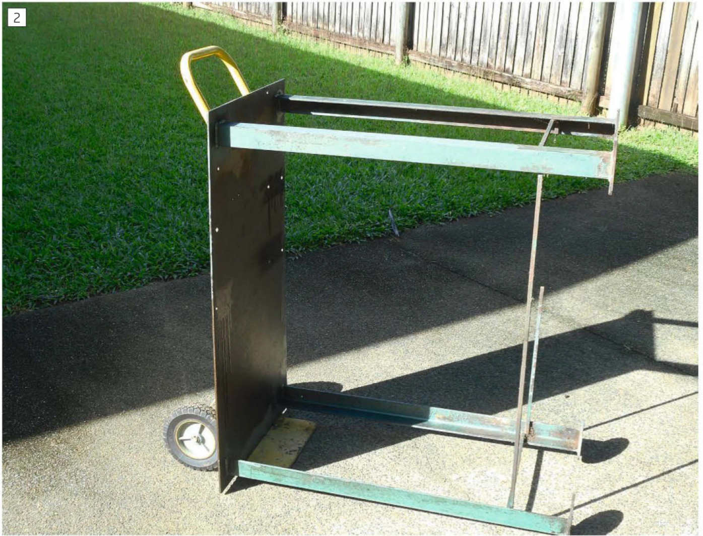
Four stout legs, but the unsupported flat plate benchtop was not suitable for the weight of a lathe.
