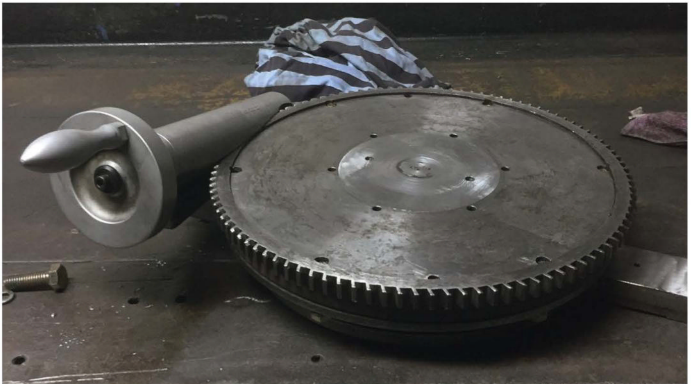
Completed rotary table.
