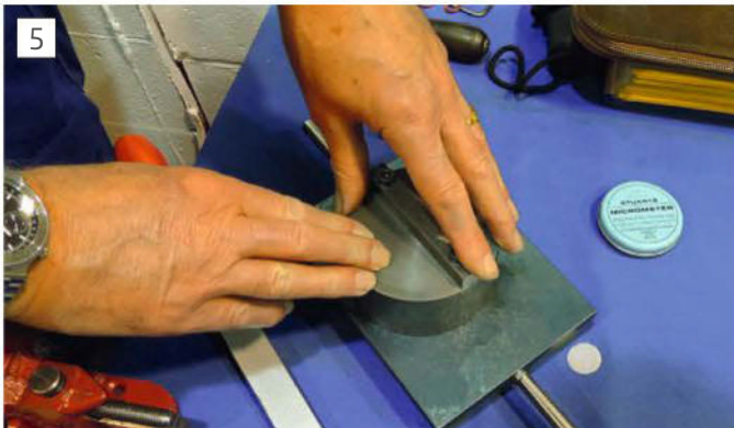
Neal Read demonstrates hand scraping in 2015.
