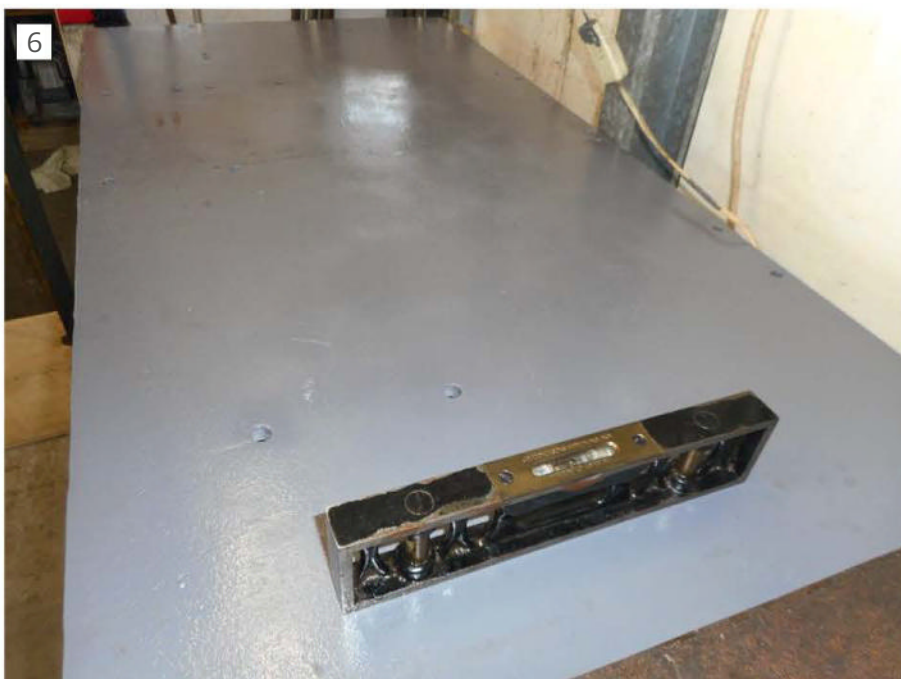
6 Standard machinists level used to set bench top to slope slightly backwards for oil drainage in the drip tray.
