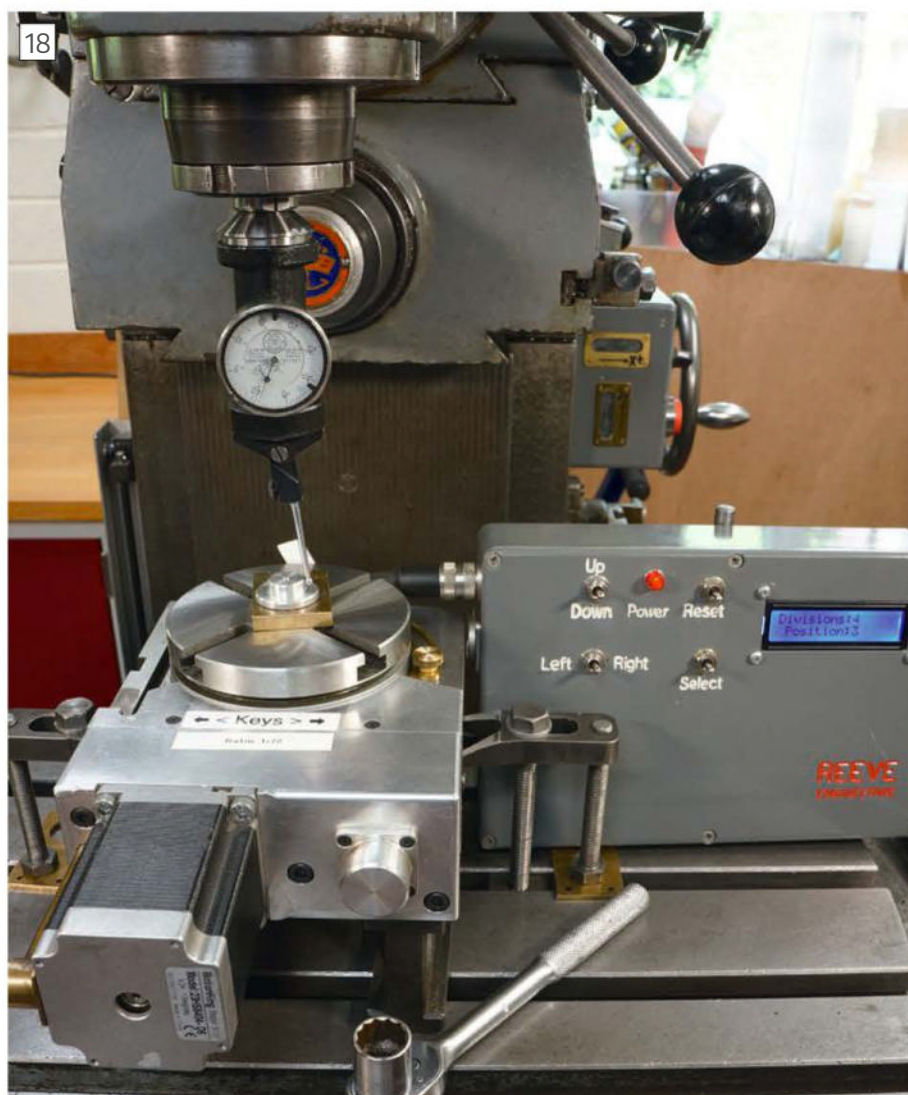
Centring drive flange on mill.
