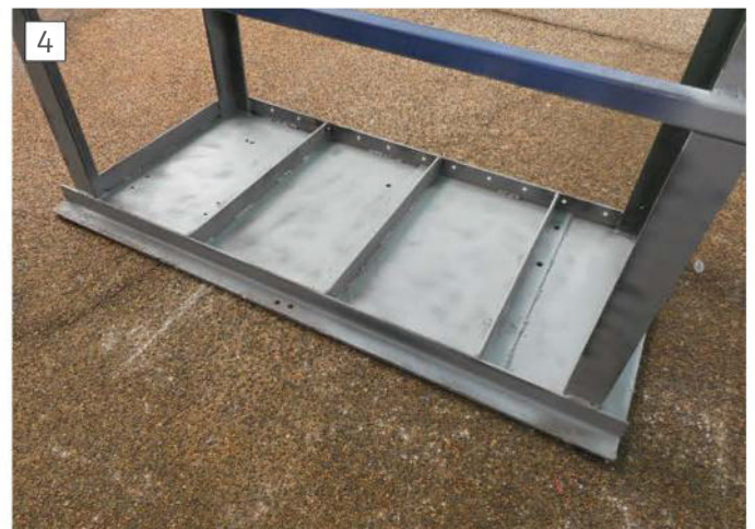
The completed bench with extra steady rail around the legs.
