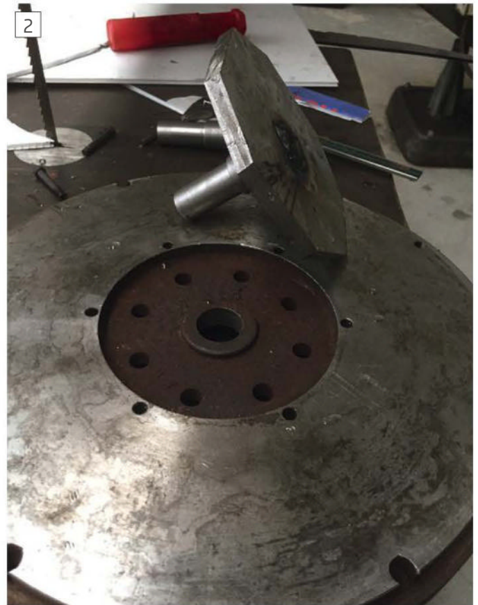
Plate welded to centre shaft.
