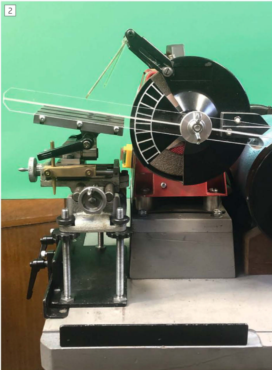
Aligning the rest's table using Ruler and Sector Plate. (This photo also shows the perpendicular lengths of angle iron to which the base of the rest may be clamped so as to face either the edge or the face of the wheel.)
