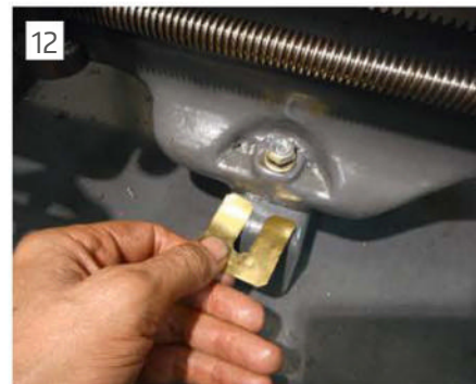
Shim slid in around mounting bolt.
