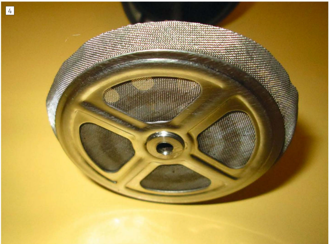
4 The reassembled filter assembly with the new nut.
