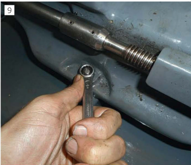
Tighten down mounting bolts evenly.
