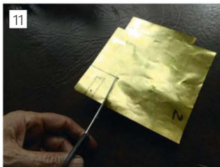
Shims cut from brass stock with scissors or tin snips.
