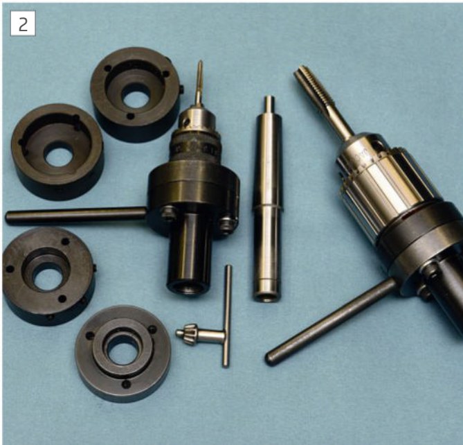
Arrand threading attachment, we believe these are no longer available but other makes in the same style can be found.
