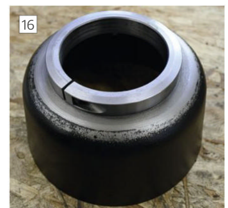
Slot cut in the steel clamp.
