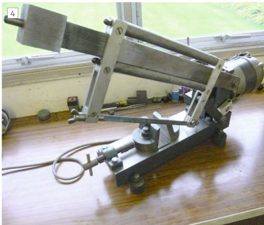
The pivoting arm locked in the setting position.
