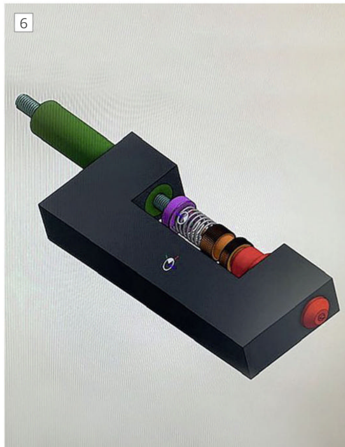
Three dimensional representation of the Cutter Holder.
