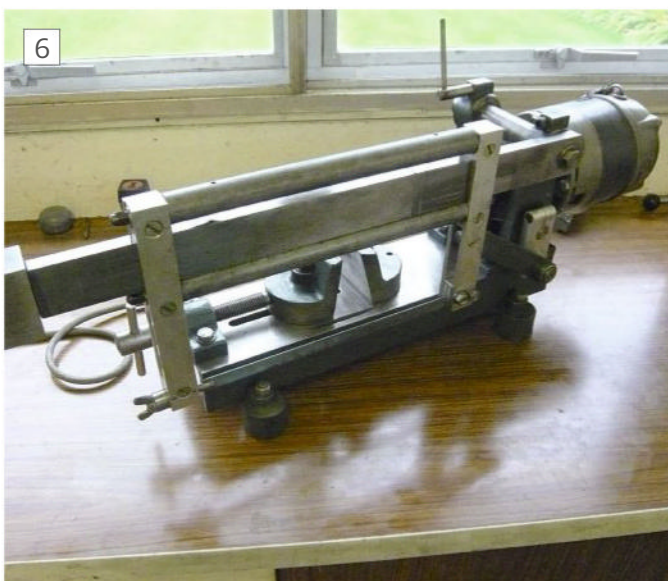
The pivoting arm in its parked position.
