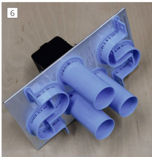
Pipe clips and joiners on the build plate.
