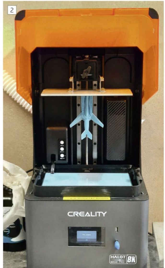
The 'Mage Arch' is a flip up lid that provides easy access. Note vent pipe at left.
