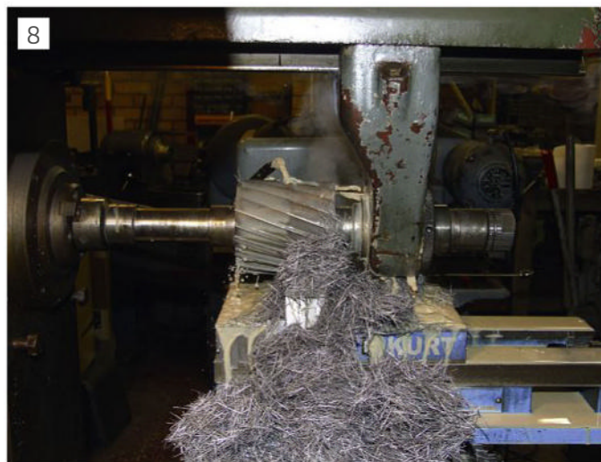
8 Slab Milling Hot Rolled Steel
