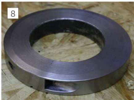
Hole for M4 clamping screw milled, drilled and tapped.
