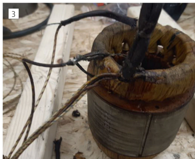
Leads as found when disassembling the stator from the motor housing.
