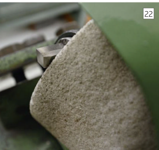
HSS tool bit ground on the freshly repaired grinder.
