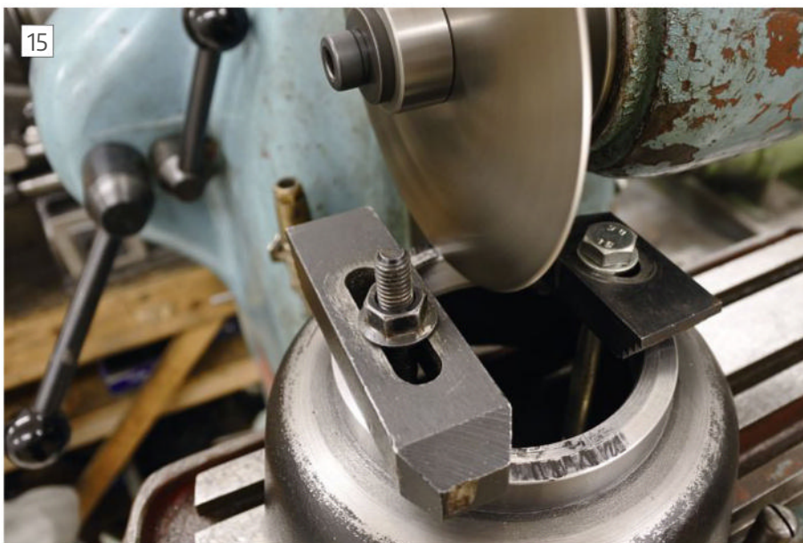
Cutting a slot in the steel clamp using a slitting saw.
