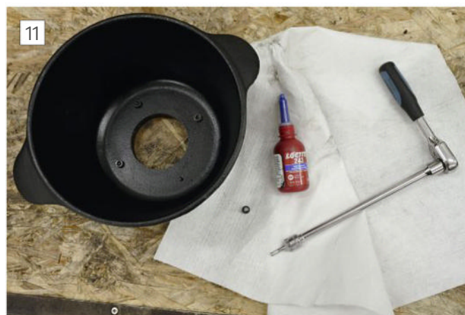
Installing screws to securely retain cast-iron pot on steel clamp.
