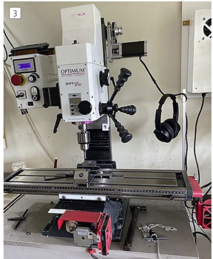
My Optimum milling machine showing some 3D printed CNC conversion components. The axis drives are mounted on aluminum parts not seen.
