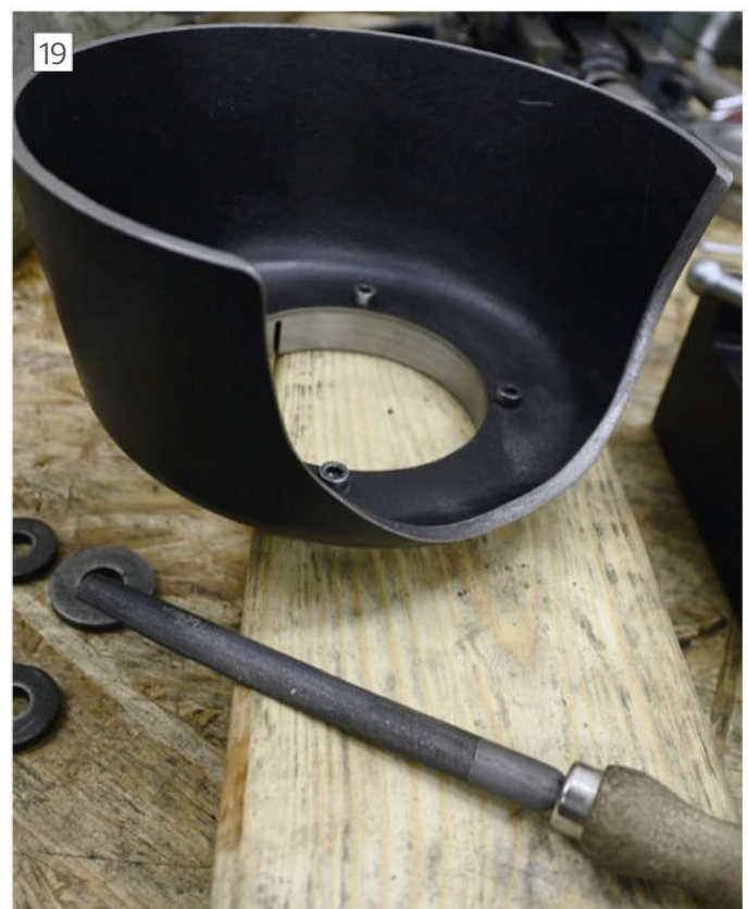
19 Finishing off the opening using hand files.
