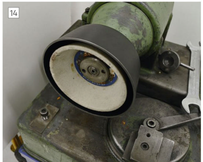
First test-fit of wheel guard to grinder.
