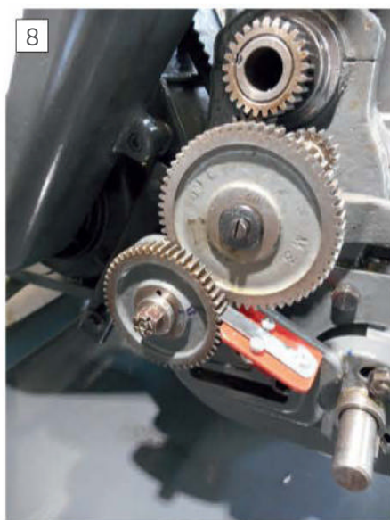
The 60 – 30/50 gear train is regulated by the hacksaw blade detente unit that allows one-way movement only and provides a positive stop for precise graduating.
