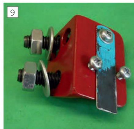
Detent was made from a scrap of steel angle and a ground down piece of hacksaw blade. Tension can be adjusted by the height of the two front screws limiting blade movement.
