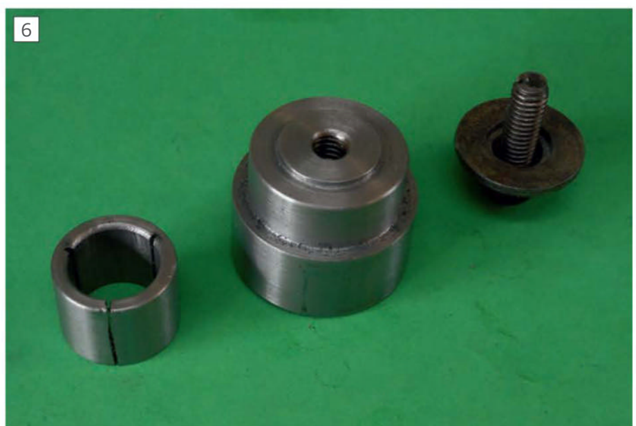
The hub's holding collar is to the left of the dial's stub mandrel, securing screw and flat washer.
