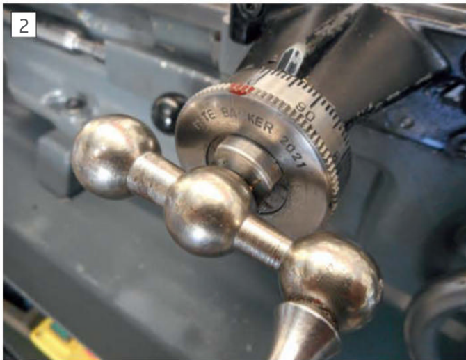
The dial is made of two main components, inner hub and outer dial, held together by a circlip at the rear.
