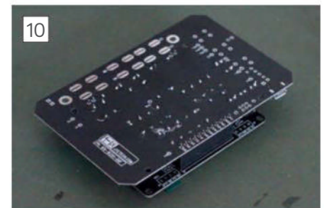
Pin strips soldered in place.
