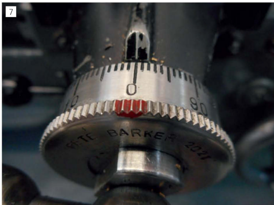
Graduations came out perfectly spaced, let down by cheap number stamps that don't line up consistently. But without the close-up shot, you will never notice it on the job.
