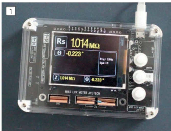
The JYE Tech M162, measuring a 1 megaohm (1MR) resistor.
