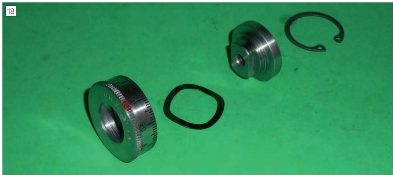
The two components and two pieces of hardware assemble in the order shown.
