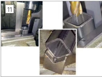
Finishing the sockets.
