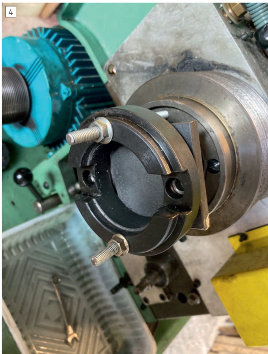
Pulling the drive pulley.
