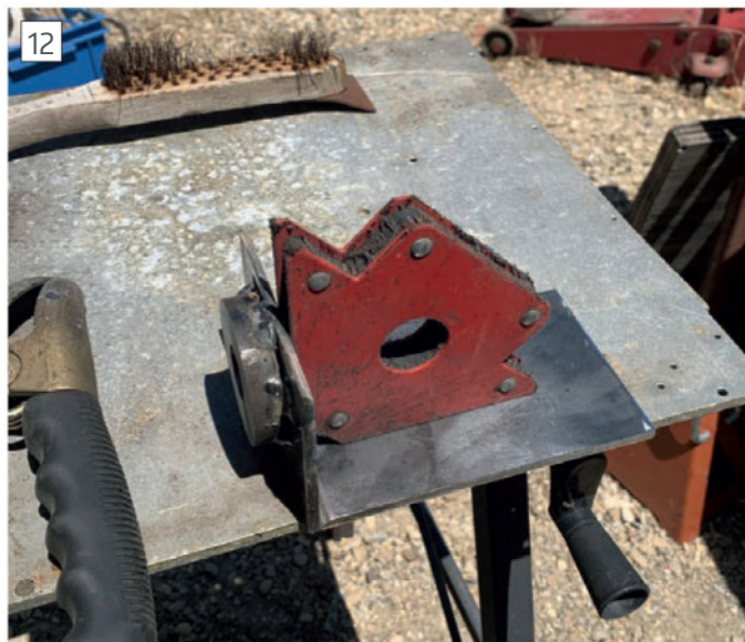
12 Initial setup for welding the end and main plates together using a magnetic clamp
