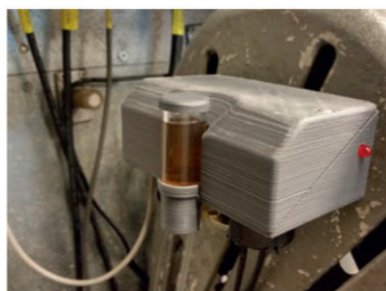
Julian Palmer put an end to pools of wasted oil under his ML7 with an electrical auto oiler.
