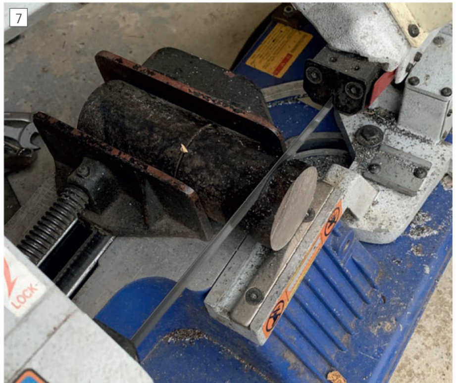
Cutting the annular ring the easy way
