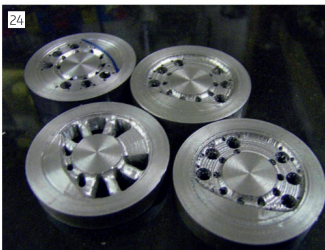
Stages in machining loco wheels from solid.
