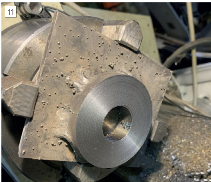
11 Returned to the lathe to make the ring face parallel to the face of the end plate
