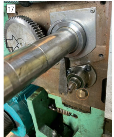
Gear flush with shaft end.
