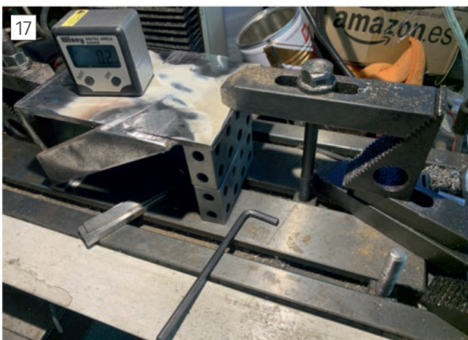
Clamping at this end stretching the supply of my spacer blocks to the limit. The 'epoxy' or whatever coating can be clearly seen along with my careless hacksawing
