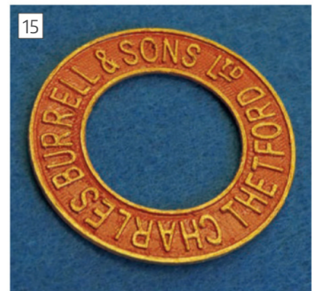
3D printed and painted, not a casting!
