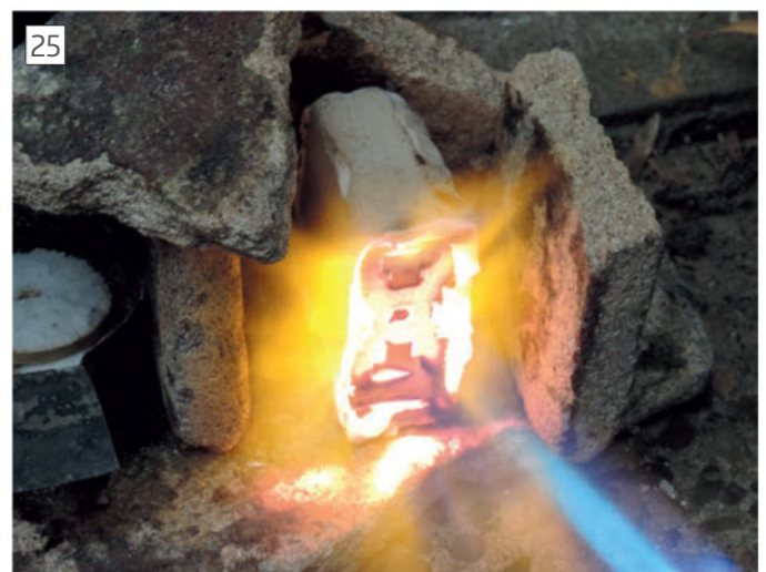
Burning out an investment mould.
