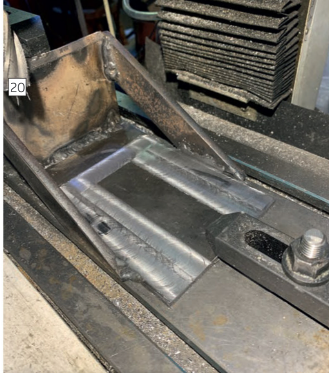
Milled surface ready for the new spindle. Note the milled reference surface on the side brace weld. Also note the continued presence of the epoxy coating on the end plate, even very close to the welded areas!
