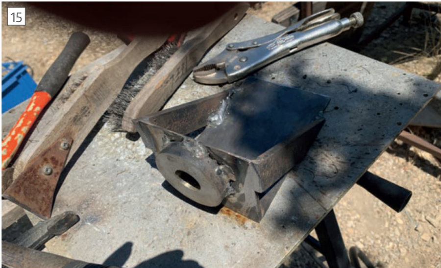
Side braces trimmed to size, ready for machining
