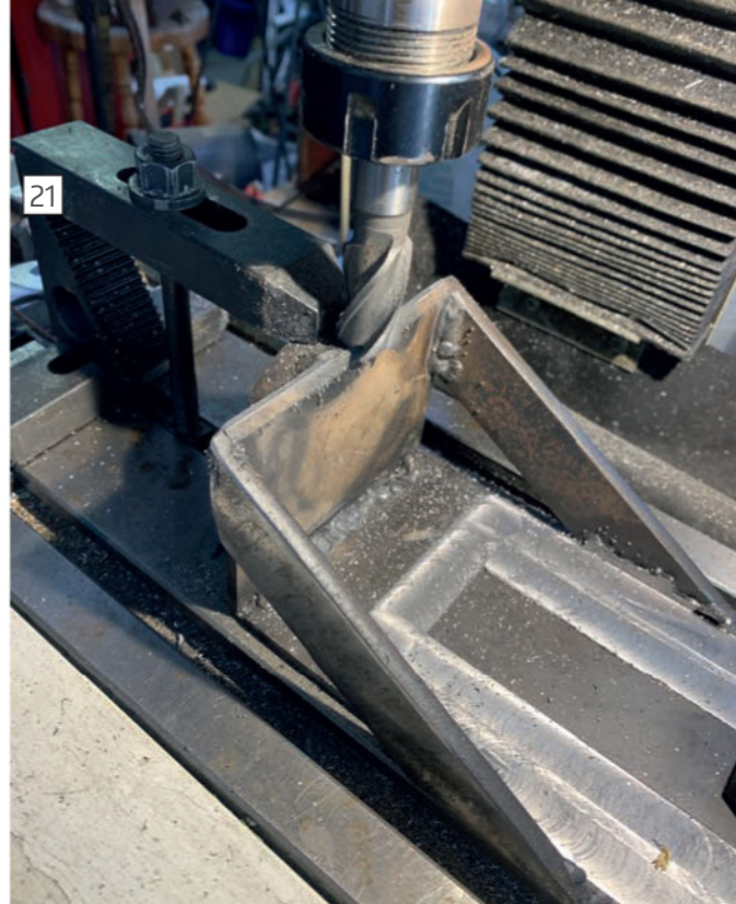
Milling the top edge reference plane, parallel with the main reference plane
