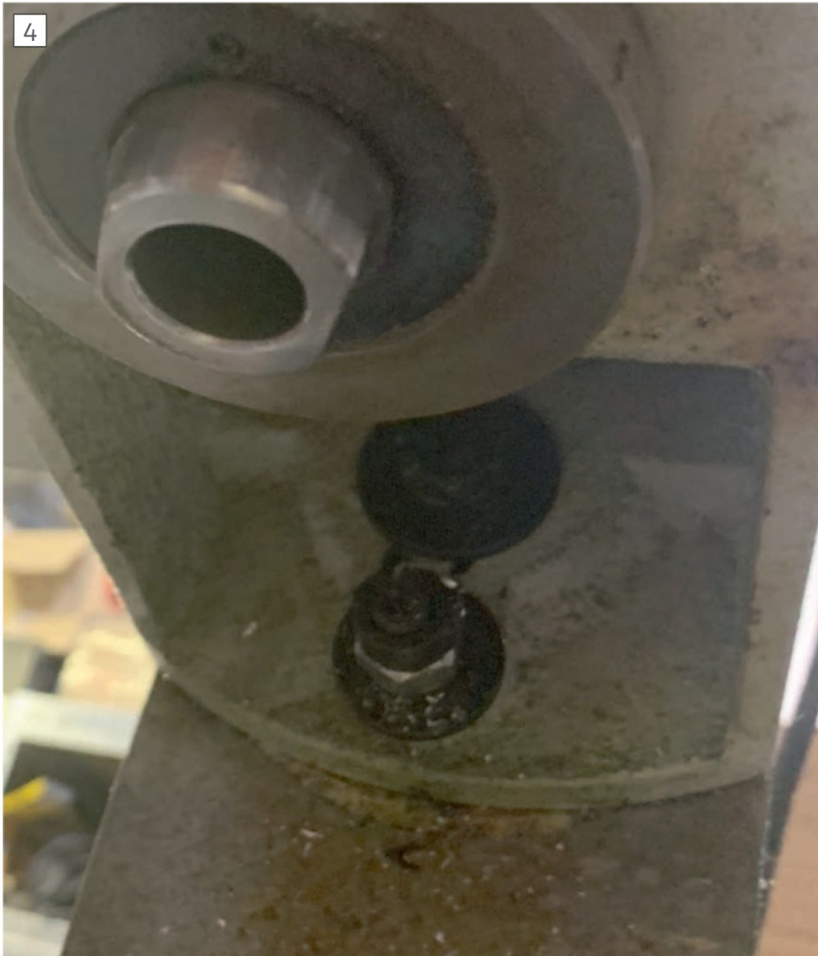
The existing mill spindle showing the reference outer face and the end face of the quill
