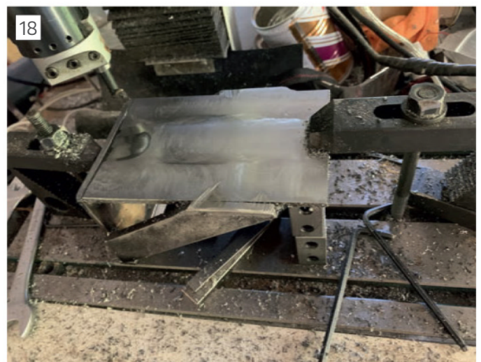
Fly cutting removes even the epoxy coating! One final cut to go to get rid of the hollow centre left
