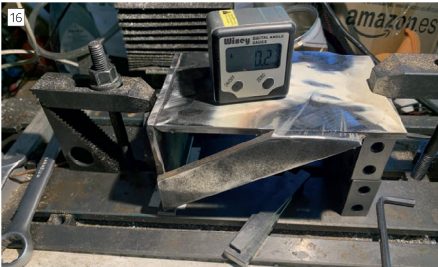
Clamping onto the annular ring, parallel and shims underneath the edge to get the reference face level with a pair of Stevenson's blocks at the other end which happened to be about the right height. Angle gauge was used for the measurement especially given the less than flat surface to work onto
