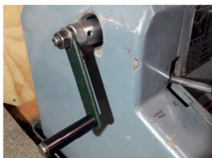
Matt Shaw's Boxford headstock tool started as a depth stop but now has several uses.
