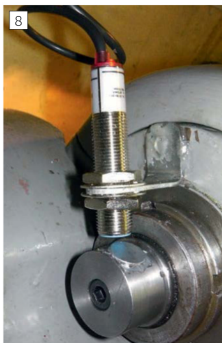
Bush with magnet and sensor in place.
