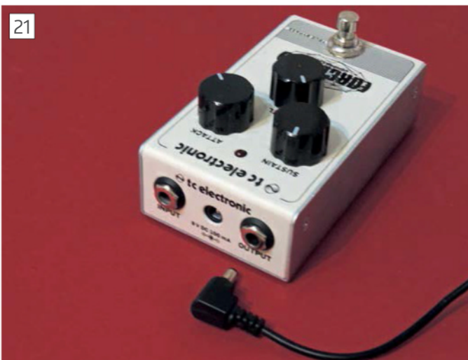
5.5/2.1mm jacks have become ubiquitous, not just for astronomical equipment, but always check voltage and polarity first!
