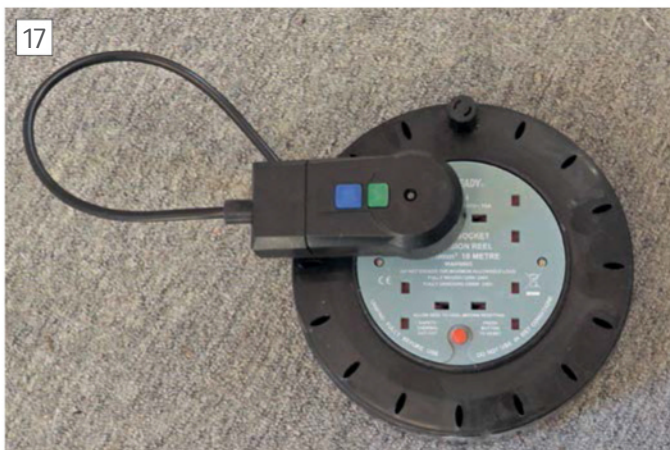
This ten-metre extension lead with the plug removed and an RCD safety device fitted provides peace of mind.
