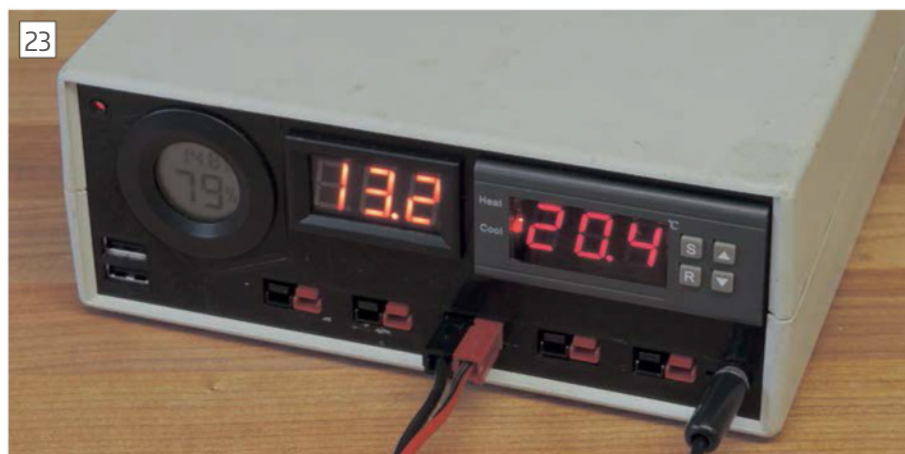
The multi-output power supply includes 5V USB outlets and 12V powerpole connections, one of which is controlled by a thermostat unit. The output voltage is now regulated to 12, rather than 13.2V.
