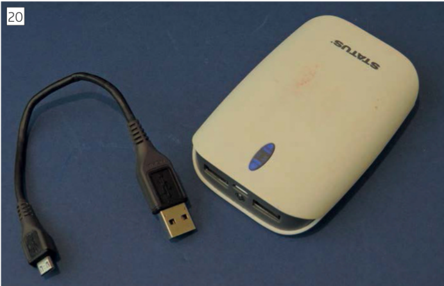
Li-ion power bank suitable for powering 5V equipment, especially those which use a USB lead for power.
