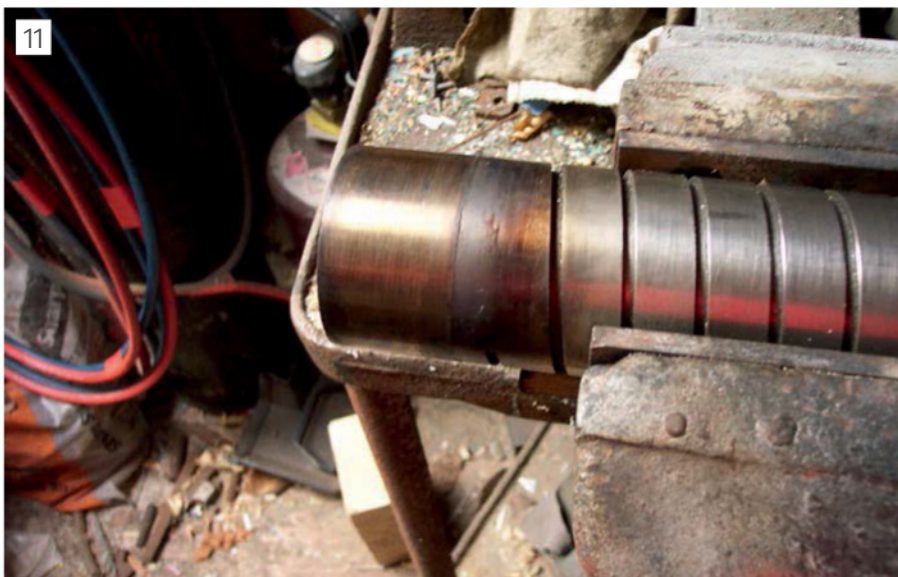
Evidence of heating to break Loctite joint.
