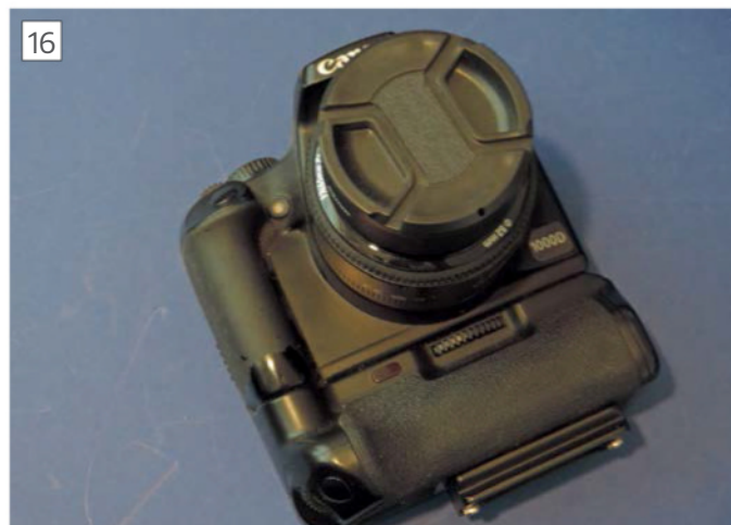
This two-battery power grip is bulky but contains a self-timer giving a self-contained solution for a night of wide-field imaging.
