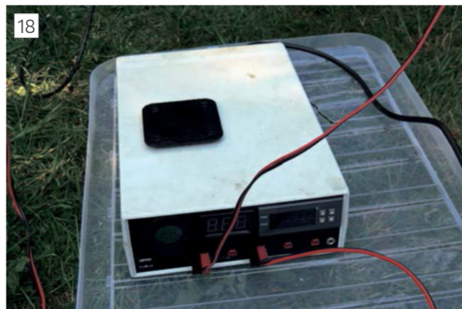
Multi-output power supply placed on a plastic lid to keep it away from damp grass.
