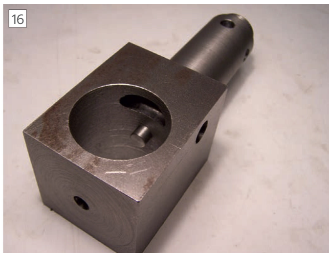
The push-rod entering the Main Body bore.
