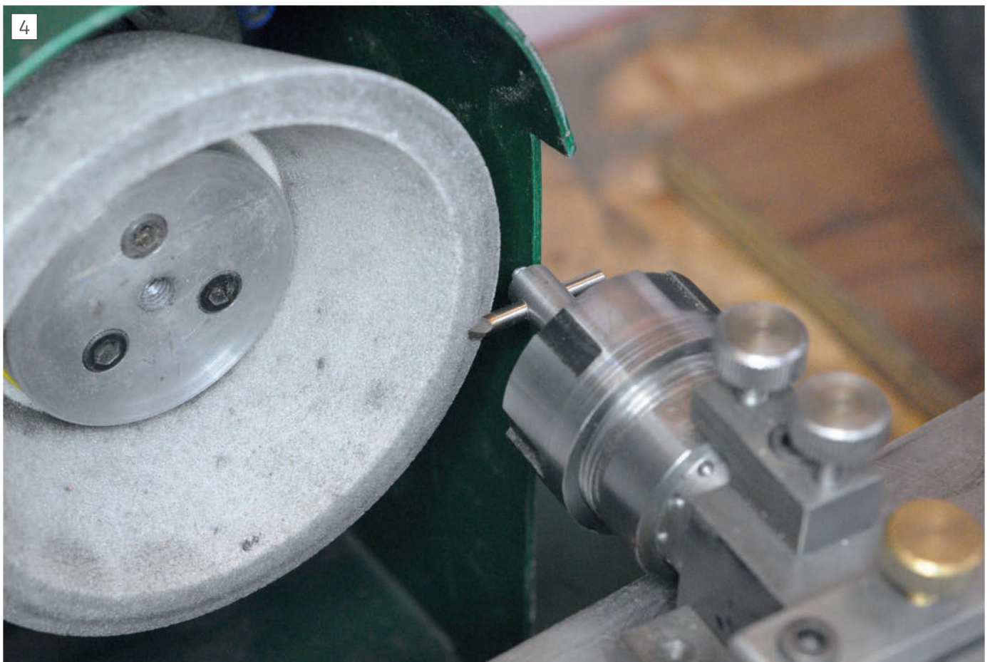
Grinding the angles.
