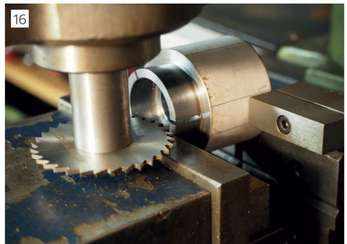
Slitting saw operations.
