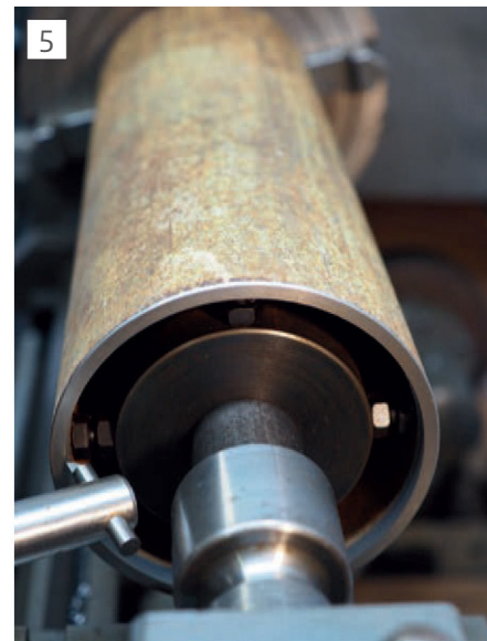
Internal cat head supporting a large tube.
