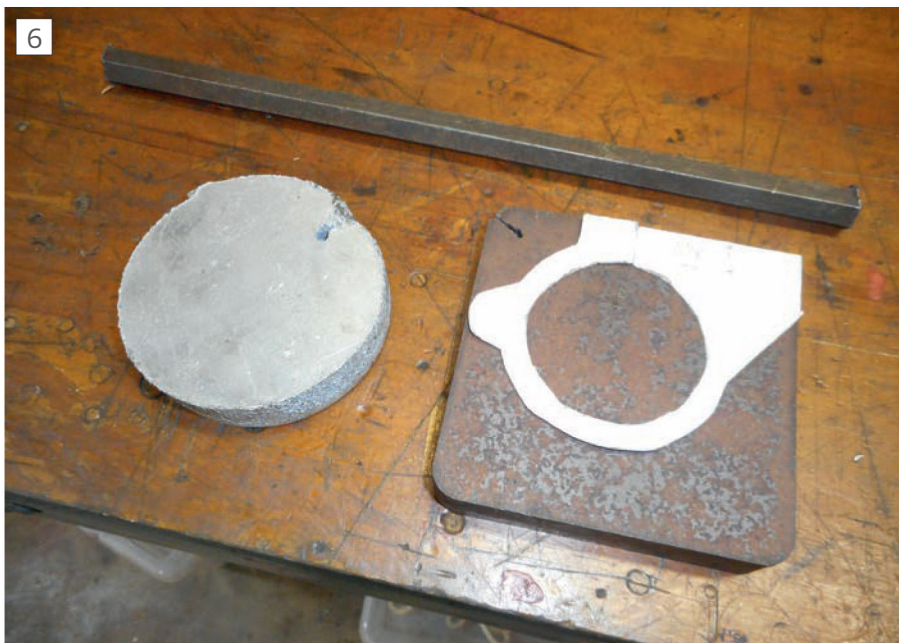
Raw materials were selected and developed with the aid of cardboard templates. The hex bar was discarded as too small.
