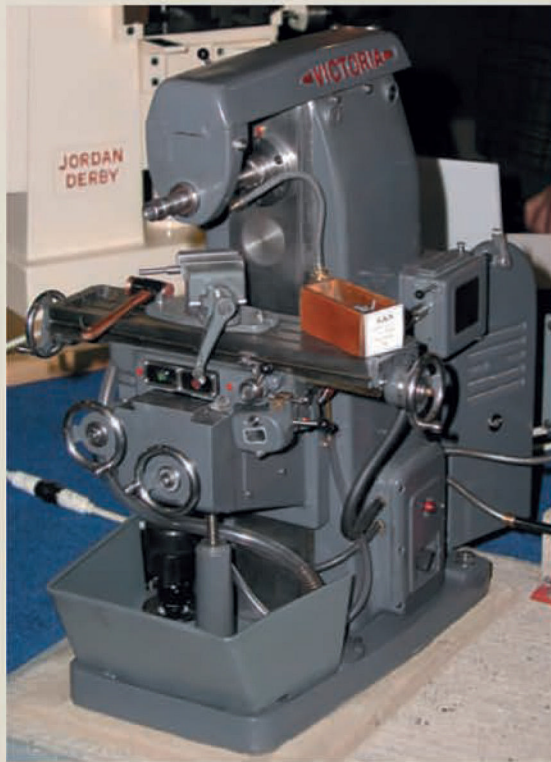
Right: Victoria milling machine by Mr M. Leafe with swivel vice and other items. Shown grouted to the floor and ready to work, it is difficult to believe that this photo is of a model. Note the excellent proportions of the hand wheels, tools and accessories.
