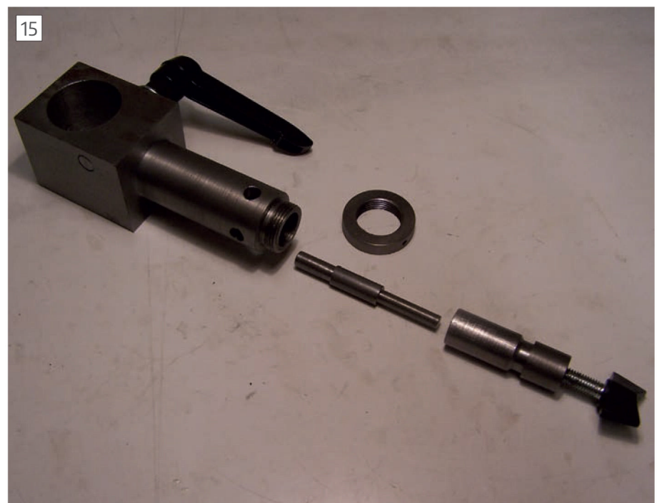
The Additional Support Arm parts ready for assembly.
