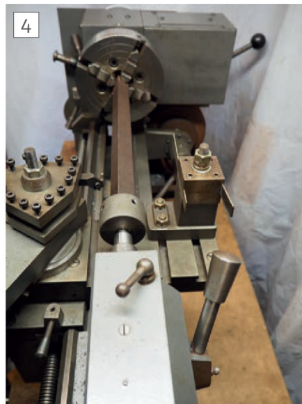
Cat head using tailstock centre support.
