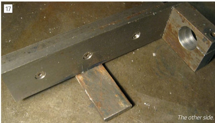
M3 screws fitted.
