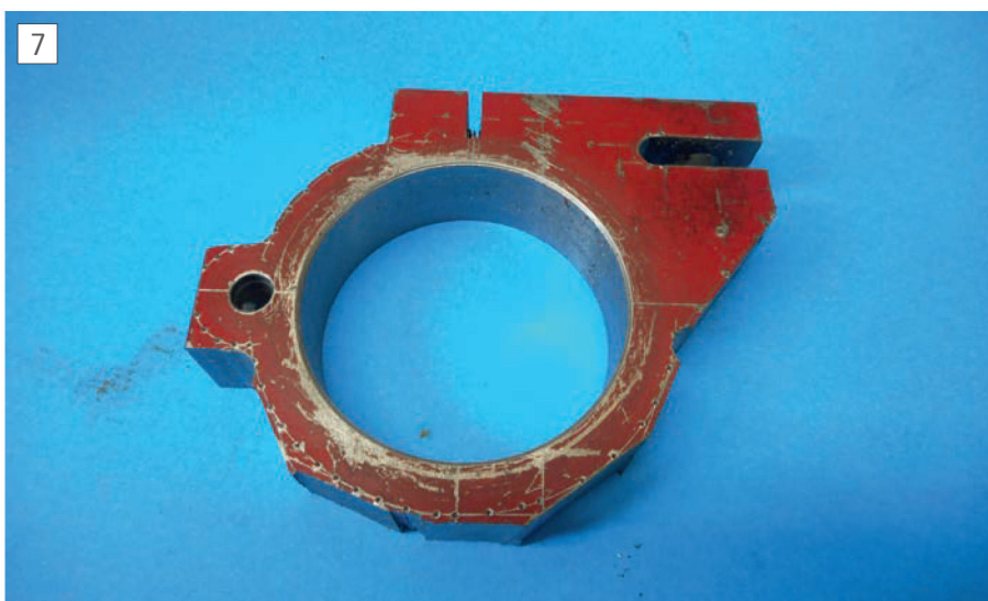
The bandsaw made quick work of the outer profile and even the 1/4" wide slot
