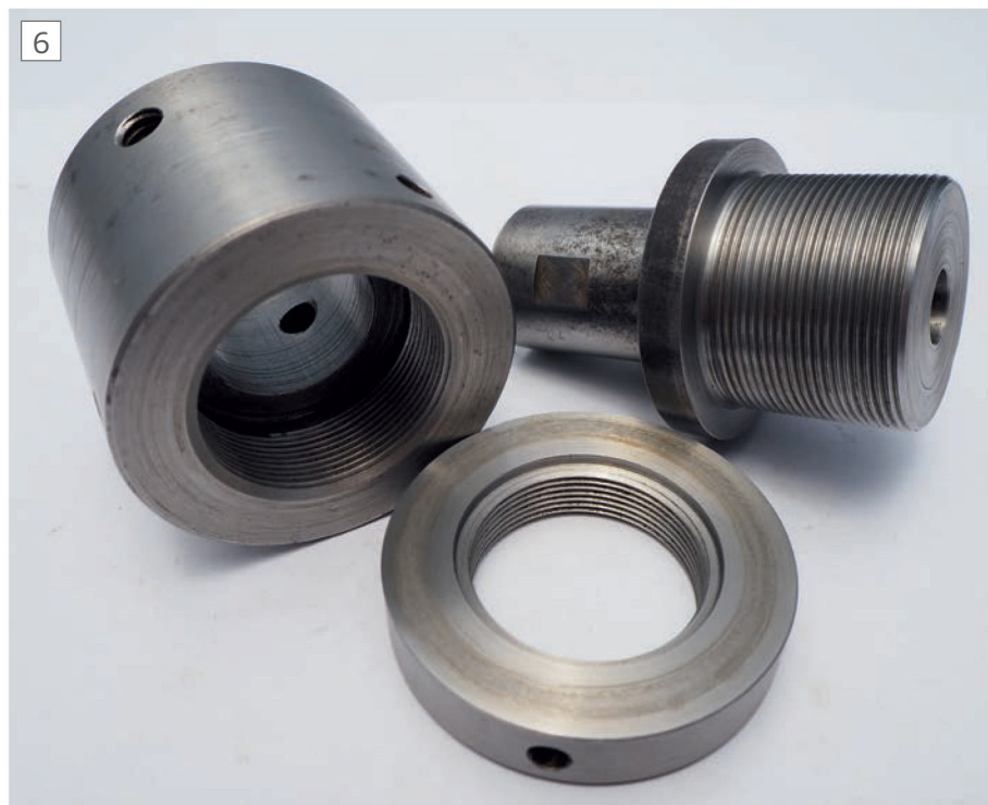
Completed threaded unit with dummy spindle.
