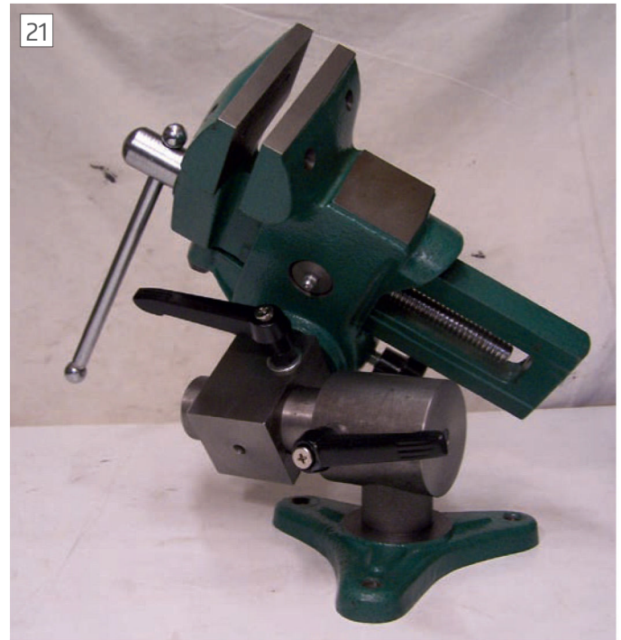
The vice can be positioned at any angle you like!
