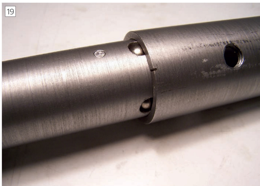
Sliding the Sleeve on - note the slight saw-cut to indicate the centre line of the 10mm hole.
