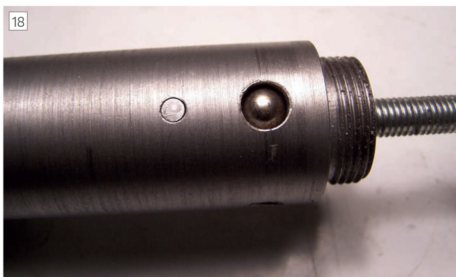
The ball bearings and the key in place.
