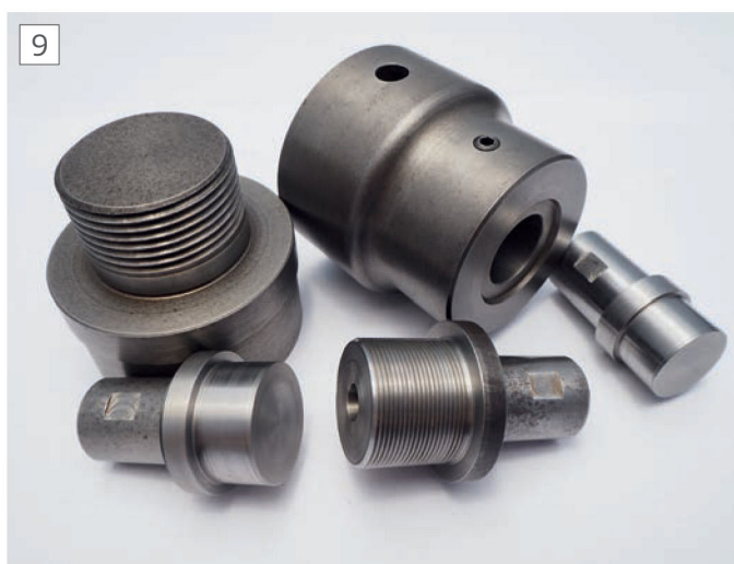
Dummy Spindles and Master chuck.
