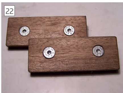
The hardwood jaw facings and screws.
