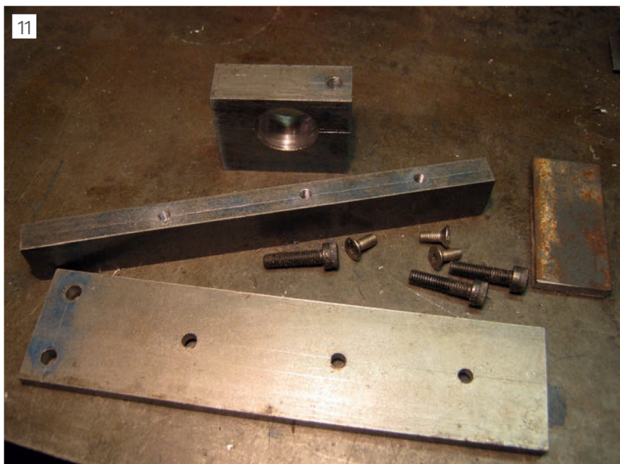
Parts after drilling and tapping.
