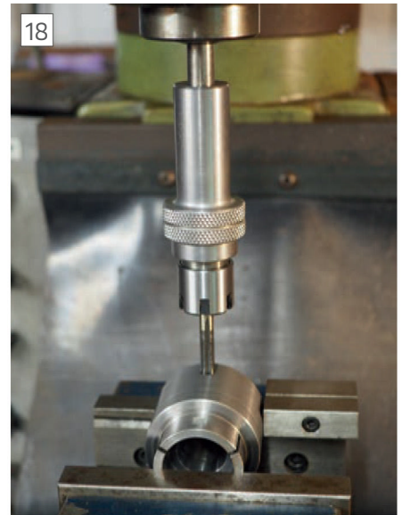
Sliding tap holder for accurate tapping.
