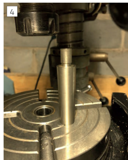
The 3mm shank plug, as well as other setting up accessories such as a cylindrical square.
