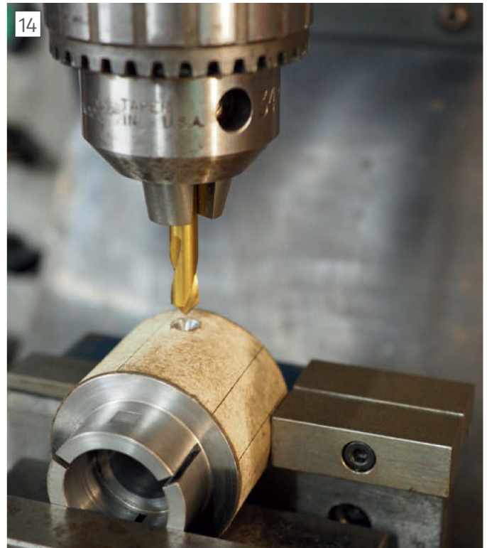
Vice Stop used to help set out screw holes.
