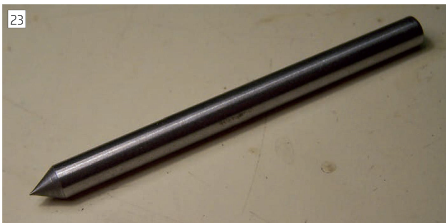
The transfer punch to mark the hole centres.
