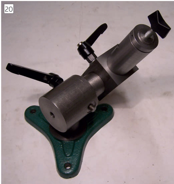
The Additional Support Arm mounted on the Offset Arm.
