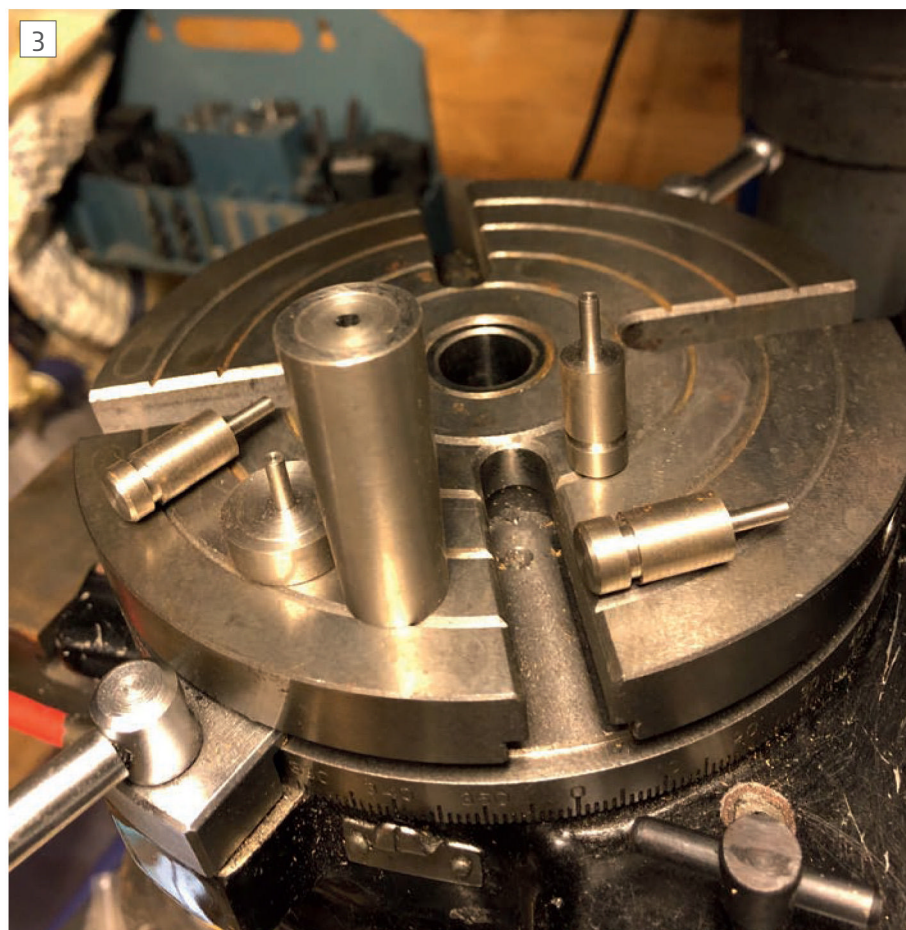
Chuck centring plug in place.
