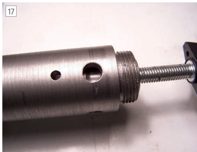
The Cam Lock in position ready for the steel balls and the key.
