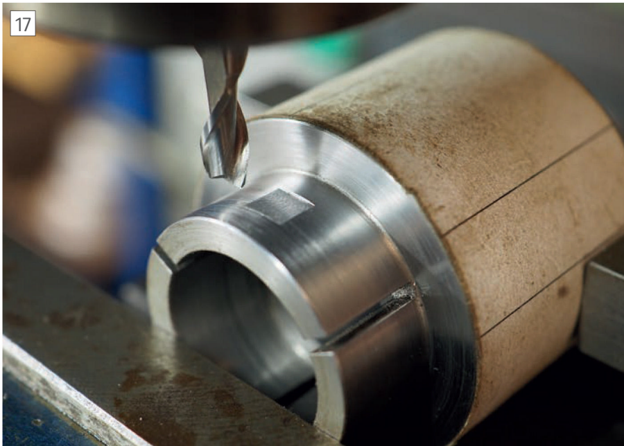
Flat to reduce damage from grub screw.
