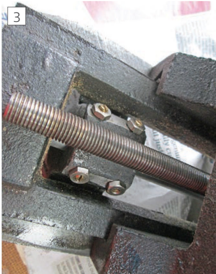
Modified sliding jaw casting showing adjustment screws.
