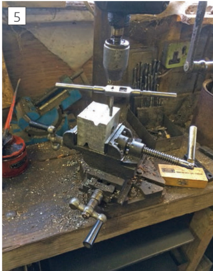
Drilling and tapping clamp fixings.
