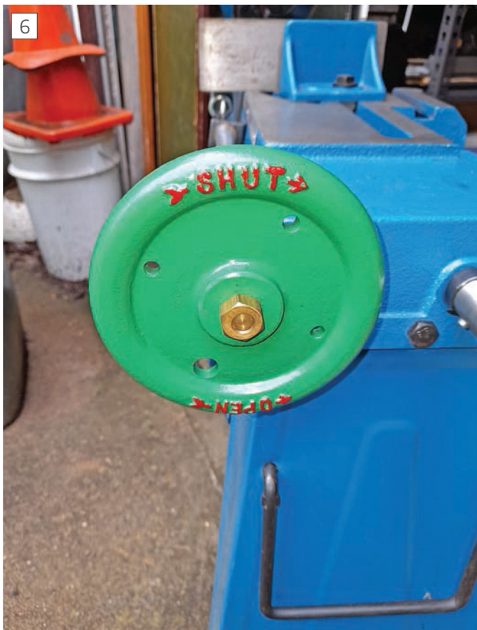
6 Hand wheel to lock vice jaw and repositioned bracket for tension operating shaft.
