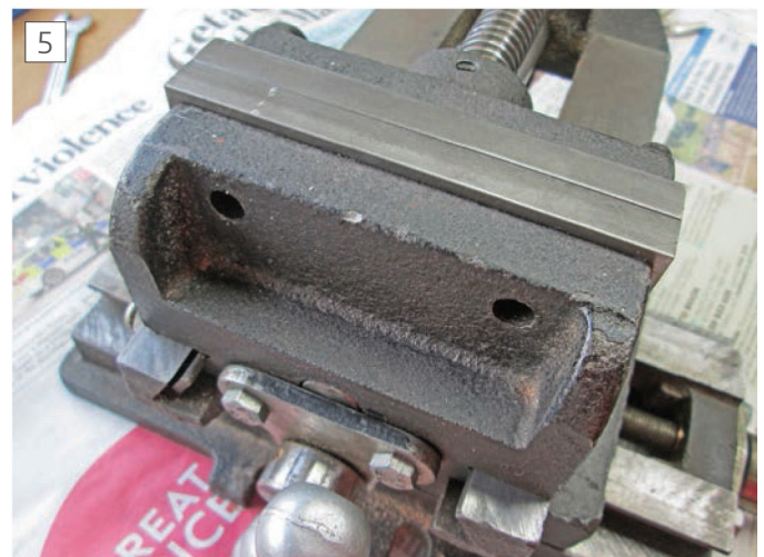
New jaw blanks ready for marking fixing screw holes.
