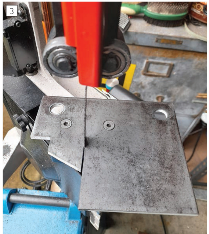
Screw replacement on upper blade guide.
