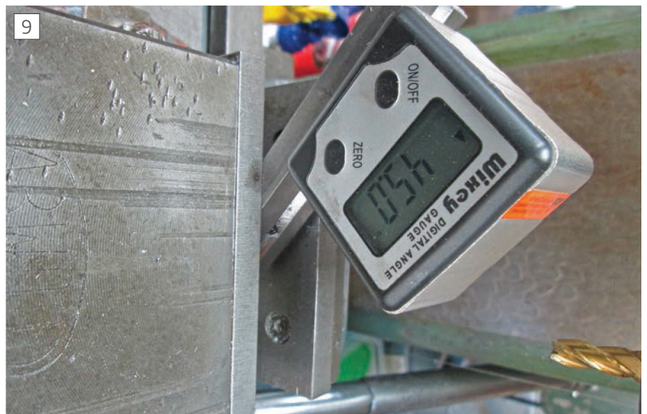
Setting jaw at 45 degrees for machining "V" slot.
