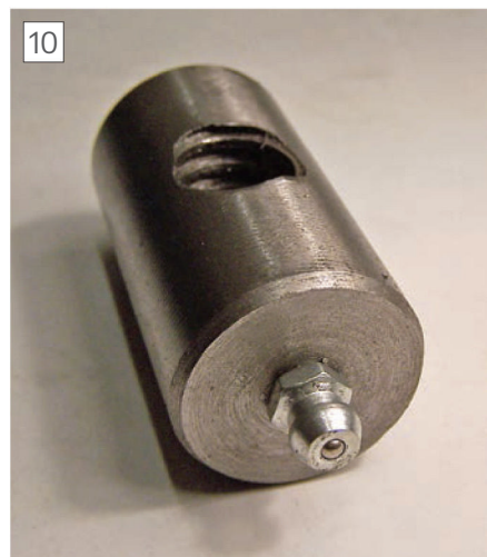
The grease nipple in the vice nut.
