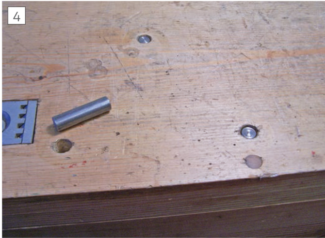
The mounting holes in the bench and the steel plugs.
