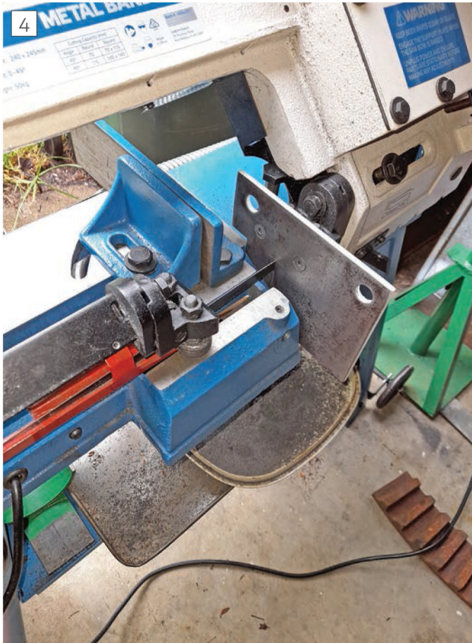
4 New smaller plate for vertical operation.
