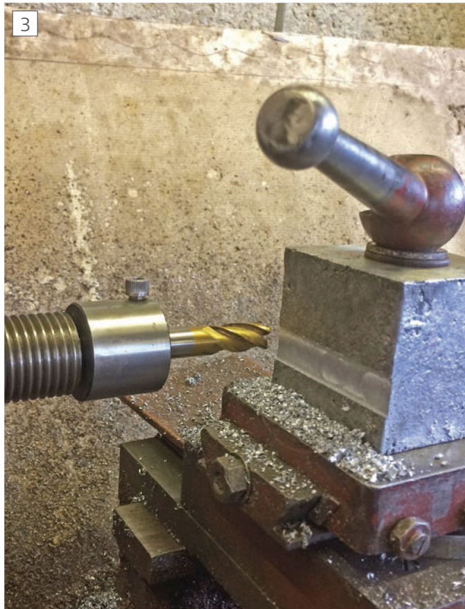
Making the first milling pass.
