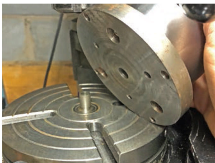
Malcolm Tierney explains how to centre a rotary table.
