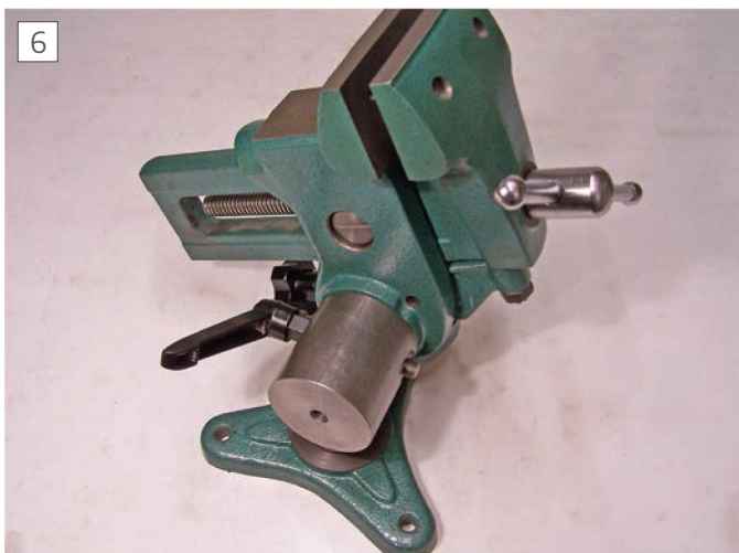
The vice mounted on the offset arm.
