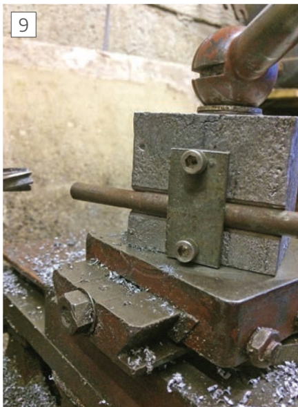
Small diameter rod mounted for drilling.
