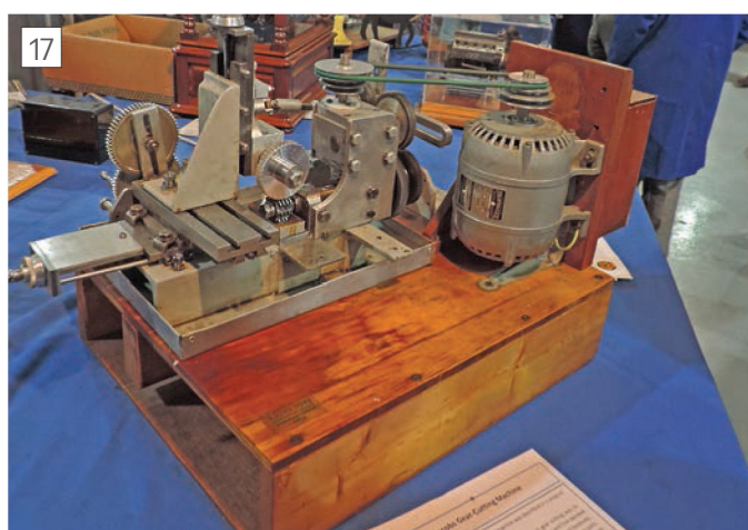
Tom Jacobs' original prototype gear hobber.
