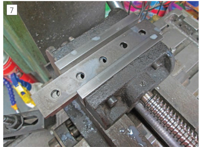
Use of parallels to rigidly clamp jaw blanks for machining.
