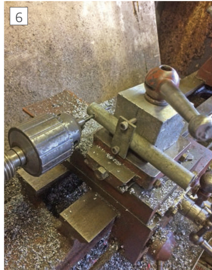
Drilling a tube.
