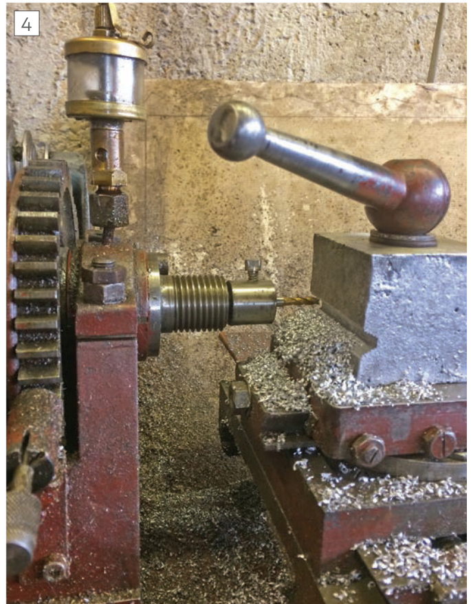
The last milling pass and finished “V”.
