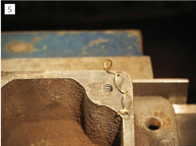
Broken screw fully removed showing undamaged tapped hole.
