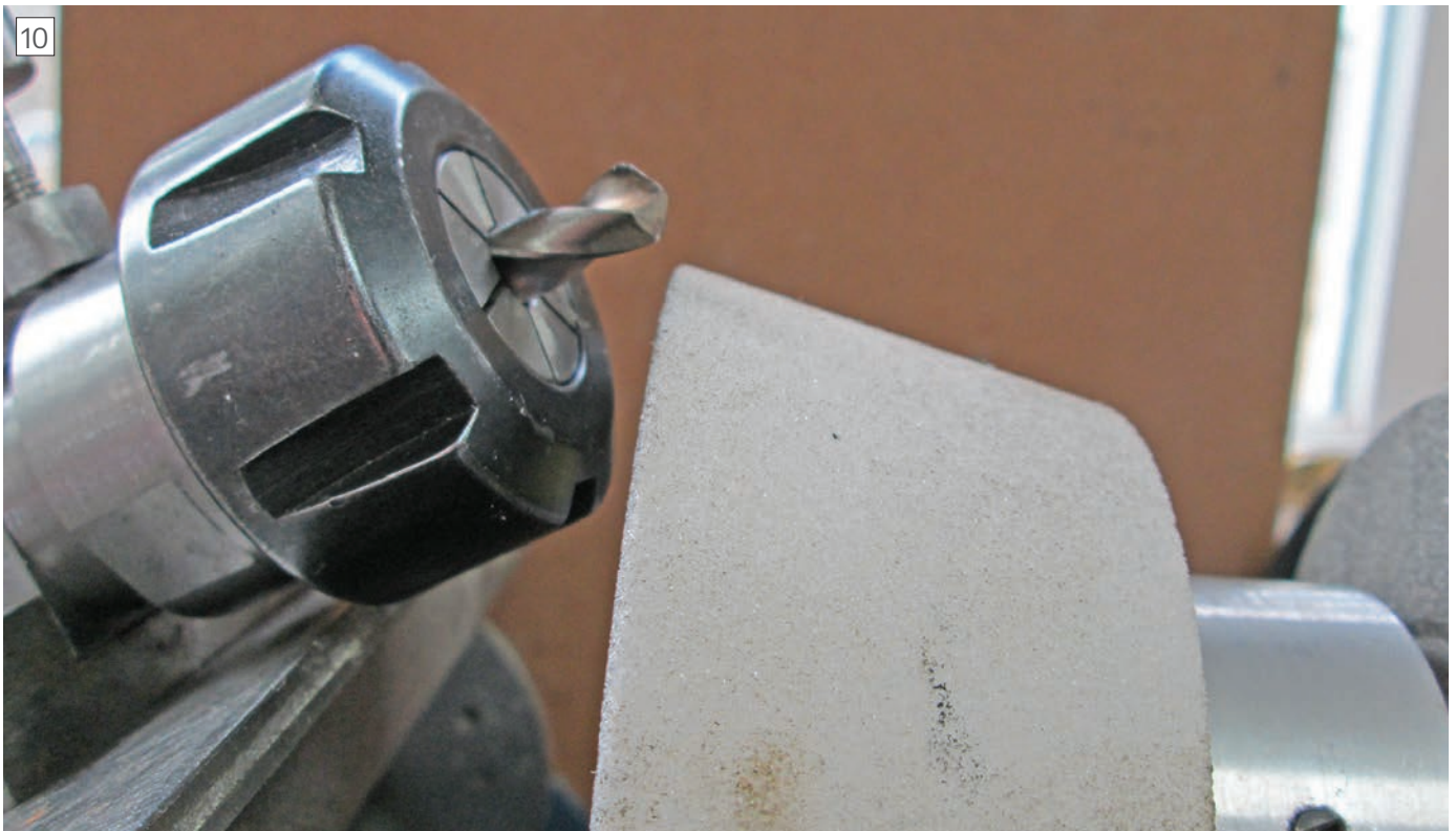
Drill loaded in the new chuck missing the grindstone – too high
