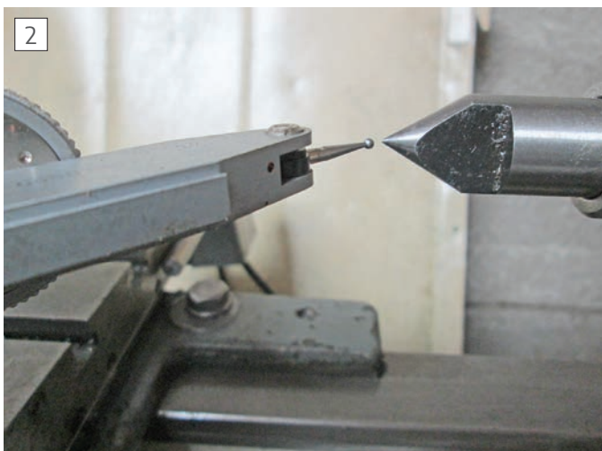
Setting the clock sensor on the lathe centre line
