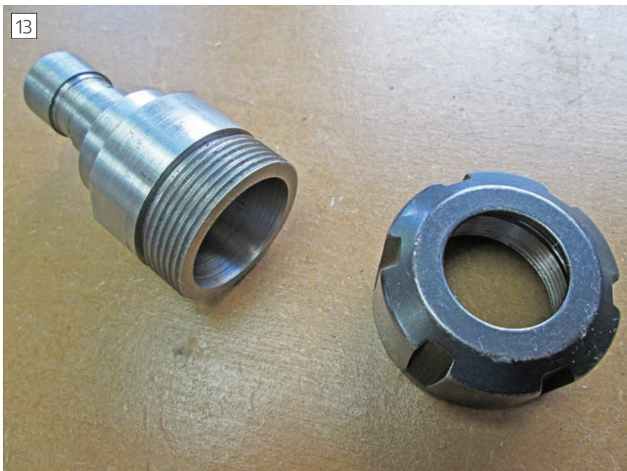
Completed ER25 chuck with bought in closure nut
