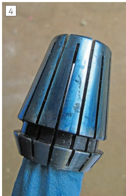
Engineer's blue applied to an ER25 collet
