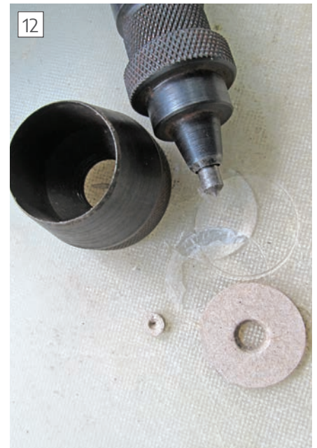
Wad punch used to make resilient washers
