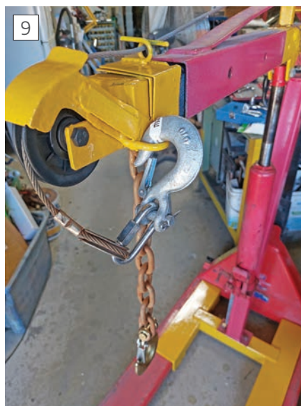
Mobile crane with winch fitted.
