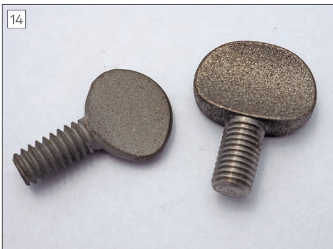
Spark finished thumbscrew compared to grit blasting.
