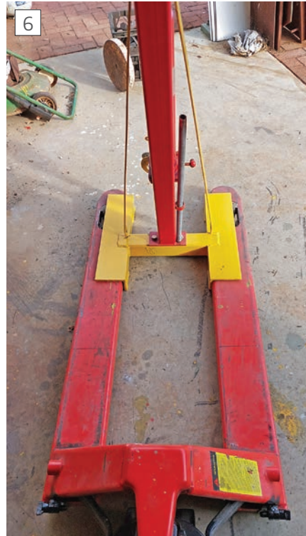
Crane on jack.
