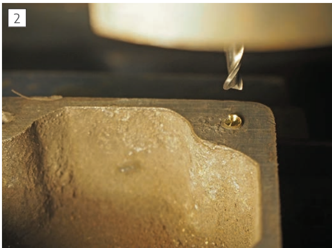
Flatten end of broken screw using a slot drill.
