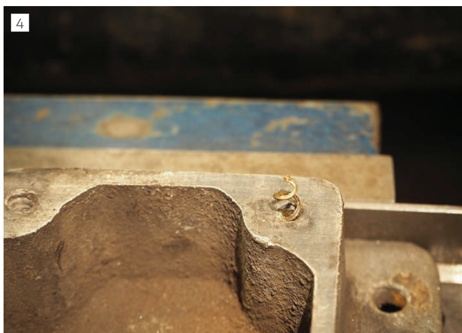
Remaining thread being worked out of the hole.
