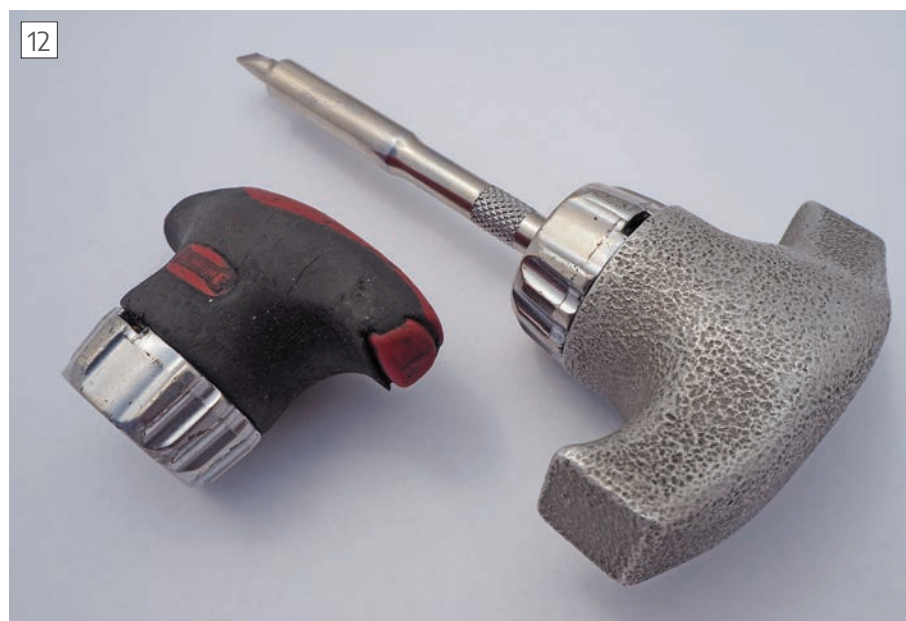
Original Tee handle ratchet and replacement aluminium handle.
