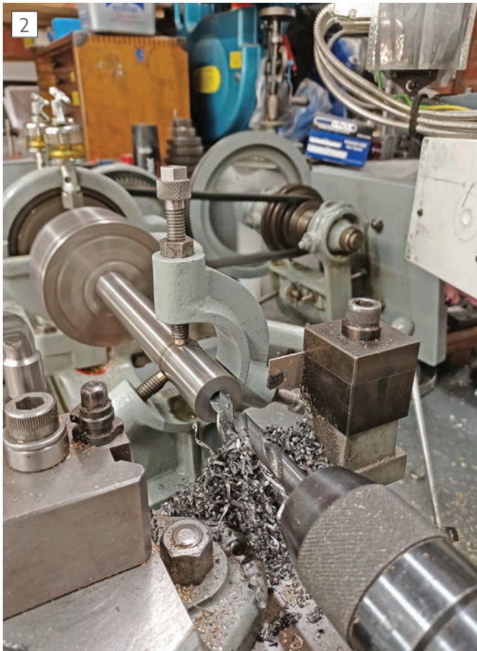
Drilling bar with steady.
