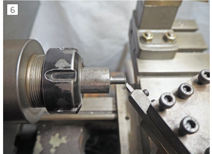
Single point screw cutting the oversize thread.
