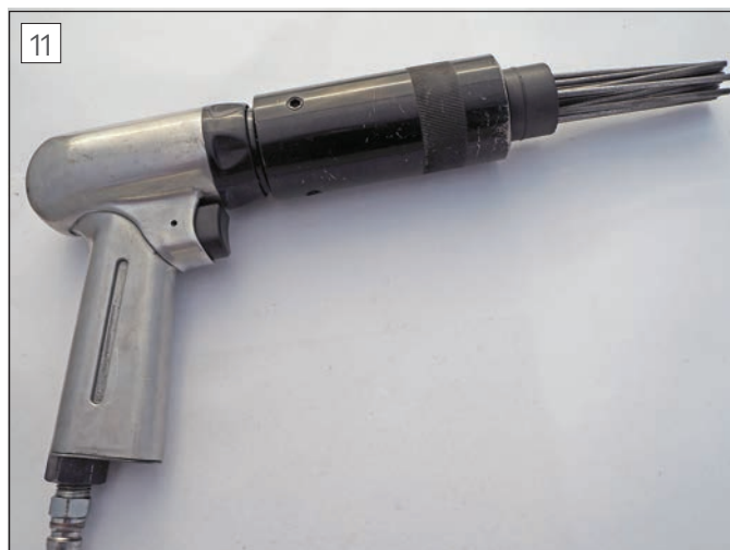
Needle Descaler attachment fitted to an air chisel.
