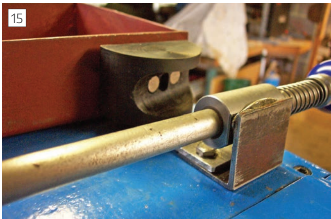
Scalloped section of nylon bar with magnets embedded
