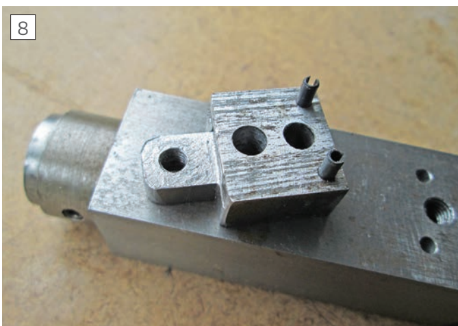
Roll pins fitted to the indexing block
