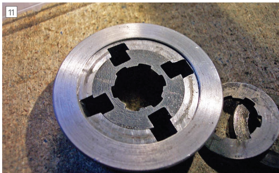
Two-part cruciform fitting, shown misaligned
