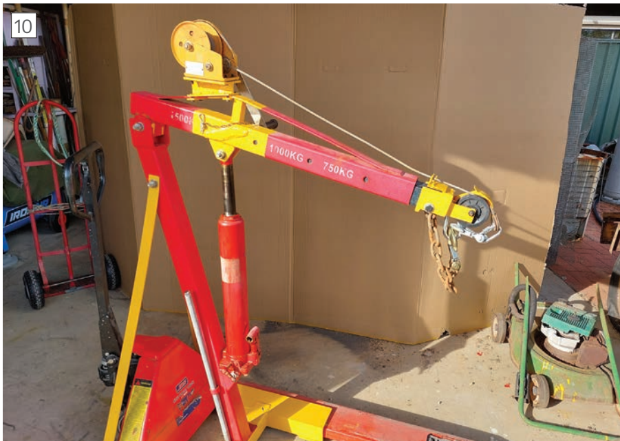
Mobile crane with winch fitted.
