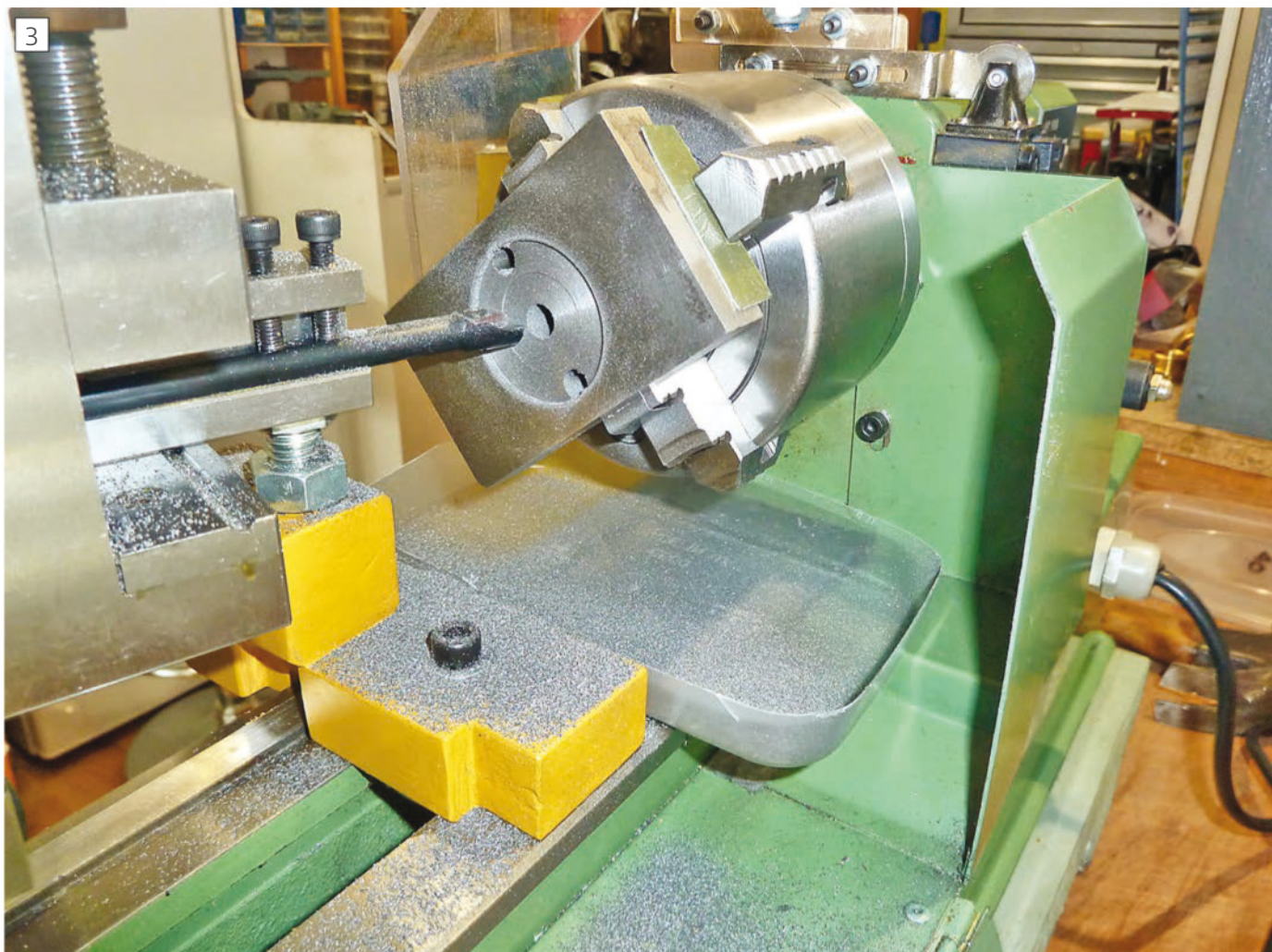
Boring the top slide base
