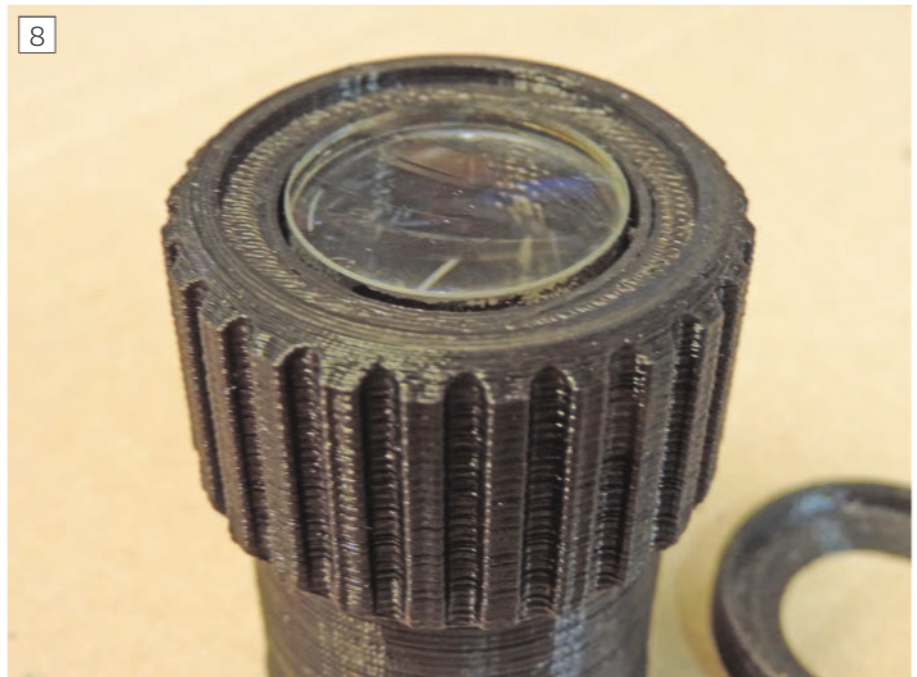
Eyecup 3D printed using flexible TPU.
