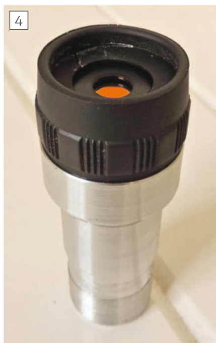
Workshop-made lens with metal body and reused rubber eyecup.
