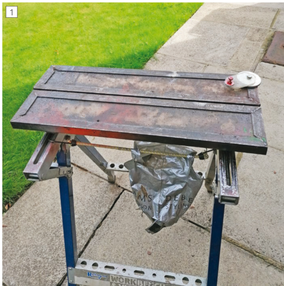
The Original work bench showing the polycarbonate top and angle iron surround.
