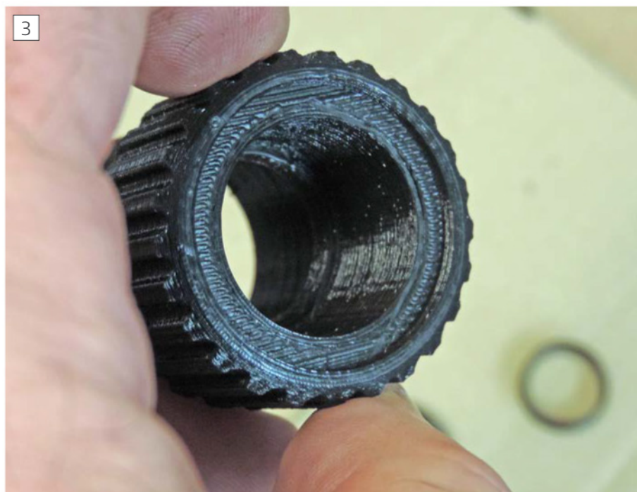
A 3D printed lens bod with internal ledge.
