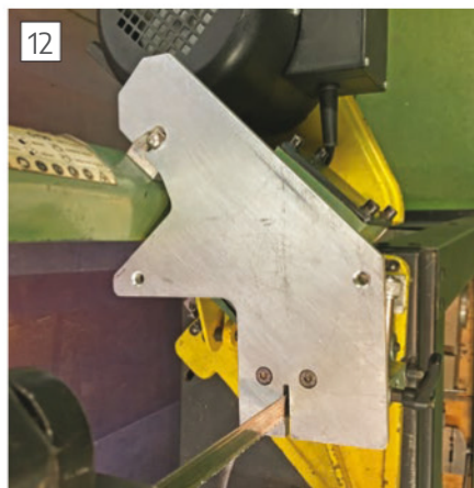
Sub-table in permanent position
