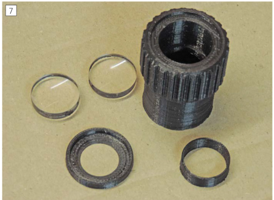
Parts for a Plossl eyepiece.
