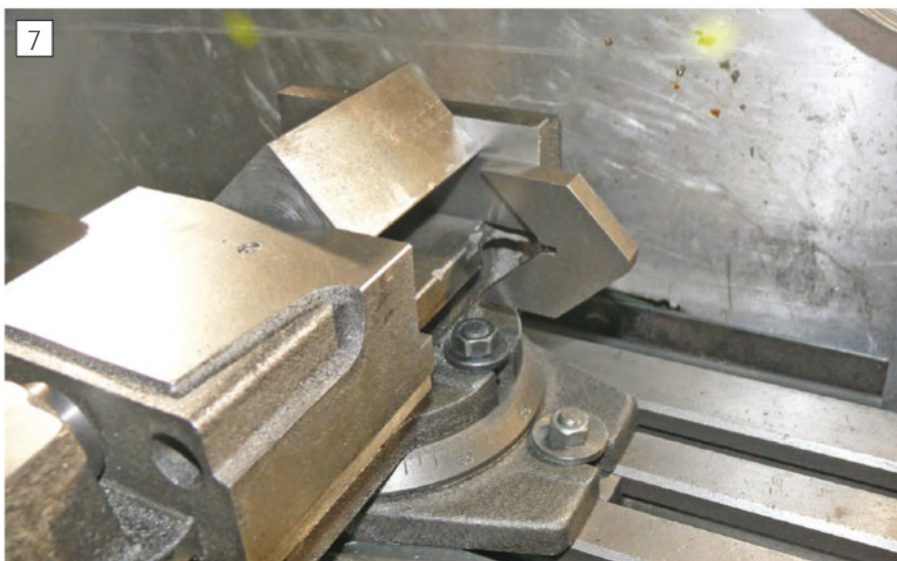
Setting the block in the milling vice.
