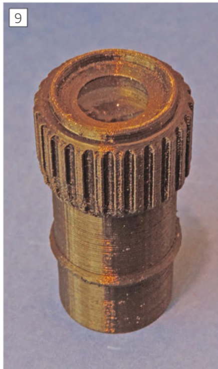
Eyepiece with a shoulder at the focal plane.
