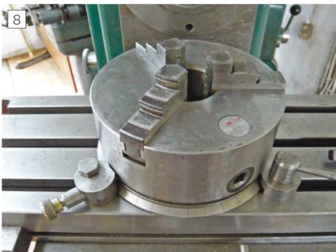
Chuck & clamps mounted
