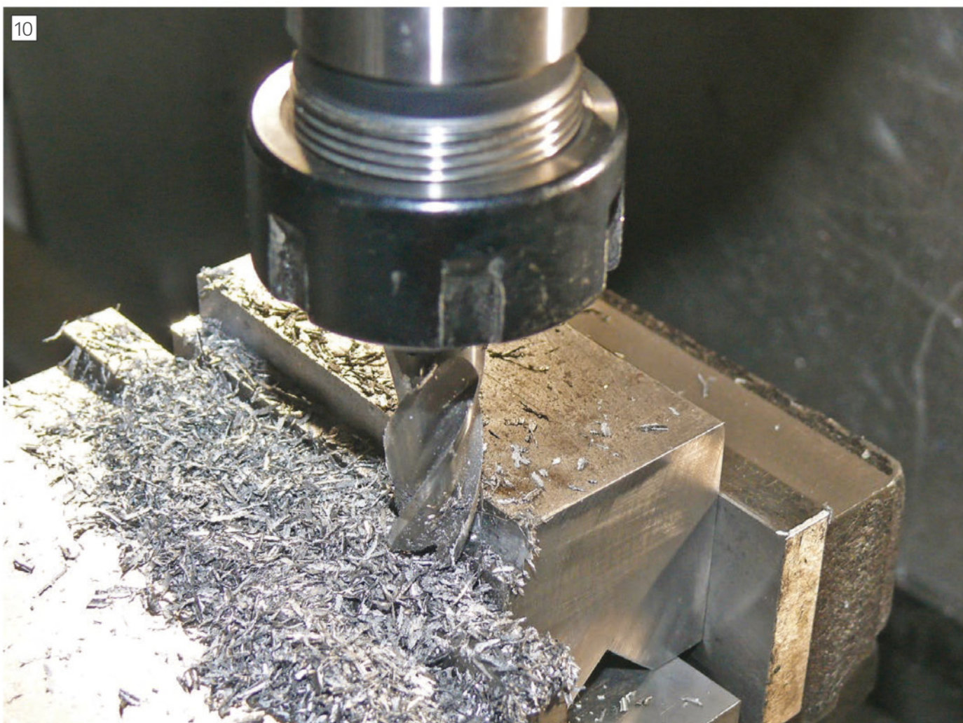
10 Machining the rebates.
