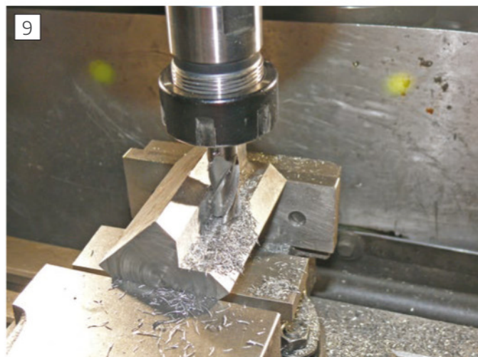
9 Machining the vee.
