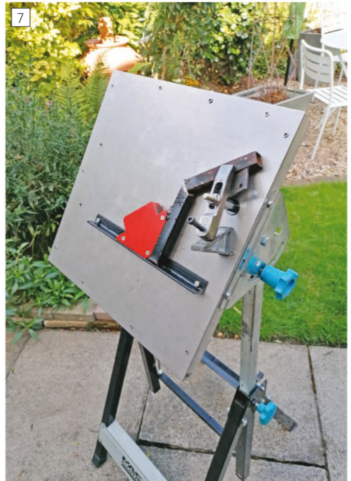
A sample of scrap tubing set up for welding.
