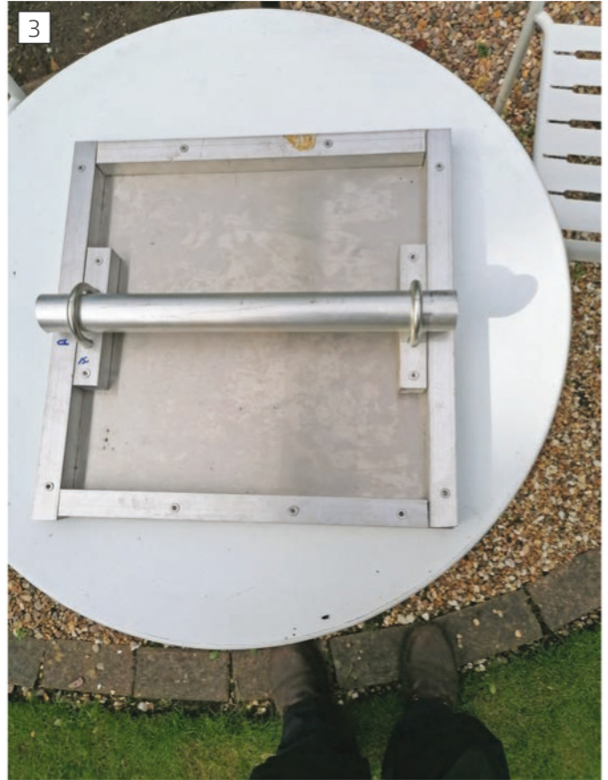
The intended pivot fixture for fitting to the builders trestle.
