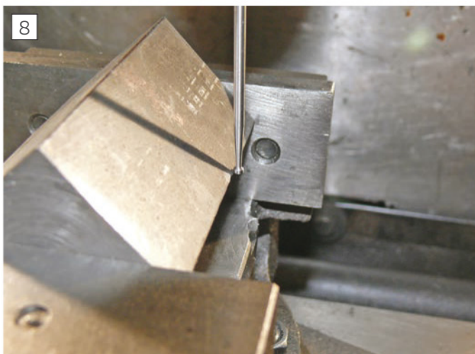
8 Finding the edge with a wiggler.
