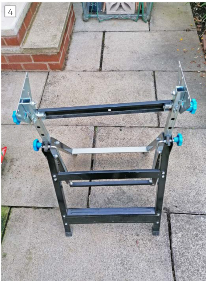
The leg structure of the commercial produced bench/vice with the top removed.
