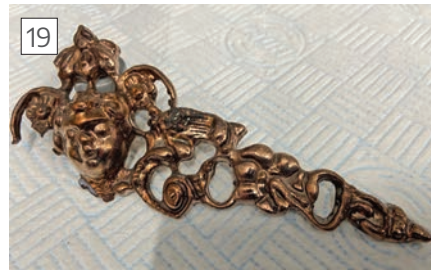
Bronze sample part showing plating burns
