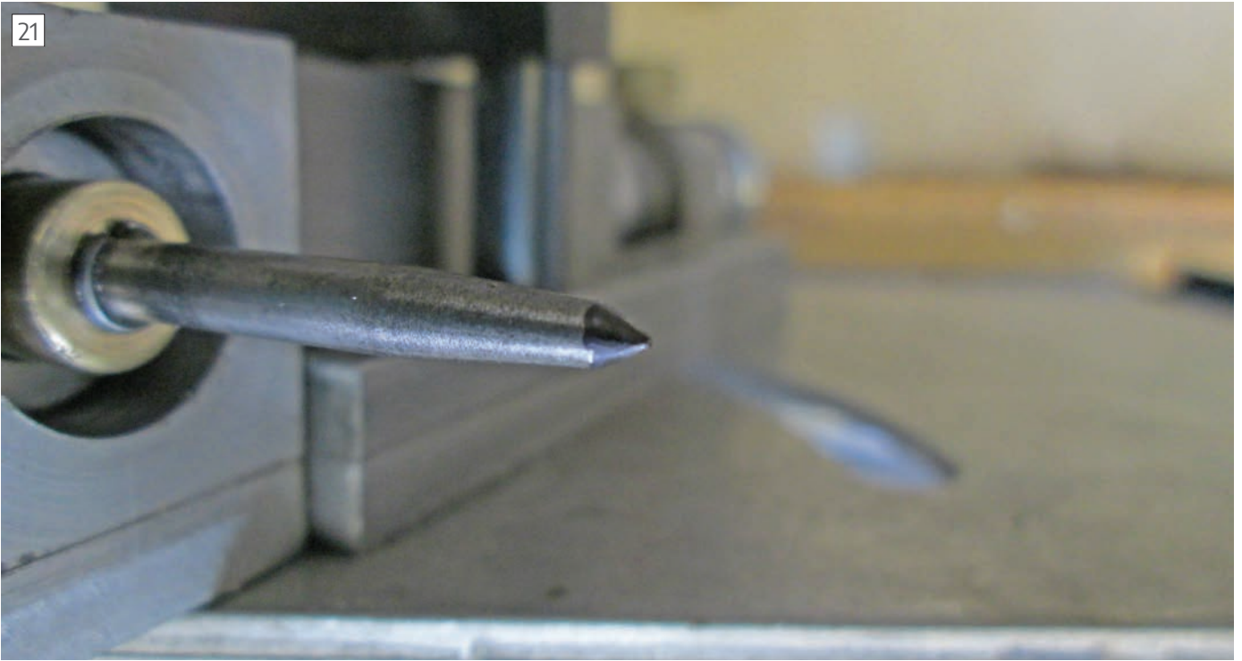
Blacked centre punch point ready for initial grind.
