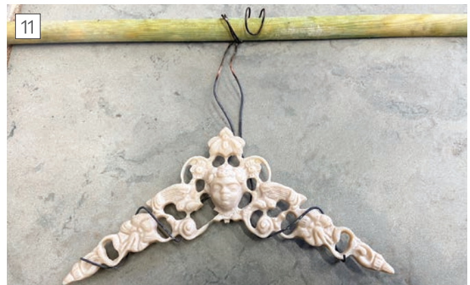
Example of copper support cradle for Cathode, during plating
