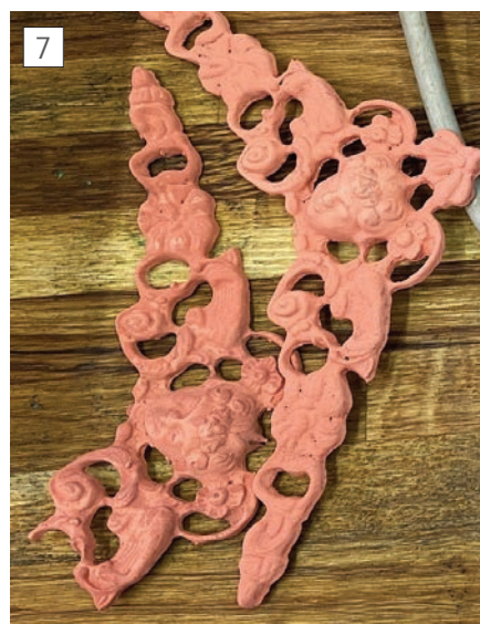
Flash coating of copper on Zinc Primer
