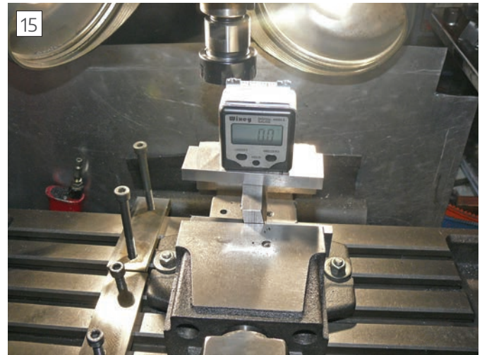
Milling the second 12 degree face
