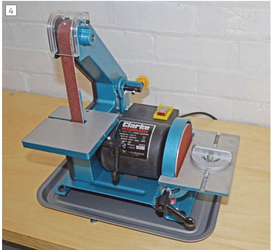
This popular belt sander has a 25mm wide belt as well as a 100mm abrasive faced wheel.
