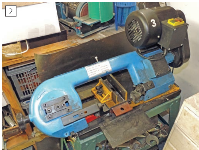
A metal cutting bandsaw can make projects that require big chunks of metal to be cut to size achievable.
