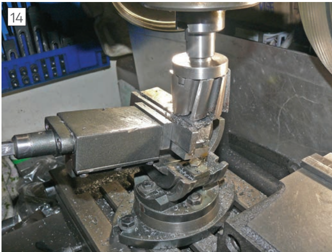
Milling a 12 degree face
