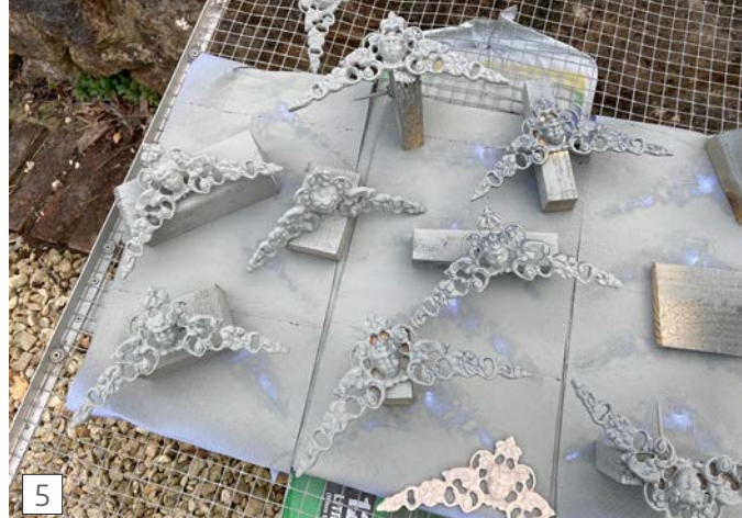
The 3D printed clock spandrels sprayed with Zinc Primer
