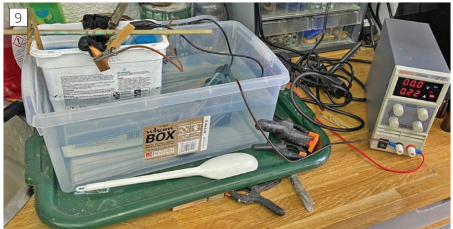
Copper Electroplating set up.
