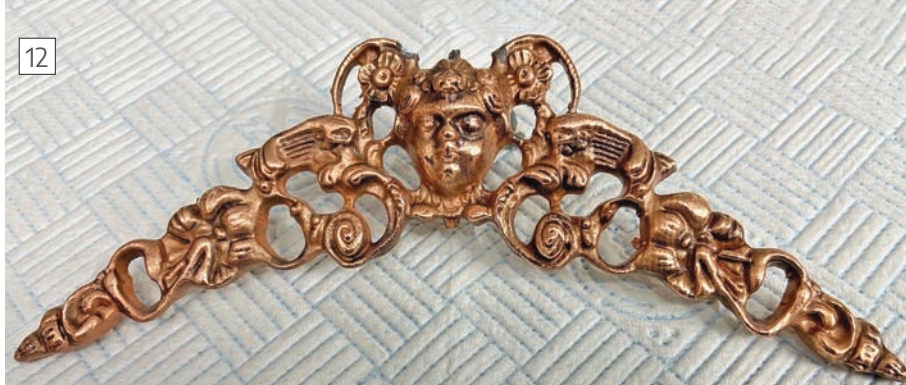
Copper plated spandrel polished by polishing mop
