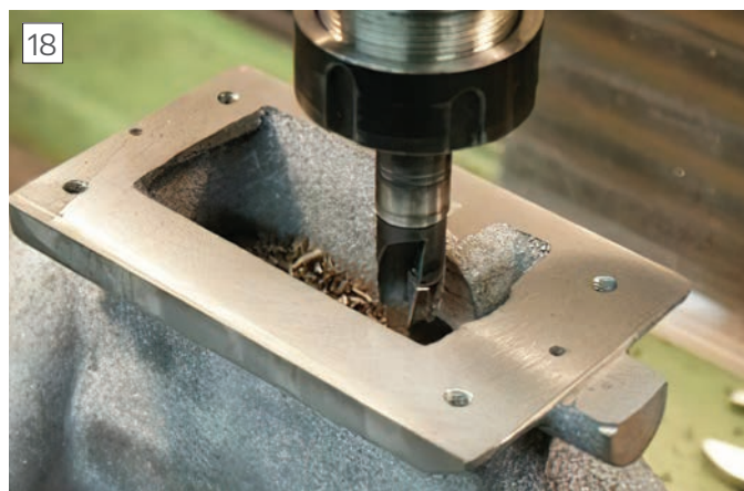
Milling the inside faces of the bosses.
