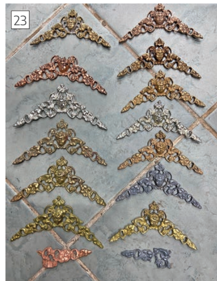
Results of my trials, the bottom left-hand corner was the original cast brass spandrel from an antique clock.
