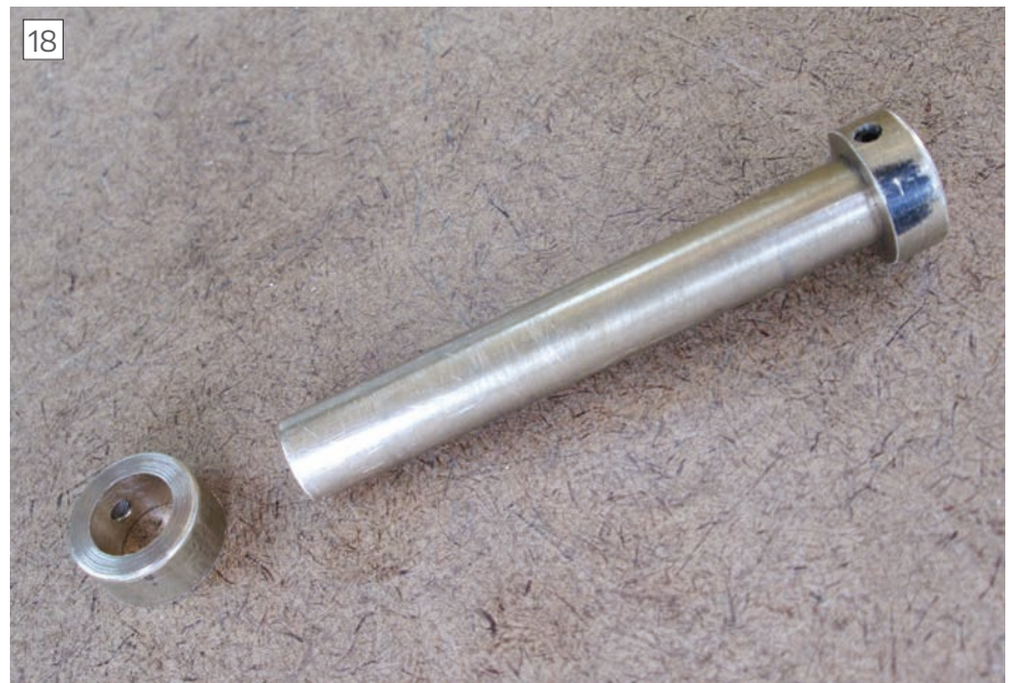
Point grinding jig with locating collars.
