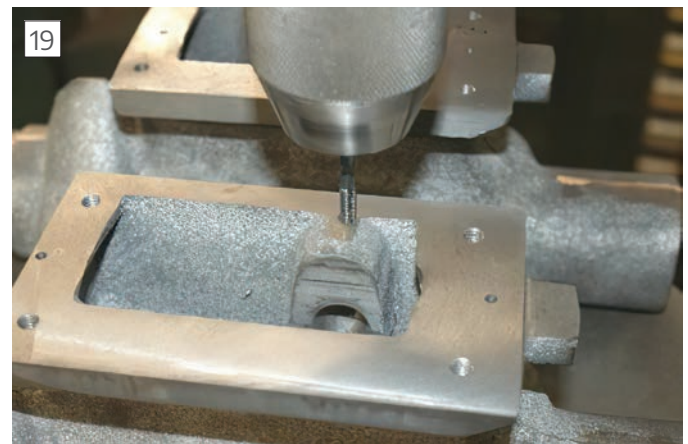
Tapping hole for locating grub screw.
