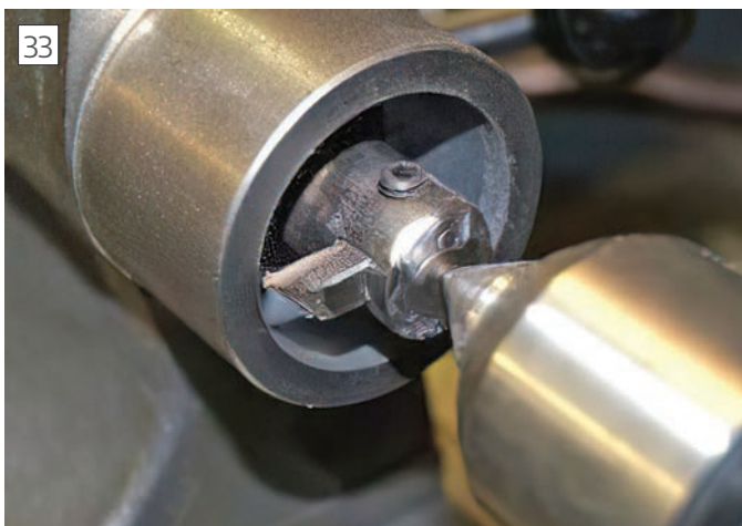
Boring out end for the thread.
