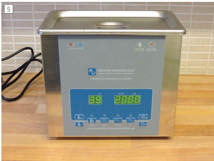
This ultrasonic cleaning tank from machine-DRO has digital control of temperature, intensity and timing.
