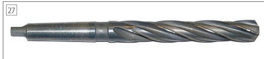
One inch diameter core drill, note the cutting faces are similar to a machine reamer.
