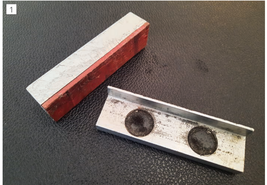
A pair of magnetic soft jaws for a bench vice.
