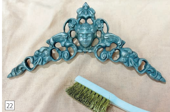
Zinc 3d part polished with brass wire brush
