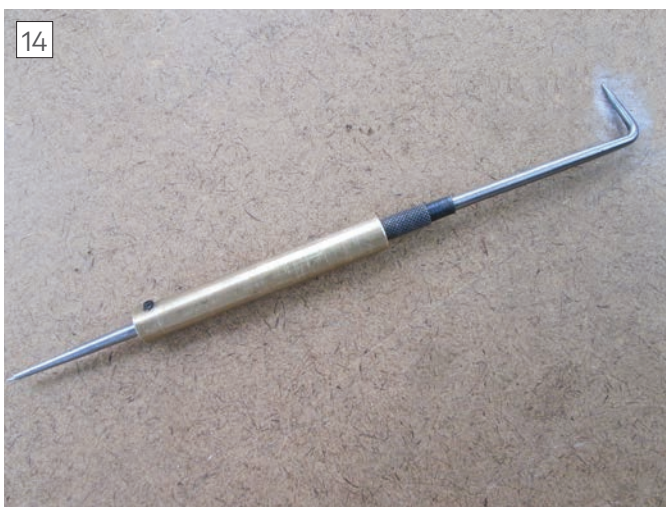
Scriber mounted in grinding jig.
