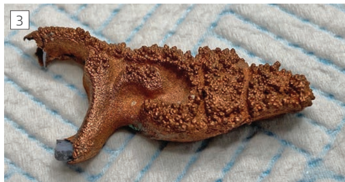
Example of dendrites and uneven copper plating.
