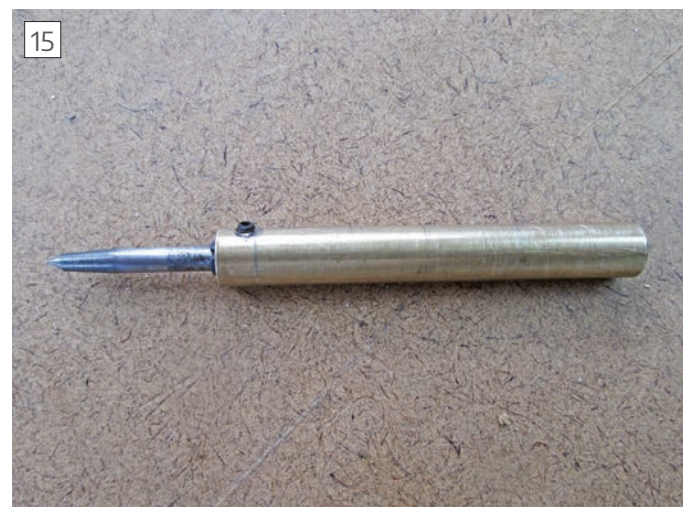
Centre punch point mounted in grinding jig.
