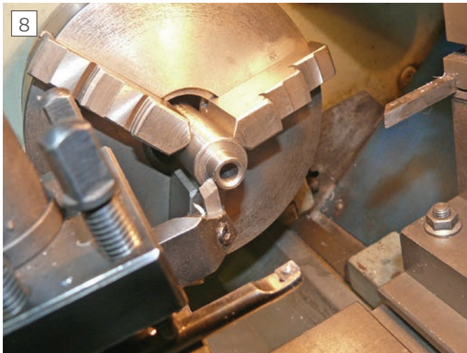
Turning the pillars for the vice alignment fixture
