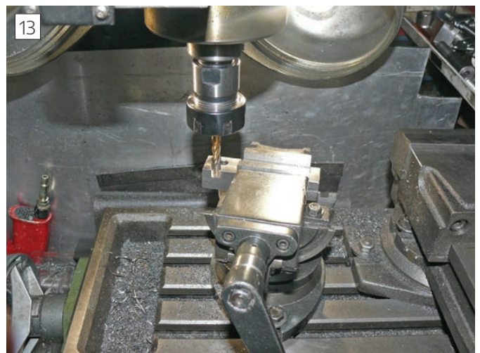
Cutting the tool slot in the final toolholder
