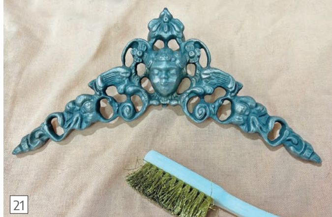
Zinc plated 3d printed clock spandrel
