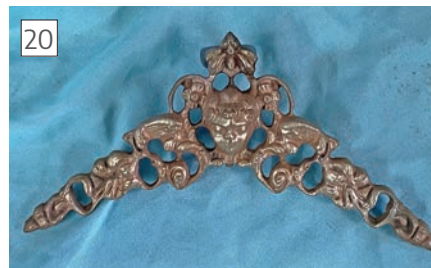
3D printed clock spandrel Brass electroplated
