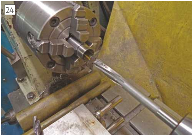
Reaming 10 mm after boring to 9.5mm
