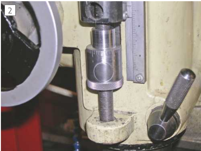
New stop installed on the mill
