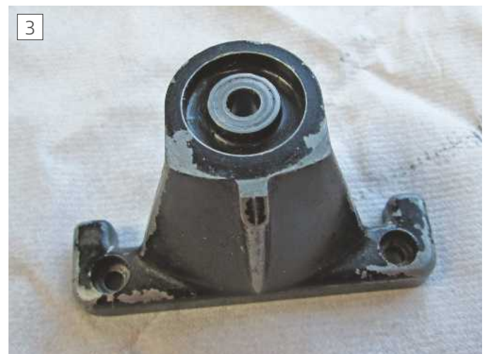
Outer thrust face of the casting showing wear
