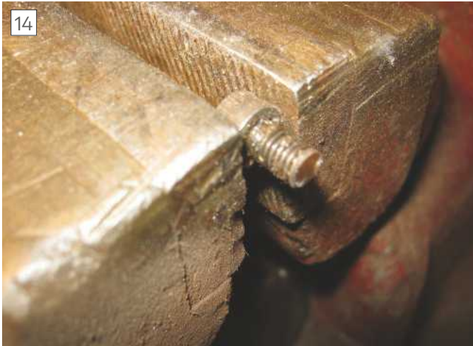
After cutting the screw to the correct length.
