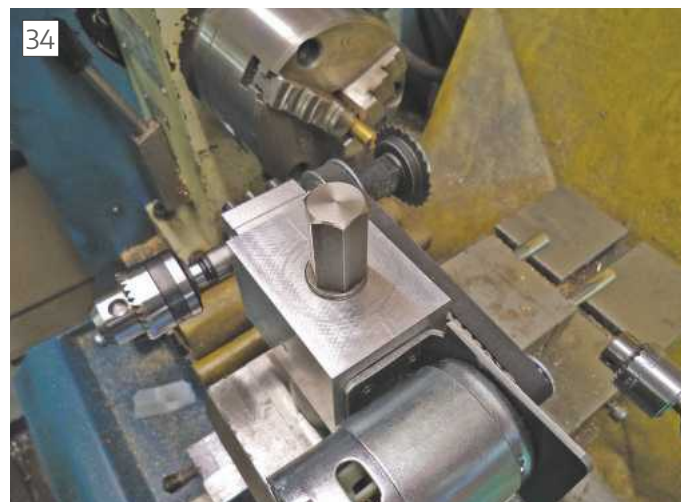
Set up for cutting screw driver slot
