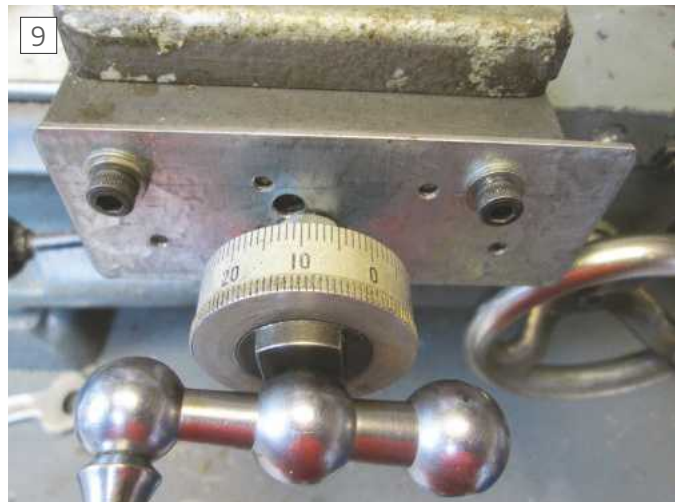
Temporary support plate assembled ready for lathe operation
