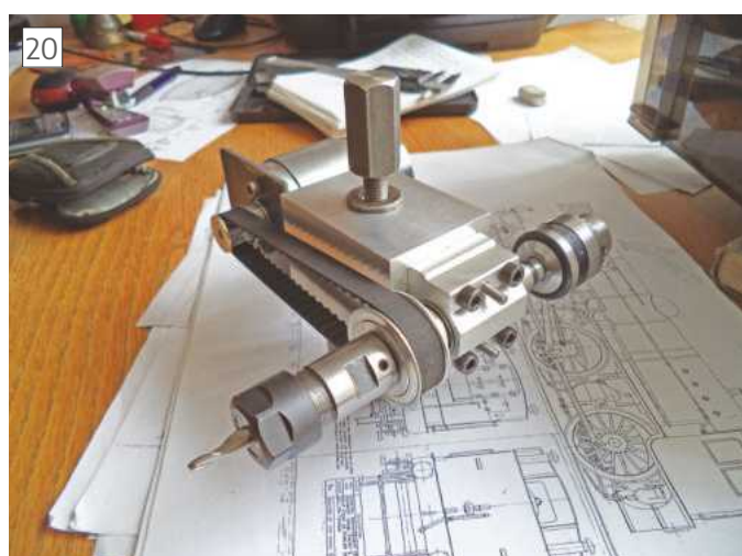
20 Completed Universal Tool Post Fixture
