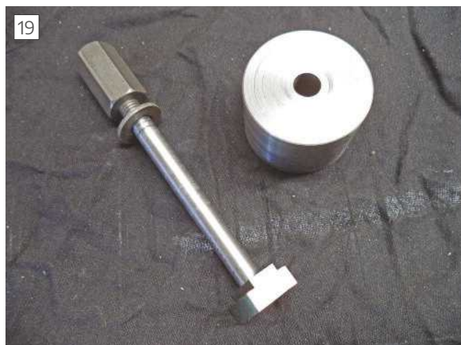
19 Completed tool post clamp and Riser Block
