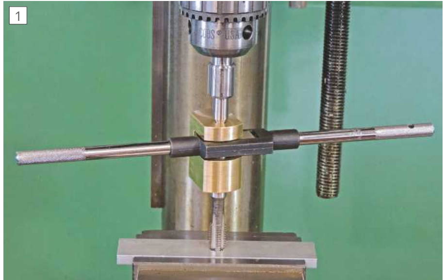
A holder in use in a mill/drill.
