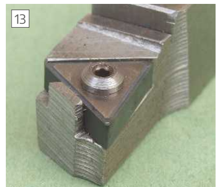
Holder for triangular tip, note tab to give restraint along two sides.
