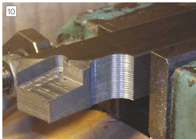
Roughing out surface 9.
