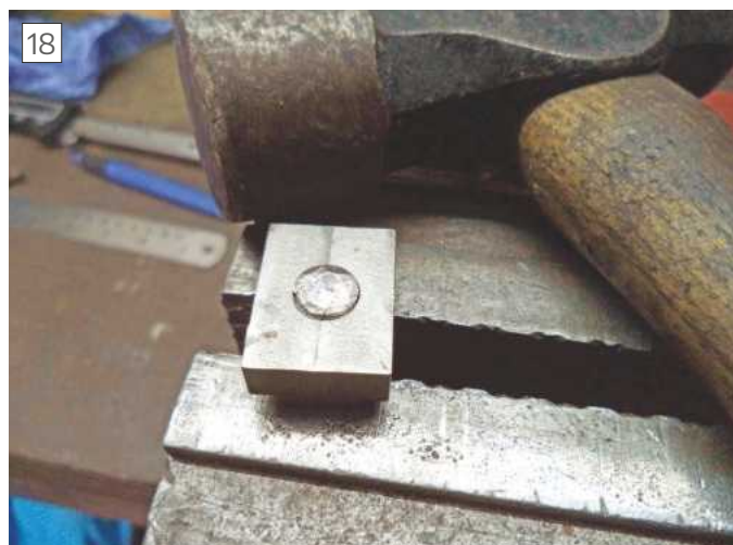
18 Riveting T nut to Bolt
