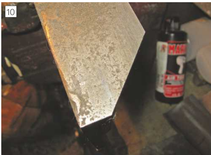
Backing after the angles were cut.
