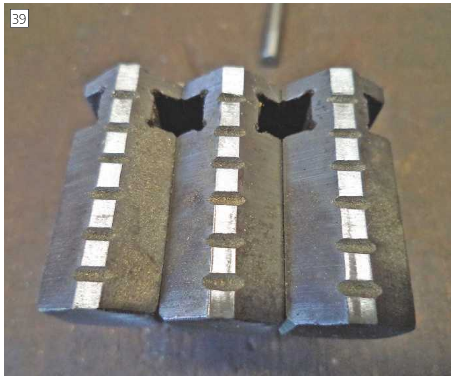
39 Worn Bell Mouthed chuck jaws ground true
