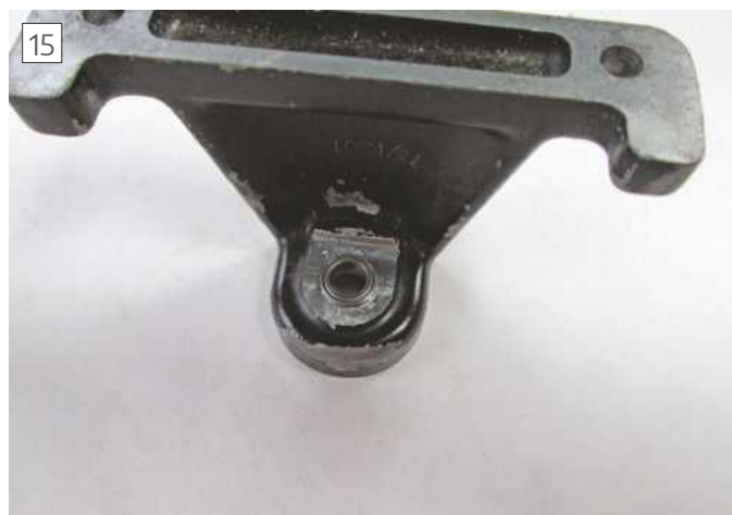
Trial assembly showing the partial fit of the ball bearing and that the milling had not been carried out to the mark
