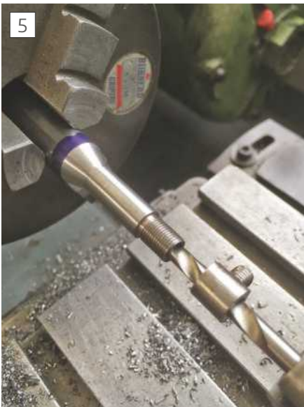
Drilling to depth
