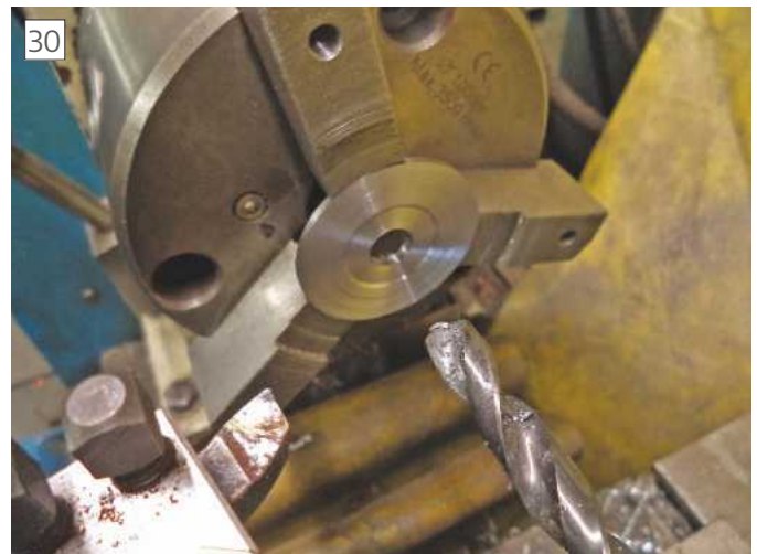
Washer drilled and face using soft jaws
