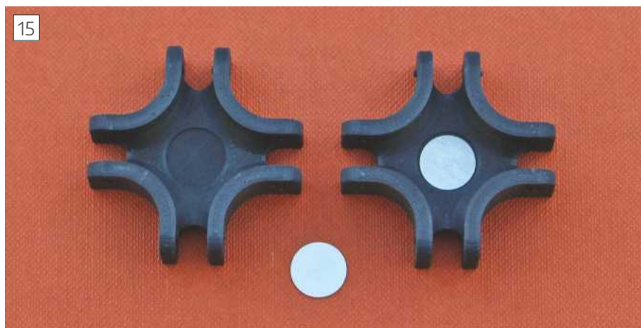
Carbon-nylon composite spider hub printed by Additive-X in a Markforged machine. An aluminium disc is bonded to the centre to act as a hard bearing plate for the ends of the spider arms.
