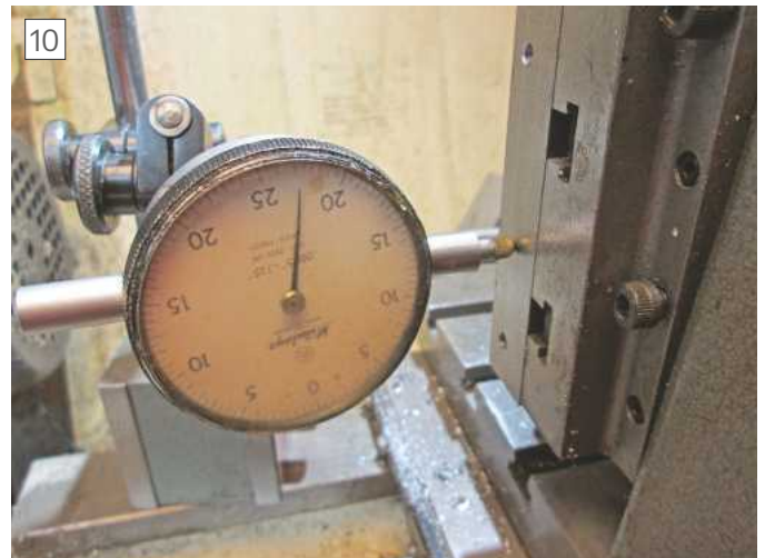
Utilising a clock gauge to set the job carrier vertical
