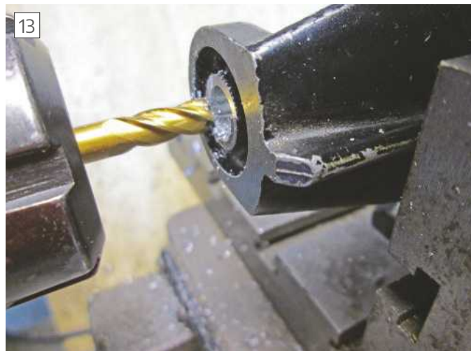
Milling the outside needle thrust bearing recess
