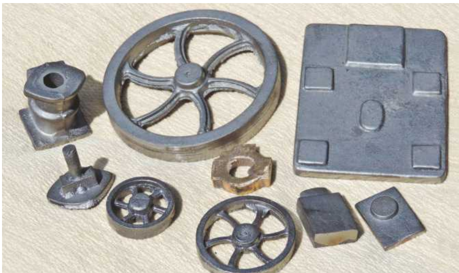
A set of castings from Blackgates Models for the Norden steam engine, mostly in cast iron but including a bronze eccentric strap.
