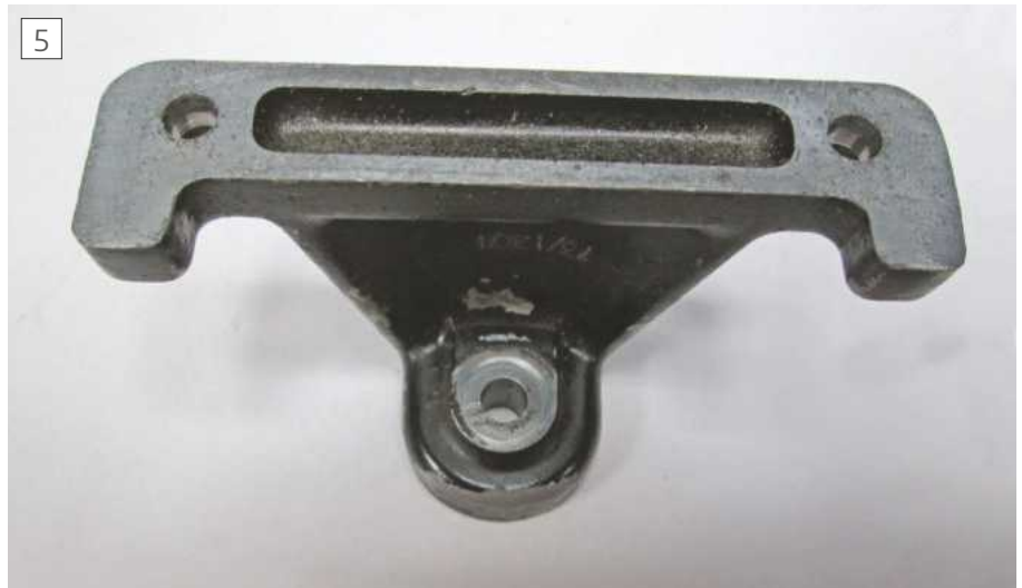
Inner face of the casting showing wear
