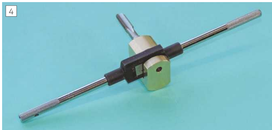
The bar wrench and a tap fitted into a holder.
