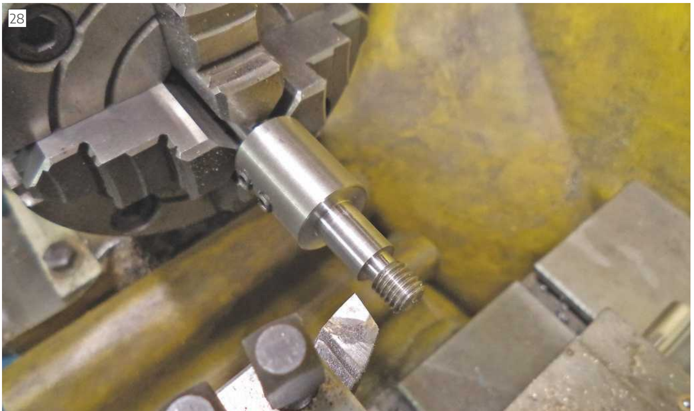
Arbour held on spindle for turning down to 8mm
