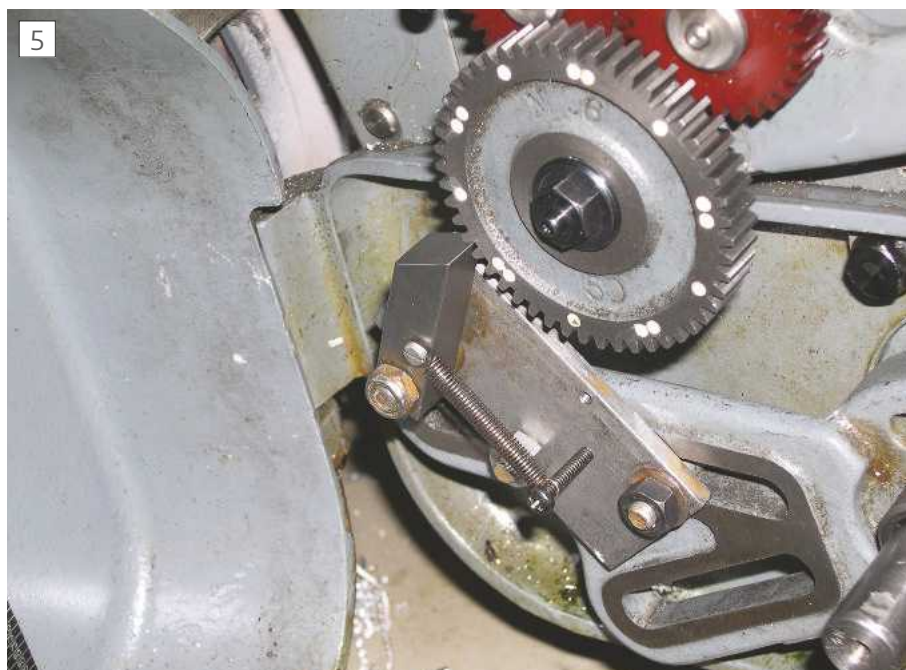
The indexing setup for graduating
