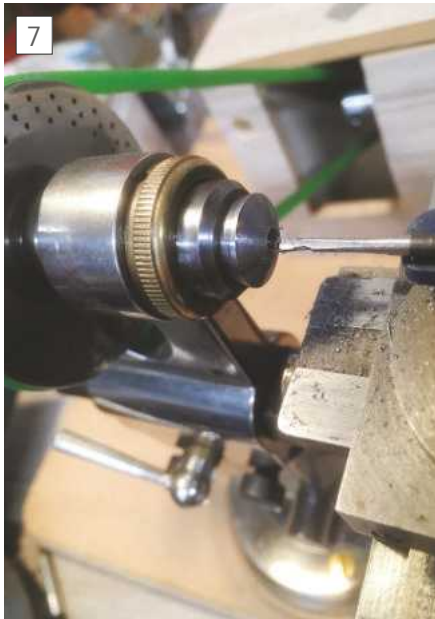
Boring to size
