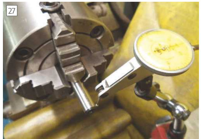
Clocking spare spindle true in four jaw chuck
