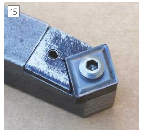
Simple tool holder using a shaped plate to register the tip position.
