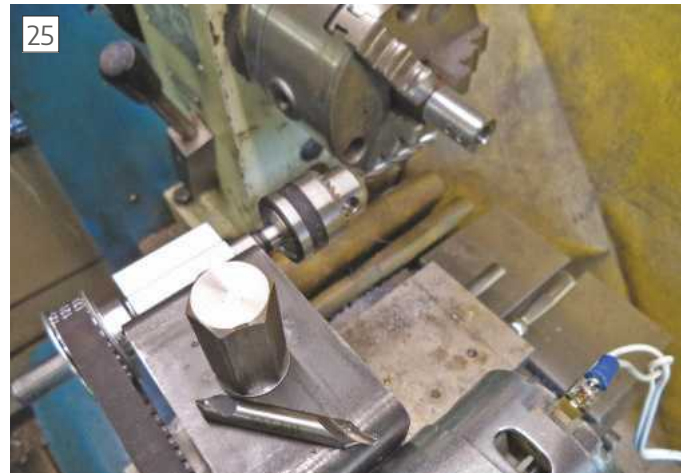
Using Fixture for the first time to cross drill for grub screws
