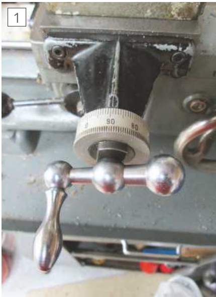
Cross slide leadscrew casting – the subject of the machining exercise
