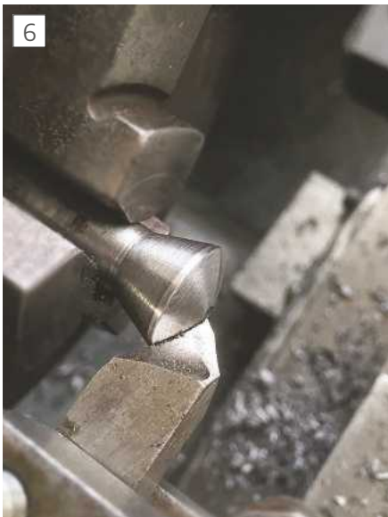
Shaping the face
