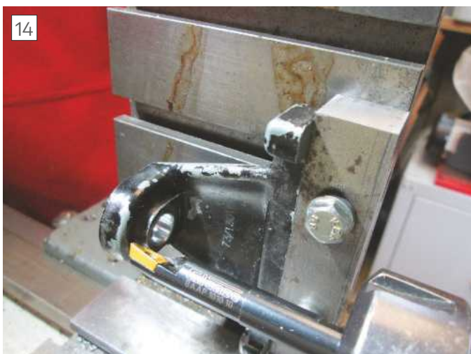
Milling the inside needle thrust bearing recess
