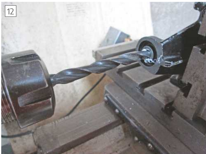
Opening the hole in the casting ready for reaming to final size
