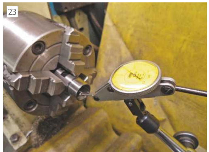
Clocking taper in Collet Holder True
