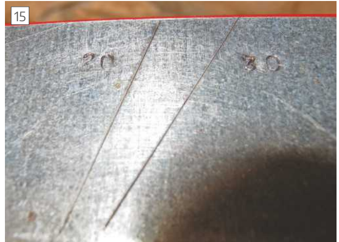
The Filing guide with angles showing.
