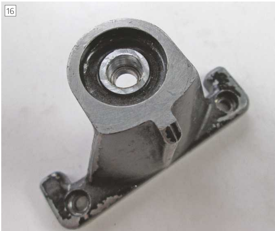
Work finished, ball bearing inserted, and ready for final assembly
