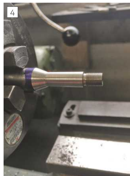
Machined and threaded collet
