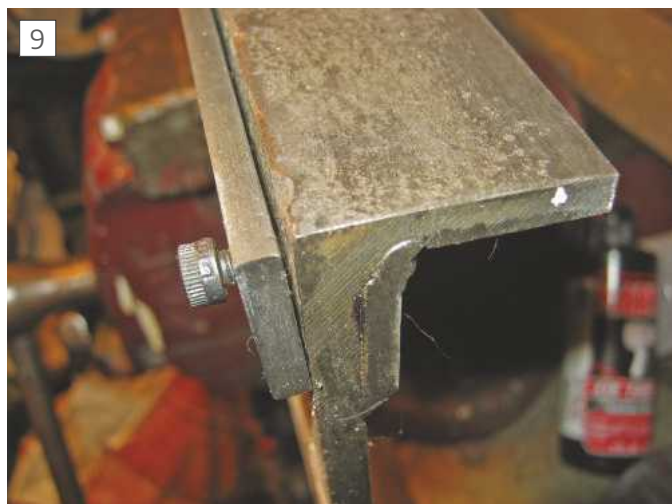
The reduced backing top end at 35mm.
