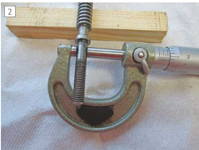
Checking the diameter of the leadscrew shaft
