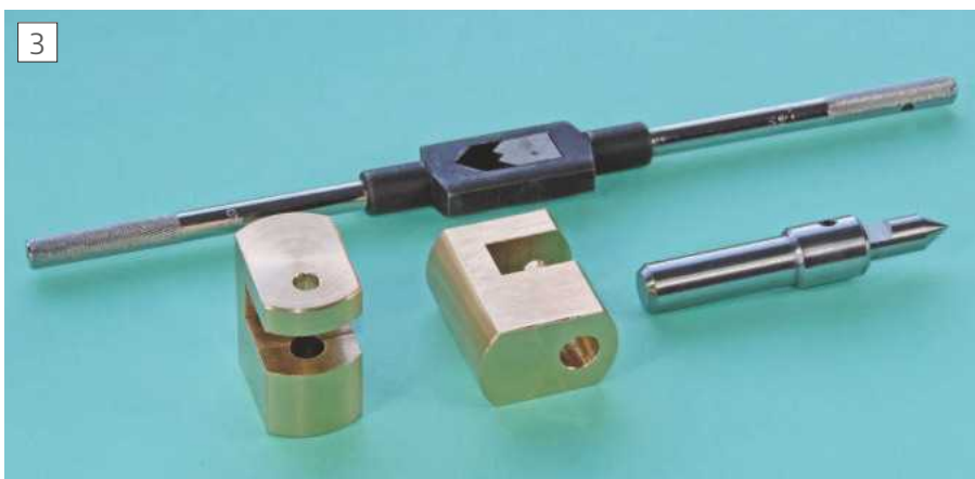
Two holders, for M8 and M10 taps, with a Hall bar type tap wrench and a spring tapping guide.
