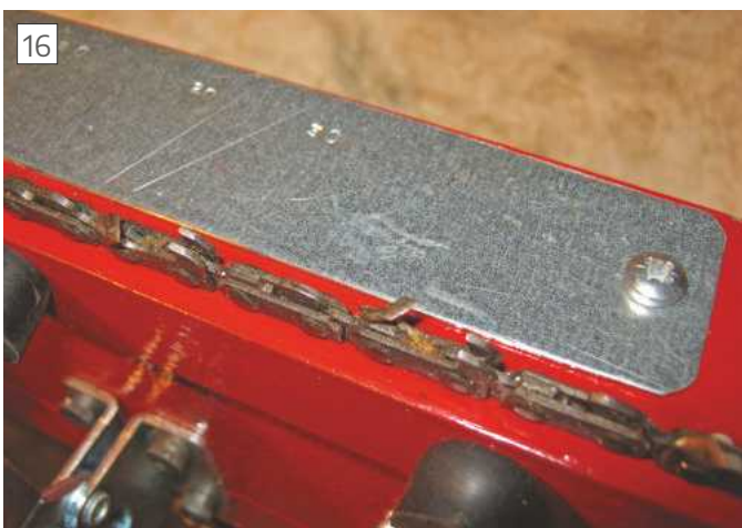
The Filing guide screwed into position.
