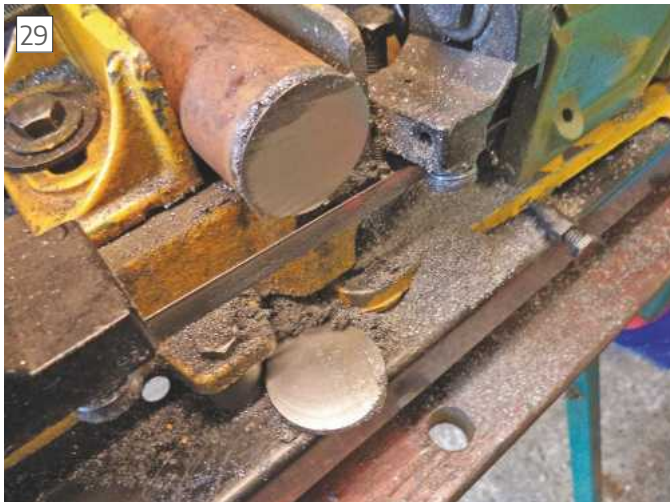
Slice cut off 40 mm diameter bar
