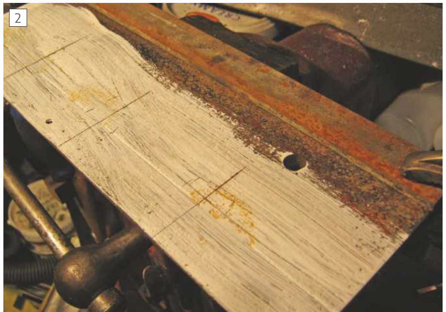
Face of backing with centre lines for clamps.
