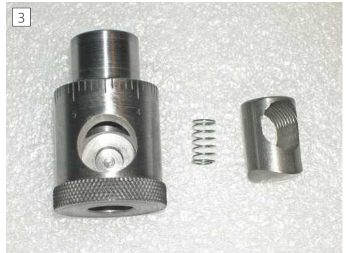
The parts of the new stop
