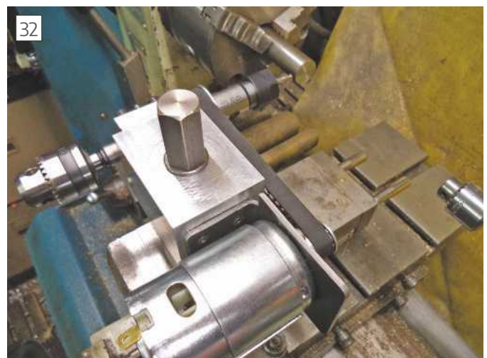
Set up for cutting key way with ER16 Collet holder and 3 mm slot drill
