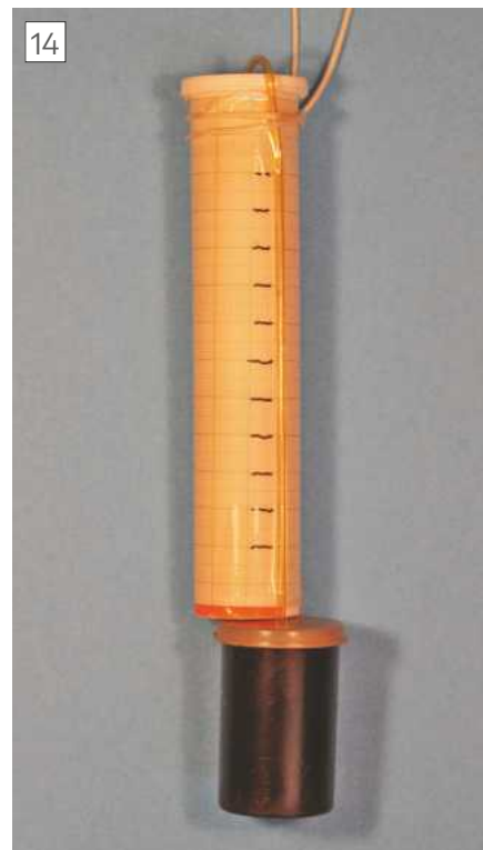
Replica of the capillary-bubbling altimeter. As the unit ascends air expands from the larger reservoir through the narrow tube and bubbles into water contained in the smaller reservoir. During the descent water is drawn up the tube to a level that records the peak altitude. Patent Still Pending.
