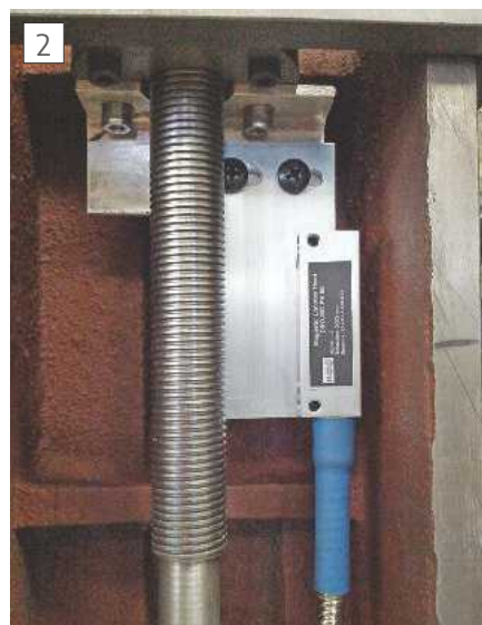
Z-axis, complete encoder mounting.
