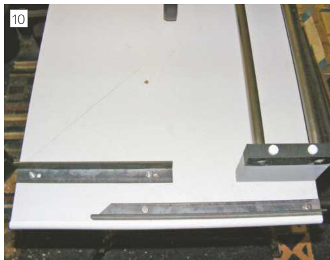
The 90-degree stop fixed to the baseboard.
