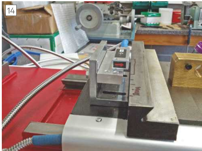
X-axis, trying the MDRO mounting kit.
