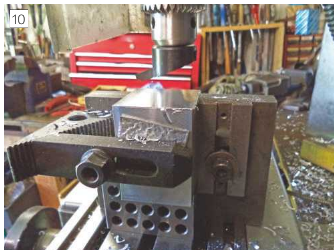
Angle Plate with Parallel used to square block to length
