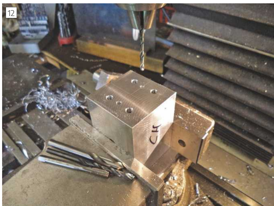
Drilling block for bearing housing; dowel holes ensure spindle is central
