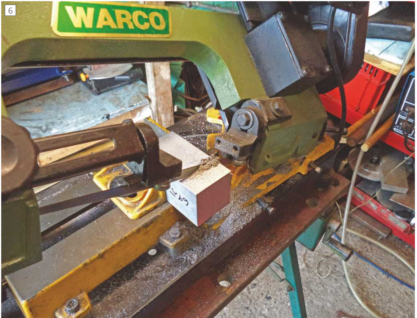
6 Cutting Block to length with Warco Band Saw
