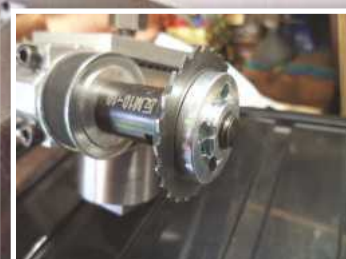
Stewart Hart fits a Universal Tool Post Spindle
