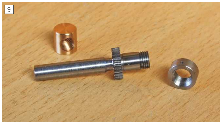
Feedscrew as yet not screwcut, feedscrew nut and locknut.
