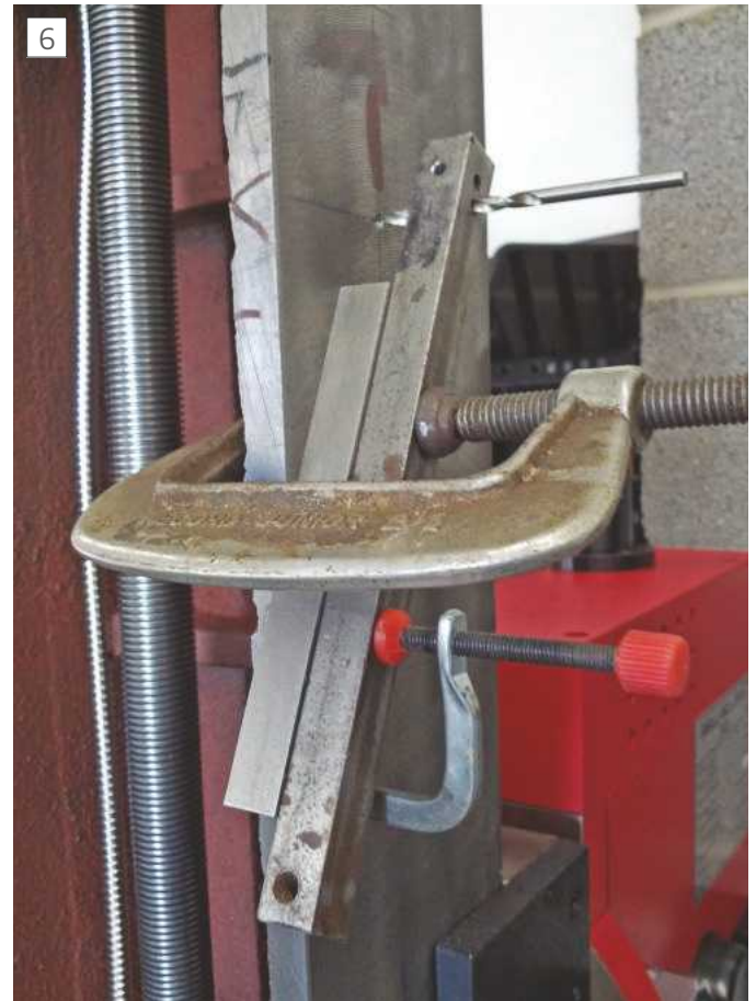
6 Z-axis, improvised drilling jig.
