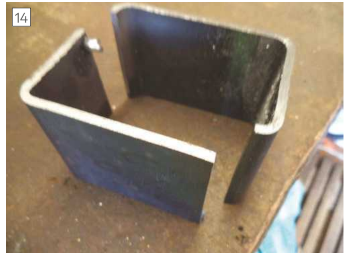
14 Bracket made from box section
