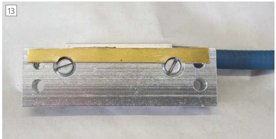
Y-axis, shim to level mounting.
