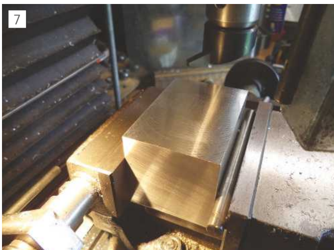
7 Fly cutting block square in Vice; Note use of bar
