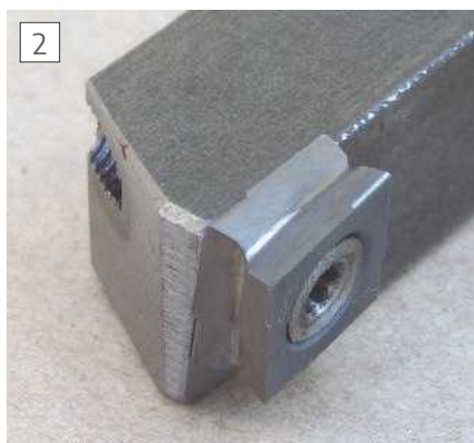
'Knife' tool used to provide eight cutting tips.
