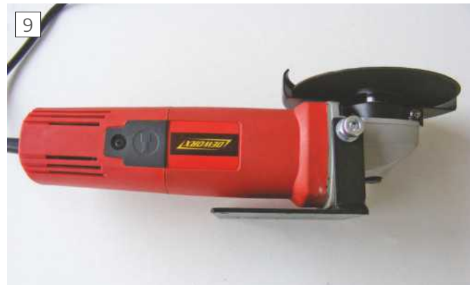
The angle grinder mounted in the bracket.
