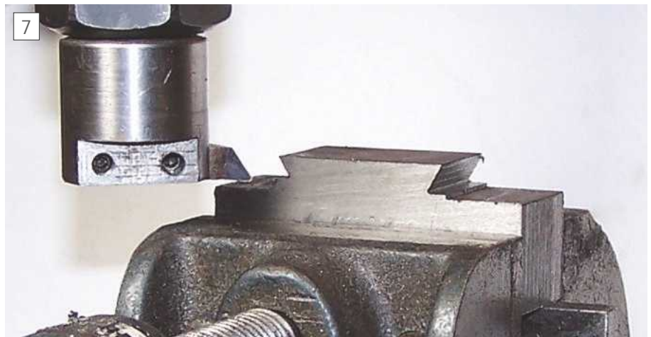
7 Cutting the dovetail vees on a tool holder.
