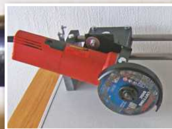
Accurate Angle Grinder cuts with this Sliding Base
