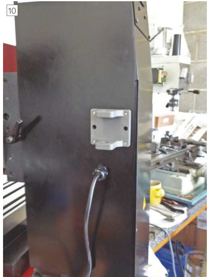
Z-axis, DRO bracket position.
