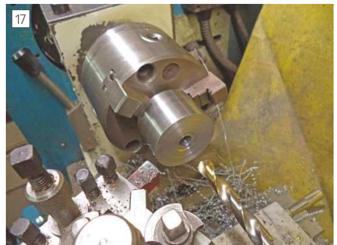
17 Drilling and facing riser block to length
