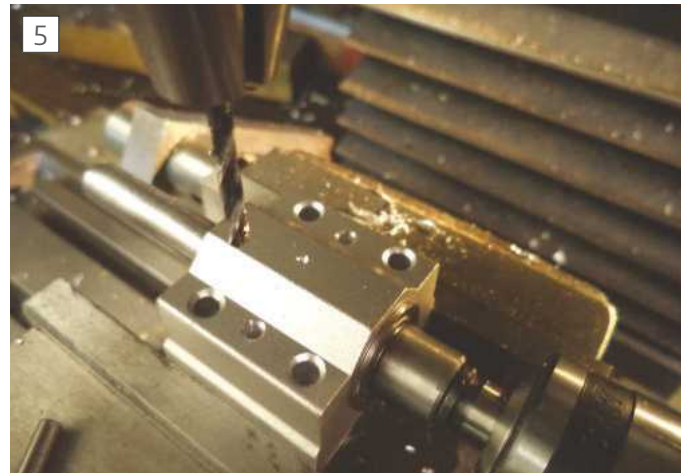
Drilling Dowel Holes
