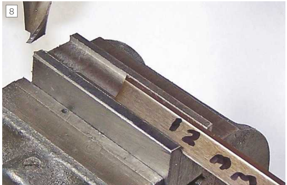
8 Checking the width of the clamping slot using the actual cutoff tool blade.
