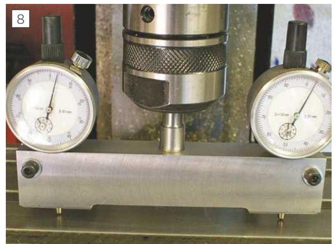
8 Homemade trammel used to set milling head square to table
