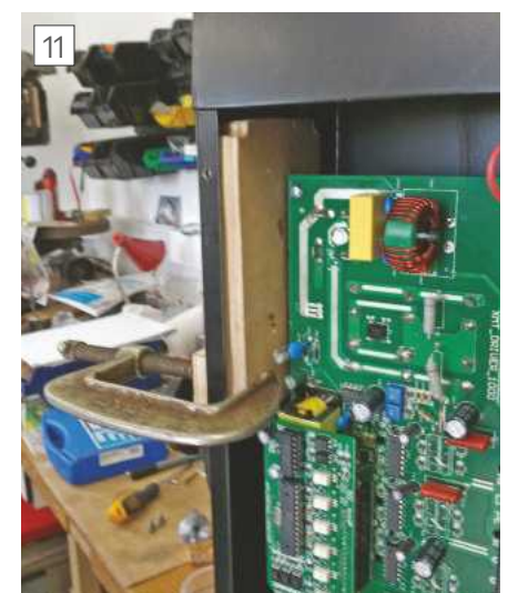
Z-axis, protecting PCB during drilling
