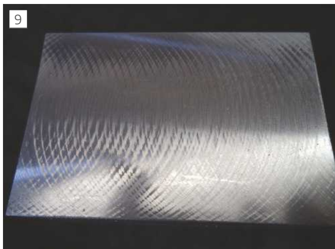
Criss-Cross Witness lines indicating that head is square
