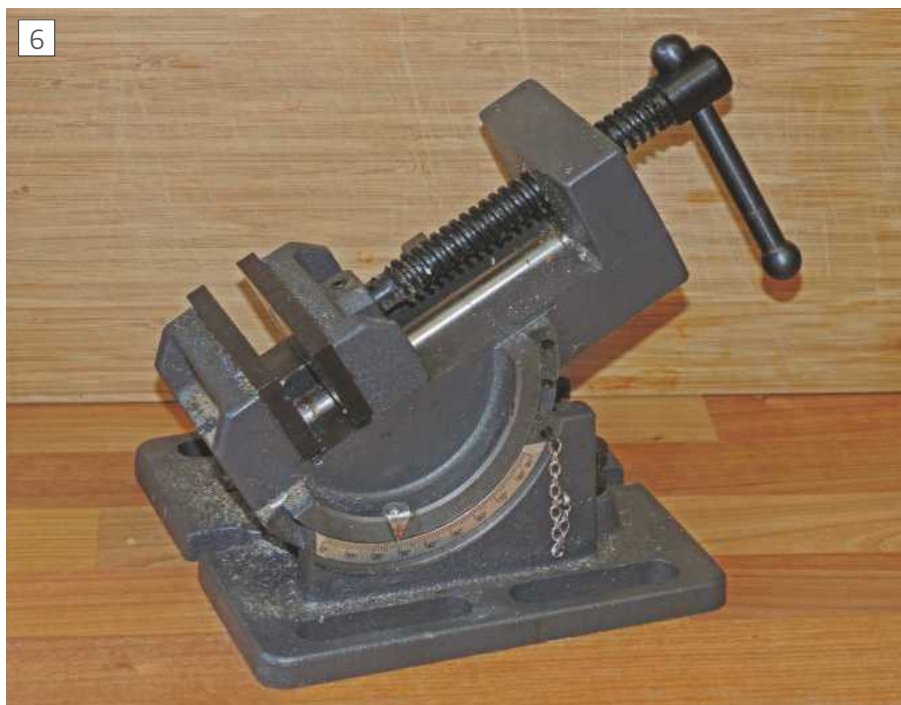
This is the more flexible of the two styles of simple tilting vice.
