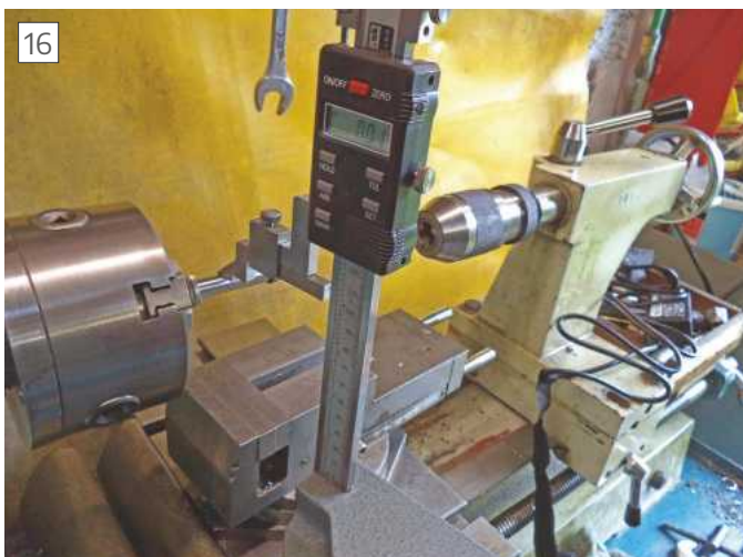
16 Measuring Centre height of lathe
