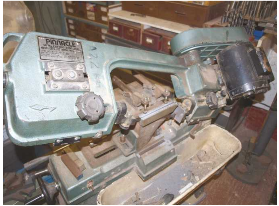
Fixture holding a one-inch tool being cut to half an inch.
