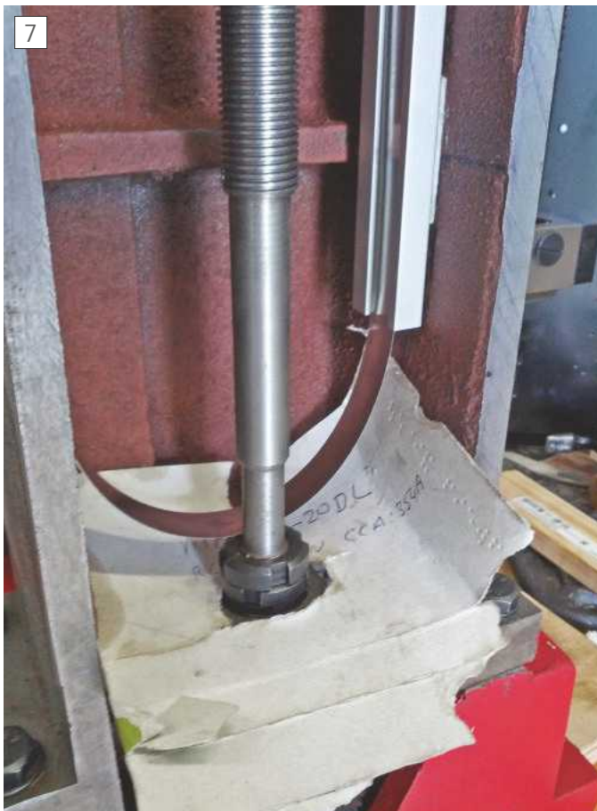
7 Z-axis, fitting cover strip.
