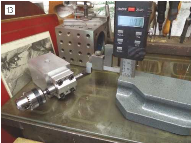
13 Checking Spindle is central using height gauge
