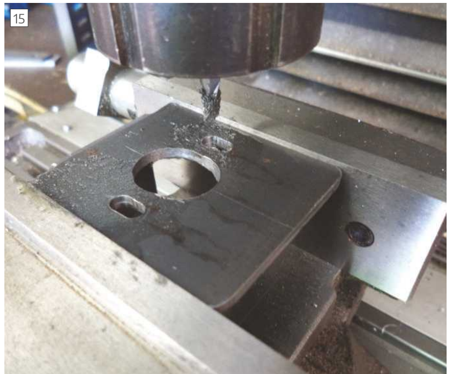
15 Milling Slots for adjustment
