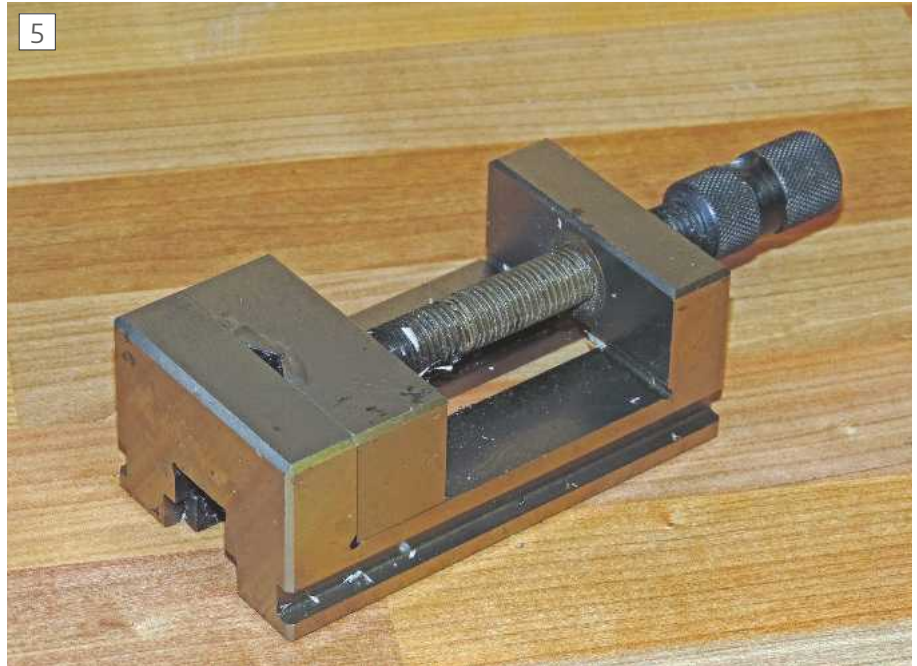
Toolroom vices are typically ground on all sides.
