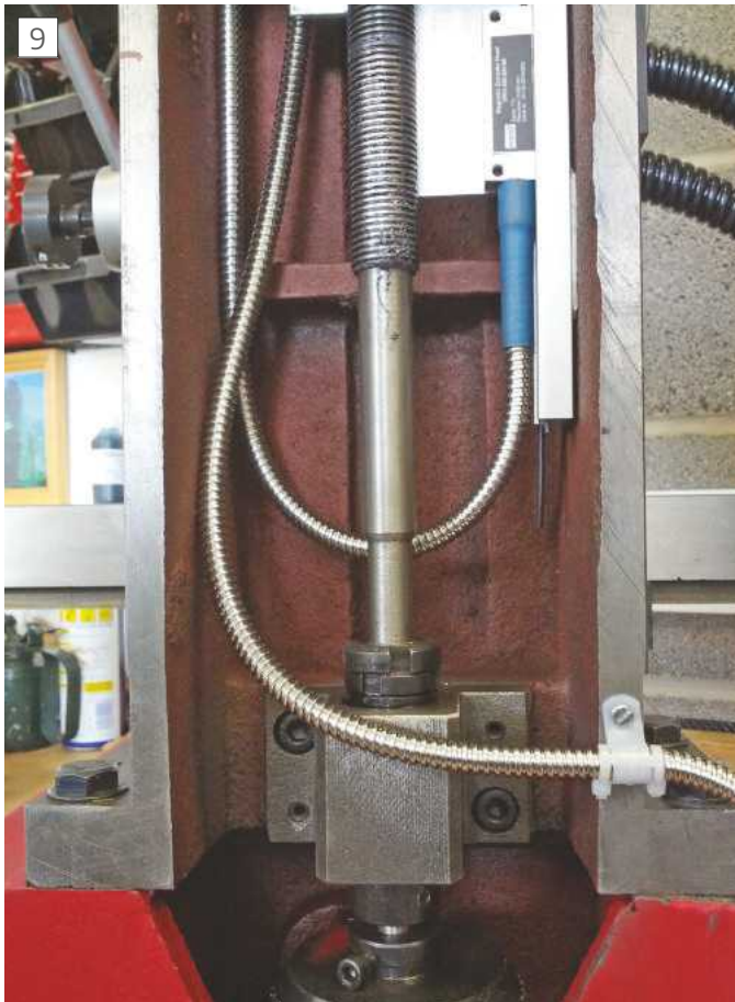
Z-axis, lower cable management.
