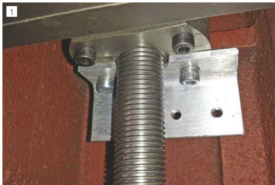
Z-axis, bracket mounting
