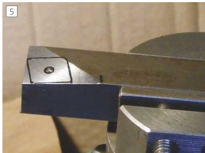
Marking contour of tip.
