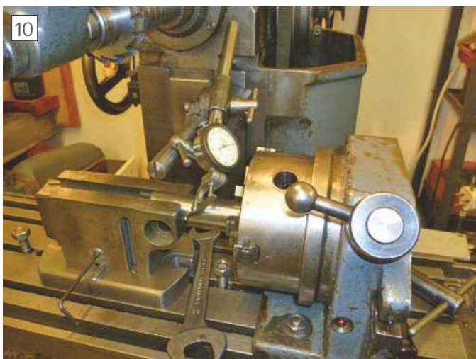
Final horizontal and vertical alignment check
