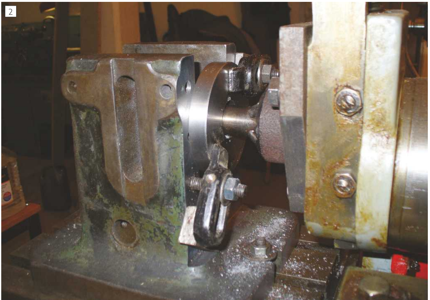
Housing used as slotting support on Alba shaper for cutting internal keyways
