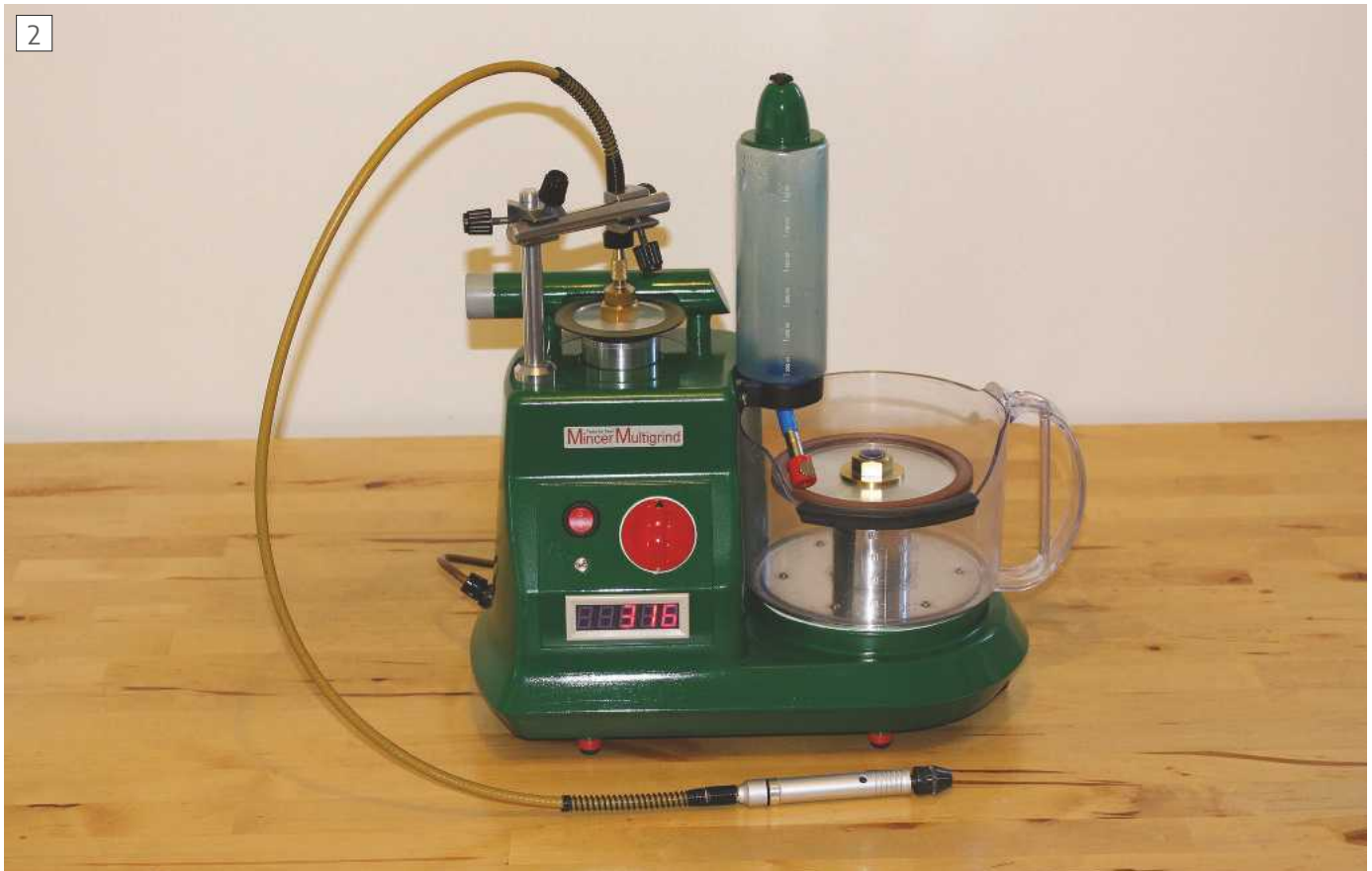
Multigrind – a flexible sharpening system base on a recycled food processor by Mark Noel.
