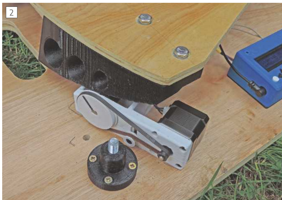
Closeup of an equatorial platform showing a 'sector' with a complex geometry.
