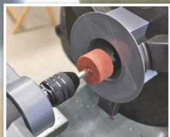
Grinding Chuck Jaws to Restore Accuracy
