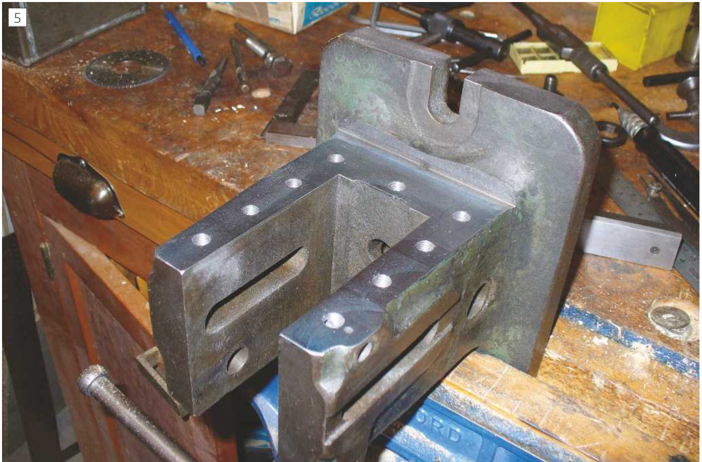
Housing modified as slotting support
