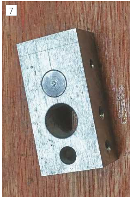
Outer jaw all holes D & T or Reamed
