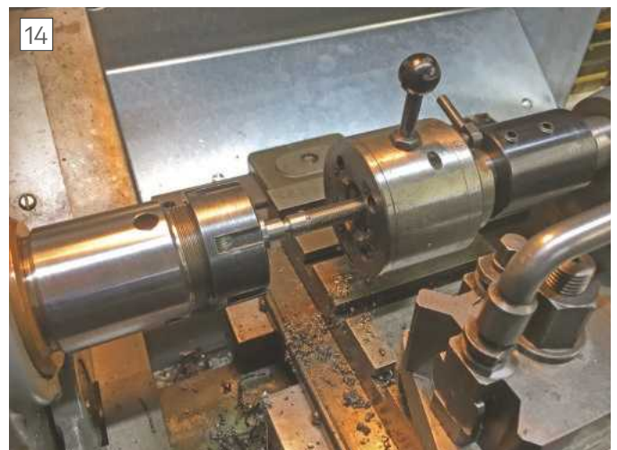
Cutting the thread with die box
