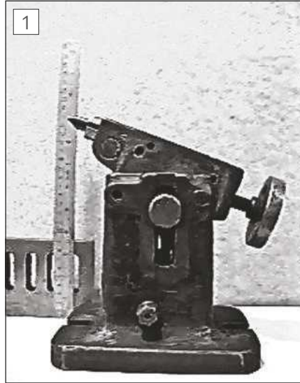
Cincinnati dividing head tailstock in original form showing vertical and angular adjustment
