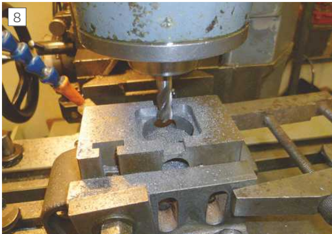
Enlarging recess in base of tailstock barrel assembly to fit alignment bushes
