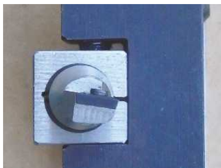
Jacques Maurel makes a tool for internal turning.
