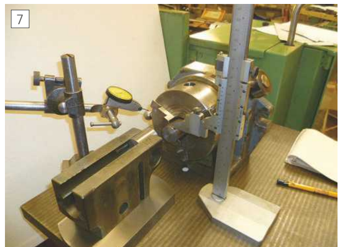
Preliminary checking of centre heights
