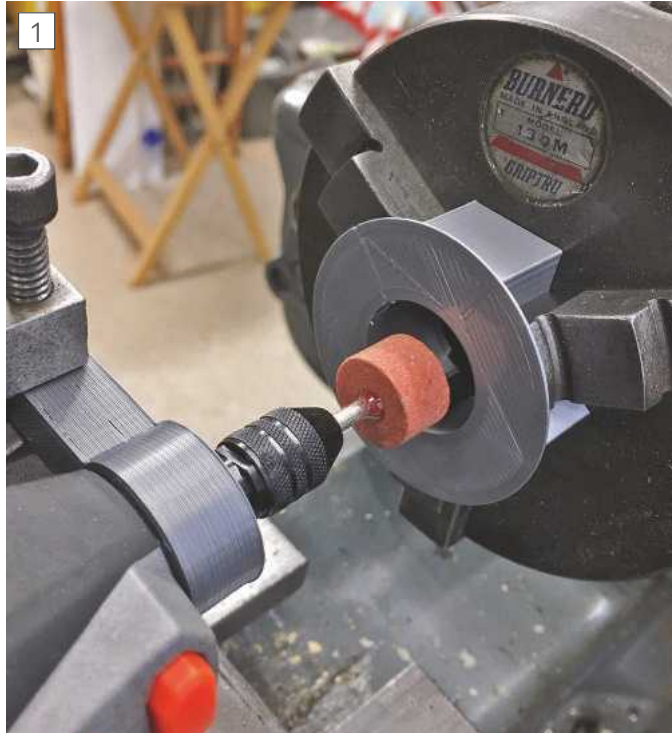
Mini grinder support and chuck jaw jig in action.
