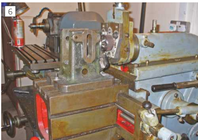
Close up of housing being used for slotting keyways on shaper (minus clapper box)
