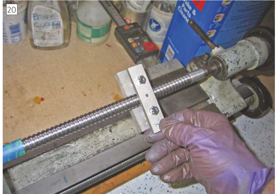
The rotary feed mechanism (as the ballscrew is being turned by hand not power the gloves pose no risk).
