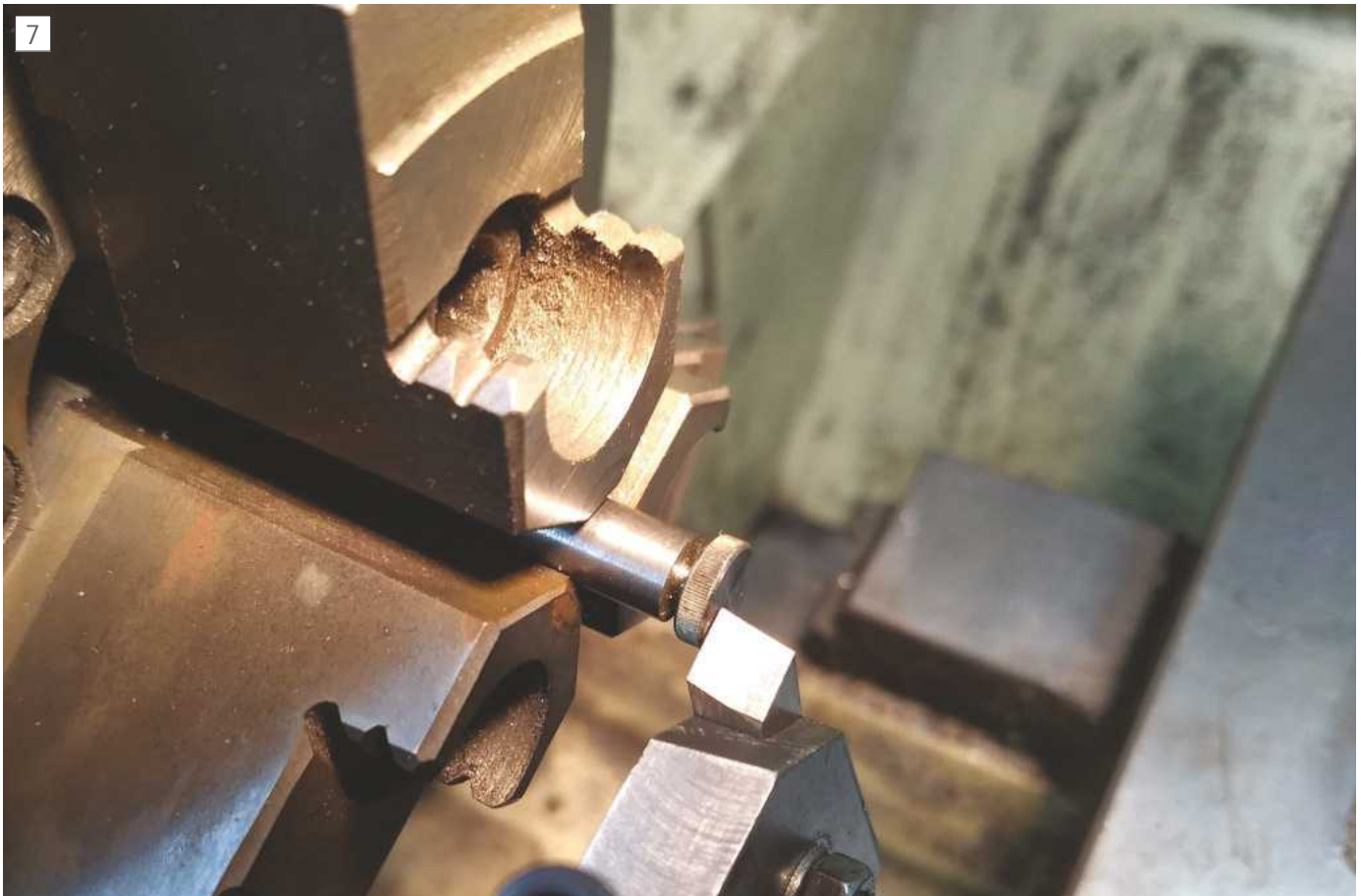
Finishing outer end.
