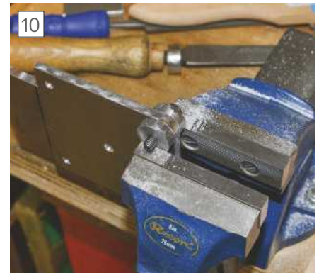
Filing a curve on the plates. No great precision was felt necessary and I used an old 6mm screw to align the filing buttons!
