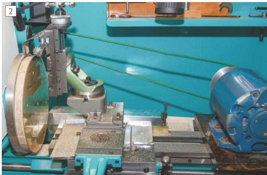
Cutting a 400 tooth clock wheel with the motor strapped to one end of the bed and the Light Milling Spindle mounted on a vertical slide with a raising block. Note the long drive belt, the brass block and clamp used as a stop on the lathe bed, and the card shielding to stop the chippings going everywhere!
