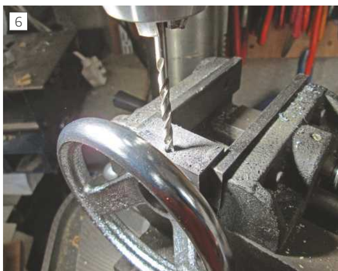
6 Drilling the collar ready for tapping to take grub screw
