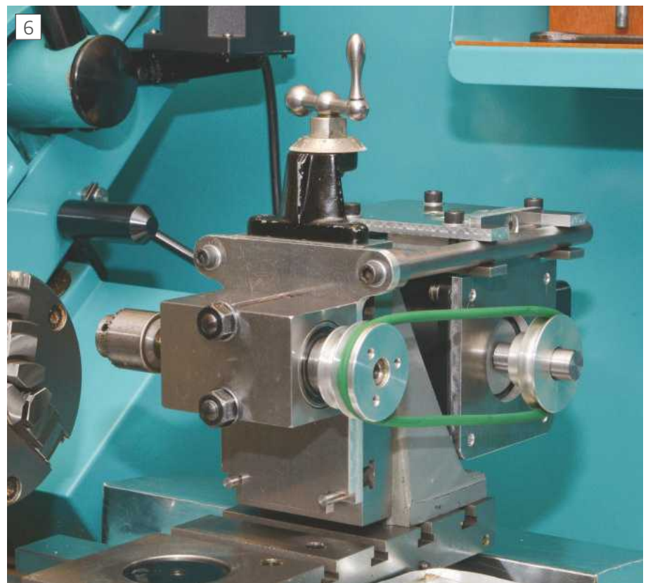
When the milling spindle is mounted in the upper T slots the spacer is positioned over the two registration pins to ensure alignment whilst tightening the clamping bolts.
