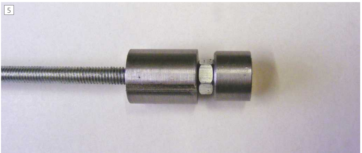
Showing the magnetic probe screwed into the stop.
