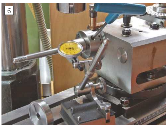
Setting Concentricity of Arbor, the GHT way.
