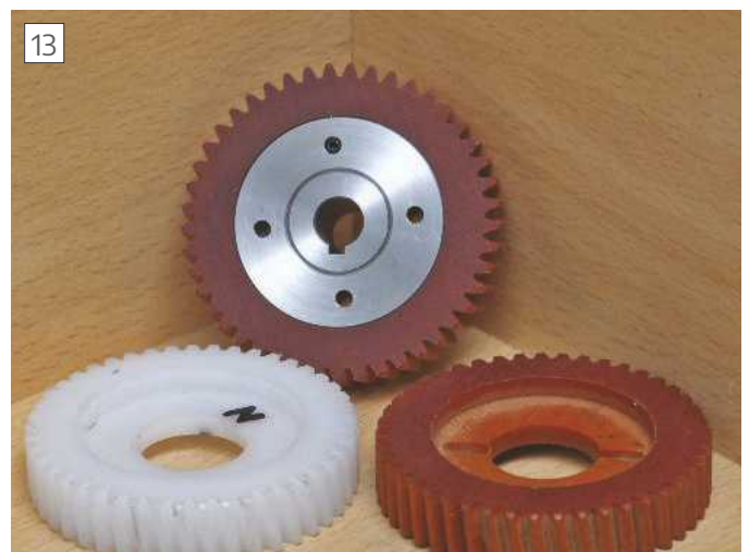
Finished Input Gear with spares, note M3 Grubscrew at 12 o'clock.
