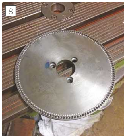
The completed 127 hole plate, also showing my error.
