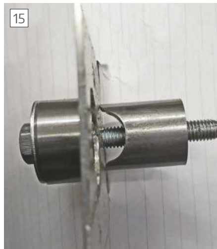
Punching 1.5mm aluminium.
