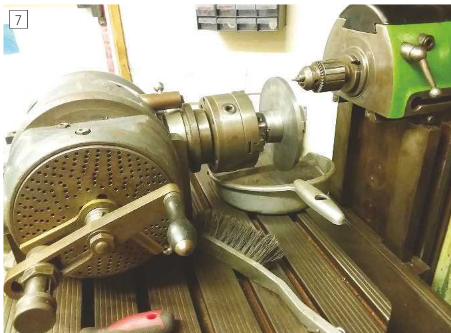
Centre drilling the dividing plate.
