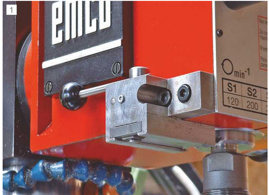
Position of ball handle when un-locked.
