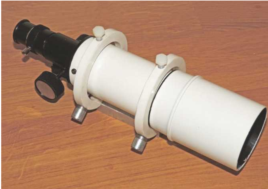
Telescope supporting rings machine from plastic sheet.
