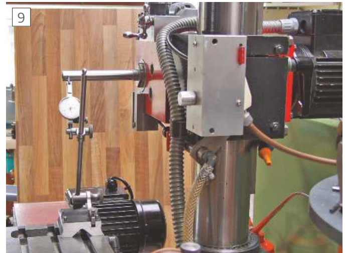
Clocking Test Mandrel Parallel with Cross-slide or Y-Axis.
