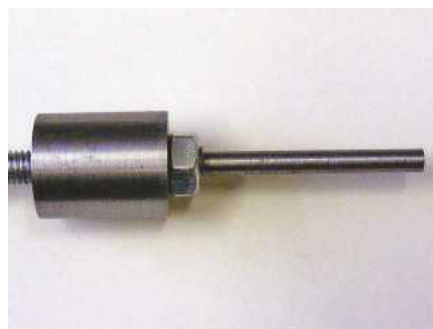
Mike Cox details a spindle back stop.
