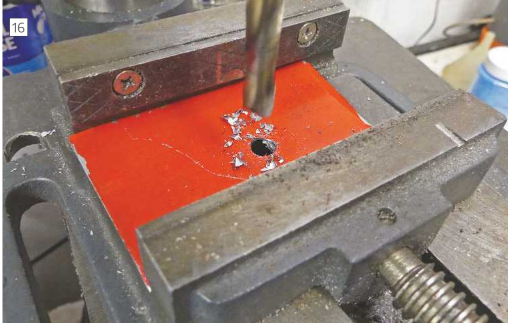
Pilot holes drilled with clamping.
