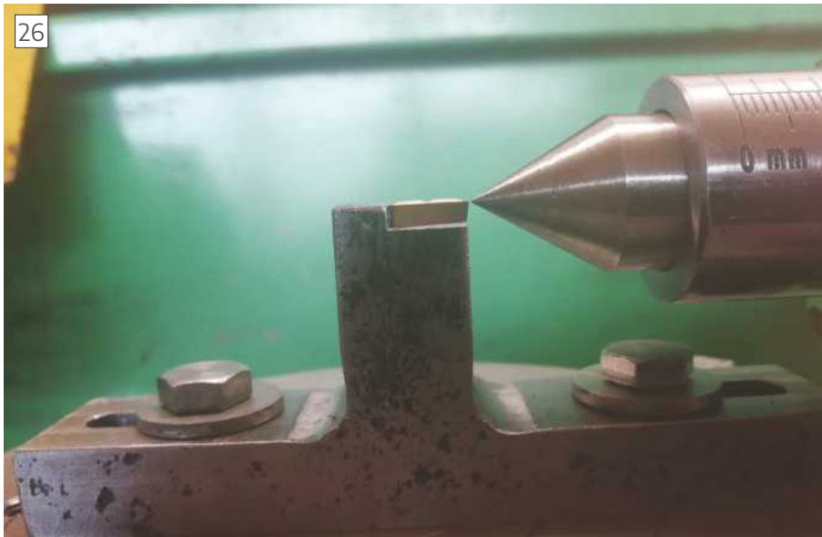
Radius tool check height
