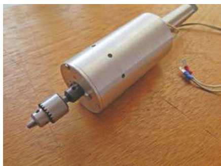
Stewart Hart presents a high speed drilling attachment.
