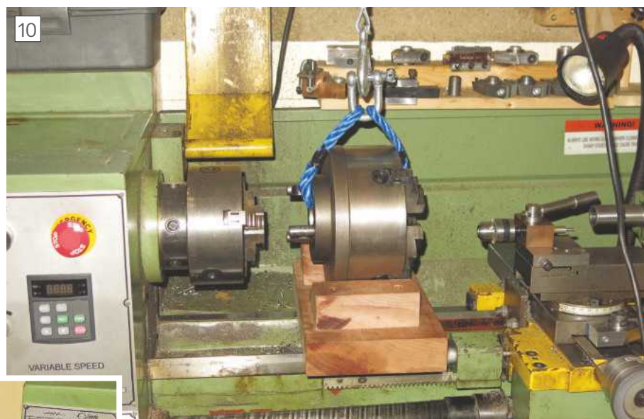
Four-jaw suspended above saddle.
