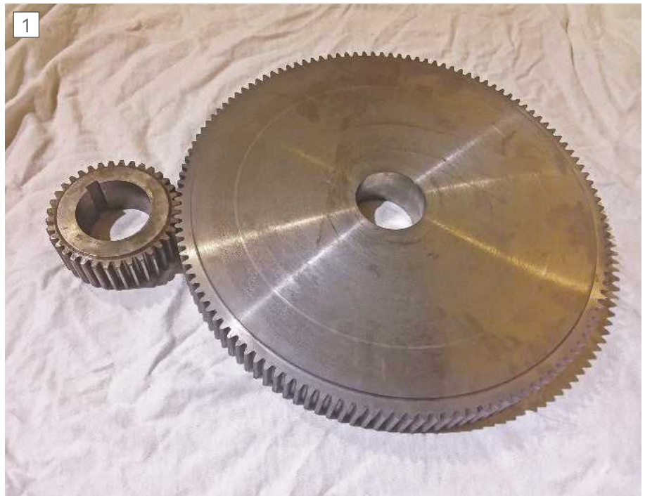
The near completed 127 gear mating with an original.
