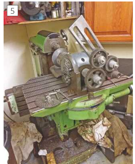
The differential indexing setup for drilling the 127 hole dividing plate.
