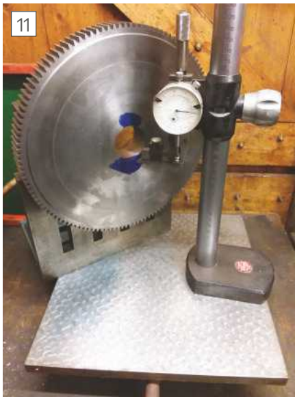
Accurately marking out the keyway.
