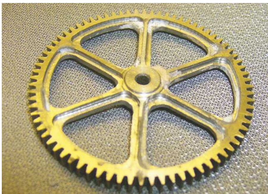
Surprisingly delicate shapes can be machined from meehanite
