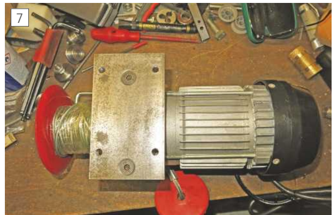
Mounting plate on winch.
