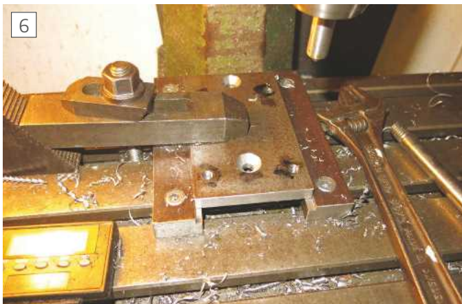
Drilling mounting plate.
