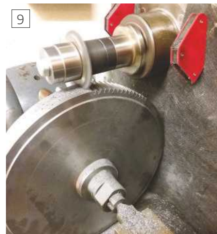
Finally cutting the 12 DP 127 gear.
