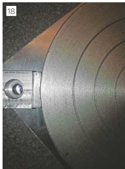
Filed radius on clamp
