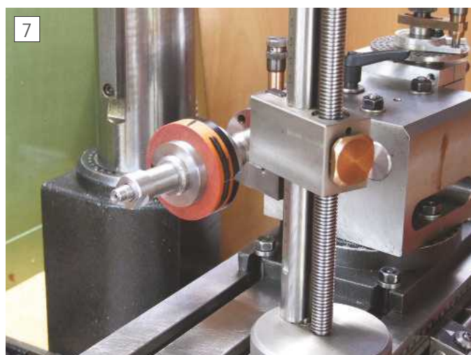
Scribing lines 0.4 mm above and below centreline.
