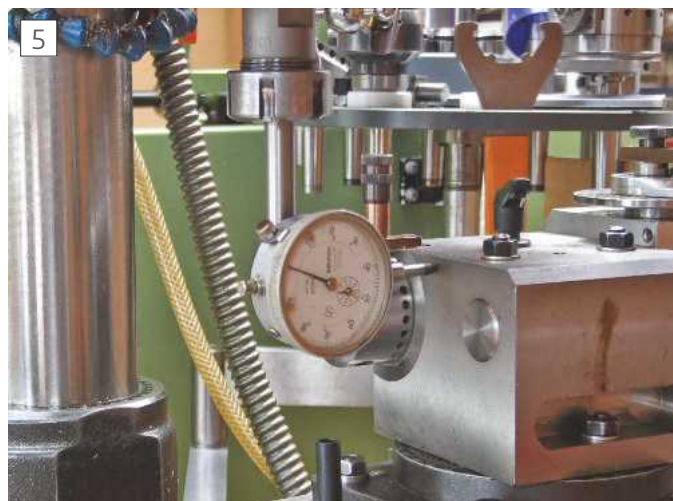
Checking the 8-degree angle setting over 30mm.
