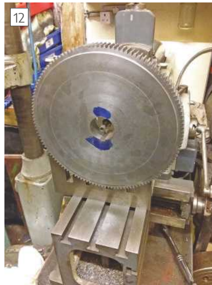
Shaping the keyway.
