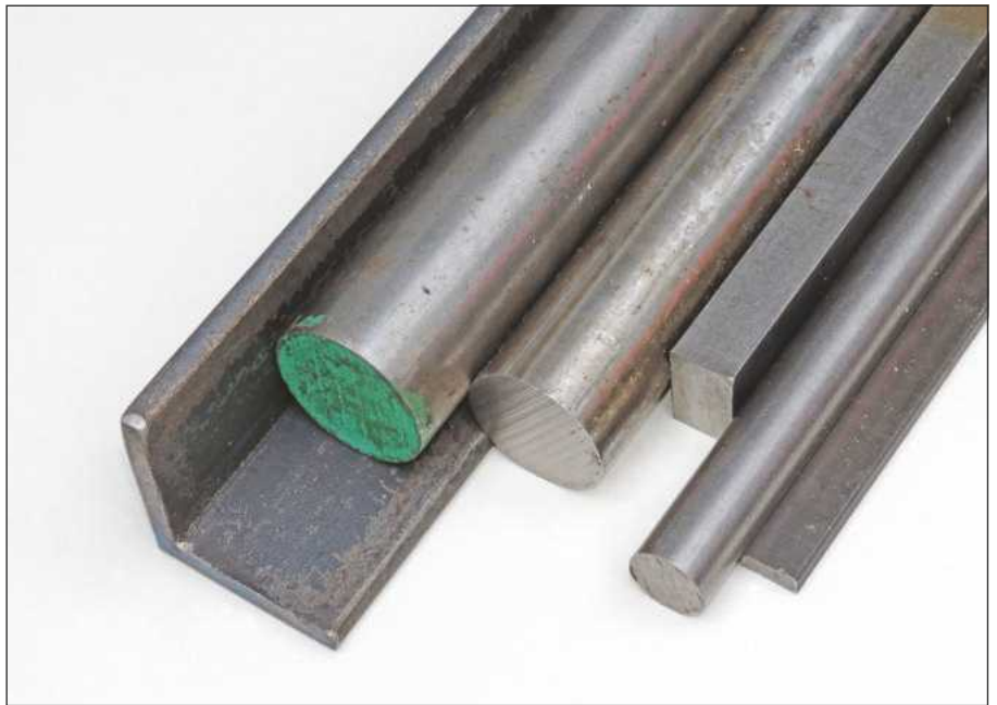
Various sections of mild and medium-carbon steels.
