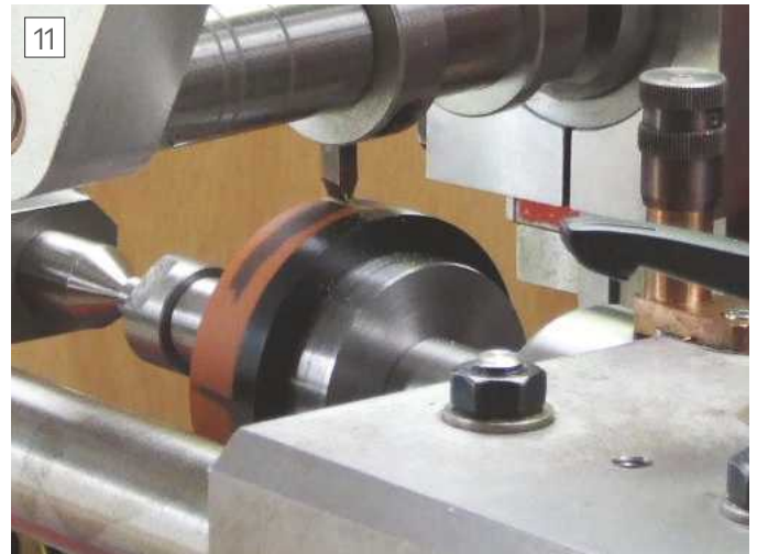
Close-up of Cutter setting.
