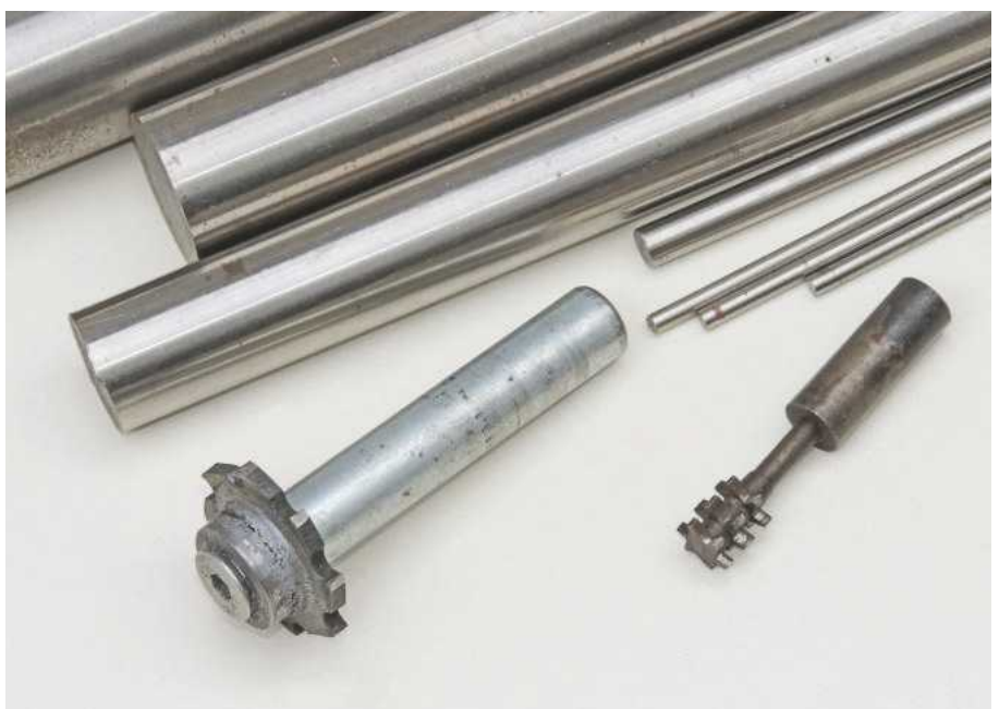
Bars of silver steel and some shop-made cutting tools made from silver steel.
