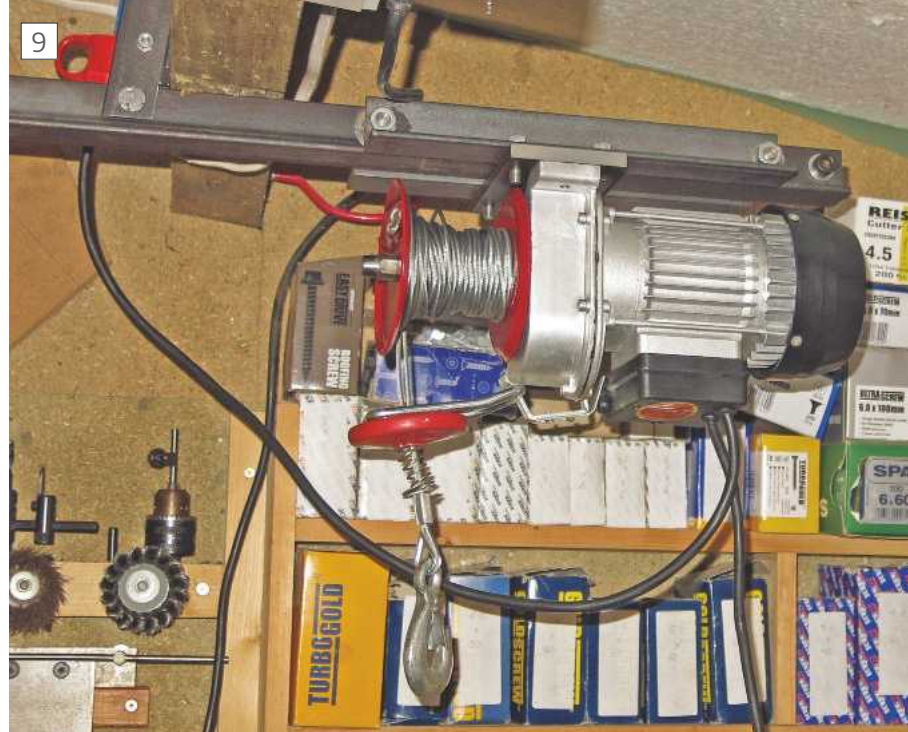
Winch on track.
