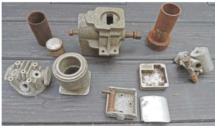
Aluminium alloy castings for an internal combustion engine.
