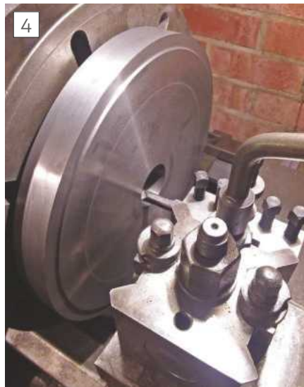
Finish turning the bore of the gear.
