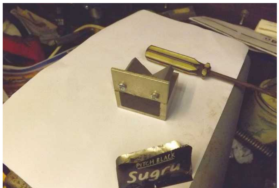
Moulding a lathe bed wiper using Sugru (John Stevenson).
