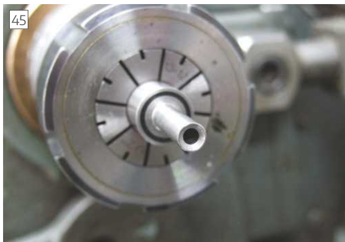
The ball seat has now been formed - note the 'land' rather than a sharp corner.
