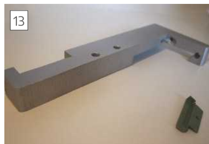
Back of the bracket. Drilled two more holes in it and tapped M8, can always come in handy to attach something to it.
