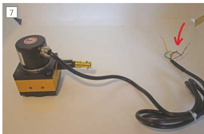
The wire encoder cable ends in colored wires, with a braided shielded.
