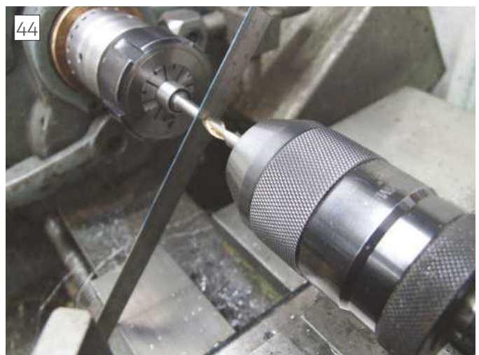
Machining the ball seat - using a feeler to help gauge depth of cut.
