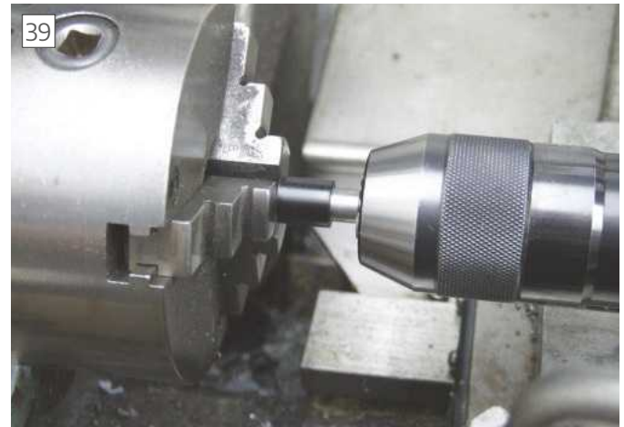
Fitting the probe blank to the insulating sleeve.
