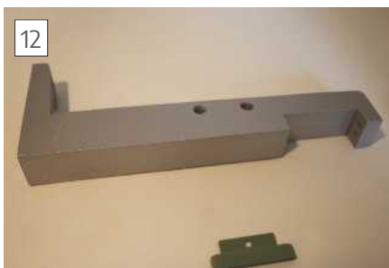
The bracket for the Y-axis. I sprayed the OBO wood with a paint can of silver.
