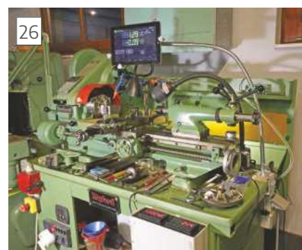
Project box closed, with digital readouts, and tablet on top of a gooseneck
