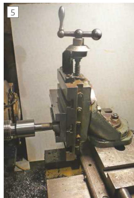
Milling lower dovetail
