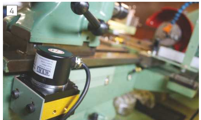
Angle bracket at the rear of the bed for X-axis setup. I also sprayed it with a spray can in machine green.
