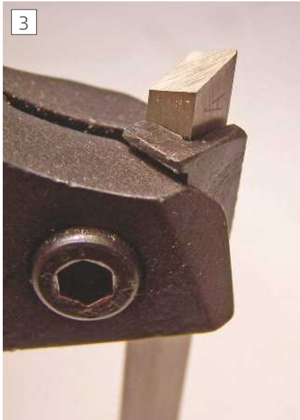
The \frac{3}{16} inch square toolbit with the packing piece
