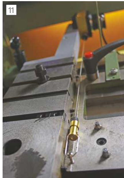
The Y-axis wire encoder with paper clip. The tool holder is removed for clarity.
