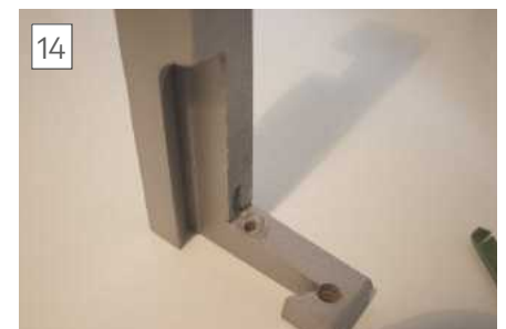
Bottom of the bracket. Mark the two holes to screw the bracket to the cross slide. Their position must be accurate. The trench is made on both sides with a dovetail cutter. ➤
