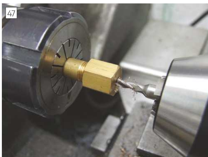
Spot facing the ball prior to producing the M2.5 threaded hole.
