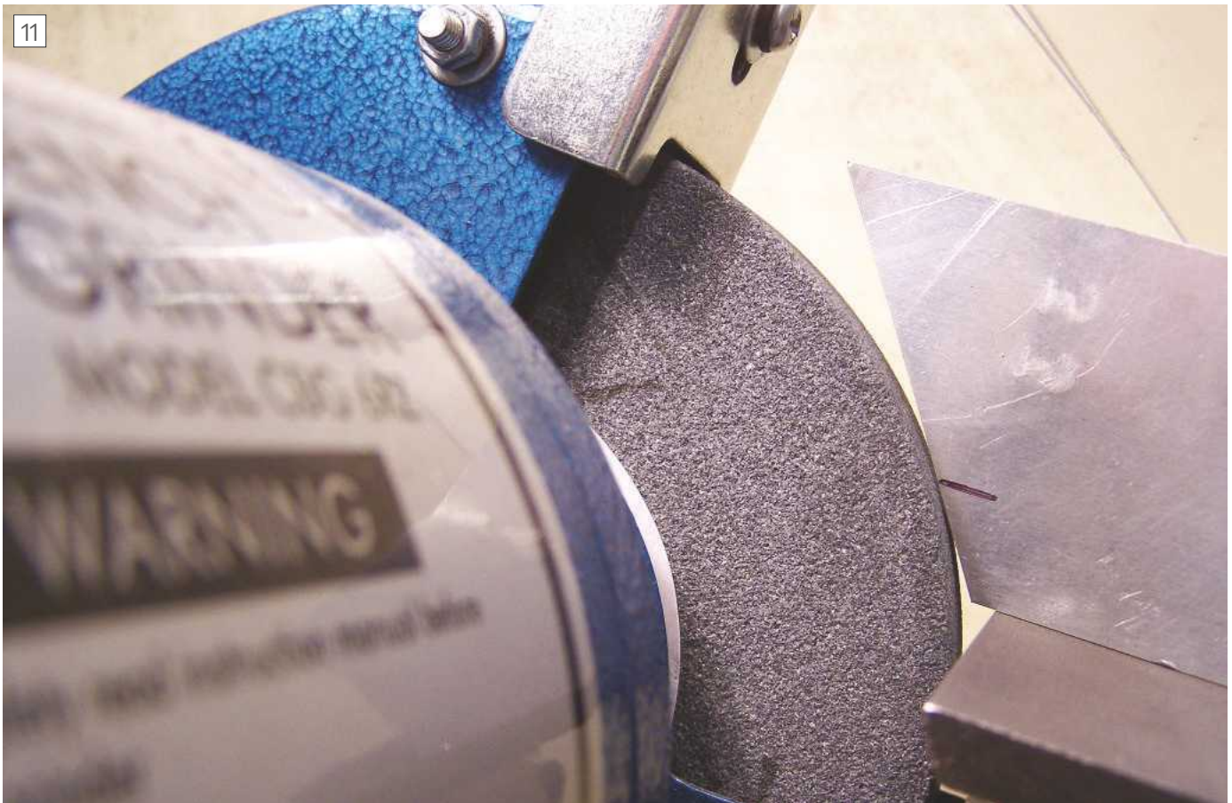
Setting the 33° angle as a tangent to the wheel
