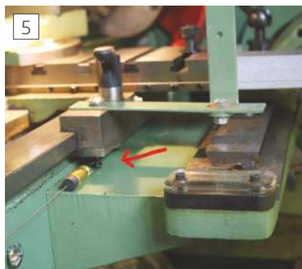
A screw hole is already provided on the underside of the cross table.
