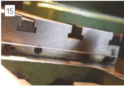
The wire will leave the T-slots open and the set screws accessible.
