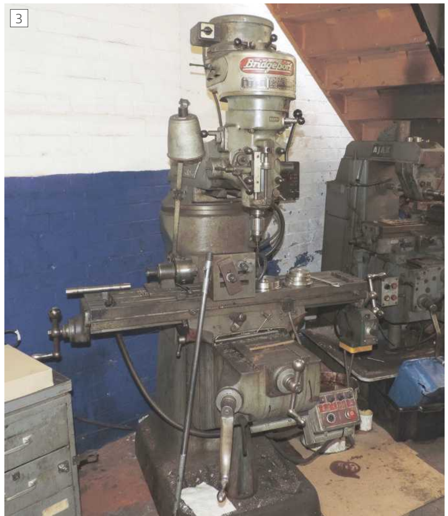
This Bridgeport Mill is typical of those found in commercial engineering workshops and much favoured by hobbyists fortunate enough to have the space for one.
