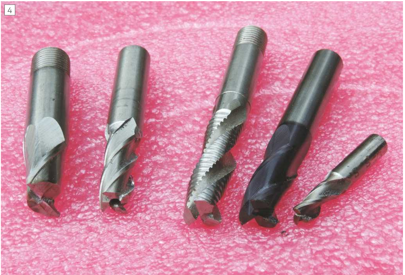
Left to right: Slot drill with threaded shank, four flute end-mill, 'rippa' cutter, three-flute carbide end mill, FC3 'throwaway' end mill.
