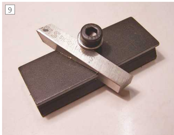
The grinding jig supplied with the tool-holder
