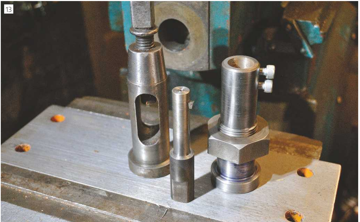
The original lantern post and the new adapter with the cutting tool in the centre.
