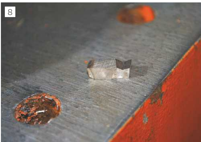
The first tool bit, shaped freehand on the bench grinder.
