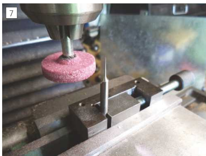
Sectioning D Bit with stone point held in the mill
