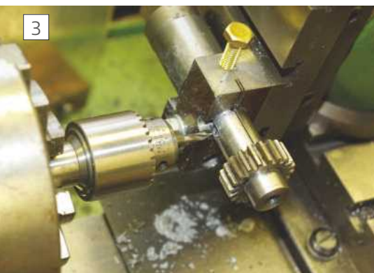
Drilling for the 8BA retaining screw. The same set up is used to mill the 4mm slot for the 8BA retaining screw.
