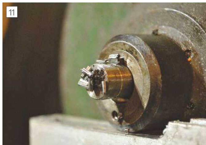
The second attempt with a new tool bit, cutting upwards, went as it should.
