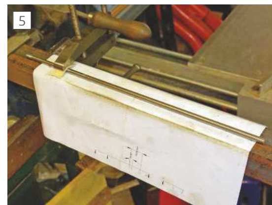
Filing the 0.5mm flat on the depthing rod. ➤
