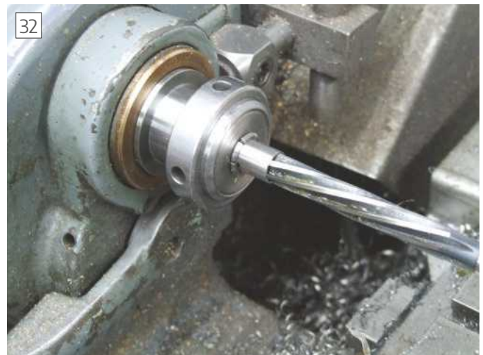
32 Reaming the 7/16" diameter bore with a machine reamer.
