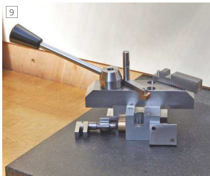
Clutch control lever and associated parts.
