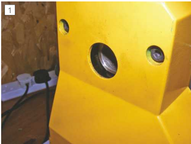
The gear cover on a minilathe. The end of the spindle is inside the cover.
