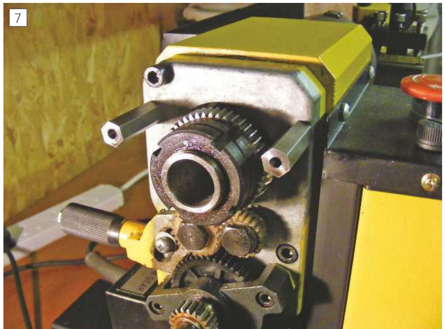
The threaded hex bars screwed to the headstock.
