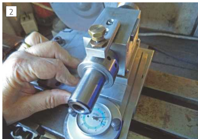
Setting the fixture to required angle
