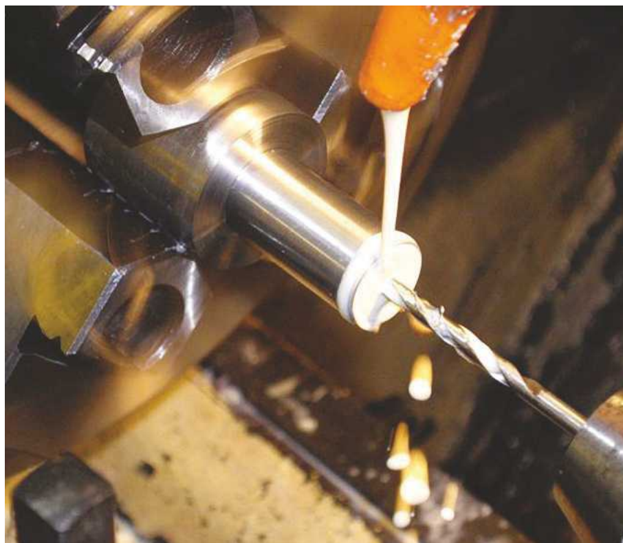
Even a relatively small drill can benefit from a constant flow of suds.
