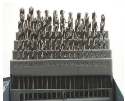
This set of number drills comes in a combined box and holder.
