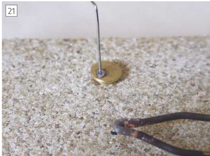
Pre-tinning the brass end cap.
