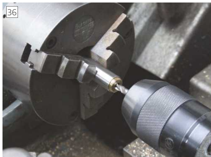
Forming the recess in the end cap, using the body as a holder.
