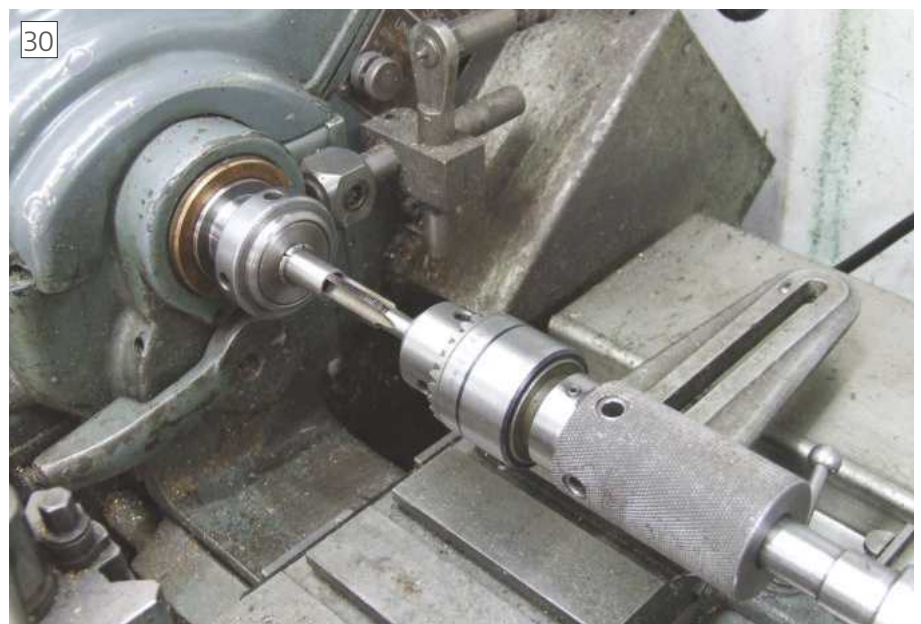
Using a plug tap to finish the 7/16" x 32 thread.
