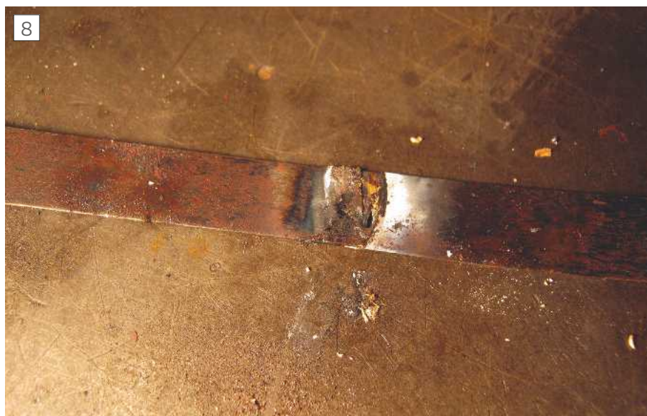
The silver soldered joint
