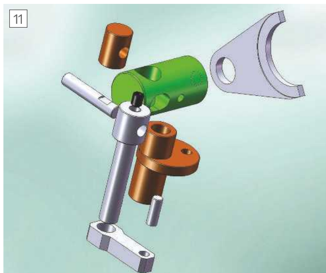
Clutch lever exploded view.
