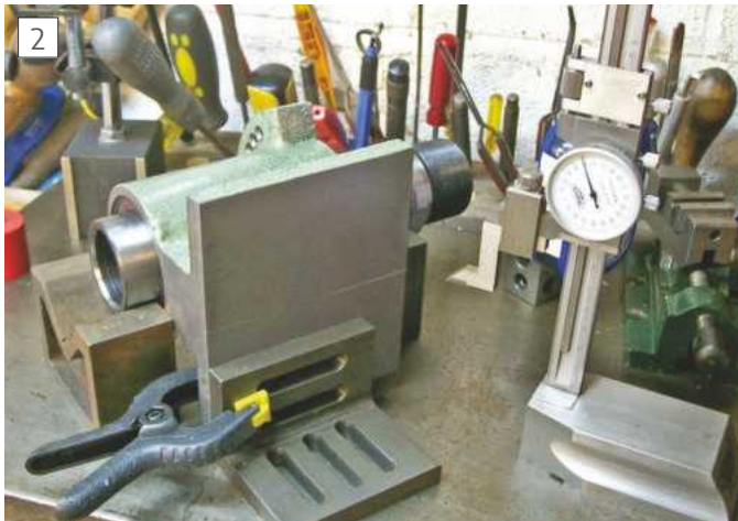
Indexer set up on a pair of matching V blocks for marking centre line
