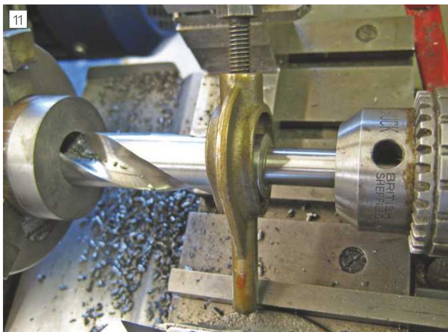
Preventing damage to tailstock Morse taper
