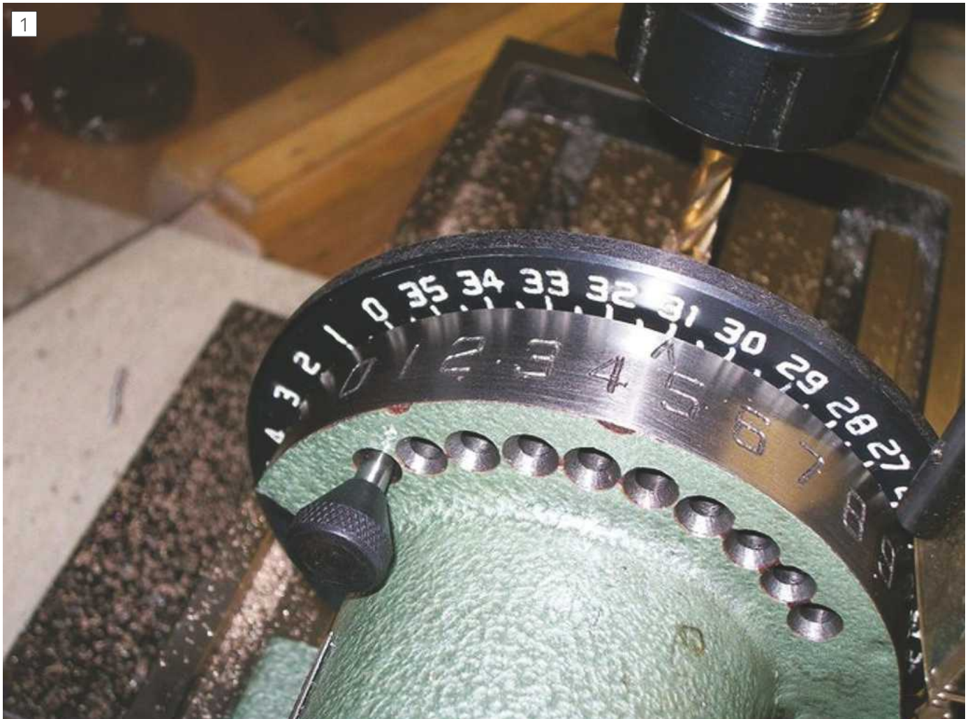
Vernier Scale to give 360 indexing steps 1° per step
