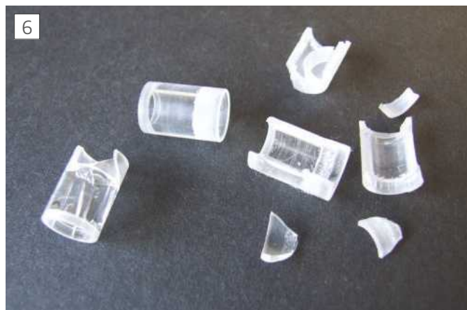
6 Broken acrylic tubes, believed to be caused by machining stresses.
