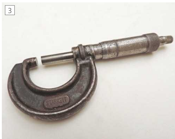
This older micrometer has only a vernier scale.
