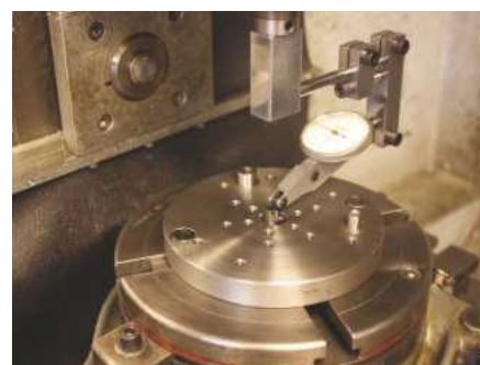
Concentrica – Pete Worden's aid to setting up a rotary table.
