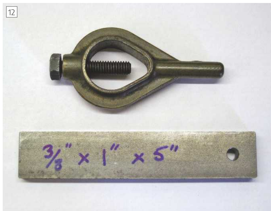
Lathe dog and steel bar to prevent rotation
