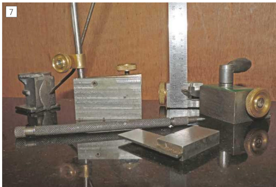
A piece of composite granite worktop used as a surface plate and a variety of marking out tools.
