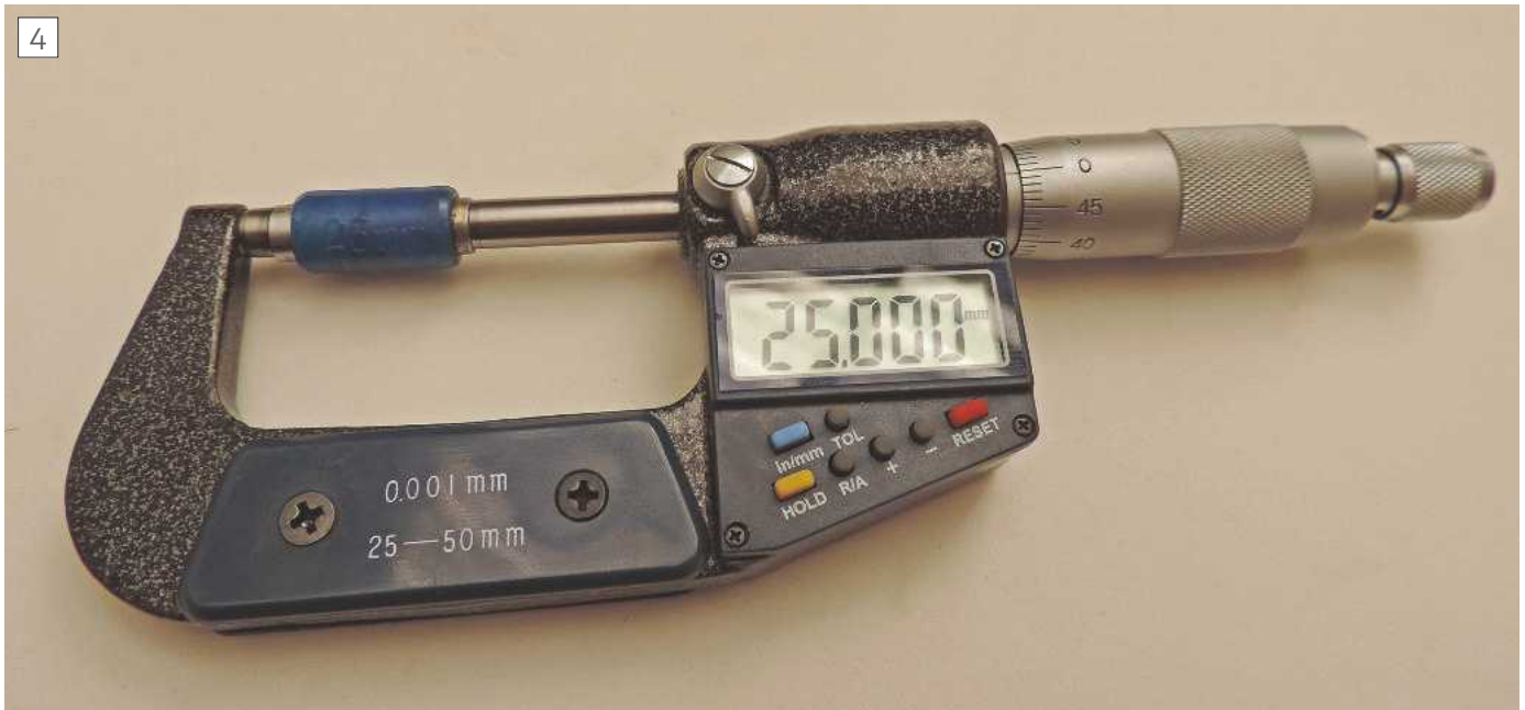
This digital micrometer has a vernier scale as well as its readout.
