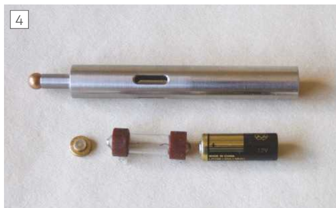
The first attempt - the festoon bulb and 12 volt battery shown here complete with insulating sleeves, contact plate and main body.
