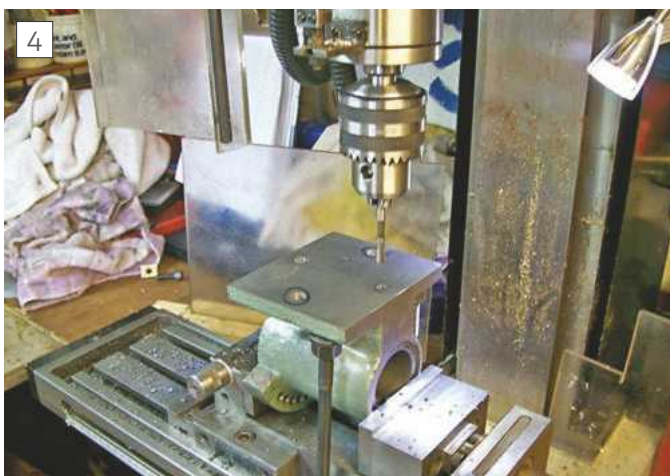
Drilling clamping holes indexer base:- note use of levelling jacks
