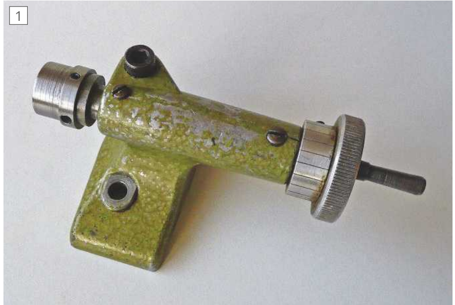
Tailstock, note threaded adaptor on nose.
