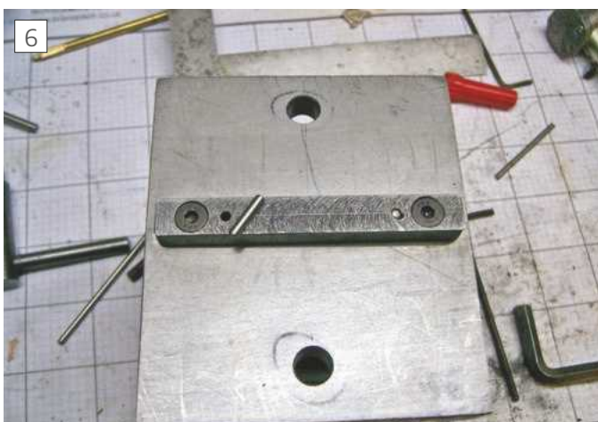
Setting bar doveled to base
