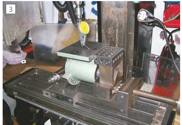
Clocking Indexer Square for drilling
