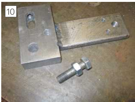
The jacking screw and threaded hole
