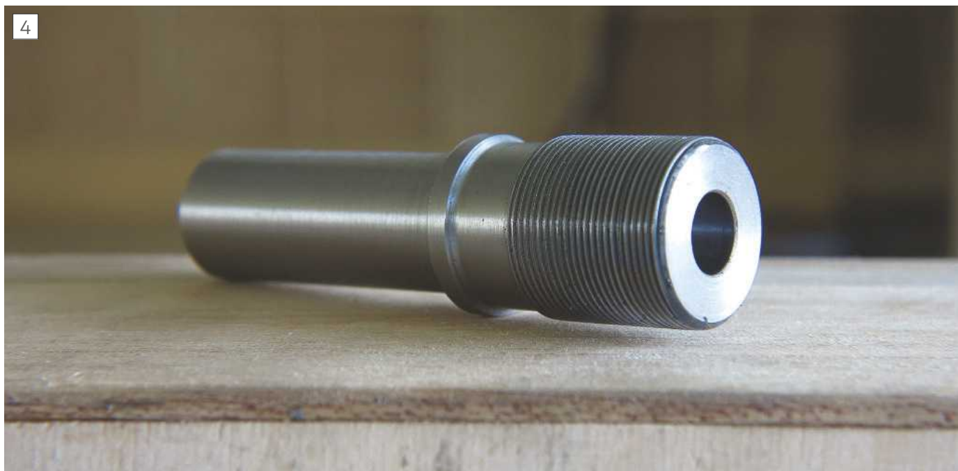
The shank's end hole takes the backstops.
