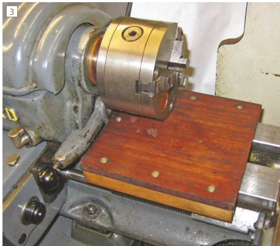
Chuck board in position
