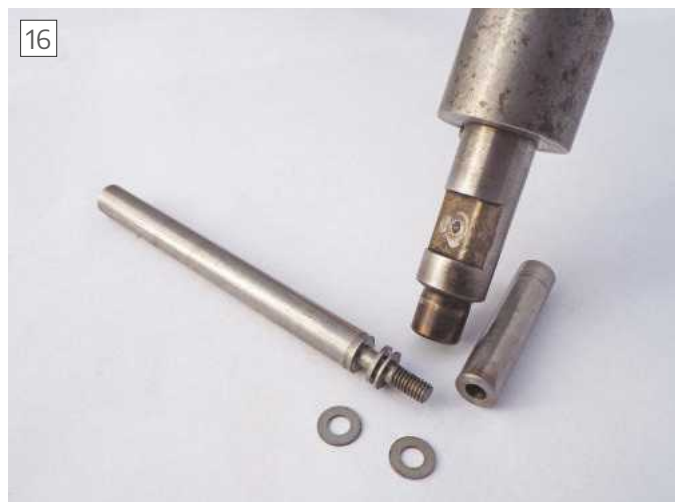
Cam and pushrod assembly
