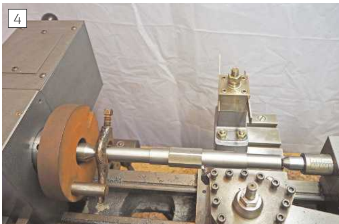
Finish turning Shaft
