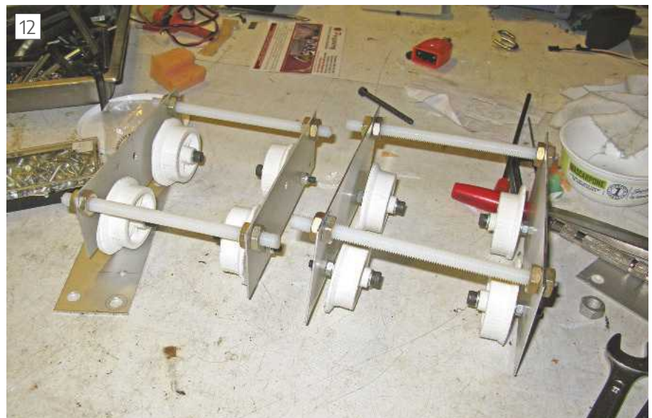
3D printed wheels and arrangement for cable trolley
