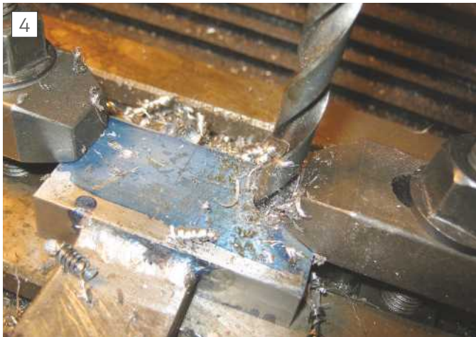
Drilling 10mm hole
