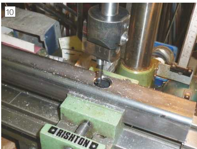
Enlarging hole to 35mm in box section
