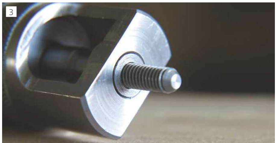
An accurately sized adaptor ensures concentricity.
