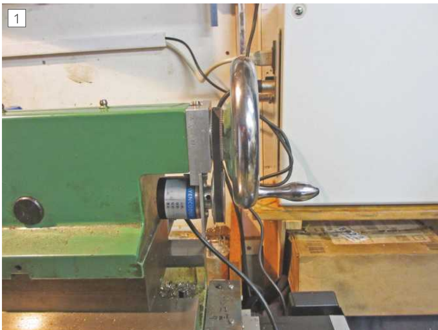
Hardware fitted to the tailstock.
