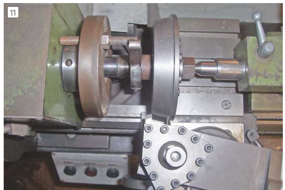
Clutch plate attached to drive plate for final finishing
