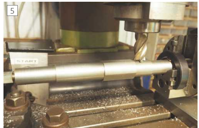
Milling hex on clutch shaft
