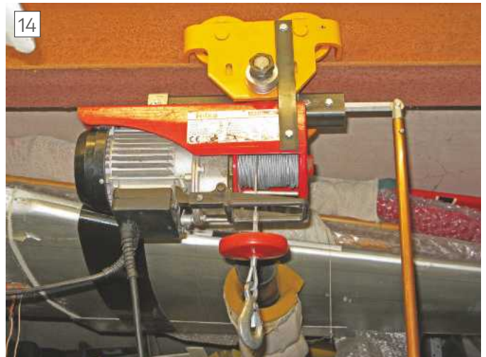
Revised bracket position after changing C of G
