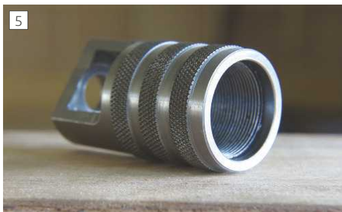
The chuck body needs to be accurately screwcut to fit the shank.
