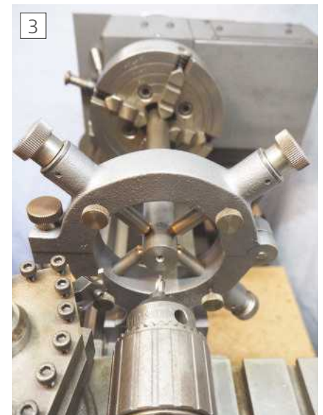
Centre drilling shaft
