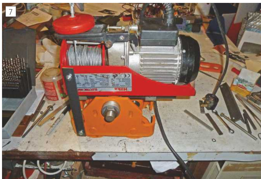
Trolley and hoist mated together (Upside down)
