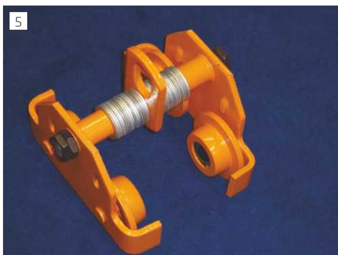
Trolley bought for fixing to the RSJ
