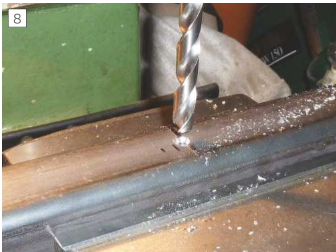
Drilling hole in box section
