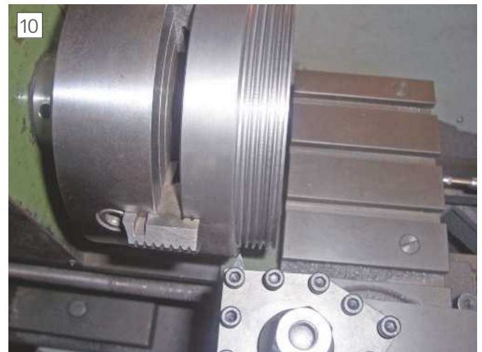
Cutting pulley grooves on main body
