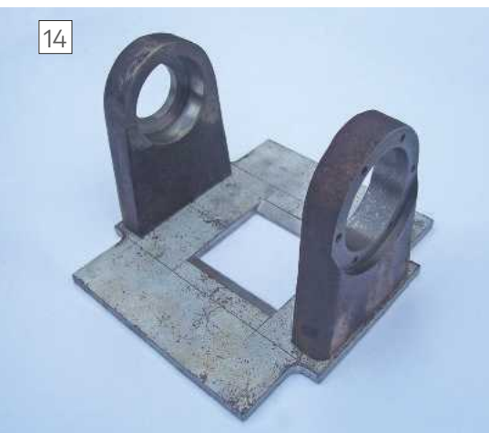
Completed base and bearing pedestals
