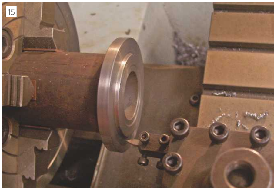
Scribing end housing for mounting screws
