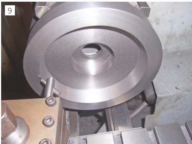
Machining clutch plate
