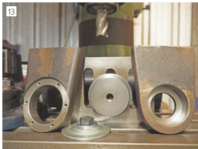
Set up to mill bearing pedestals to equal height
