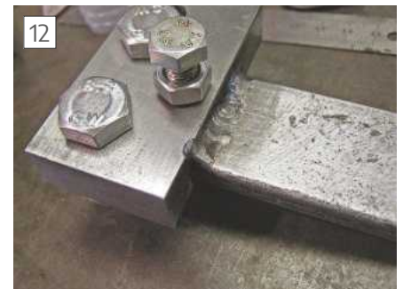
Top side of jacking screw
