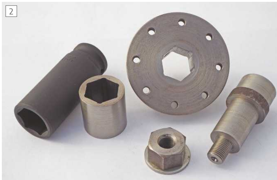
Drive plate, deep socket, machined socket and arbor
