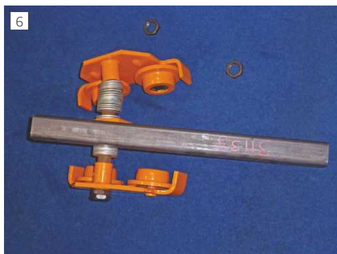
Trolley with box section on to dowel
