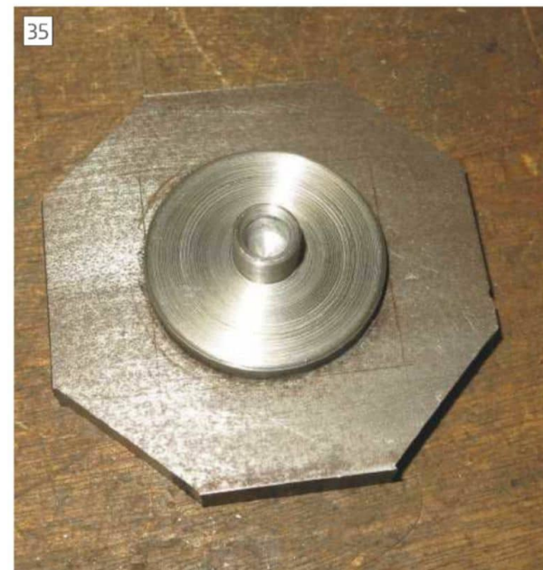
Blank with corners cut and superglued on pivot.
