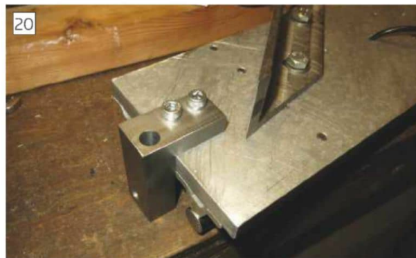
Stop body screwed to saw attachment.
