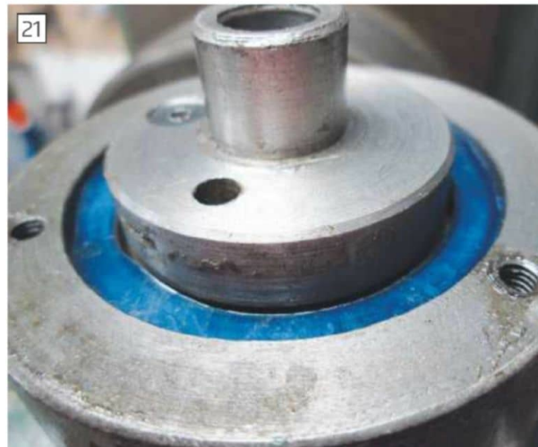
Shim in Place on Race Outer.
