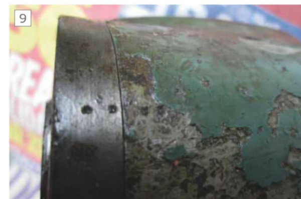
Marking the Cover to Ensure Correct Re-assembly.
