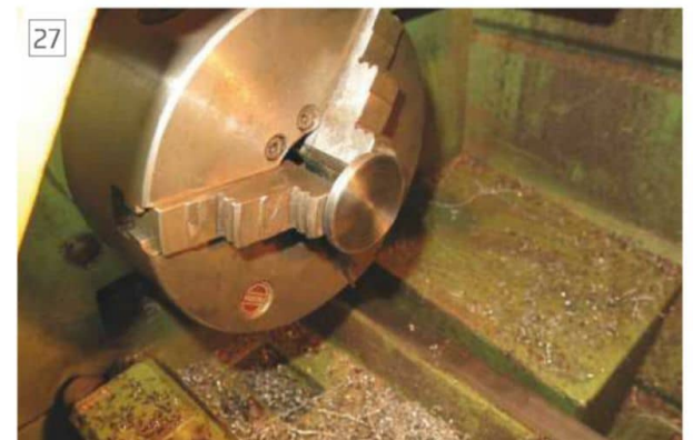
Facing and thickening the no hole pivot.
