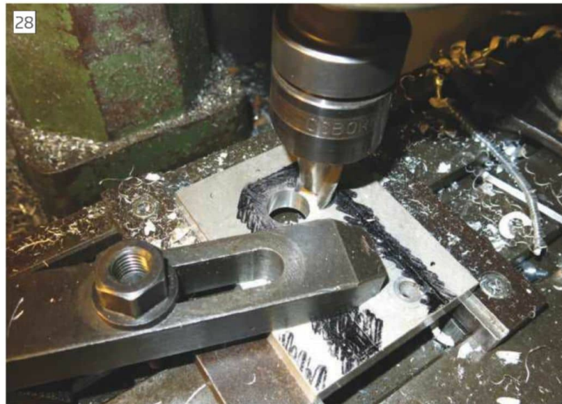
Milling the end slot in the G-clamp.
