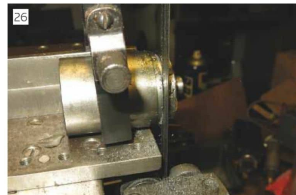
Sawing the no hole pivot off.
