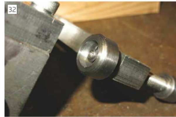
Clamp screw and pad fitted.
