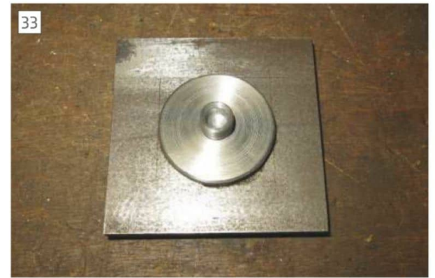
No hole pivot superglued to blank.
