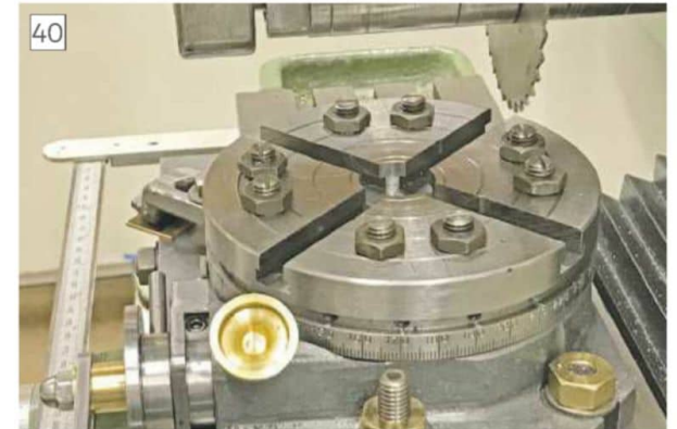
Slotting the grub screw heads.
