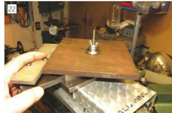
Setting for a 45 degree corner cut.
