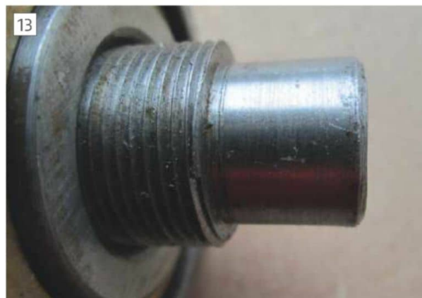
Damage to Shaft Thread.
