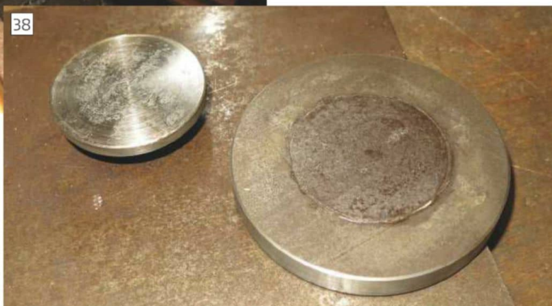
After separating with blow torch.
