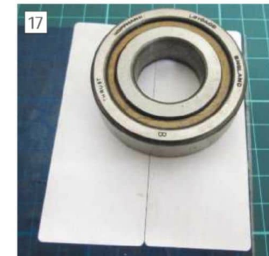
Self Adhesive Labels Stuck to Shim Material.
