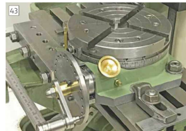
Completed, painted, notice the oiler nipple for the eccentric quill.
