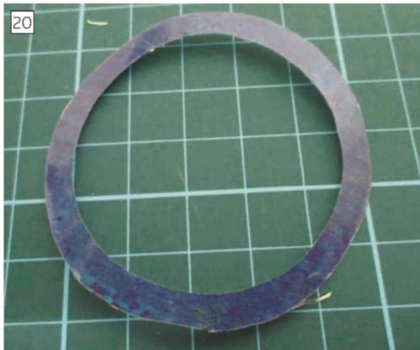
Shim with Label removed ready for fitting.
