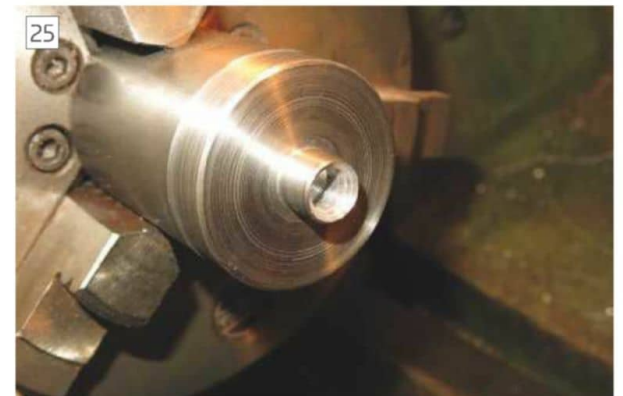
Turning the no hole pivot.
