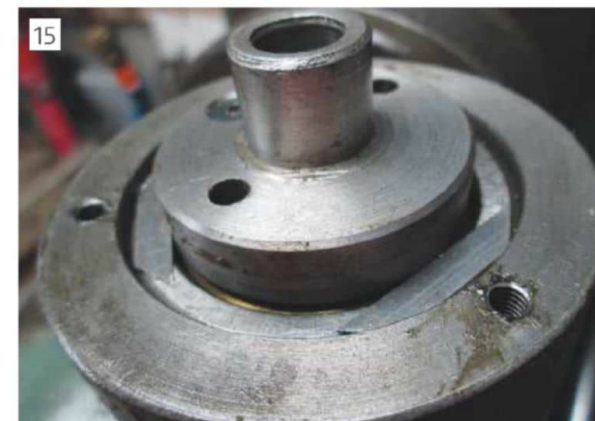
'Calibration' shim material in place.
