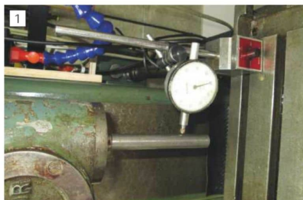
Checking that the Head has been Set Vertical.
