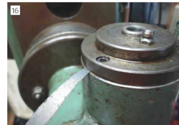
Checking the Gap between the Cover and the Casting at One of Three Points.
