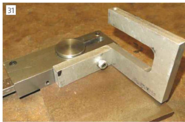
Pivot and G-clamp attached to the main body.
