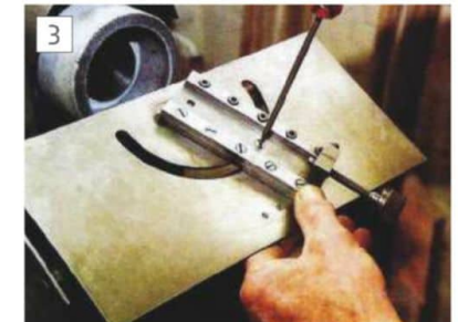
The angle of the slide creates the clearance.
