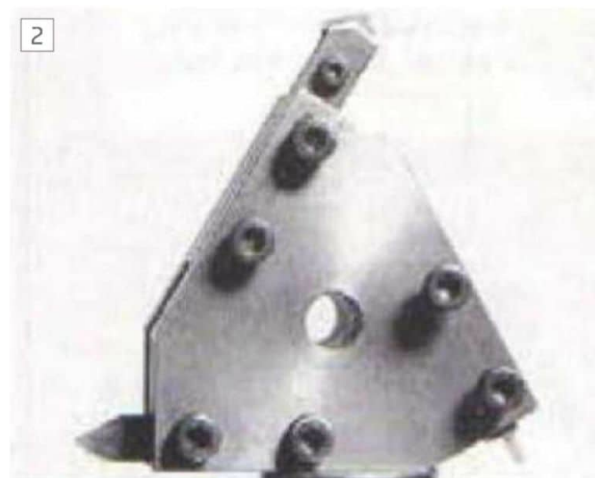
Another similar toolpost loaded with zero-rake tools for cast iron and brass. Note one holder is loaded for carrying triangular tungsten carbide tips.
