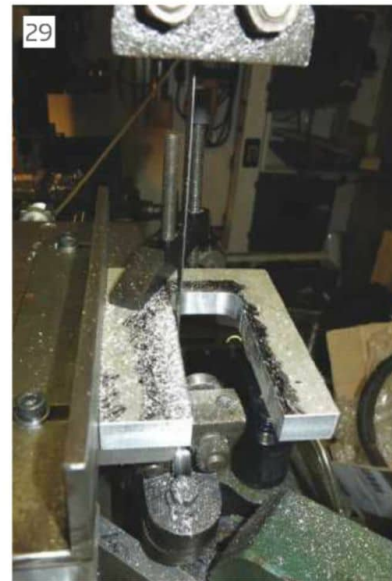
Sawing out close to size.
