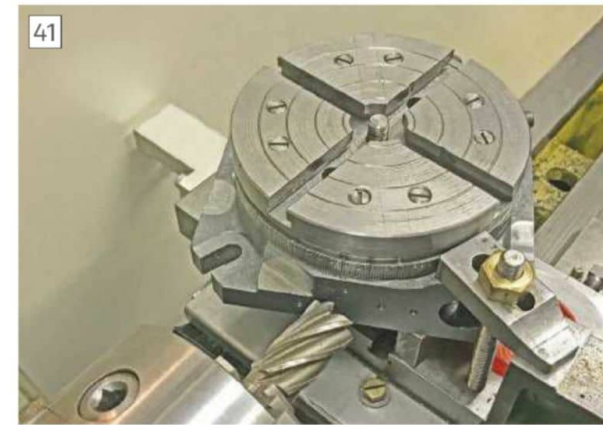
Milling the flat for the 'U' shaped brass stop.
