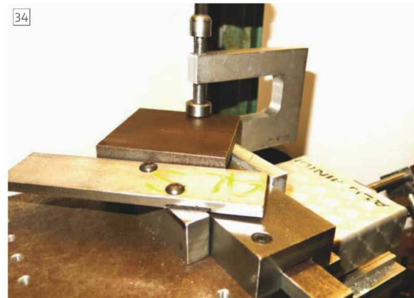
Setting the first corner and clamping.
