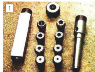
ER20 spring collets, normally used in the Morse taper chuck (right) can be fitted to the square holder (left) and used to hold a wide range of drill diameters.
