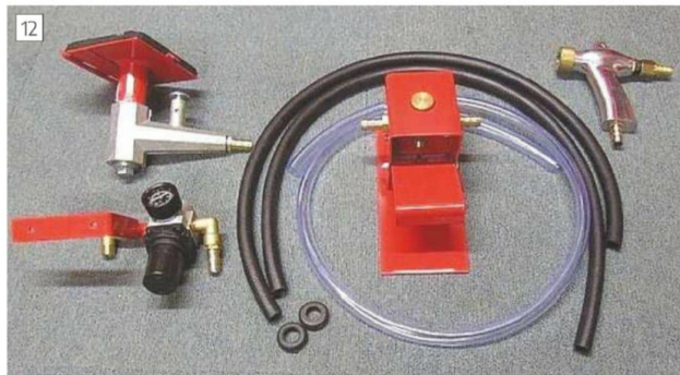
A typical foot pedal conversion kit for grit blasting cabinets
