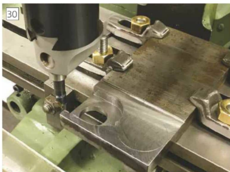
Part 15, retainer for the eccentric quill being milled out.
