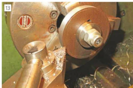
Turning round on a stub.
