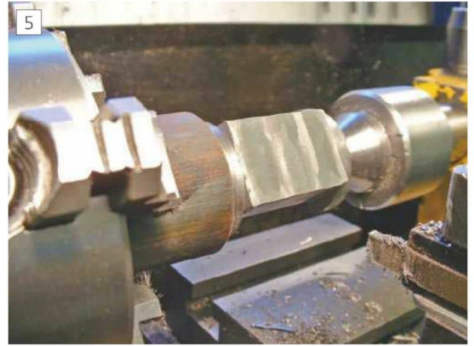
Turning cylinder flanges.
