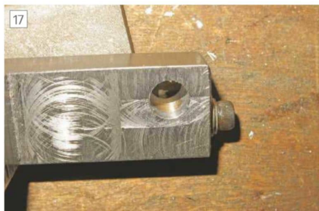
Cross drilled for stop rod.
