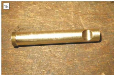
Brass ready for sawing across dimple.
