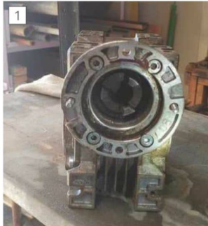
The coupling recessed inside the gearbox.
