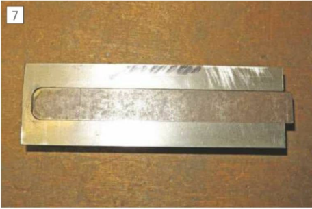
Slide end filed to fit the body.
