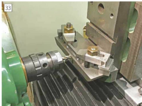
Milling the slot in the plunger arm.
