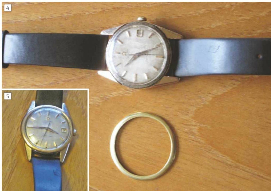
Restored watch after plating of the bezel.
