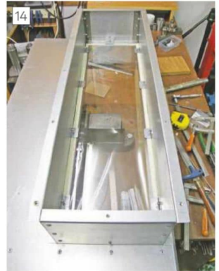
The light box i built on the top of the cabinet with film protected glazing
