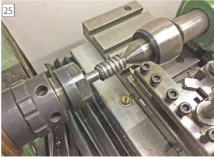
Indexing worm being cut, Part 7.
