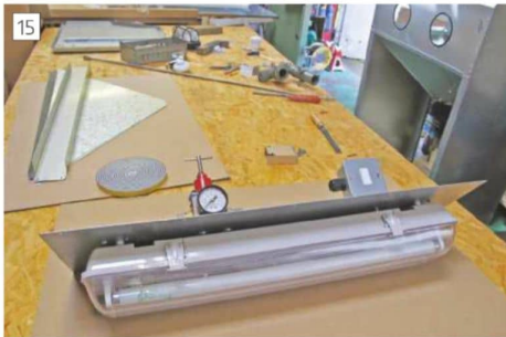
Light box top cover complete with strip light and inlet pressure gauge
