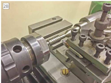
Forming the adjustment/clamping worm.
