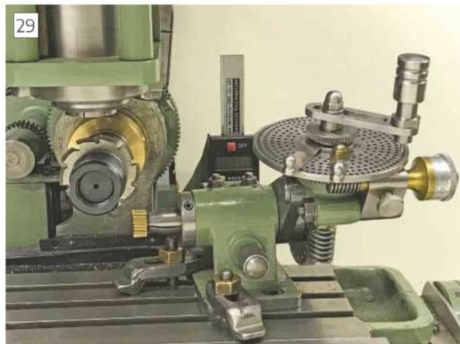
Milling the worm wheel, at helix angle 7.243°
