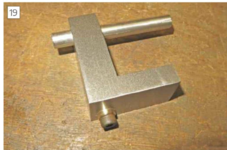
Locking trial with temporary caphead.
