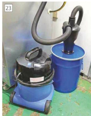
Cyclone dust extractor powered by vacuum cleaner.
