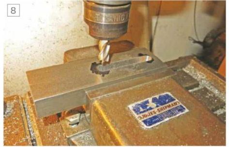
Milling the slot for the pivot.
