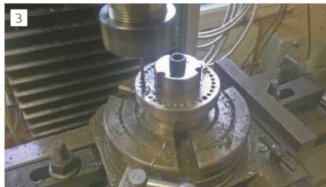
Drilling index holes.
