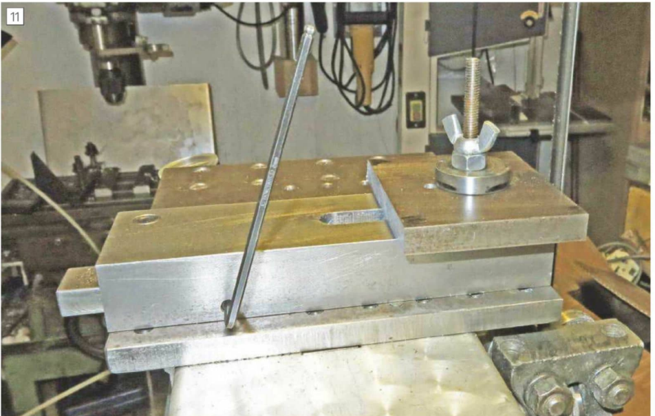
Adjusting the slide to lineup work edge with blade.
