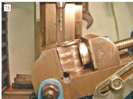
Drilling steam passage.
