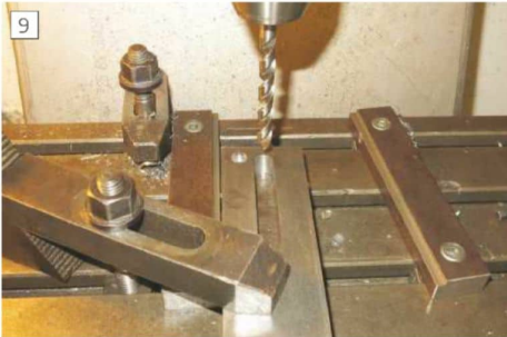
Drilling the slide through the body.
