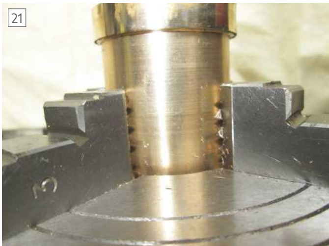
Result of slippage when being too confident trying the knee nut
