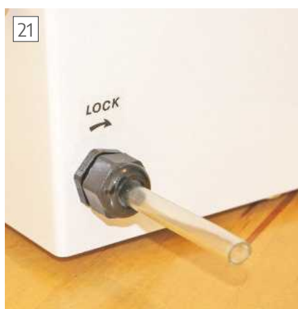
Right hand side of the box with the cable gland that acts as an in-out lock for the Tube Retract Guidance System.
