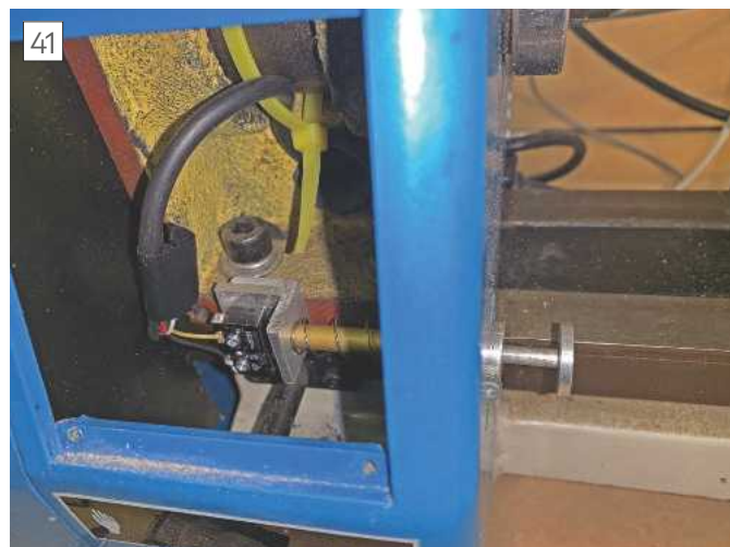
Autofeed limit switch.
