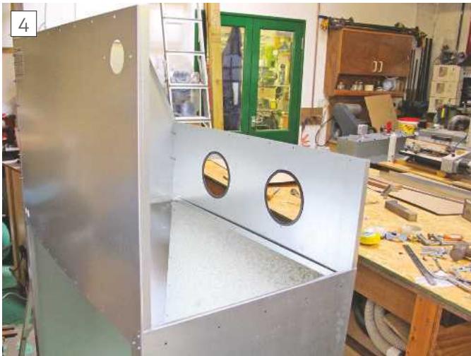
The author's cabinet with loosely fitted hopper - found to be 5mm too short and needing a make-up strip to achieve a good seal
