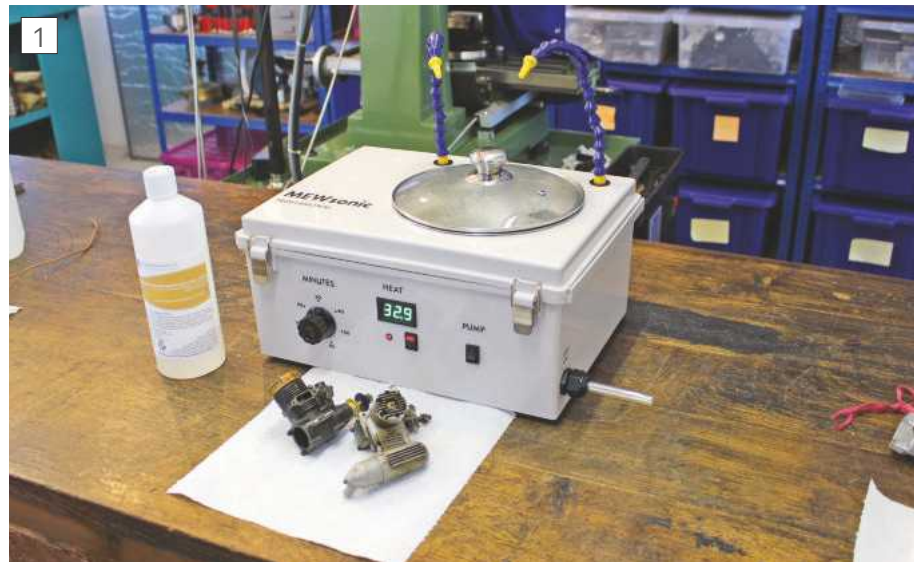
The completed MEWsonic Professional. The blue flexi-tube on the right is for sucking cleaning fluid from the tank, while the one on the left is used to suspend parts for cleaning.
