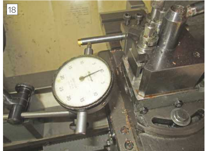
Aligning the ACME threading tool with clock gauge
