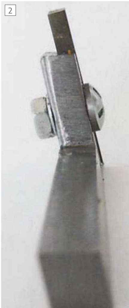
Note the parallelogram shaped shank
