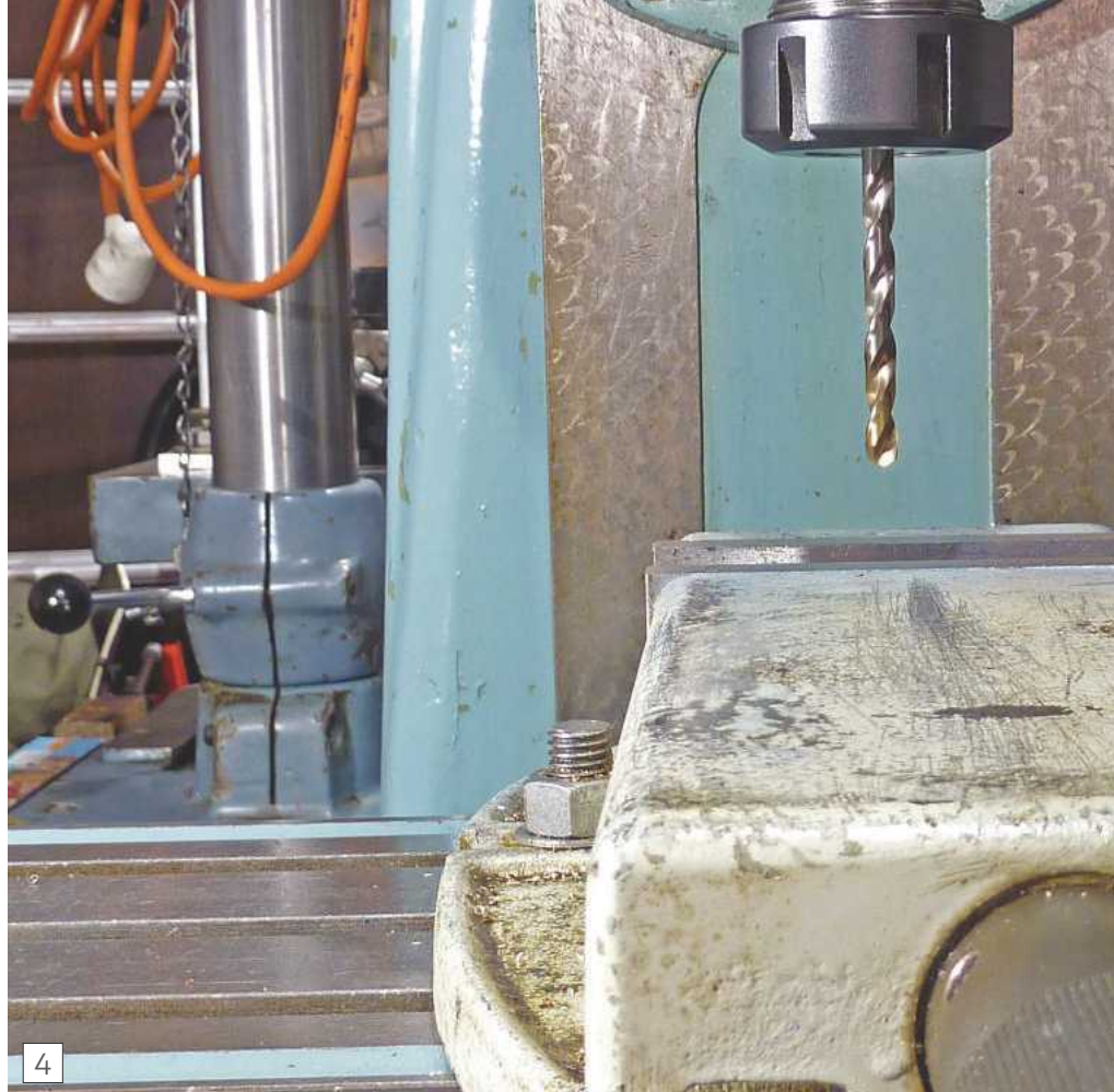
Poor working distance on Haighton mill using ER32 collets
