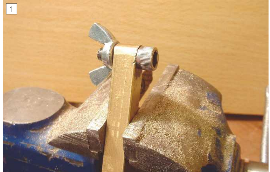
Using a bolt as a filing button
