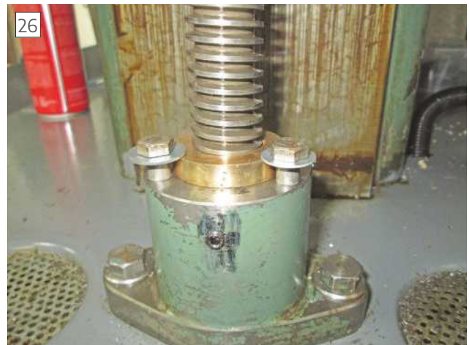
Temporary knee nut retainer
