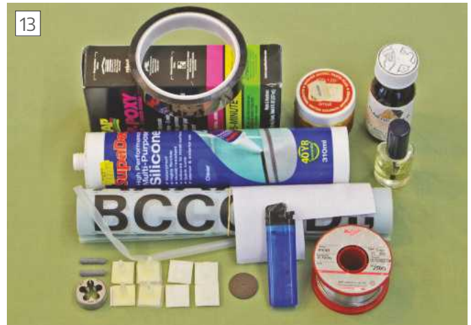
Various adhesives etc needed to assemble the cleaner, plus a pocket lighter for flame polishing acrylic.
