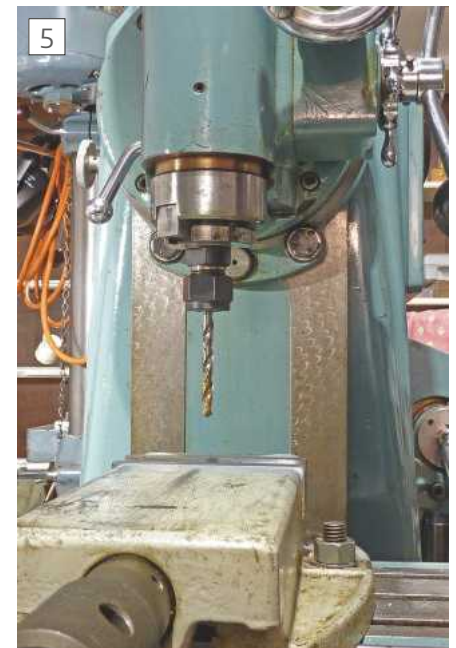
Slight improvement using DA200 collets
