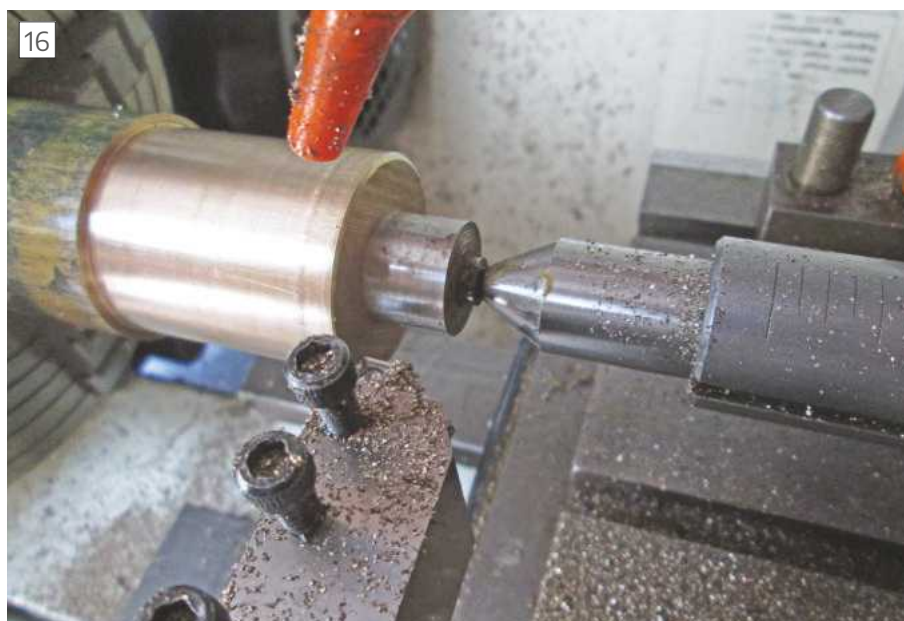
Turning the outside diameter of the knee nut showing the temporary plug for the centre
