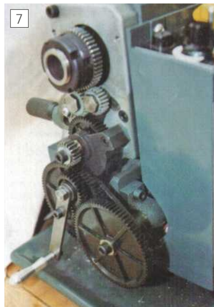
The swing arm arrangement to disengage the leadscrew.
