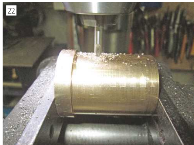
Using a centre drill to make the locating dimple in the knee nut
