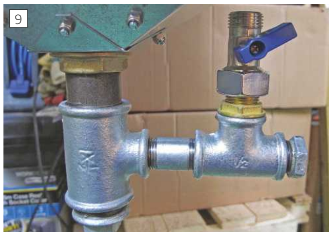
Collector head with bottom drain plug and tap adjustable air mixing valve.
