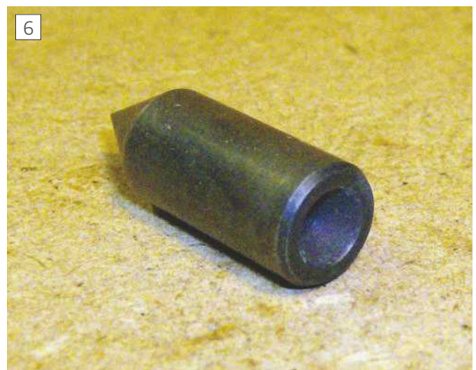
The centre is centre-drilled at the other end
