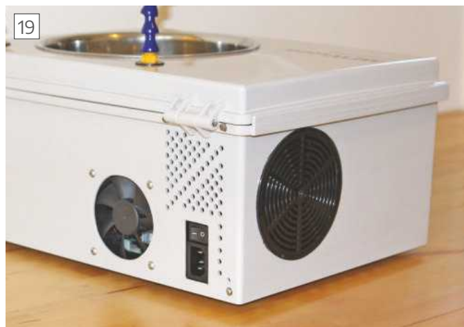
Rear of the ultrasonic cleaner with mains connection and vents for fans cooling the ATX power supply and ultrasonic driver board.
