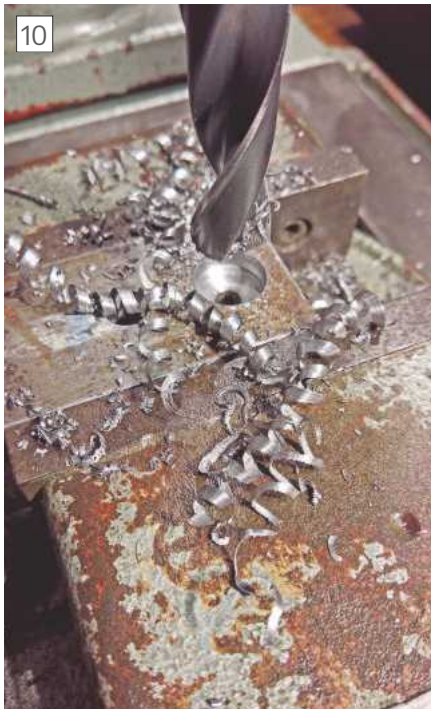
Good curls of steel swarf using large drill
