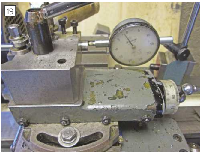
Clock set up on the end of the threading tool to monitor increase in cut
