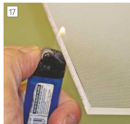
Flame polishing the sawn edge of acrylic that forms the tube guide.
