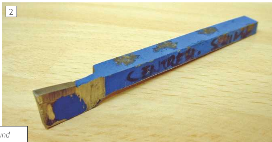
A carbide parting tool, the front face has been ground for clearance.
