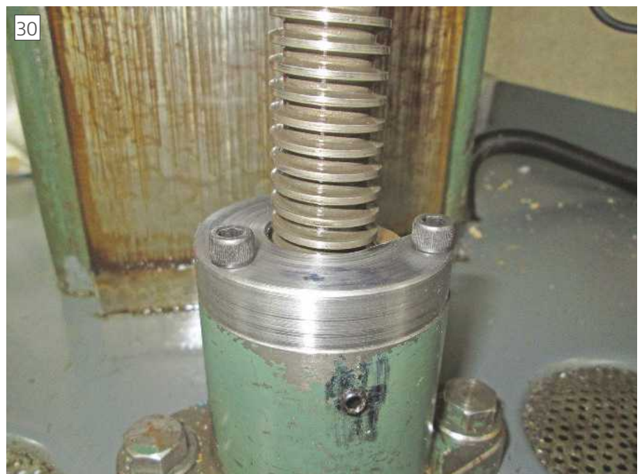
Completed collar Installed
