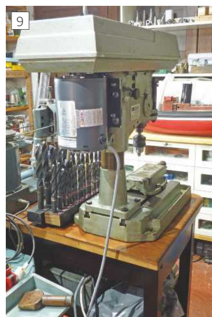
Three phase motor fitted to drill
