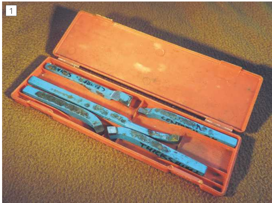
A typical set of inexpensive brazed carbide tools.
