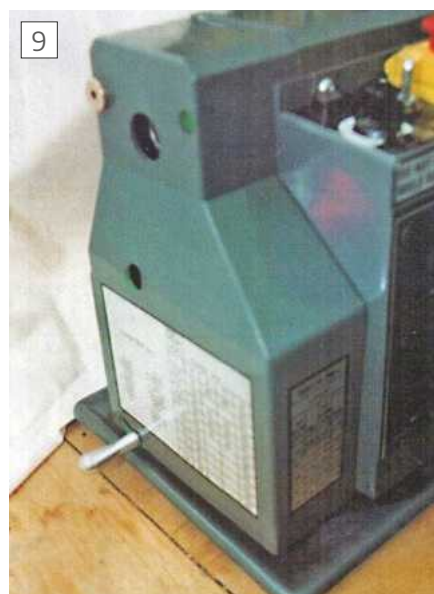
The small slot in the end casing and the swing arm operating lever.
