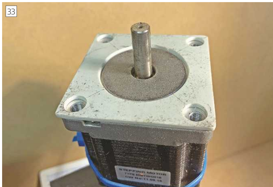
ABS spacer on top of stepper motor.
