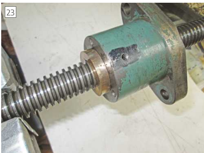
Trial fitting of knee nut in the support casting showing the locating grub screw
