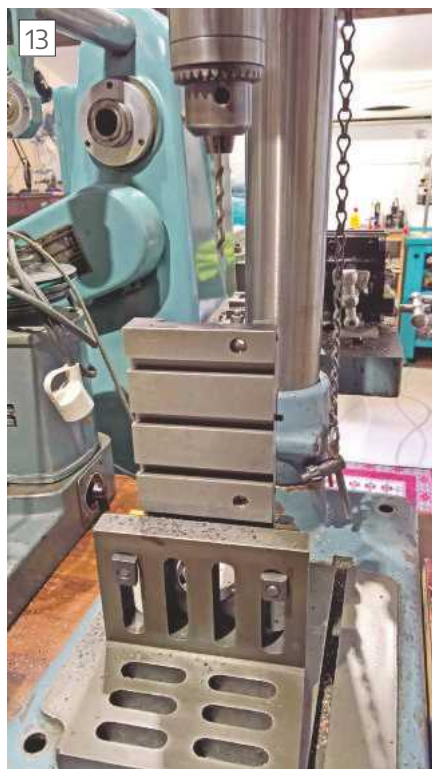
The Boxford used to drill the Myford cross slide
