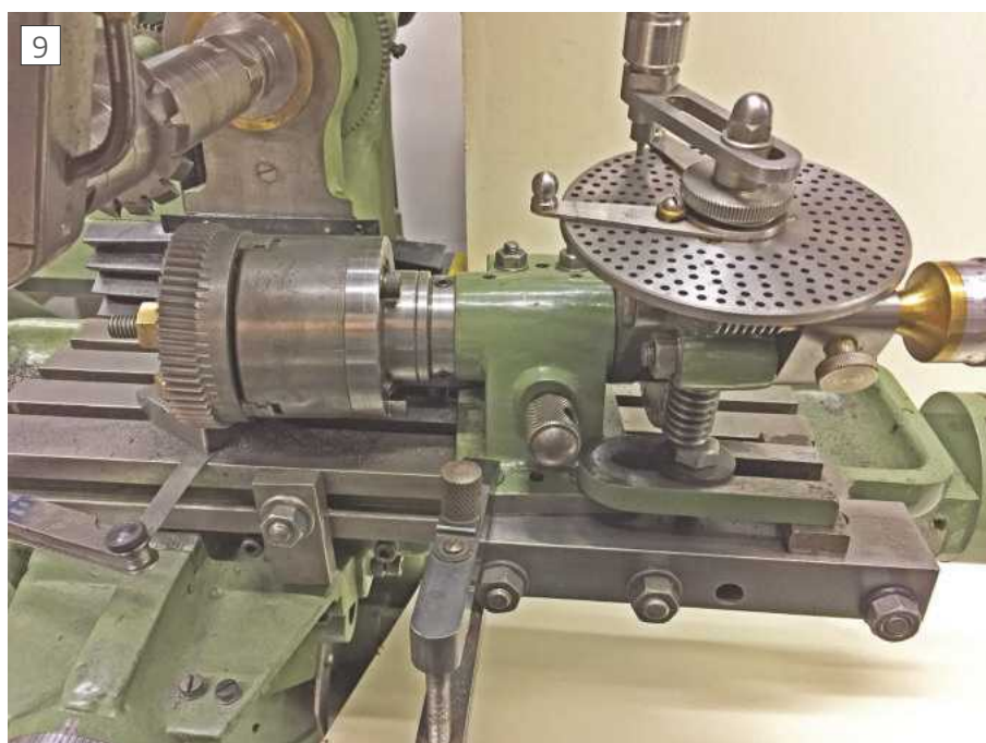
Setting the helix angle of 5.5247°
