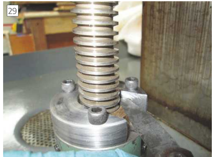
Checking the gap to give full seating
