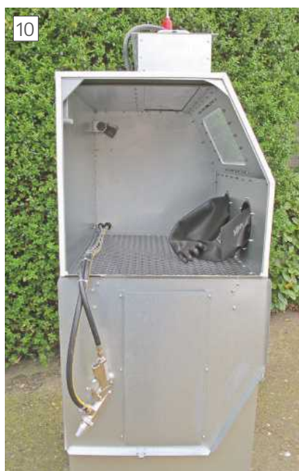
Internal view of my completed cabinet with gun resting outside to accommodate easy removal of the work and the expanded metal floor
