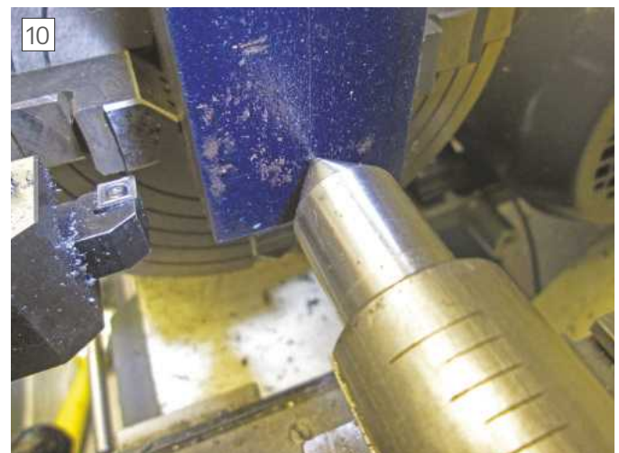
Setting up the cross feed nut housing ready for boring
