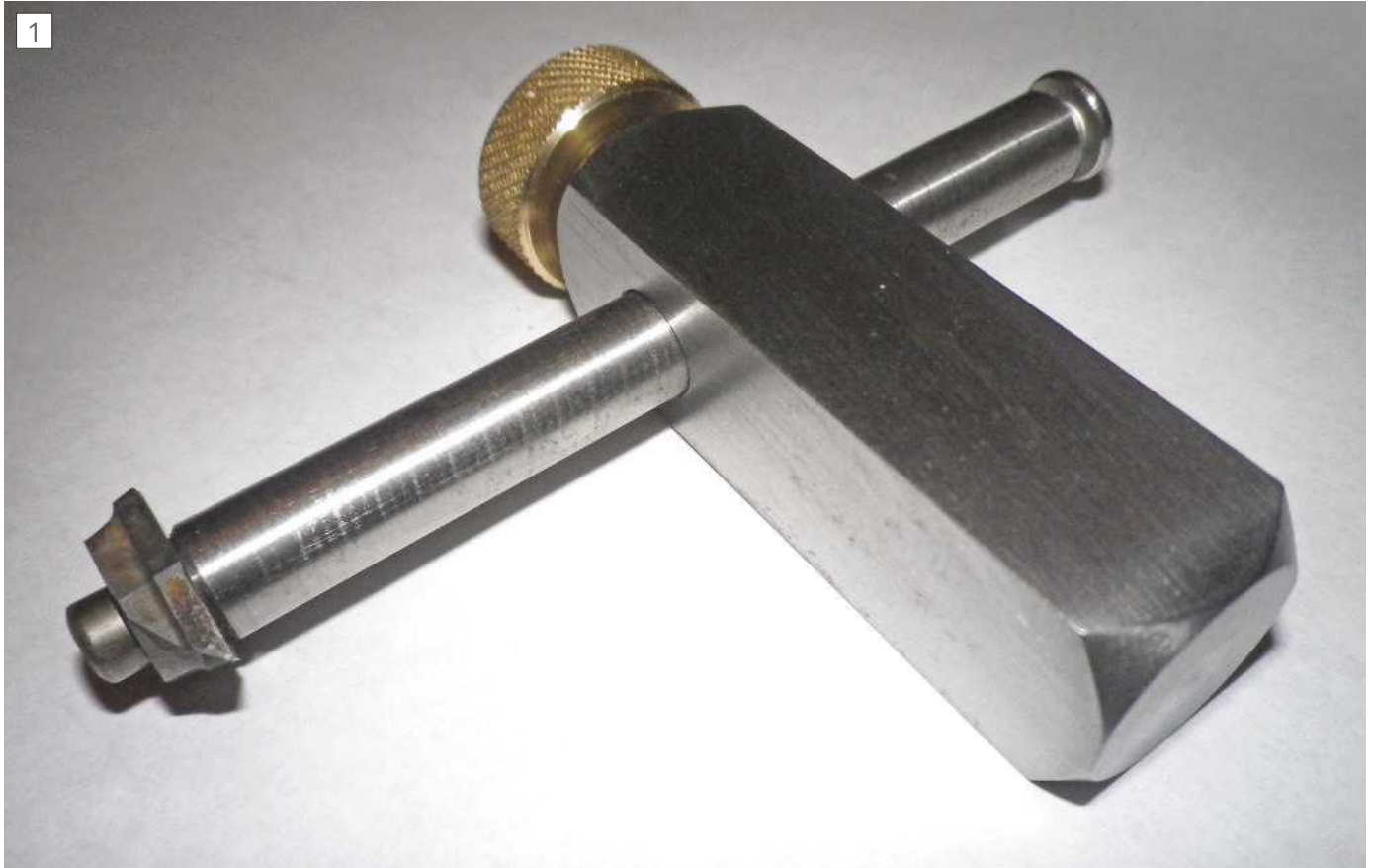
This neat scratch gauge offers greater precision than odd-legg or 'jenny' calipers.
