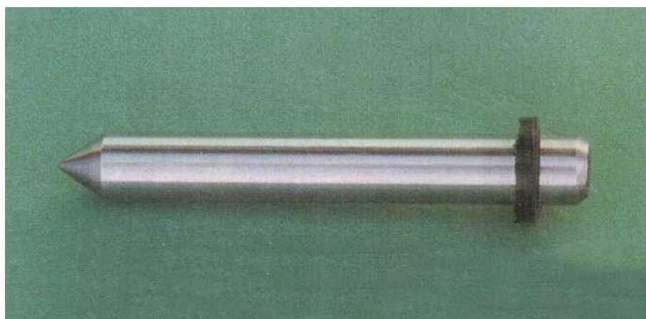
The centre punch. This, too, should be a sliding fit in the body; the 'O' ring at the top has no effect on the operation of the tool but makes it easier to handle.
