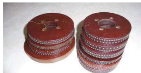
Photo 32: The range of home-made dividing plates available for use on the dividing head. (CH)
