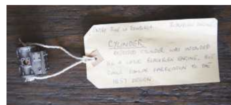
Photo 43: The rejected cylinder fabrication, of which the lower cylinder cover stud bosses were just too long, was used as 'supporting evidence' when the 1857 Blackburn engine was entered for the 'Duke of Edinburgh Trophy' competition, which it won. (JL)
