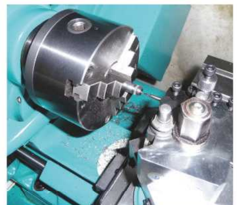
Photo 39: Slotting the worm wheel keyway on the Myford. The bore is 9/32in. diameter and the keyway is .024in. wide. (CH)
