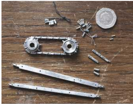
Photo 22: Some items of the rear cultivator drive of the 1863 Blackburn engine, showing how some of the chain components are developed. (JL)
