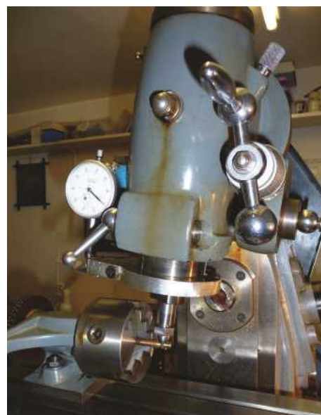
Photo 30: The Centec ‘A’ milling machine set up for gashing a worm wheel. (CH)
