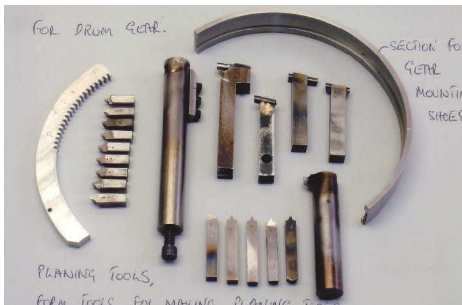
Photo 42: The tools used to cut the internal gear seen in photo 41 with the 'tools' used to make the tools. (CH)
