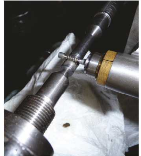
Photo 37: Lapping in progress – always remember to protect the lathe bed! (CH)
