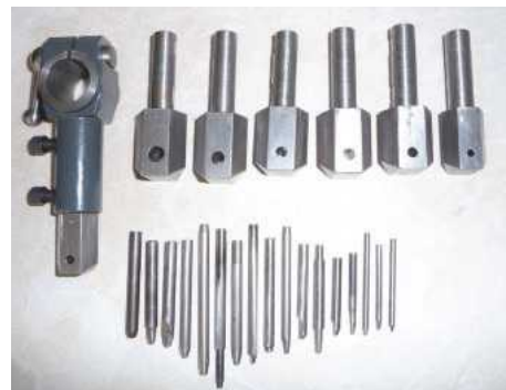
Photo 29: The tools of various diameters are located directly in the adapters which are plugged into the special top arm. (CH)
