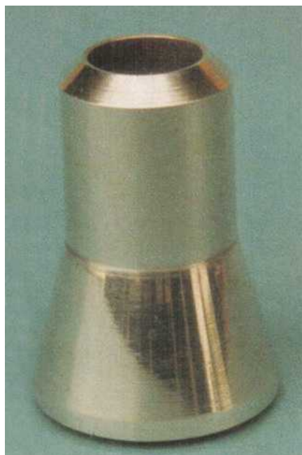
The body of the optical centre punch; this one is from aluminium but almost any material will do.
