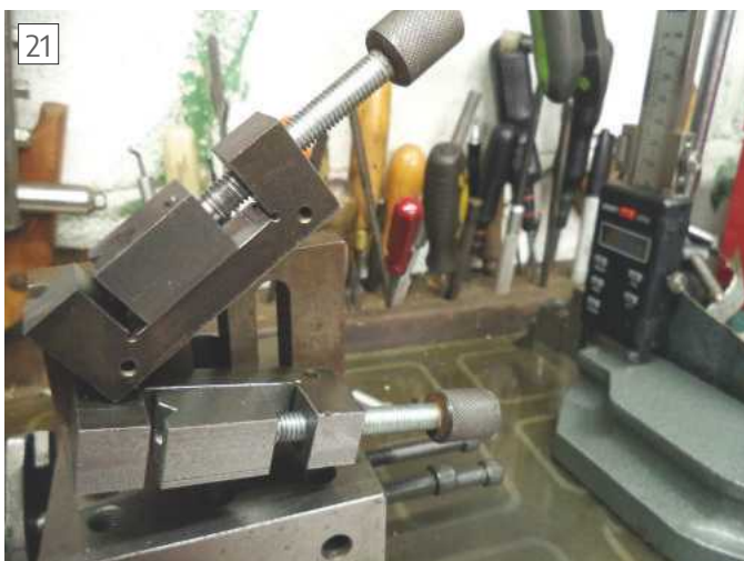
Clamps fixed to an angle plate in different orientations.
