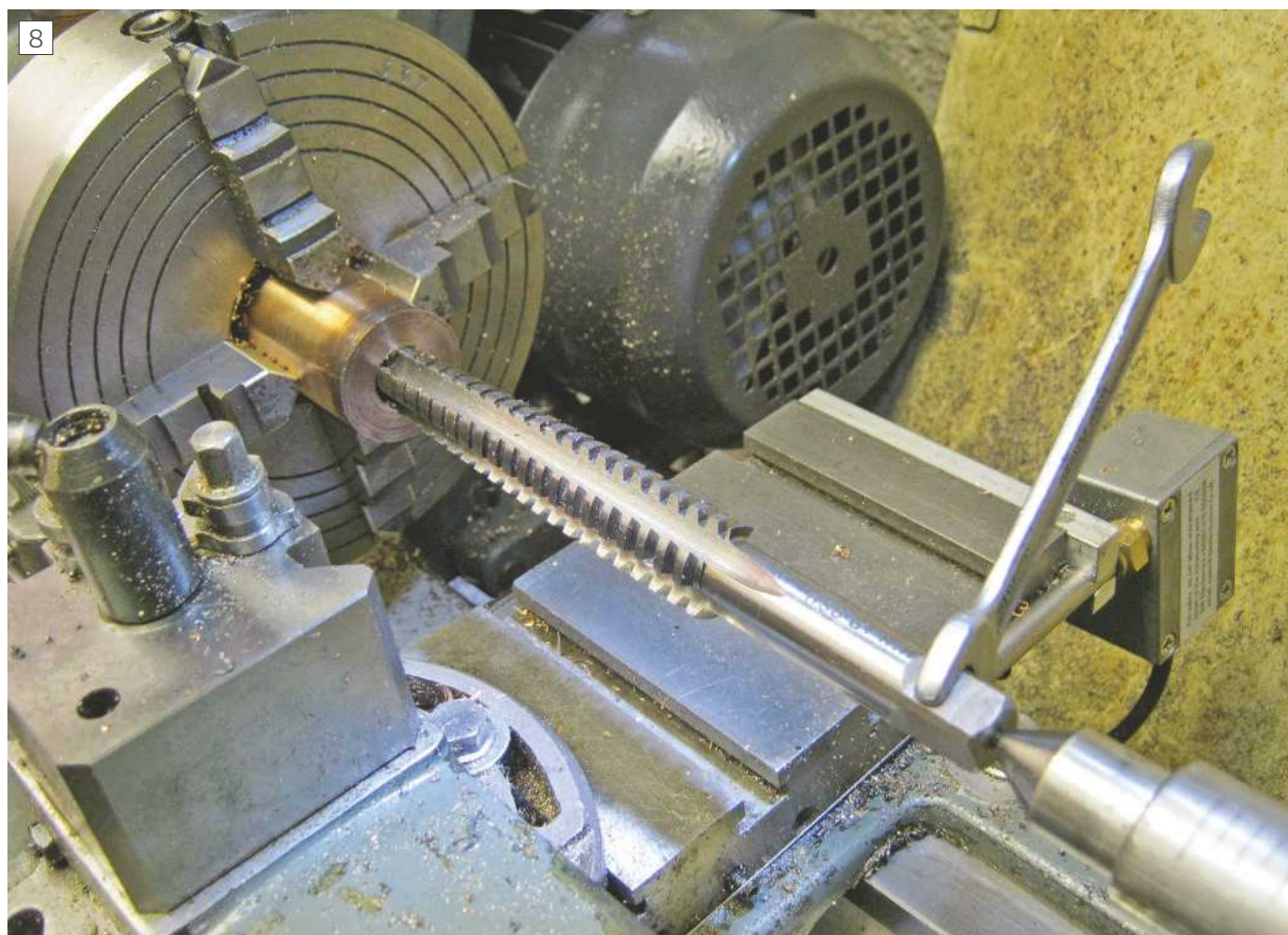
Tapping the table feed nut
