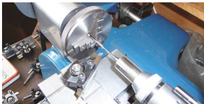
Photo 34: Machining a worm gear on the IME 100 lathe. (CH)
