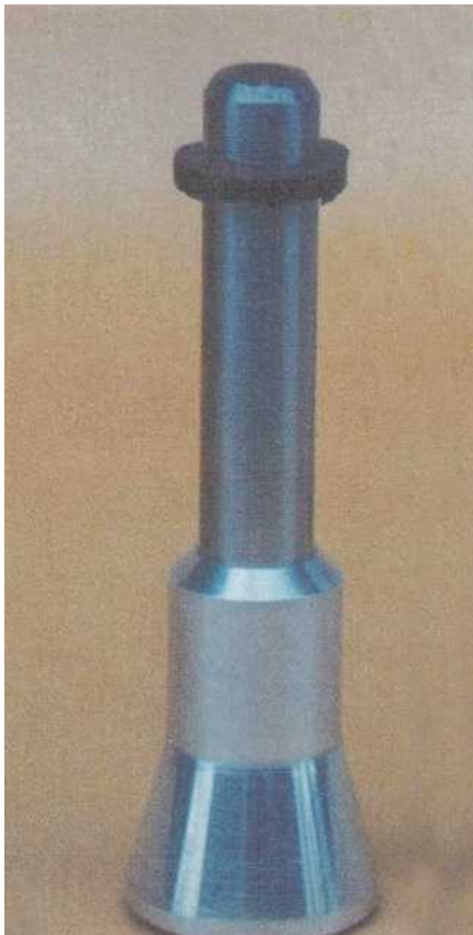
When the body is in the correct position the magnifier is removed and replaced by the centre punch.
