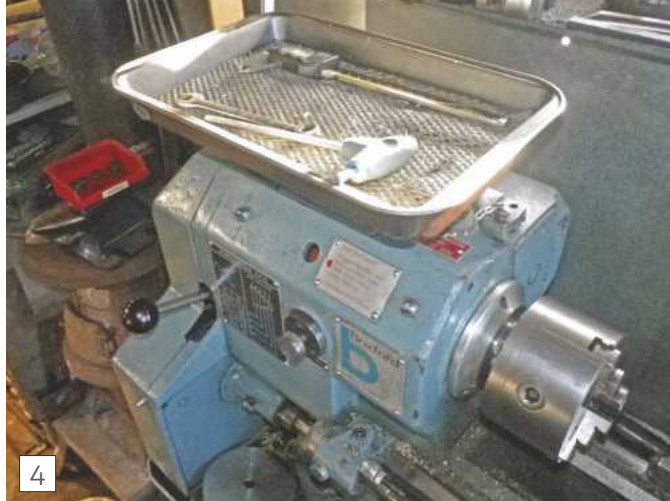
4 A simple tip for a magnetic tool tray that will suit many lathes with a large leadscrew gearbox.
