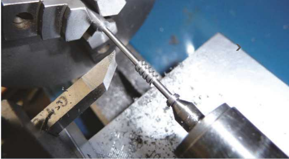
Photo 35: A slender worm shaft requires carefully sharpened tools and fine cuts! (CH)
