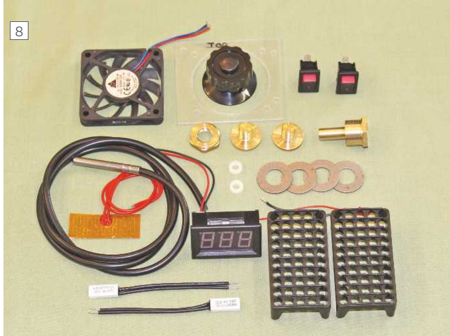
Additional small parts used to complete the build, including 4 brass components made from \frac{1}{2} " to \frac{1}{4} " BSP brass couplings. The centre pair are for fixing transducers, the other two are for plumbing the pump to the PVC tubing and for mounting the crane.
