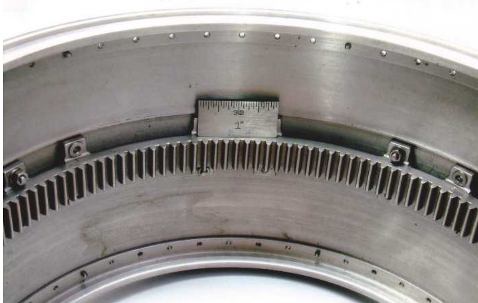
Photo 41: More gear cutting, but this time the internal gear which can be seen on the inner periphery of the drum in photo 2. (CH)
