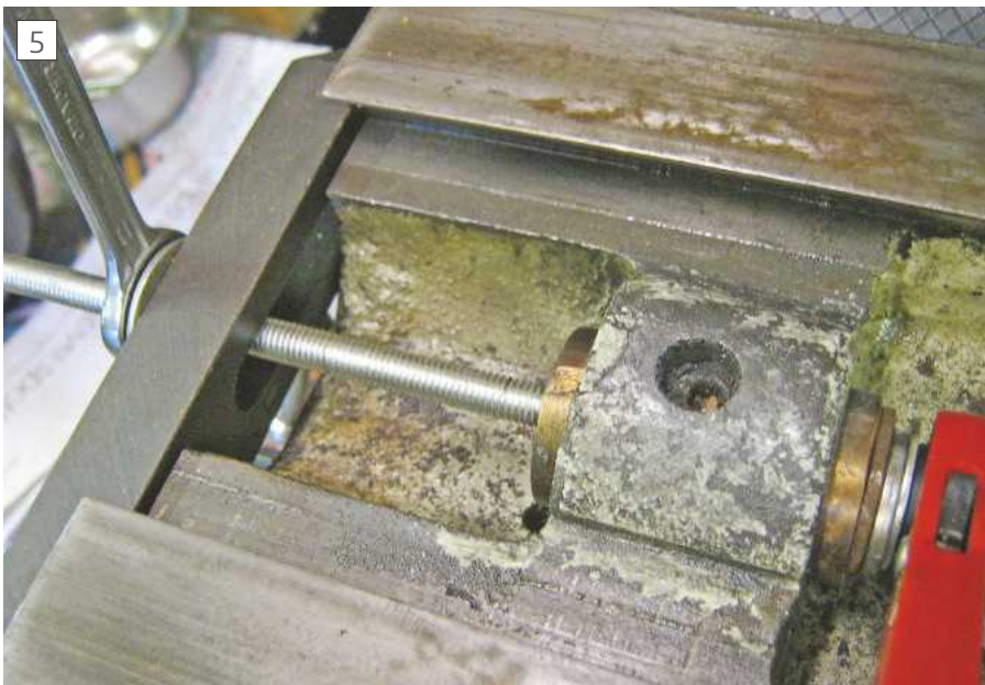
5 & 6 Removing the table feed nut from its housing in the cross feed casting
