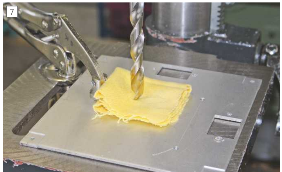
The alternative method of drilling thin sheet metal by plunging a twist drill through a wad of fabric into the metal. However, this technique is not always effective.
