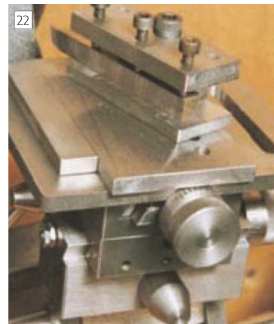
Using the square tool holder on the swivel base to sharpen a lathe tool.
