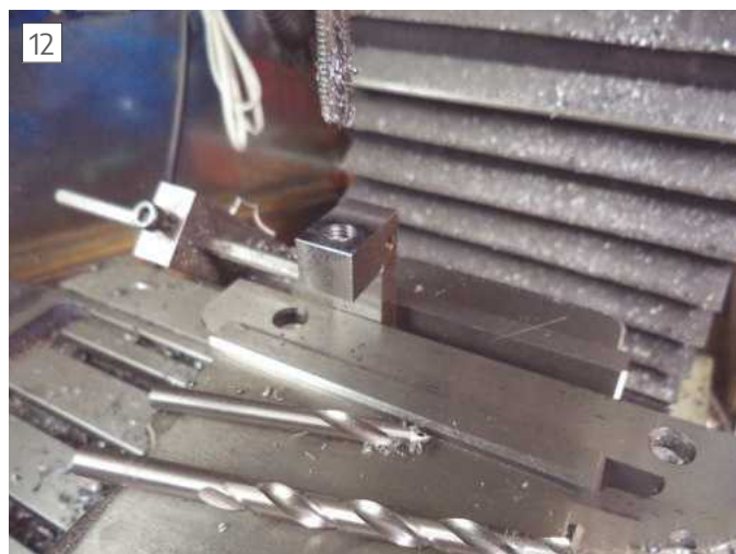
Drill and tap m8, note use of end vice stop.
