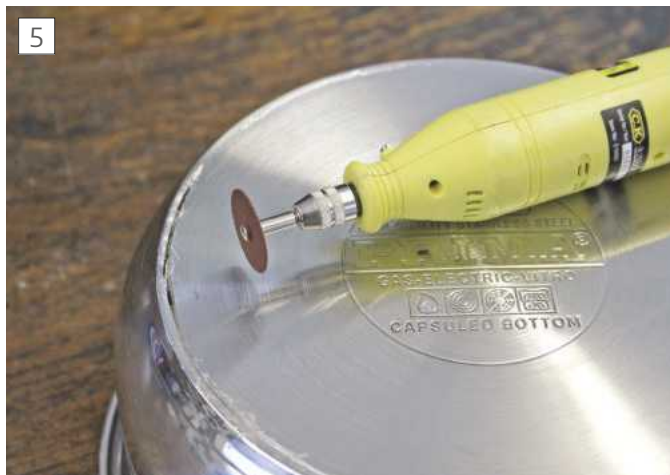
Using a carborundum disc in a rotary tool in an attempt to remove the encapsulated outer layer. The outcome was to puncture the bowl.
