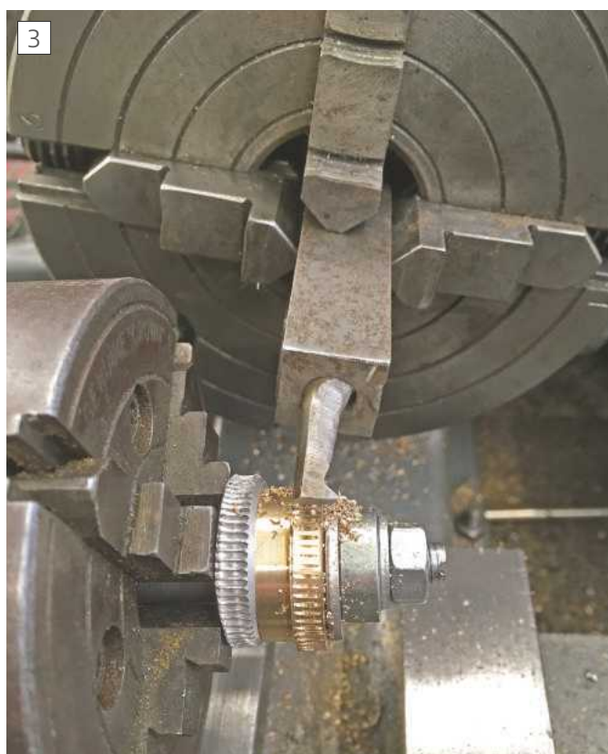
Setting the tool to cut the worm gear.
