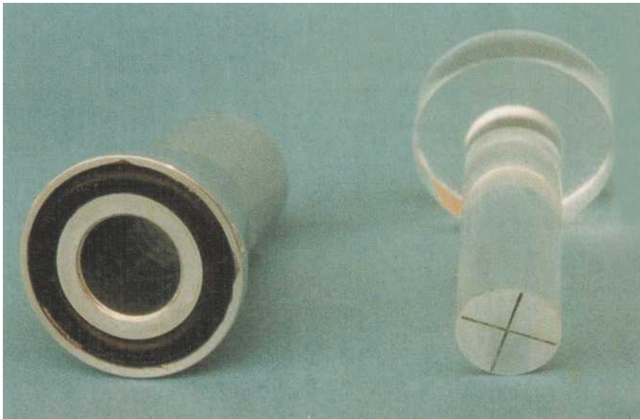
The ends of the body and magnifier. The 'O' ring recessed in the body prevents accidental movement when adjustments are made. Black felt-` tip pen ink wiped over the base of the magnifier picks out the cross-hairs.
