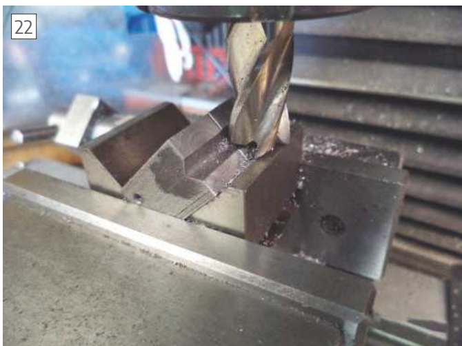
Milling a vee across the jaws with an end mill.
