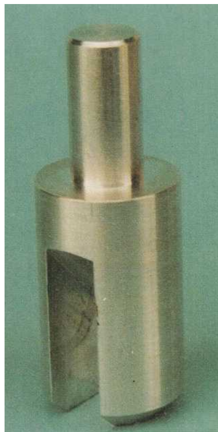
The body of the centre-finder showing how the slot has been milled out to accept the lens.
