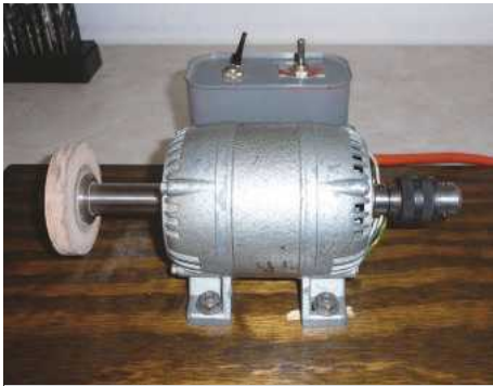
Photo 21: A simple buffing and polishing spindle is a vital tool when imparting the high finish which Cherry achieves. (JL)
