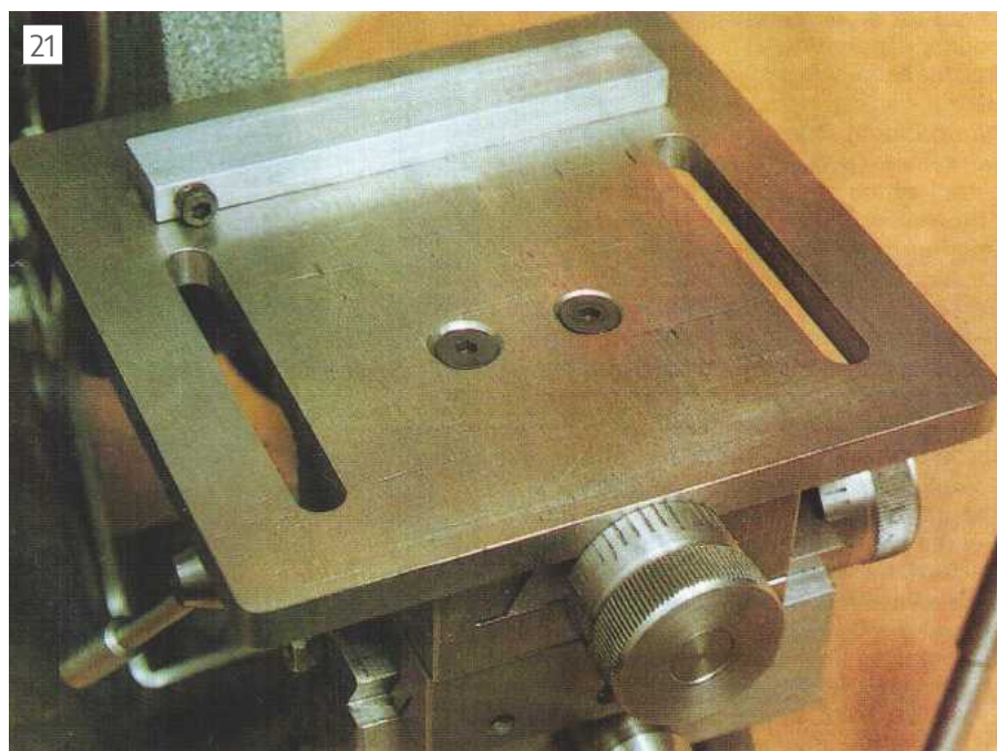
The finished fence in position.
