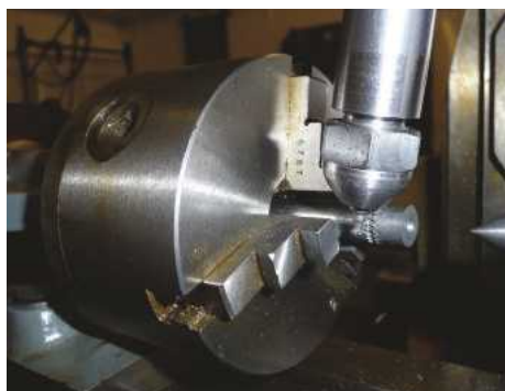
Photo 33: The gashing of a worm wheel nears completion. (CH)
