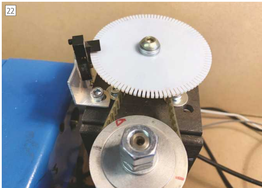
The setup for measuring the speed of the cutter spindle.
