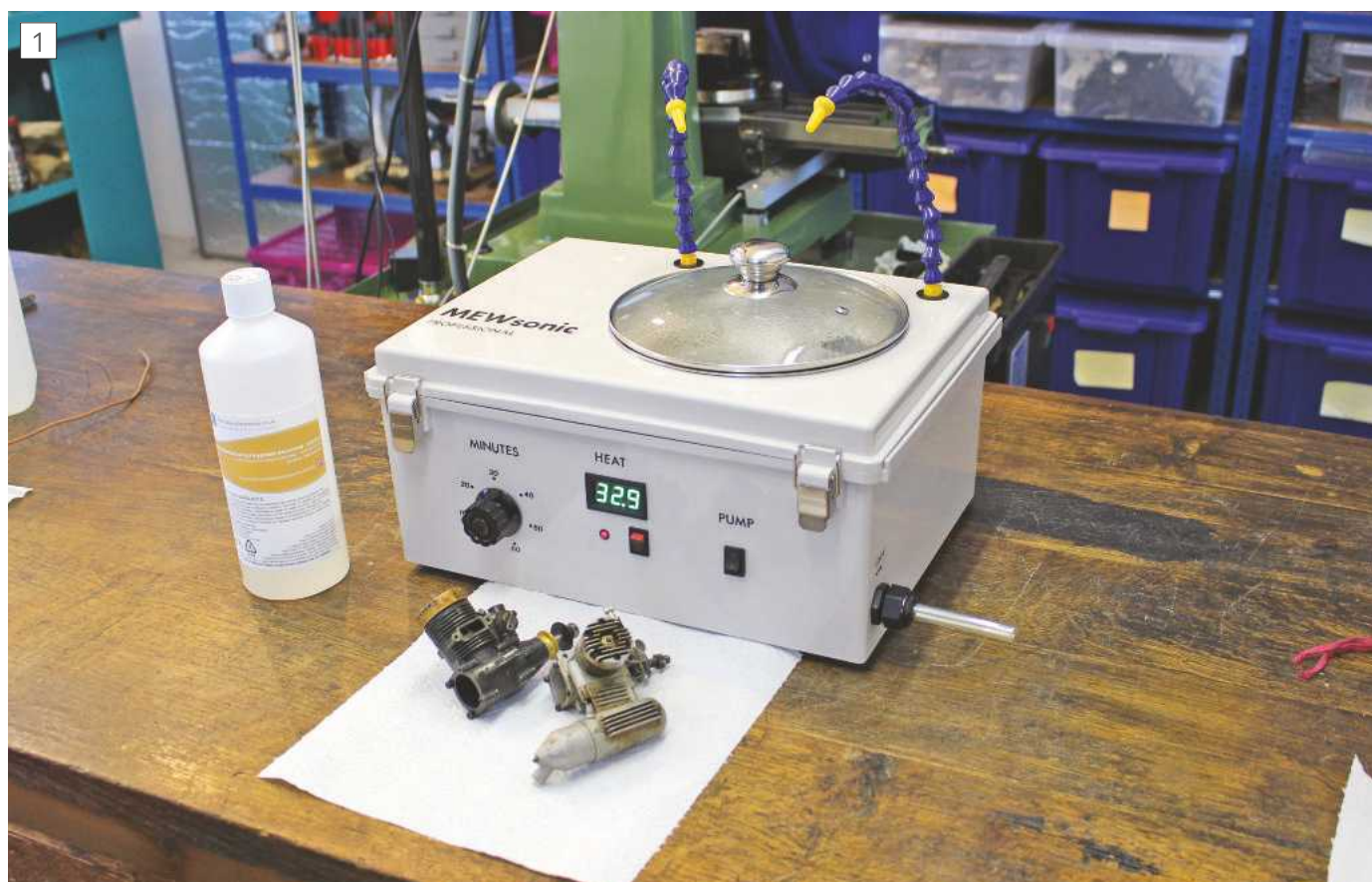
The completed MEWsonic Professional. The blue flexi-tube on the right is for sucking cleaning fluid from the tank, while the one on the left is used to suspend parts for cleaning.
