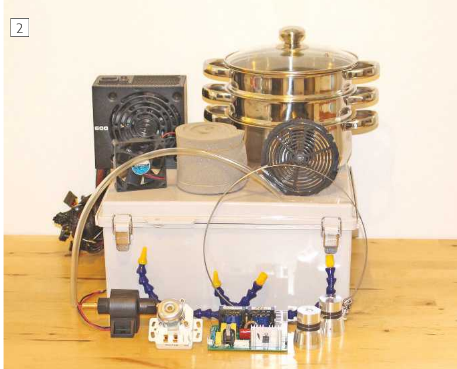
Major components for constructing the ultrasonic cleaner, including the lower pan of a steamer set and an ABS box by CamdenBoss. The pair of 40kHz transducers and driver board are seen at lower right.
