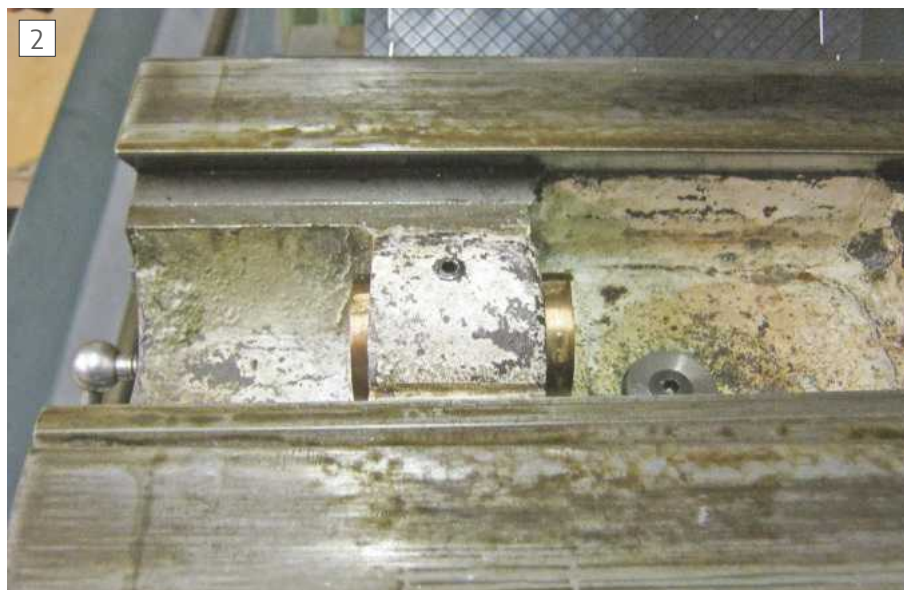
The table nut in situ in the cross feed casting
