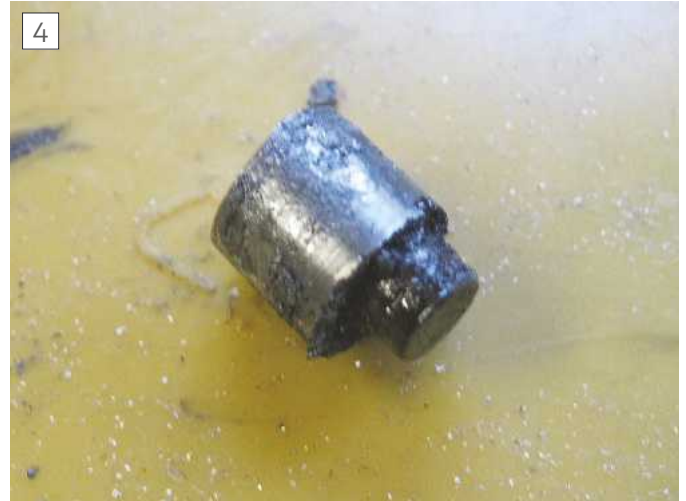
The removed grub screw with surrounding metal of the casting
