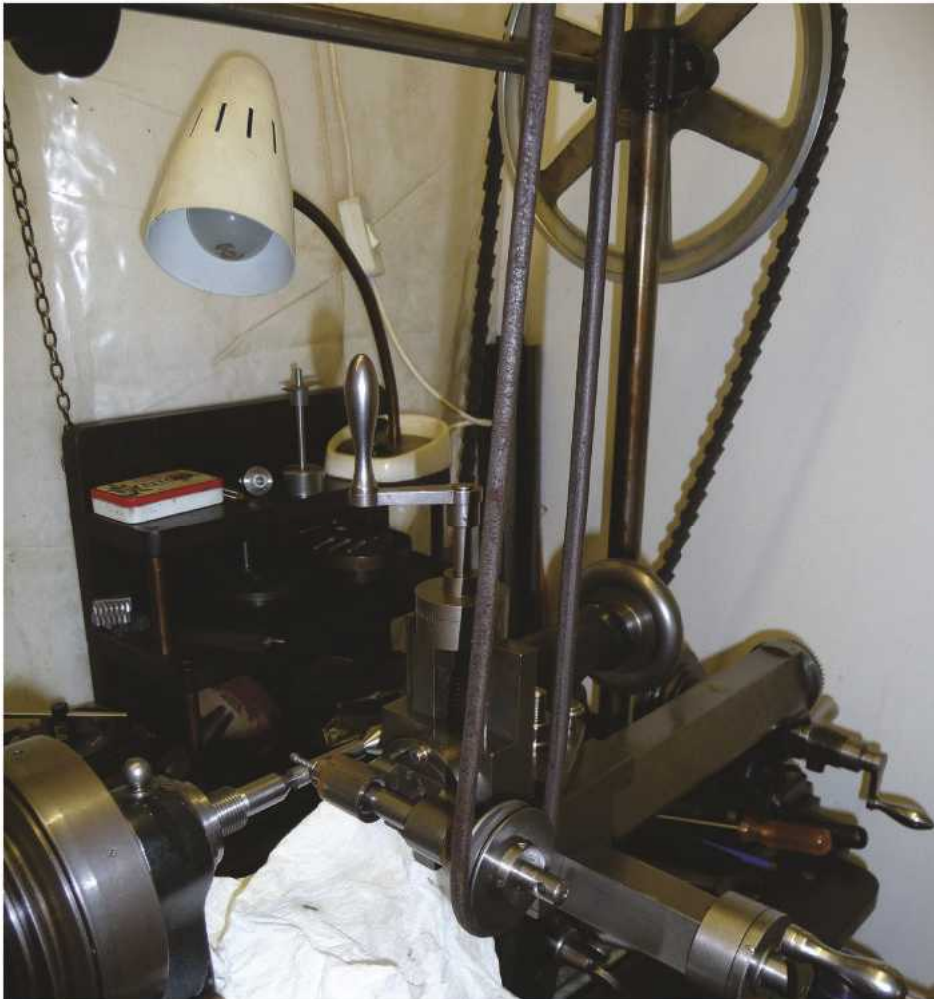
Photo 36: The Pittler lathe and overhead drive set up for lapping a worm gear to its worm wheel. (CH)
