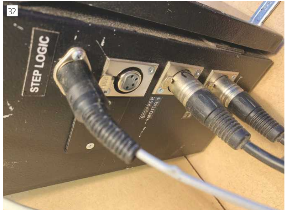
32 Sockets for stepper motor XLR plugs and DIN socket for connection to Arduino.
