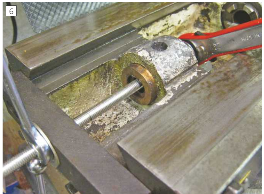
5 & 6 Removing the table feed nut from its housing in the cross feed casting
