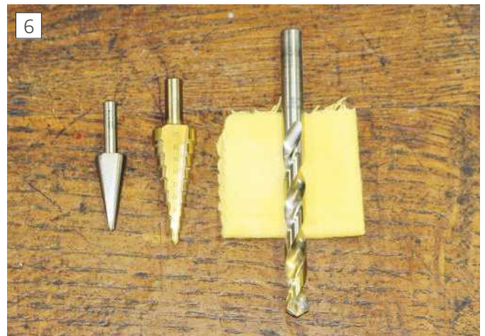
Choice of drills for safely boring holes in thin sheet material. Sometimes the combination of a plain twist drill and a fabric wad can be effective.
