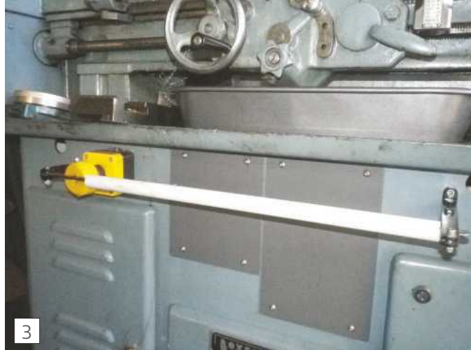
3 This rod across the front of the Boxford BUD is arranged to provide a reliable leg-operated emergency stop.
