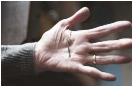
Photo 24: The small size of Cherry's models requires the manufacture of a significant number of special tools, many of them being special spanners such as this, each being hardened. (JL)
