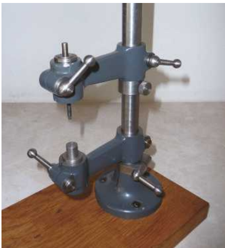
Photo 27: The UPT set up in 'light' staking mode i.e. with the 'anvil' set in the arm, rather than in the base. (For heavier riveting and staking, a set-up similar to that shown in photo 28 is used.) (CH)
