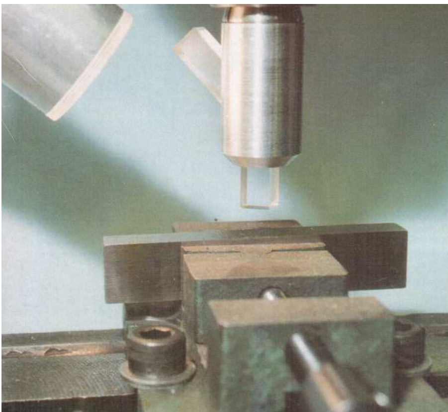
The completed optical centre-finder in the milling machine; in actual use it would be brought closer to the work than shown in order to line it up accurately.
