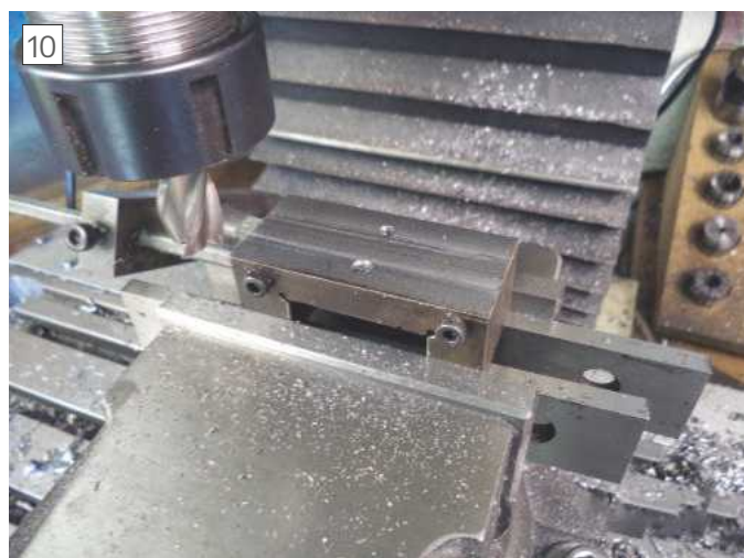
Skimming off distortion.
