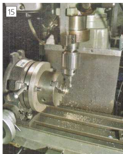
Set up using rotary table to mill hex on pivot post.
