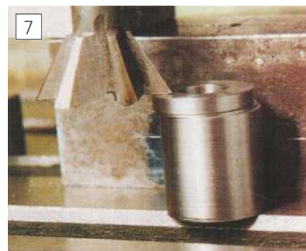
Setting the depth of dovetail using distance pieces.
