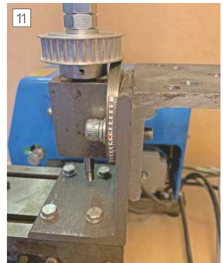
Spindle backplate and motor mount bolted sandwiched either side of mounting plate.
