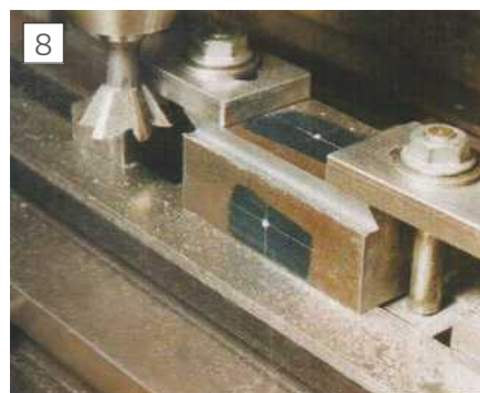
Cutting the dovetails in the lower slide.
