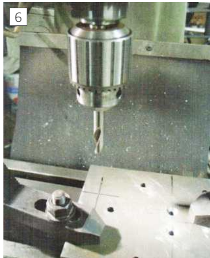
Initial marking out by felt tip pen although the c/s hole spacing was accurately controlled.
