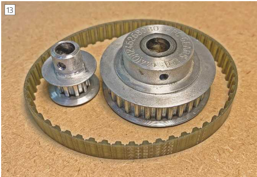
Spindle timing belt and pulleys.
