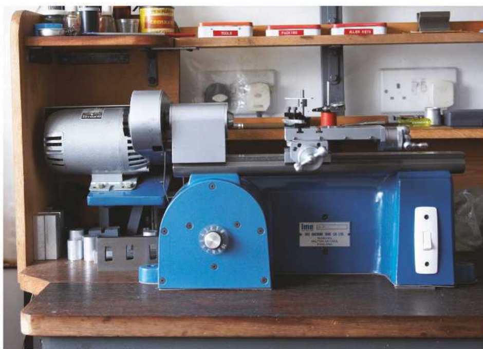
Photo 18: IME lathes were made by The Ideal Machine Tool and Engineering Company of Kingsland Road, London E8. Cherry's is one of the Model 100 Series. (JL)
