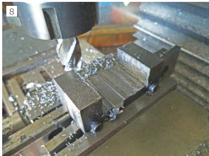
Rough out using end mill.
