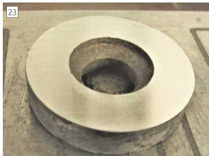
Spacer- surface fully ground
