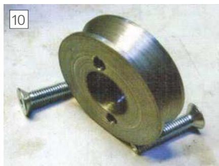
The finished spigot showing the relieved inner area of the abutment face.
