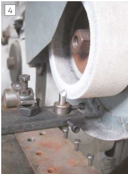
Grinding flat on top of insert
