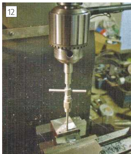
Tapping using a pump centre for alignment.
