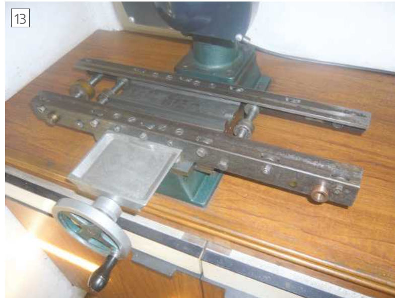
Guide bars mounted on the cross slide block
