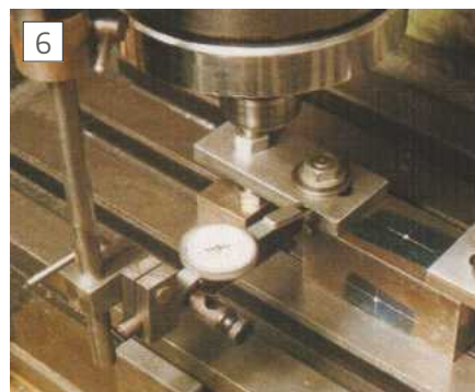
Positioning the lower slide prior to cutting the dovetails.
