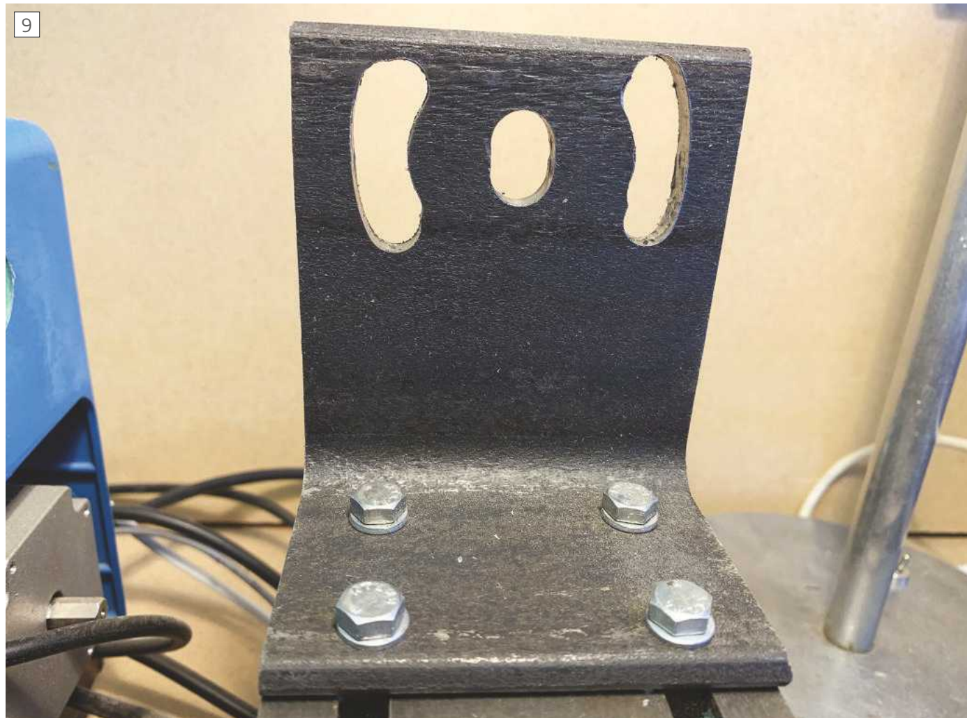
Spindle assembly mounting plate bolted to crossslide.
