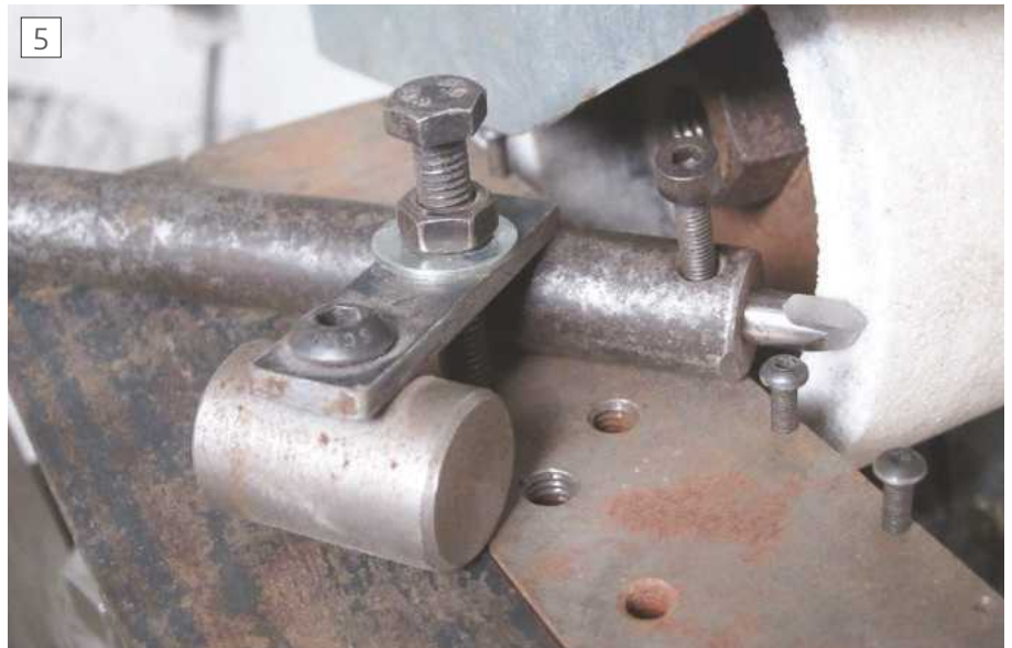
Grinding insert for boring bar, rake obtained by rotating holder
