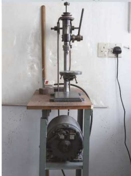
Photo 17: Another survivor from the Hines family original workshop is this small sensitive drilling machine. (JL)
