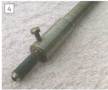
A sharpened tool from silver steel.
