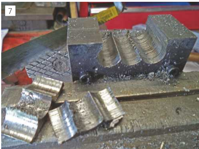
Excess material quickly removed.
