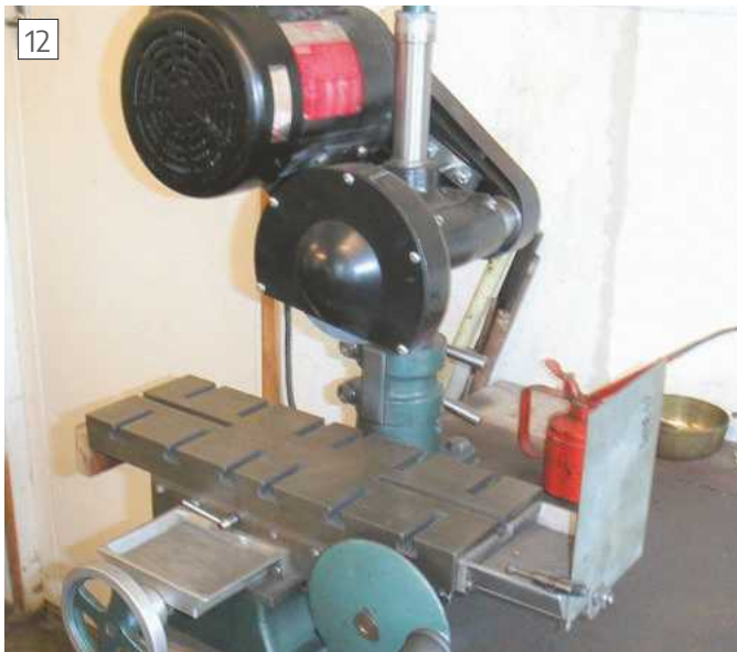
First table drive & original motor
