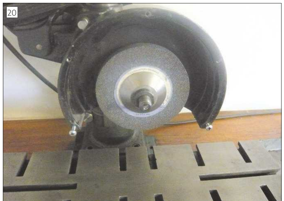
Grinding wheel with front cover removed
