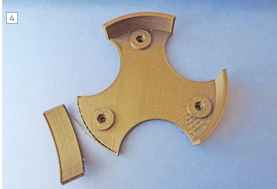
Firm hand pressure was enough to snap this prototype part along the layers.
