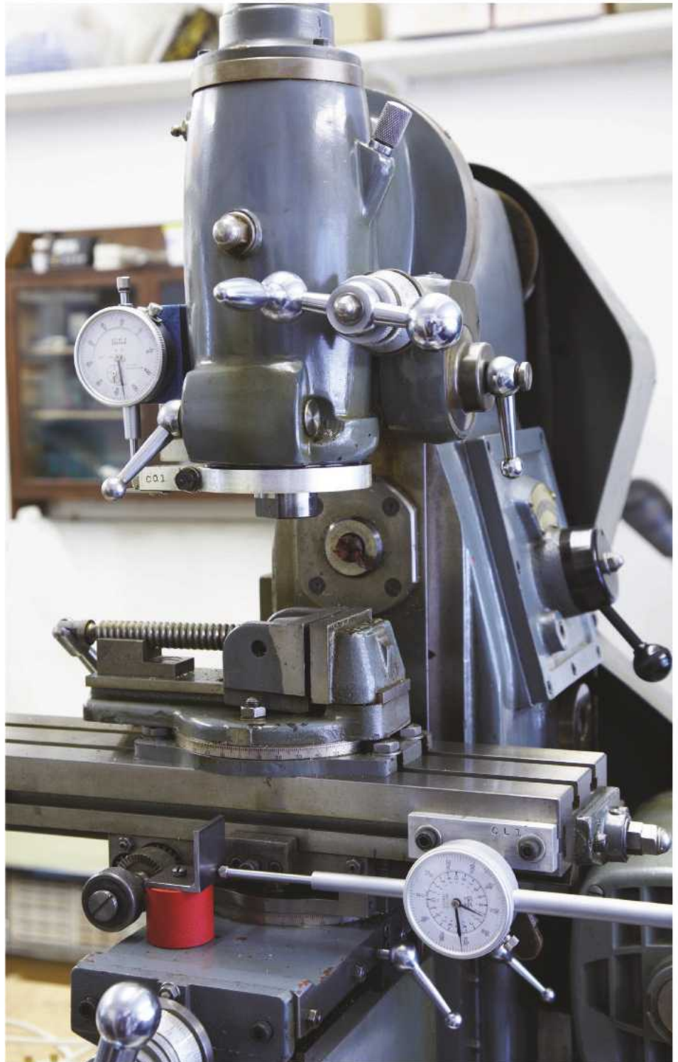
Photo 14: The Centec 2A has been fitted with dial gauges to measure travel on the X and Z axes. (JL)
