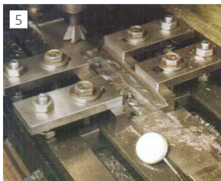
Finishing the dovetails in the slide swivel pieces.
