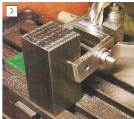
Machining the ends of parts cut from 50mm square bar.
