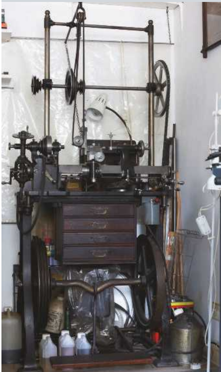
Photo 8: The 1913 Pittler lathe is set up for dividing and milling, having been motorised at some stage of its career. (JL)
