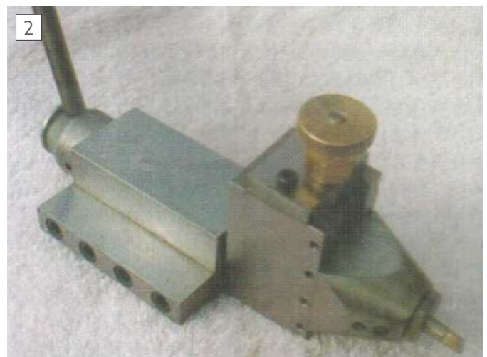
A ball turning tool based on that marketed by Hemingway kits. ➤
