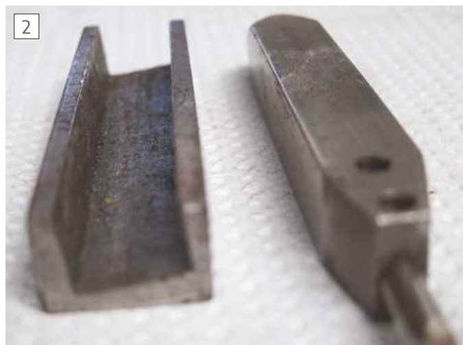
Profile of jig to obtain side rake
