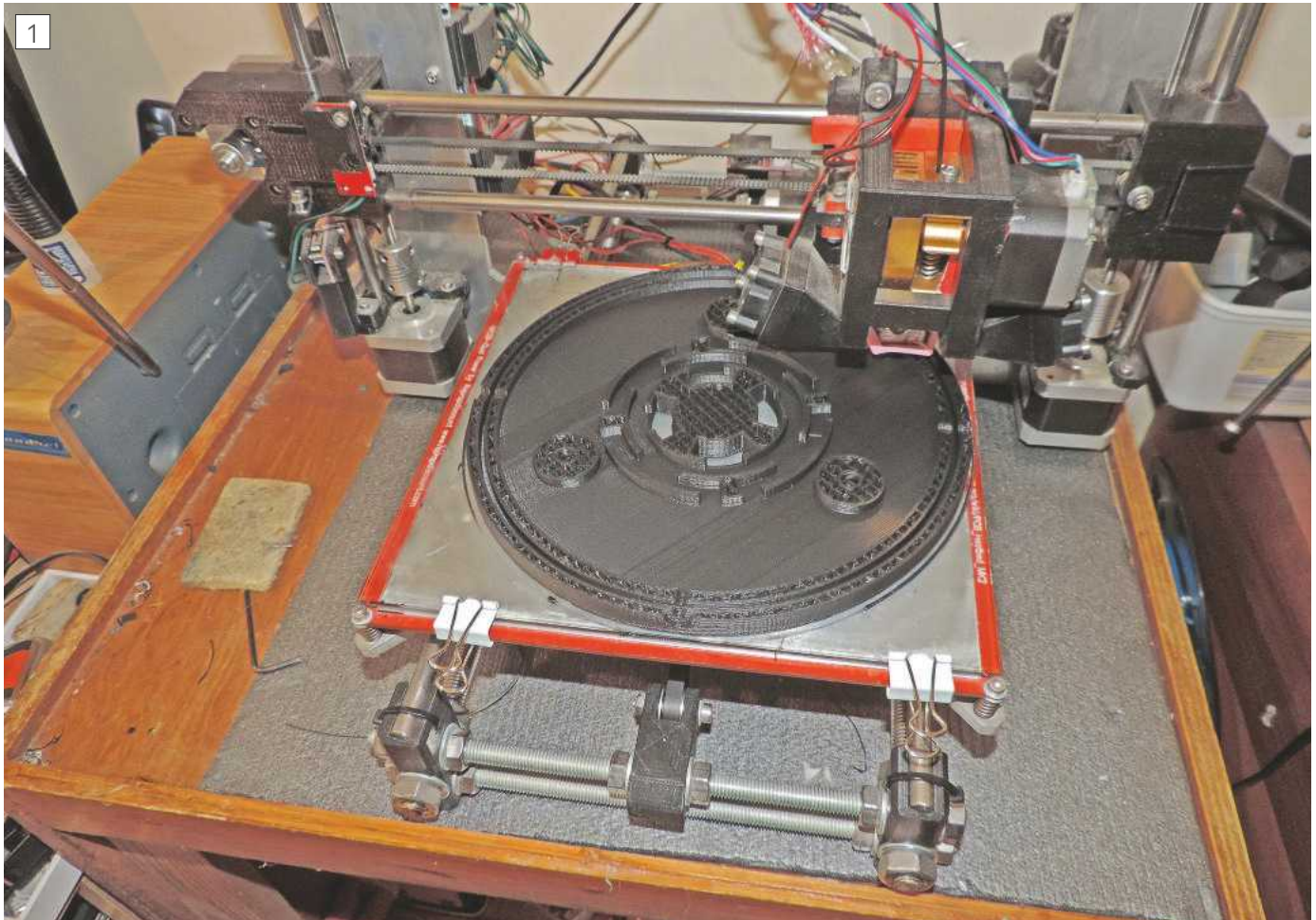
Printing the base for the mirror cell.
