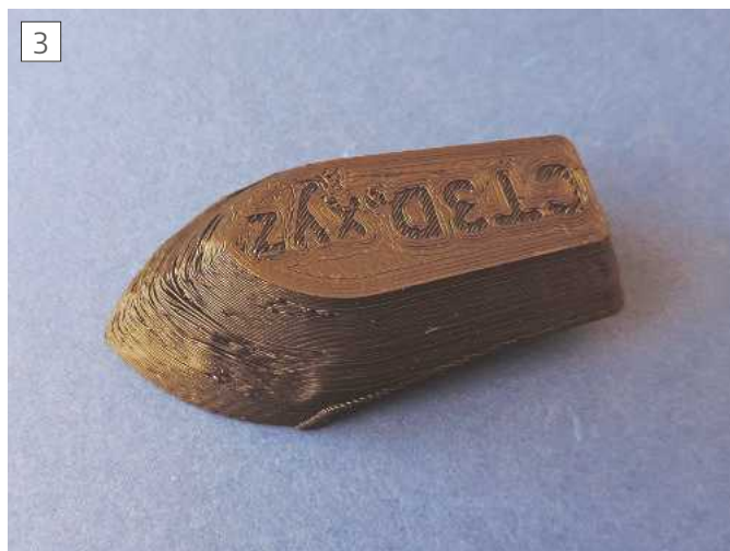
The underside of an aborted print of a 3D Benchy shows warping and poor adhesion on the overhang.
