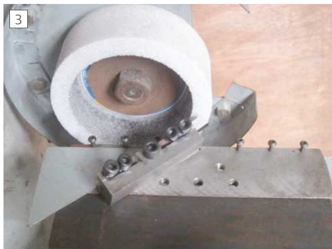
Jig set up turning tool insert
