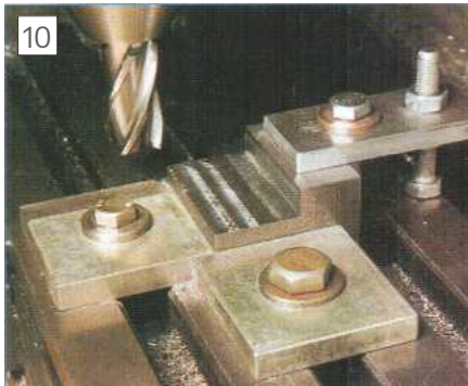
Machining the lower arm spacer. With only one clamp being used the supports are essential for added security whilst machining.
