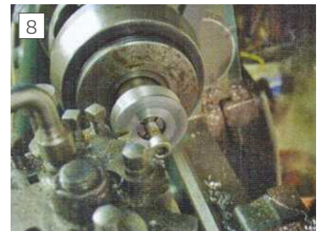
The spigot located on an expanding mandrel.
