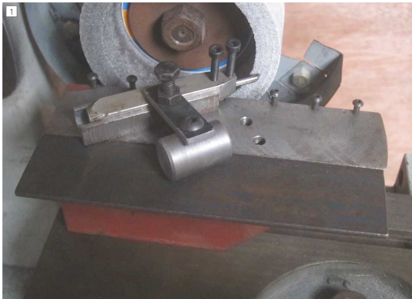
Jig set up for screw cutting insert
