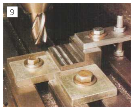
Cutting the slot in the lower slide.
