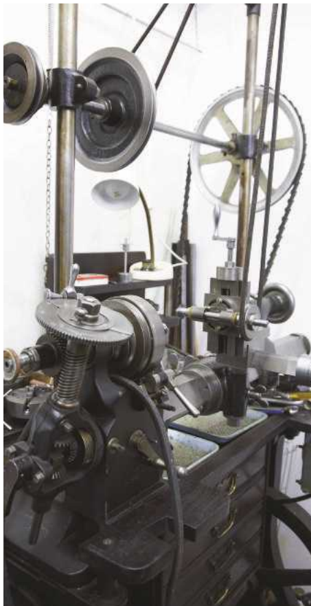
Photo 9: The Pittler overhead drives the cutter frame. (JL)
