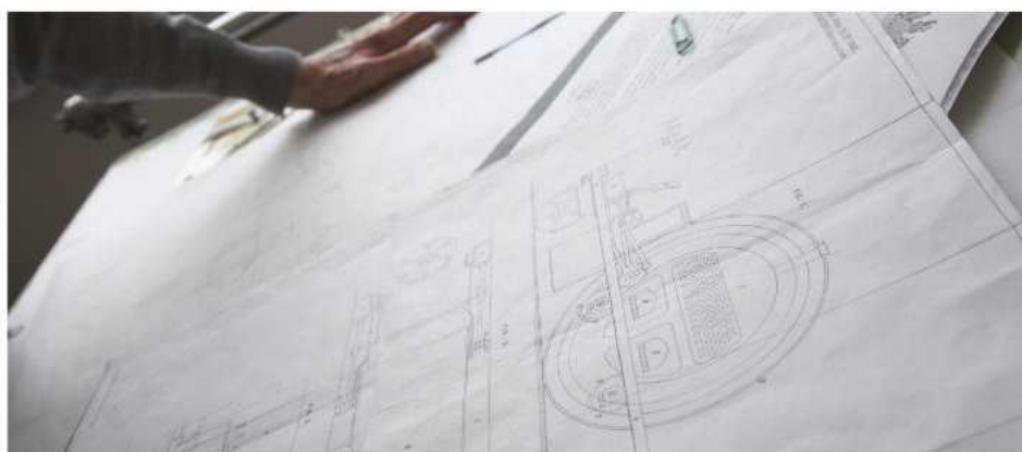
Photo 4: Drawings are still made in the traditional way, without the aid of electronic equipment, drawn at either full size or ten times full size. (JL)
