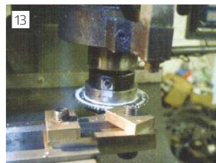
Cutting the slot in the adjuster slide with a slitting saw.
