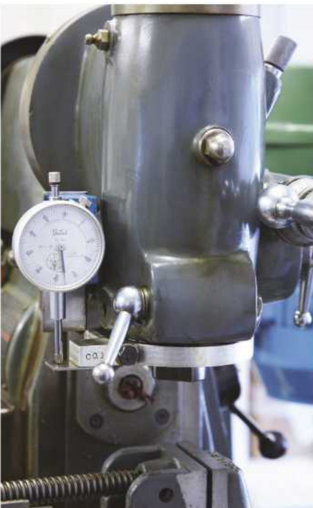
Photo 15: A simple collar clamped to the quill bears against the plunger of the Z axis clock. (JL)
