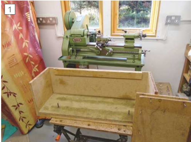
The ML10 re-assembled, grease cleaned off, and in pristine condition out of the crate after 9 years storage; the crate has hold down bolts through the base to hold the bed in place and all loose parts were bubble wrapped and held securely.
