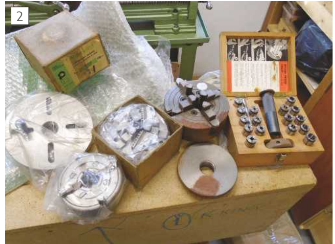
Right and wrong; chucks and faceplate to the left were greased up/sealed in poly bags and like new but 4 jaw and catchplate were just in a cardboard box. The rust is clear as is some on the collets which were in the collet box in a plastic bag but the bag was tied not taped closed.
