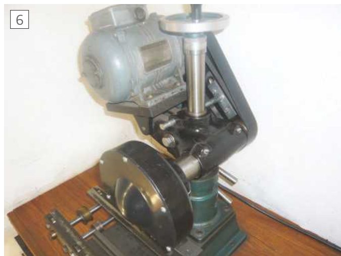
Vertical Support column shortened
