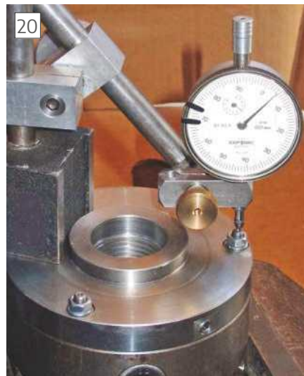
Measuring stud elongation.
