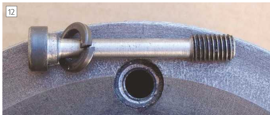
already tapped in the chuck body. Here a stack of two Belleville washers (parallel stack, full contact between the washers) is used as spring as there is some room to fit these washers. The washers dimensions are diameters 6.3 and 16mm, thickness 0.8mm, height 1.3mm, the “until flat” force is near 1000N so 2000N for two washers stacked in parallel.
