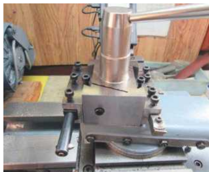
Warren Jacobs' Easy Quick Change Toolpost.
