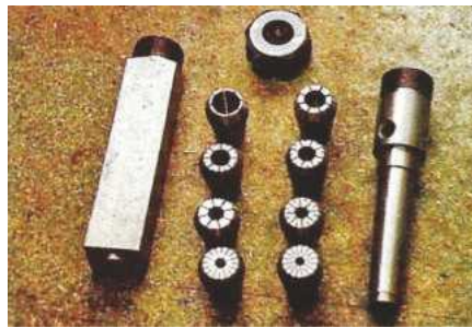
ER20 spring collets, normally used in the Morse taper chuck (right) can be fitted to the square holder (left) and used to hold a wide range of drill diameters.
