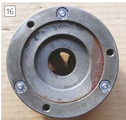
Hexagonal broached holes for nuts.
