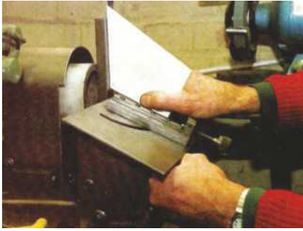
Setting the tip angle by tilting the table.
