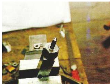
A sharpened drill in the ER20 spring collet.
