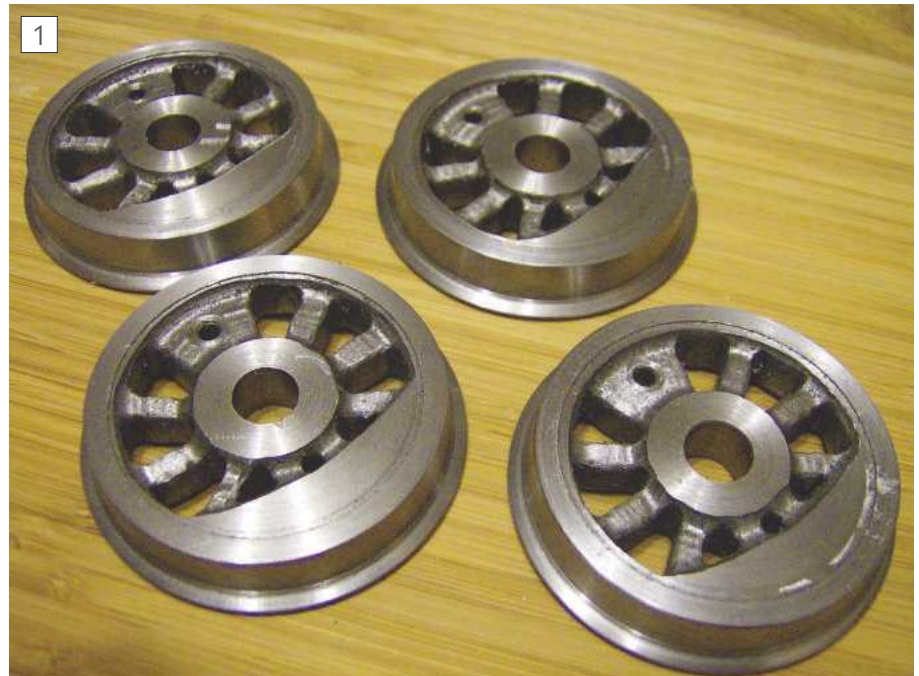
EN1aPb was used for these locomotive wheels which involved complex milling with small cutters.
