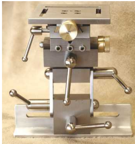
Grinding Rest by Rik Shaw made to Harold Hall's popular design:
