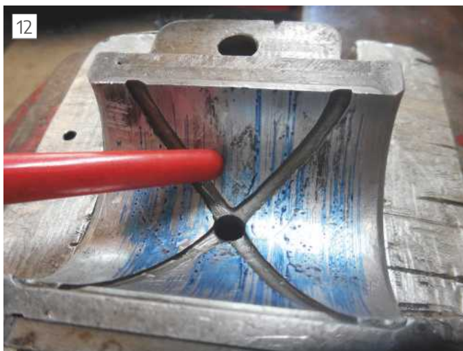
Shiny spot indicates very high spot with metal contact.
