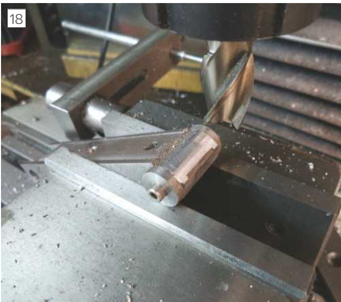
Milling facets to rough out radius
