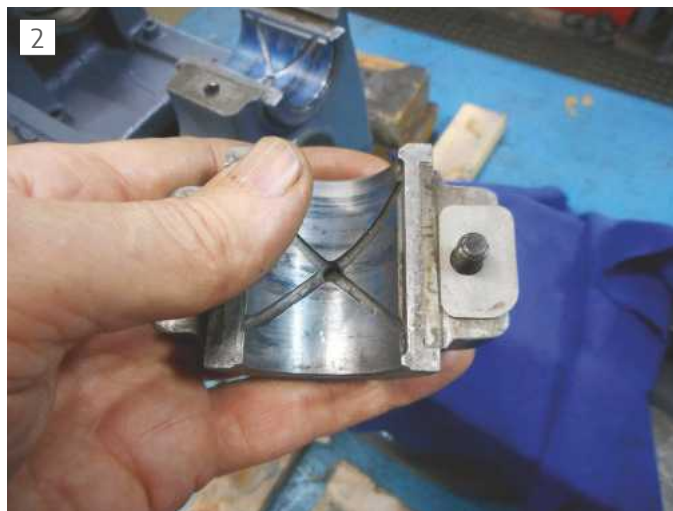
Shims between halves set bearing clearance.
