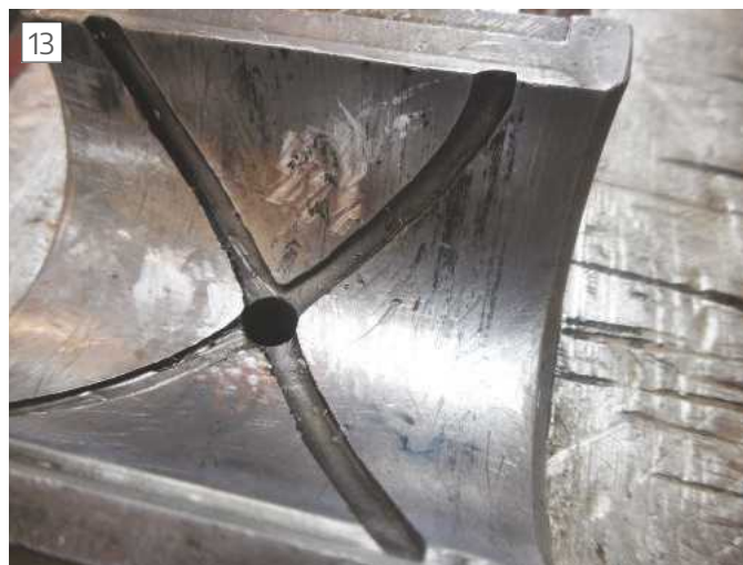
Very high spot is aggressively scraped.
