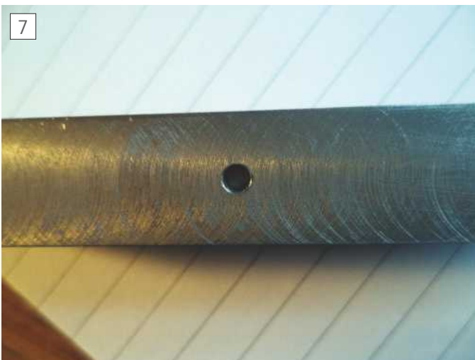
Witness marks confirming the mill is set up square
