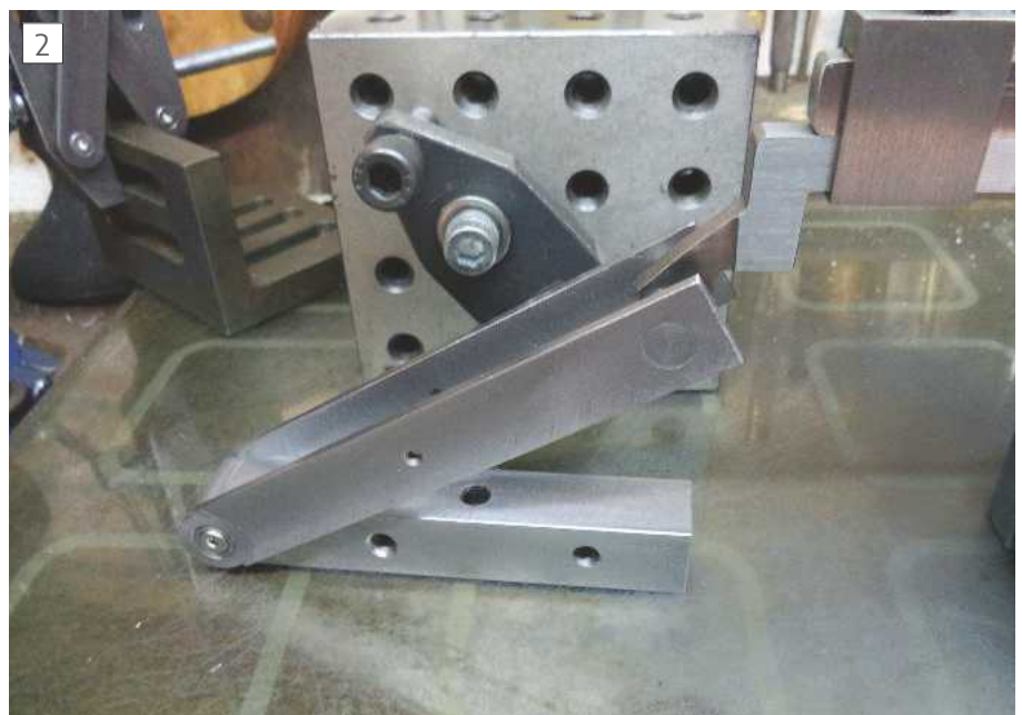
Height gauge 50mm sets protractor at 30 degrees
