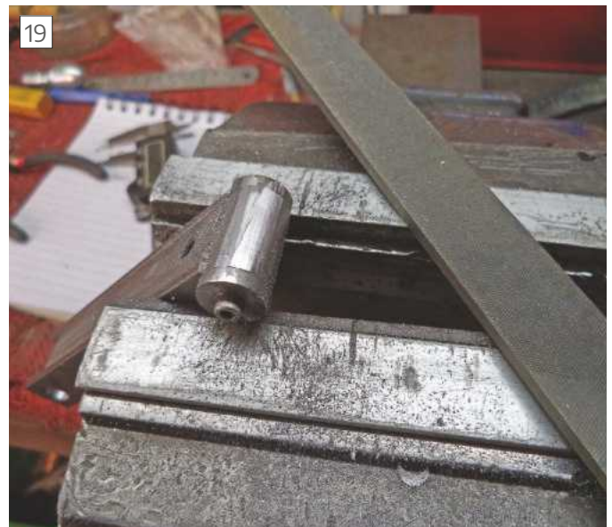
Finish off radius with a file
