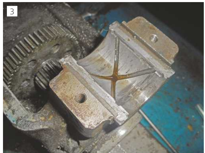
Bearing shell was scored and burned.
