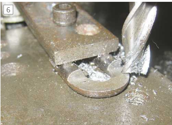
Machining the link
