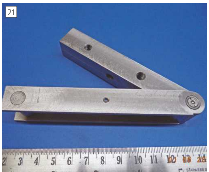
Completed Sine Protractor
