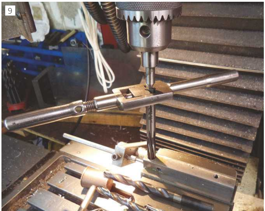
Using a hand 10mm hand reamer to finish
