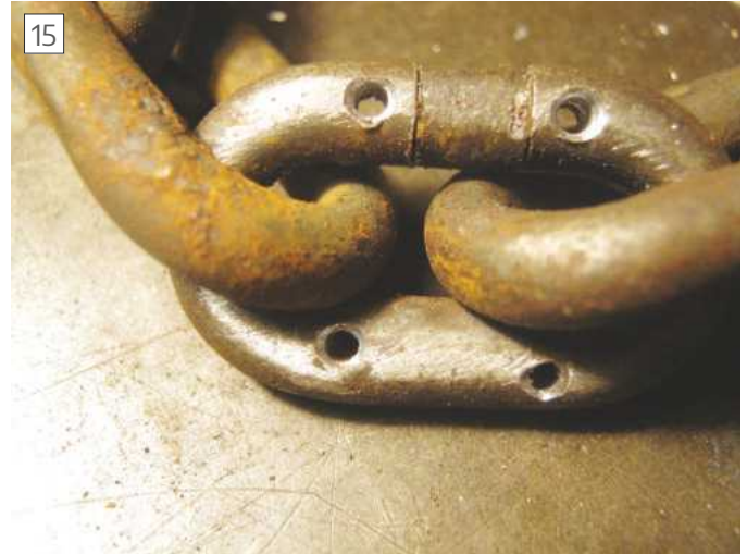
Ready for riveting
