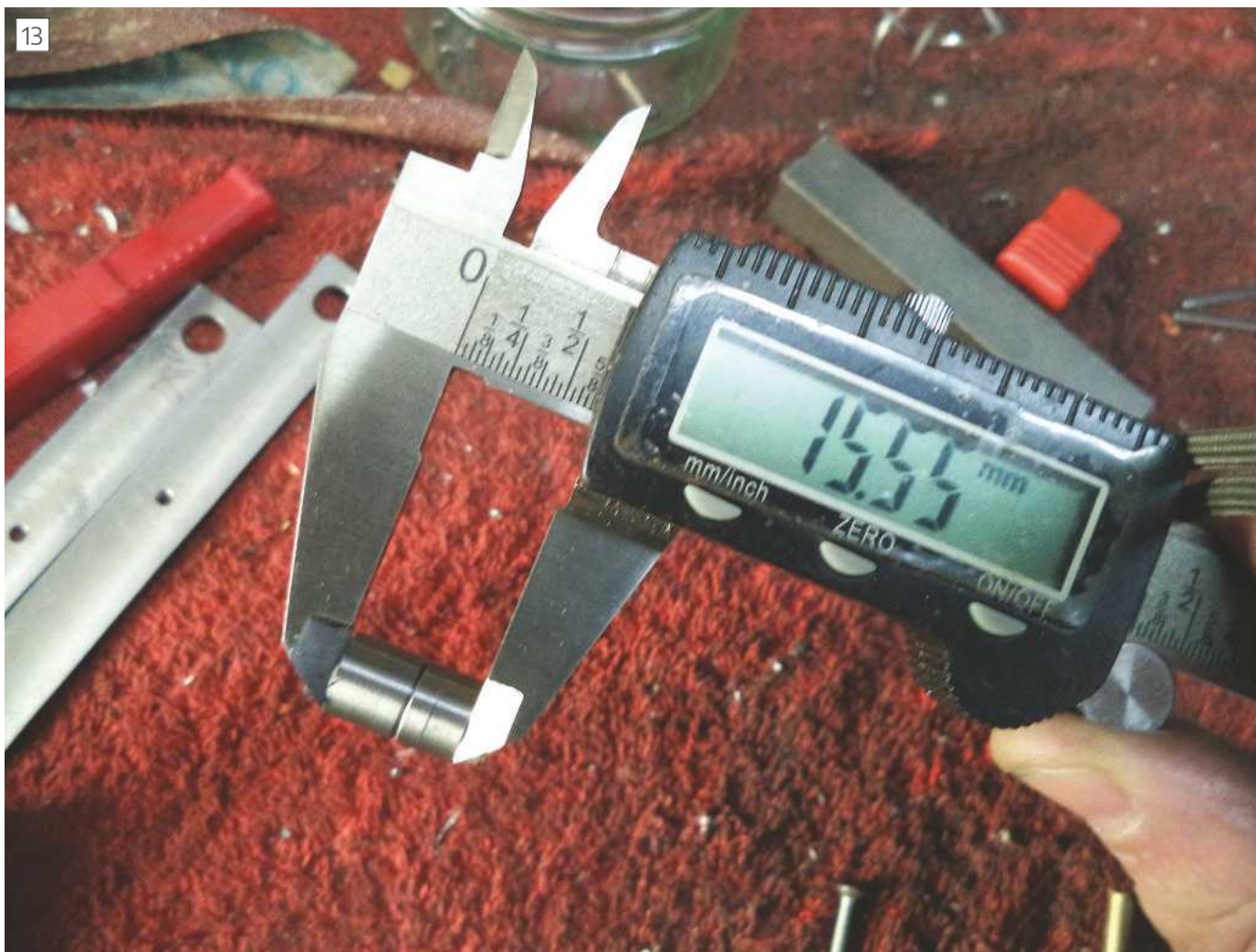
Checking combined width of pinch rollers
