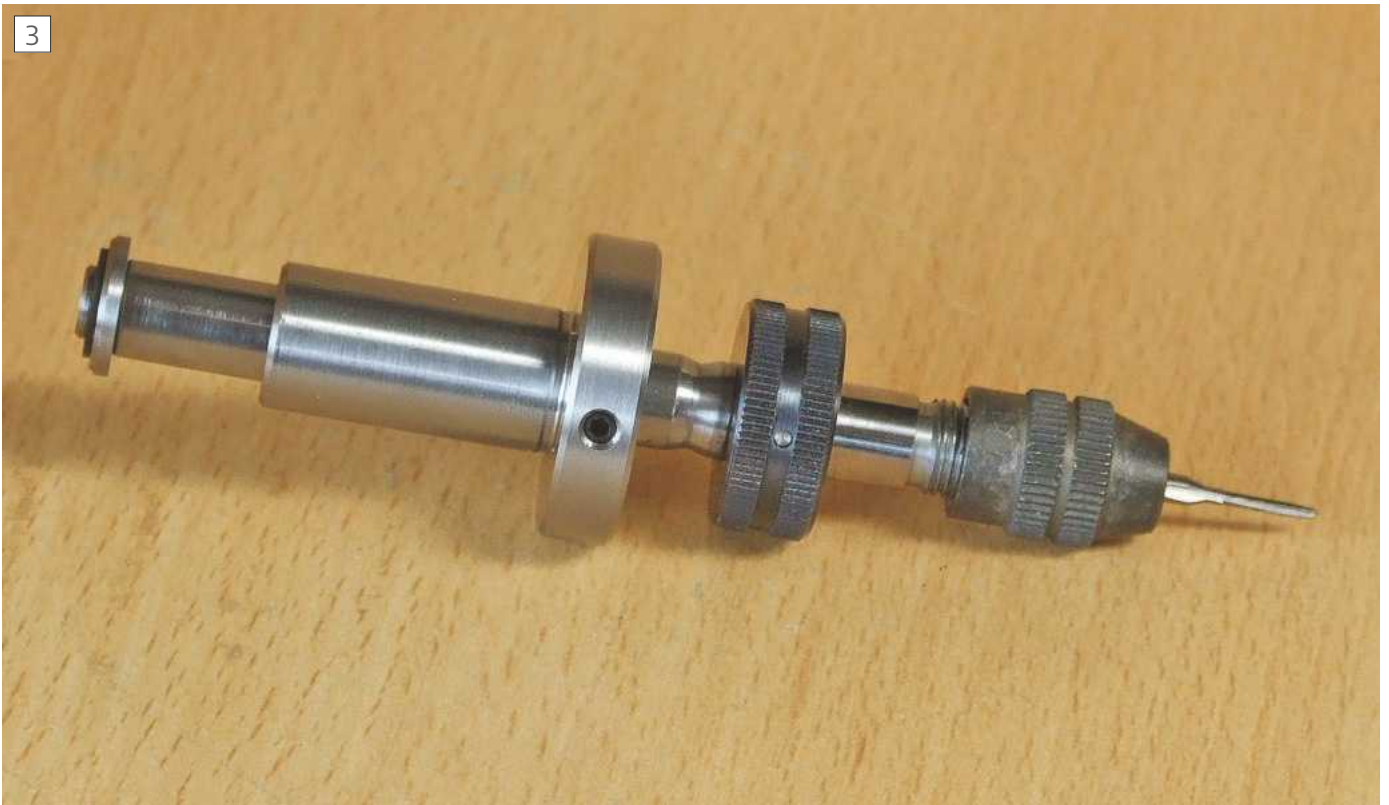
The attachment with 12 BA tap, note the small pin to locate the Knurled ring
