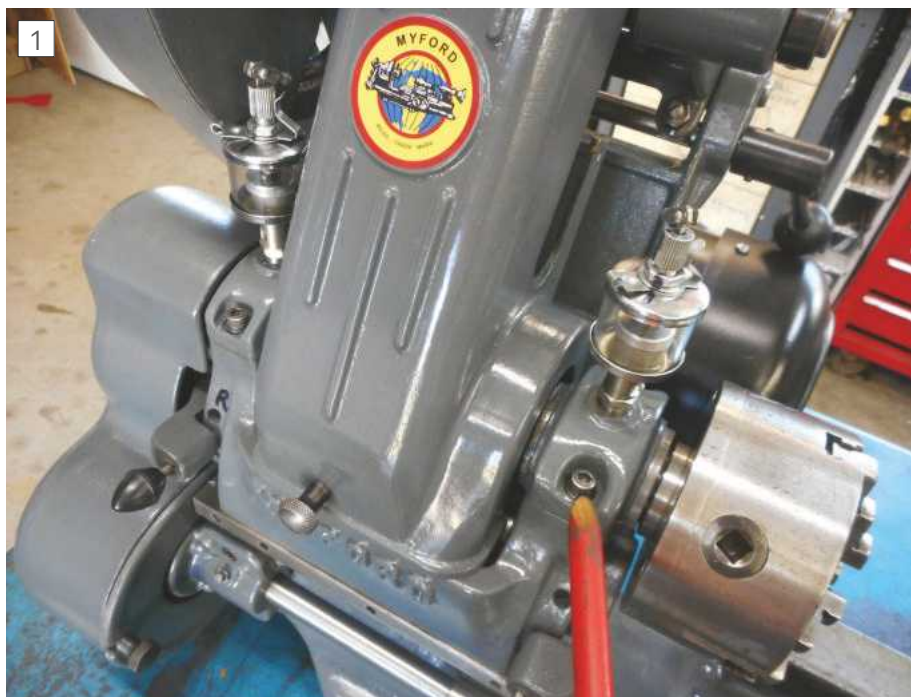
Two bearing caps hold white-metal split bearings in place.
