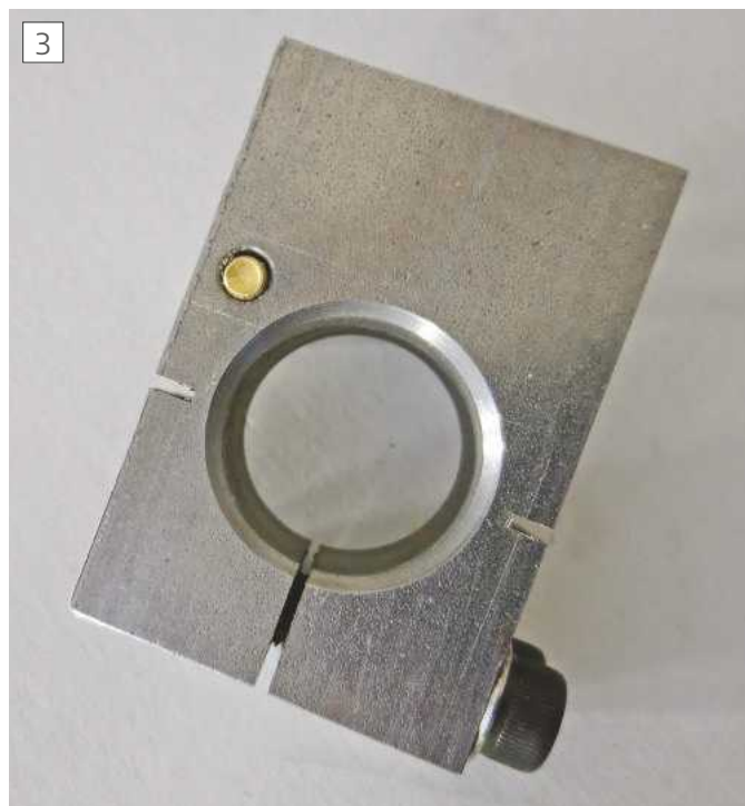
Underside showing chamfer needed to fit the tool post and brass height adjustment screw.
