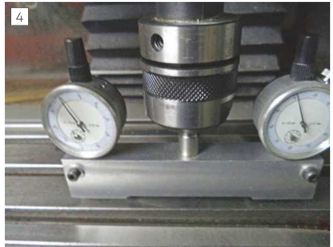
Traming the mill head square
