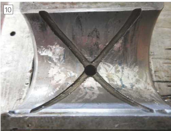
Scrapper marks in diagonal criss-cross pattern.
