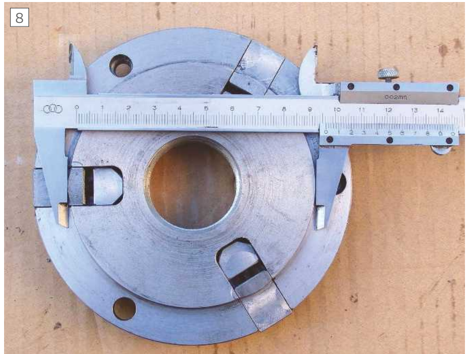
Adjusting plunger to shoulder distance.
