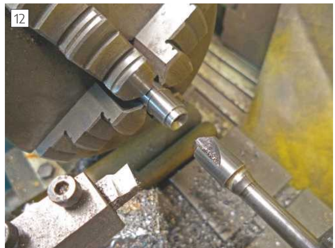
Countersinking pinch roller
