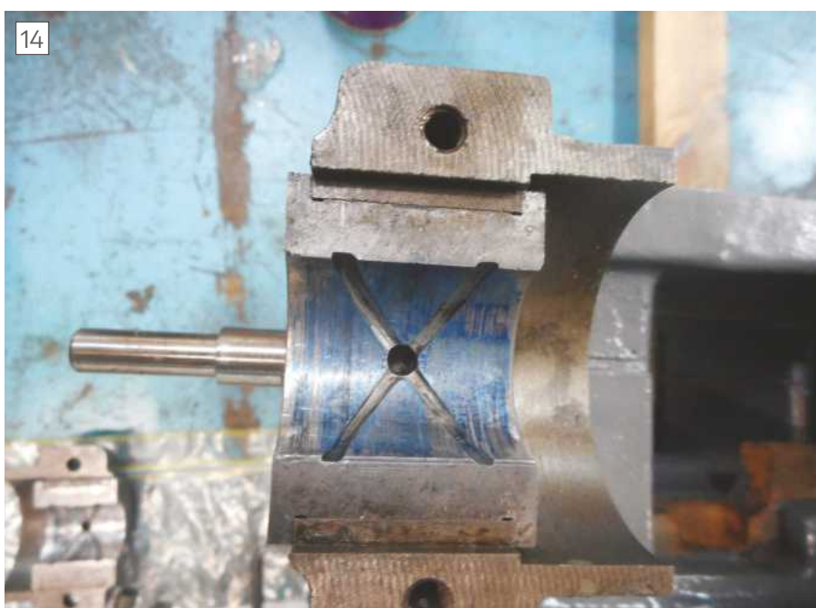
Good overall reading of blue on this bearing.
