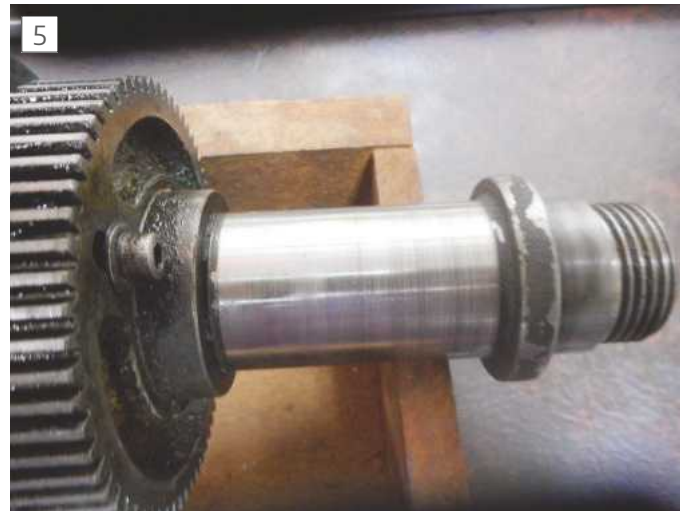
Light scoring or ridging can be dressed with emery tape.
