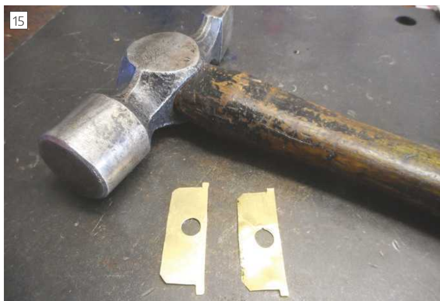
Tap shim edges down flat with a hammer.
