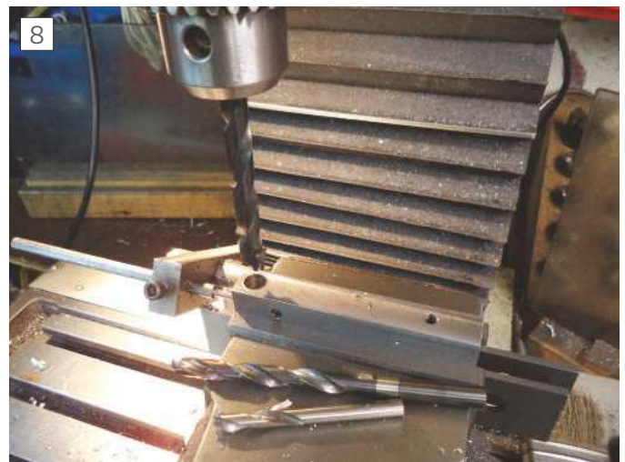
Centre drilling and rough drills
