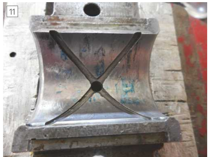
Thin layer of blue gives very fine spotting of highest points.
