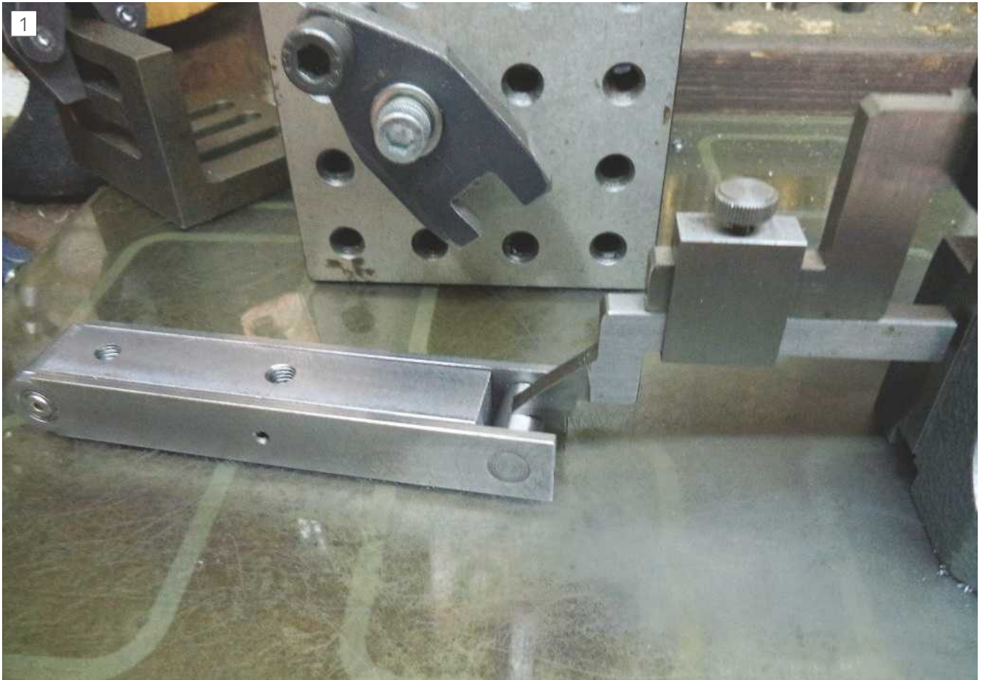
Zeroing the height gauge
