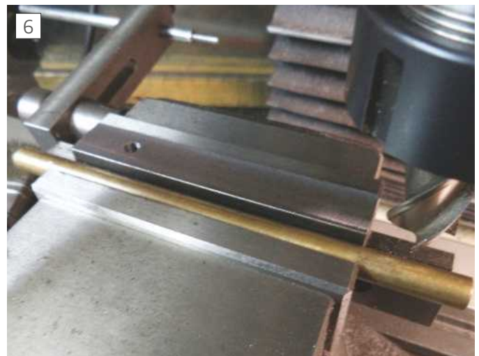
Using a round bar to eliminate the effects of jaw tilt
