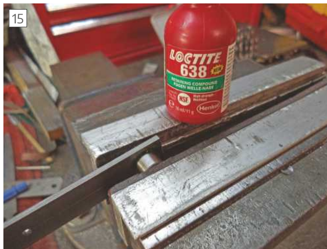
Press fitting the pinch rollers
