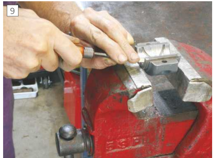
Use both hands to hold the scrapper and use a diagonal motion.
