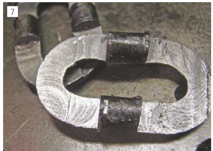
The links after machining
