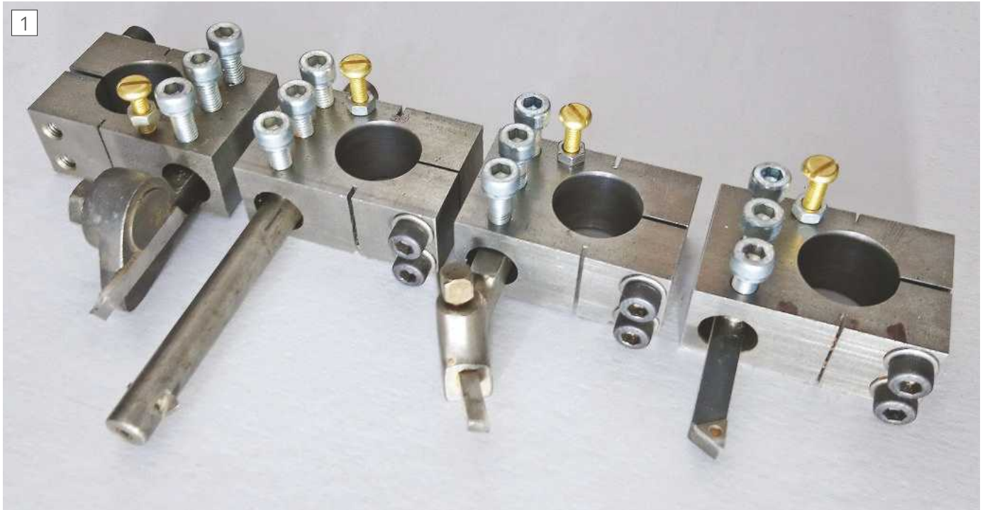
Finished tool holders showing the broad range of tools that fit can be held.
