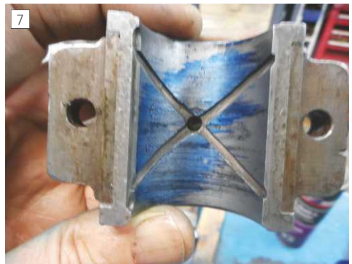
Poor contact is shown by unblued areas.
