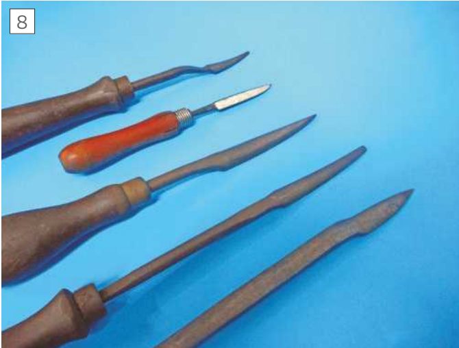
Scrapper second from left was small enough for the job.
