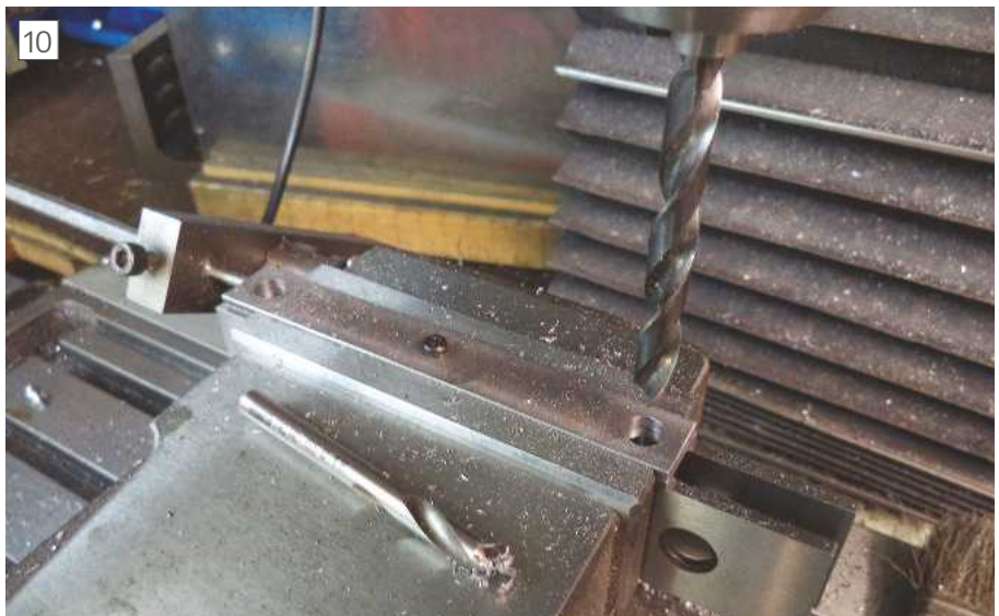
Drilling side plates together
