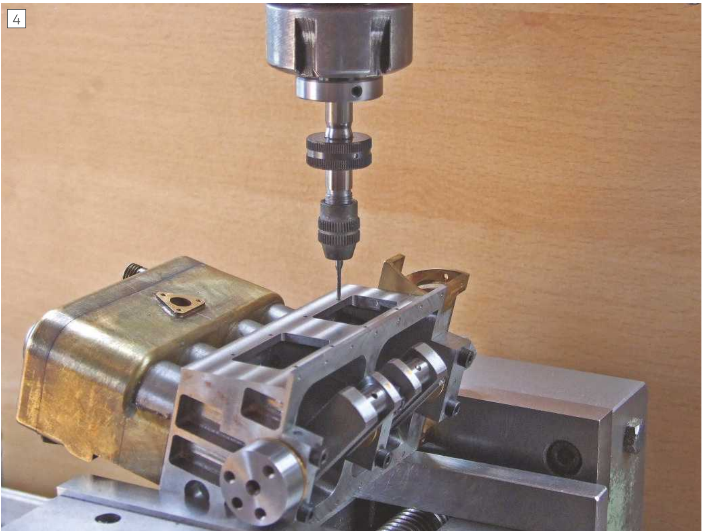
Proxxon Small tap attachment, tapping 12BA threads in my Fiat 702 Tractor Engine
