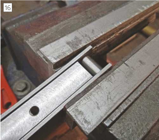
Press fitting the rollers
