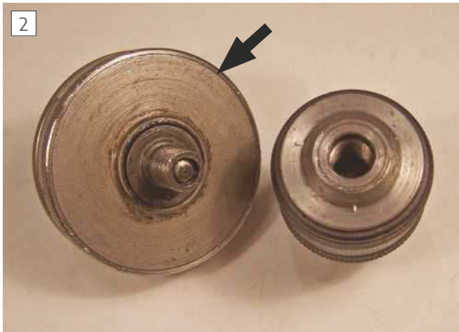
The chuck removed and the inner spindle revealed
