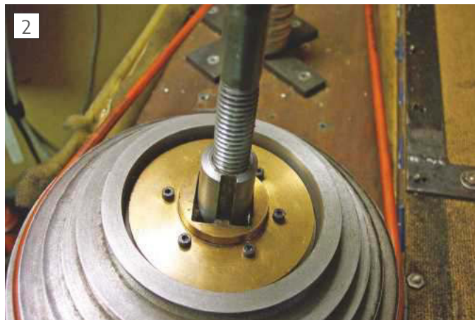
Slug of M12 thread in the mouth of the hole of the drive tube
