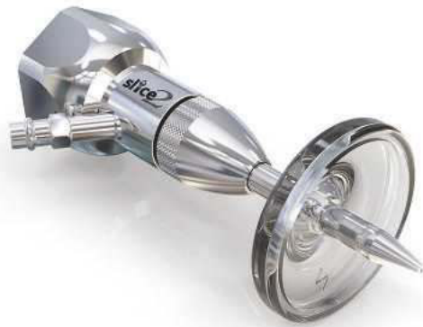
Slice2 abrasive waterjet cutting head by Diamond Technology Innovations. It incorporates a diamond orifice to minimise wear by the abrasive and is engineered with a slim body to facilitate multi-axis cutting. Image courtesy of DTI.
