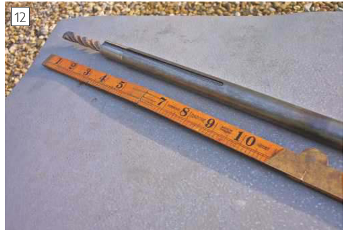
SDS drill after drilling the drive tube
