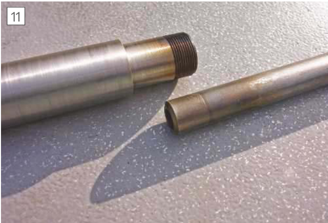
Evidence of the degree of heat needed to break the loctited joint
