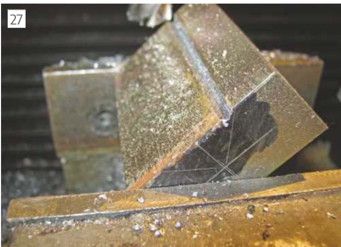
The marking out lines
