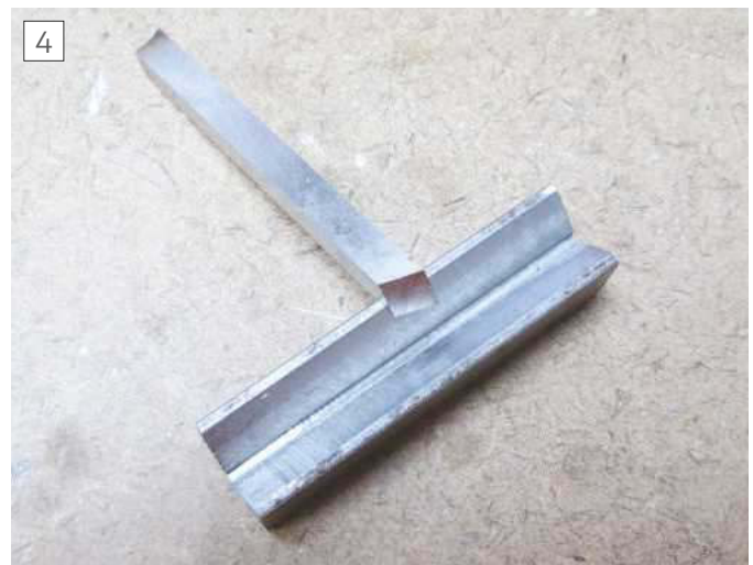
Completed Attachment and Ground Bit
