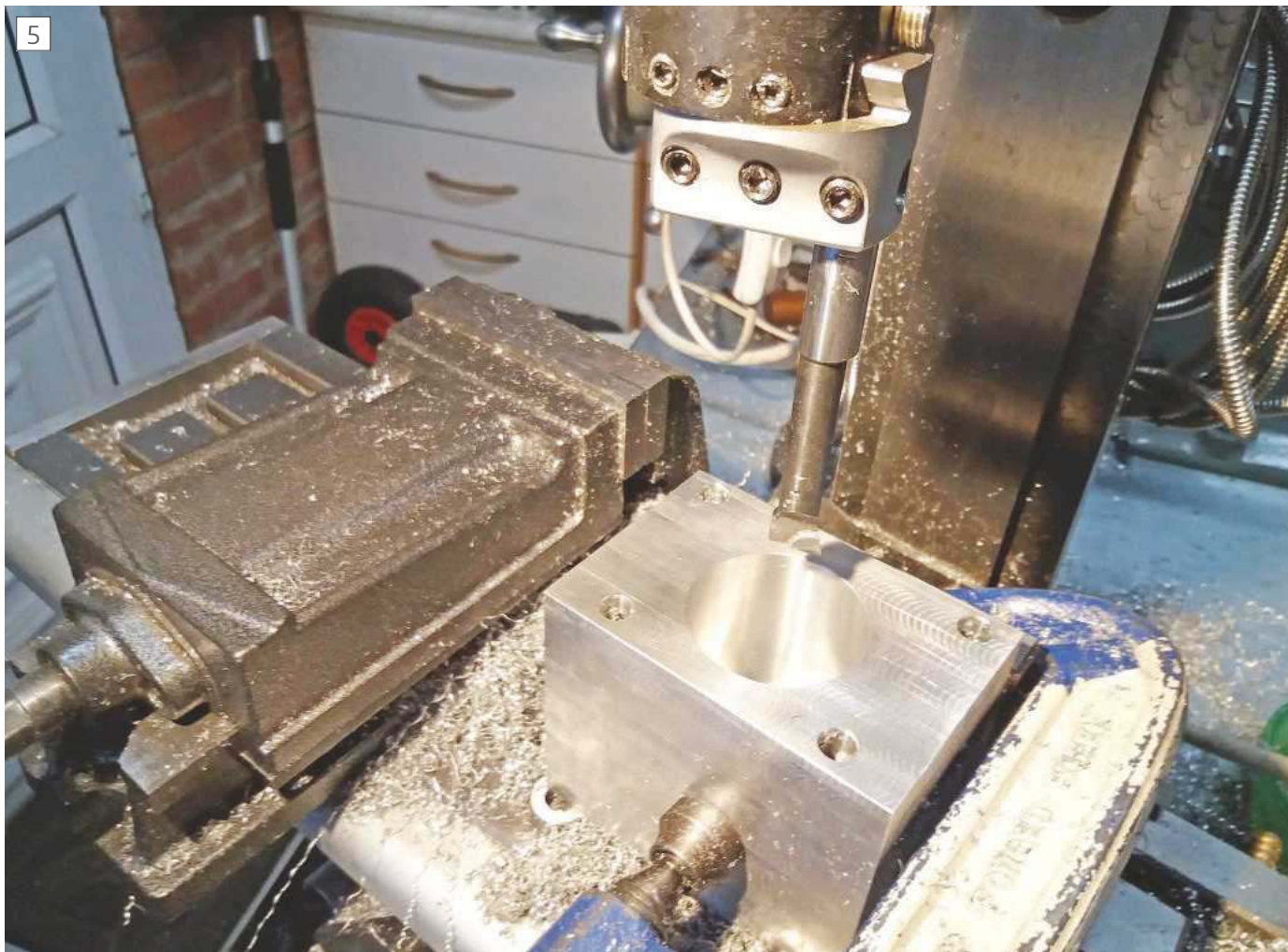
Boring main holes.
