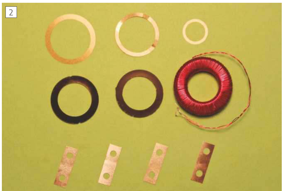
Top: three sizes of mumetal cores for making fluxgates. Middle: two halves of an epoxy former used to house the core and the assembled core with toroidal coil. Bottom: four stainless steel flexures used to make a cross-leaved hinge for a seismometer.
