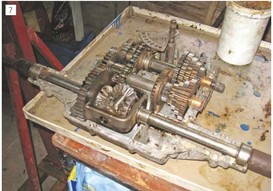
Gearbox opened up. No synchromesh here!
