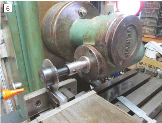
Cleaning up the Bottom of the "V"
