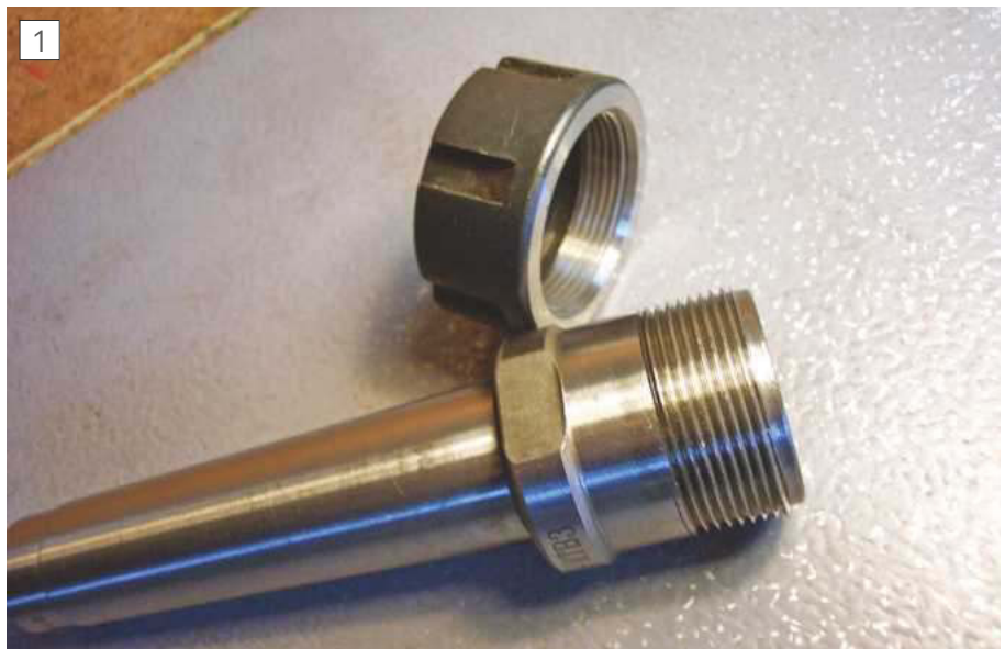
Damaged thread on old ER 25 collet chuck
