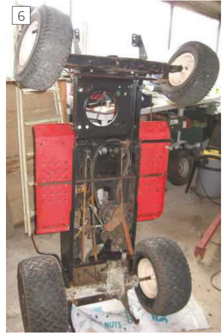
Underside showing drive train.
