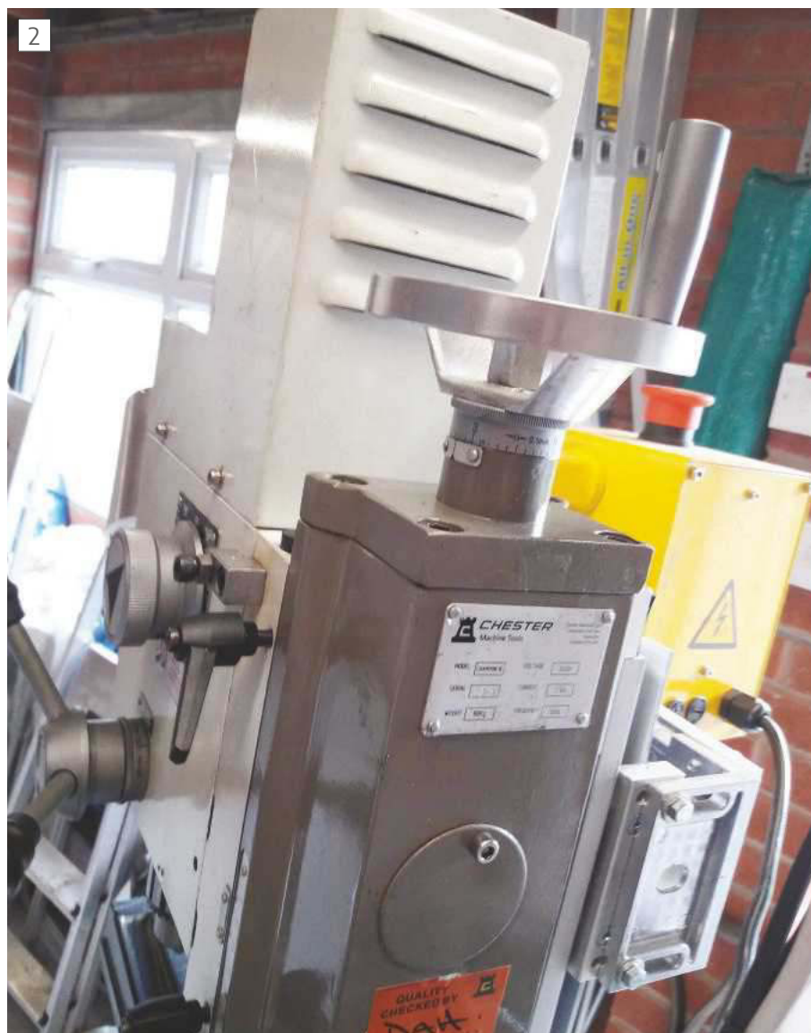
The Z-axis handle is situated on top of the column, behind the head.
