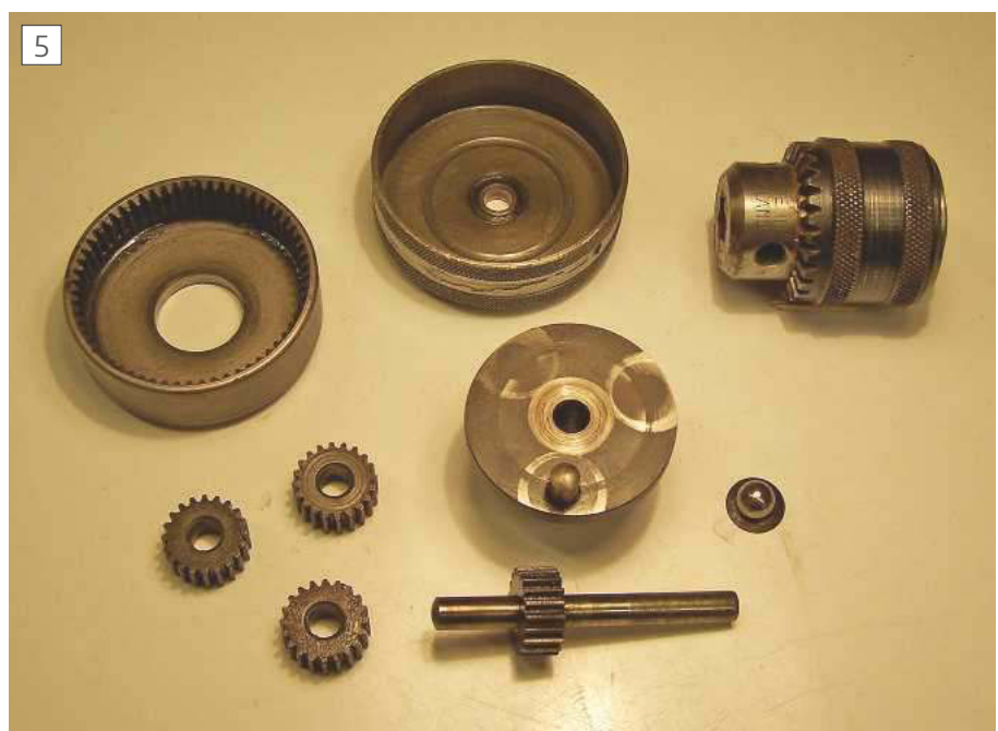
The gearbox dismantled
