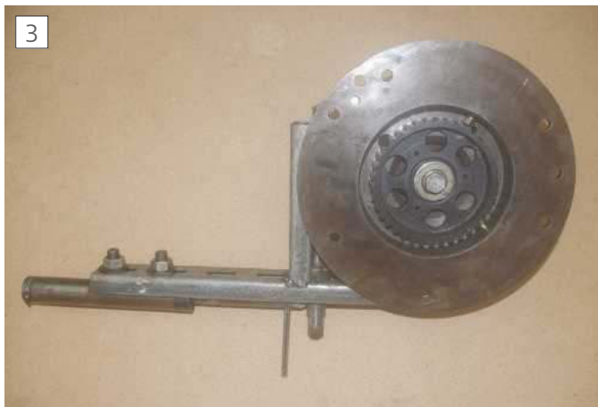
The end float arrangement
