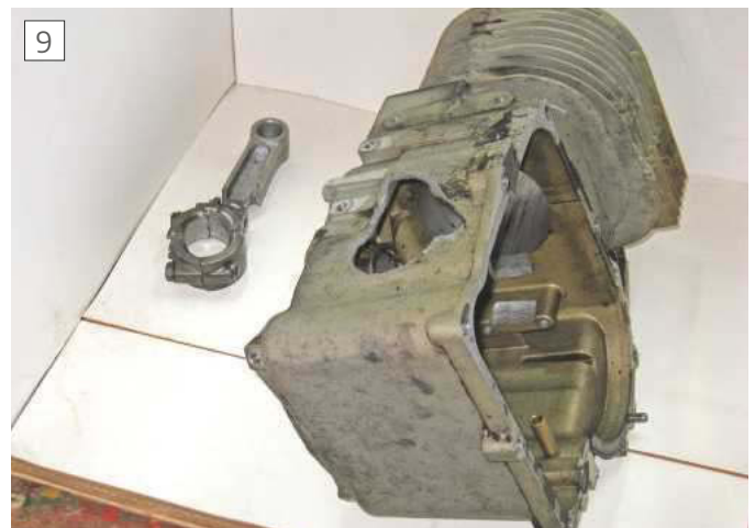
Crankcase and broken conrod.
