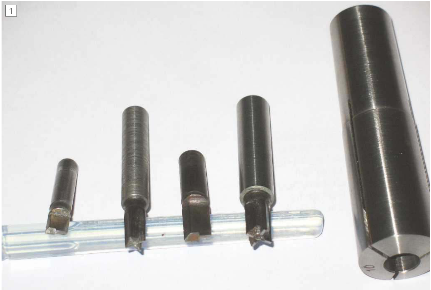
Cutters sleeved & unsleeved and an MT3 direct collet.
