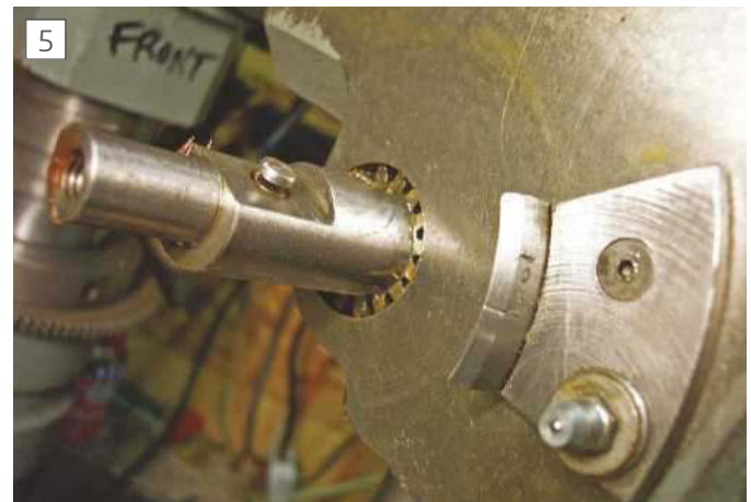
Spring removed, note the drive peg to hook onto the spring tab
