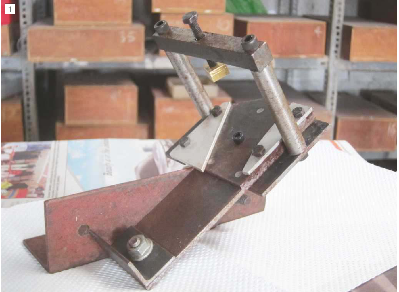
Jig number 2 for four-facet drills.
