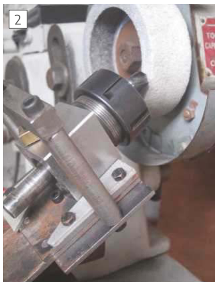
Sharpening a four facet drill (guard removed for clarity).
