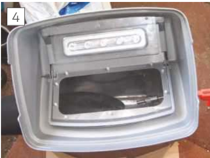
Inside the top of the bin, note battery operated LED light with protection screen.
