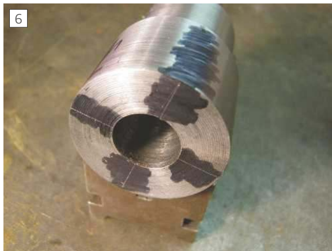
Marking out for holes
