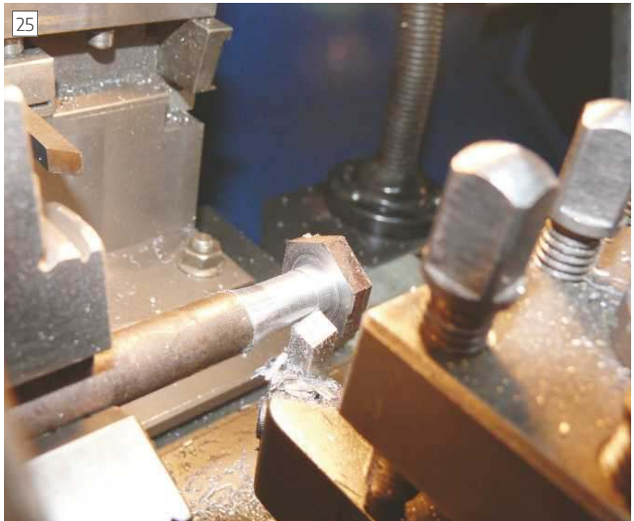
Starting to make the Tee nuts
