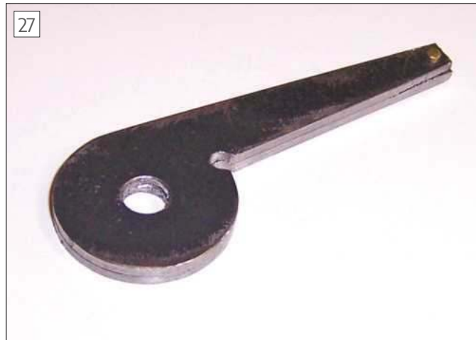
Smooth the profiled edge with a file.
