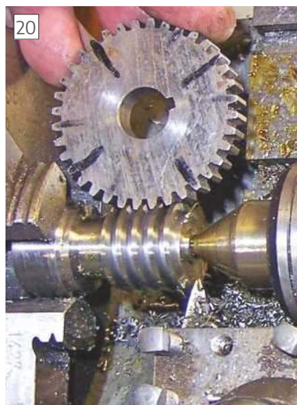
Checking the mesh of a steel worm for a South Bend lathe.
