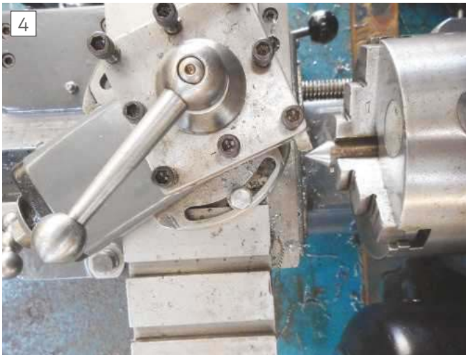
Top slide is offset 30 degrees to turn live centre in situ.
