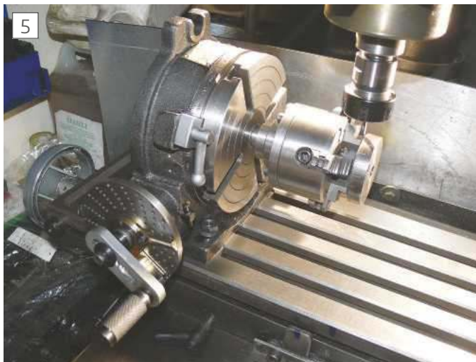
Graduating a handwheel
