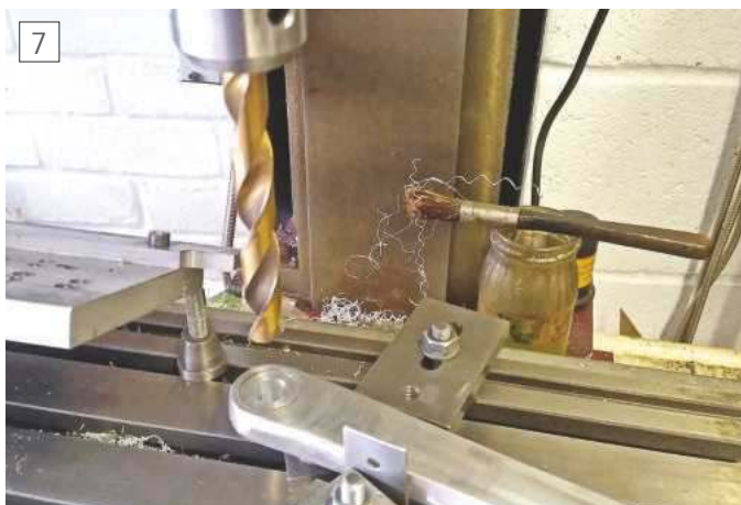
Drilling the insert to tapping size.
