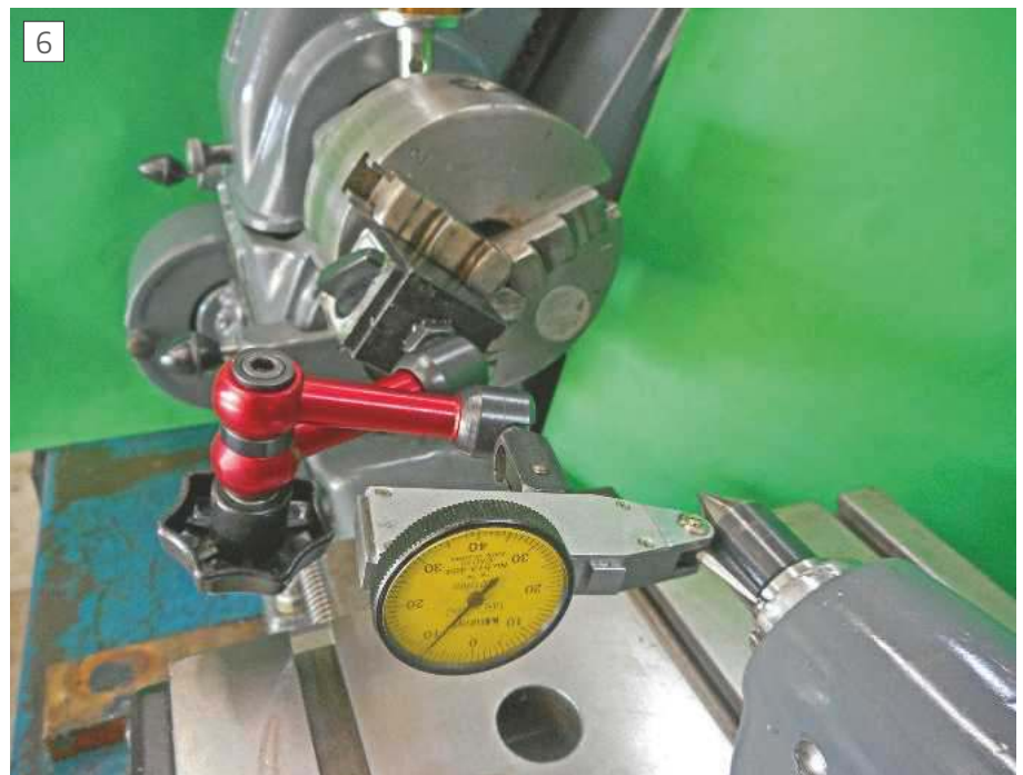
DTI readings are taken at the 3, 12 and 9 o'clock positions.
