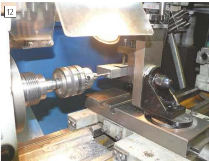
Drilling the end of the slide
