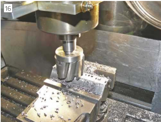
Milling the sloping face of the moving jaw
