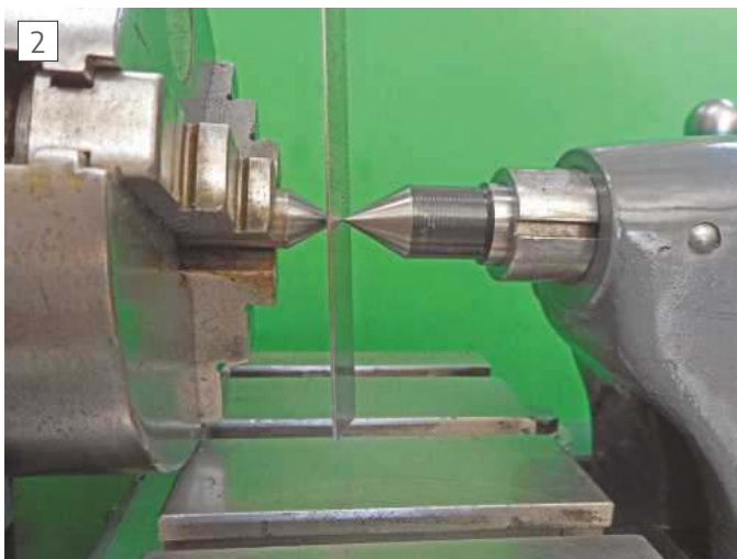
Steel ruler between centres stands straight if the points align.
