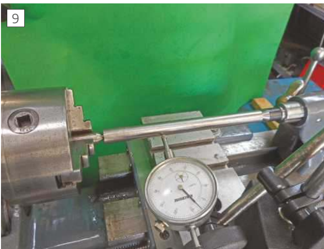
Using the turned test bar and dial gauge to check alignment.
