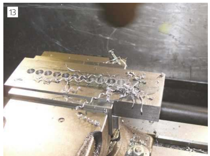
The series of drilled holes in the slide
