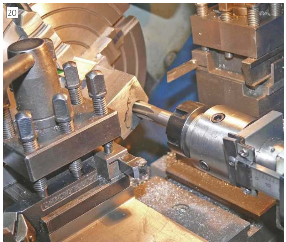
Reaming the moving jaw
