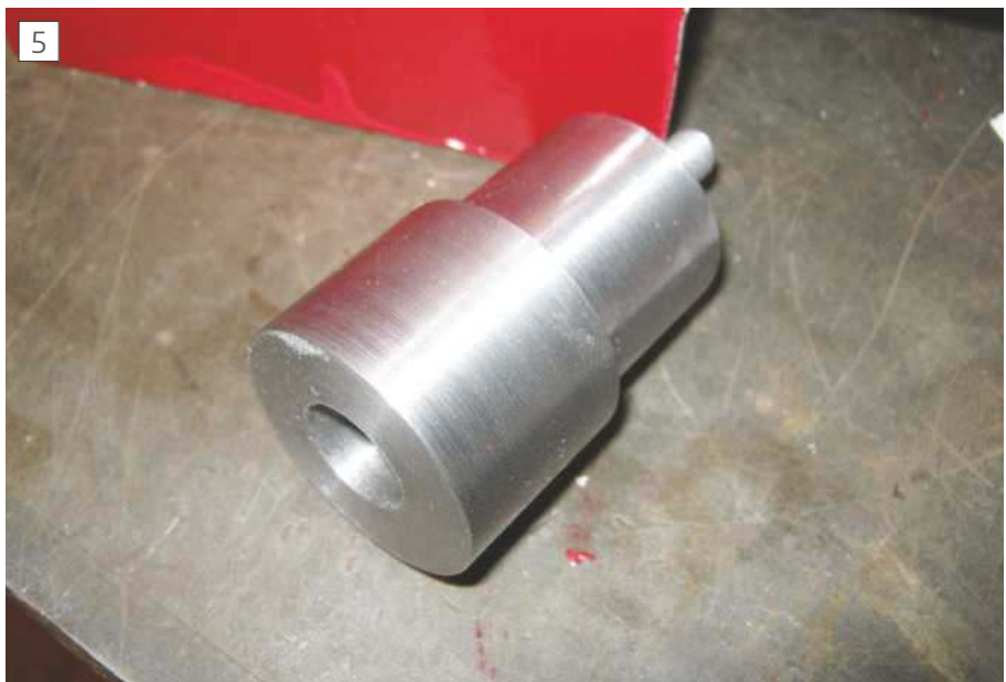
Semi finished chuck
