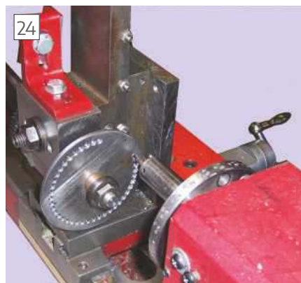
24 Drilling the holes in the index plate using a centre drill to put a small countersink on the hole at the same time.
