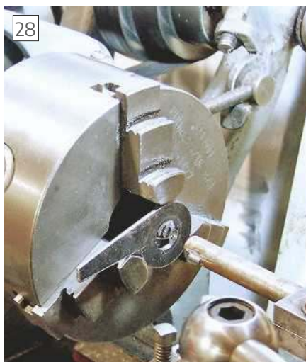
Boring the sector arms.
