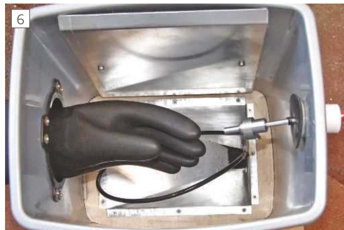
All the workings, sump pan directs media to suction pipe. Filter protection Baffle at the rear also reflects light from the LED.
