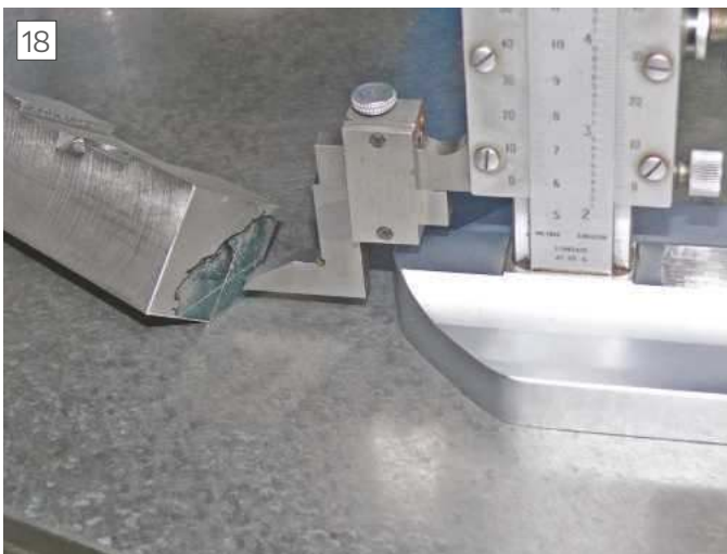
Marking out the moving jaw
