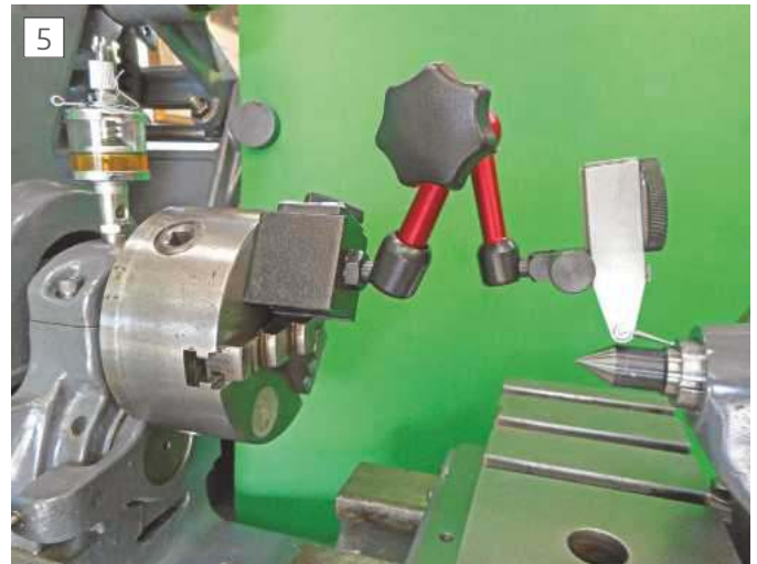
DTI is brought to bear on the centre's mounting taper
