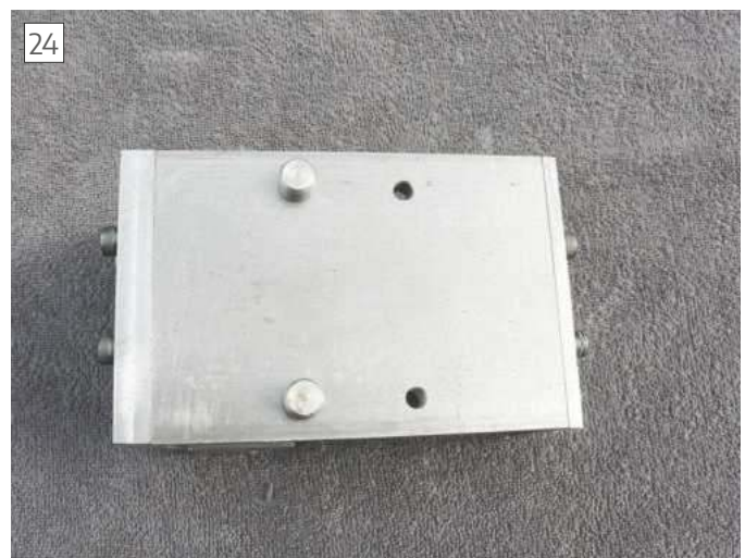
Fixing holes and dowels, in place
