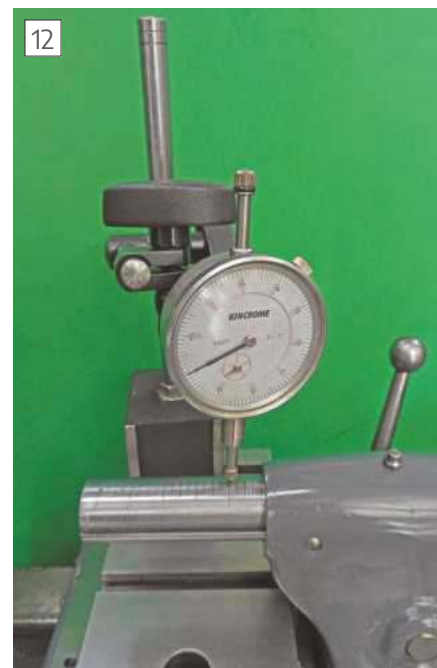
12 Checking tailstock barrel is sitting parallel to bed.
