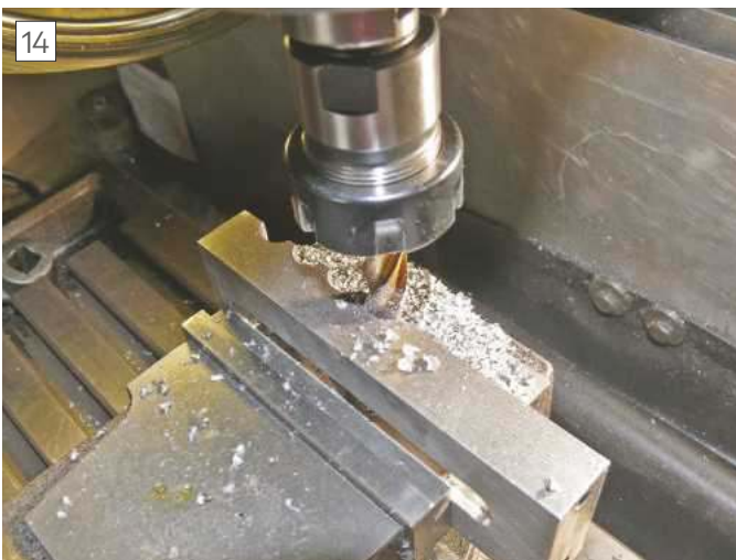
Milling slots on the underside of the slide
