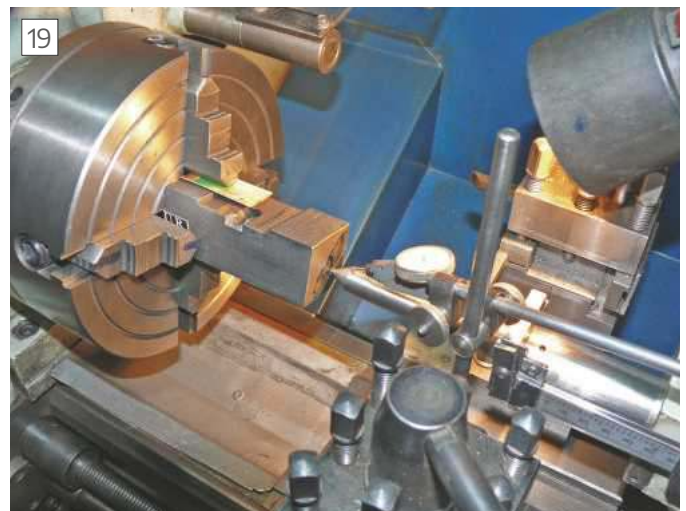
Centering the moving jaw for drilling and reaming
