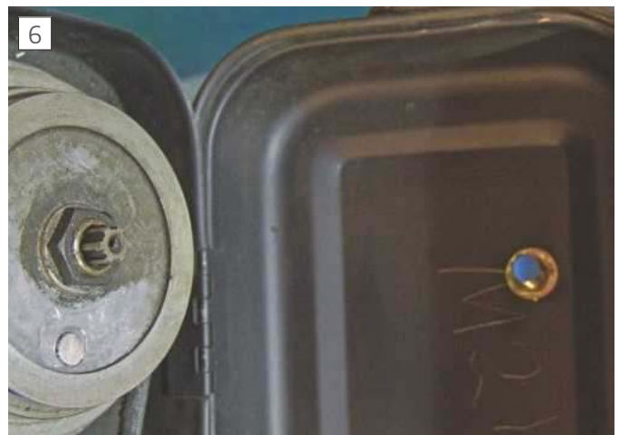
Setup to fit tachometer to drilling machine.
