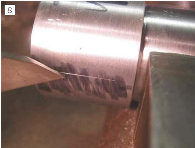
Marking lines on side of chuck
