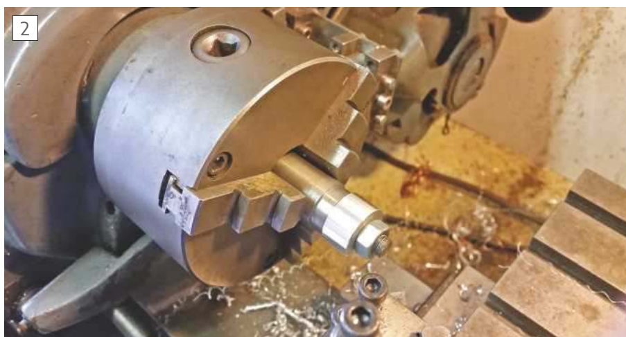
Machining the insert on the lathe.
