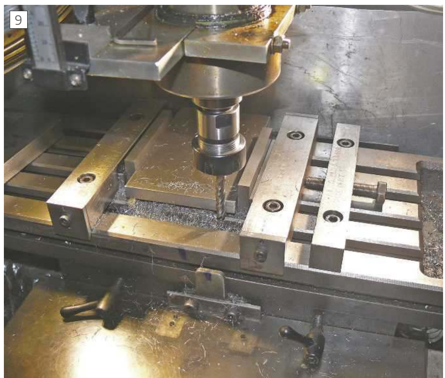
Trimming the edge of the vice base
