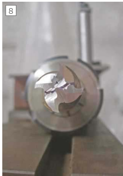
Gashing to cutter in photo 7
