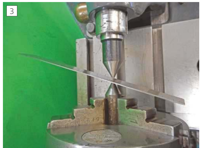
Steel ruler shows tailstock is misaligned towards the operator.
