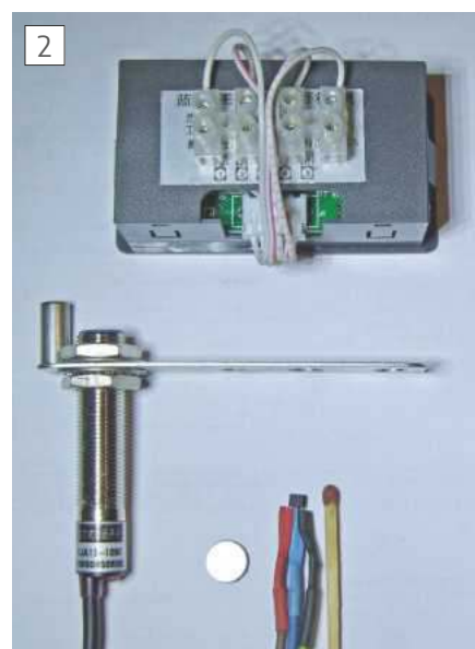
Supplied sensor compared to bare hall effect IC.
