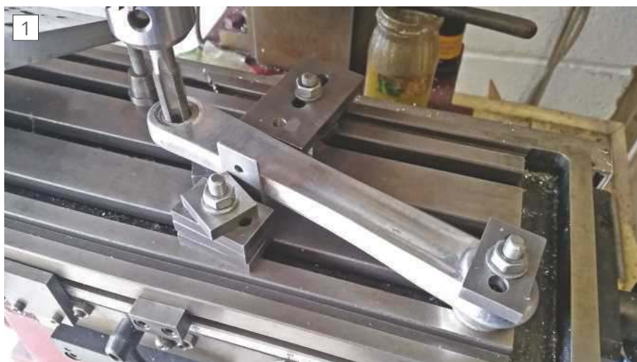
The workholding set up on the mill table.
