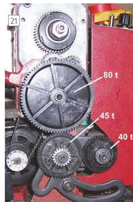
The change gear setup to cut 8 tpi on a mini lathe.
