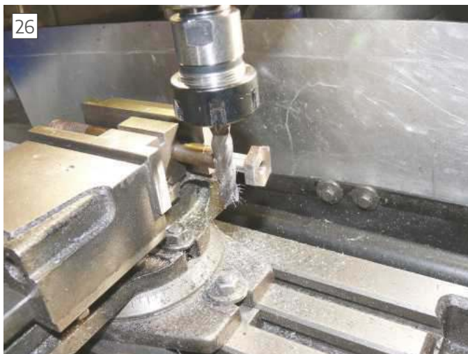
Milling flats on the Tee nuts
