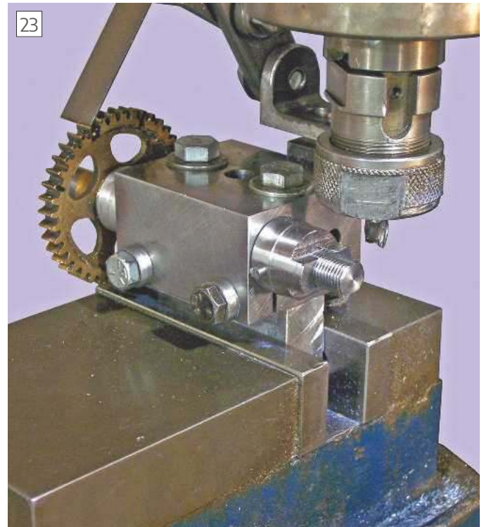
23 Cutting the flats on a vertical milling machine with the shaft held in the MDH.
