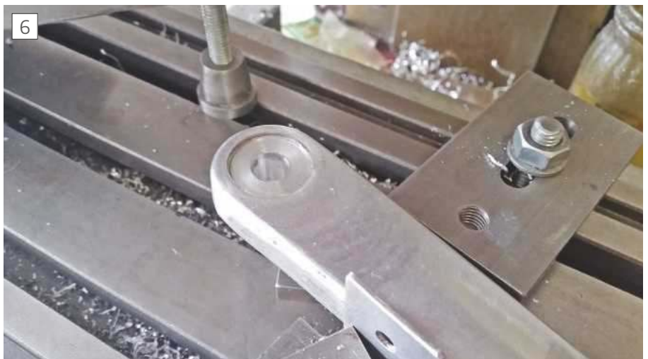
The insert ready for boring and tapping.
