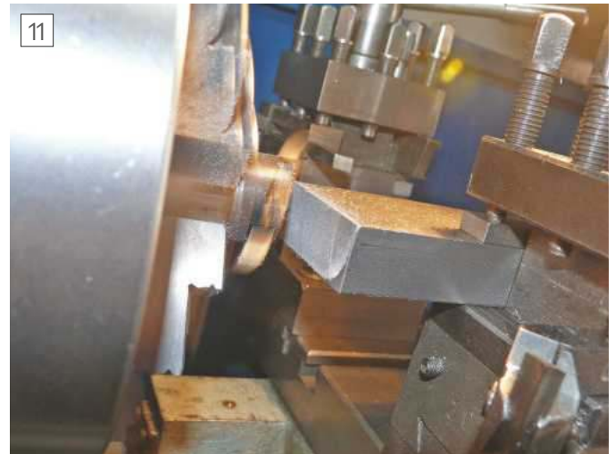
Flycutting the end of the slide
