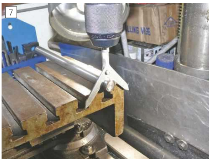
Centering over a Tee slot
