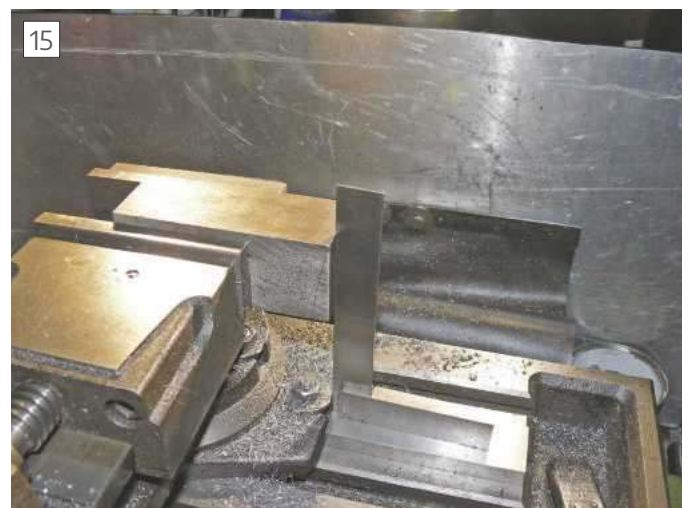
Setting up the moving jaw
