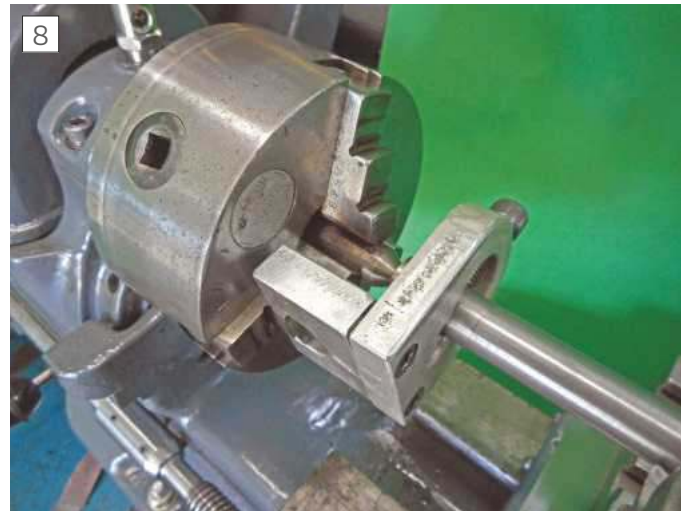
Homemade drive dog for use with live centre in the chuck.
