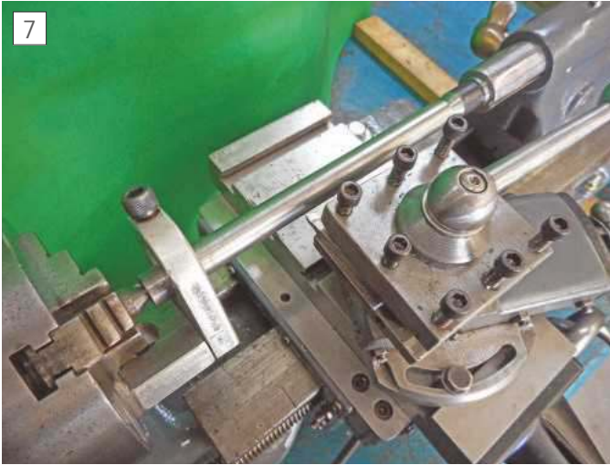
With correct alignment a turned test bar will be parallel for full length.
