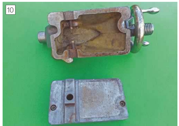
Mating surfaces of tailstock body showing adjusting screws and base showing tenon.
