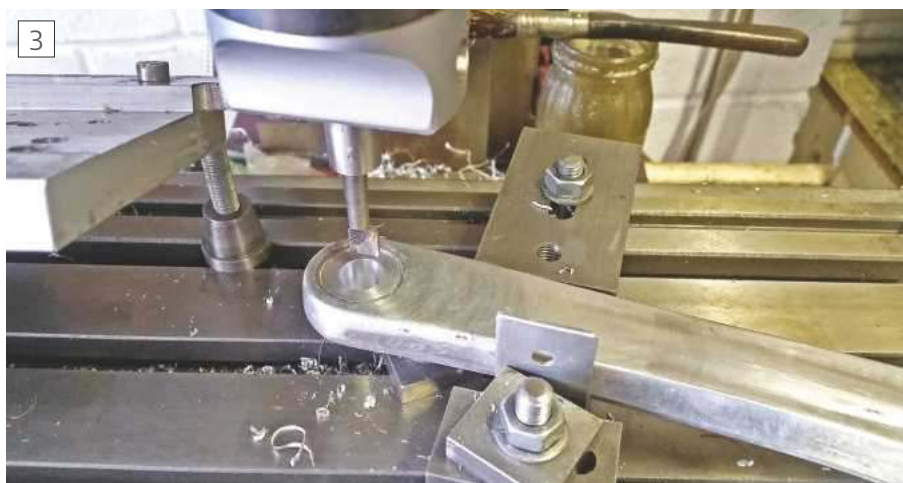
Boring the insert on the mill, using a boring head.
