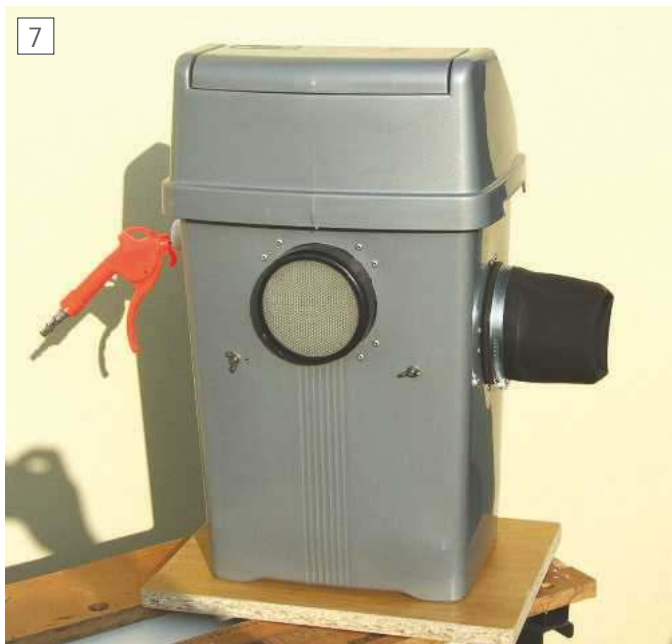
View from the rear showing rubber glove attachment and filtered air exit.
