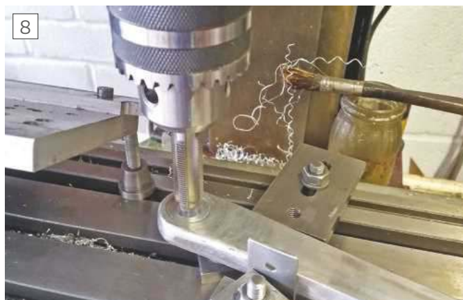
Starting off the tap in the mill to ensure squareness, rotating the mill spindle by hand.
