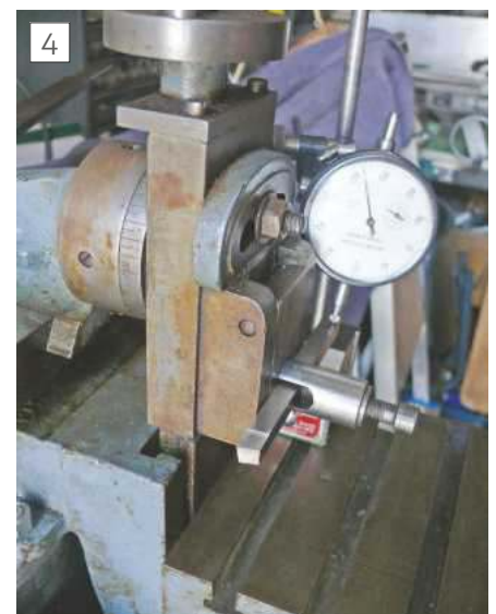
Checking the vertical feedscrew pitch
