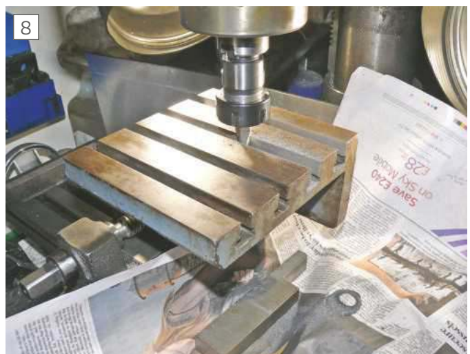
Cleaning up a Tee slot
