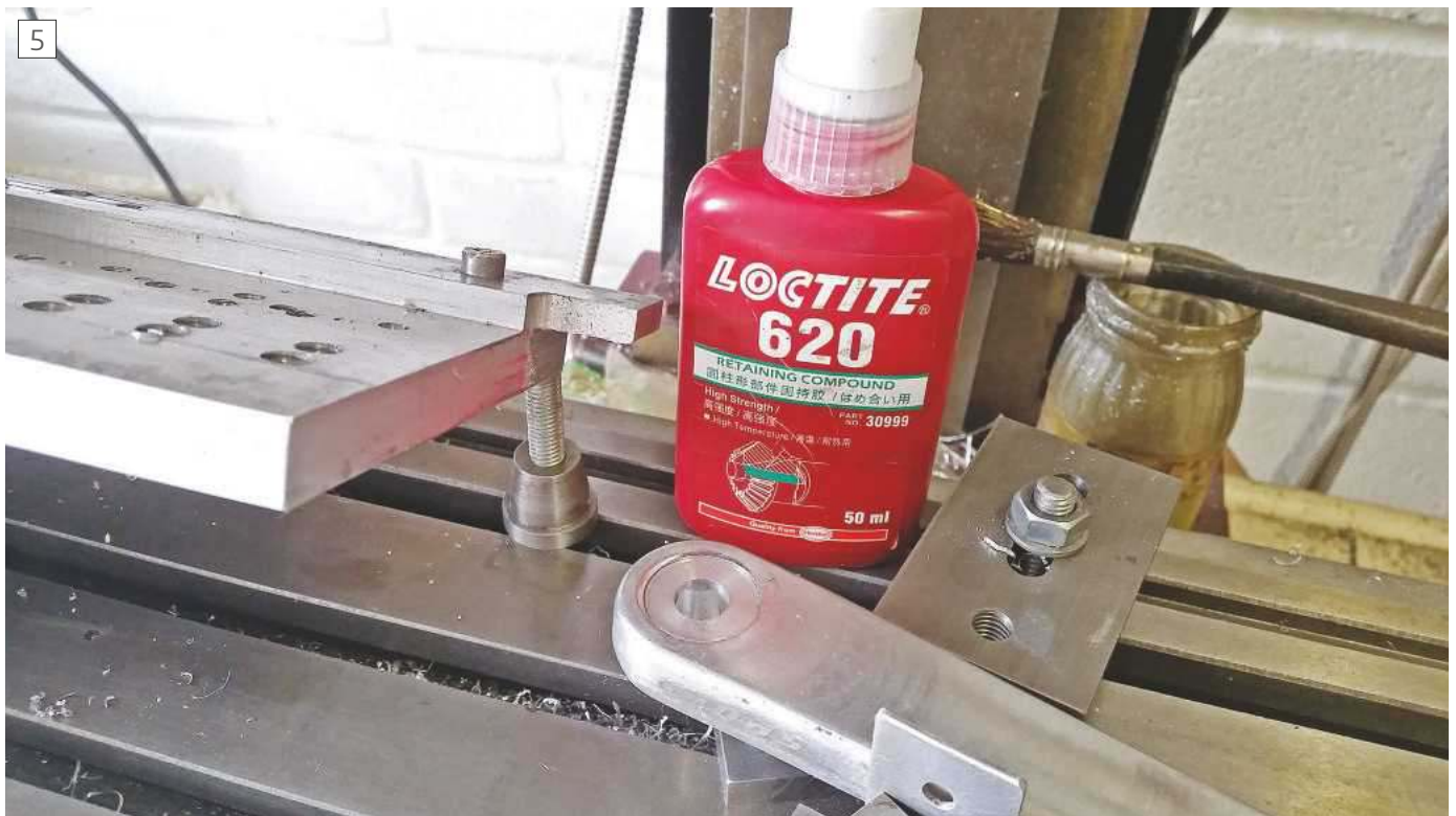
The insert fitted to the crank with retaining compound.
