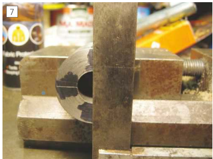
Lining up the chuck
