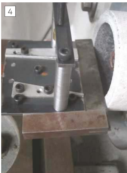
Setting jig square to grinding wheel
