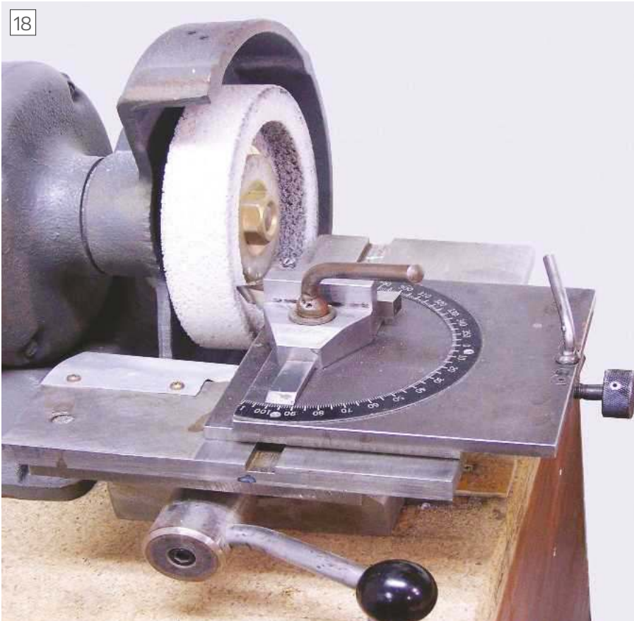
Shaping the toolbit for cutting the worm.
