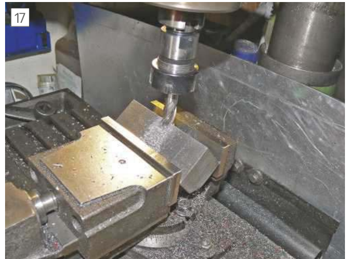
Milling for the clamp screw
