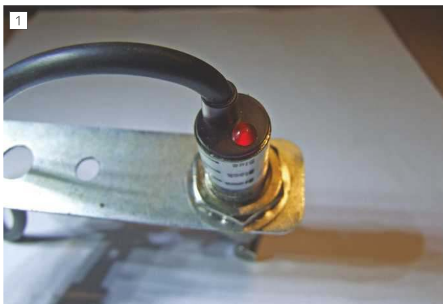
LED at rear of sensor.
