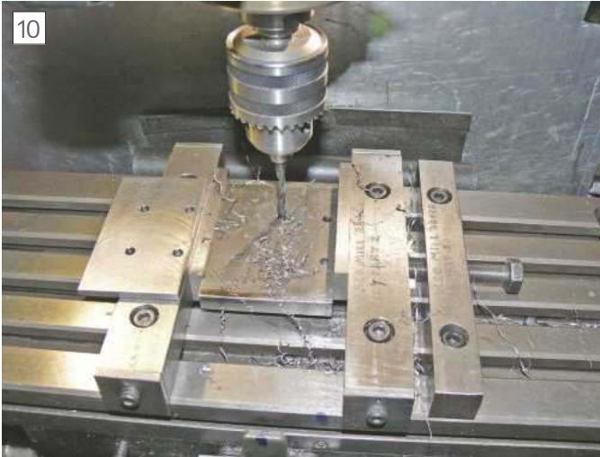
Co-ordinate drilling an end plate
