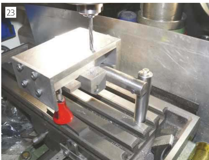
Reaming the dowel holes in the Base
