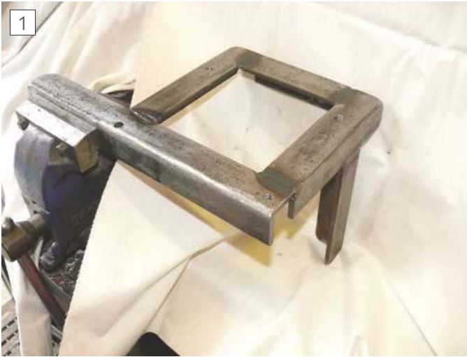
The Frame to mount the Shaper
